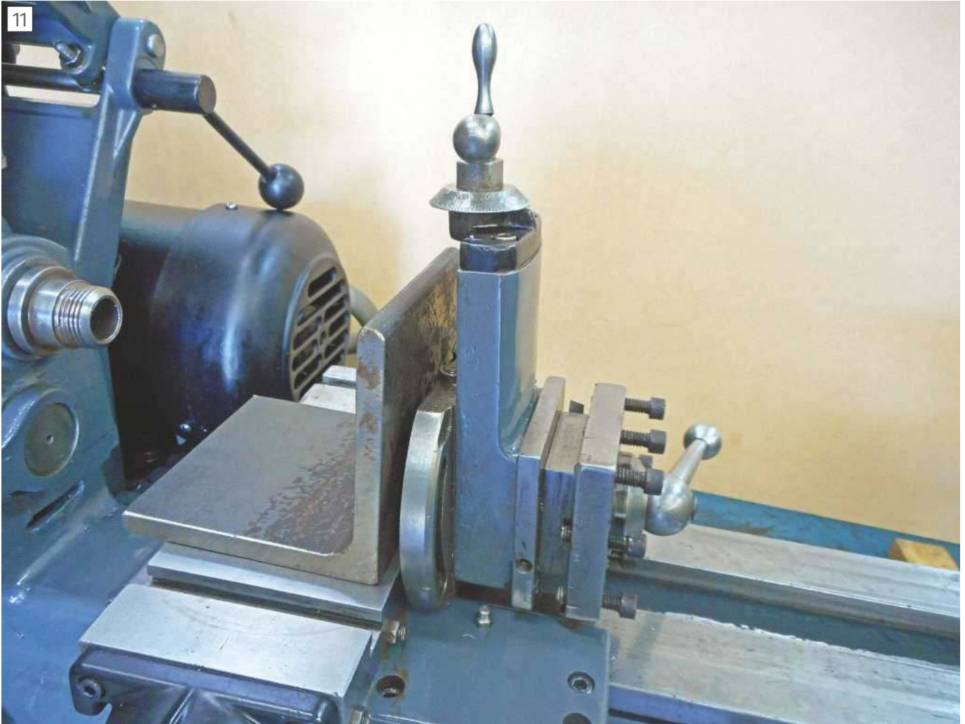
Mock-up of top slide replacing the vertical slide to do the same job.
