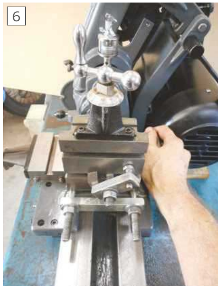
Hold both sides of the cross slide and pull the saddle toward the tailstock to take a cut.
