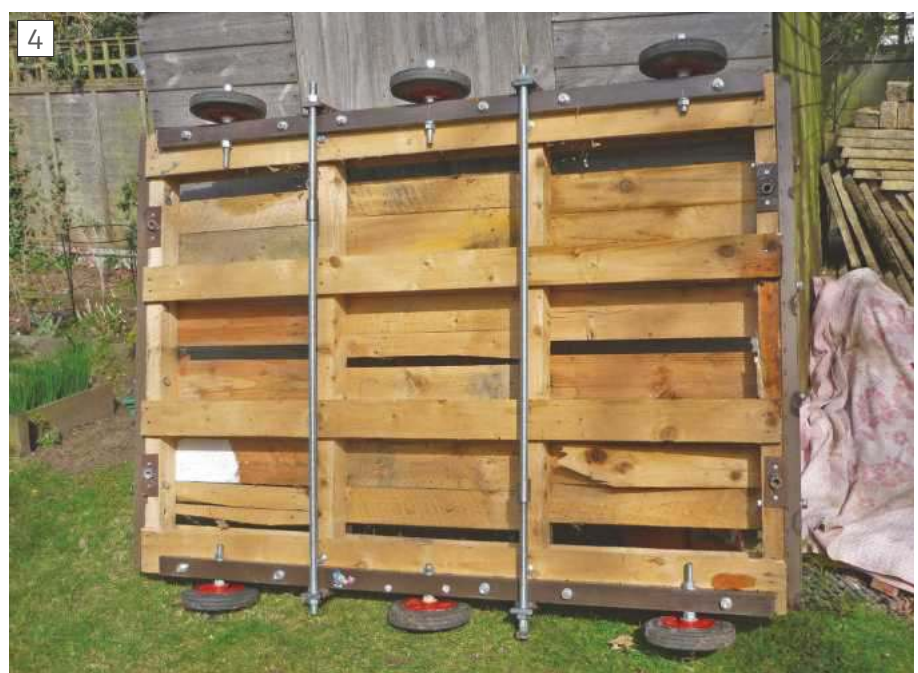
Tie Bars Beneath Trolley
