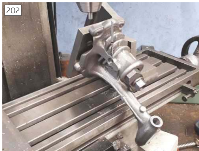
Drilling angled hole for grub screw
