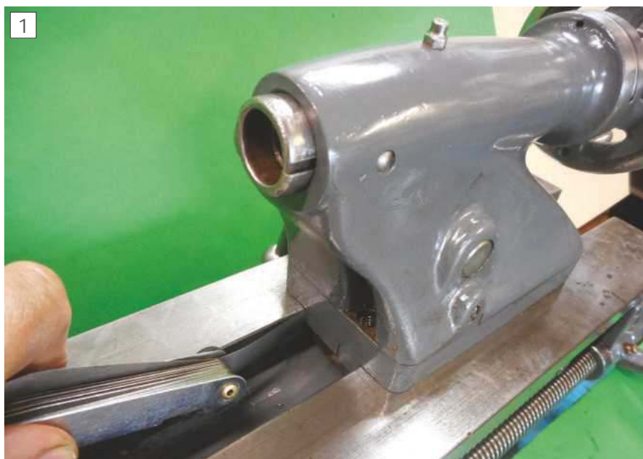
Measuring gap between bed shear and tailstock guide block with feeler gauges.
