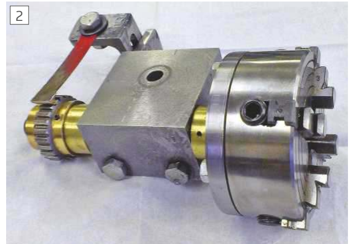
This version uses a four jaw chuck instead of threaded spindles, photo credit C.Peters)
