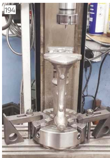
Drilling mounting and dowel holes
