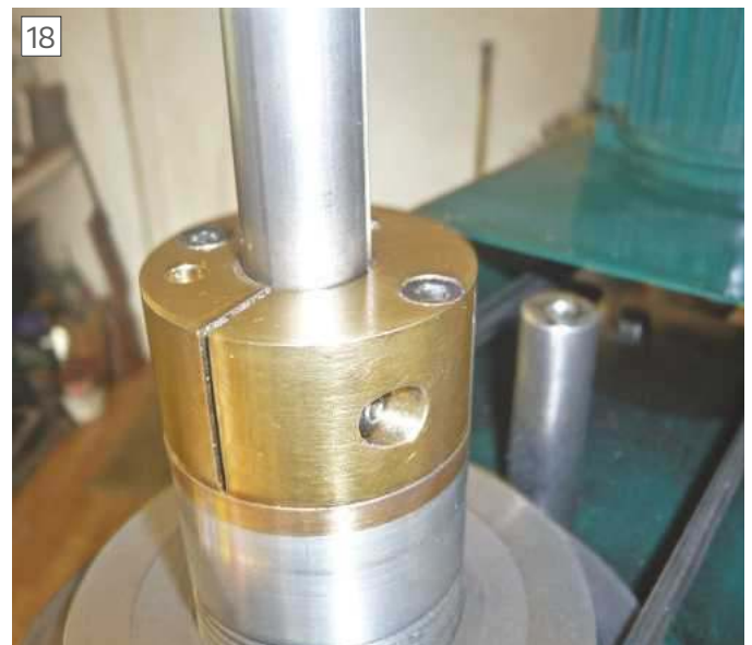
Overhead view of the brass damper
