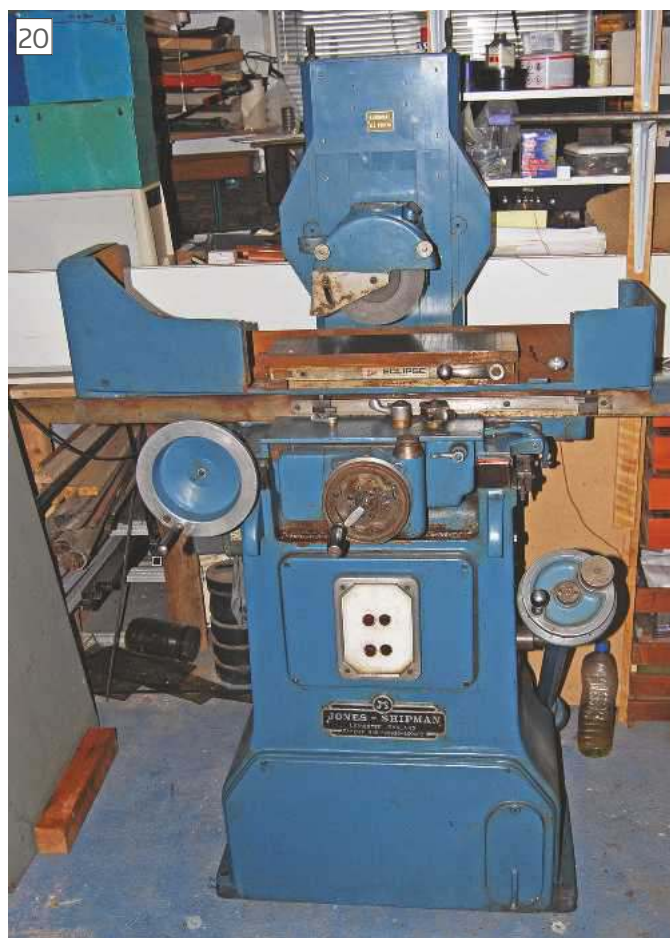
Surface Grinder Ready for Re-commissioning
