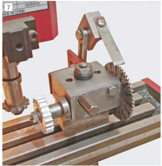
The basic head set up to cut a gear on a vertical mill.
