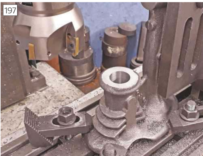
Milling the top of the cylinder to height with indexable shell mill
