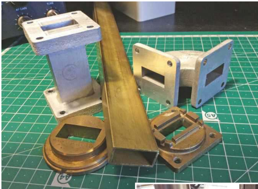
A very mechanical aspect of radio – waveguide to conduct microwave signals.
