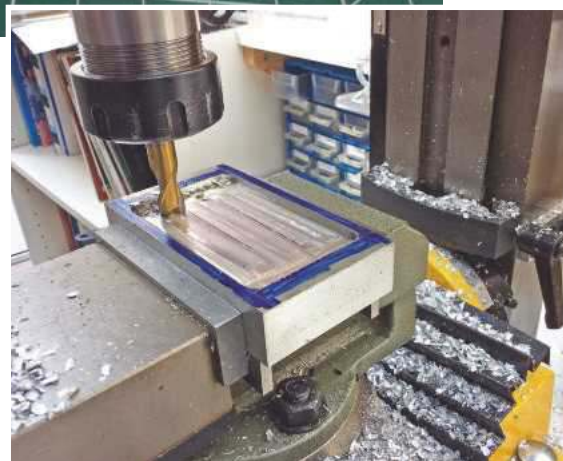
Starting to mill out the enclosure for the power amplifier from a piece of aluminium.
