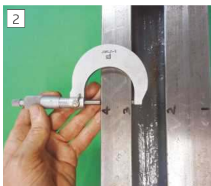
Measuring width across bed ways with micrometer.
