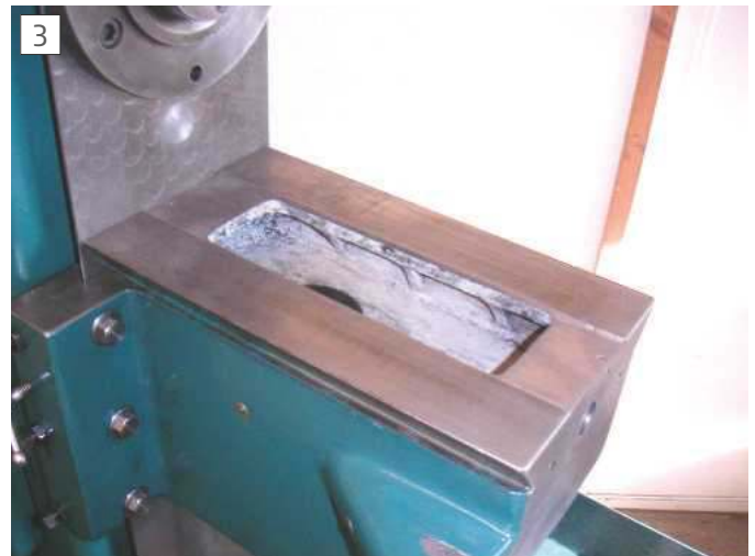
Recess completed & knee re-assembled
