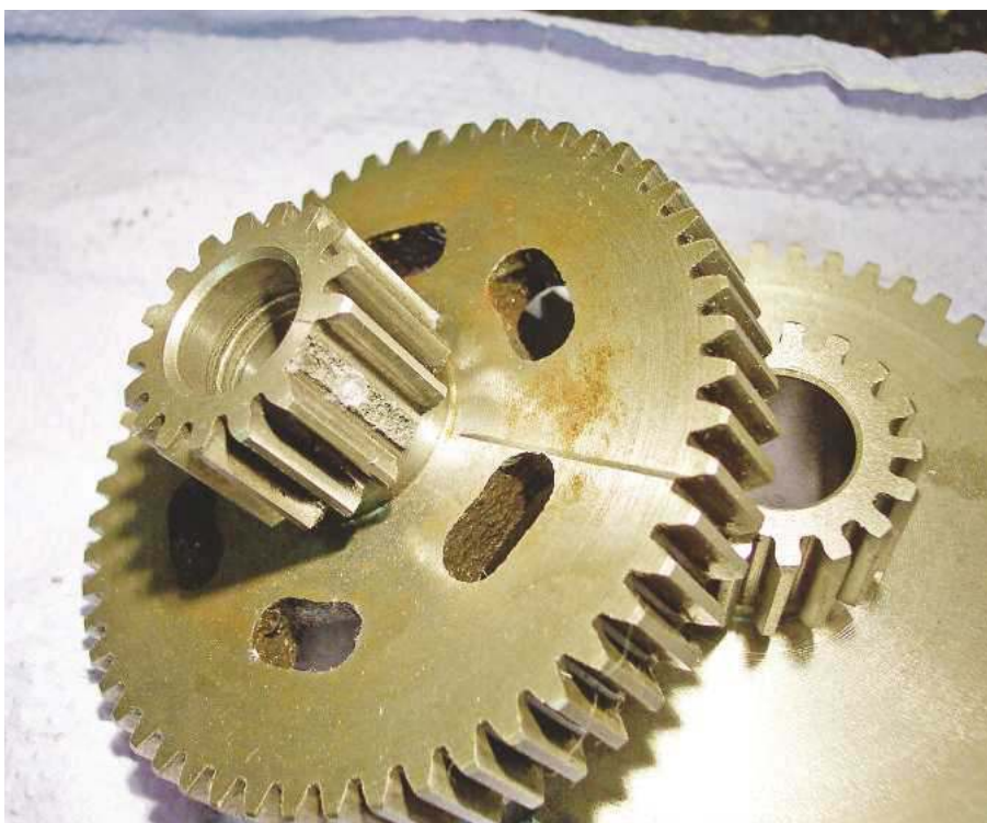
Binding damage in the bore of the old cluster.
