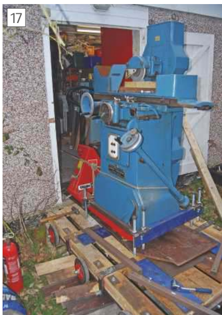
Lifted and Pallet Truck Inserted
