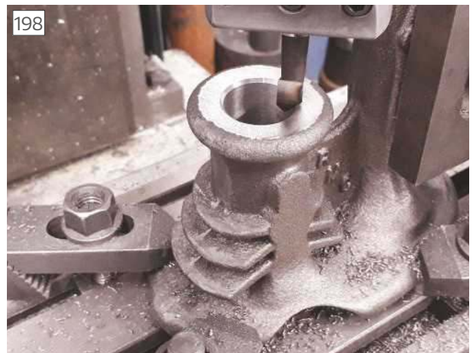
Chamfering cylinder edge with boring head
