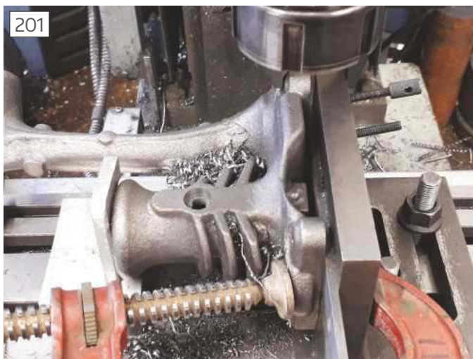
Machining features on side of casting
