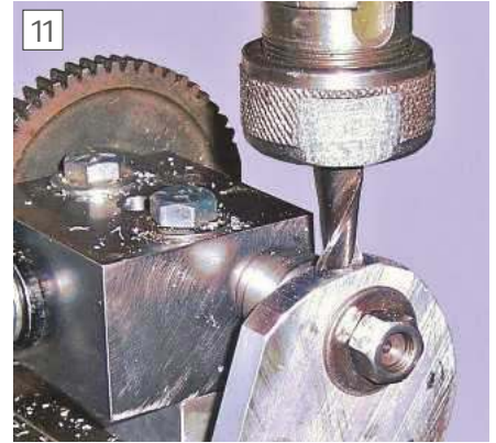
11 Profiling a radiused end by cutting a series of small facets.
