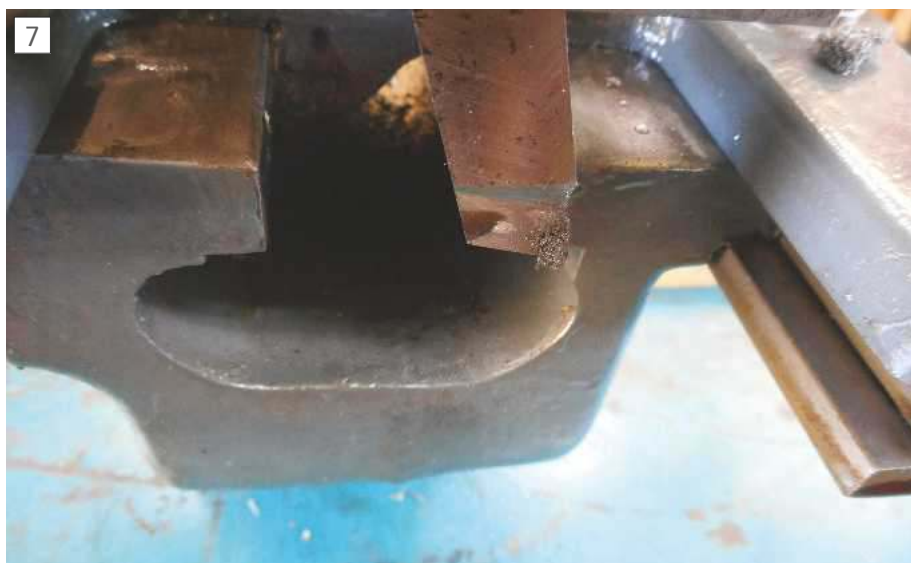
Pull the saddle until the tool just passes the end of the bed.
