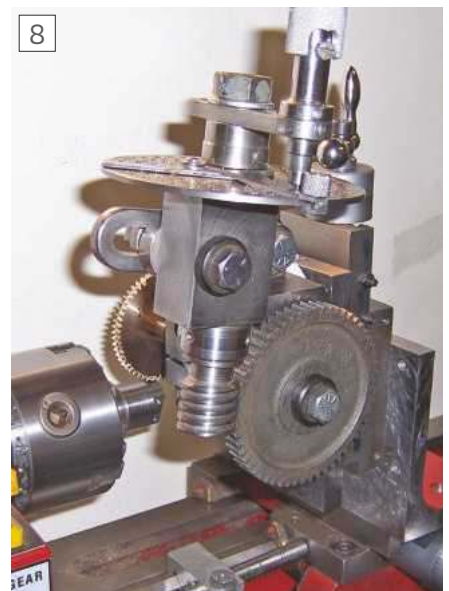
Cutting a spur gear with the MDH mounted on a vertical slide in the lathe.
