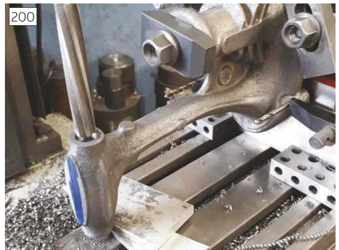
Reaming main bearing hole
