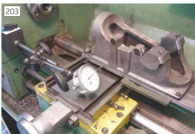
Setting machining plate to lathe axis
