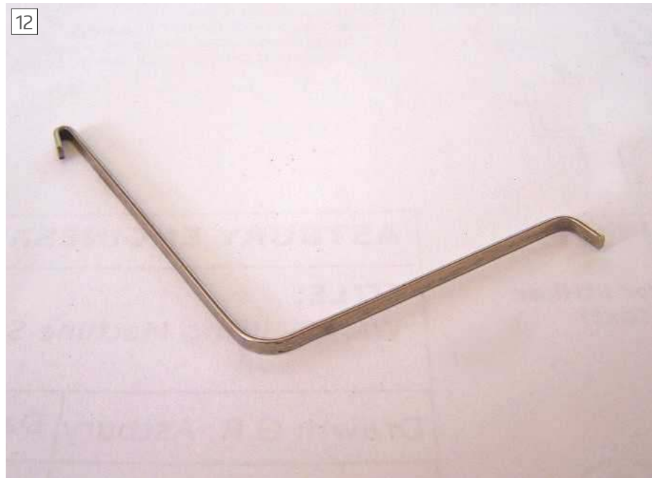
The spring made from stainless steel spring used in a windscreen wiper.
