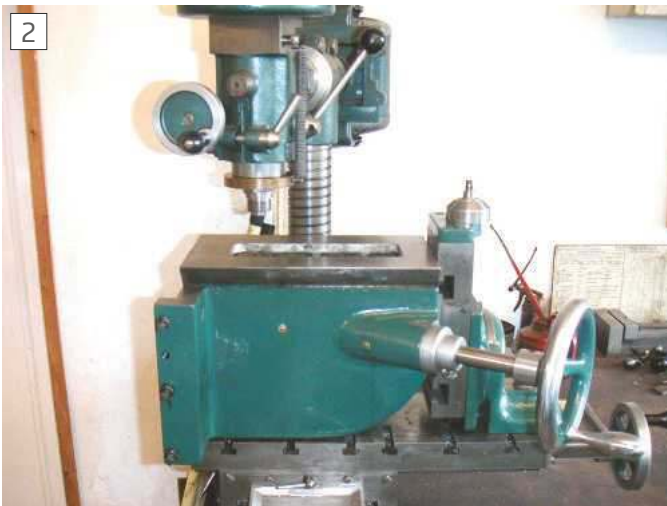
Machining a recess for the slide plates
