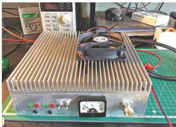
The completed amplifier with extruded aluminium heatsink covering the top surface and fascia with control switches, indicator lamps, power meter and output socket.
