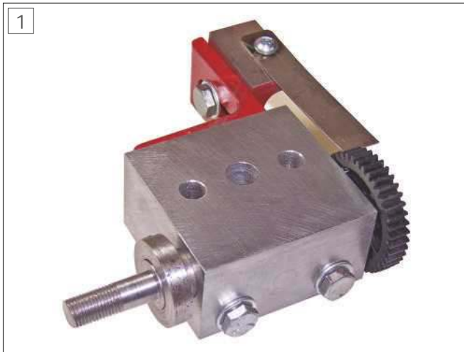
The basic indexing head with a threaded spindle for holding the work.
