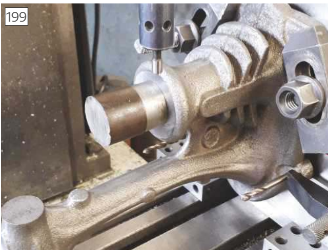
Using edge finder to locate cylinder centre line
