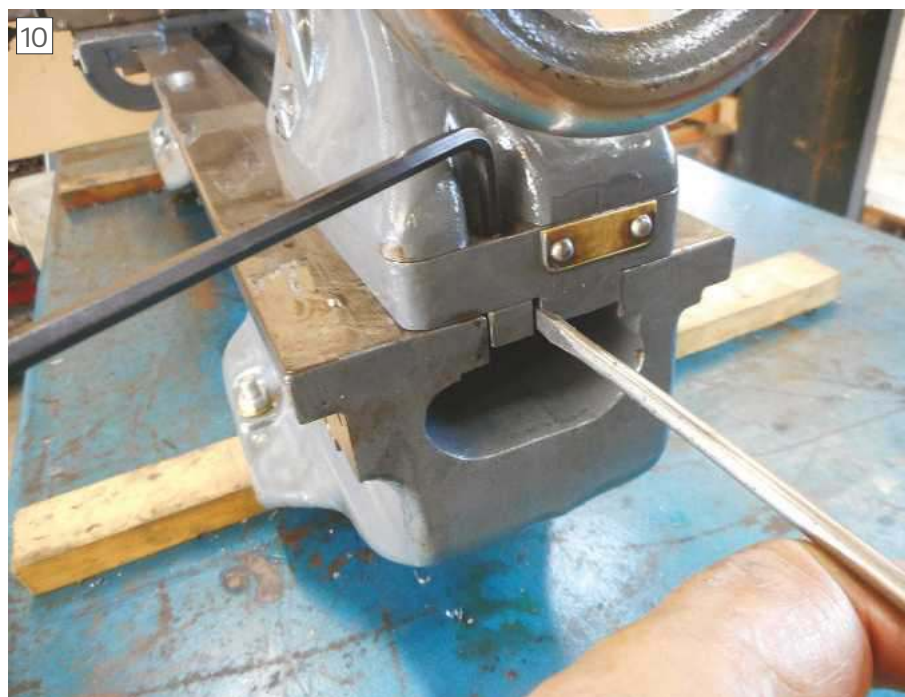
Setting tailstock gib for zero drag, zero shake.
