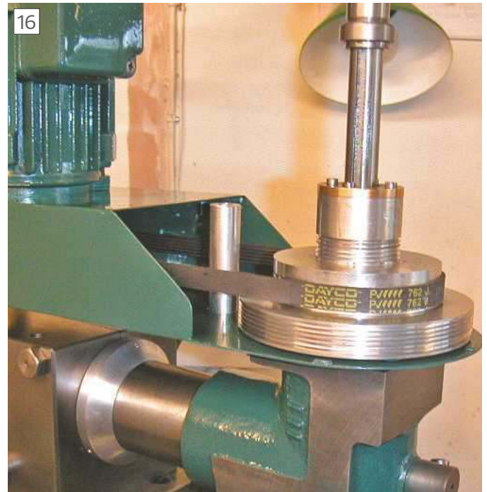
Polyvee pulley on milling head
