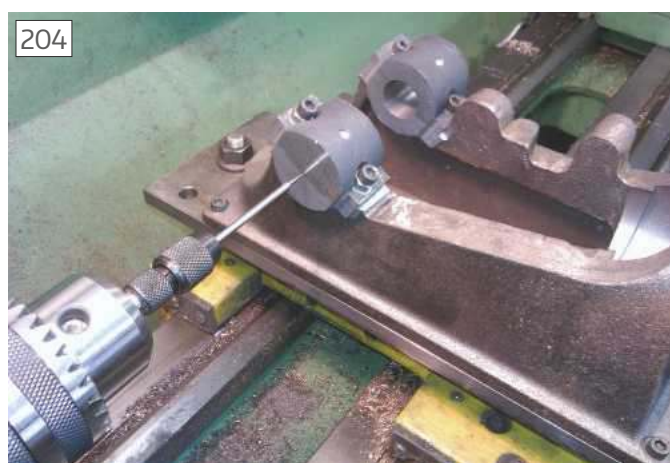
Machining plate set across lathe axis to bore bearings
