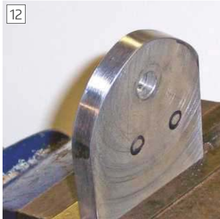
12 The finished piece after a few strokes with a file to smooth out the stepped surface. This profile required three different radii from three different centres. The black circles show the approximate locations of the centres.
