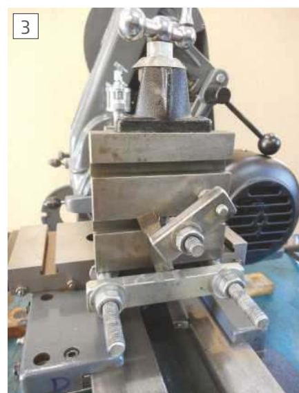
Vertical slide and cutting tool set up to recut No. 3 vertical shear using the saddle as a hand-powered shaper.
