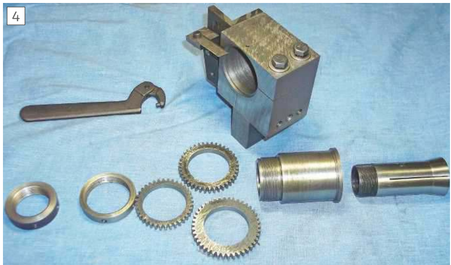
The parts for the 5C collet Dividing Head. Note the three shop-made interchangeable gears, photo credit L.Hoy)
