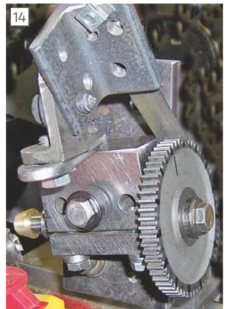
14 The setup to cut a pinion gear using the MDH mounted on a vertical slide in the lathe. ➤
