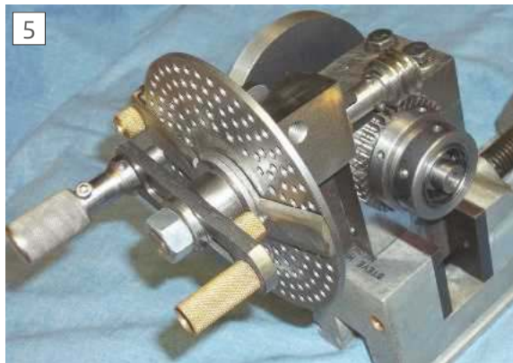
All of the other features of the MDH design are retained in the 5C adaption, including the use of the worm module, photo credit L.Hoy)
