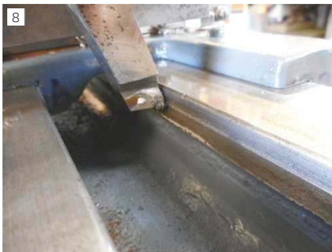
Cut progressing down No. 3 shear shows new and old surfaces.
