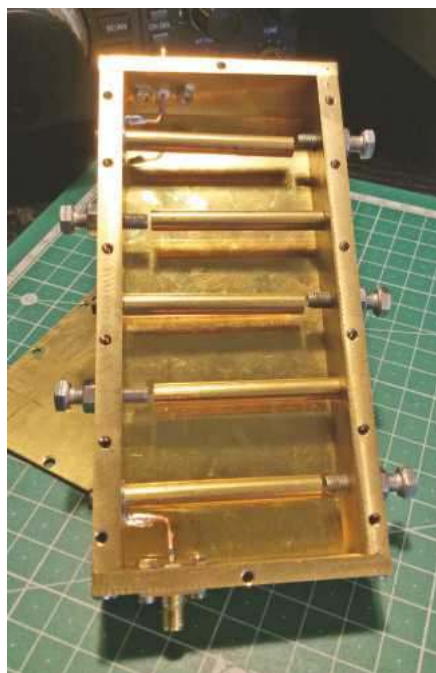
An interdigital filter constructed in brass. This passes a selected band of frequencies and rejects everything else.
