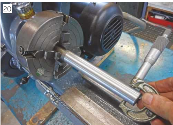
Six-inch turning test piece with no tailstock centre showed zero taper, well within Myford's tolerance of 0.0008".
