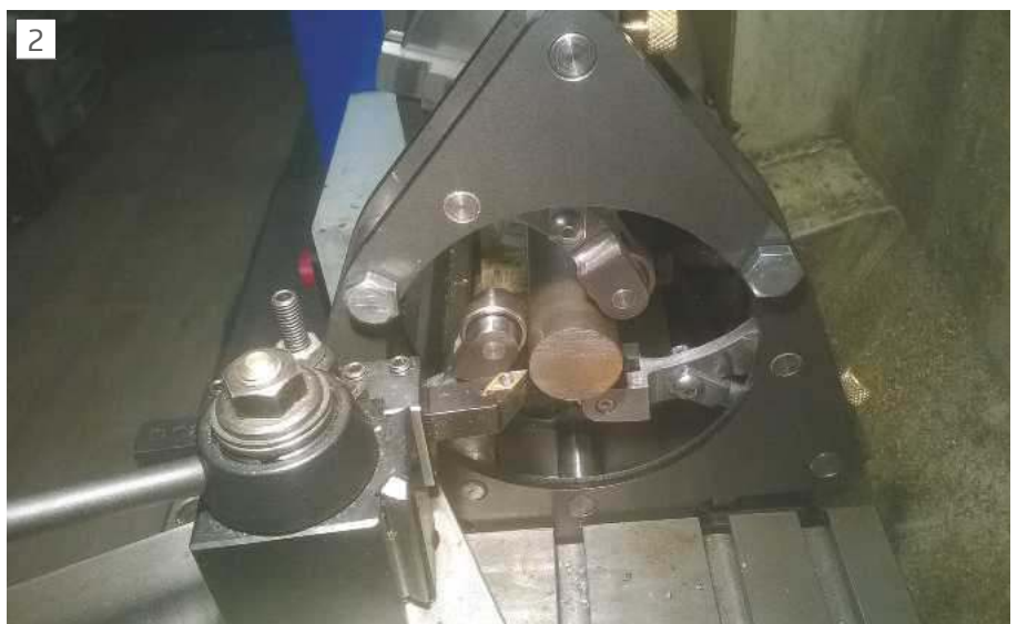
Finished steady attached to the cross slide
