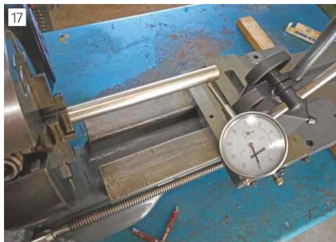
Measuring headstock spindle to bed way alignment with a piece of scrap steel bar and dial indicator.
