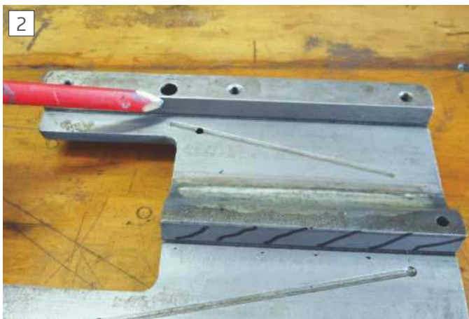
Narrow guide surface with diagonal felt-pen lines. Pencil points to wide-guide surface.
