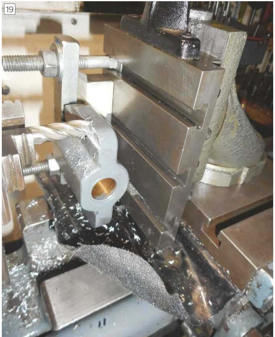
Right hand bracket was clamped by its two studs on a parallel bar for milling on The Flagellator's vertical slide.
