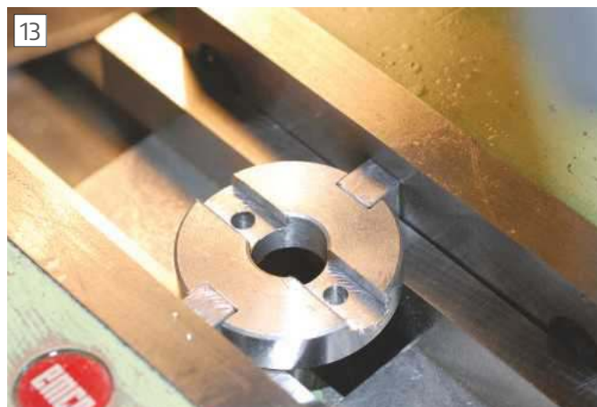
Using tenons to locate block.
