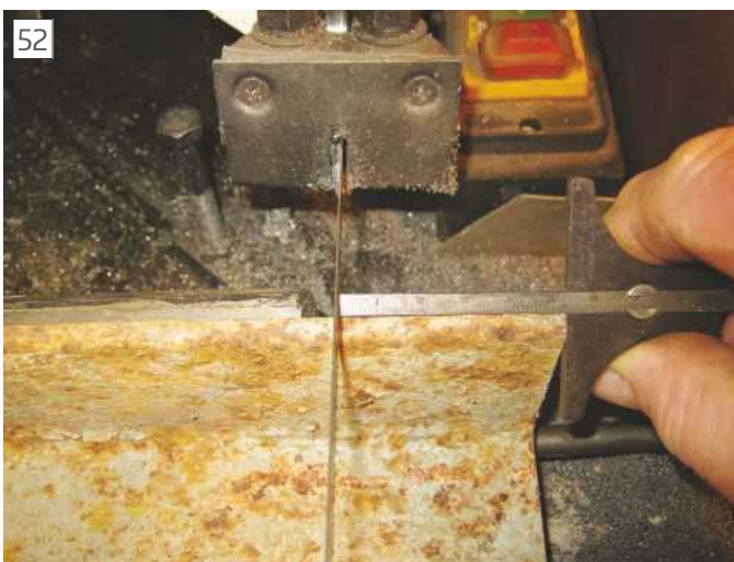
Measuring for cut on two part base bed
