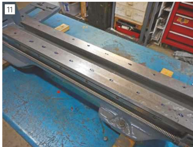
11 Small dabs of bearing blue along the bed ways.
