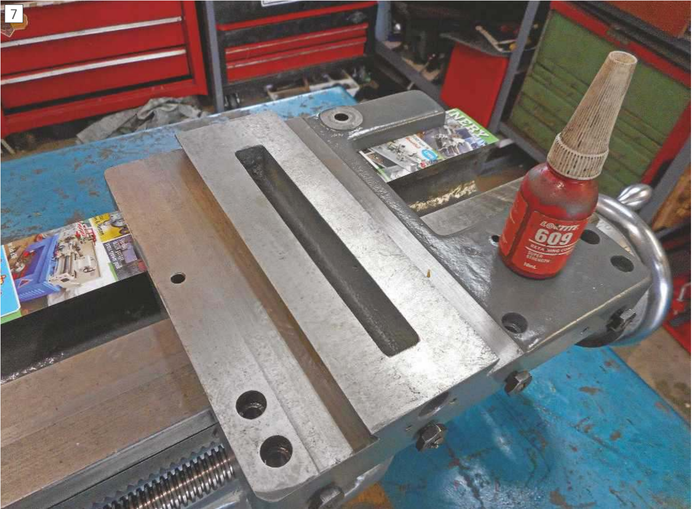
Attaching gauge plate strip to saddle with Loctite. Gib screws clamp saddle and strip in place. MEW cover prevents strip sticking to bed.
