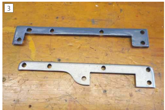
Wide-guide felt wiper housing above, narrow-guide version below.
