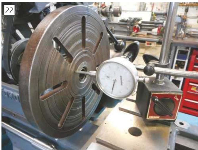
22 Checking cross-slide travel is parallel to the faceplate and thus square to the spindle axis.
