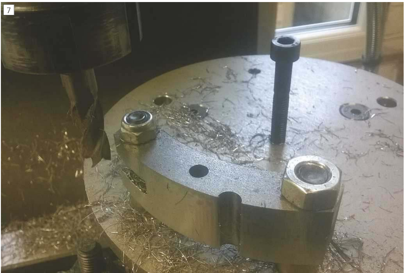
Finger outer curve completed
