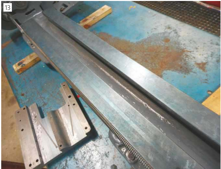
The even thinner layer of blue used for final, accurate spotting.
