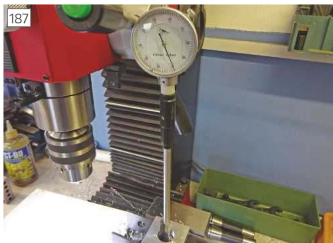
Checking size with preset dial bore gauge
