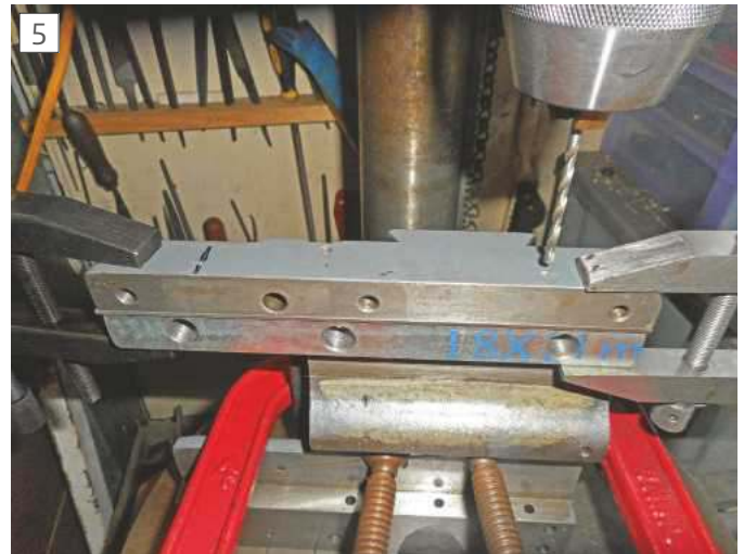
Drilling the dowel holes through the saddle and gauge plate.
