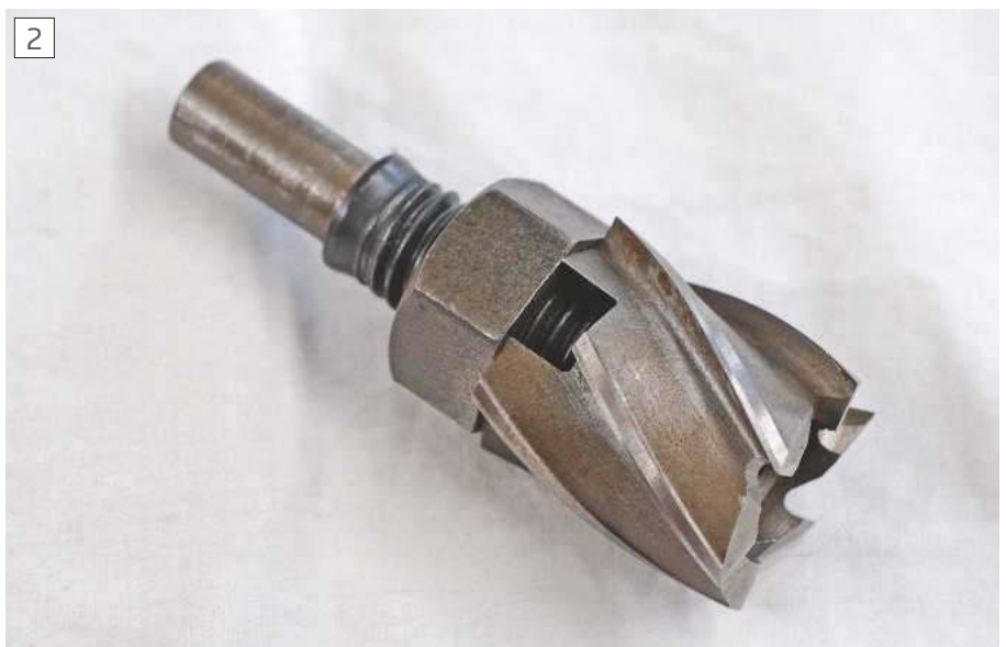
Temporary solution – cutter mounted on a bolt.
