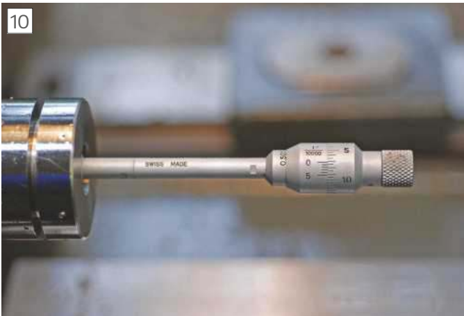
Checking bore for size.
