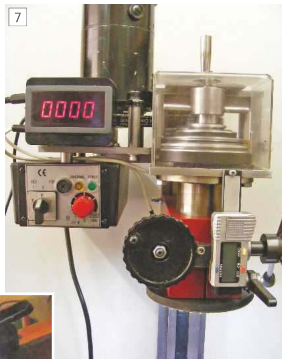
Top of headstock showing the captive draw bar and the new tachometer.
