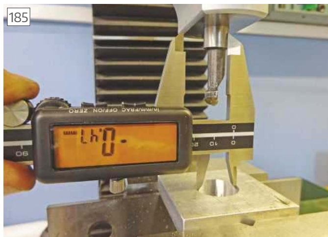
Checking progress of cuts with digital calliper
