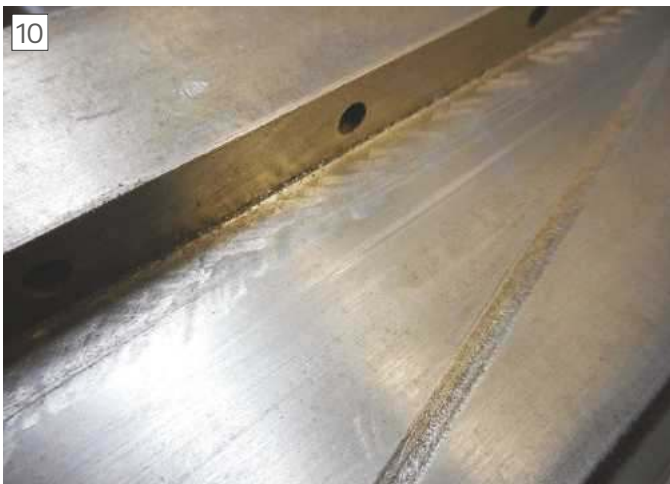
10 First pass of diagonal cross-hatched scraper marks to remove unworn metal.
