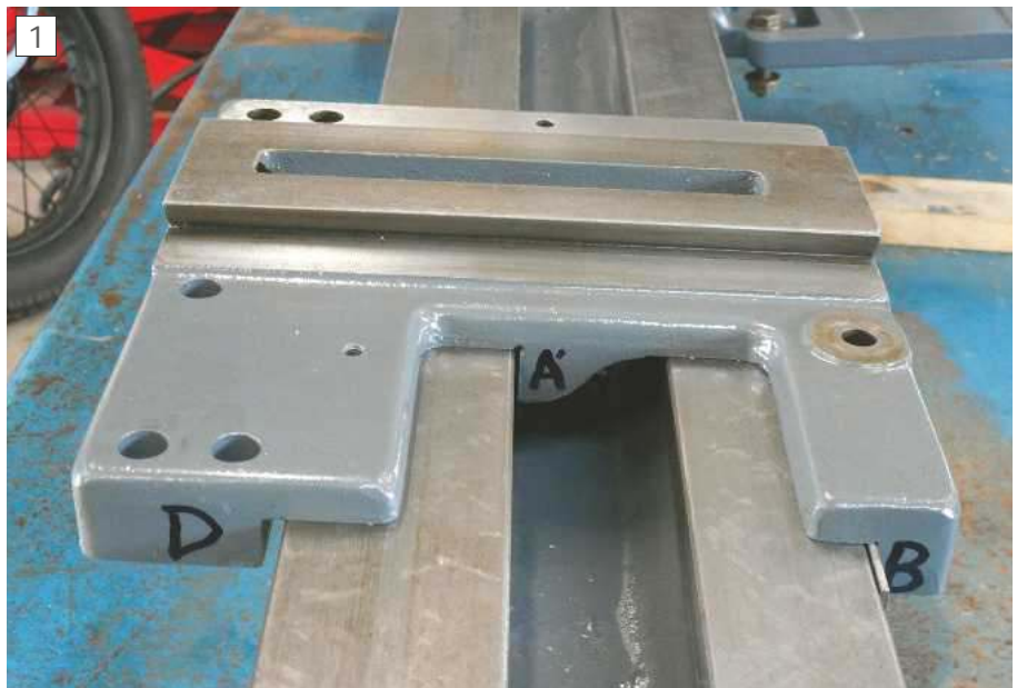
Narrow guide is at A, wide guide at B and gib strip at D.
