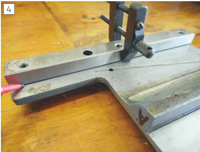
Strip of gauge plate in position with chamfer along bottom edge for scraping clearance.
