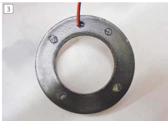
Rear view of MDF ring showing the lead out and the magnets.
