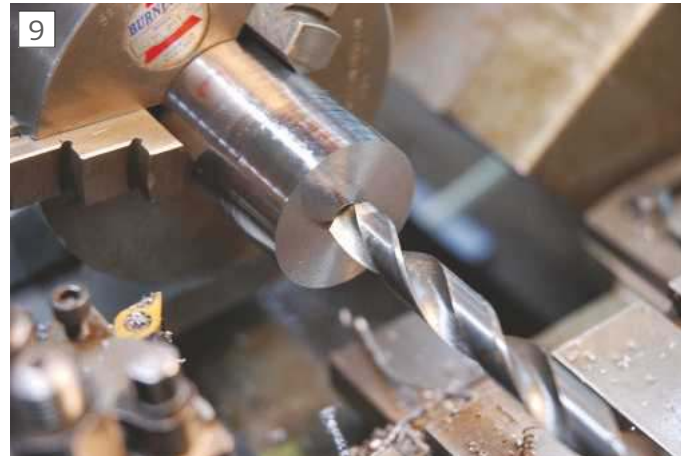
Drilling embryo locking plate.
