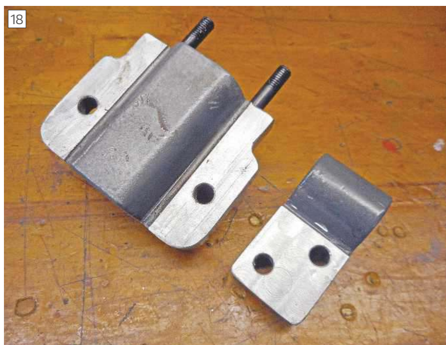
Both lead screw brackets were milled down to align with new apron position.
