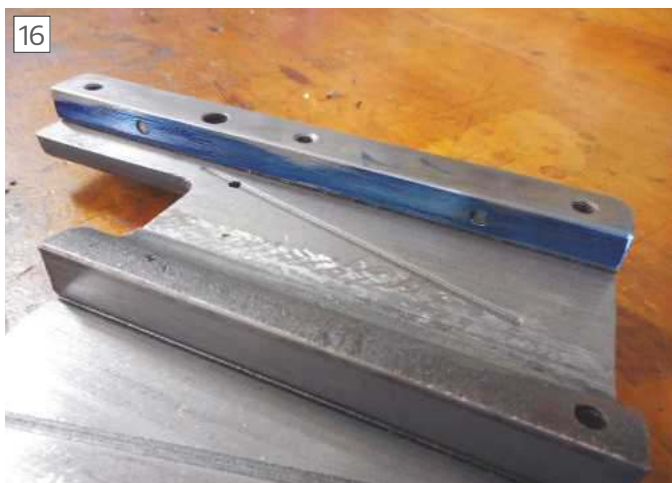
A good reading of blue on the gauge plate strip ensures a good bearing surface. Laid on a bit thick here to show up in the photo.
