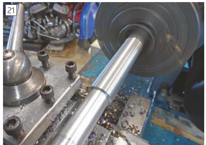
Taking a .100" deep cut with no chatter, tailstock centre in place this time.
