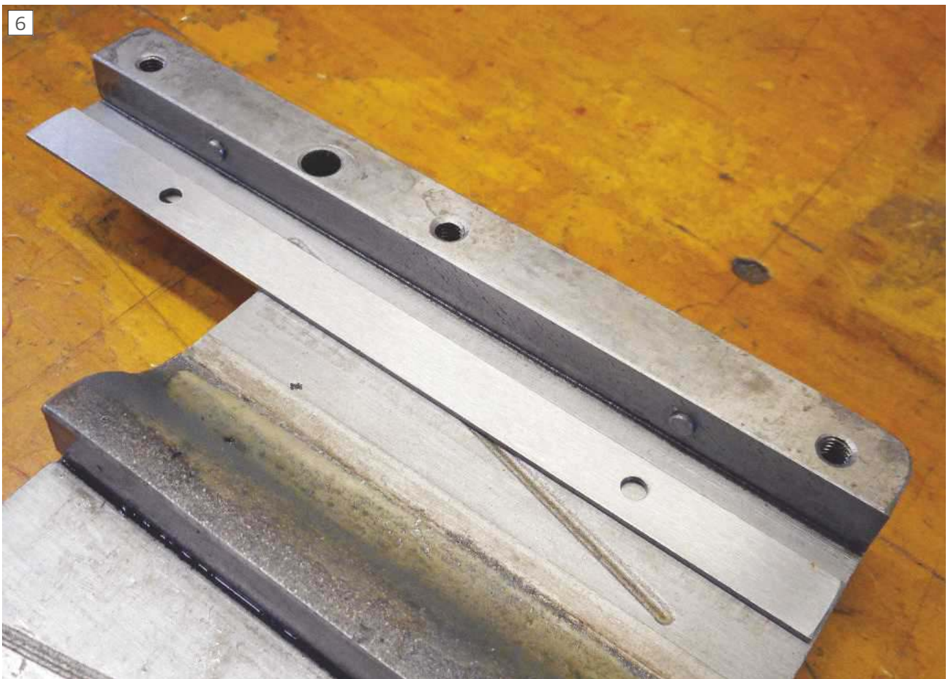
Dowel pins stand 0.040" to 0.050" proud of the saddle surface.
