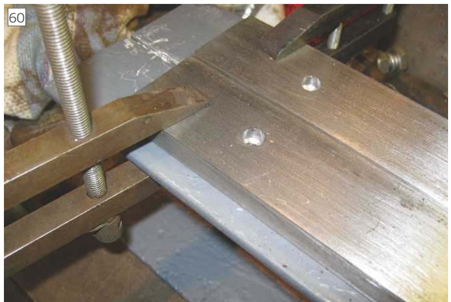
60 Wear plate clamped in position
