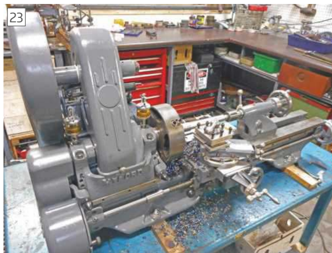
23 Thanks to the wide-guide conversion this once tatty old lathe now cuts as good as new - if not better.
