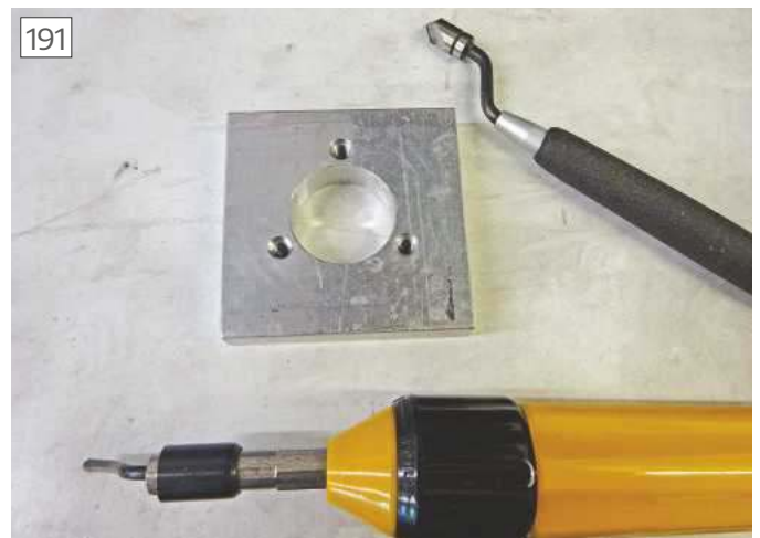
Deburr work on completion
