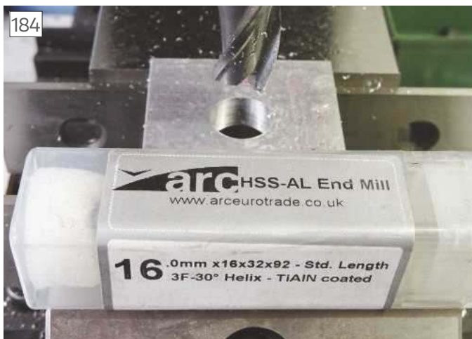
16mm milling cutter used to enlarge hole
