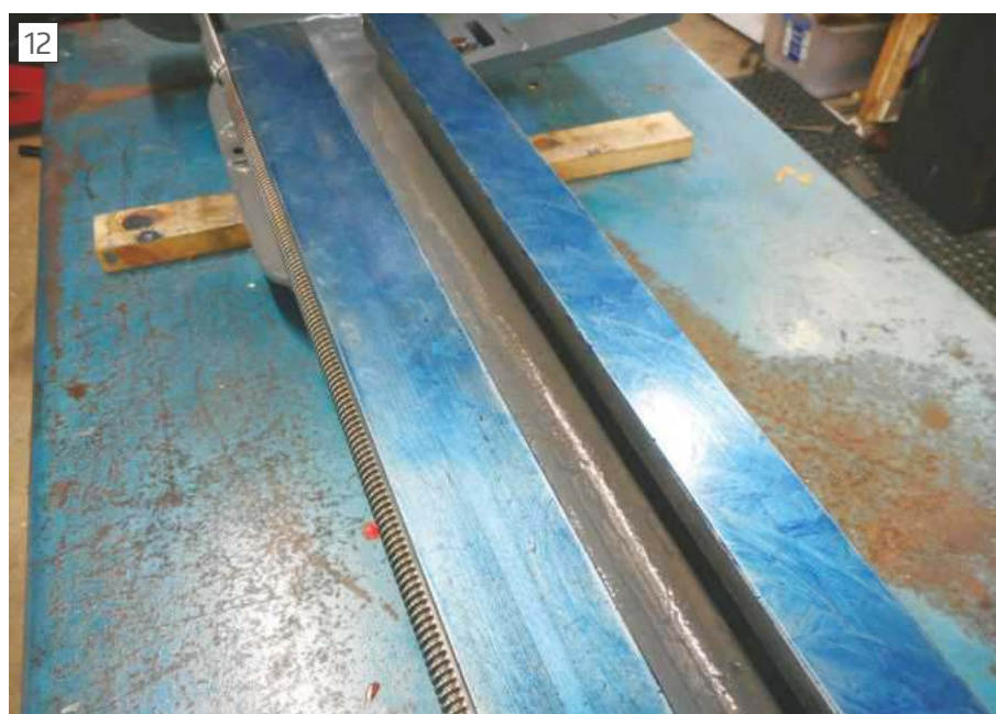
12 Smear the blue on with one clean finger; wipe it off with another to leave a thin layer.
