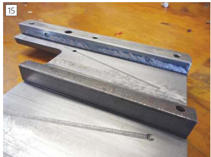
First run of scraper marks along the added strip of gauge plate.
