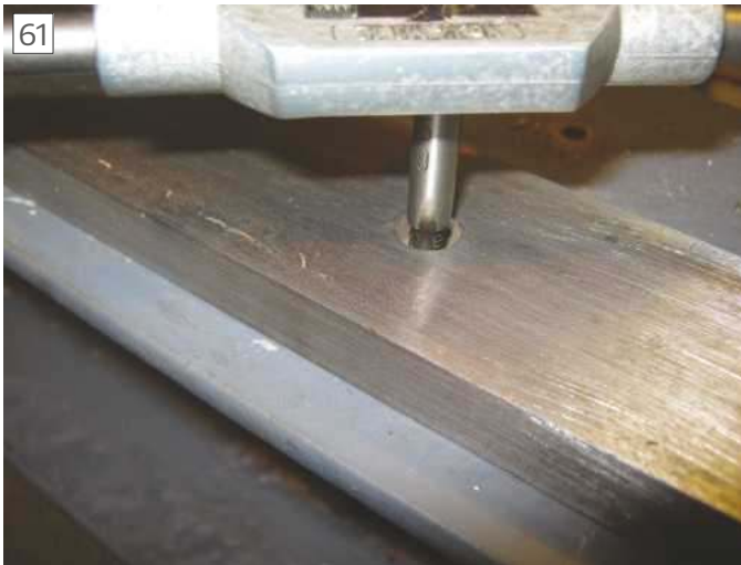
Using wear plate as tapping guide
