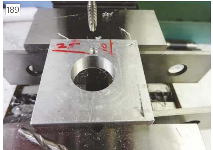
Deep spot drilling of first hole
