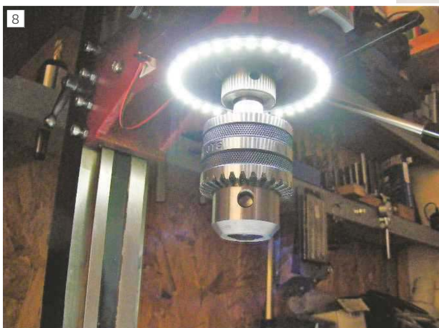
The 100mm ring light installed.
