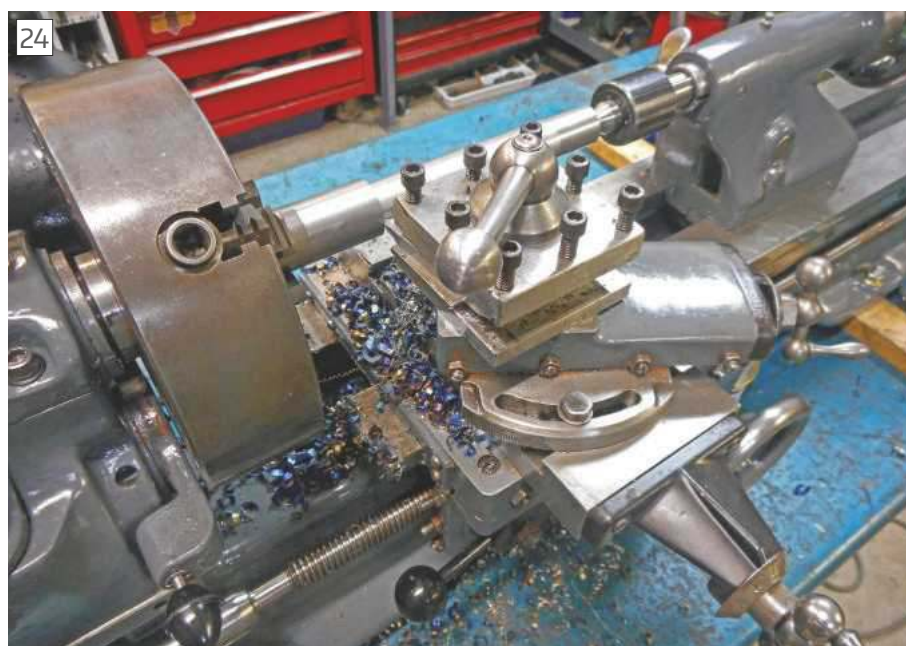
24 A once discarded machine now turning out productive work, evidenced by thick blue swarf with no chatter.
