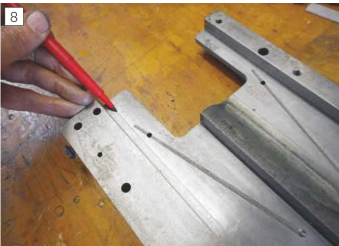
Unworn section of saddle needs to be relieved to clear bed way in new position.
