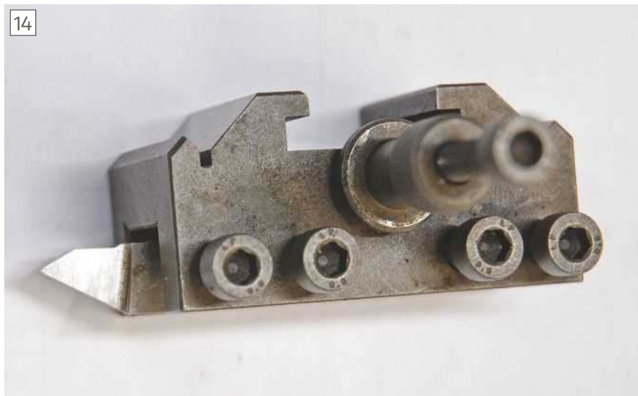
Hand ground thread cutter.
