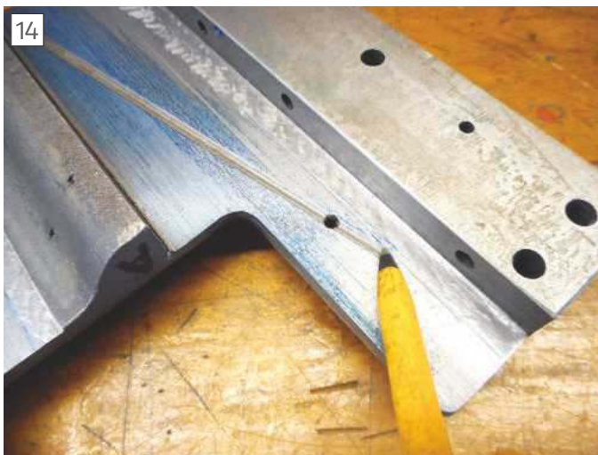
High spots on the saddle ways were further scraped back.
