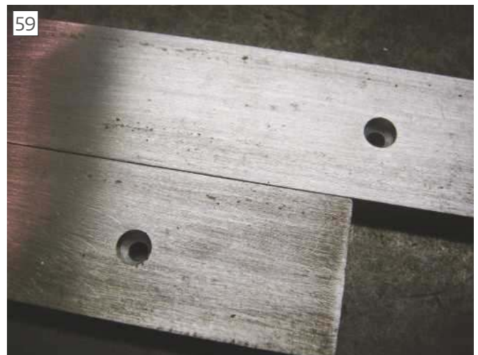
59 Counter bored holes on wear plate
