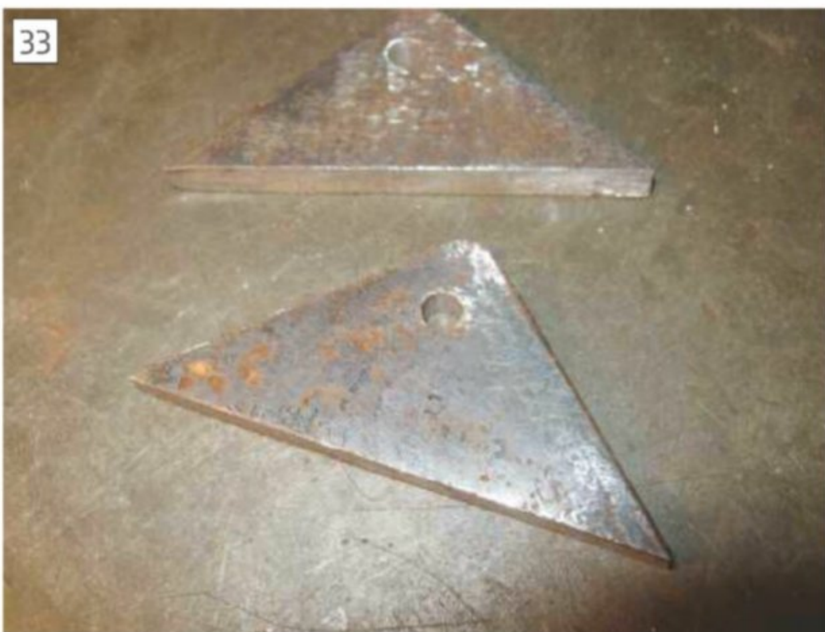
Spring supports drilled
