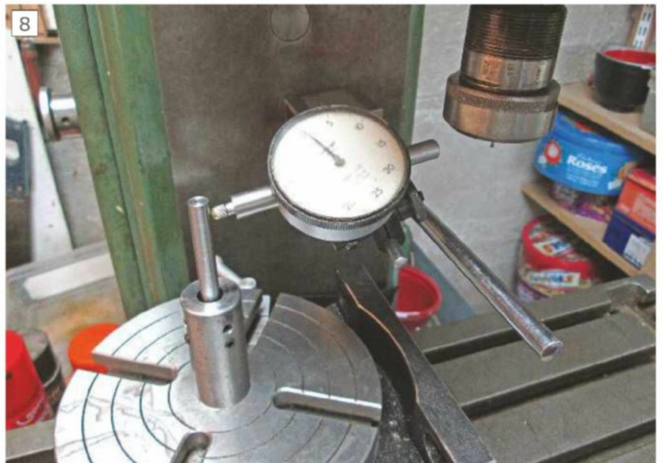
Checking that the holder is mounted vertically
