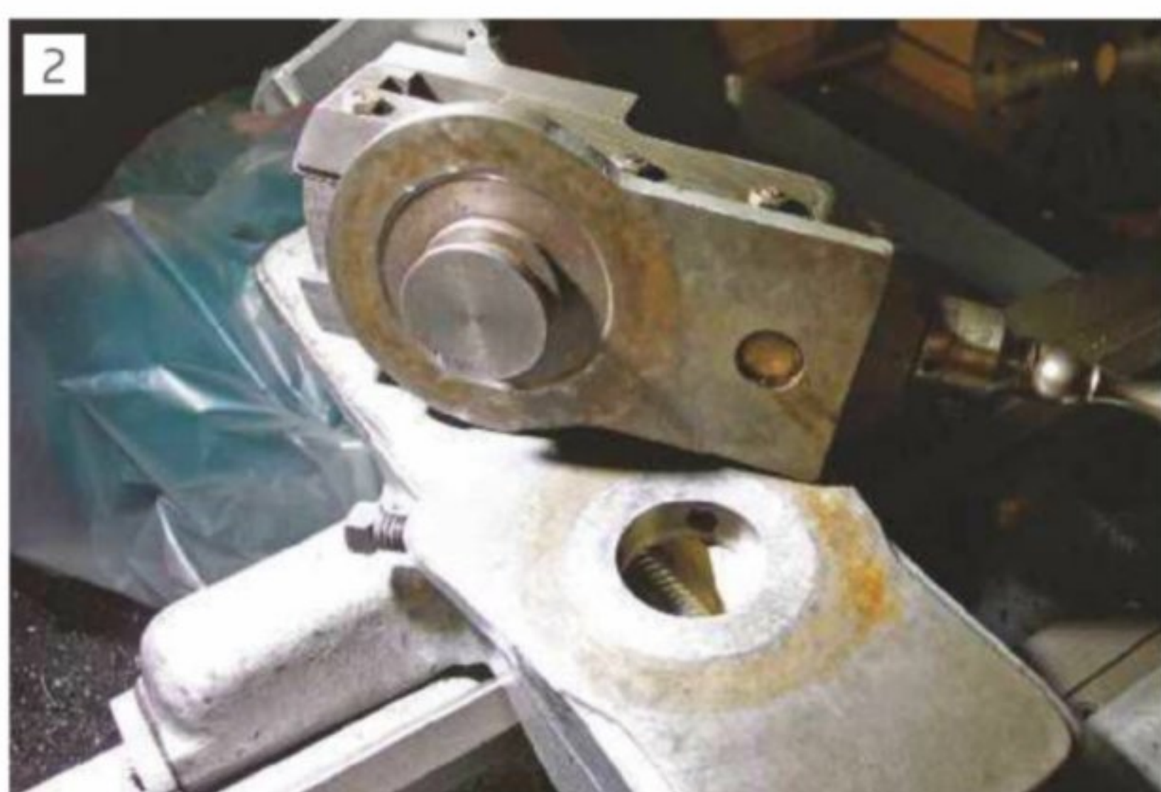
The normal mounting method for the compound slide
