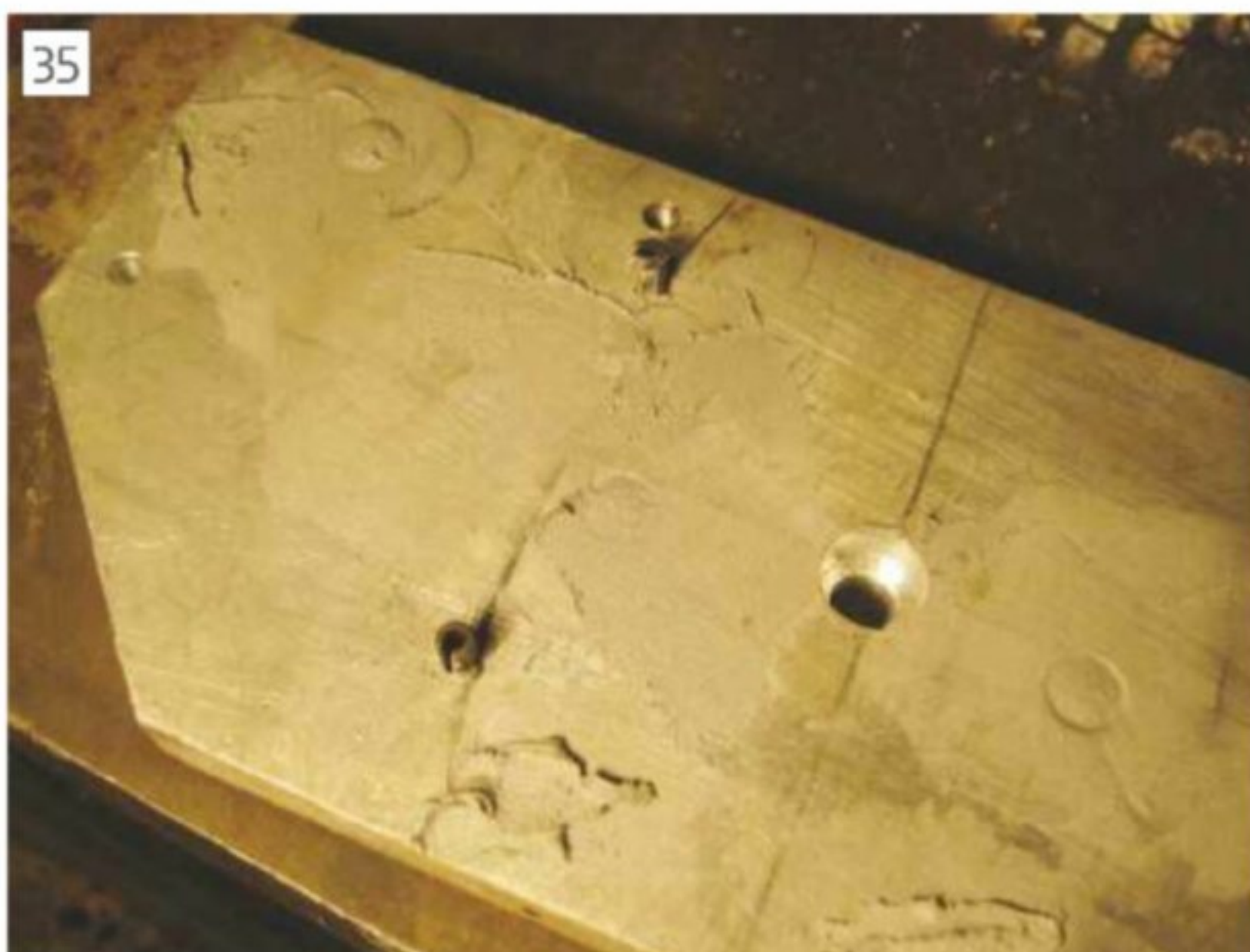
Holes in ram plate filled with filler
