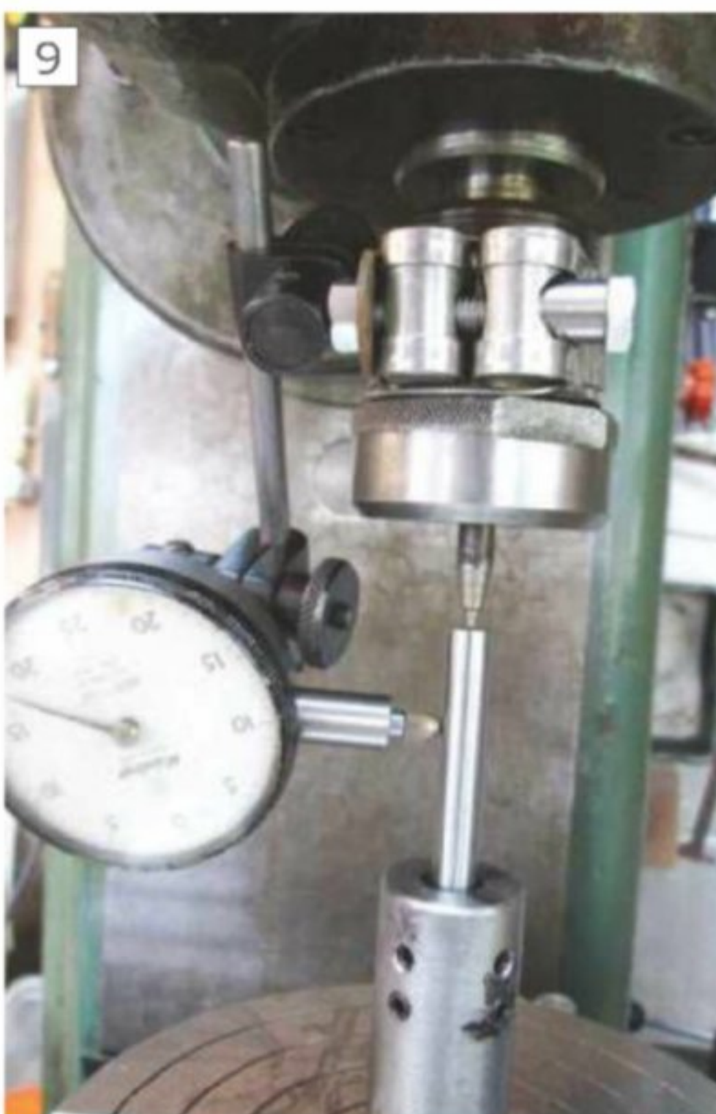
Checking that the holder is mounted concentrically
