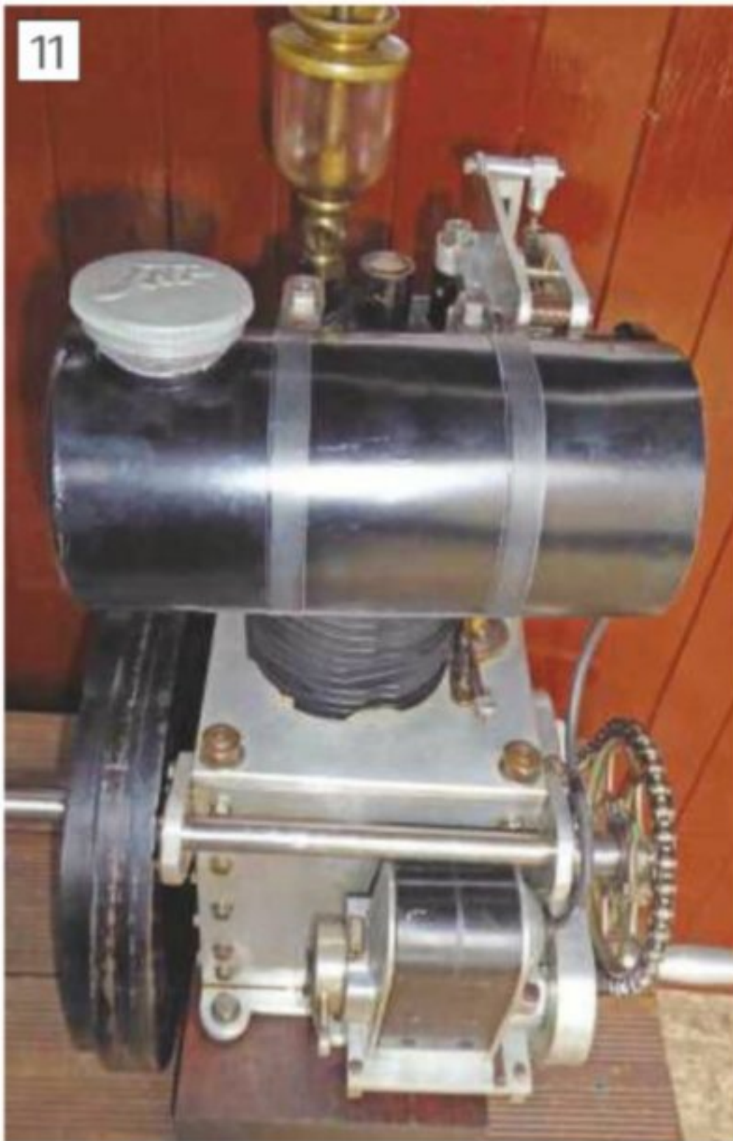
Engine with JAP fuel tank sourced by Allen Berman from eBay. Allen Berman 2018
