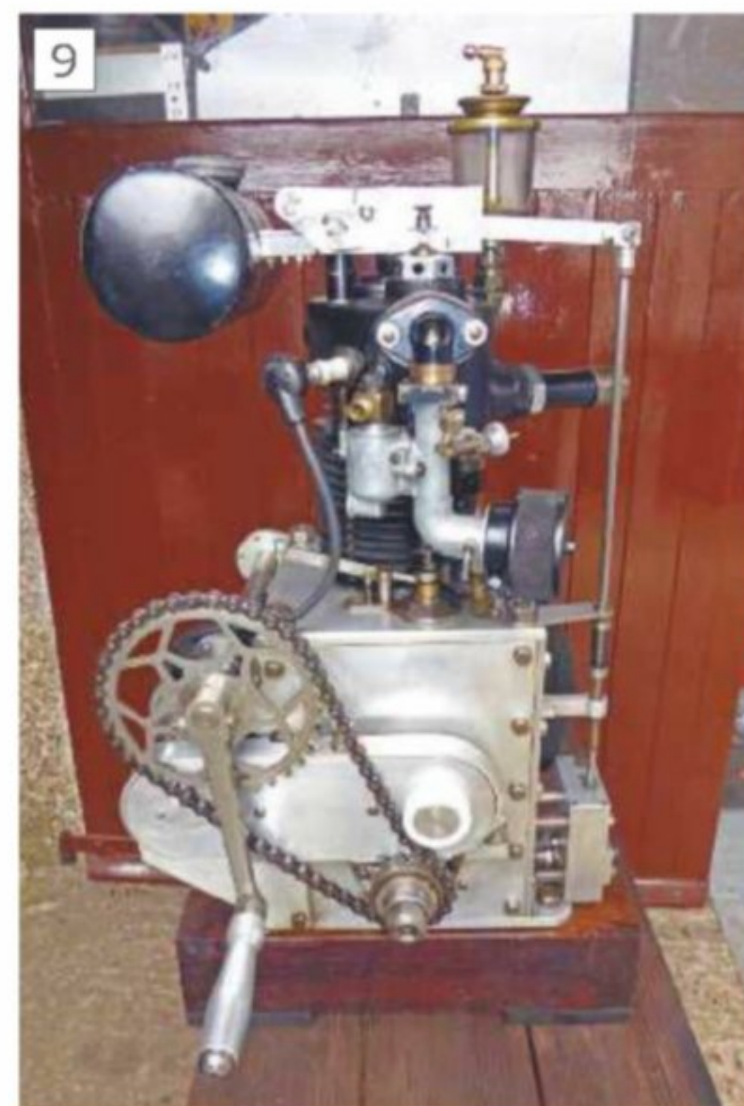
Engine with link rod and lever controlling inlet valve
