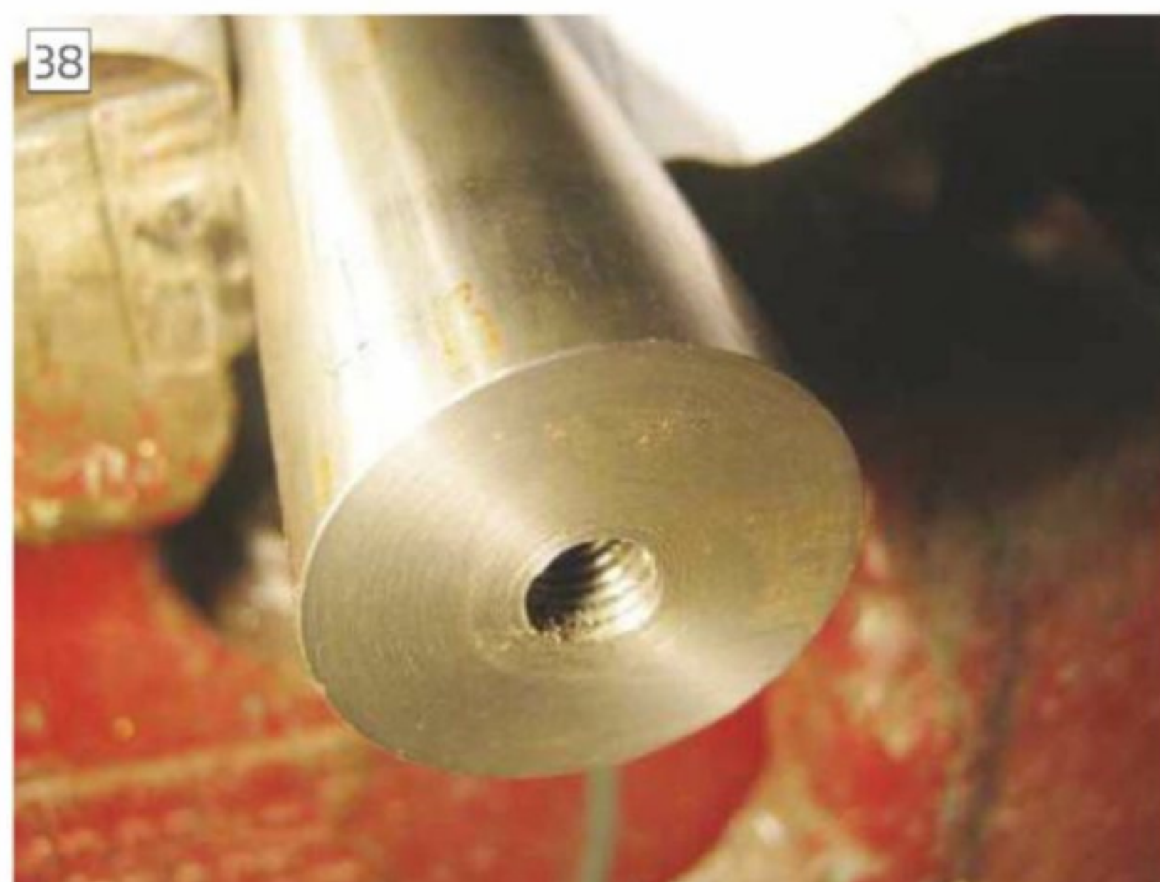
The first ram thread finished
