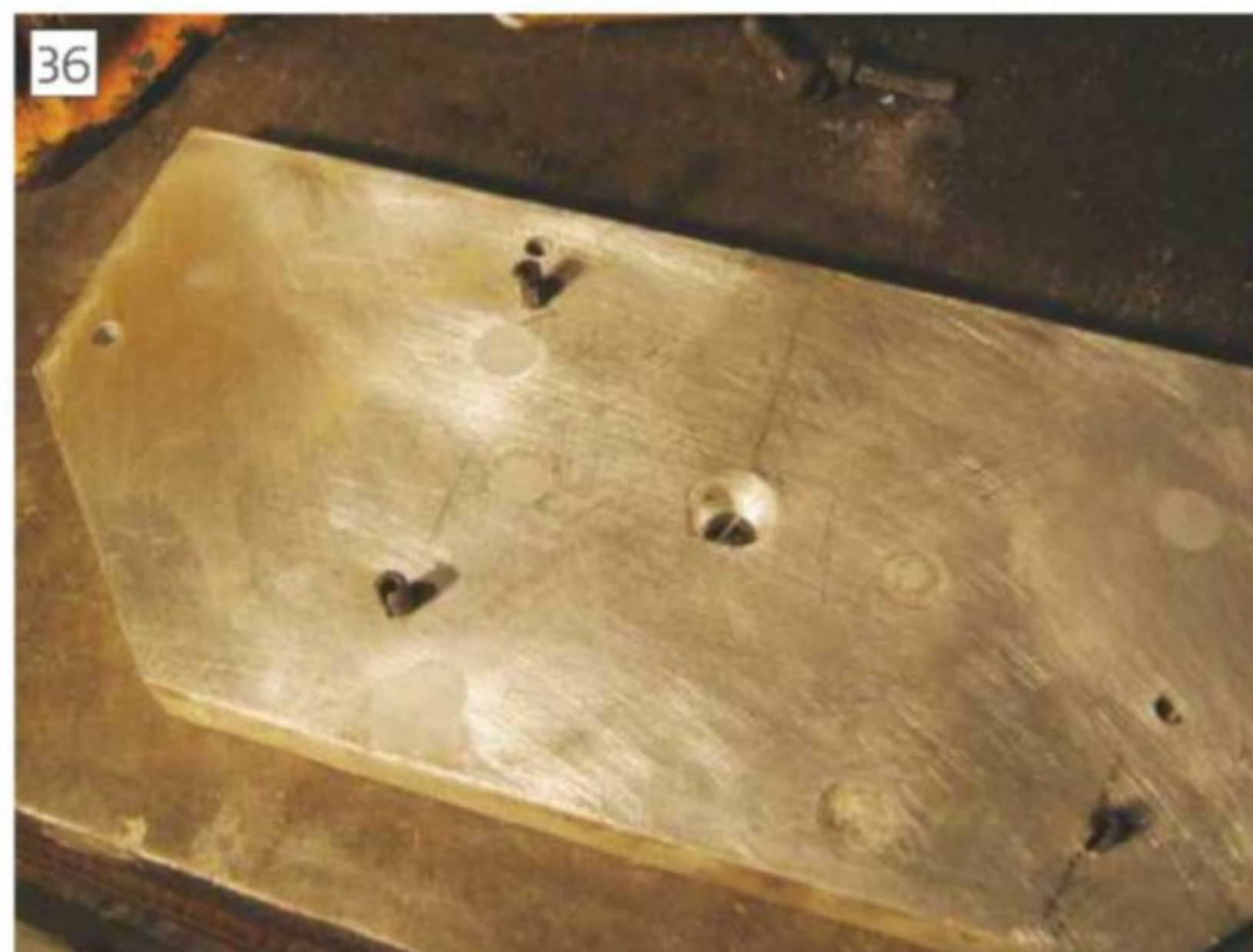
Ram plate holes partly cleaned
