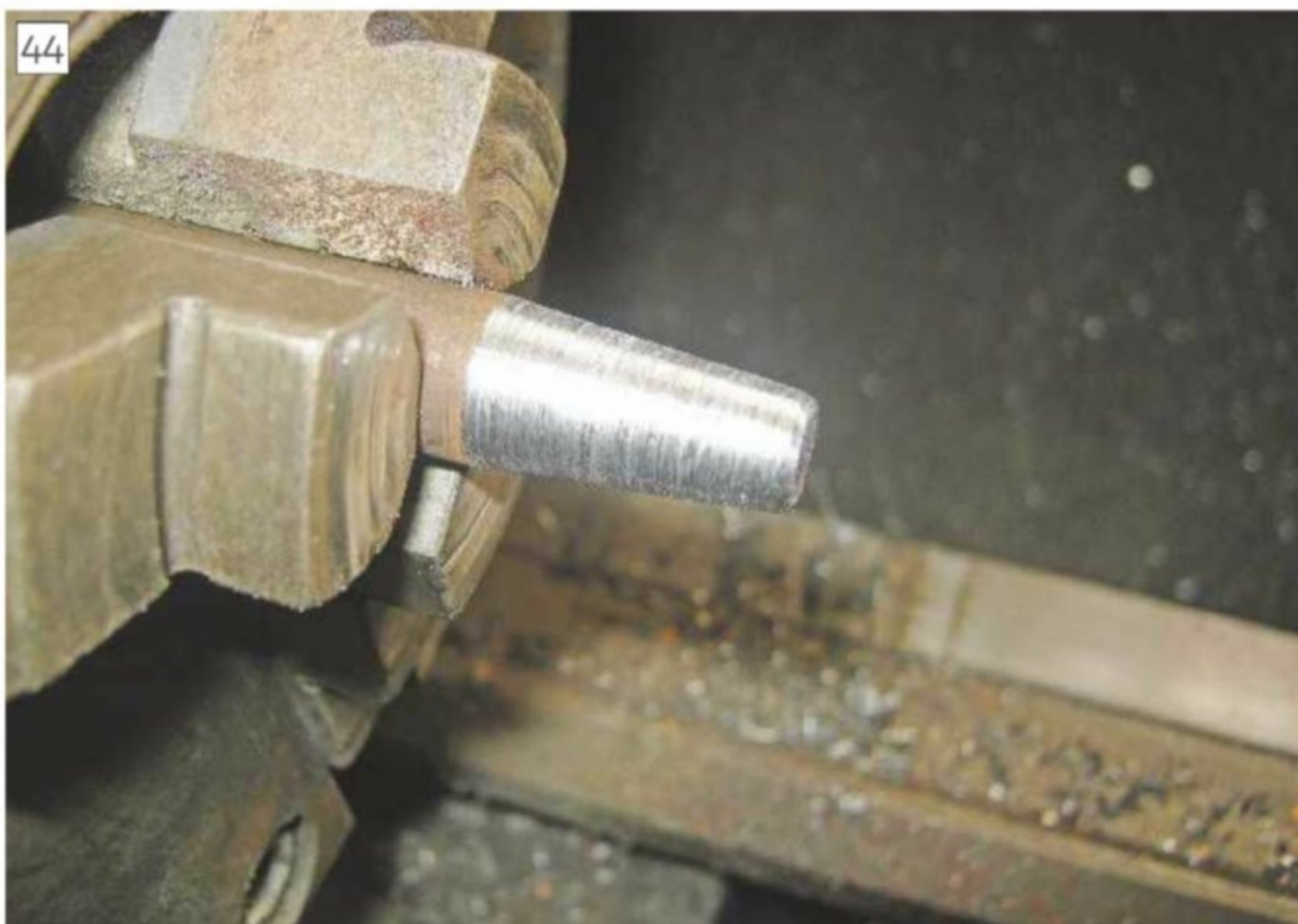
Taper on base frame support pins
