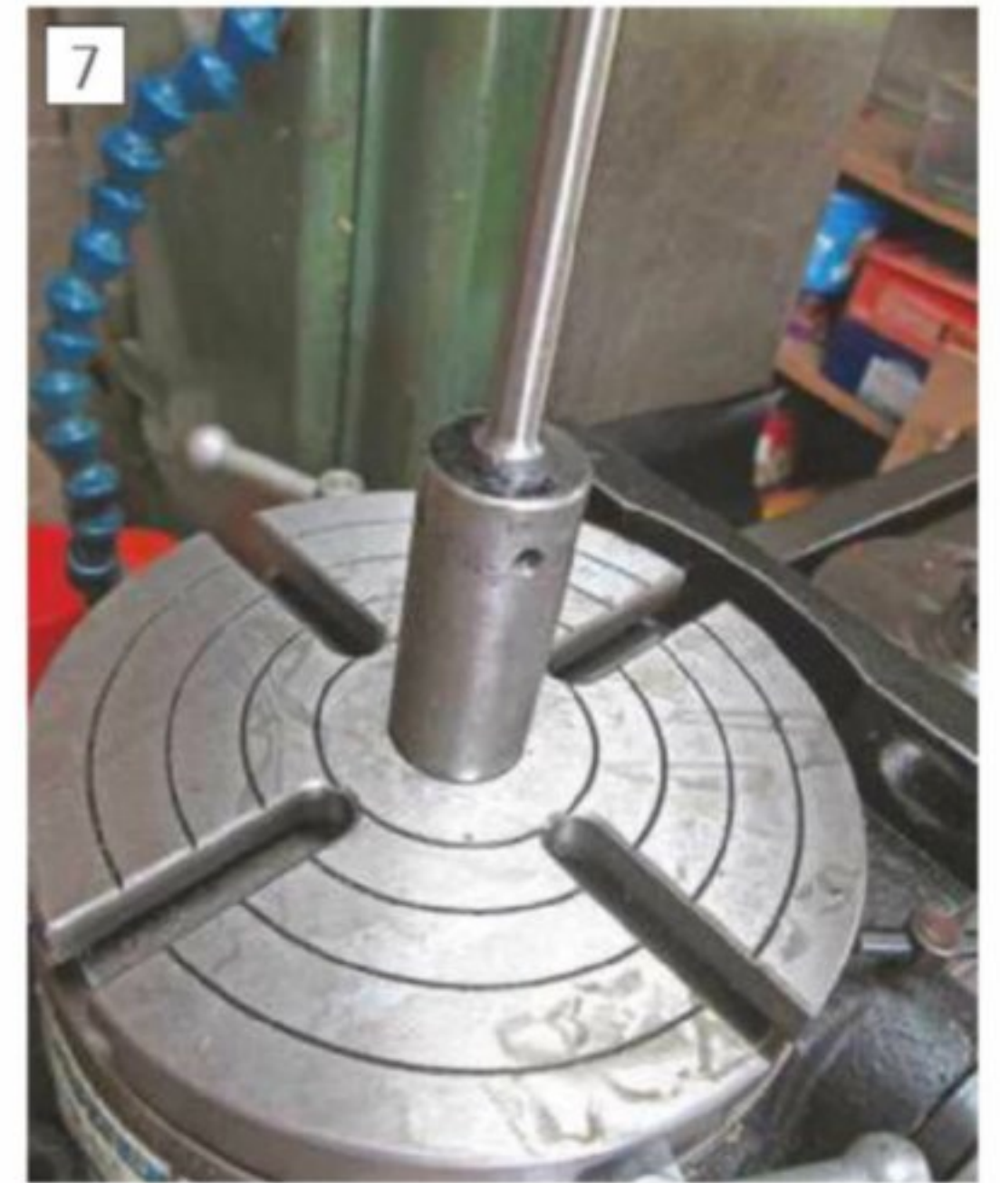
Mandrel and holder mounted on the rotary table
