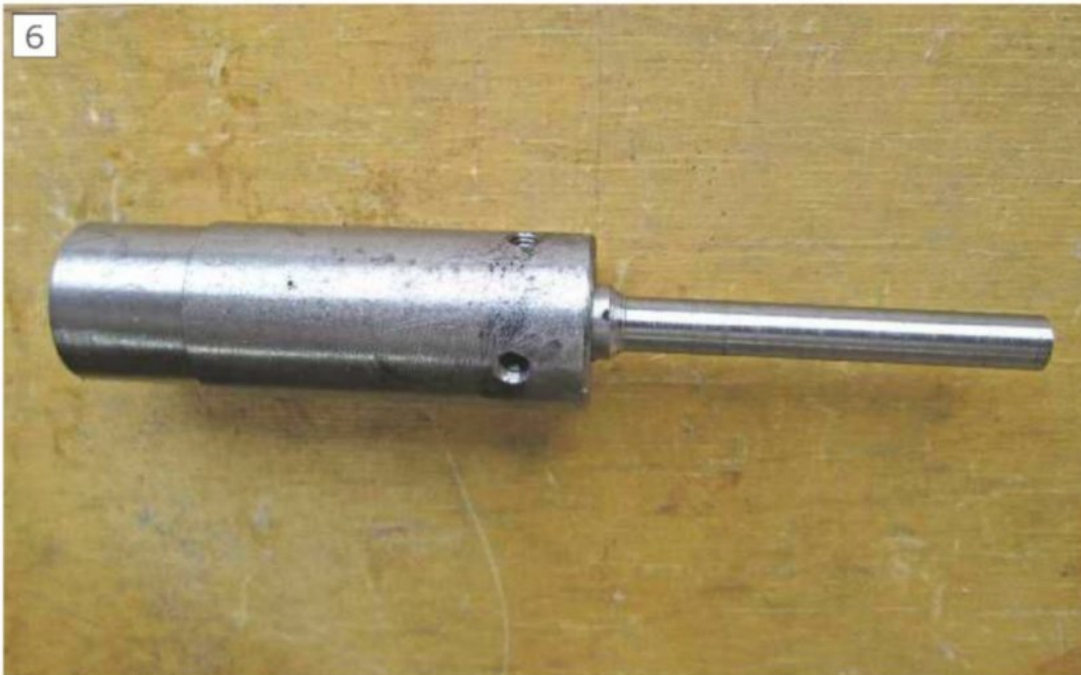
Holder mounted in mandrel showing retaining screws
