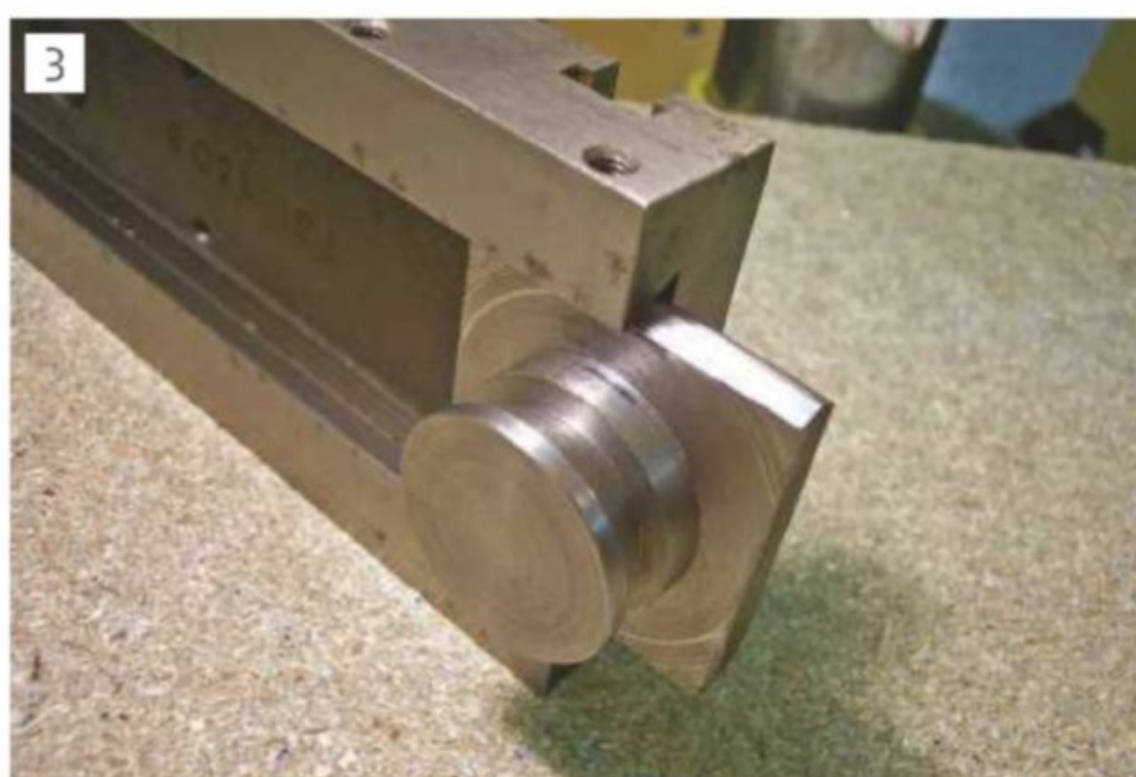
A mounting foot machined to fit the Myford slide
