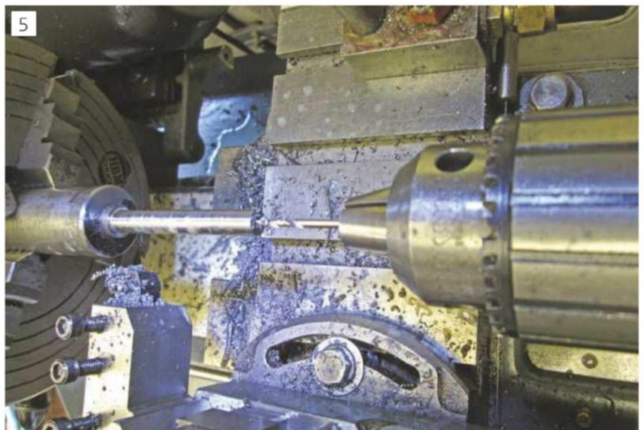
Holder held in mandrel mounted in 4 jaw chuck being drilled tapping size
