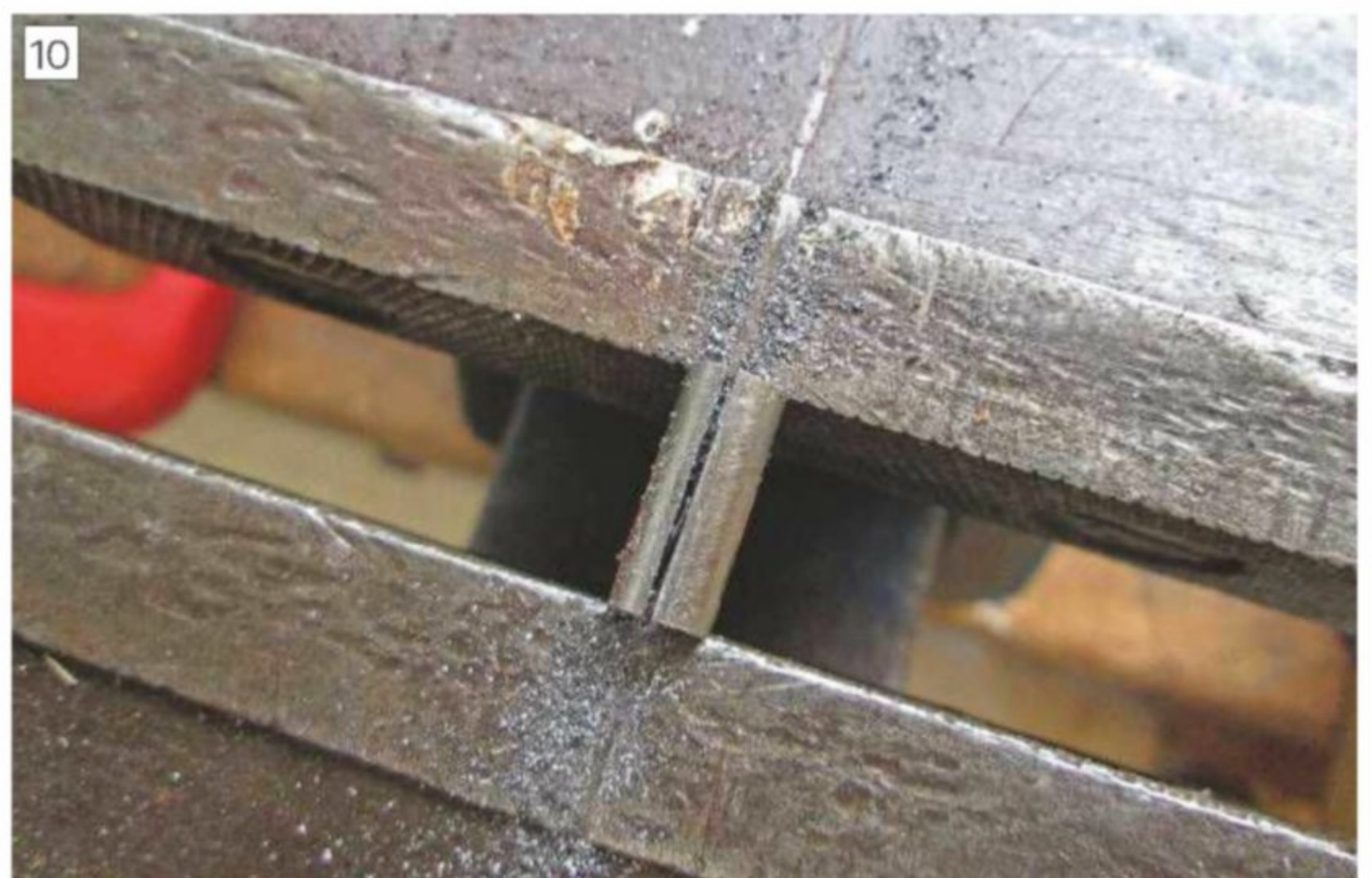
Split sleeve to enable milling cutter to be mounted in the collet
