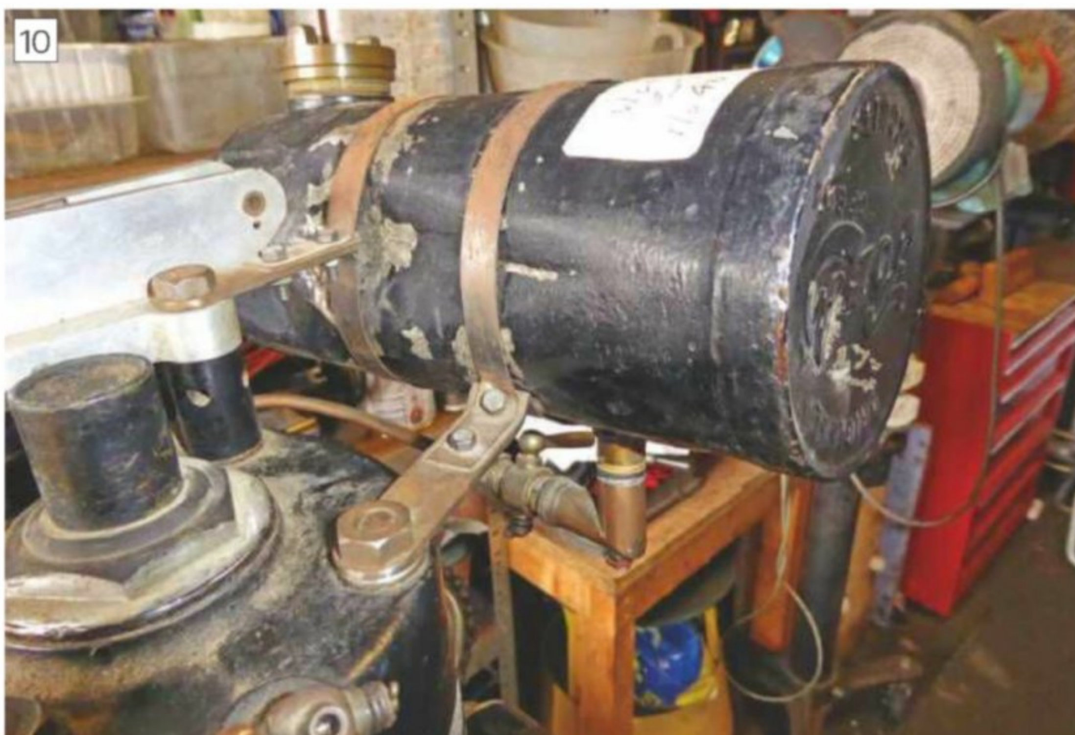
Damaged fuel tank before replacement. Allen Berman 2018
