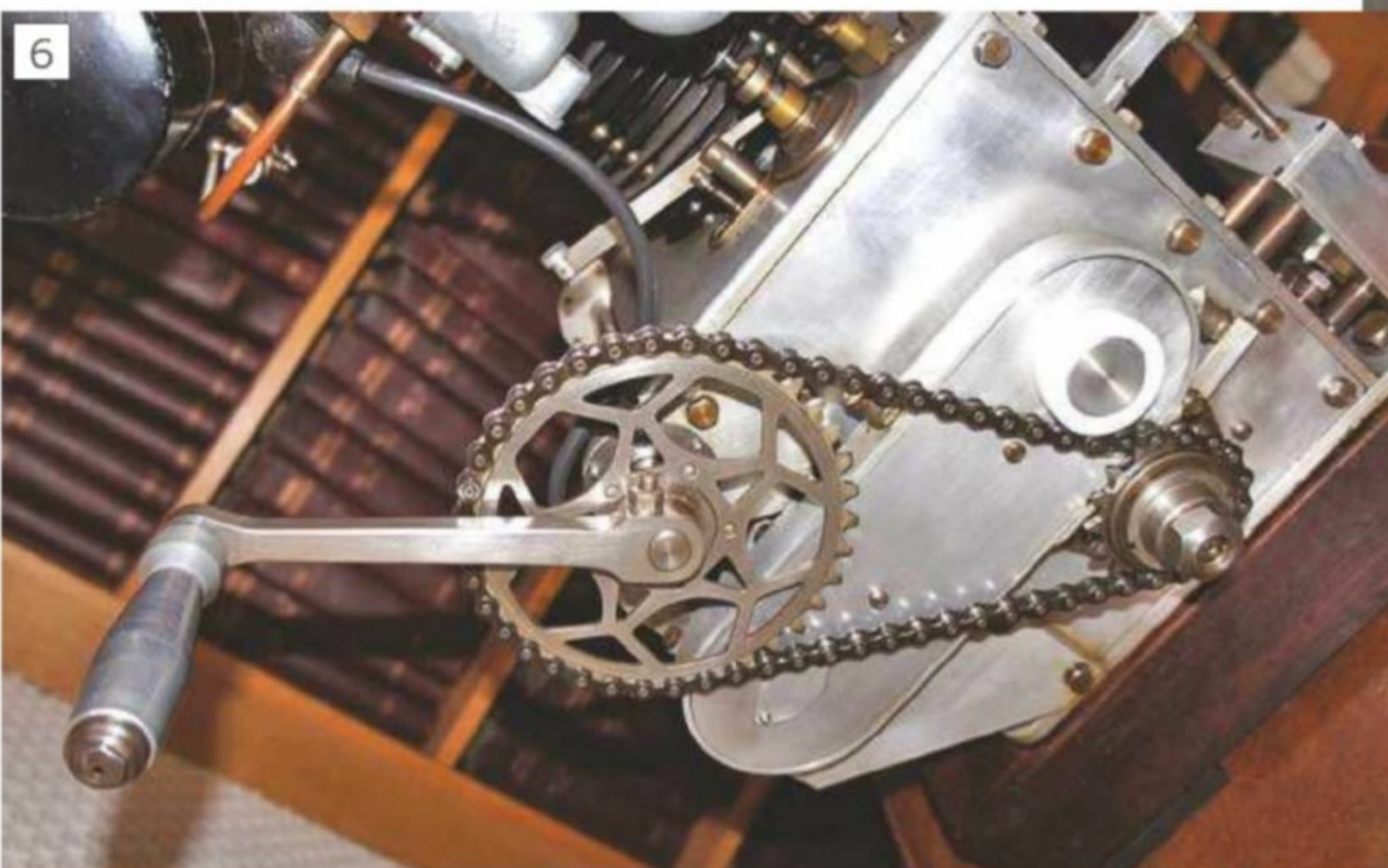
Starting handle and chain, with PTFE roller added to tension chain. This is removable in line with sound conservation practice. © Allen Berman 2018
