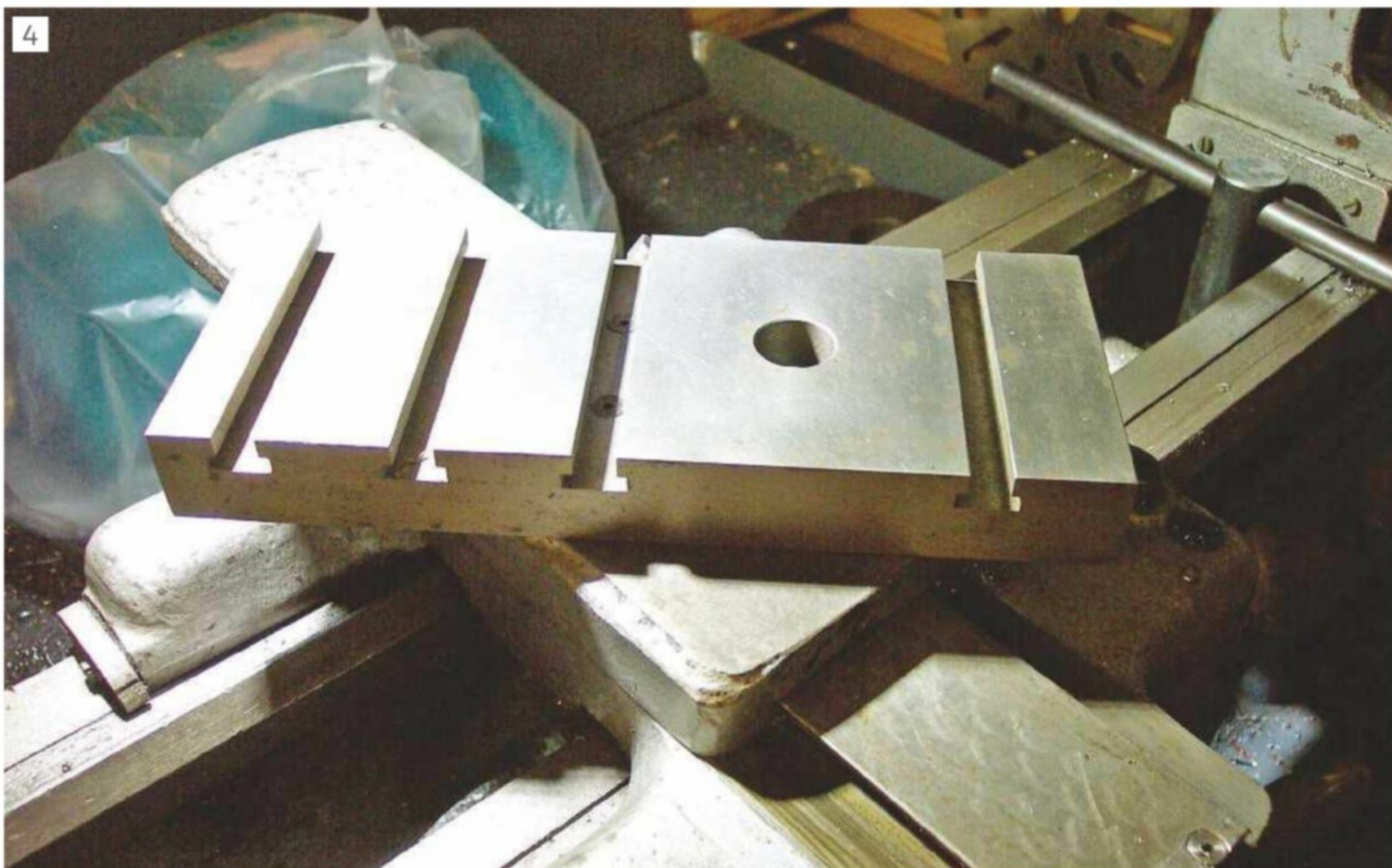
Myford slide in place of the Sabel compound
