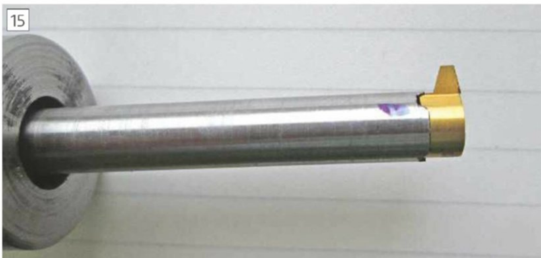
Mounted Acme insert on holder Drawings
