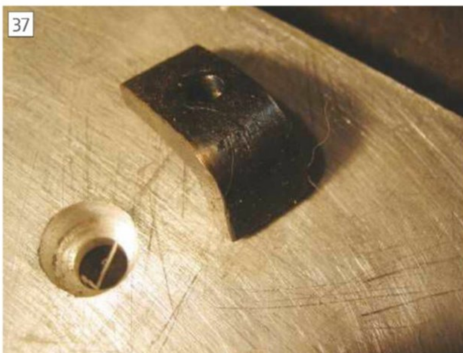
Small jack clamp after blueing
