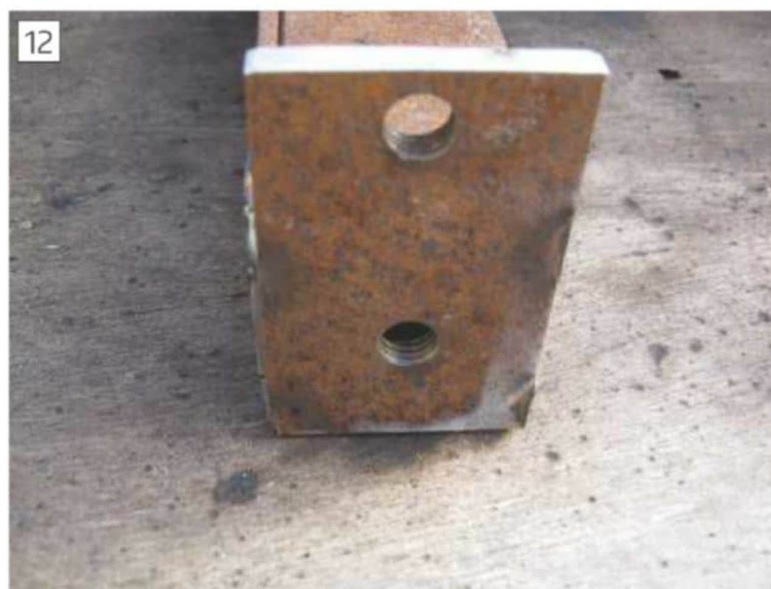
The end plate fitted
