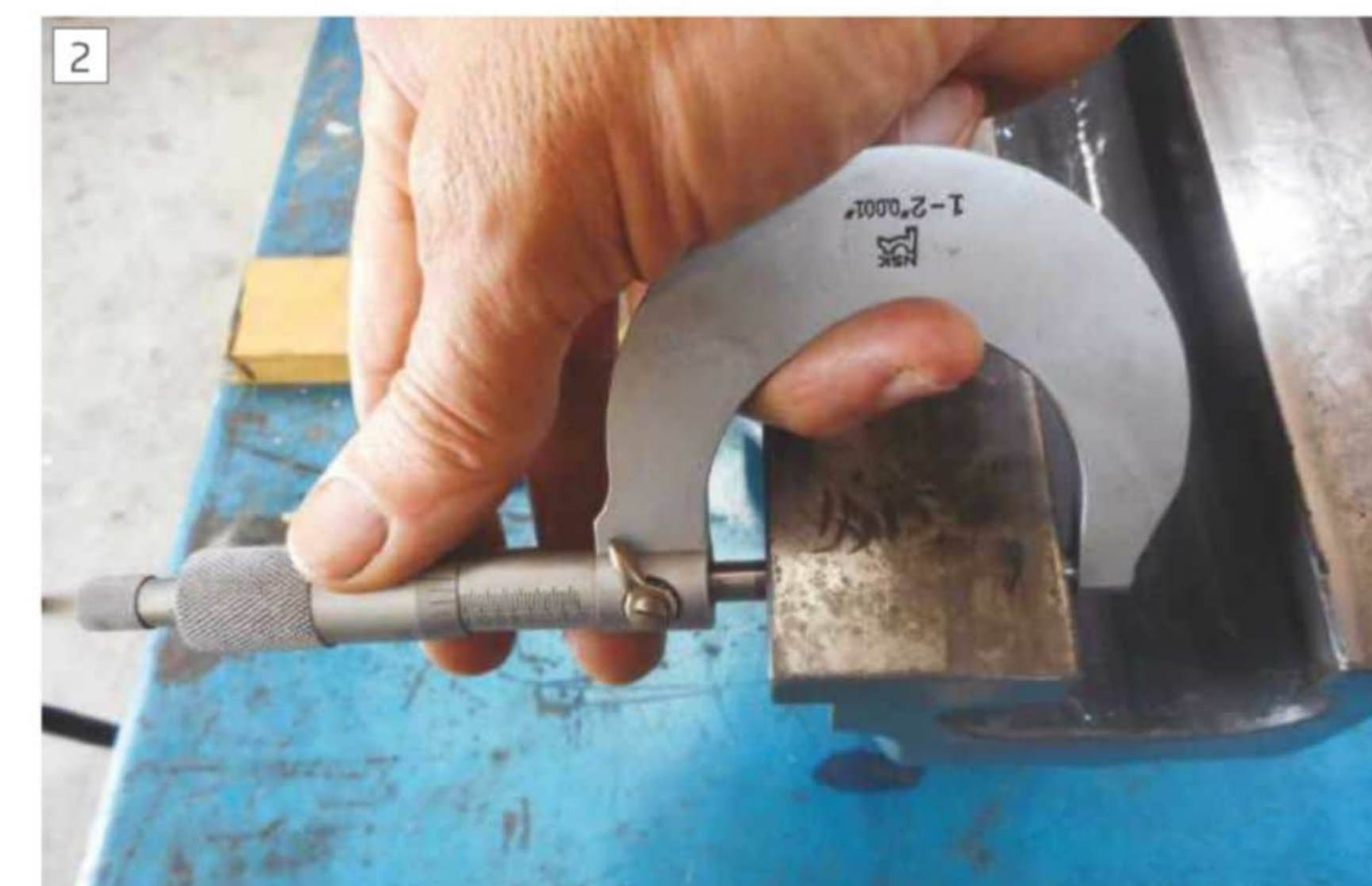
Bed Wear. Measuring the width of the front shear at the unworn right-hand end.
