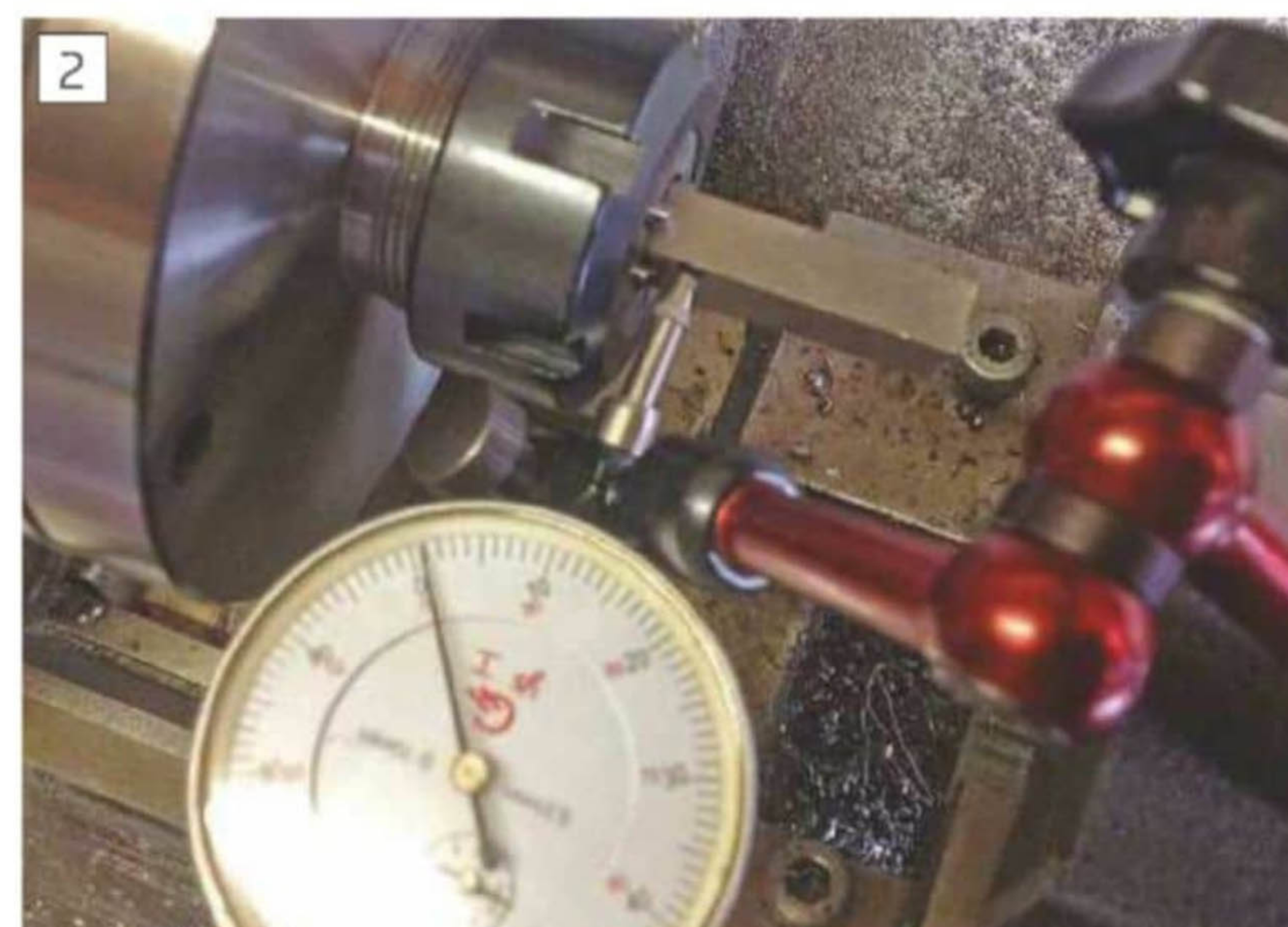
Closer to the collet, gauge reads 0.01mm.
