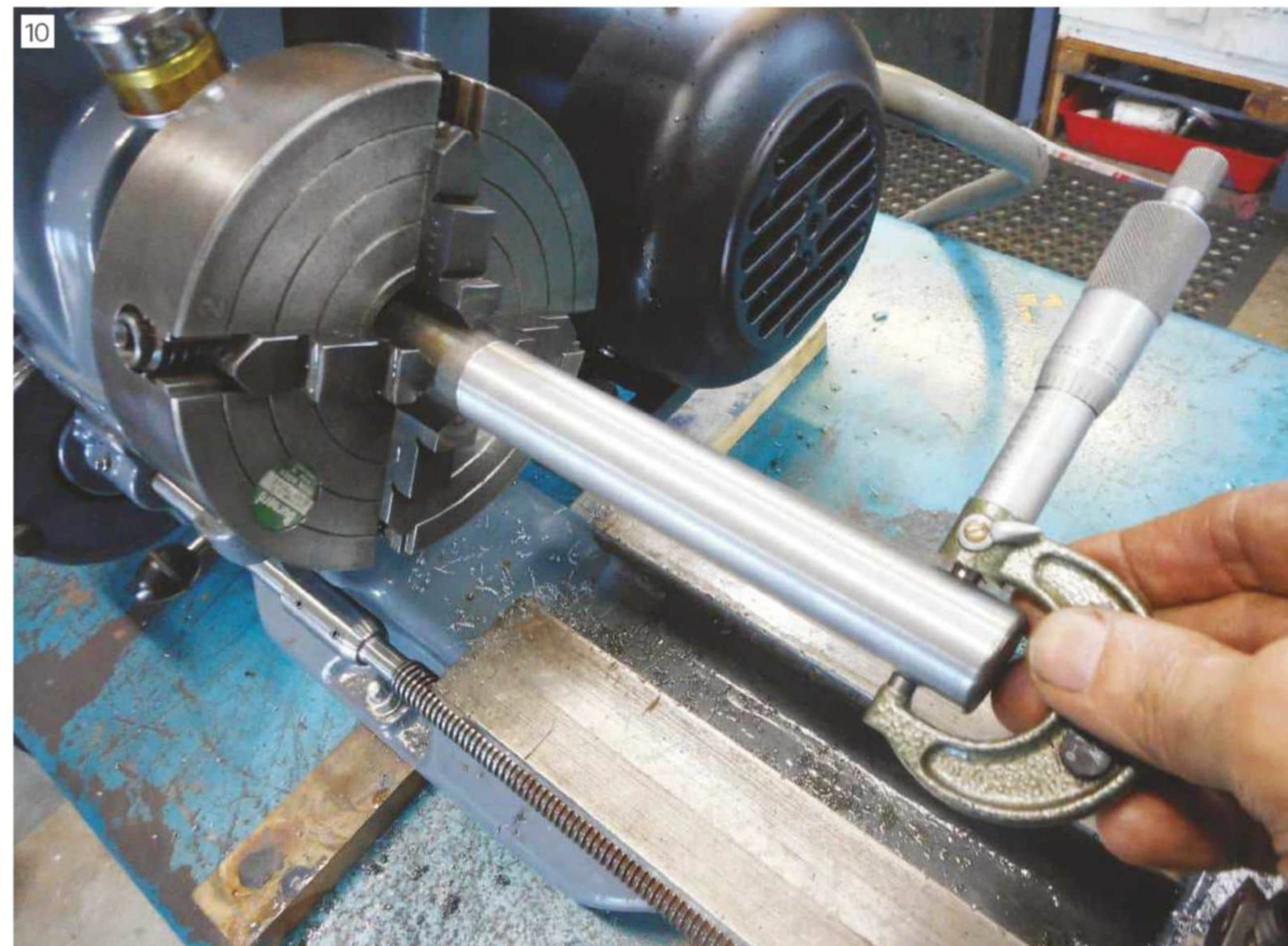
Result! Zero taper measureable over a six-inch test cut without regrinding the bed after a bit of work.
