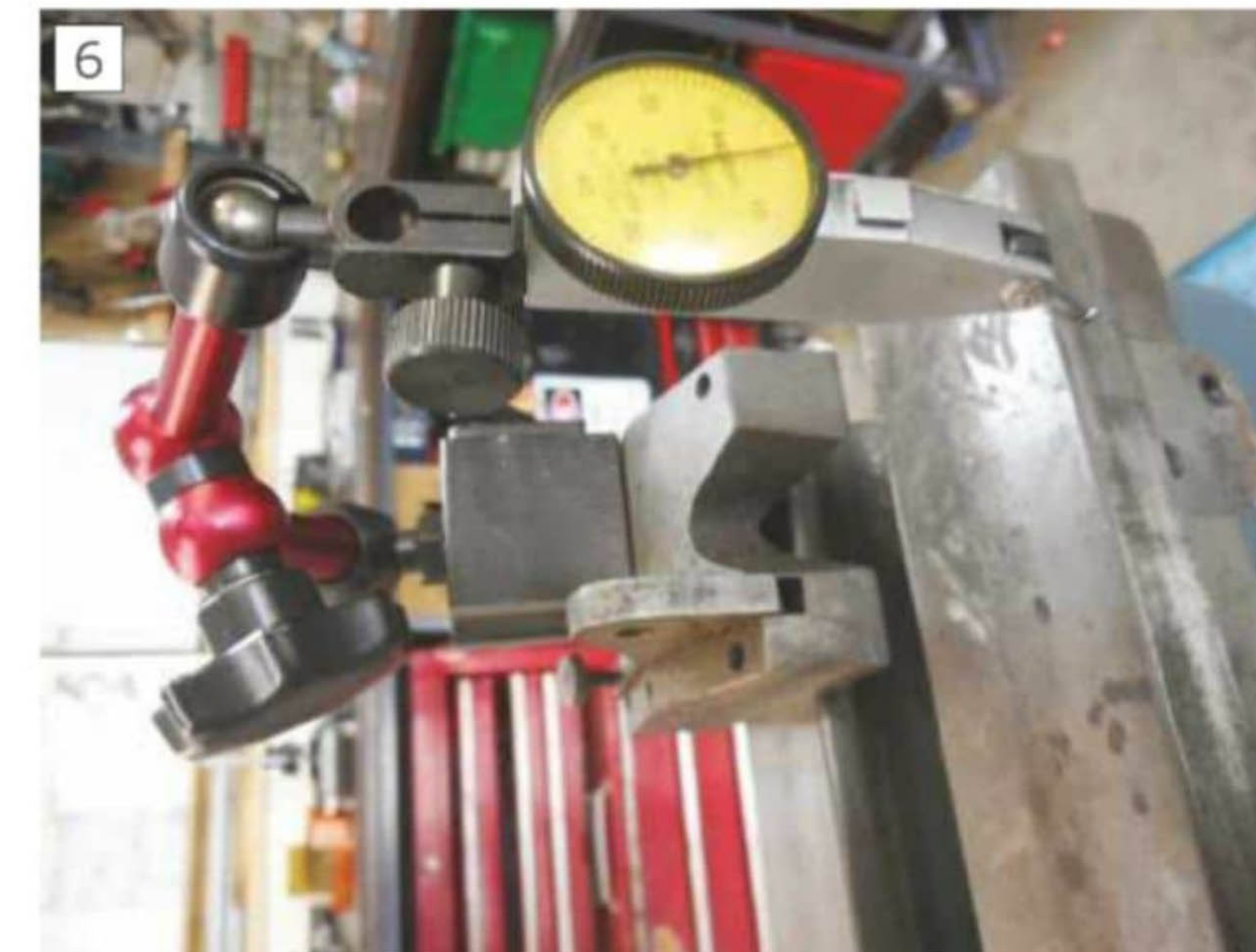
Dial indicator mounted on sled to compare the distance between the two outside vertical shear surfaces.
