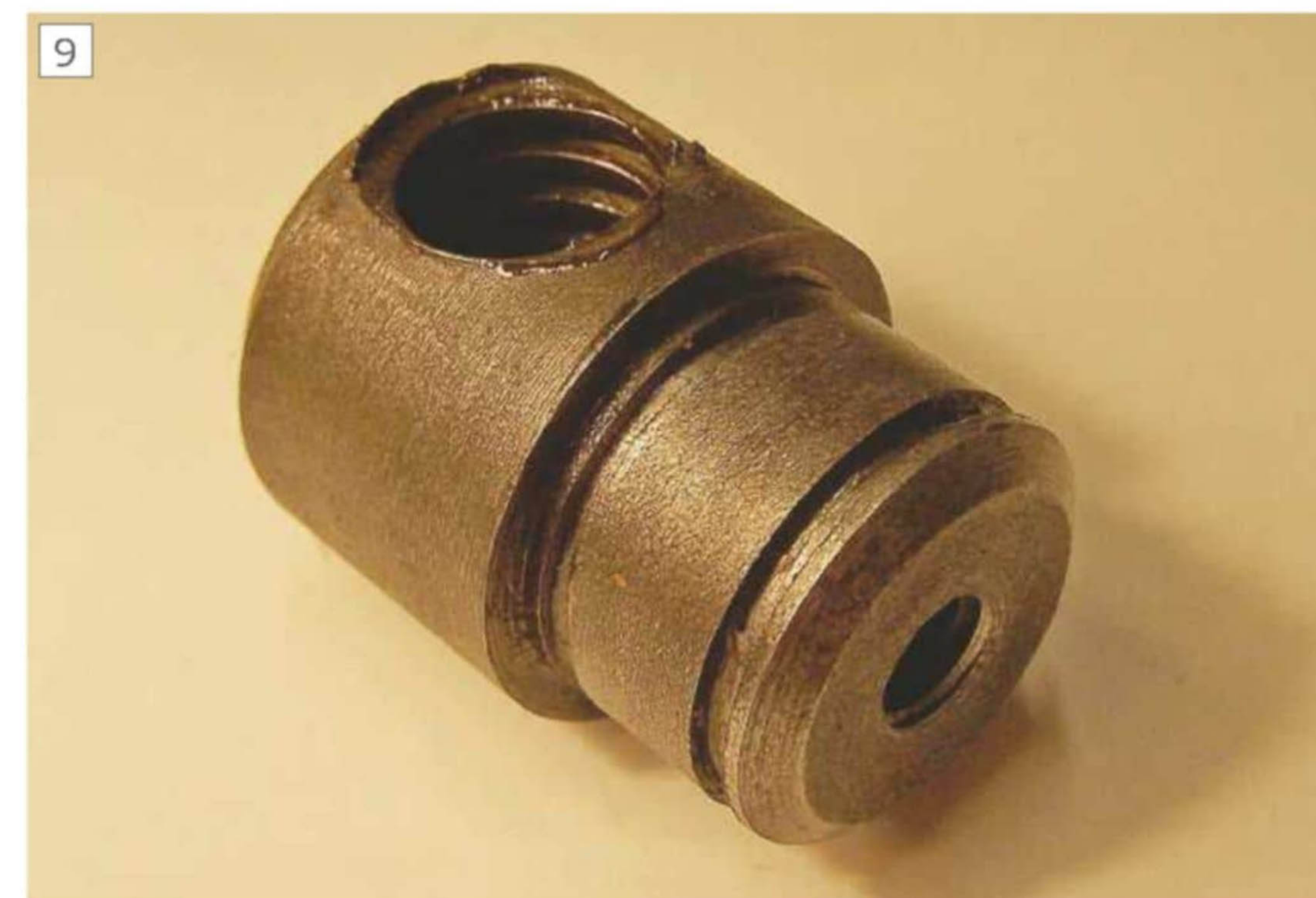
The two o-ring grooves machined into the spigot
