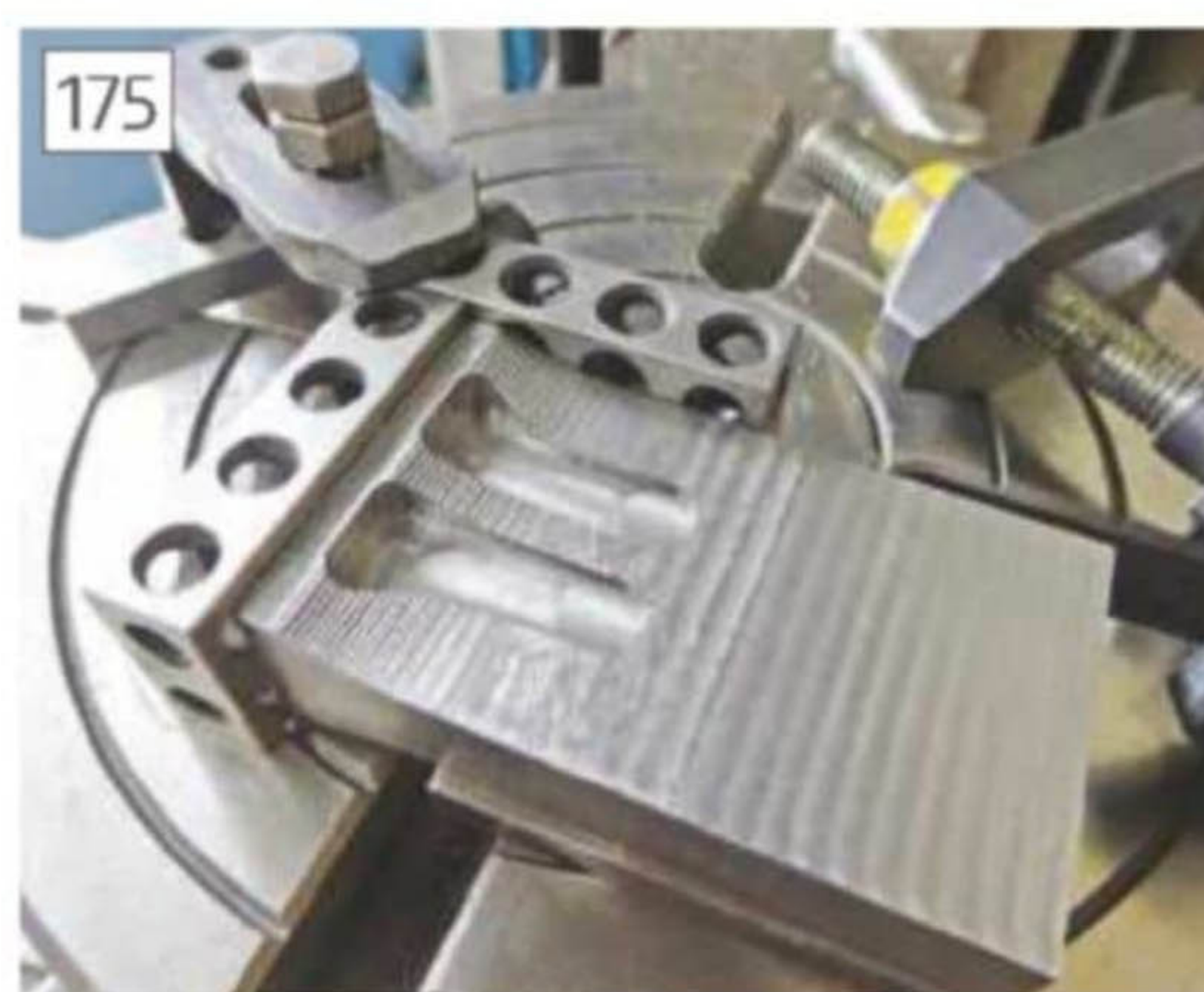
10-20-40 blocks used for repeat setups
