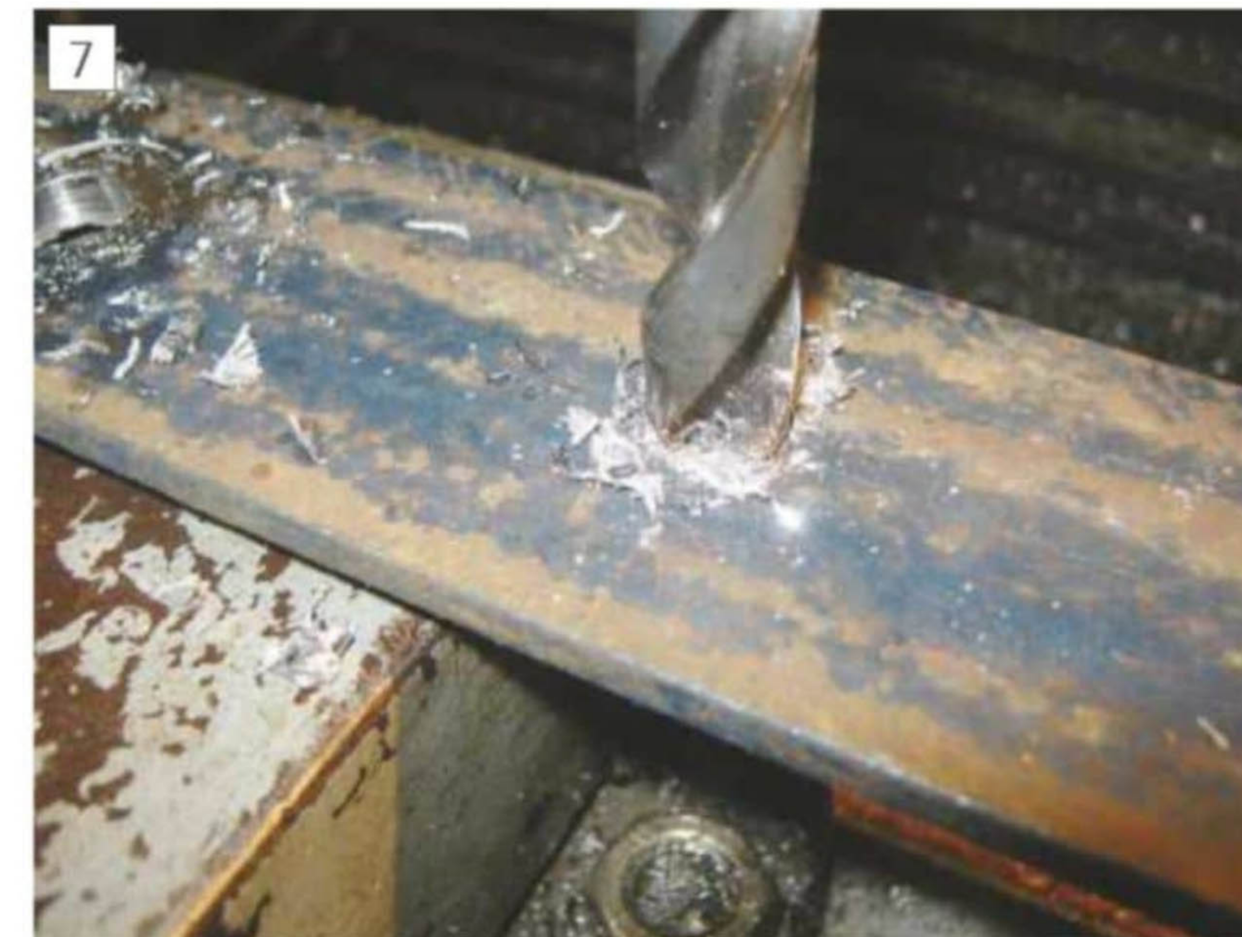
Drilling the side rails
