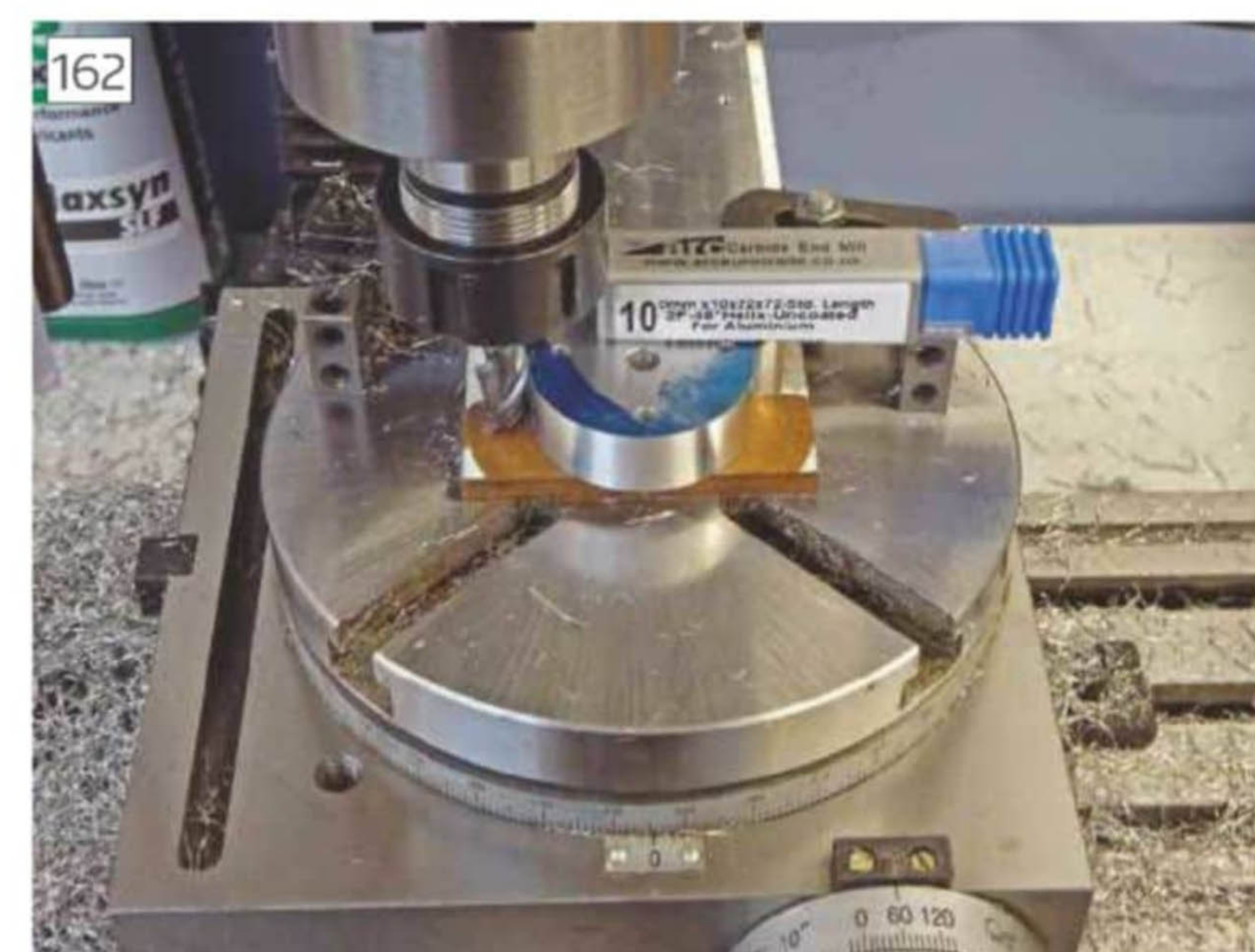
Simple rounding over of an aluminium base plate
