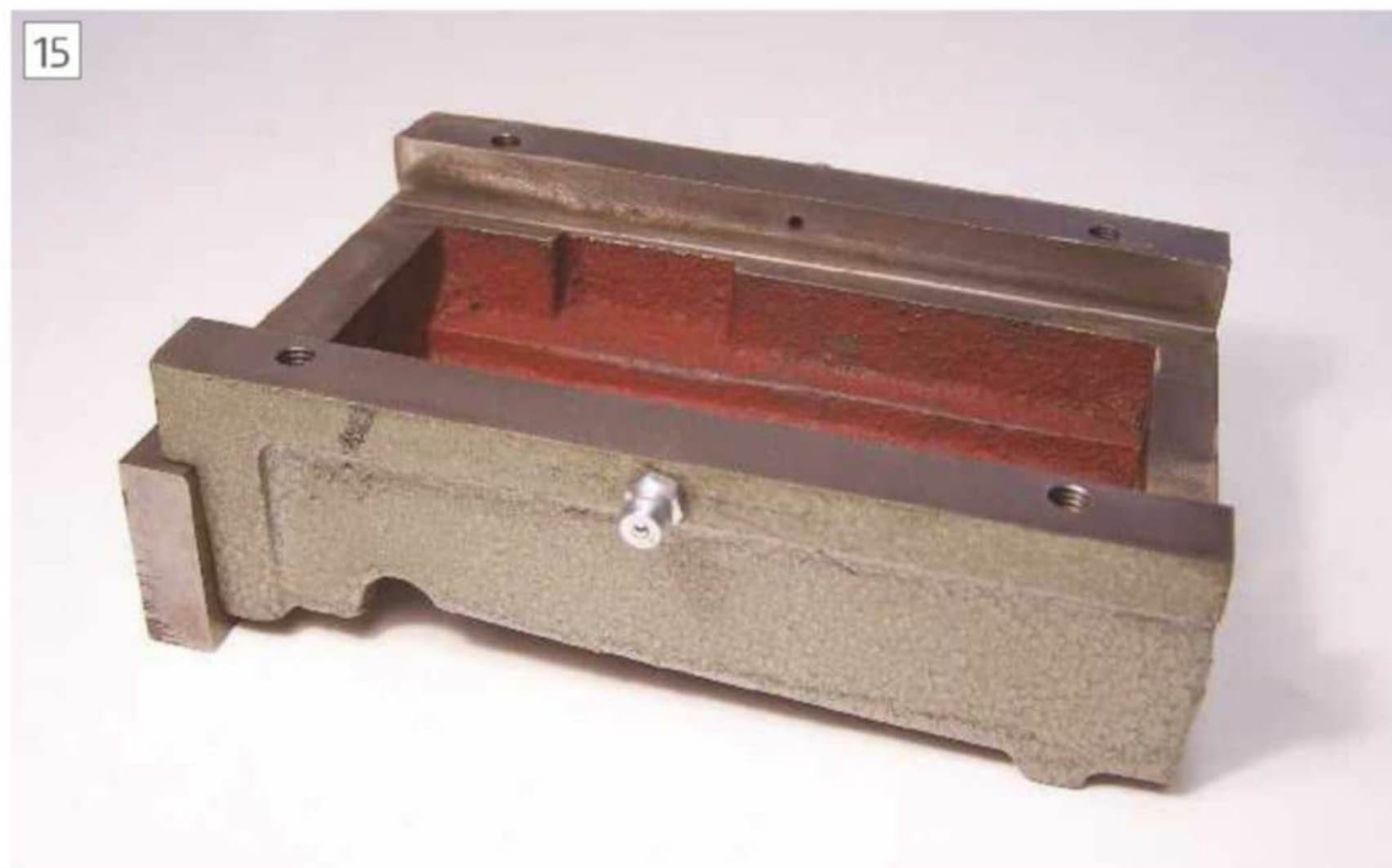
The slideway lubrication points on the moving jaw
