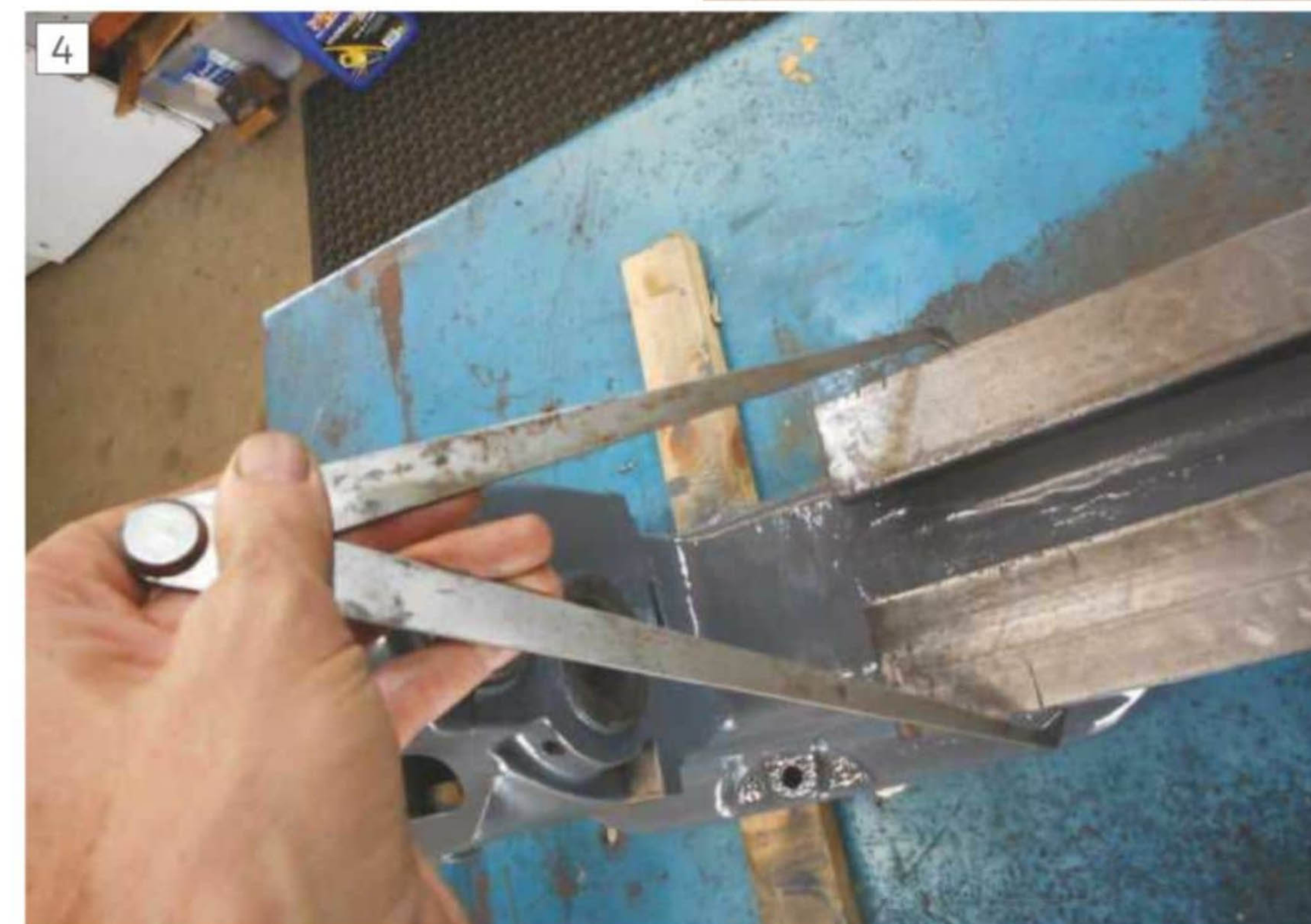
Unworn rear vertical surface provides a reference for measurement on narrow guide models.
