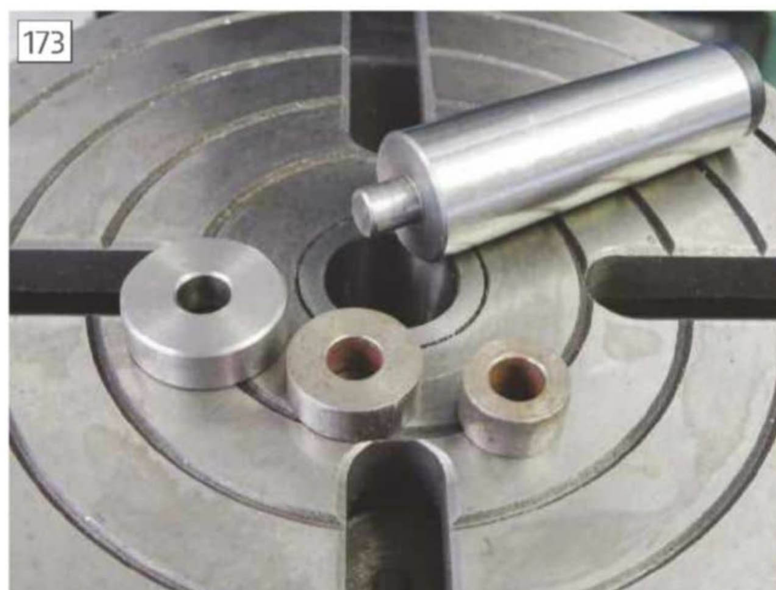
Morse taper location pin and bushes
