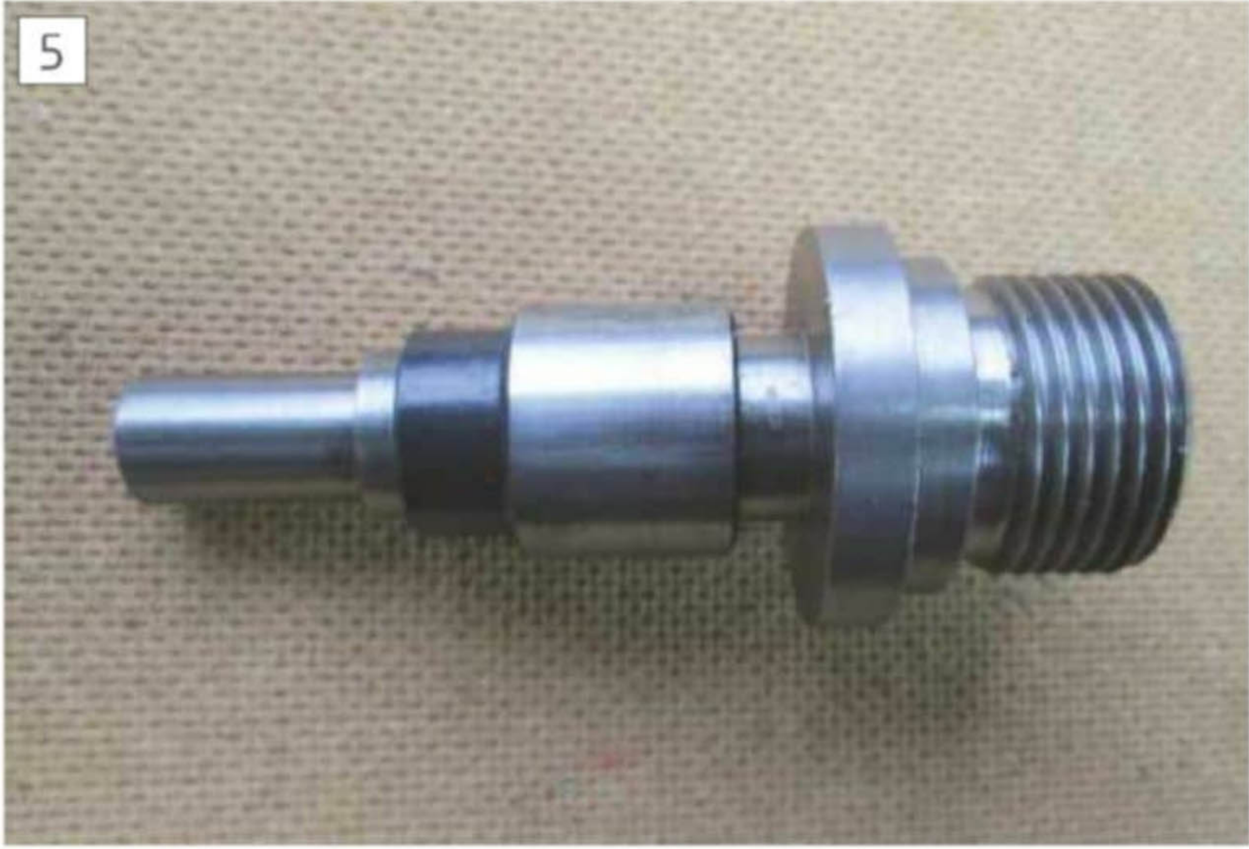
The small land between the bush and the threaded head of the chuck
