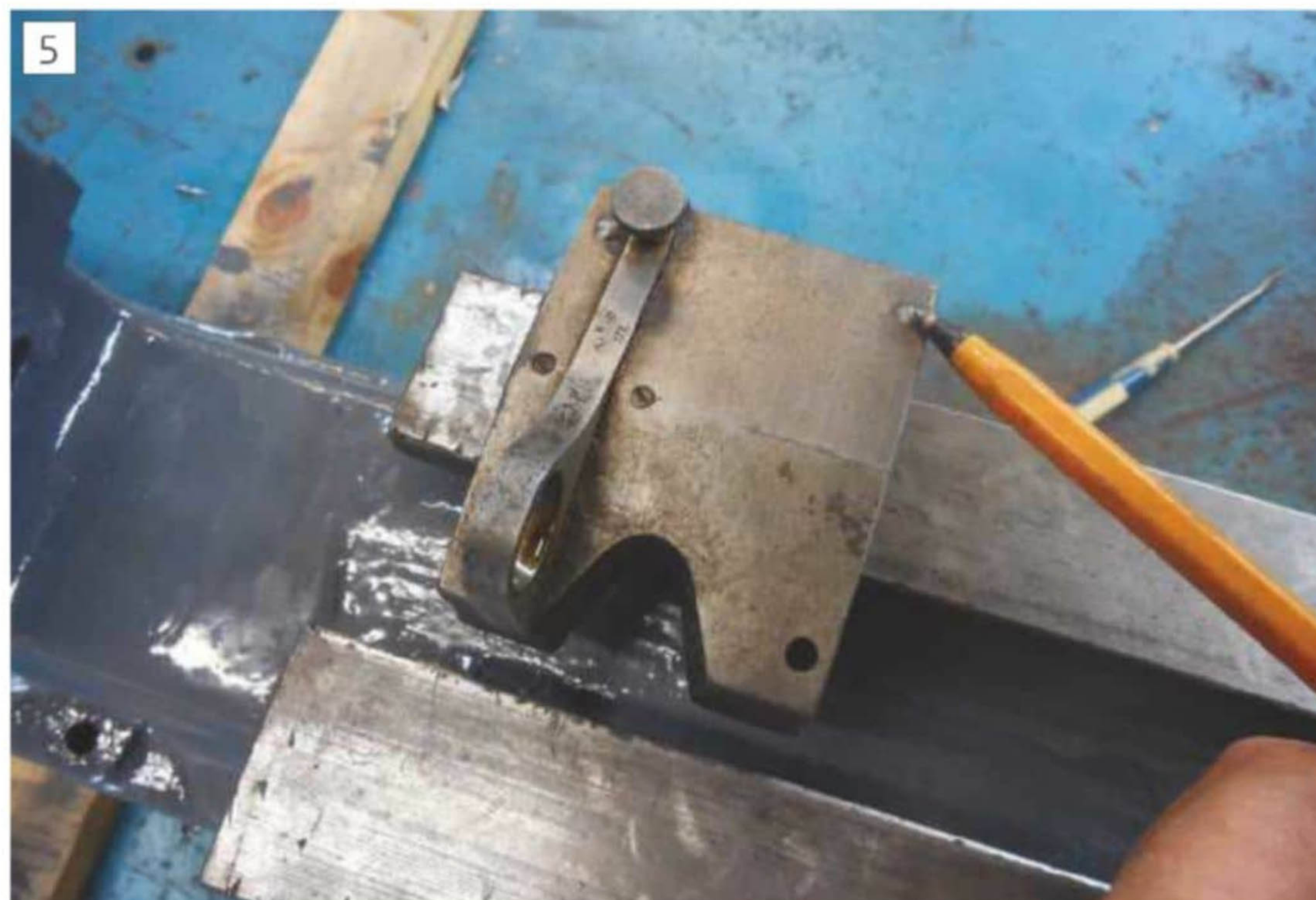
Pins on the marking gauge base follow the rear vertical surface.
