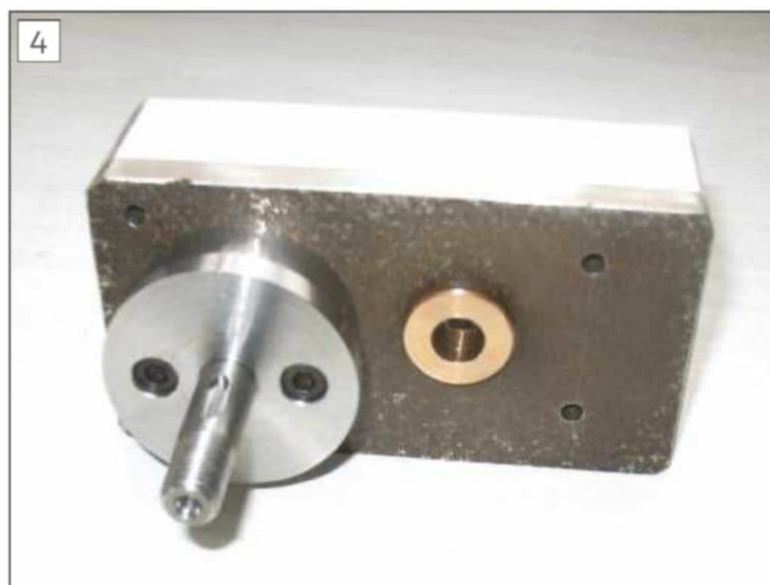
Gearbox assembled, note bush for feedscrew.
