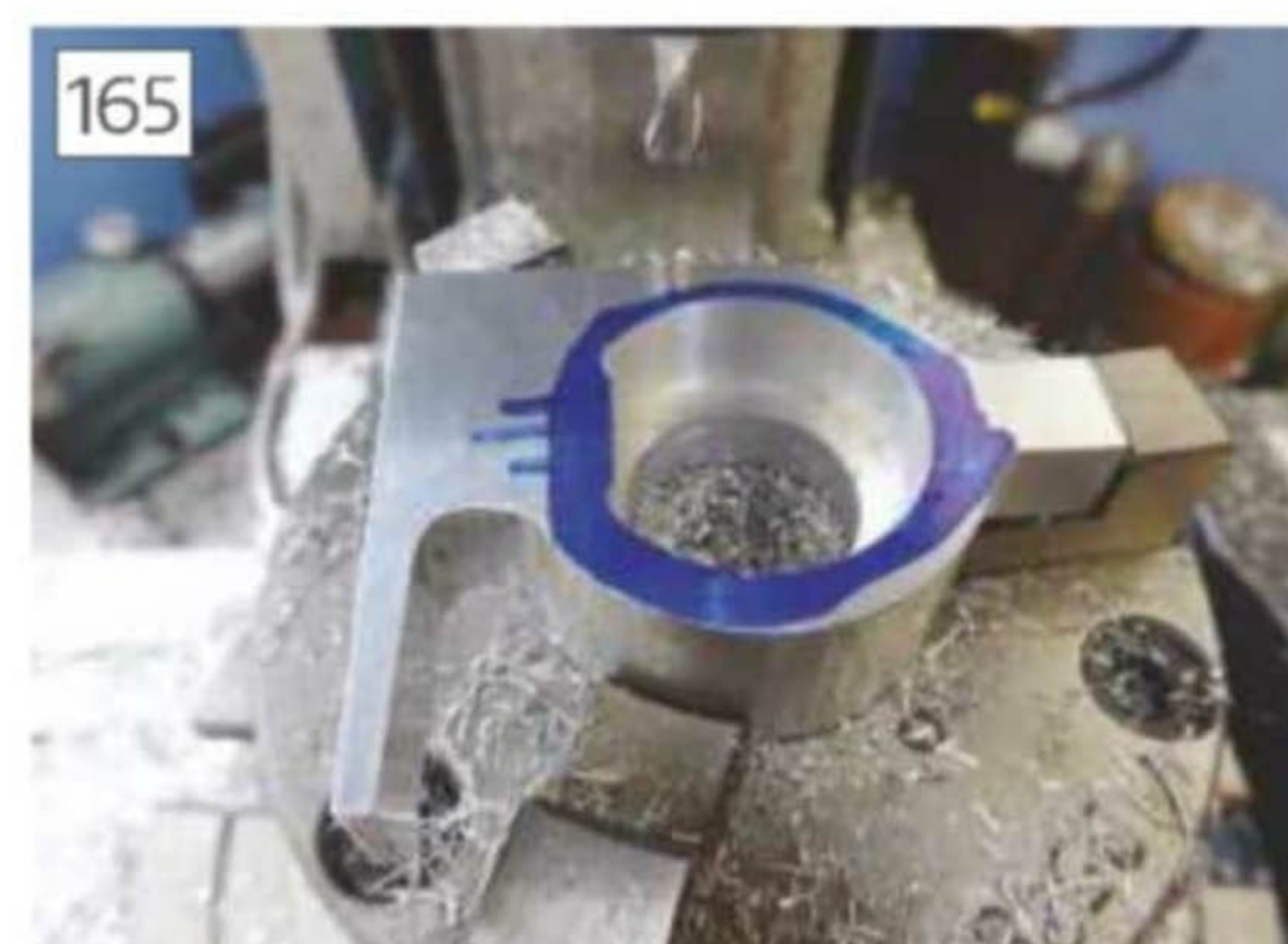
Straight and curved cuts all done at one setting
