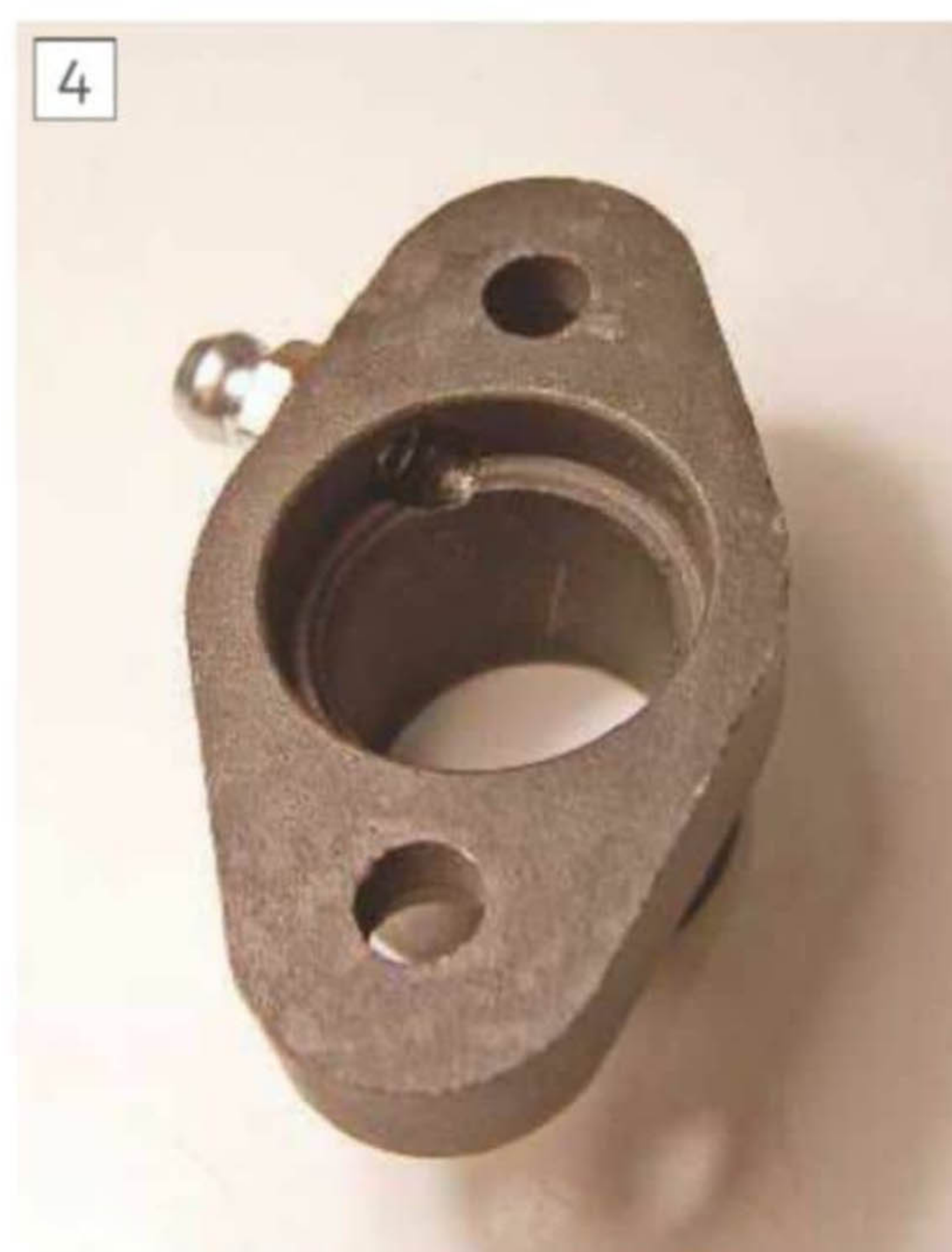
The grease nipple fitted to the screw retainer
