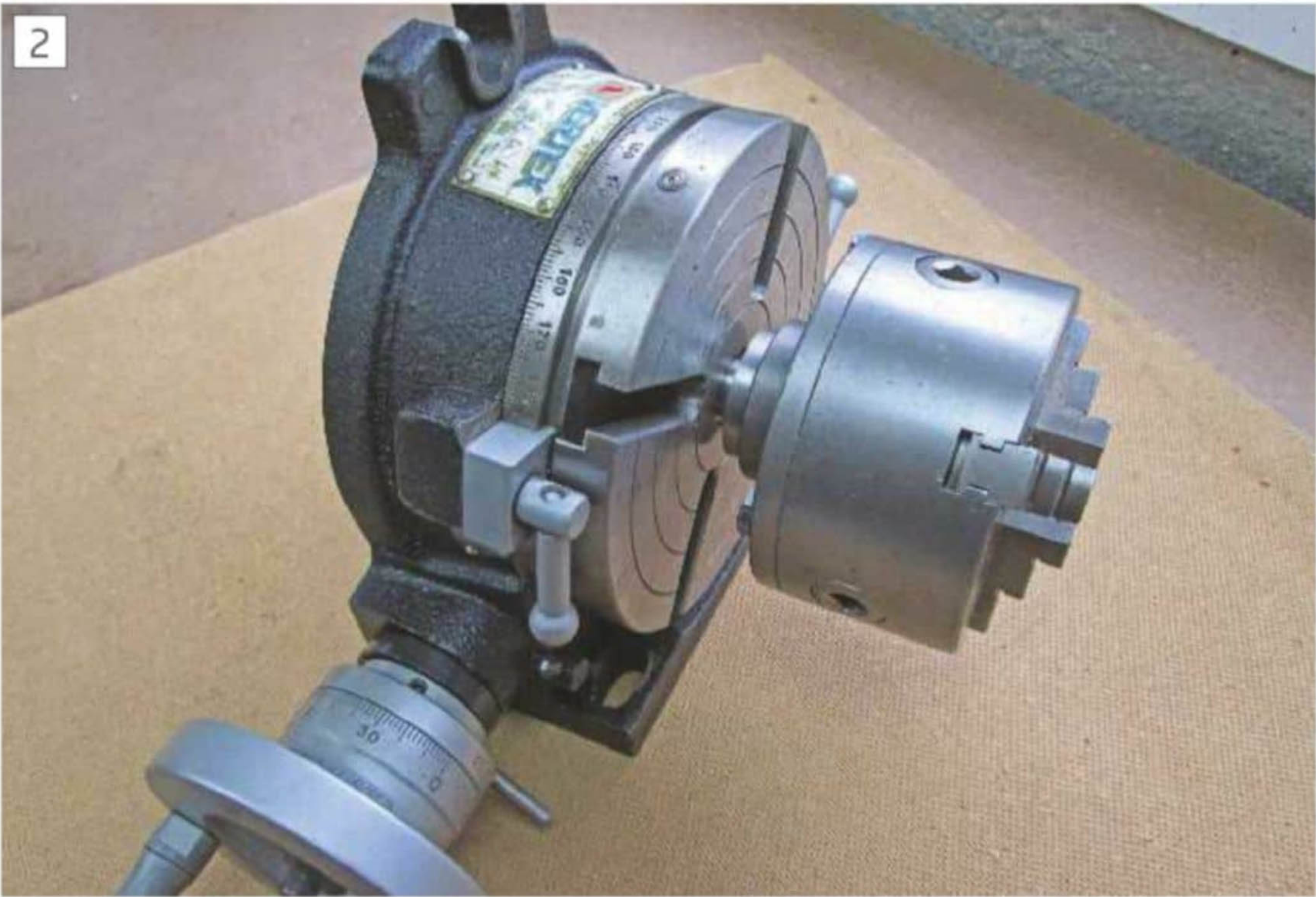
Chuck mounted on mandrel
