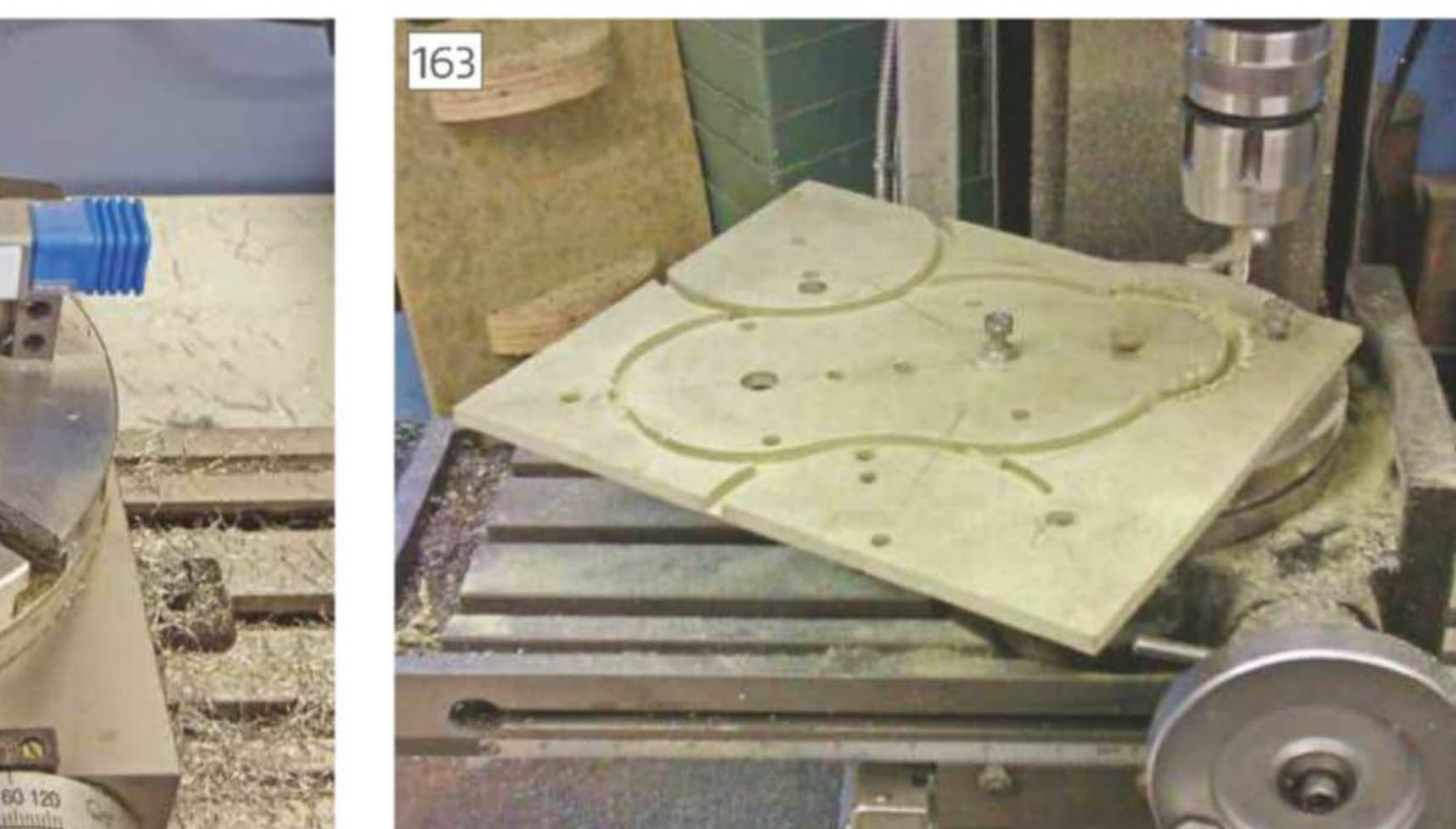
Multiple curves being cut to form a MDF template
