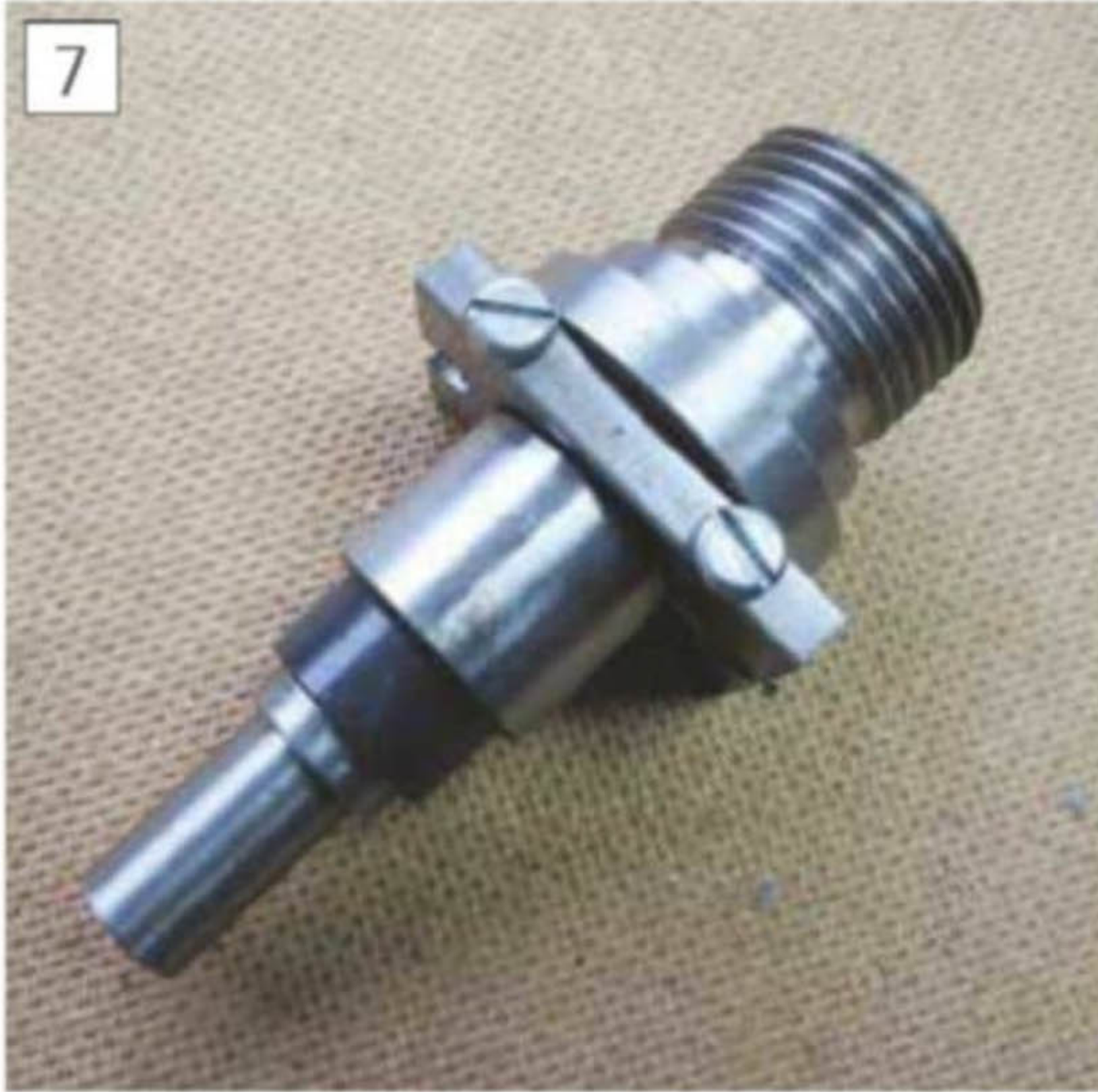
Separator assembled around the mandrel
