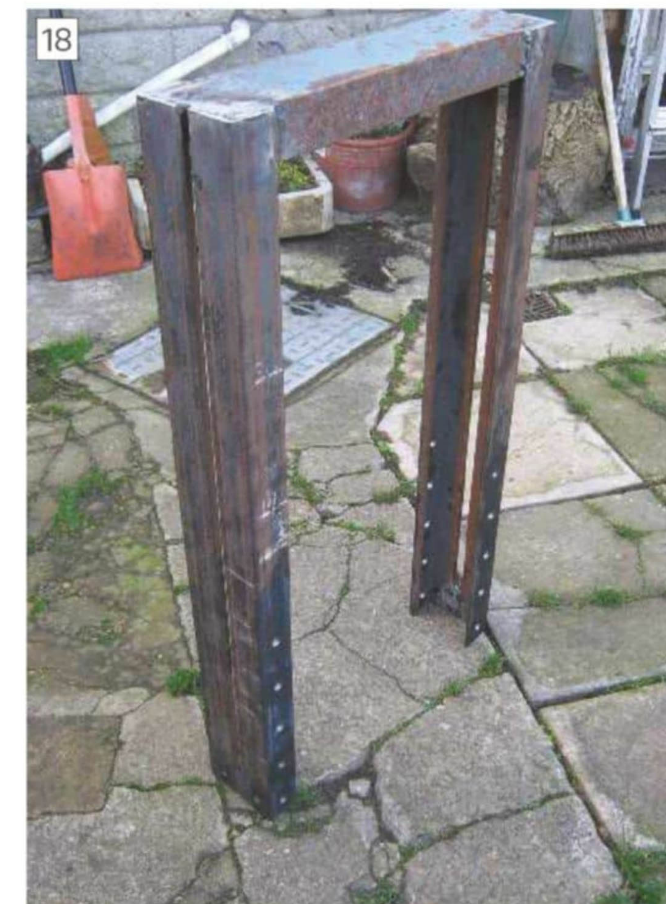
The welded frame
