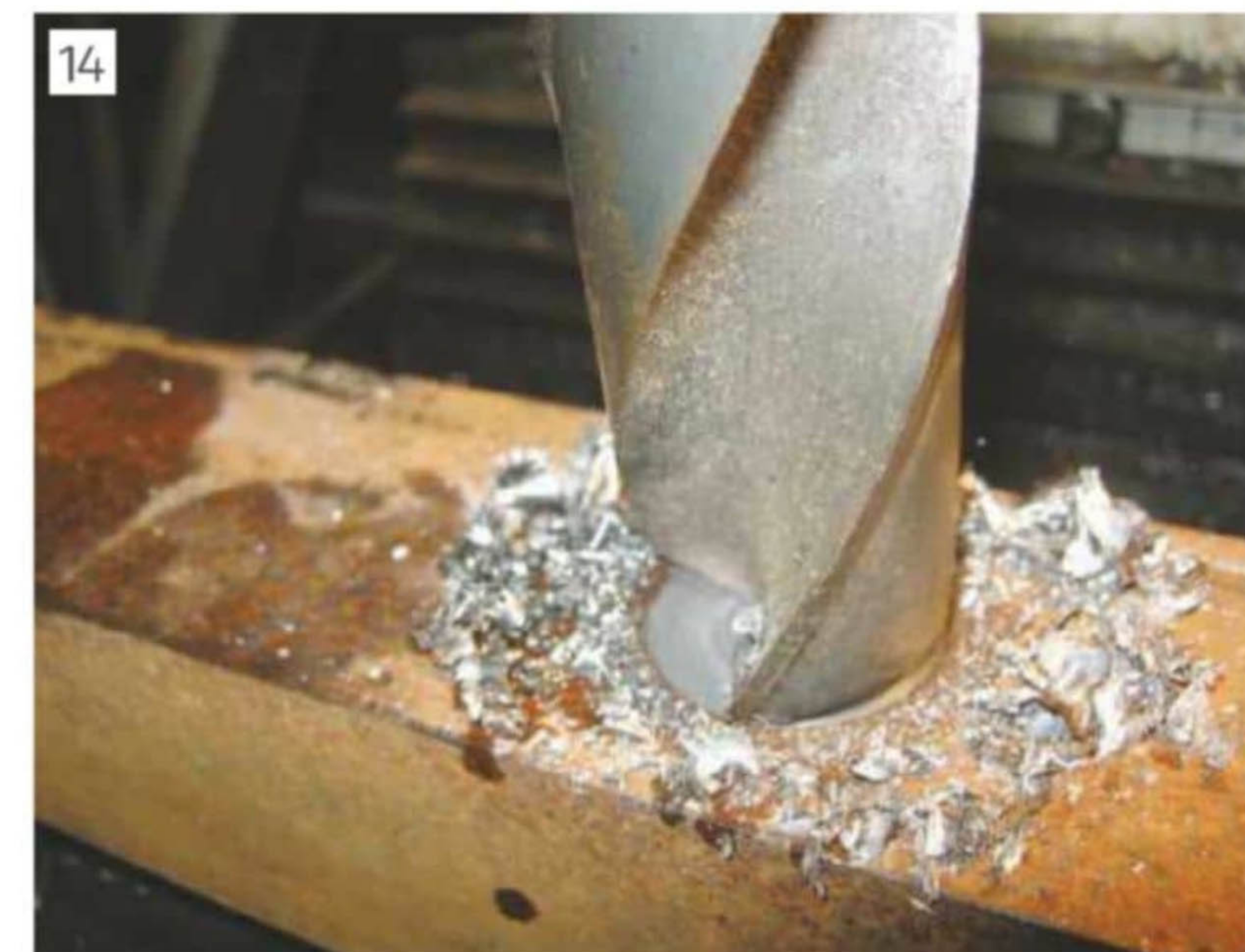
Start of drilling with 33mm drill
