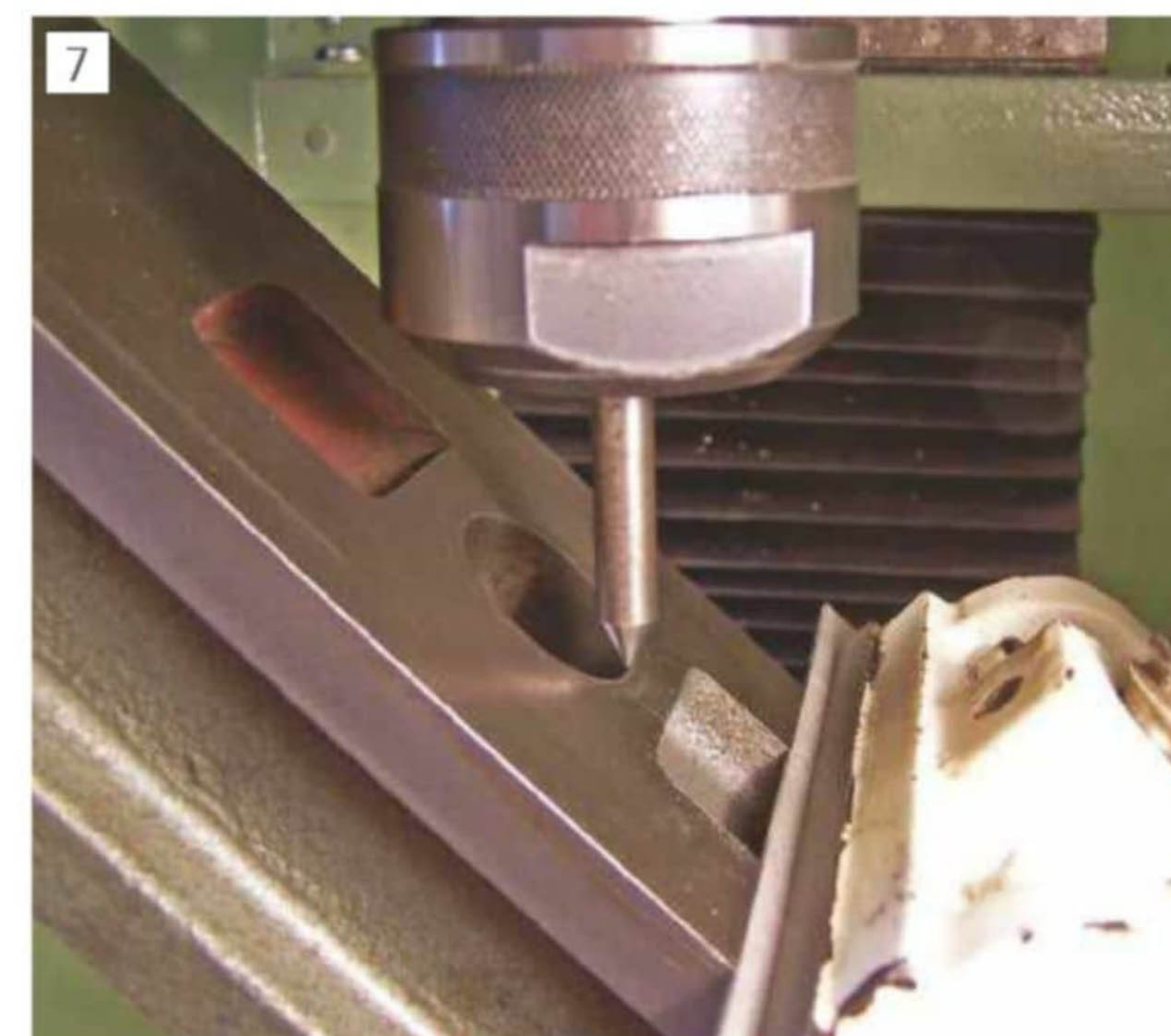
Setting the milling chuck centre line to the edge of the hole
