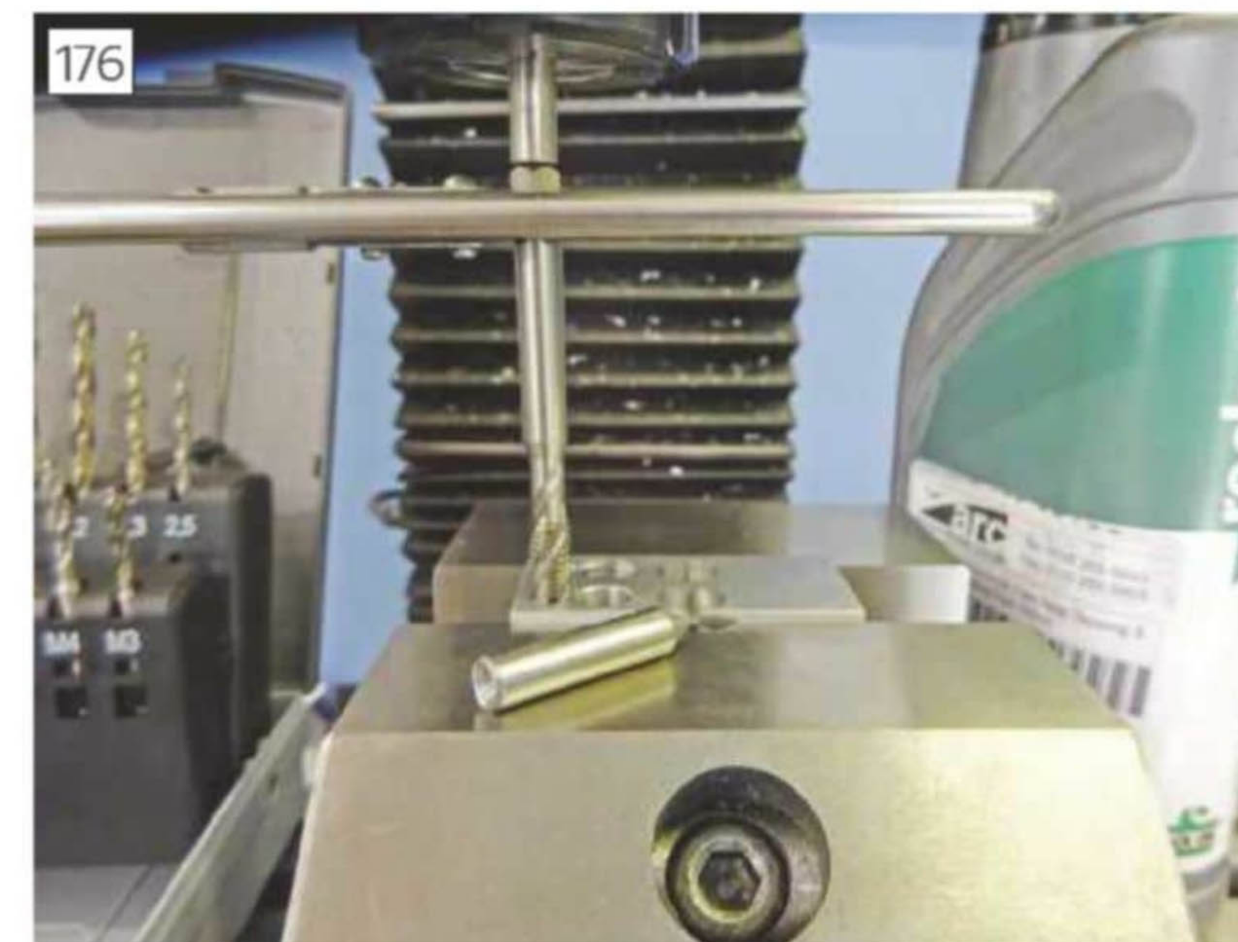
Simple homemade tap guides
