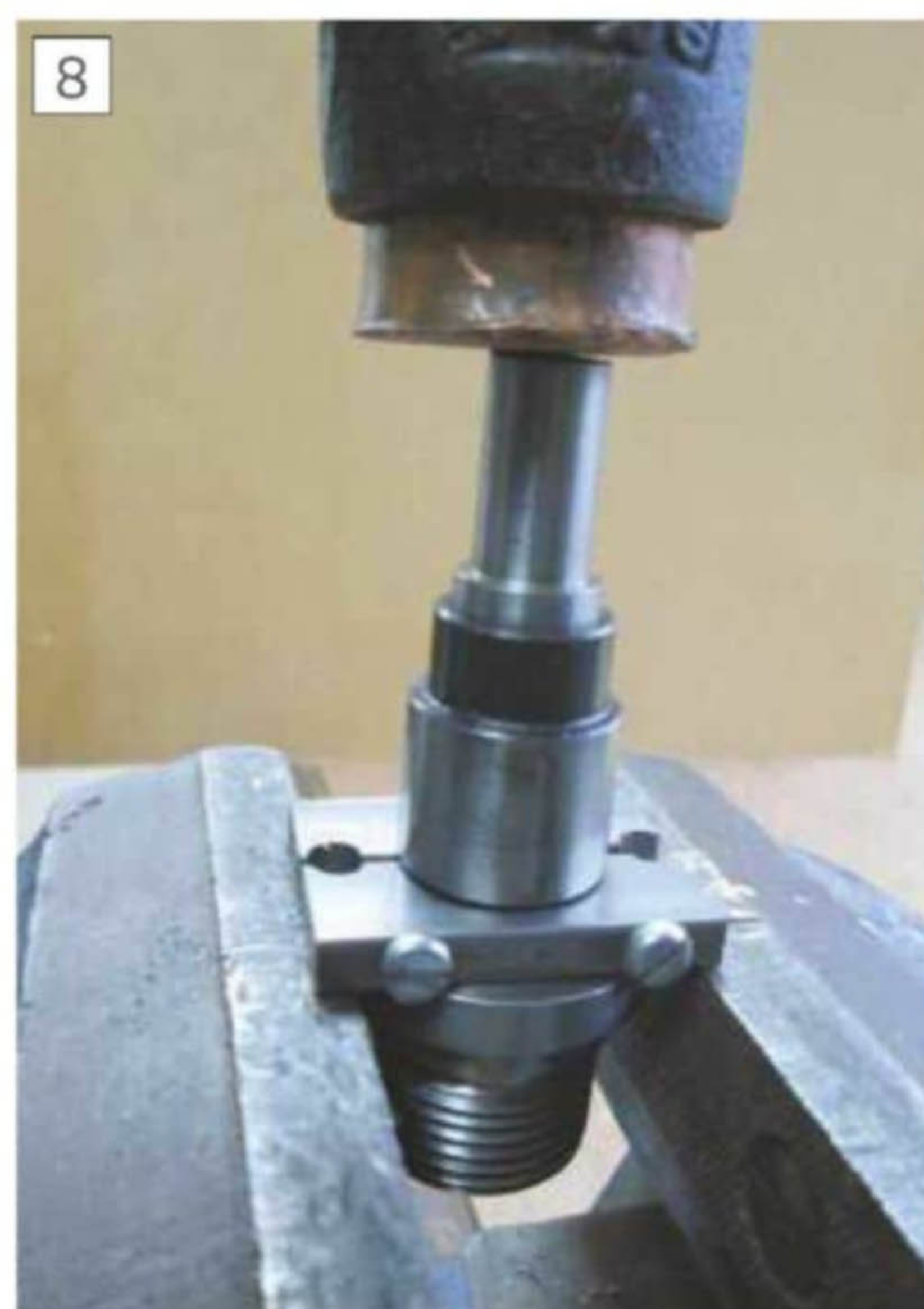
8 Mandrel/separator mounted on vice ready to be separated
