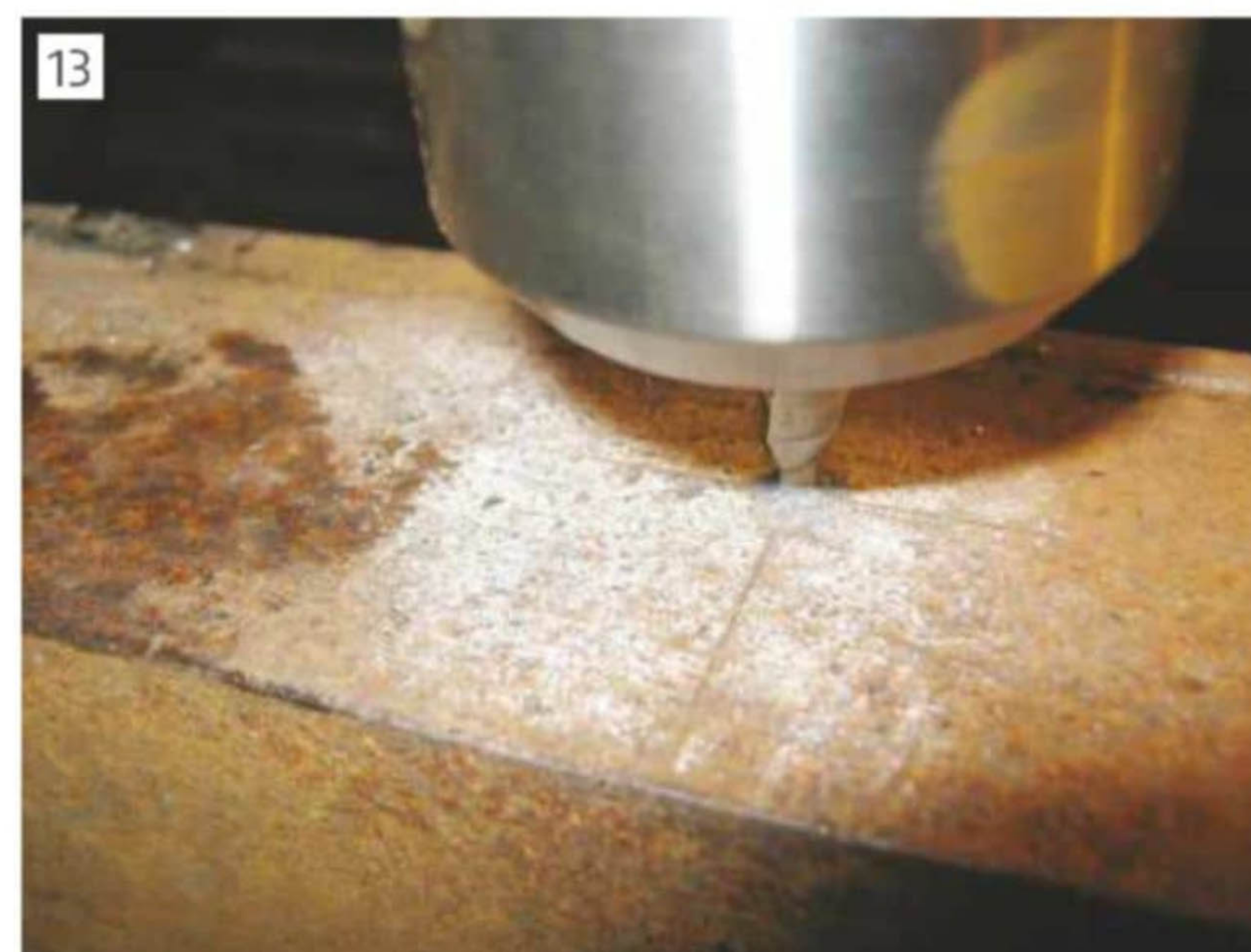
Centre drilling the ram support
