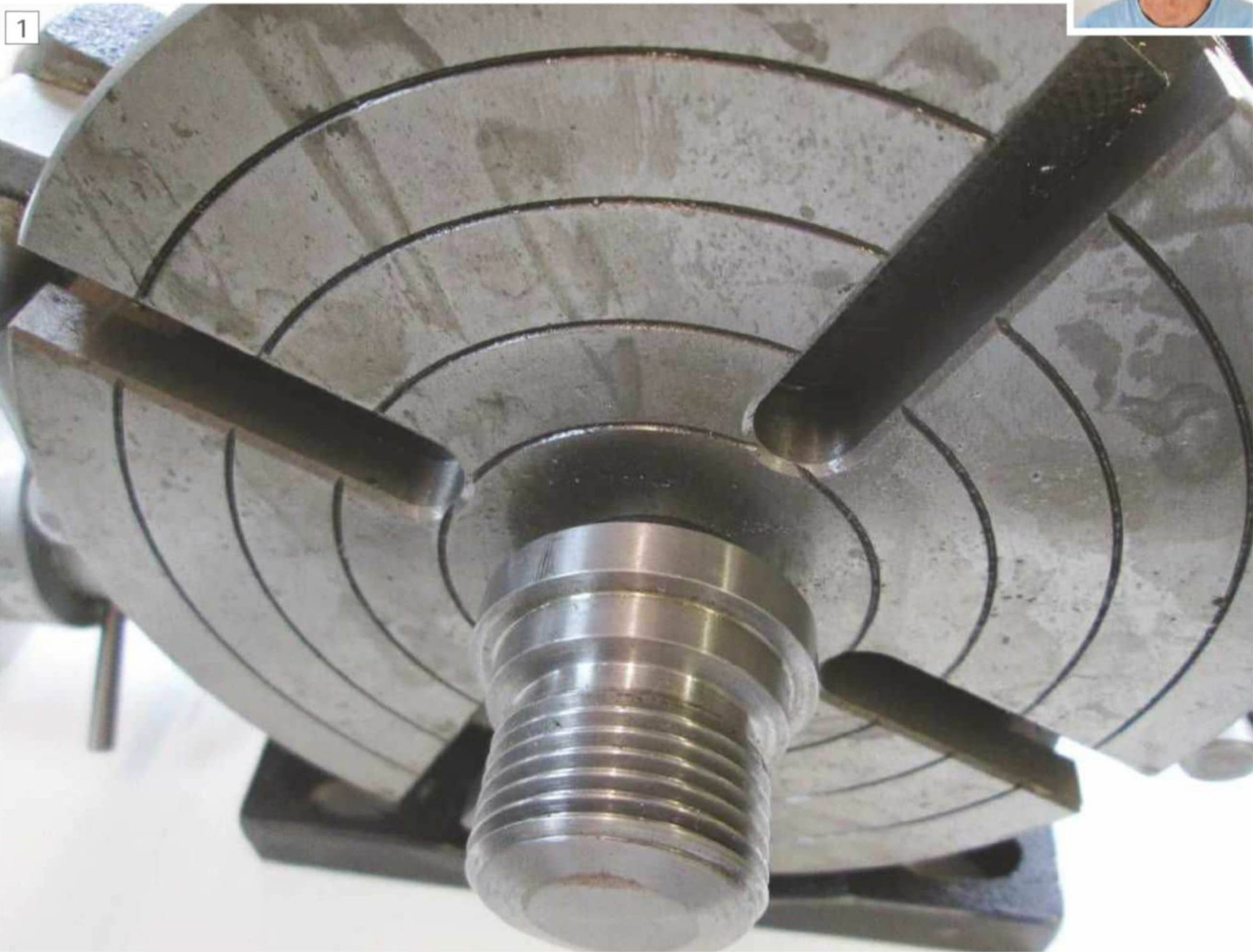
Morse taper mandrel inserted in rotary table
