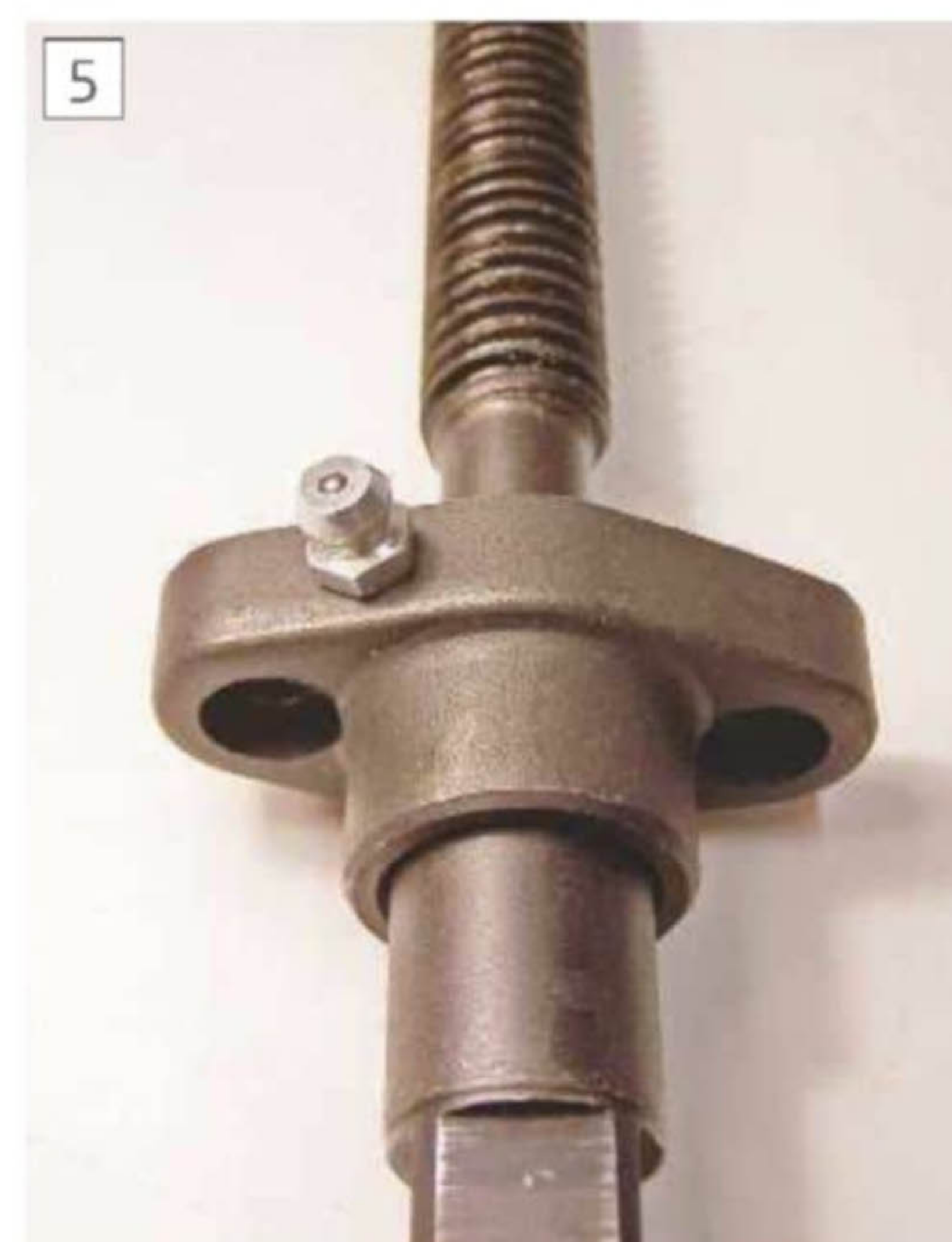
The screw retainer assembled onto the screw
