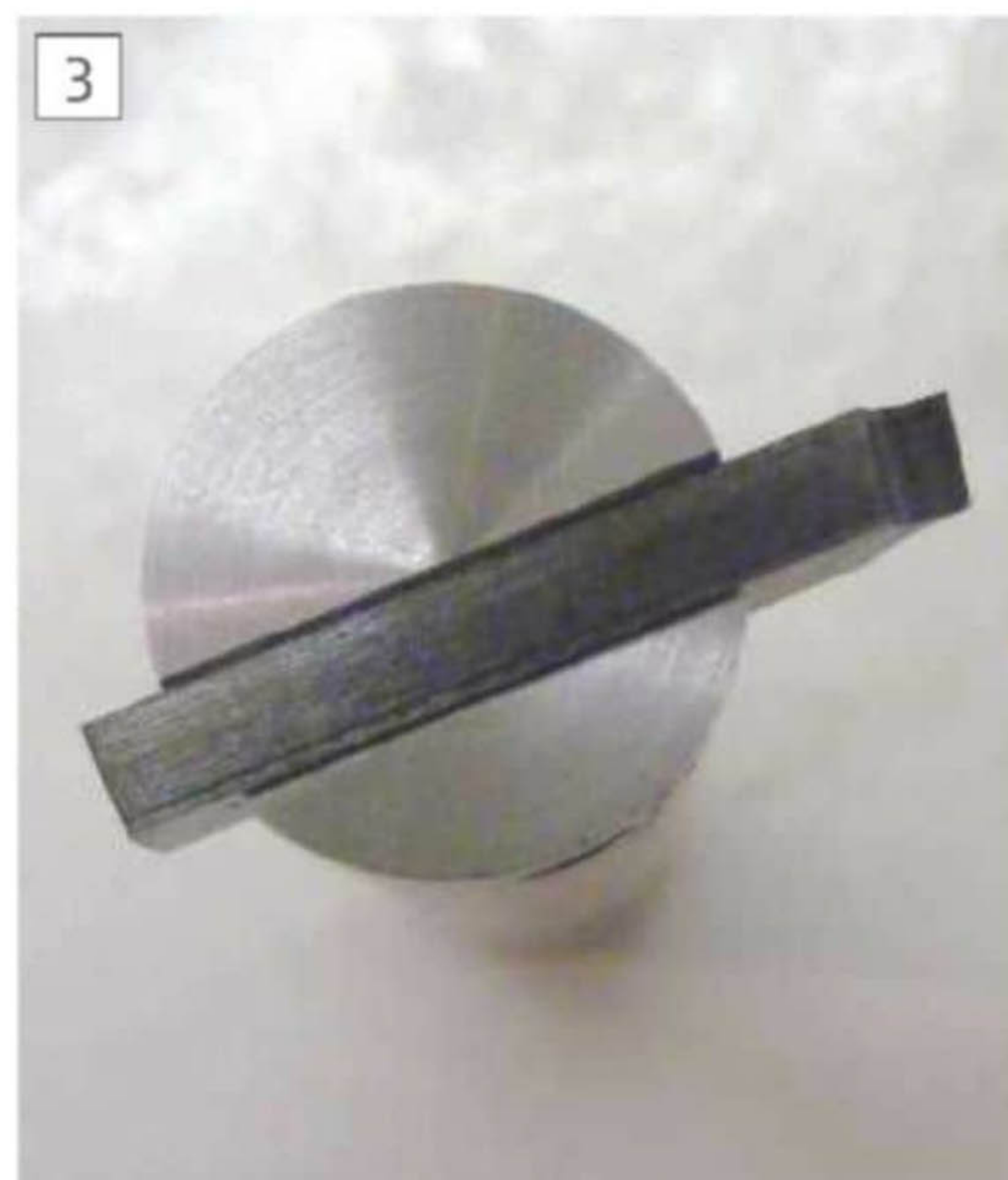
Cutter mounted on diameter of 16 mm arbor.
