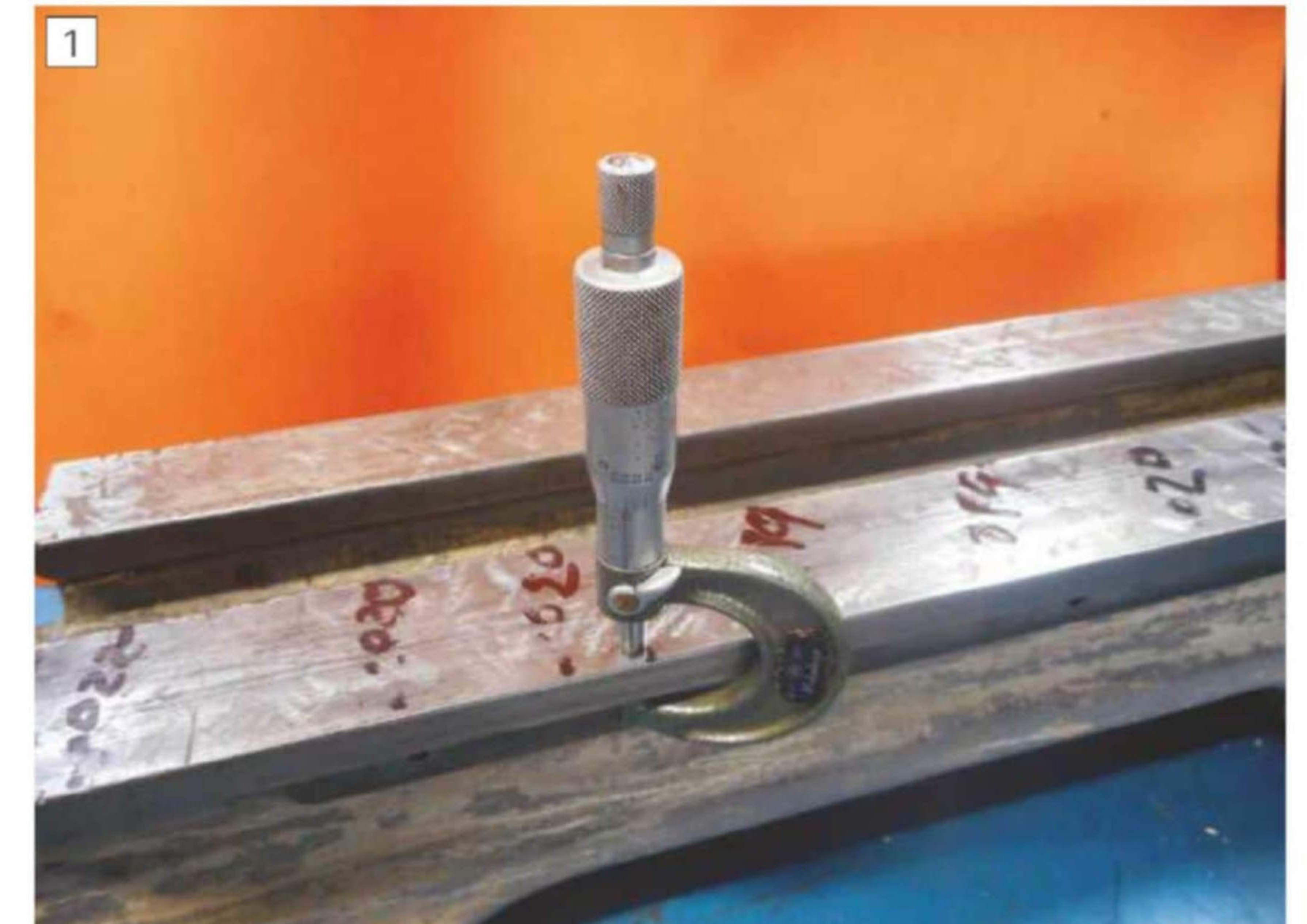
Measuring front shear thickness.
