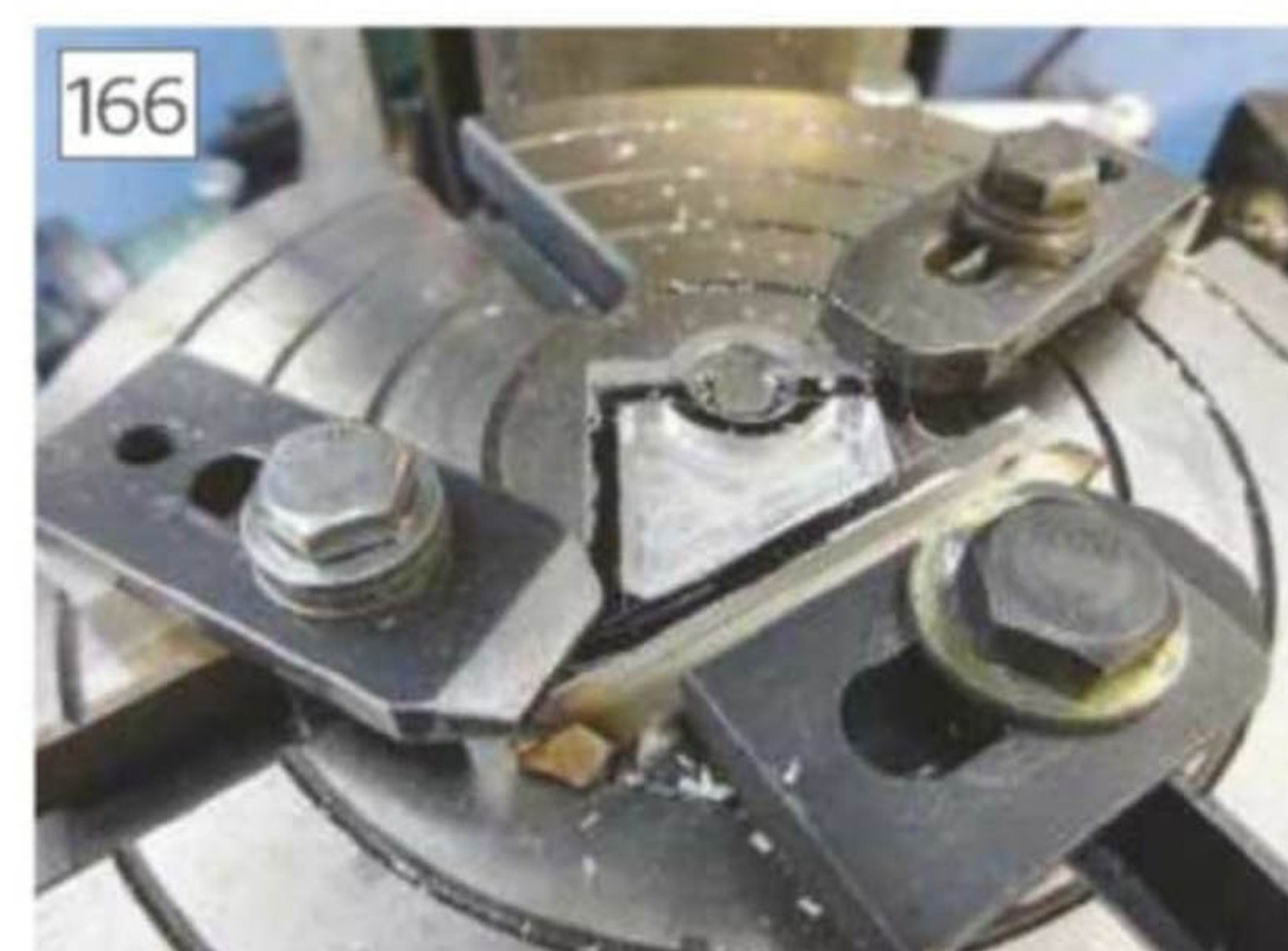
Straight and angled cuts on the same part
