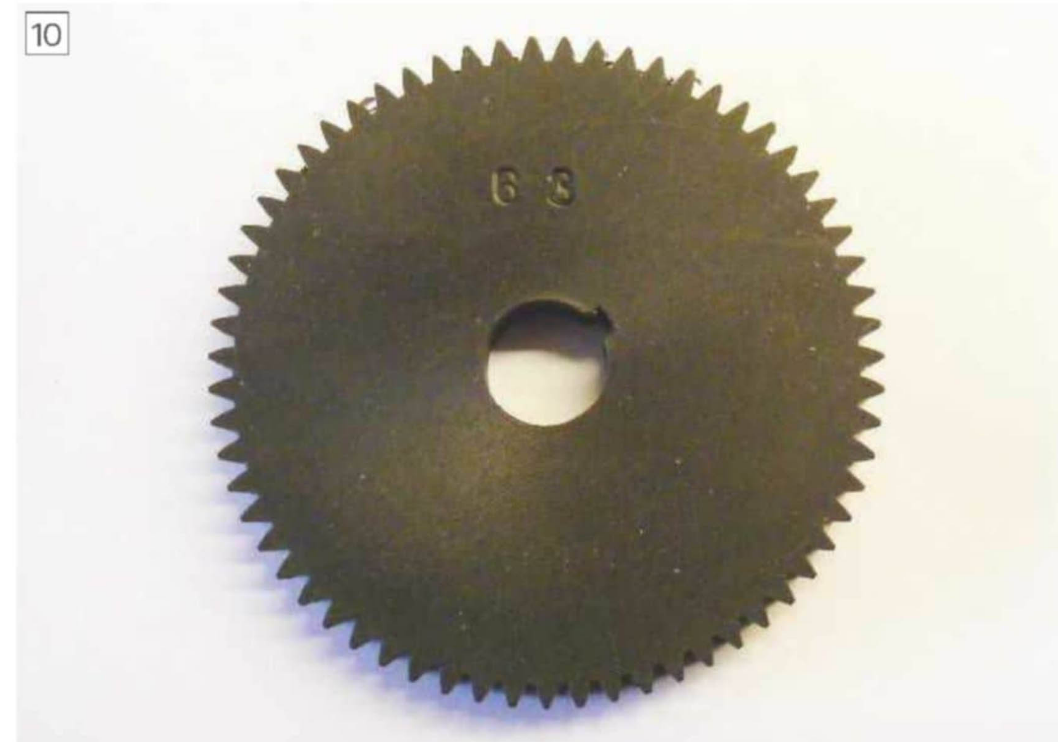
A 63 tooth gear in Delrin.
