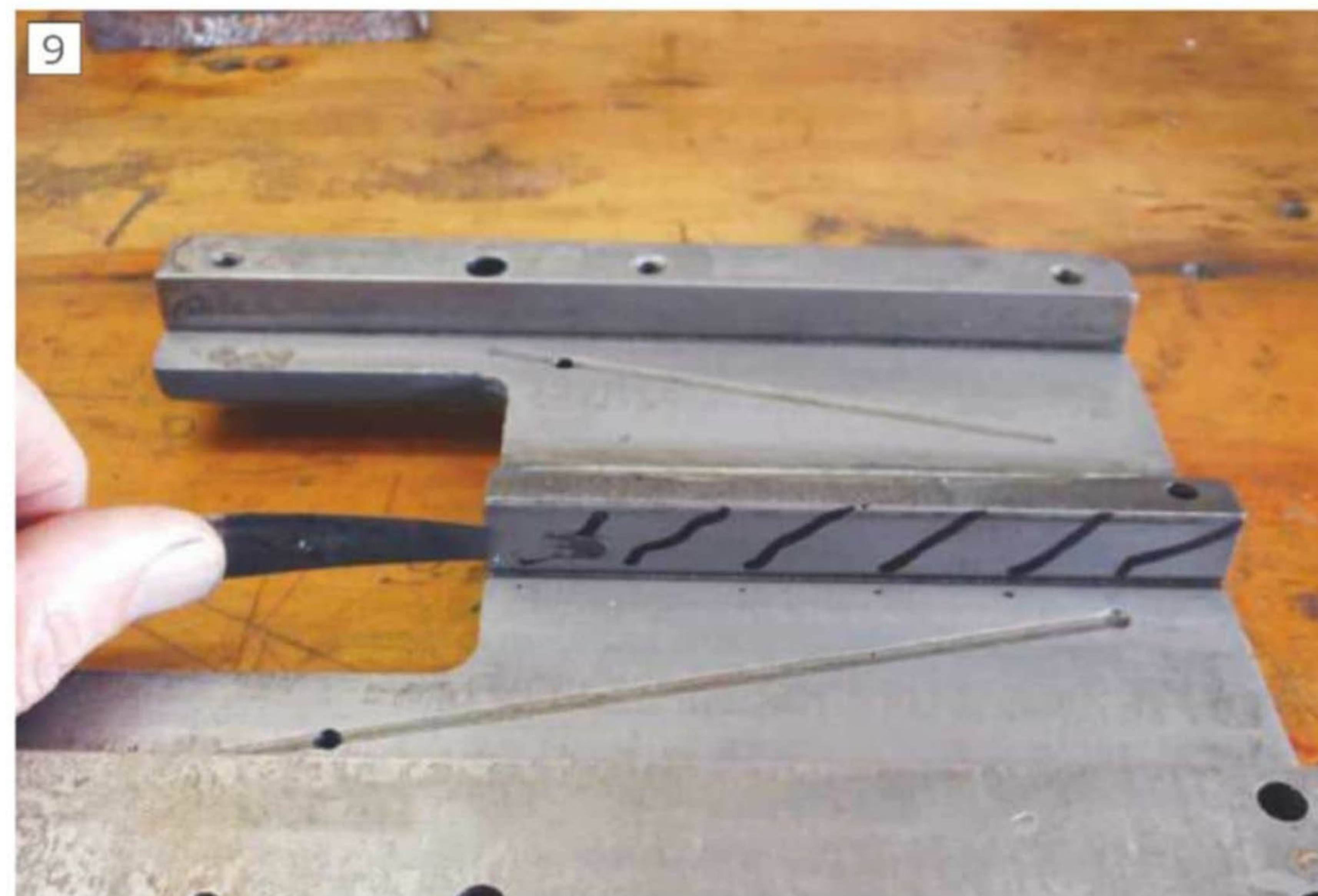
Most saddle wear was found on the marked vertical surface and measured with a feeler gauge against the unworn strip at the top.
