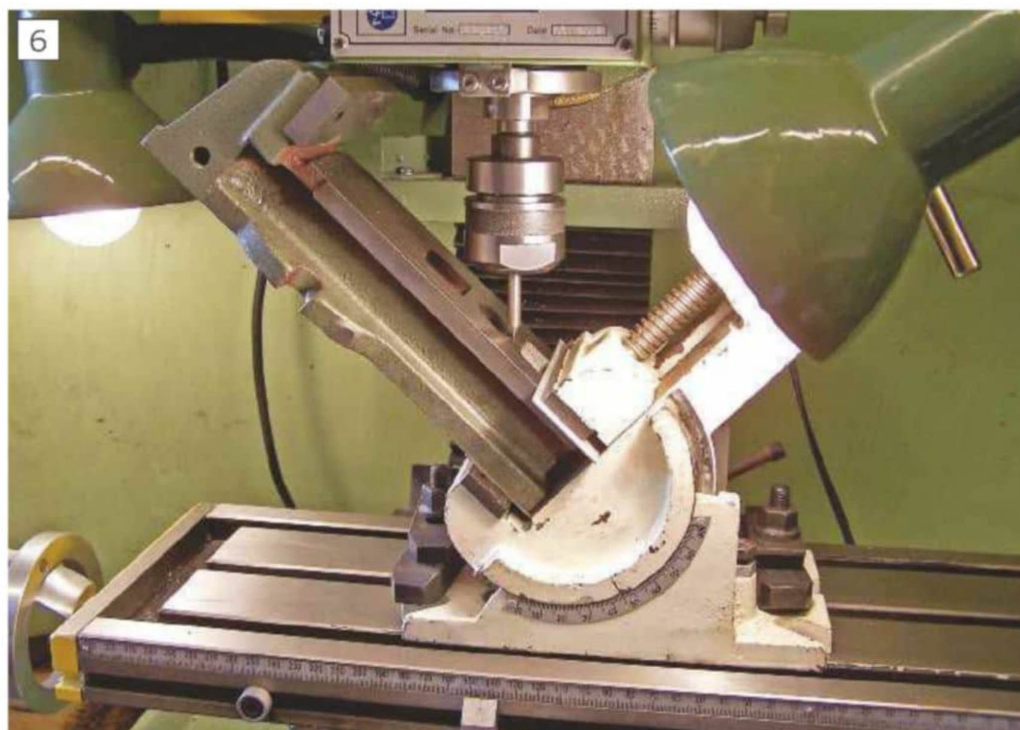
The set-up for drilling the angle hole
