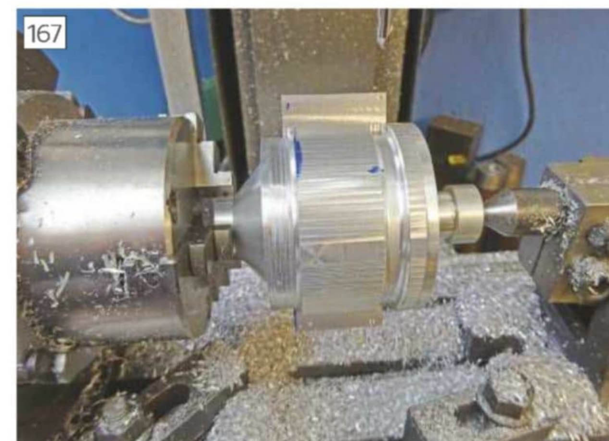
Vertically mounted for cutting radial grooves
