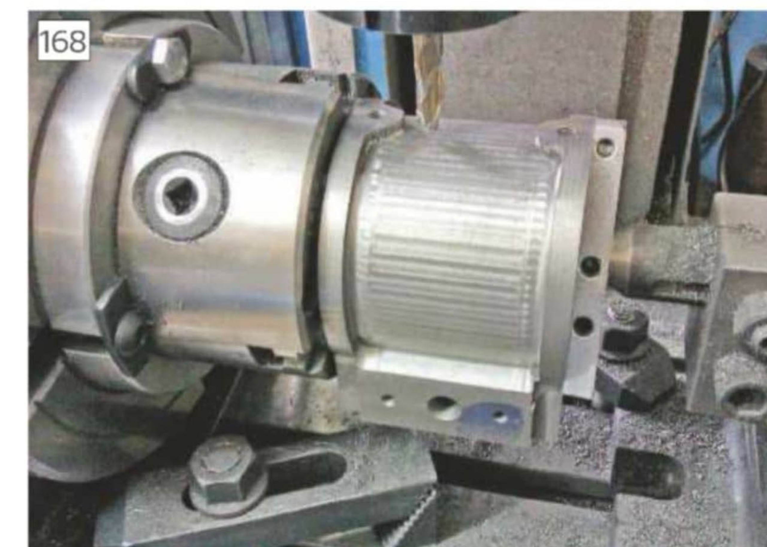
Straight and radial cuts with tailstock support
