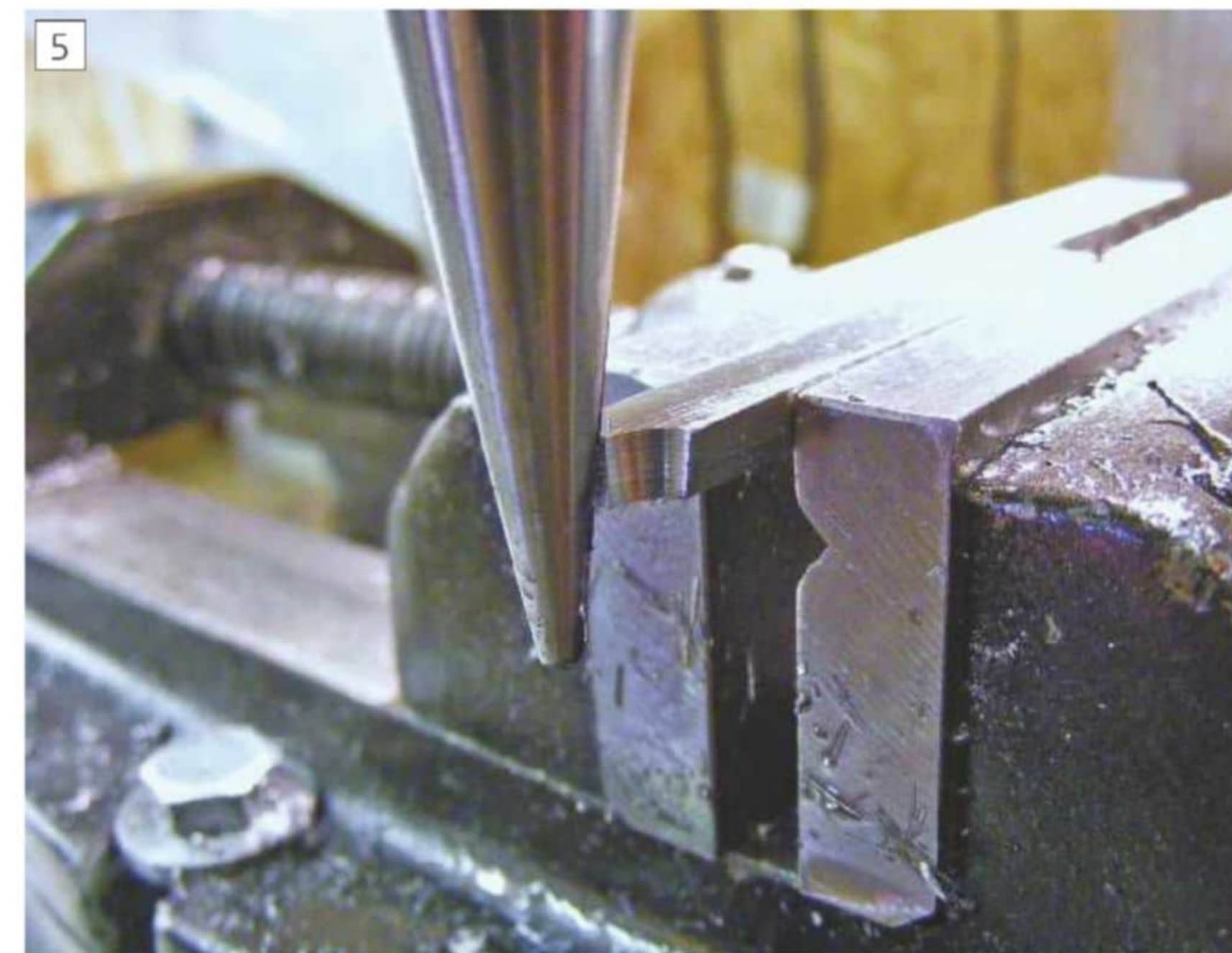
Profiling the cutter with the cone drill.
