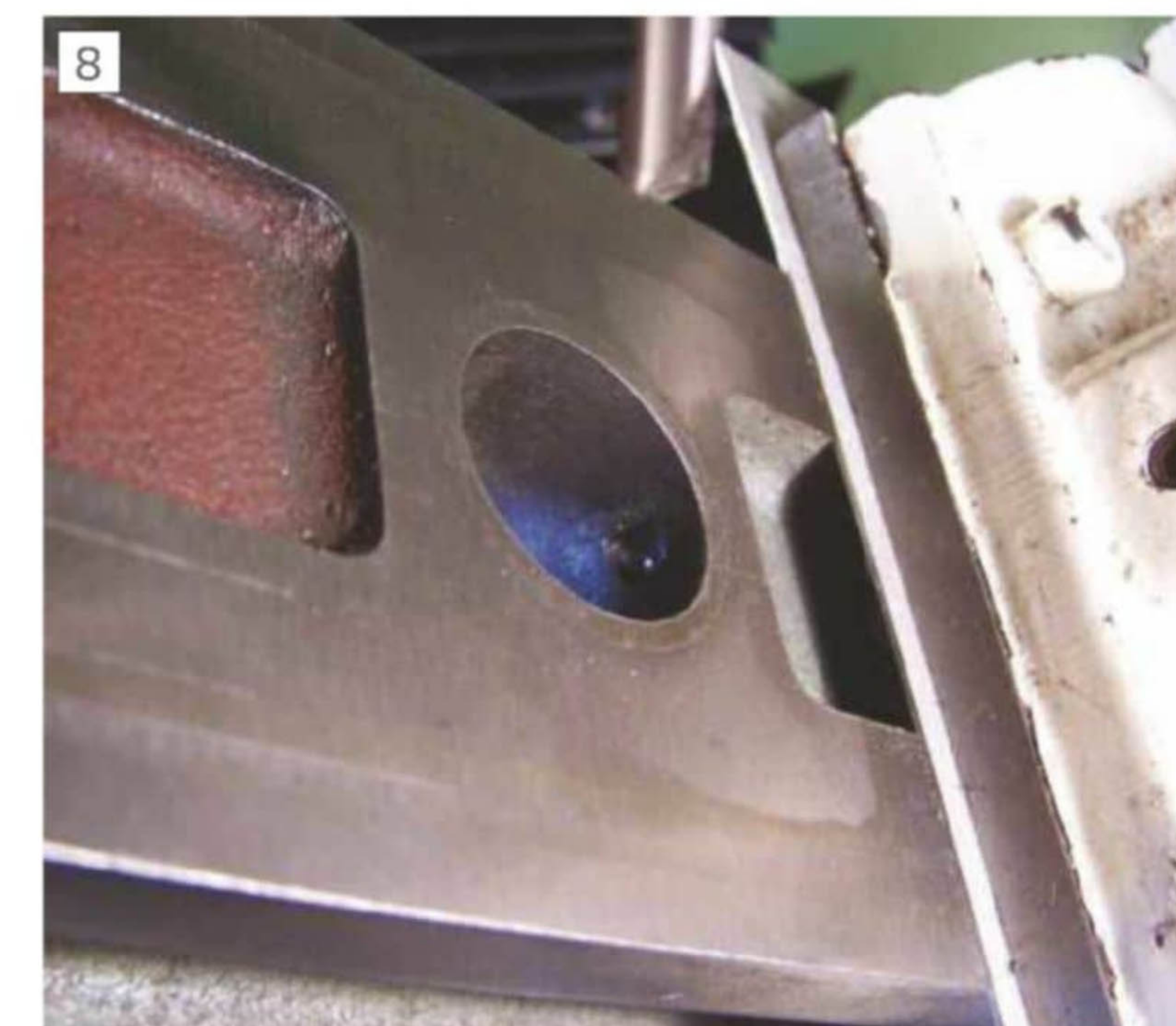
The spotted mark ready for drilling
