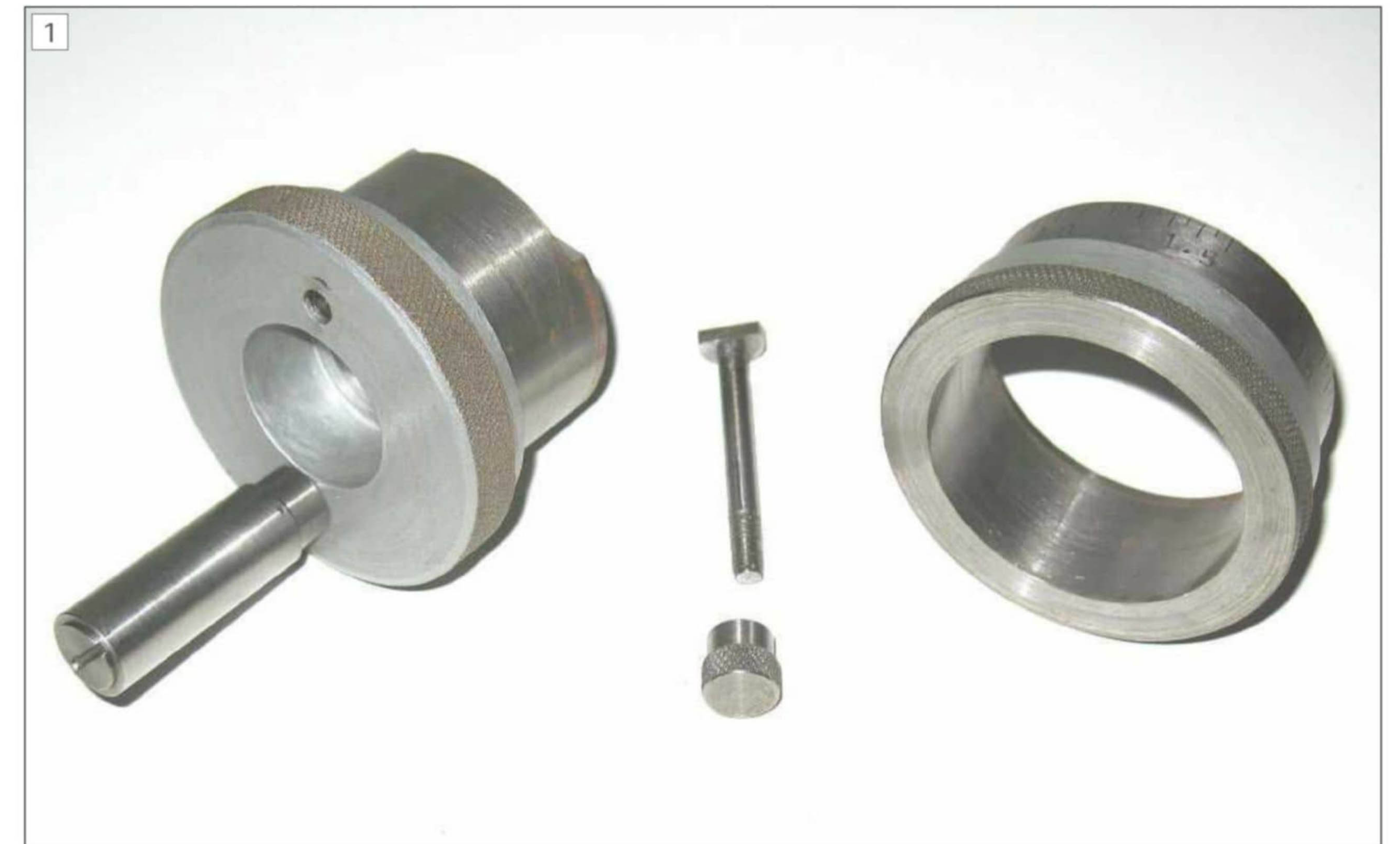
Micrometer Dial Ring, Locking Pin, and Handwheel.
