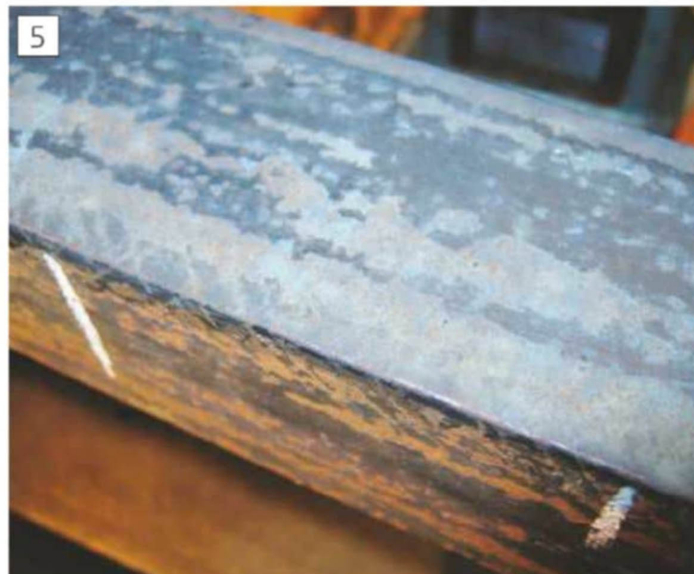
Angles mark out with layout blue
