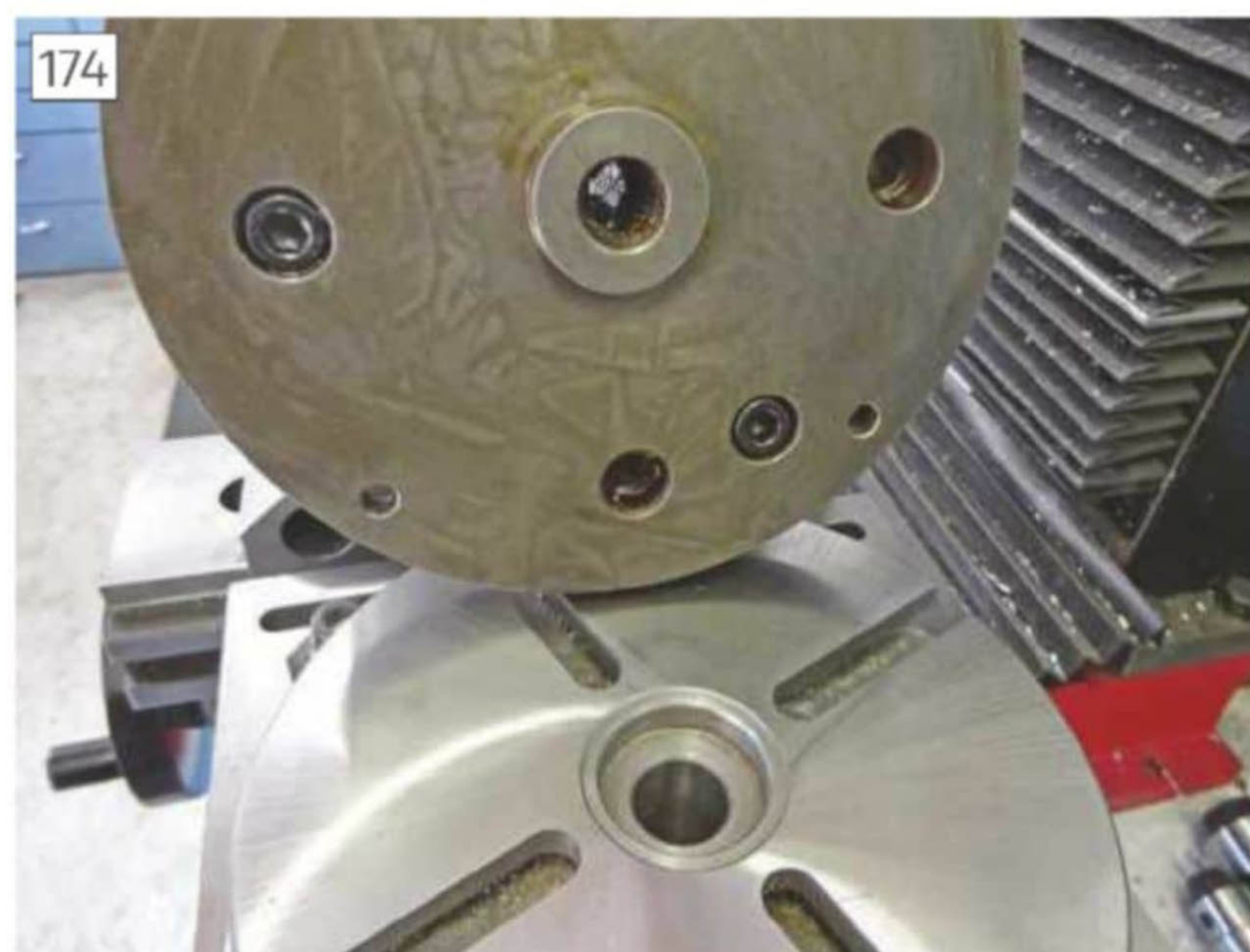
Location recess in table and mating spigot on backplate
