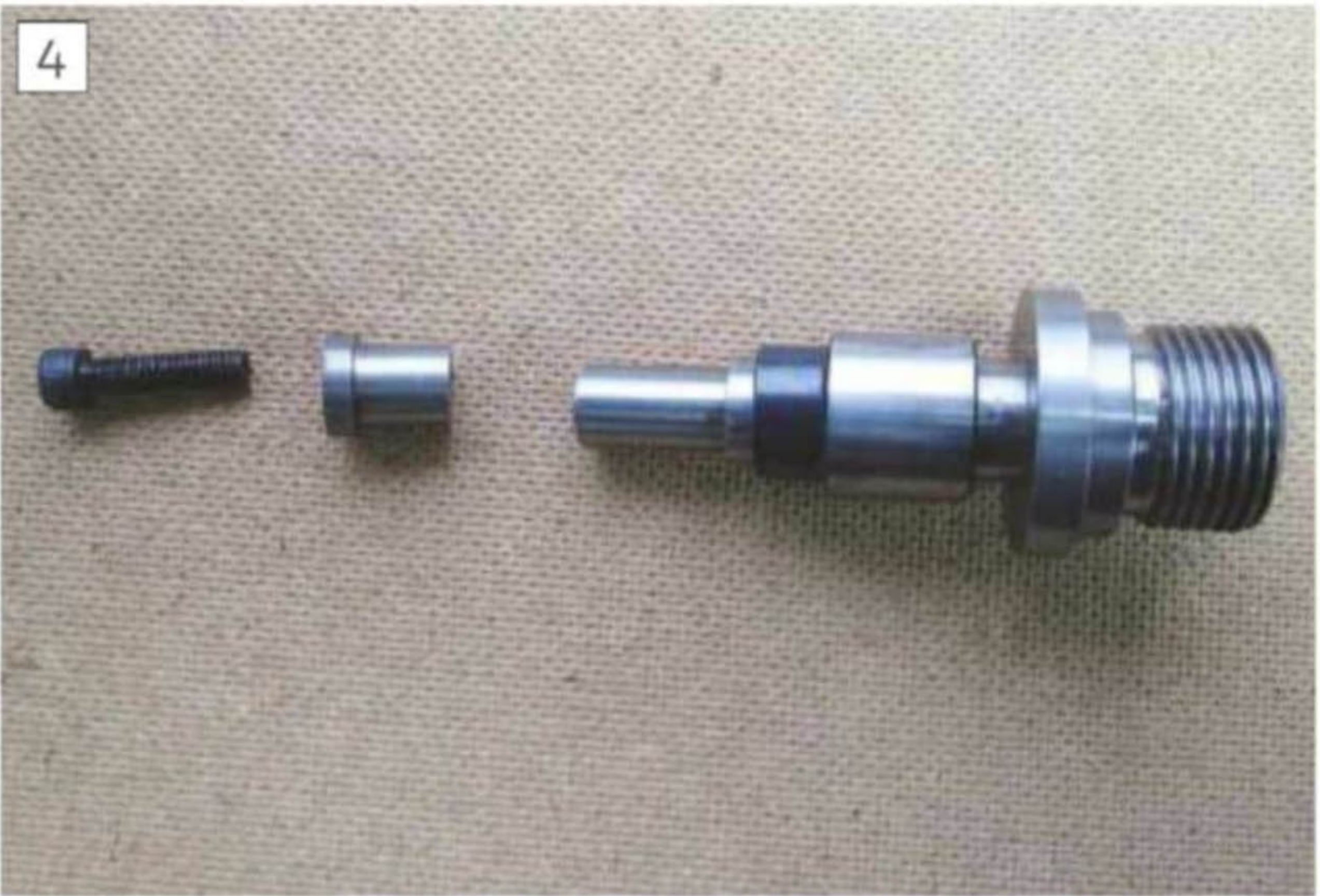
Mandrel and parts to fix it to the table
