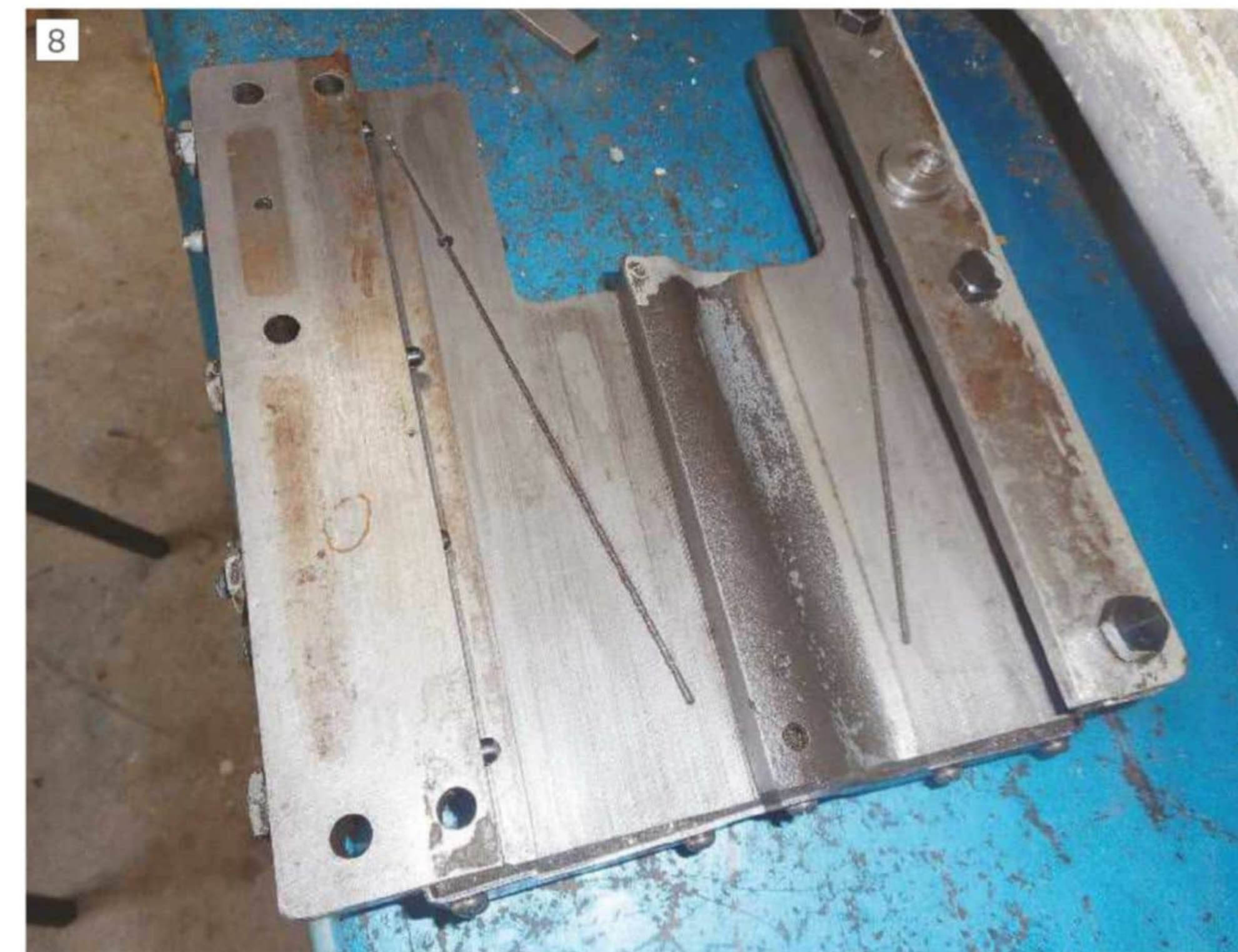
Unworn strips to the left of the two scored contact areas provide references to measure wear.
