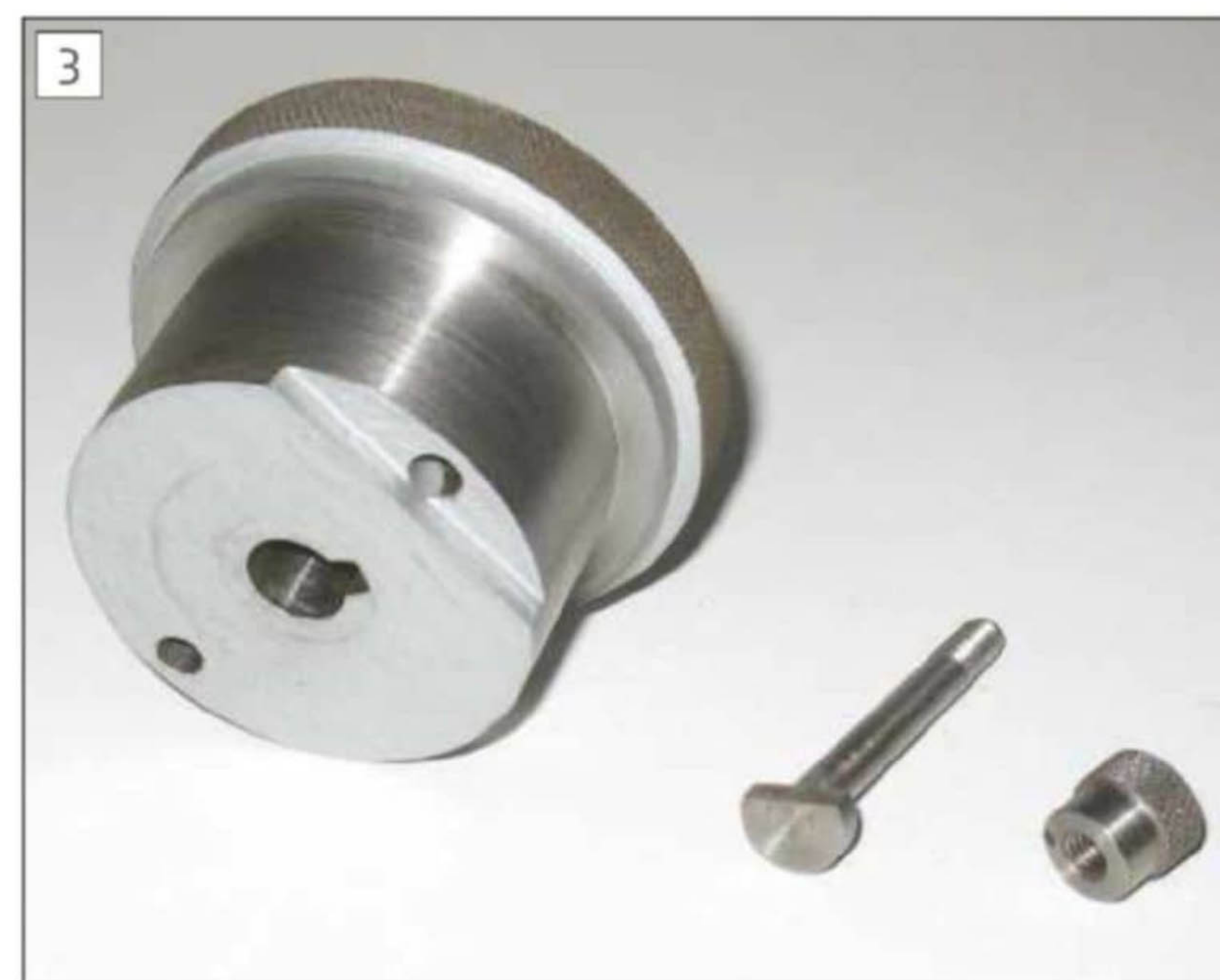
Clamp Bolt & Nut, along with rear view of Handwheel.
