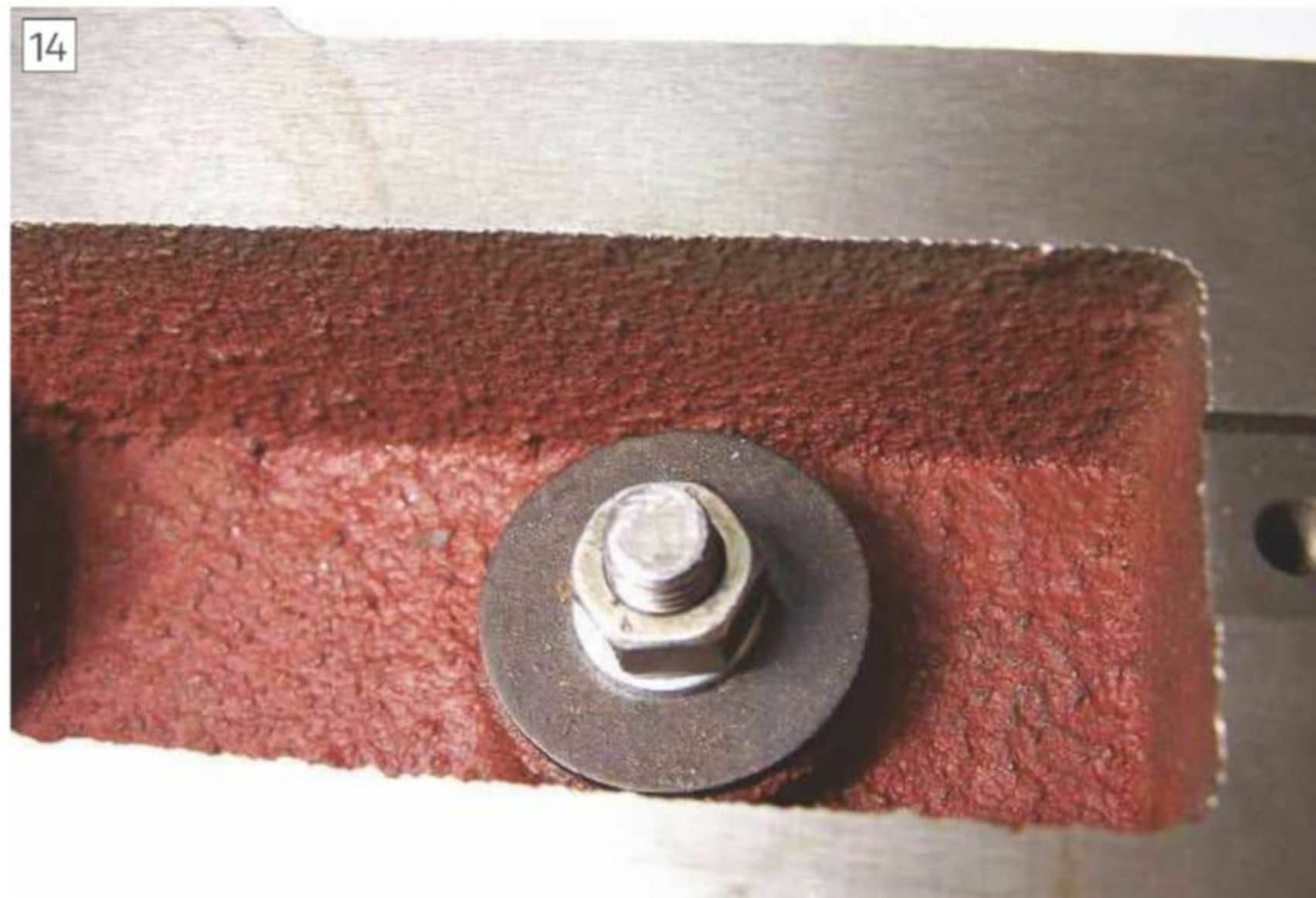
The M8 nut securing the main vice nut
