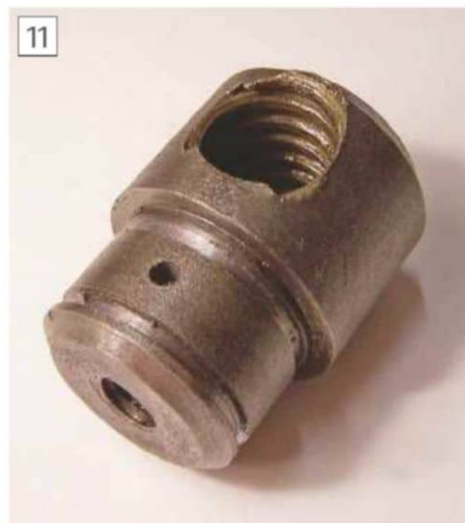
The 2.5mm hole to allow the grease through
