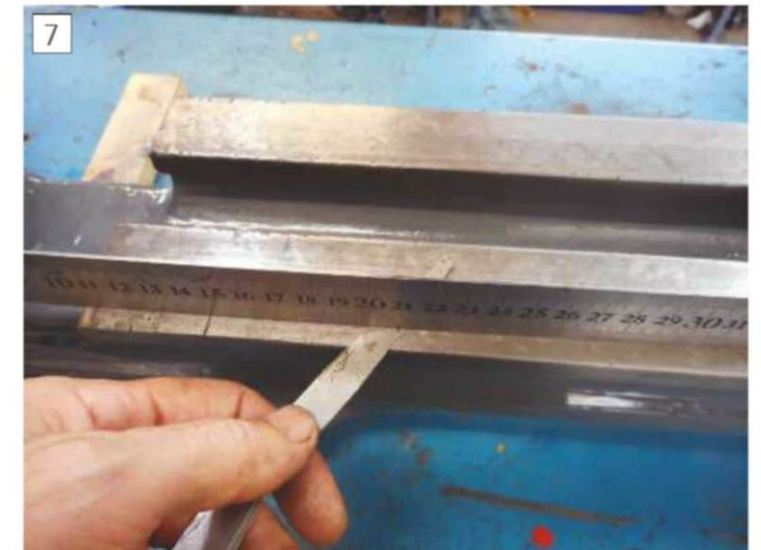
A long steel rule and feeler gauges can be used in a pinch to assess bed wear, or to confirm our micrometer readings.
