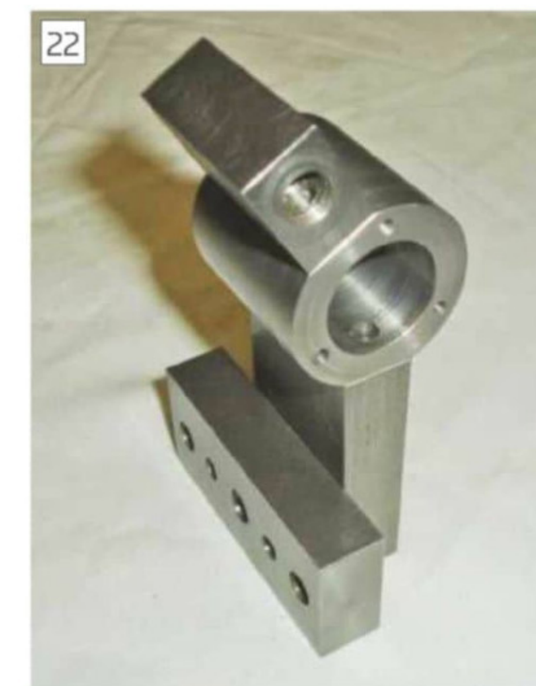
The stop block assembled and ready for silver soldering (Paul Clark)
