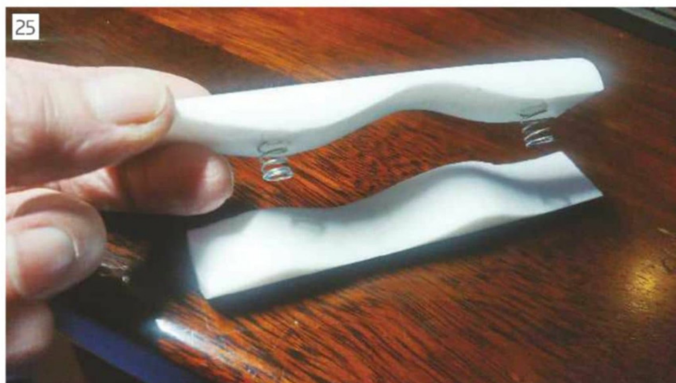
Completed charging elements with springs.
