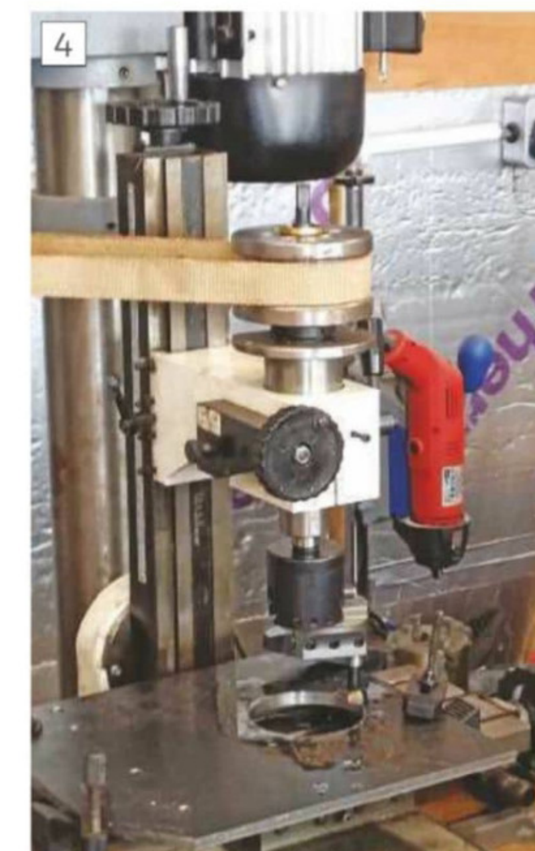
Boring the new motor mount plate
