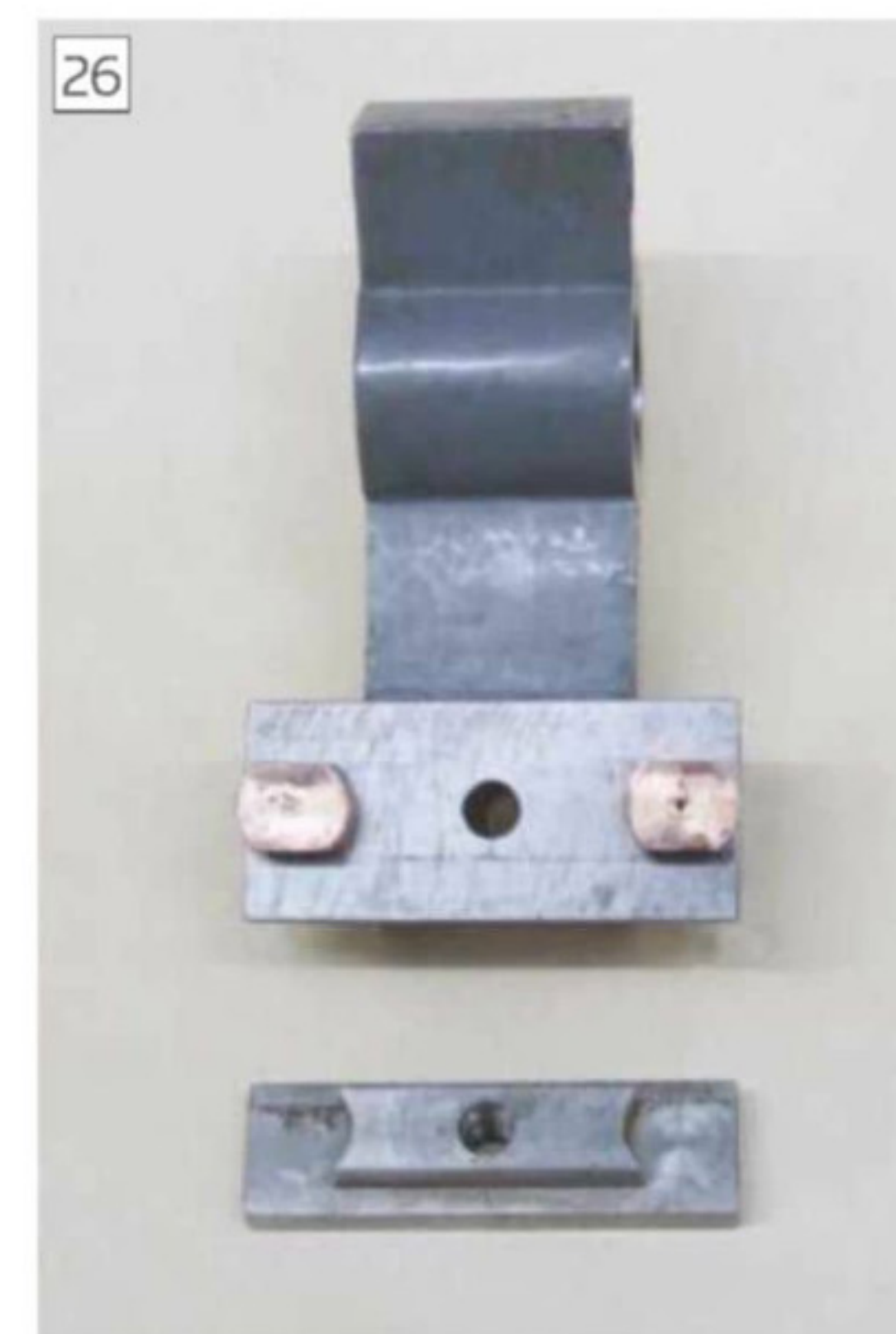
The guide pegs have now been fitted to the stop block, shown with the tee-nut bar
