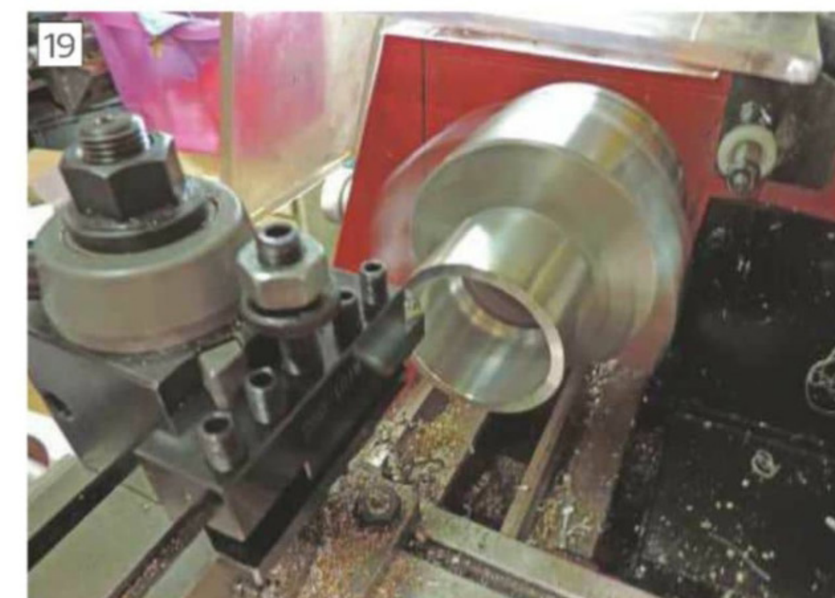
Internal chamfer with tool raised well above centre height.
