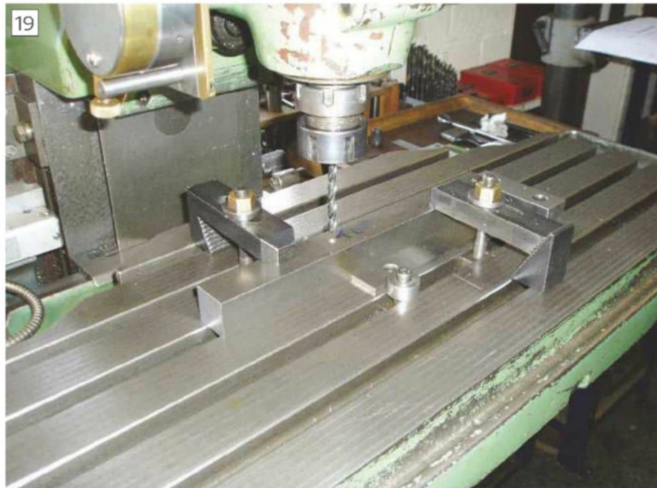
One method of setting the mounting bar on the milling machine table (Paul Clark)
