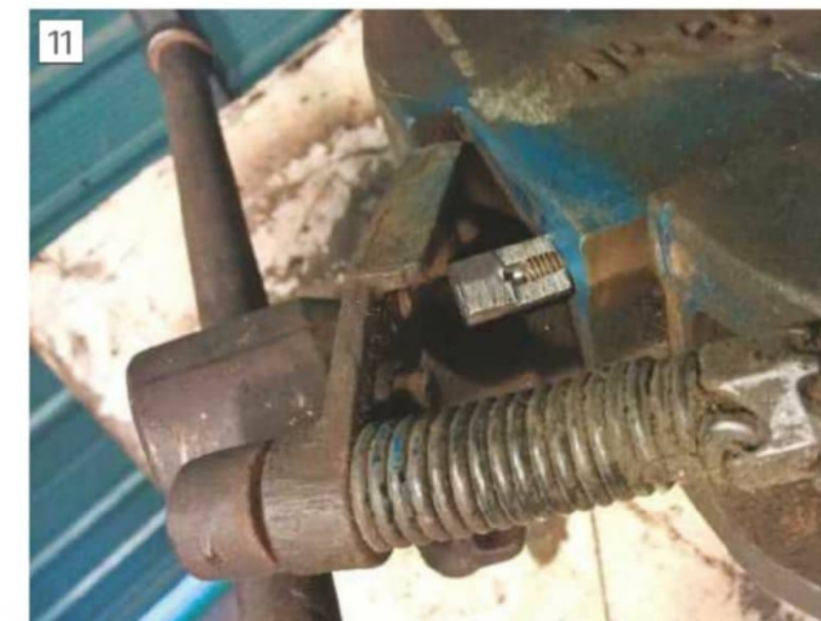
Weld on head ready for welding
