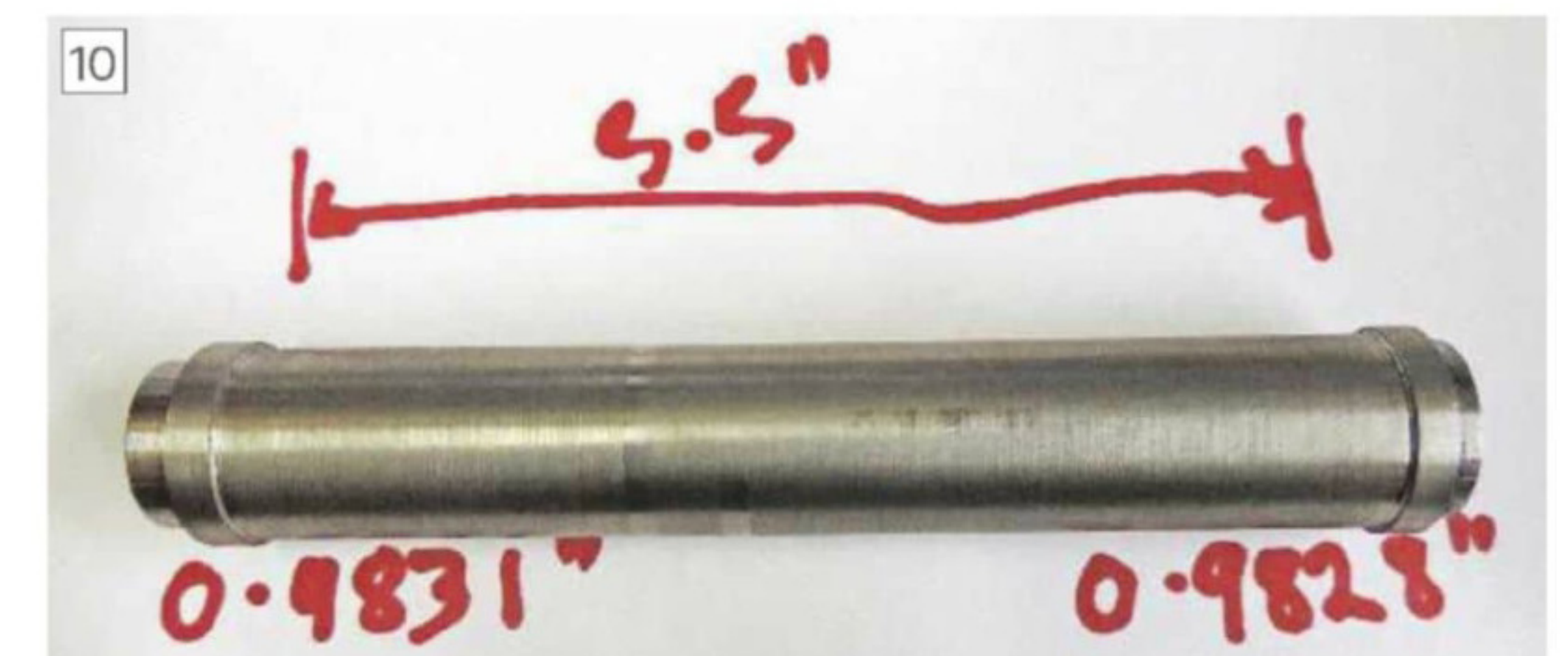
Tailstock setting bar, used between centres with a dial indicator in the toolpost.
