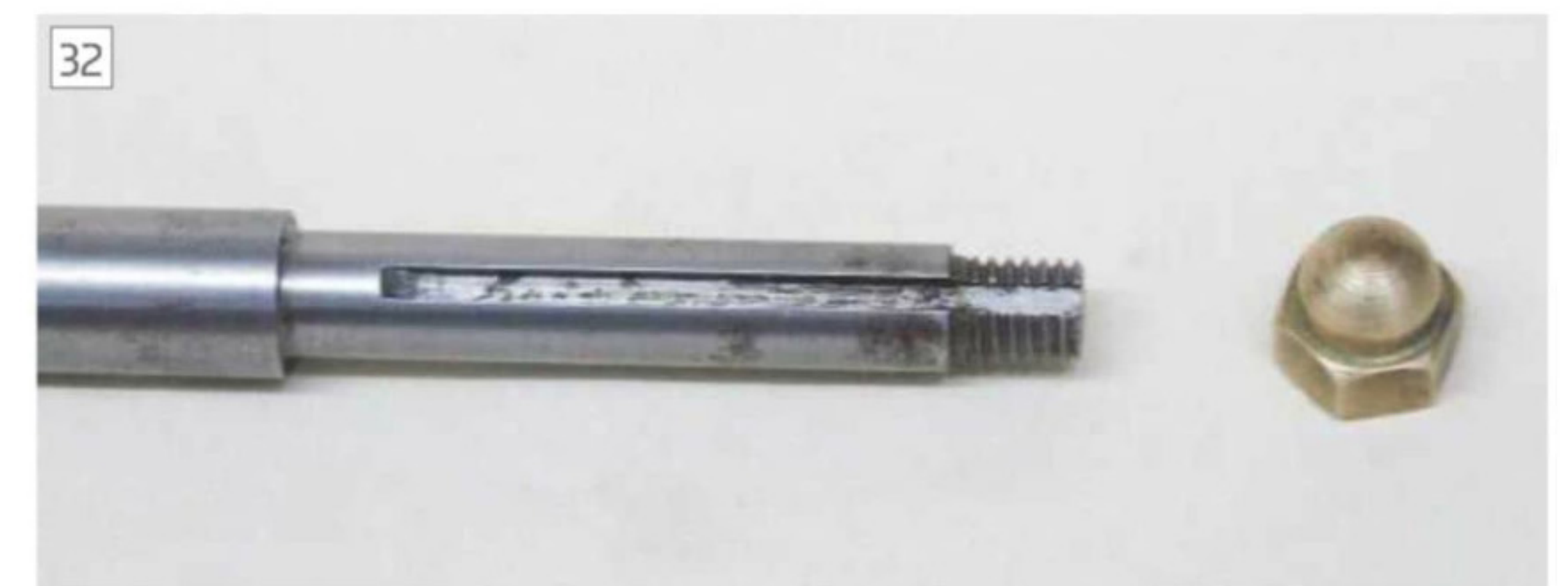
The completed keyway and acorn nut
