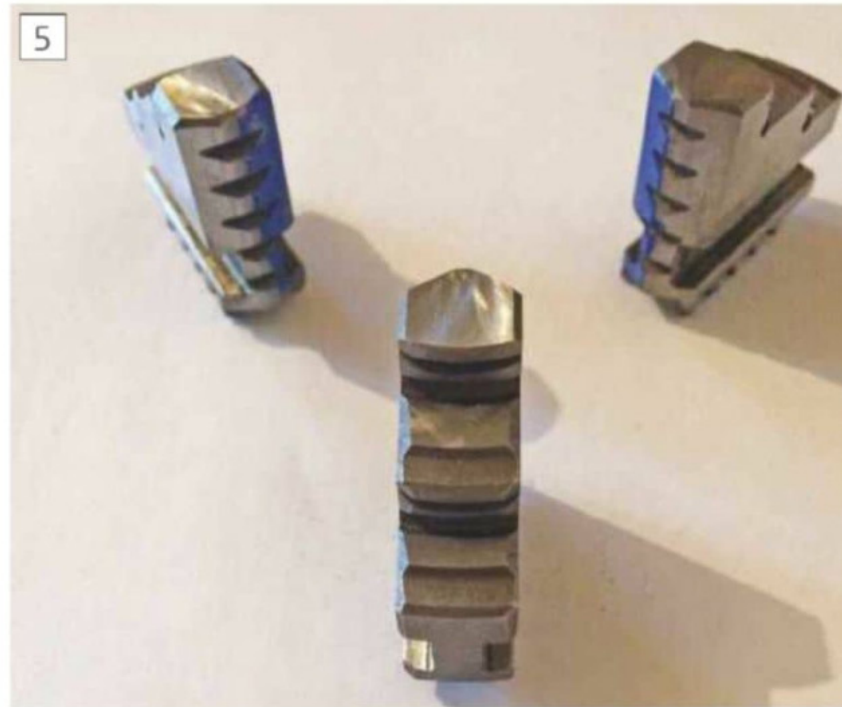
The three jaws and the surfaces to be corrected.
