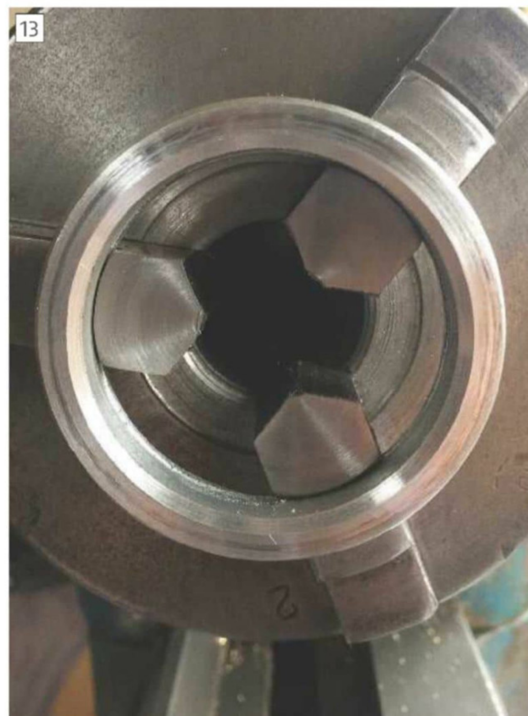
Securing jaws open under light pressure, restrained by circular band.
