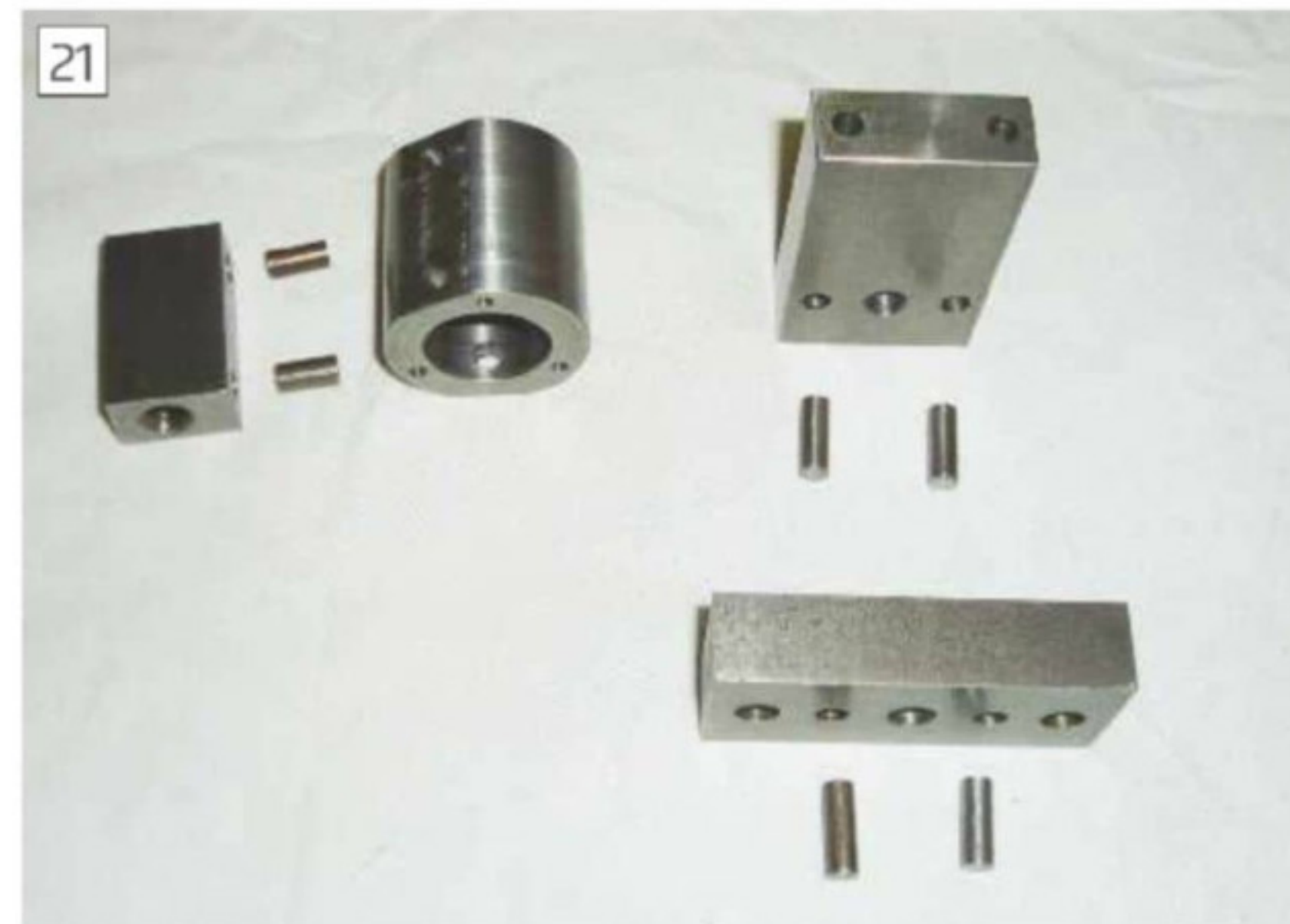
The component parts for the stop block before silver soldering (Paul Clark)
