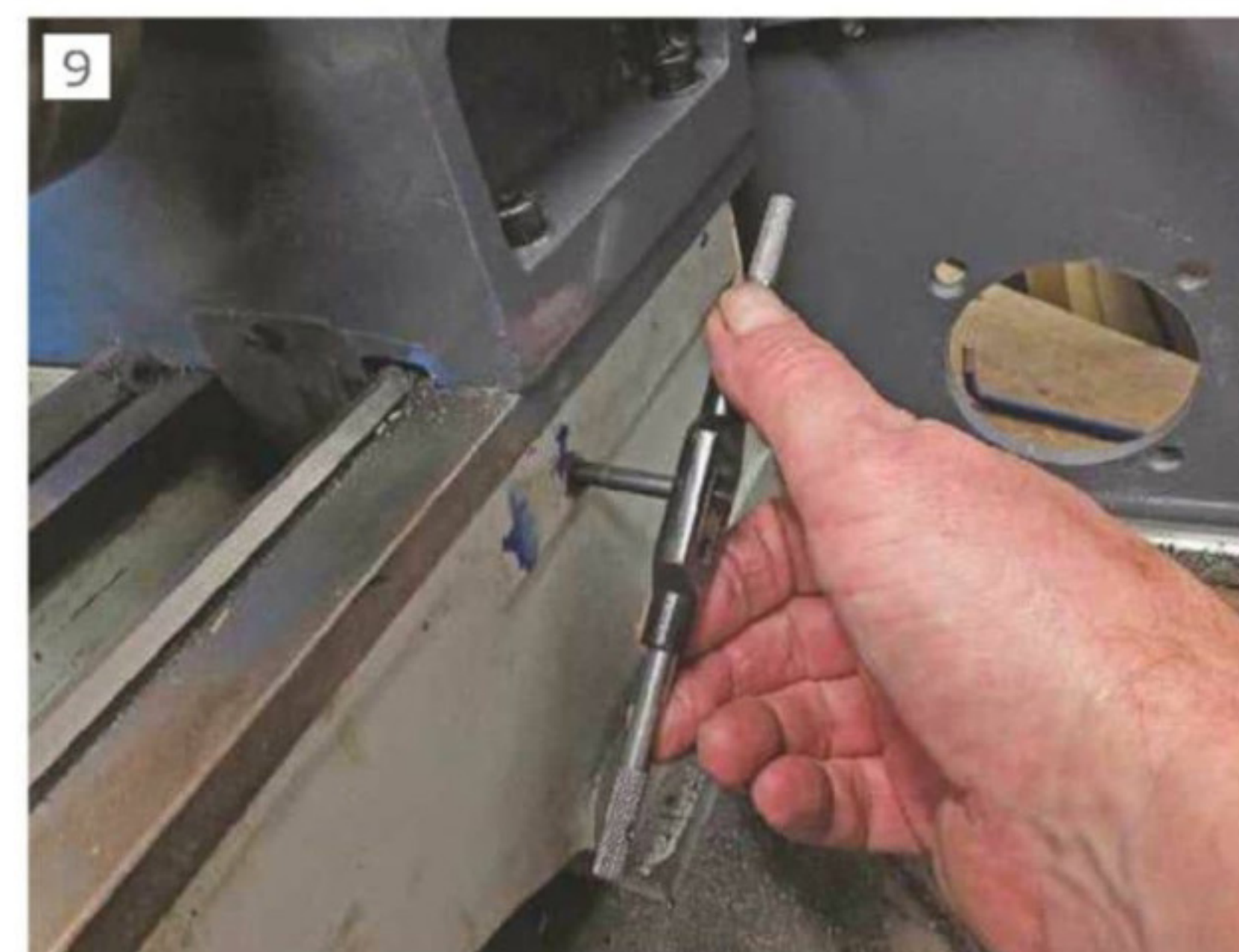
Tapping the main casting
