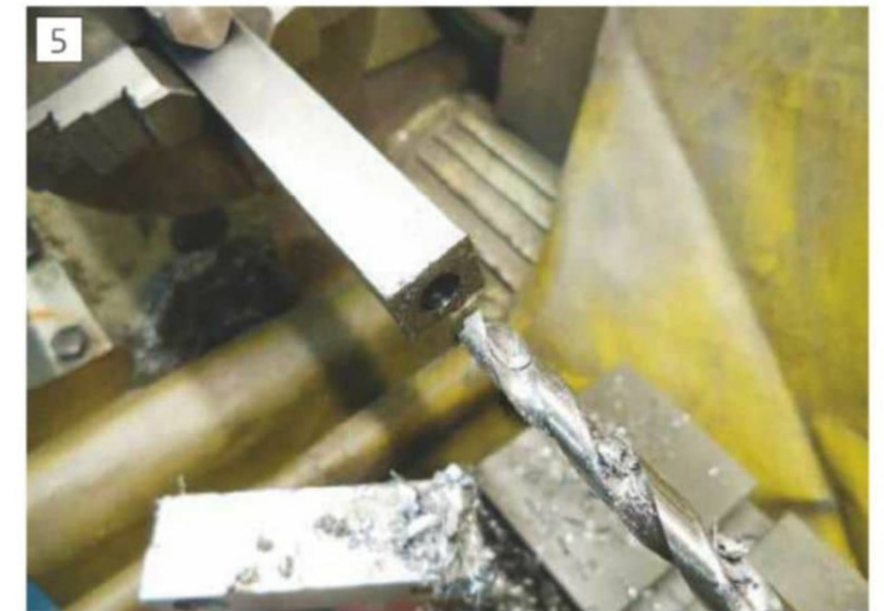
Drilling to depth
