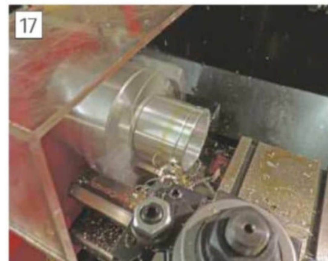
Parting the end off the adaptor, thread protected by a screwed ring.
