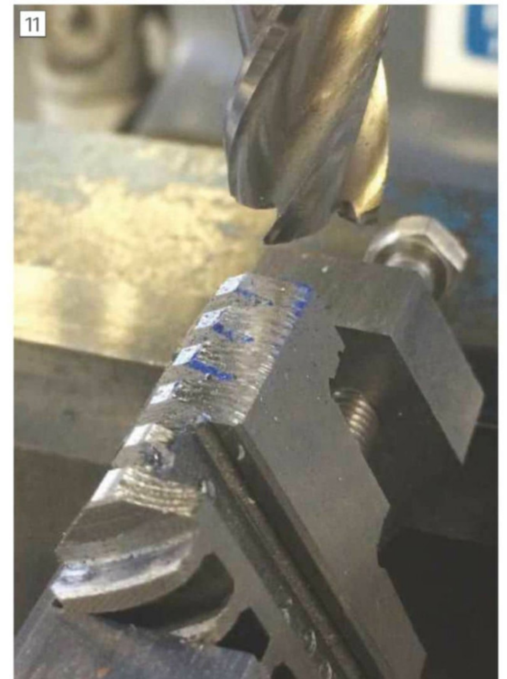
Surface removed by shallow cutter action.
