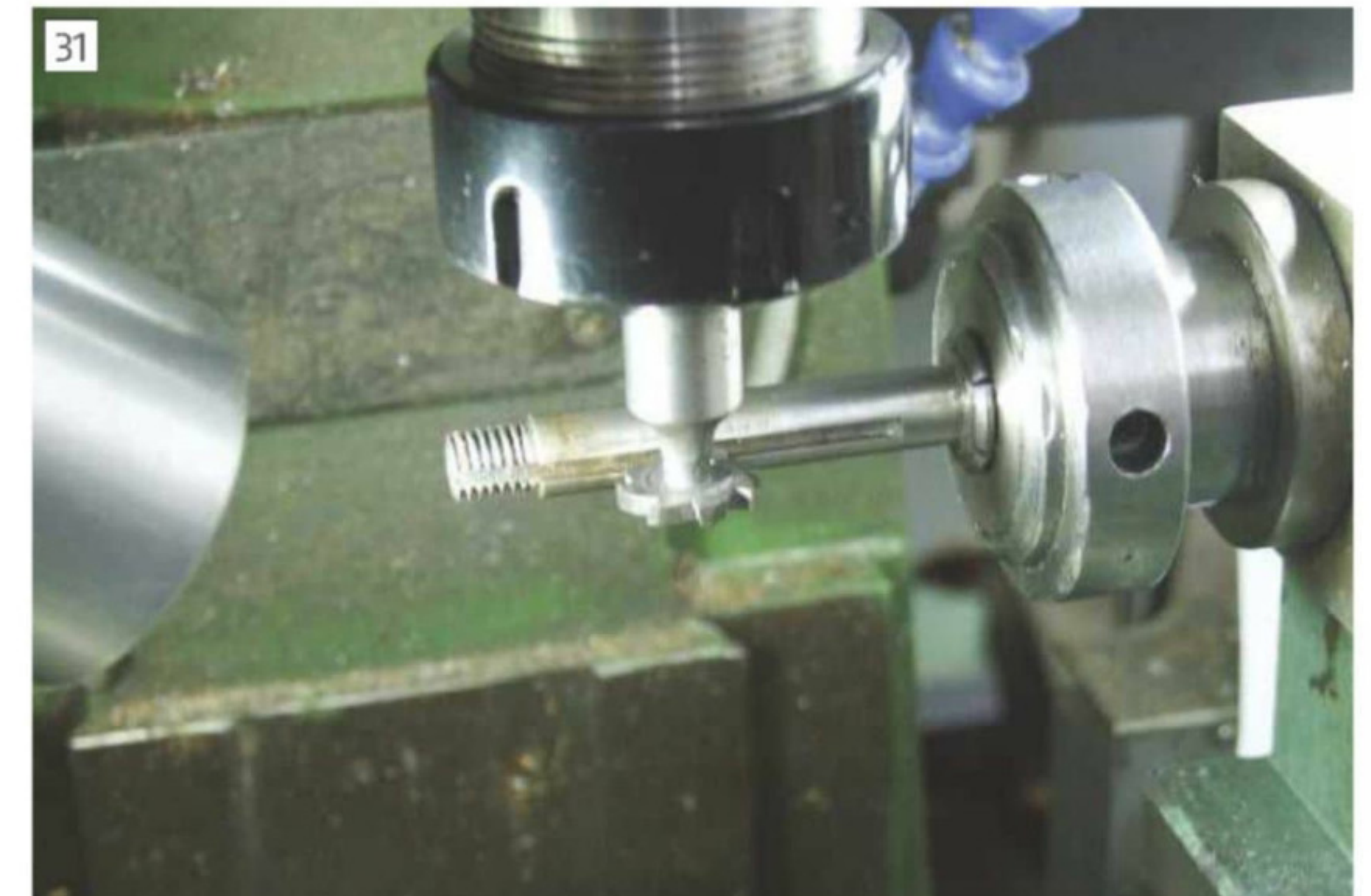
Milling the keyway on the stop rod using a Woodruff cutter (posed)
