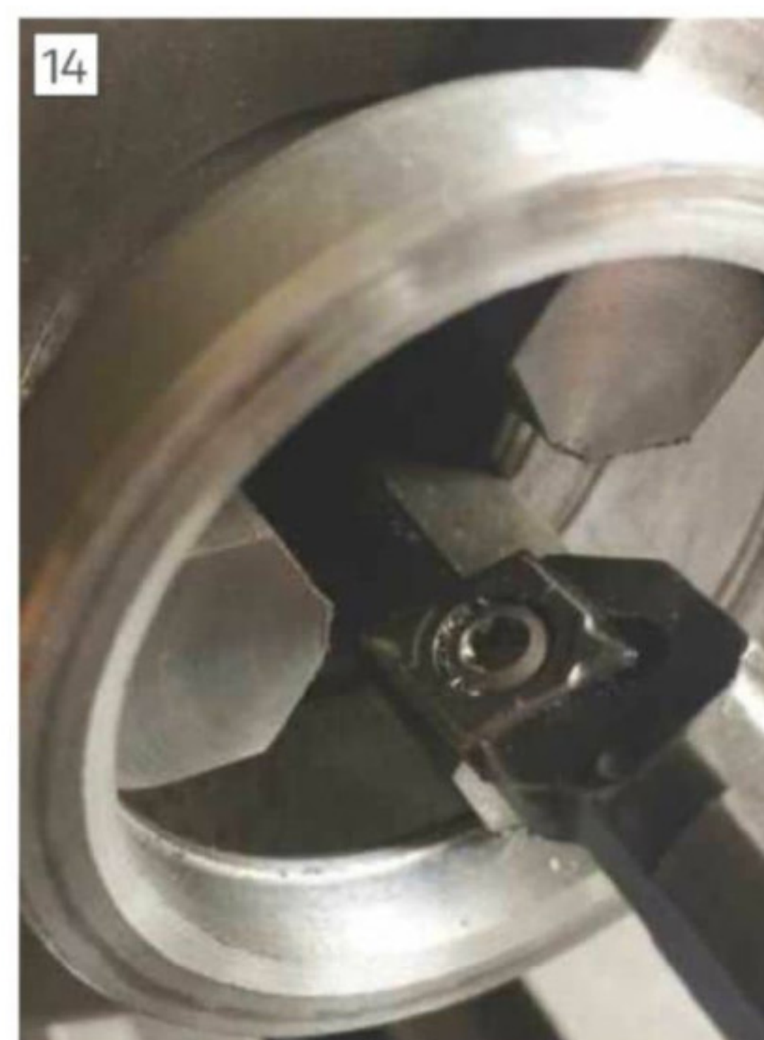
Machining an old chuck. Method to recreate the tips of the three jaws.
