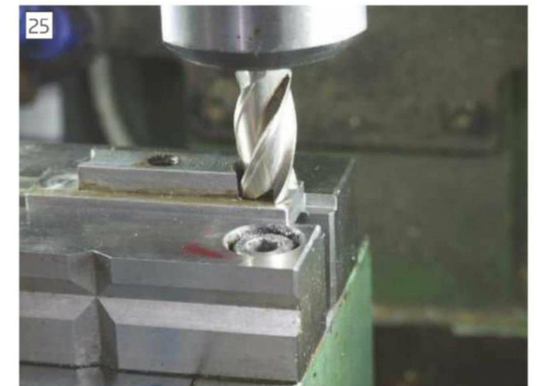
Machining the recesses in the tee-nut bar (posed)
