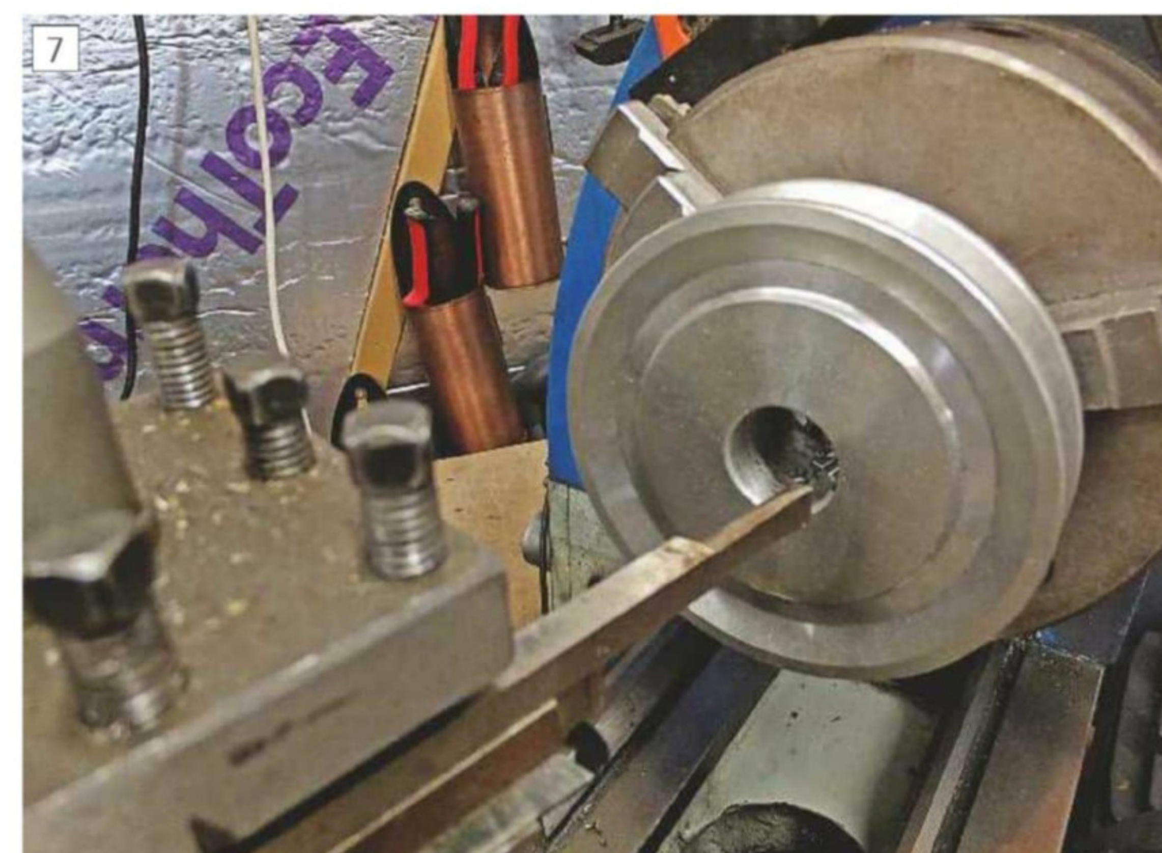
Motor pulley keyway cutting
