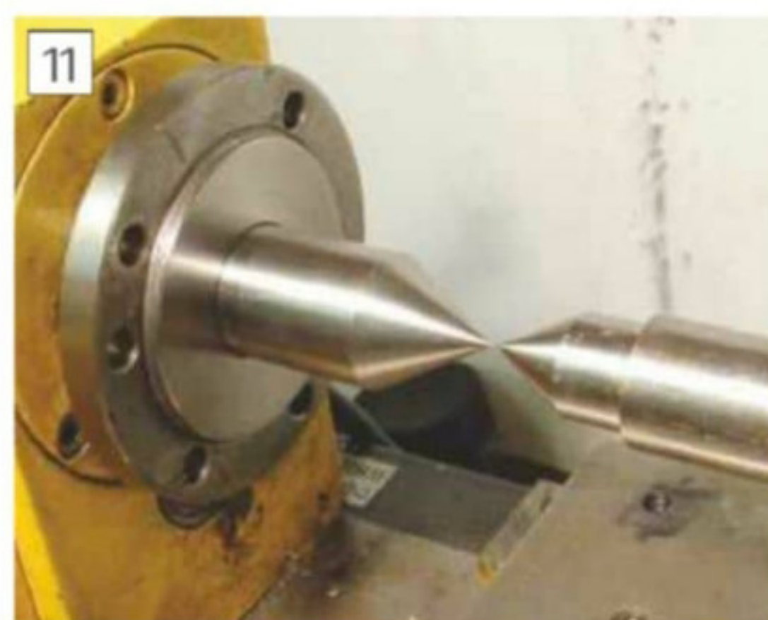
The simplest way to set the tailstock in a hurry.
