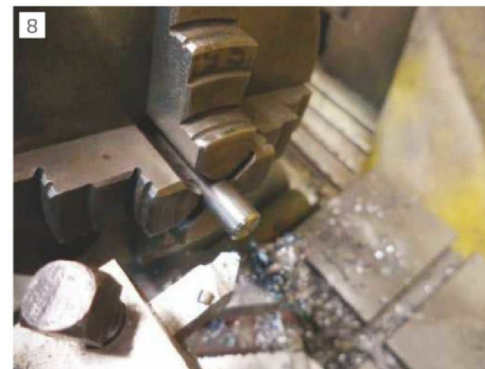
Reduce length of plunger to suite spring
