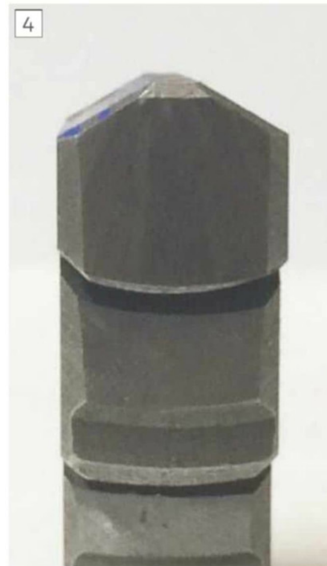
Chuck jaw showing surfaces of unequal length.
