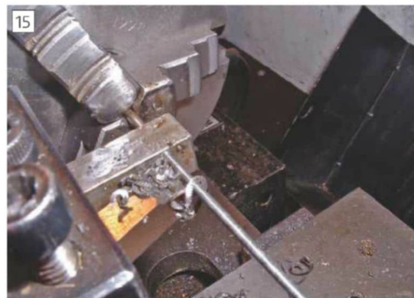
Improvised running down tool.
