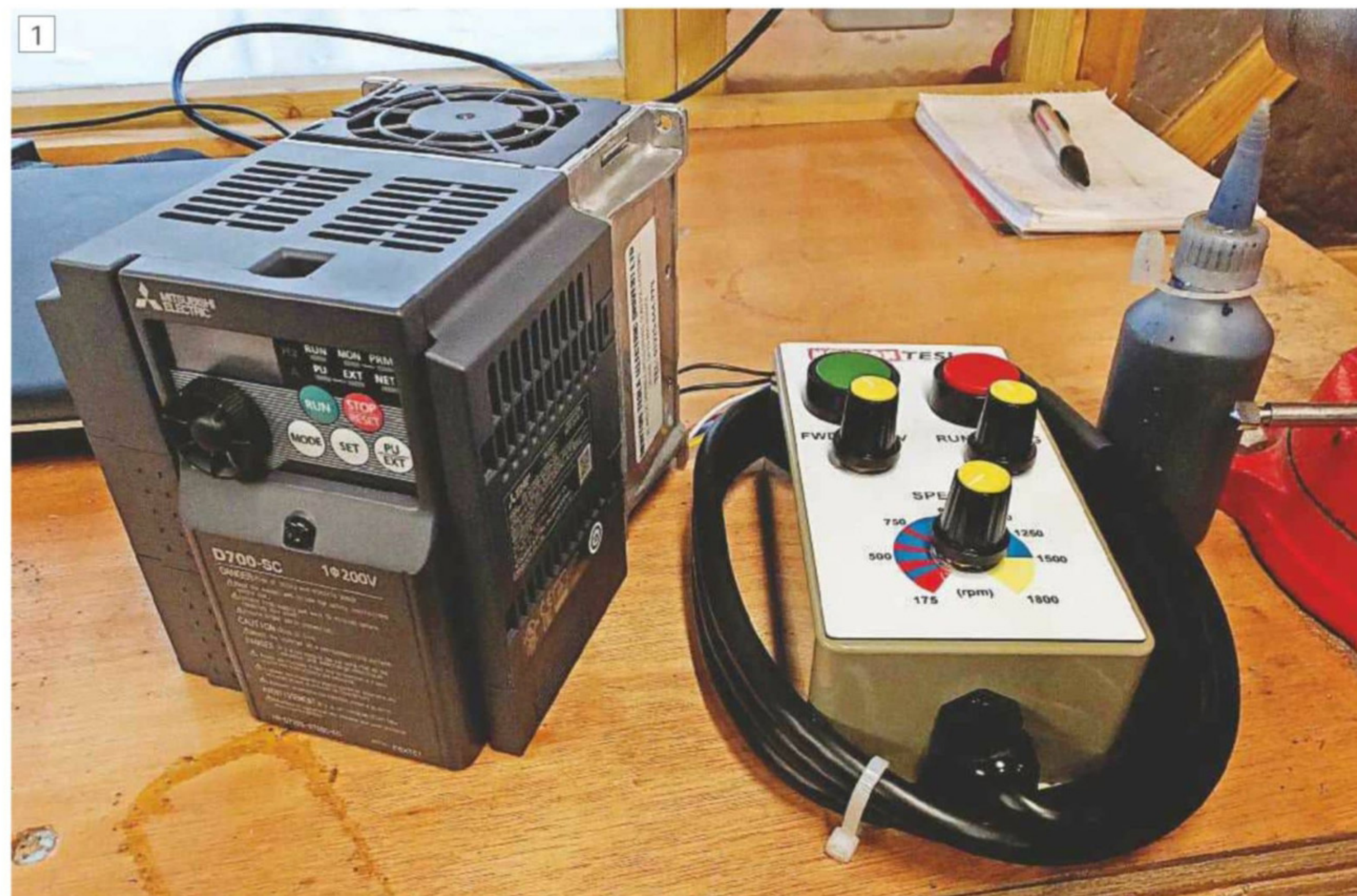
Inverter and Control
