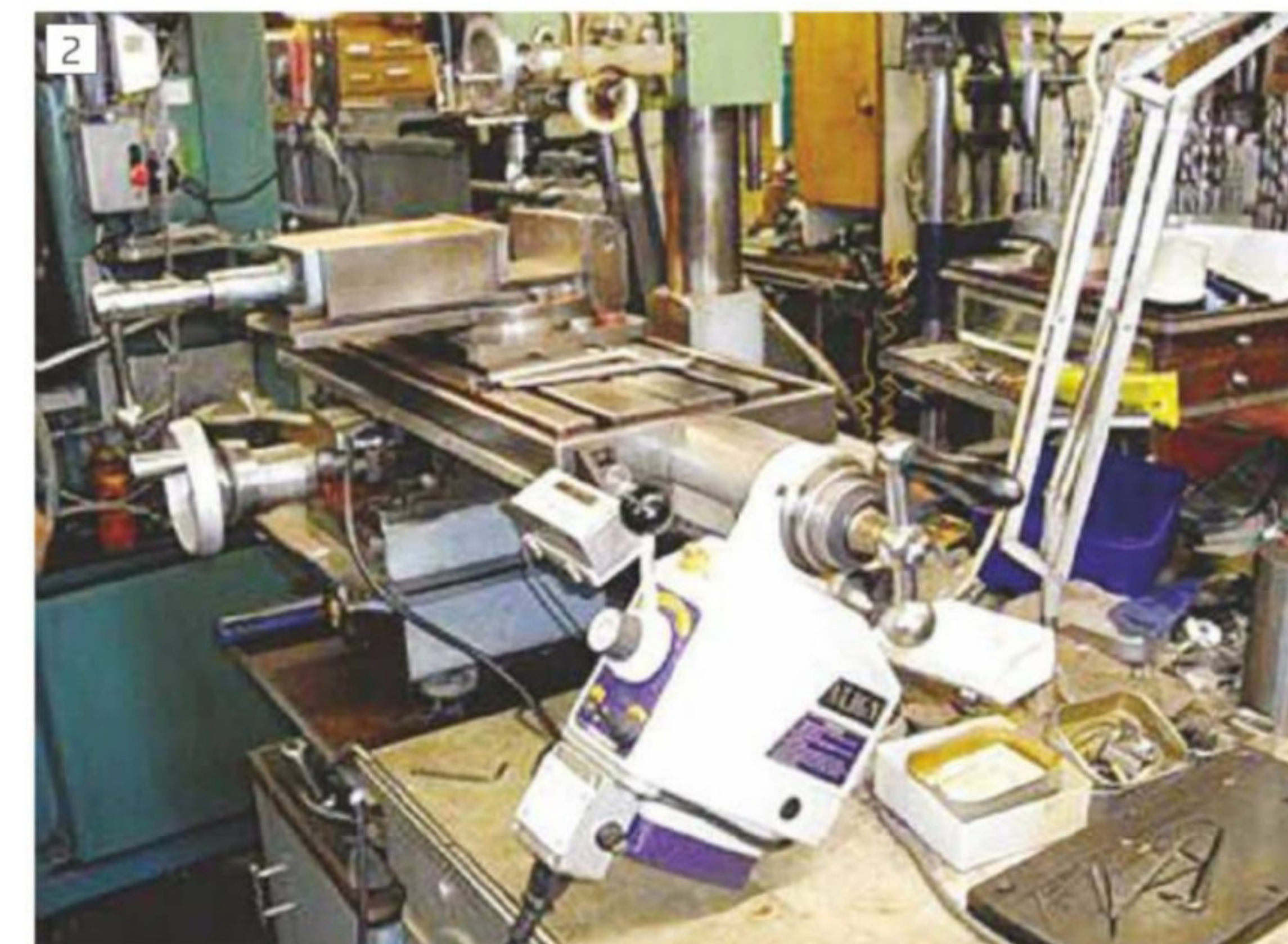
The compound table and power feed.
