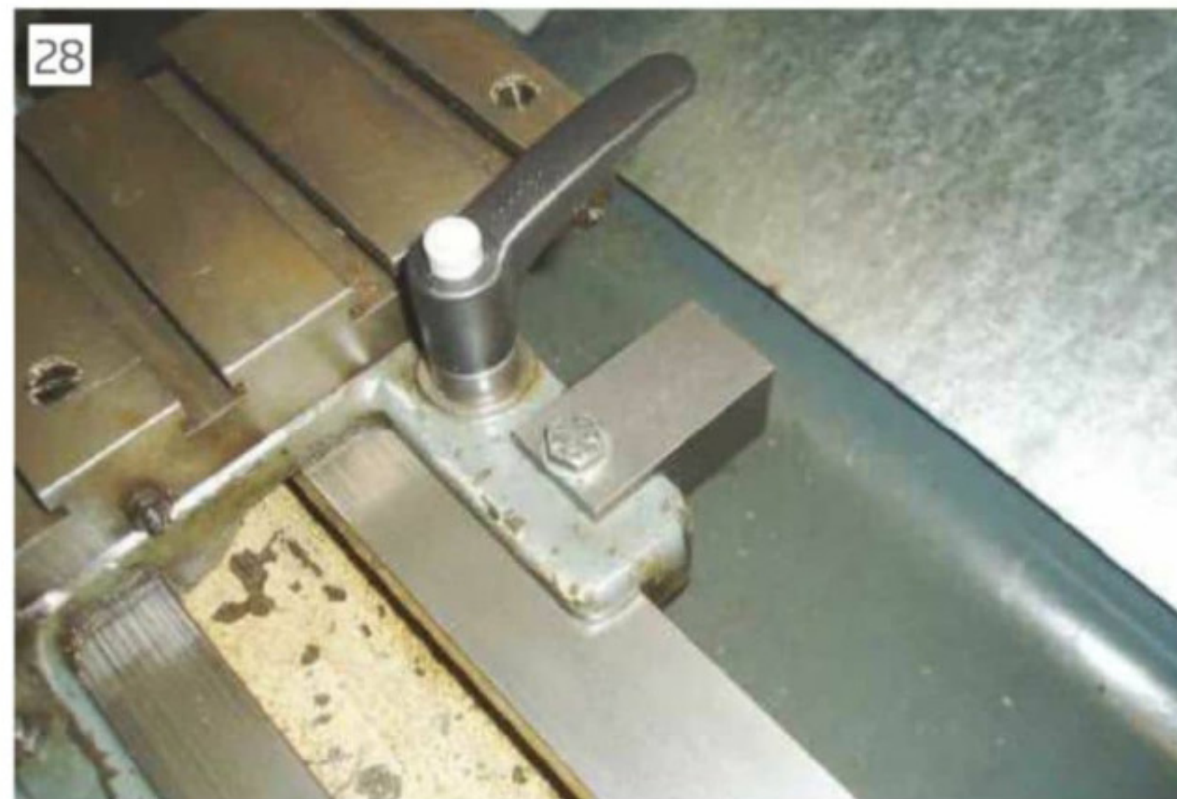
The machined attachment block for the saddle before drilling the hole for the stop rod (Paul Clark)
