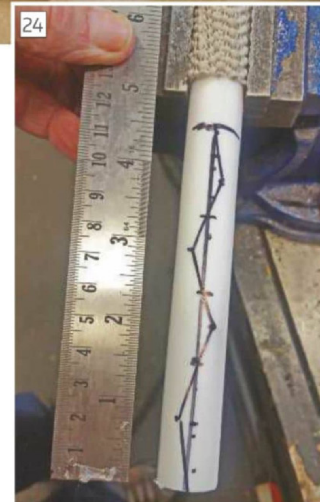
Suggested chicane cutting path drawn on PTFE stock.
