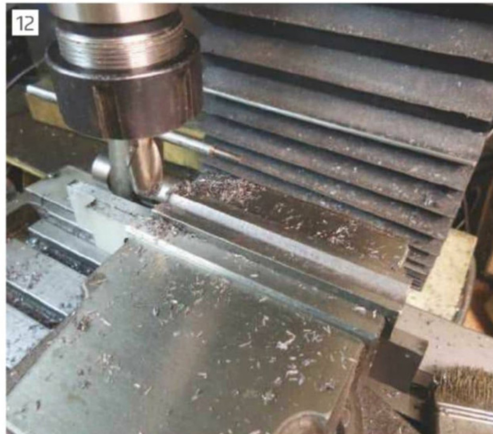
Fluting the body with a bull nosed end mill
