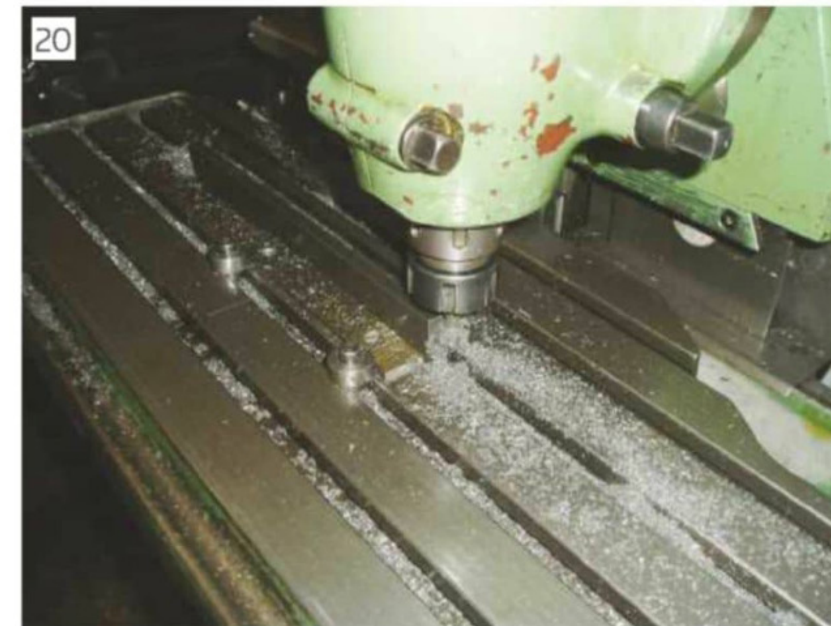
Milling the tee-slot in the mounting bar (Paul Clark)
