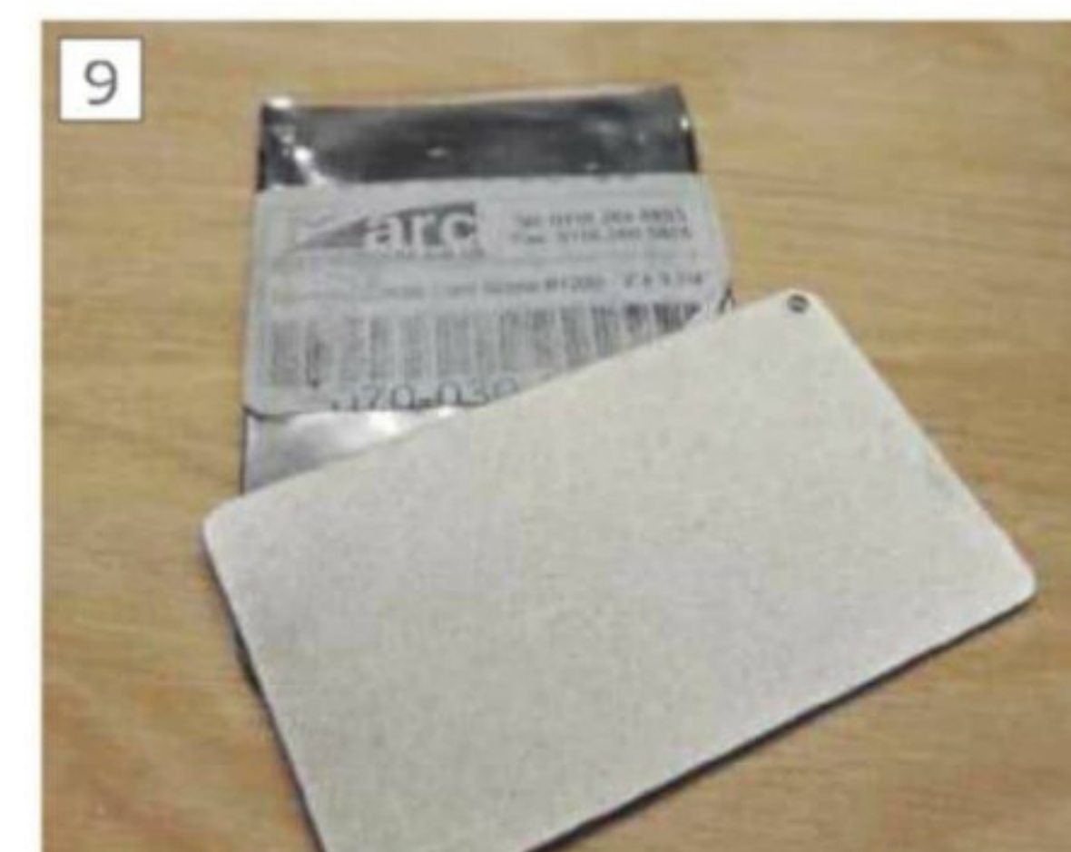
The credit card diamond sharpener.
