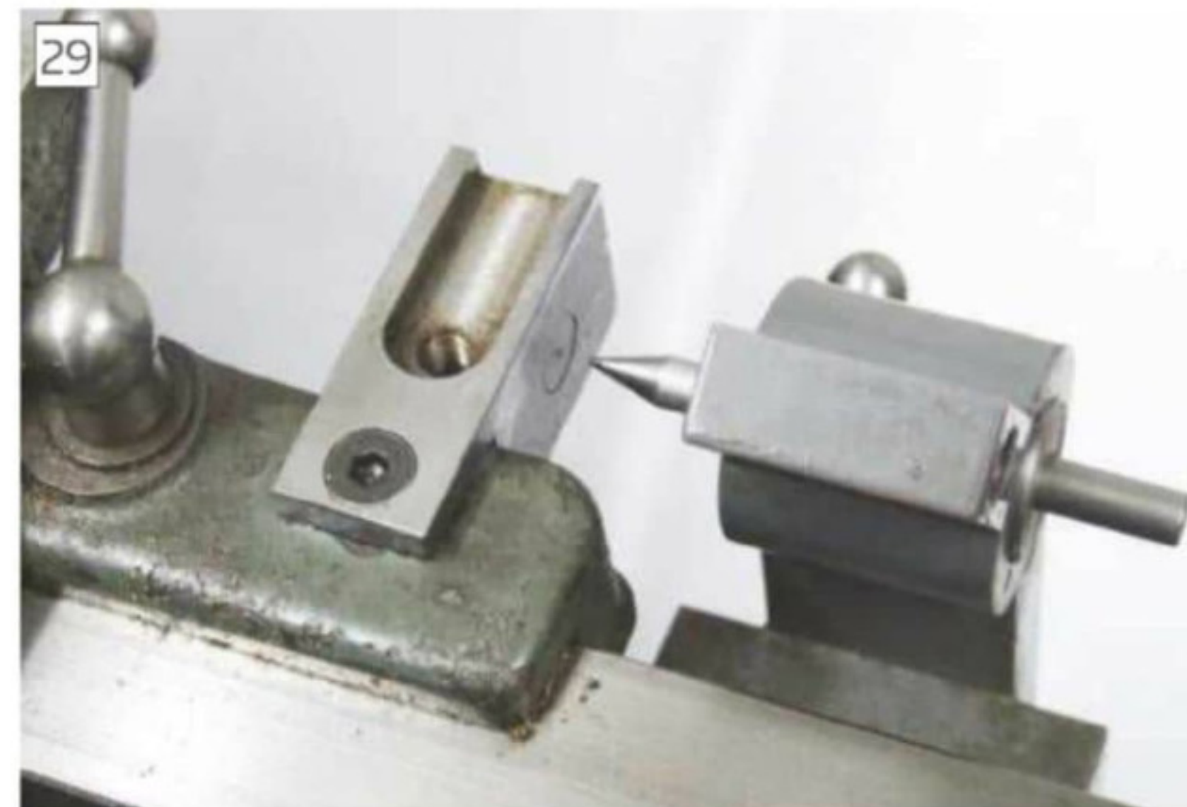
Marking the hole position for the stop rod in the attachment block on my machine (posed photo)
