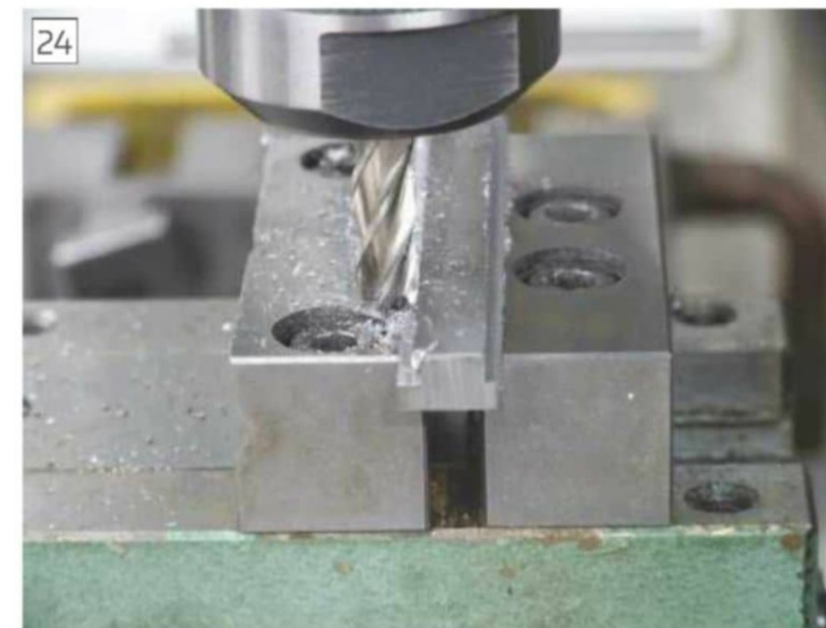
Milling the clamping faces on the tee-nut
