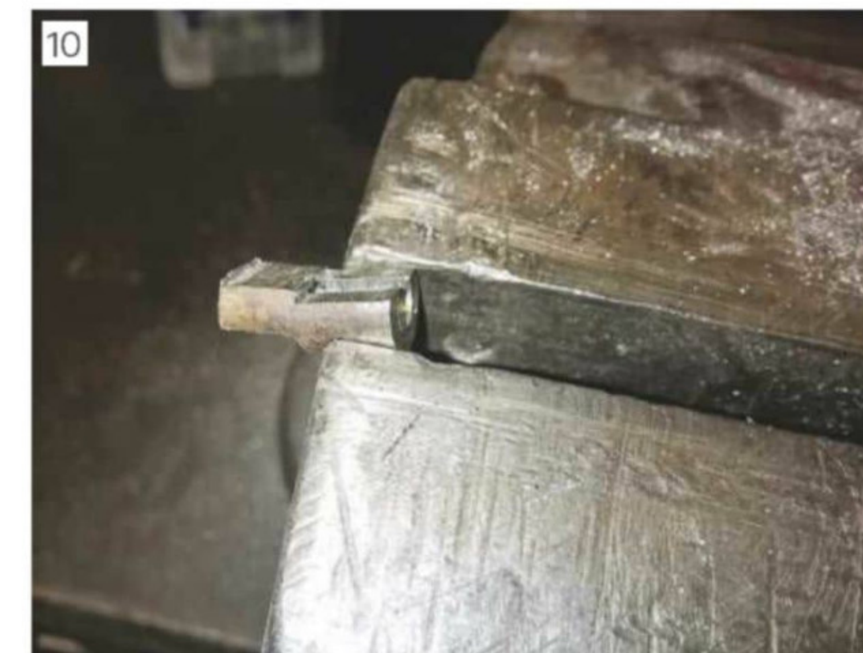
Weld on head prepared
