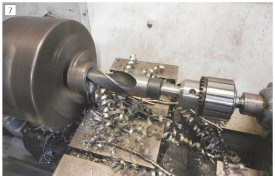
Taper does not budge under load when drilling a one-inch hole with heavy feed.
