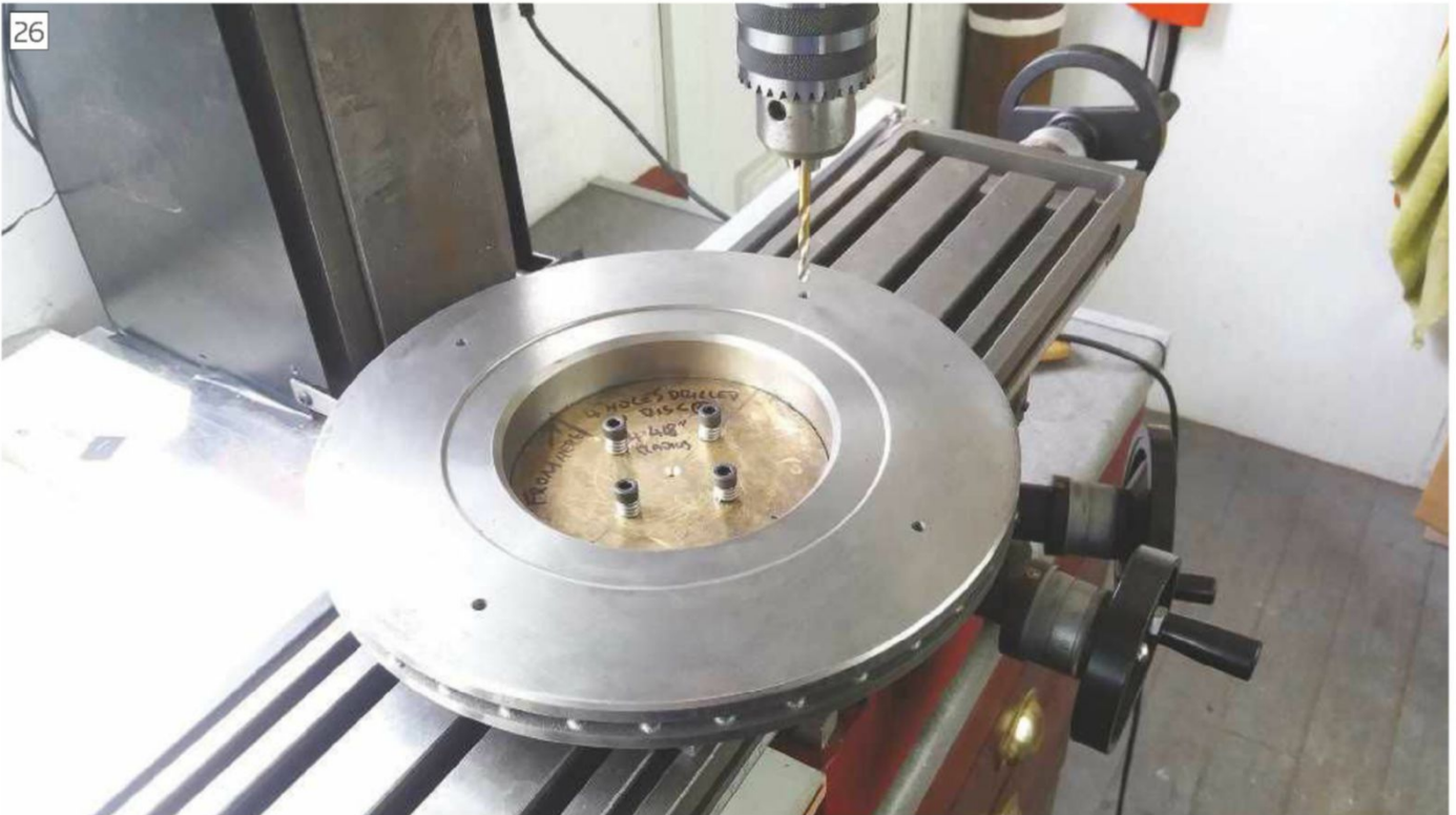
Drill and tap four M6 holes in the face of the disc
