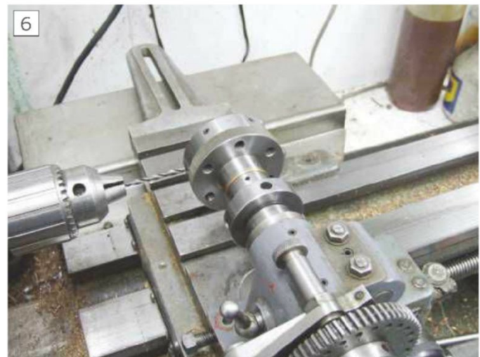
Drilling the turret body at the index positions (posed)
