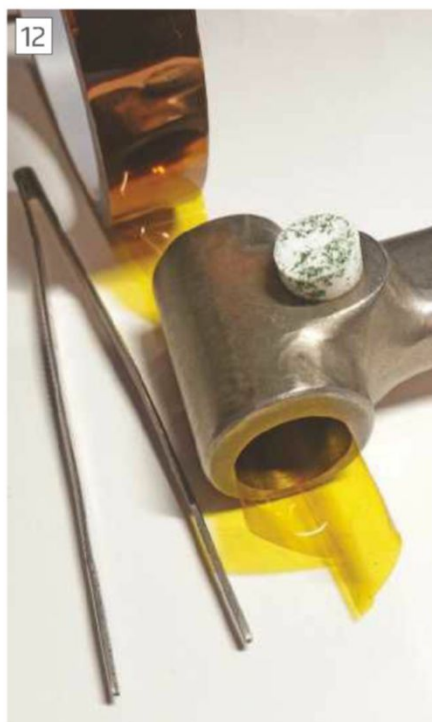
Internal bores are covered with Kapton tape trimmed flush.
