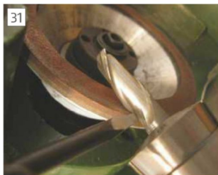
Grinding is achieved by rotating the cutter counter clockwise against the finger rest starting this in the root flute and pulling towards you at the same time.
