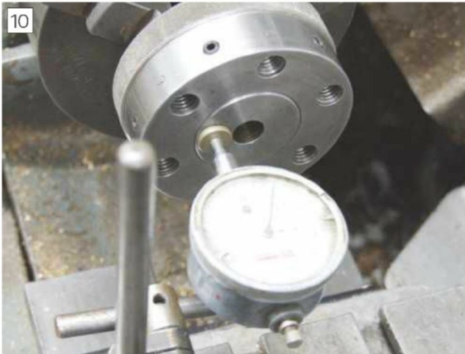
Measuring the turret body and indexing boss as an assembly
