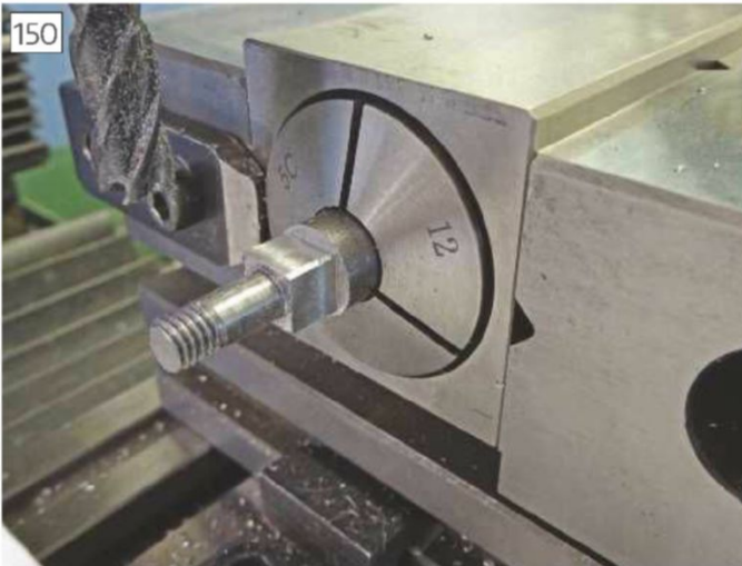
5C block in use showing positioning stop
