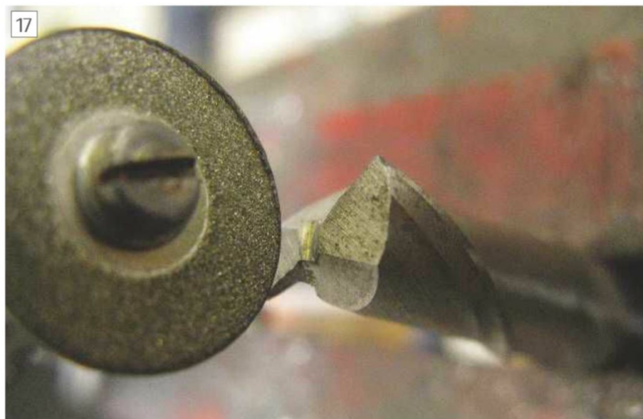
Use a mini disc to enlarge the gash if needed
