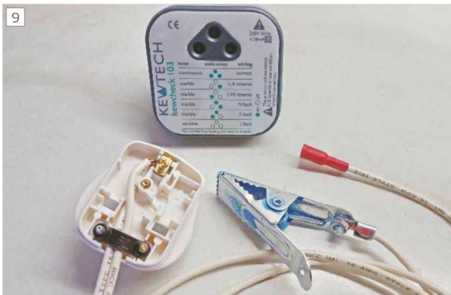
Plug and cables for domestic ground connection.
