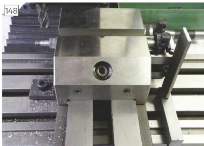
Close-up of square used to index the vee block
