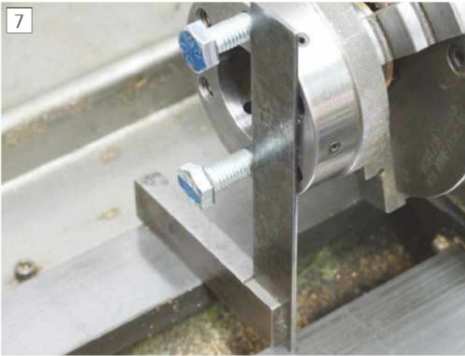
Setting the turret body in the VDH ready for number stamping (posed)
