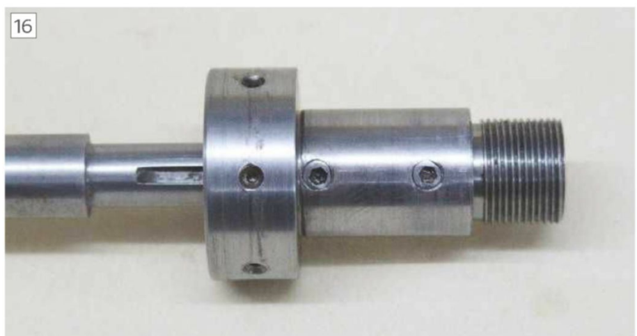
The peg keys have now been fitted to the indexing hub - shown with the stop rod
