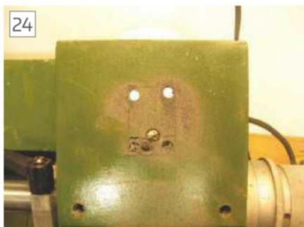
Cutting the toggle switch hole in the front of the machine. Much easier than expected.
