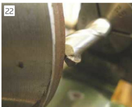
Slacken the penguin stop on the front bar and swing it into contact with the machine frame. Rotate the setting dial until it just starts to move the arm. Add the required 4 turns plus 0.2mm to fully enter the gash to match the 4mm long lip length. Lock the penguin arm to the main bar which itself is unlocked. Move the cutter to the right then back off the penguin screw to zero rotating the main bar, thus adding precisely the required 4mm advancement of the cutter onto the grinding wheel and the gash will be centred on the very corner of the wheel and the short lip is protected. (The final stages are in the text).
