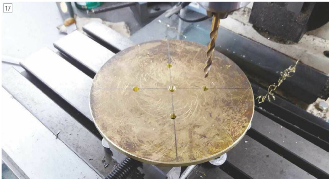
Mark out and drill four 6mm holes
