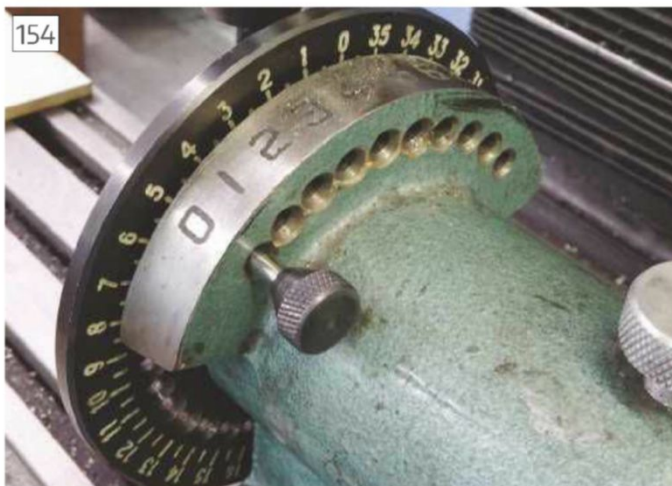
Pin and hole locations in spin indexer at position zero
