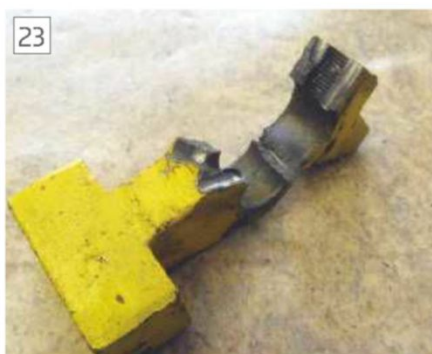
The crude inaccurate and redundant original feed control, drill then split with a chisel.
