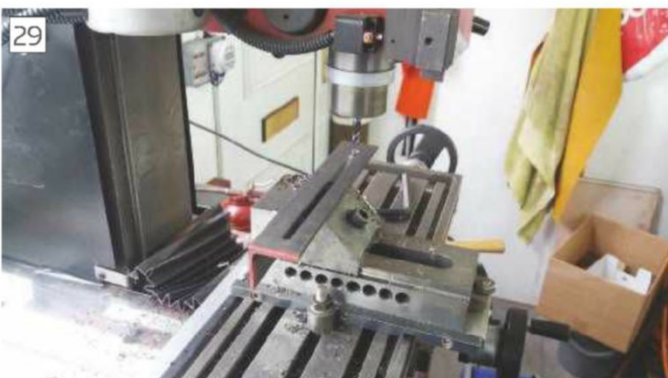
Machining a slot in the stop
