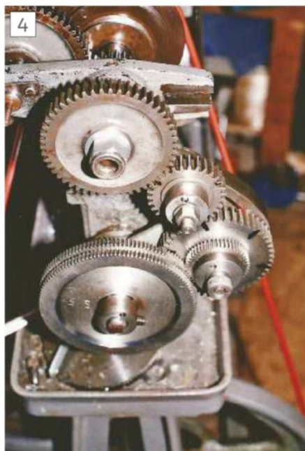
Gear train set up for metric screw cutting.
