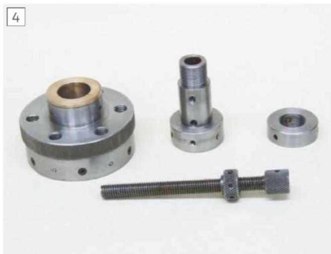
Turret body and parts (bronze bush has already been assembled into the body)
