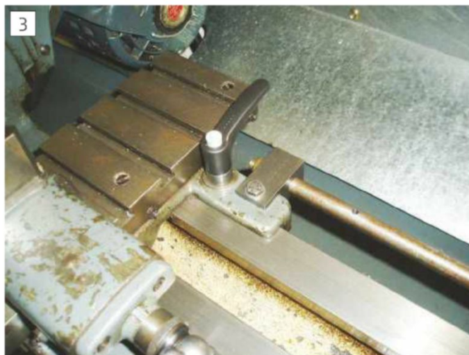
Attachment to the lathe saddle (using an existing tapped hole) (Paul Clark)
