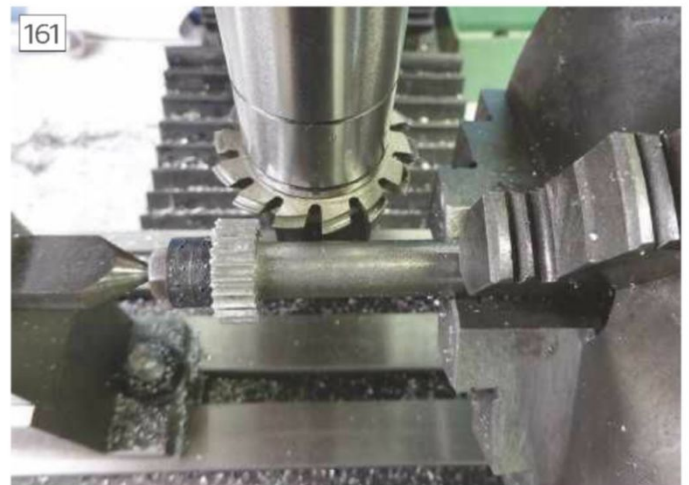
Close up showing cutter clear of work and chuck
