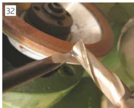
End of the cut. After doing the first edge, switch off, note the feed setting on the main bar then back off, rotate the cutter, to the next edge, switch on, add cut and so on. Because of the geometry of the machine, the grinding will be extended further than the original but will not have flute which is not a problem.
