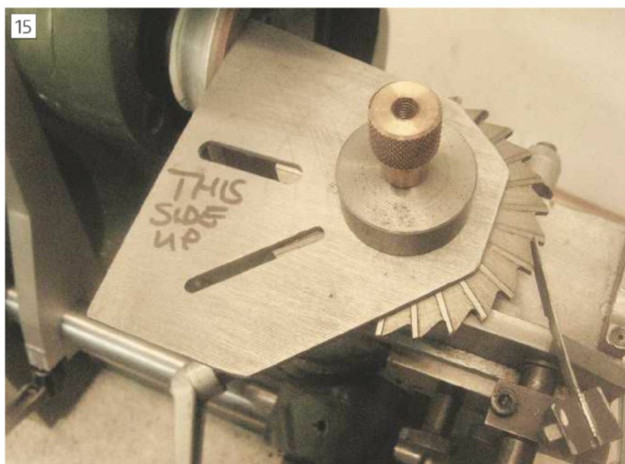
Setting a slitting saw, note the position of the cutter edge in the setting window and the pressure on the detent causing it to bend.
