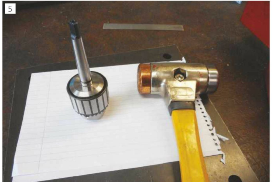
Arbour and chuck are wrung together and placed on solid surface before the arbour is driven home.
