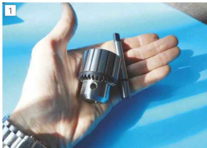
Chuck and arbour arrive in two pieces, ready to be assembled.
