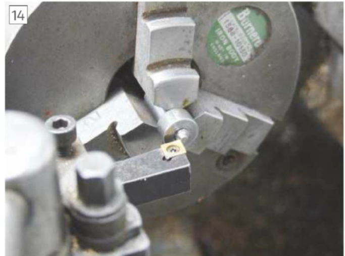
Machining a peg key in the special holder
