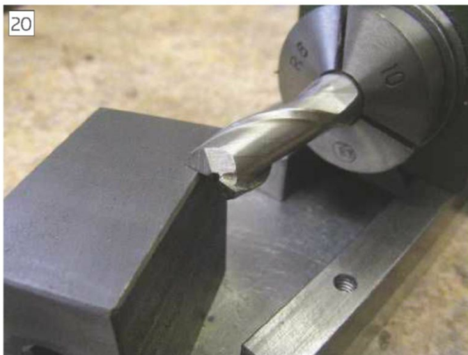
Using the setting block to set the cutting lip level. On some end mills the cutting lips are not radial so then just get the gap between the edge and block parallel. Lock the spindle, tighten the collet and finally zero the degree scale on the work head for "indexing".
