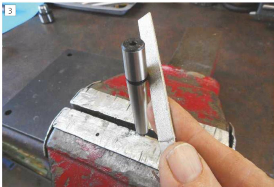
Great care must be taken to remove burrs from the taper ends.
