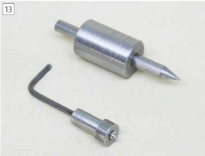
The holder for machining the peg keys and the special centre punch
