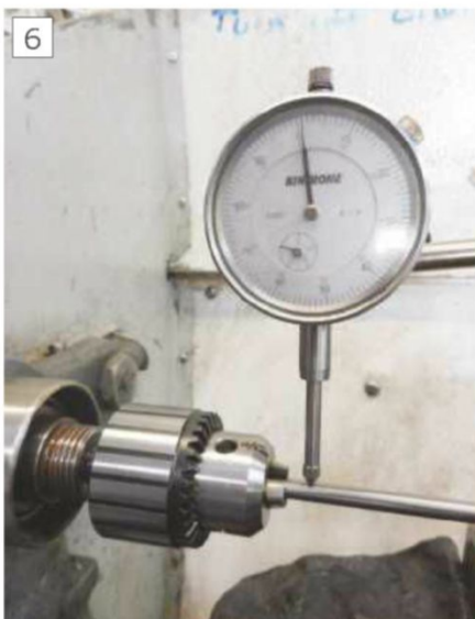
Test piece runout is measured at .001", a good result.
