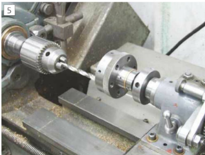
Drilling the turret body for length screws (posed)
