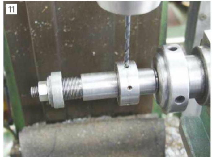
Spotting the index positions in the indexing hub (posed)
