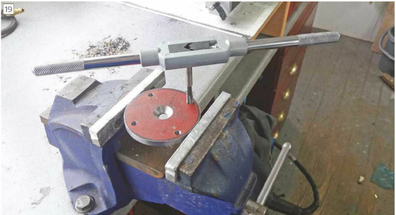
Drill and tap the steel disc
