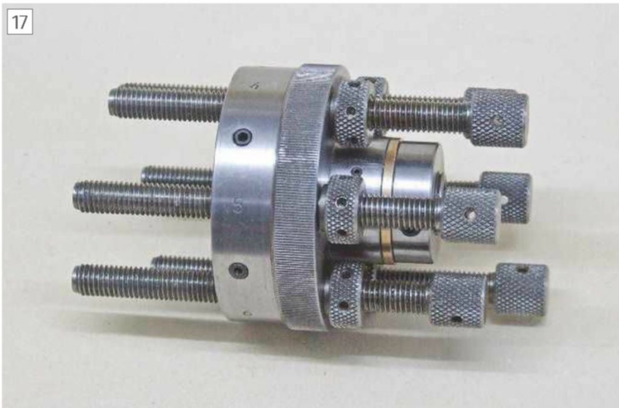
The turret assembly complete and ready for fitting
