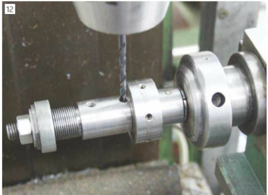
Drilling tapping size for the peg keys (posed)
