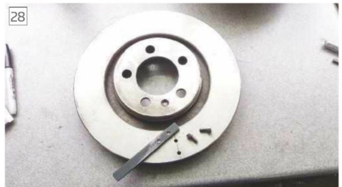
Drill and tap for the stop bar
