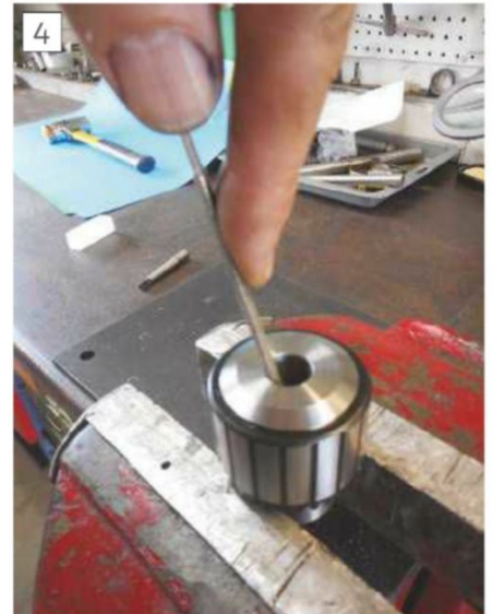
A round file works best to deburr the end of the chuck taper.
