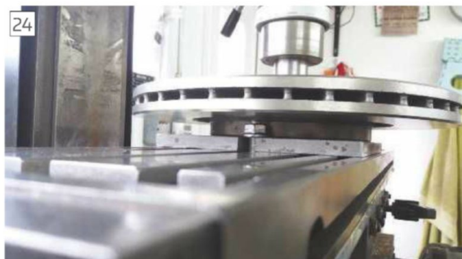
Tighten the base plate mounting bolts
