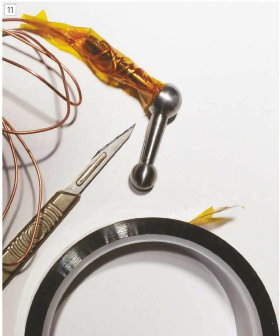
Kapton tape is used to mask threads.
