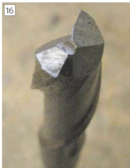
The start of the grinding process, an obviously blunt and sad 10mm slot drill
