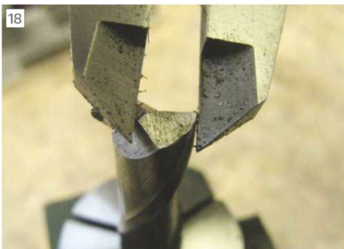
With digital callipers, measure the length of the long lip to the centre of the gash and make a note of this. Zero the callipers. Gosh they didn't look that dirty!
