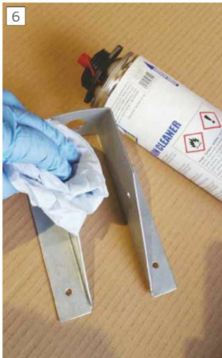
Wiping down with acetone removes all traces of oil.
