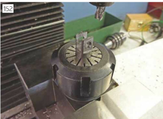
Milling a slot central and at right angles to hole
