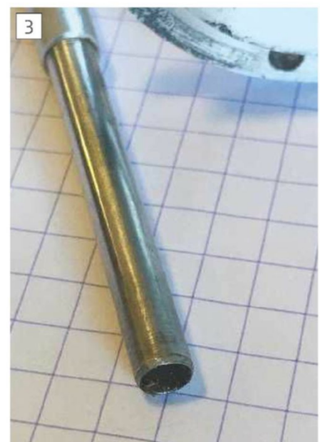
The shaft after being cleaned up. The thin walls around the centre drilling are clearly visible
