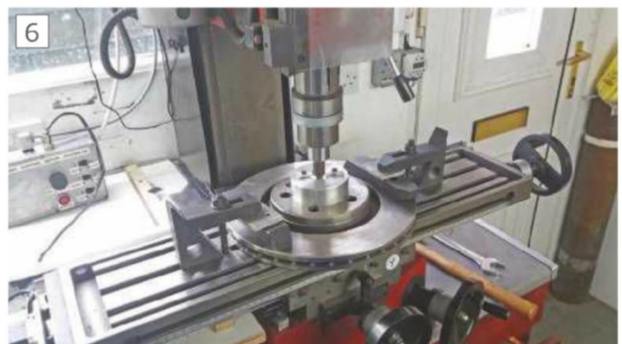
Centring in the mill
