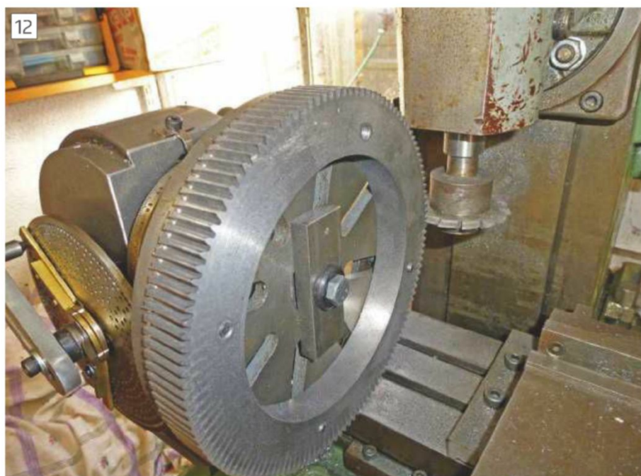
Cutting the 127T gear for the Imperial screw cutting attachment.
