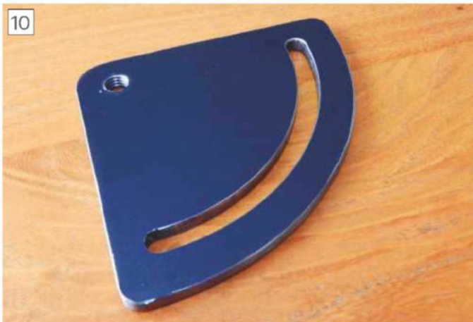
Protractor plate to set the grinder in a fixed angular position
