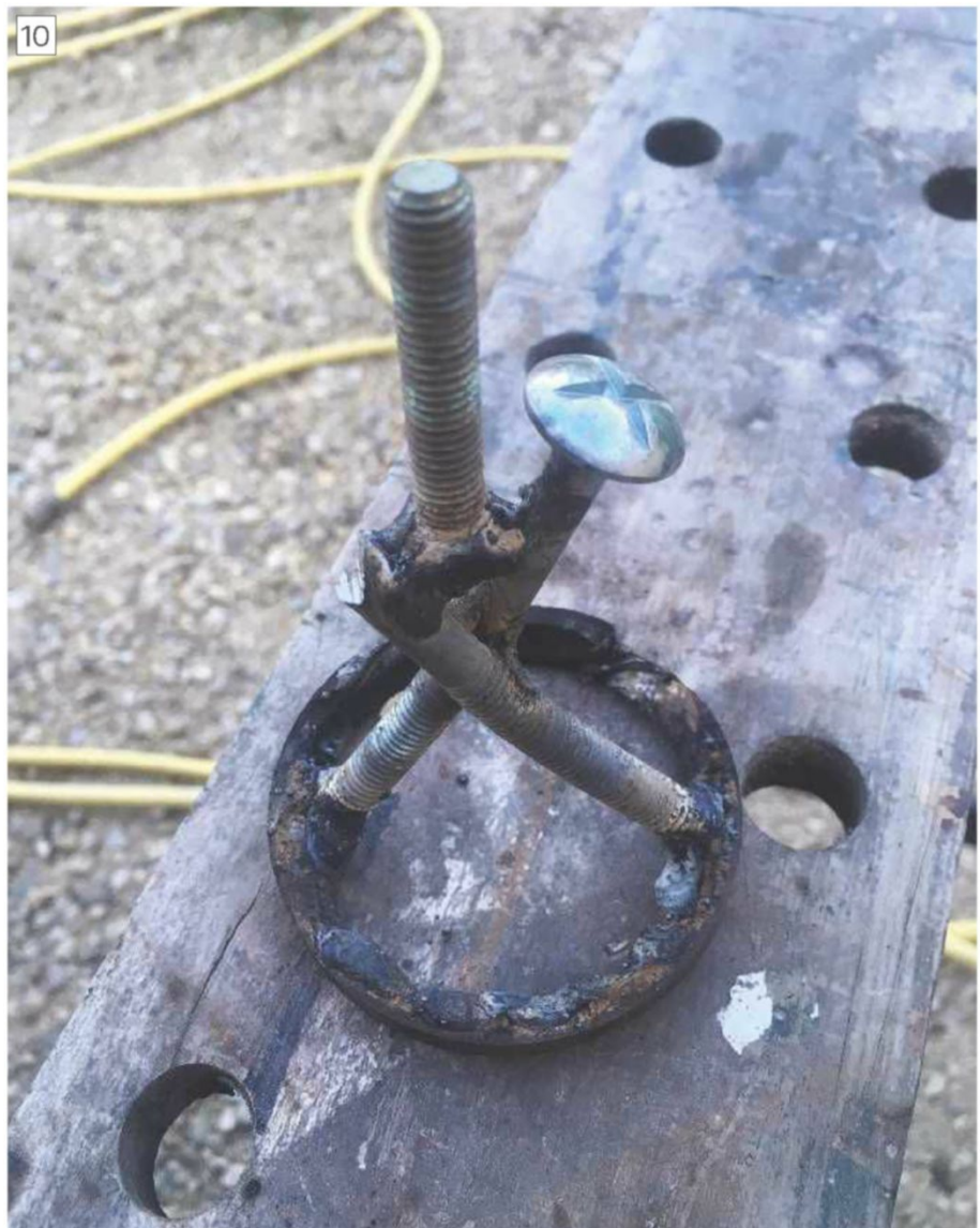
Some Dremel work is visible upper right where I was too enthusiastic and welded bearing to drum. The studding for the slide hammer can be seen as well
