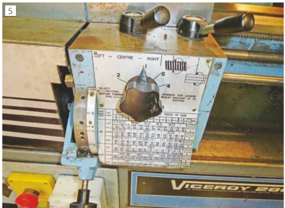
Screw cutting gearbox and its controls.
