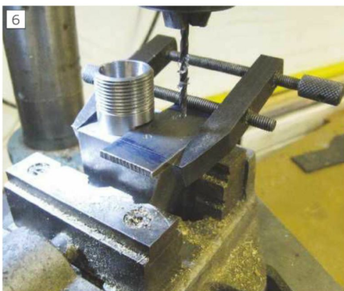
The setup for fixing the indexing plate, drill both pieces tapping size then open up clearance, 4mm deep to the drill lip without unclamping.
