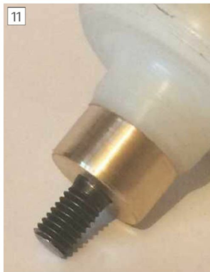
Unthreaded space on 8mm attachment screw.
