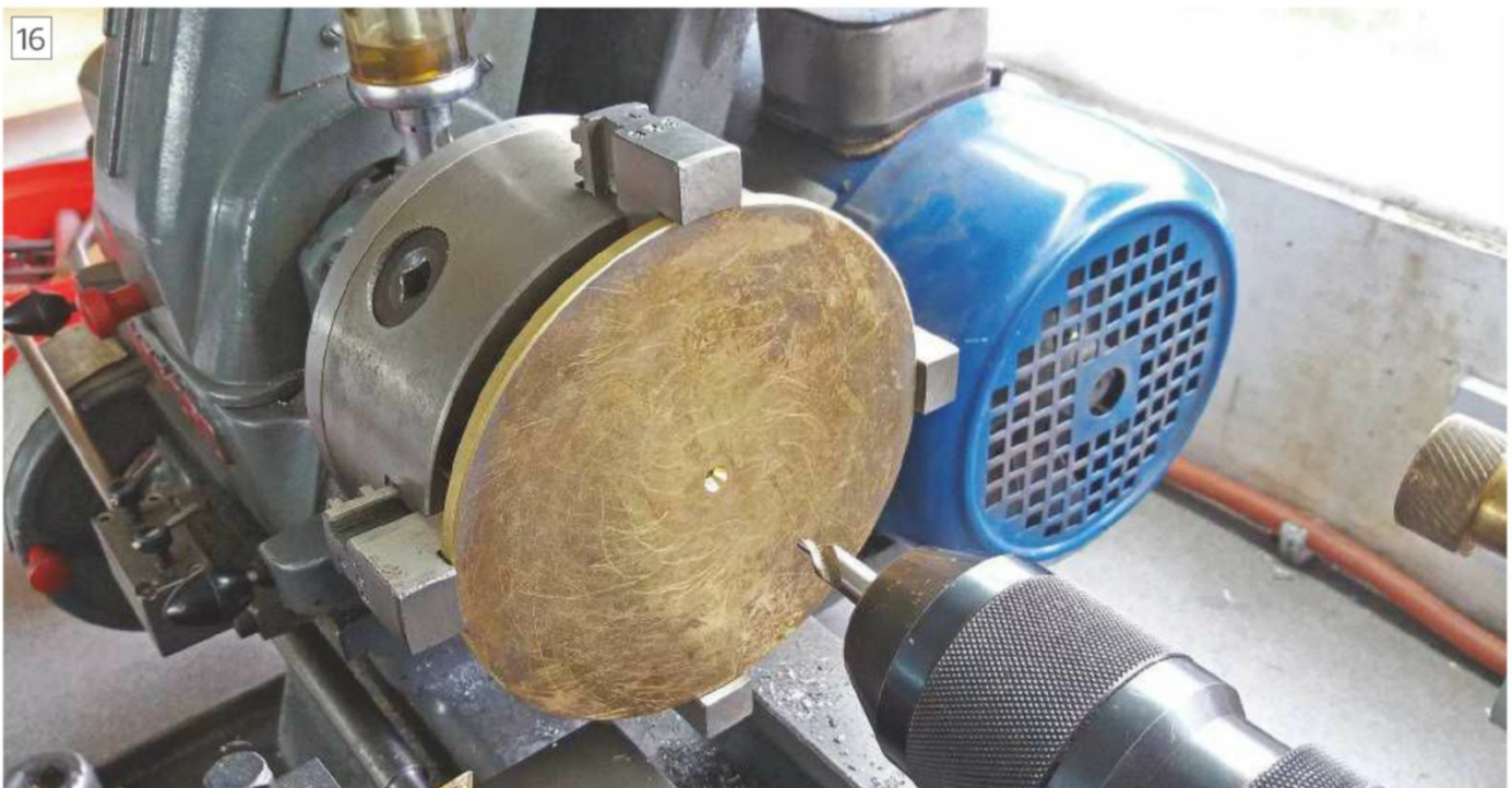
Centre drilling the brass plate
