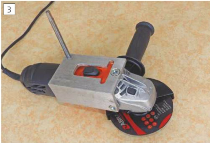
Saber' angle grinder with mounting cradle
