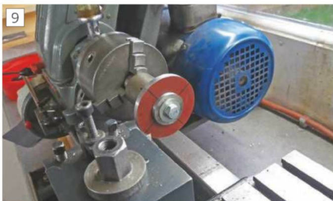
Turning the 6mm steel disc to size
