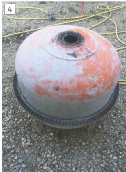
Mixer drum – the entire weight is born by 2 bearings about 70mm or so apart
