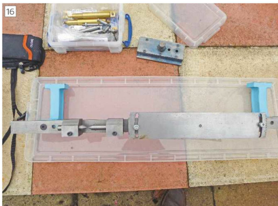
The complete taper turning and copying attachment awaiting fitting to the lathe.
