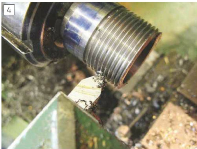
Screw cutting diameter 25 X 1.5mm
