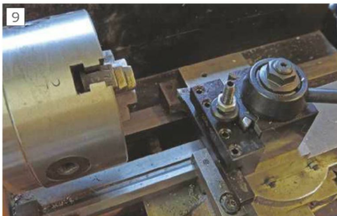
Model 000 toolpost fitted to a mini lathe (the lathe has a 100mm chuck fitted, which makes the QCTP look smaller than it really is).
