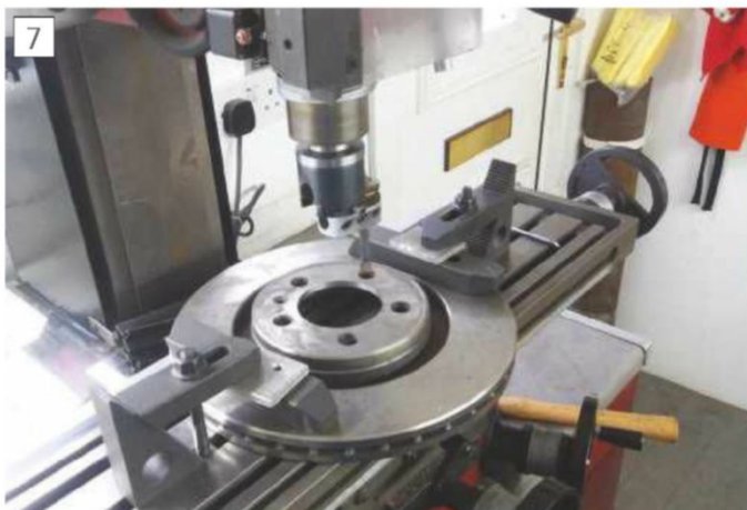
Removing the chamfer with a boring head
