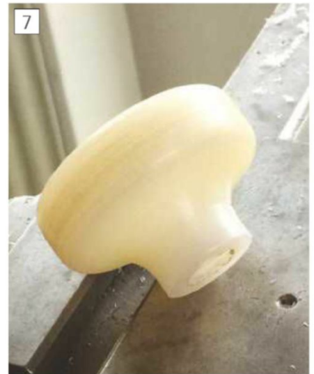
Completed profile, prior to fitting of central bush.
