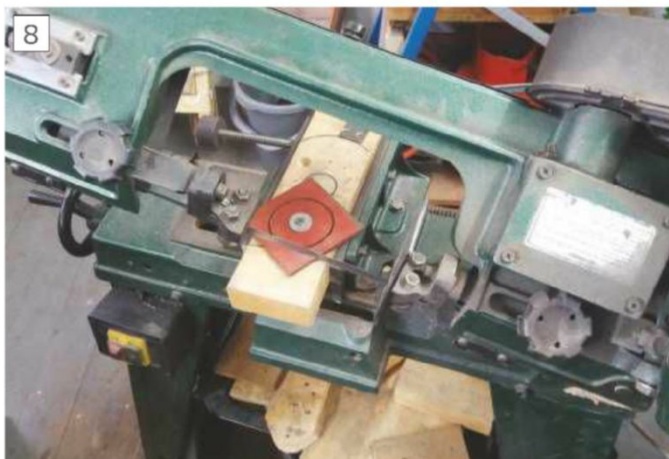
Rough cutting the 6mm steel disc
