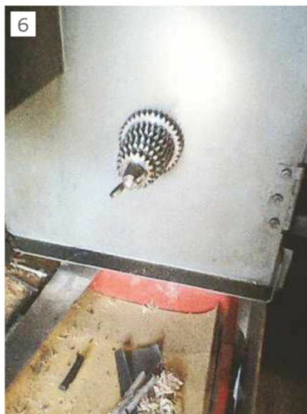
Spare screw cutting gears stored inside gear cover.
