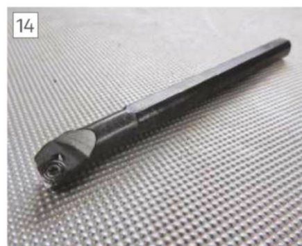
Inserted tip boring bar with flats
