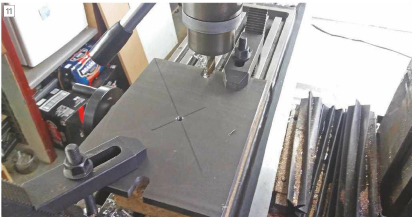
Drill and tap and slot the base plate
