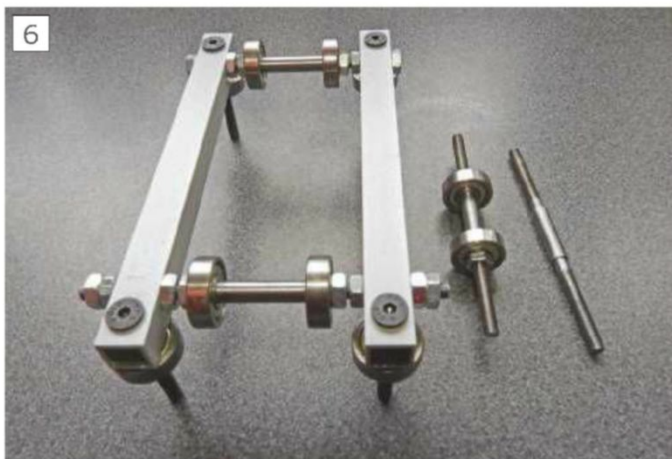
Constructing the sliding carriage
