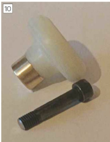
Finished with bush and M8 screw.
