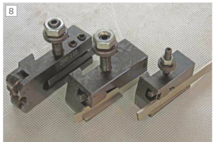
Special purpose QCTP toolholders, a knurling/toolholding combined holder and 000 and 100 parting tool holders
