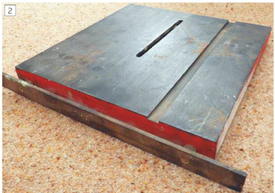
Original cast iron table 305 x 290mm
