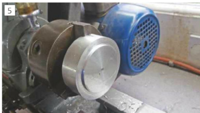
Turn and centre drill a scrap of aluminium
