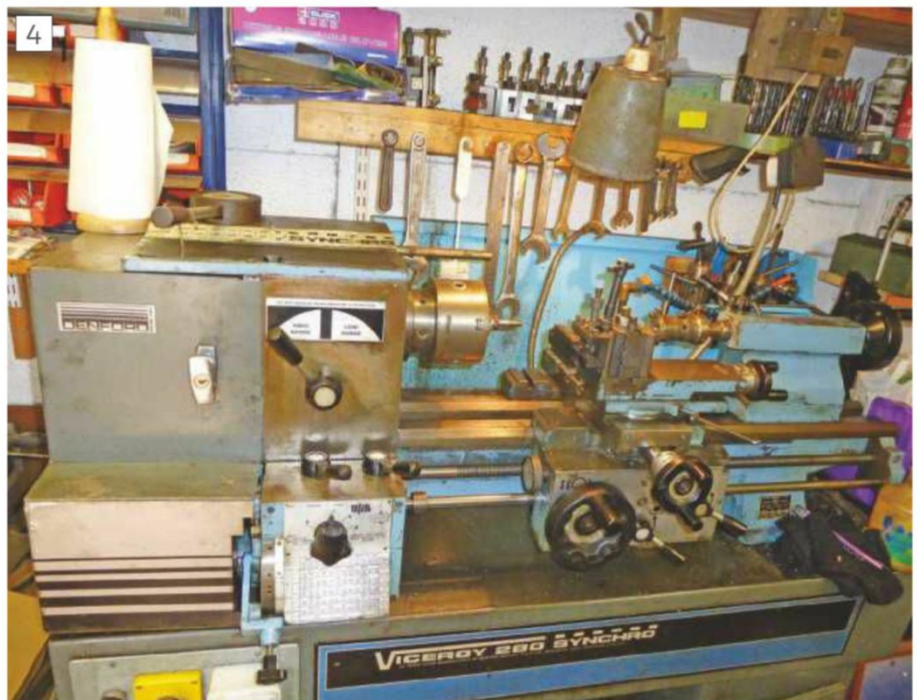
The Denford 280 Synchro lathe as installed in my workshop.
