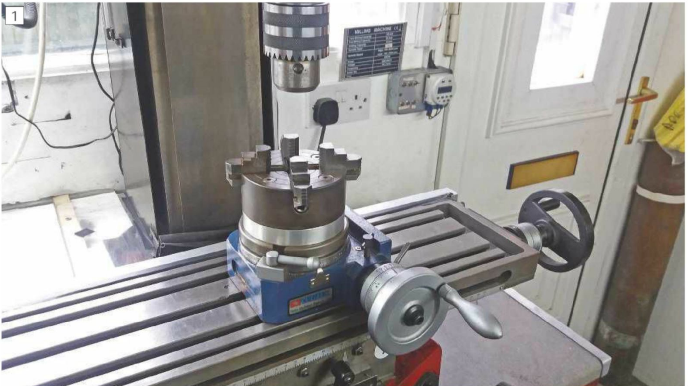
My 4" rotary table with 4-jaw independent chuck fitted
