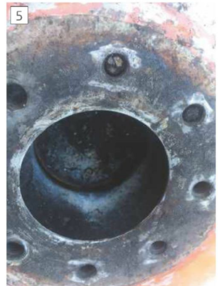
Less than simple access – the out of focus ring is the edge of the remains of the bearing outer
