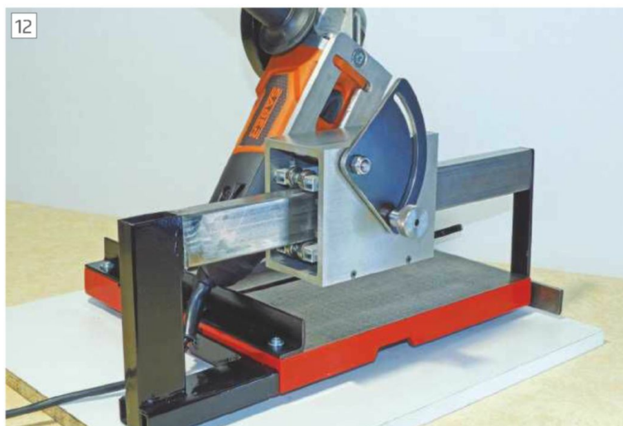
The protractor plate and grinder in raised position to allow on/off switch operation
