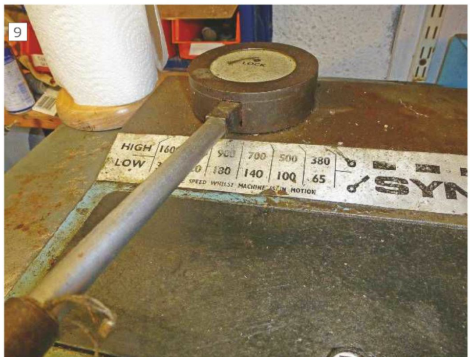
Headstock speed control. The lever controls the variable speed pullies and can only be moved when the lathe is running.
