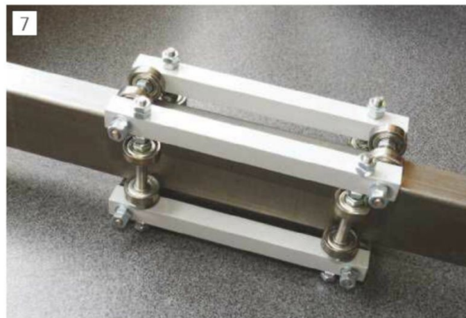
Finished sliding carriage assembly
