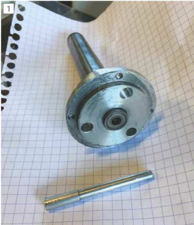
Bearing partly returned to blind hole
