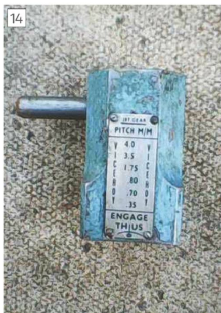
Alternative Thread Dial Indicator fitted with 28T gear cut by myself.
