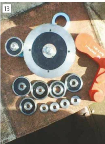
The completed imperial screw cutting attachment with all the gears. The red item is the foundry pattern for the quadrant.
