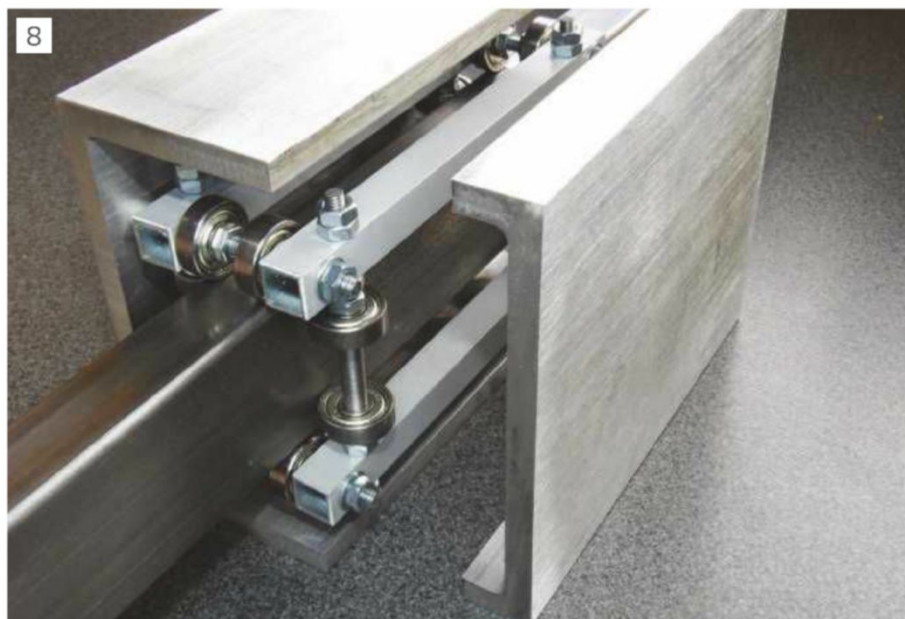
Sliding carriage enclosure
