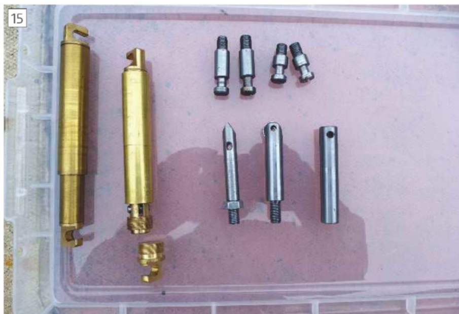
Spring housings and stylus for taper turning and copying attachment.
