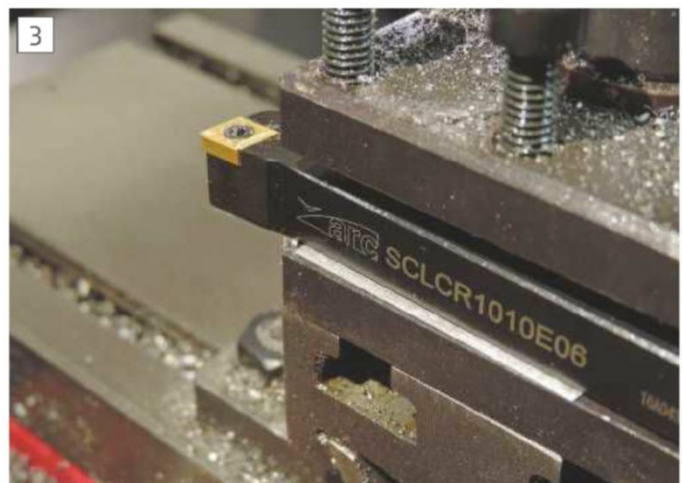
Using packing strips to set a tool at centre height
