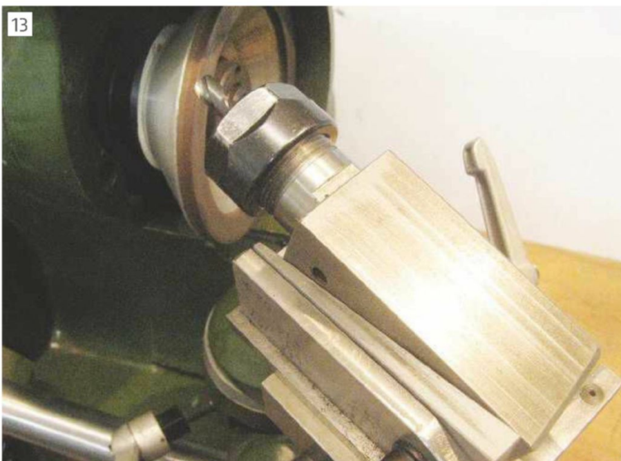
Using the wedge, here the block sits on its angled face.
