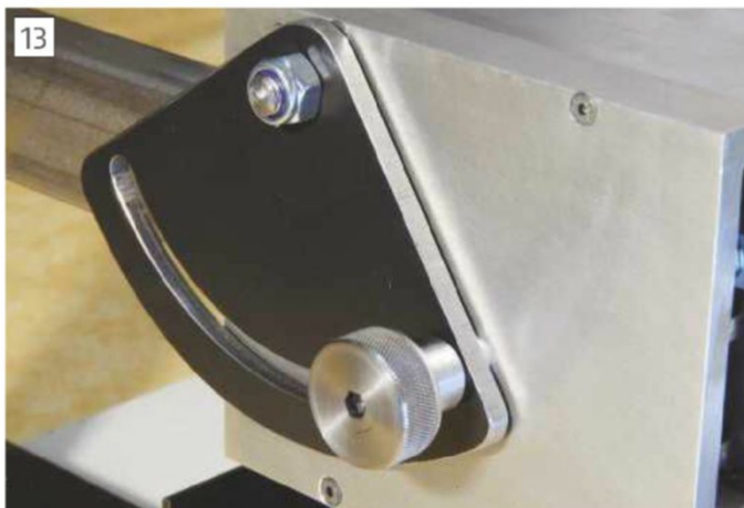
Protractor locking mechanism
