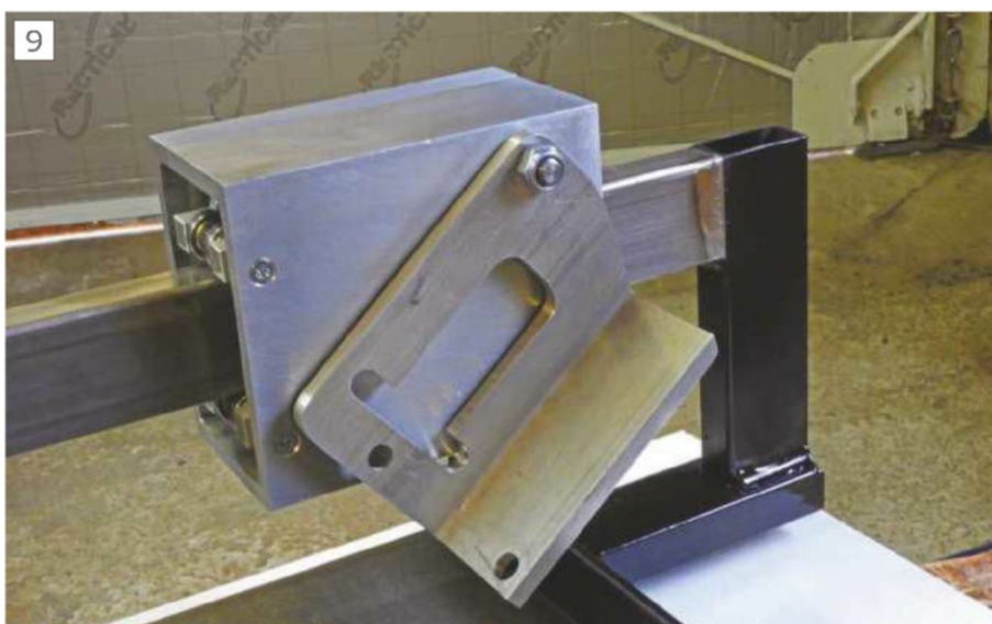
Tilting mechanism fixed to the enclosure
