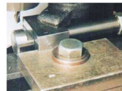
Set up for machining the lock screw using the parts illustrated in SK1.
