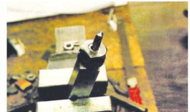
5. A sharpened drill in the ER20 spring collet.
