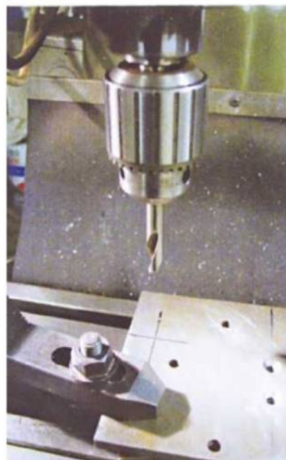
Initial marking out by felt tip pen although the c/s hole spacing was accurately controlled.
