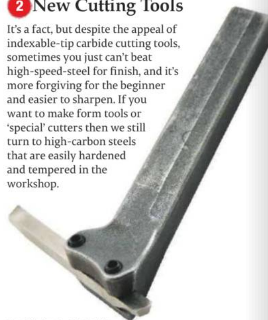
The Wimberley Toolholder, combining HSS and an innovative holder.
