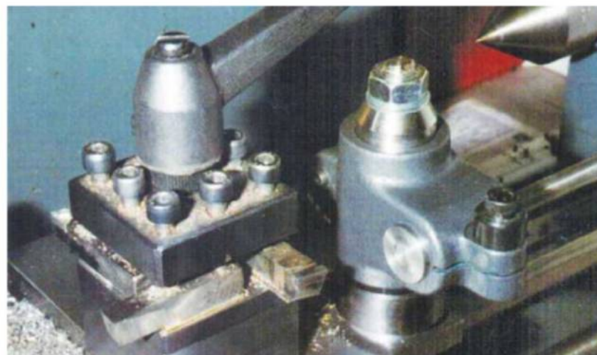
Four-way toolpost and boring bar holder fitted to fixture.
