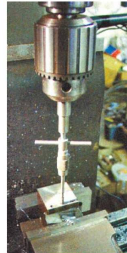
Tapping using a pump centre for alignment.
