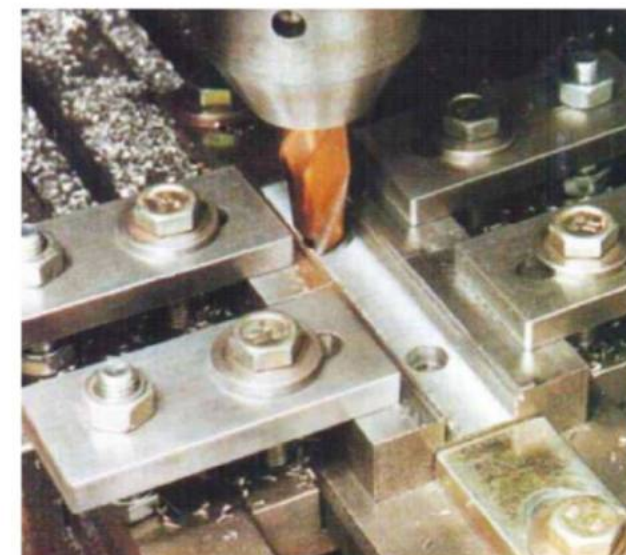
Preliminary work on the dovetails.
