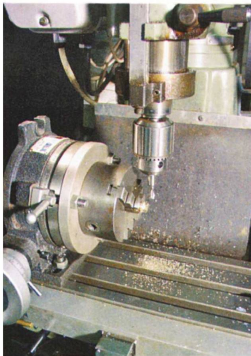
Set up using rotary table to mill hex on pivot post.
