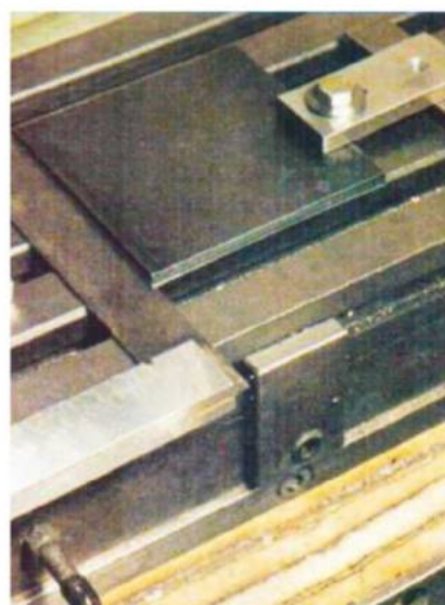
Positioning the table in preparation for machining its edges.
