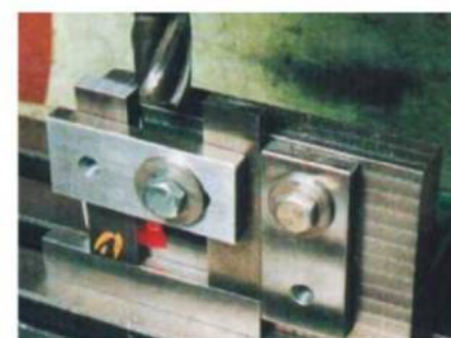
Machining the ends of the side arms. Some second thoughts obviously resulted in the setup being changed between photos 11 and 12.
