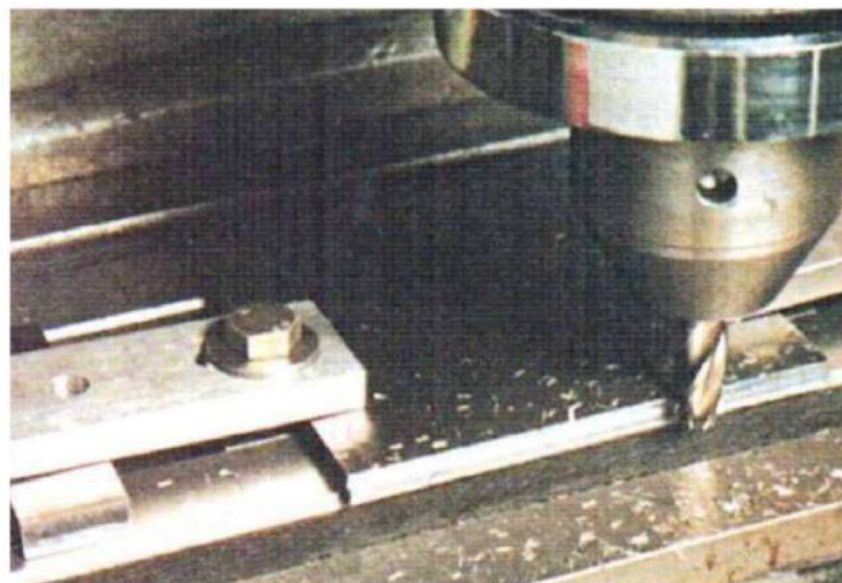
Machining the table's edges.
