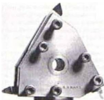
The Lammas Three Way toolpost loaded with raked tools for cutting steel and aluminium.
