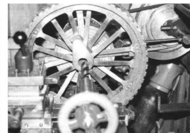
Typical use, a hub for a traction engine hind wheel (one jaw reversed). 380mm wheel being bored true. An extended jaw is visible between the two uppermost spokes.
