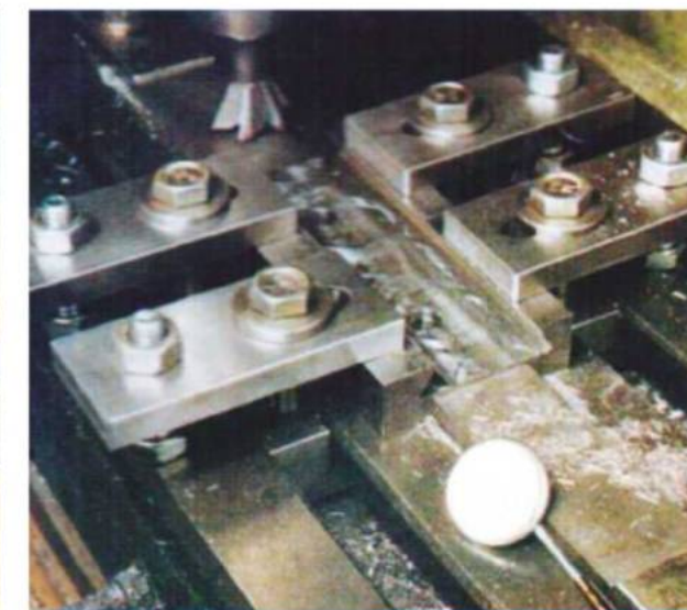
Finishing the dovetails in the slide swivel pieces.
