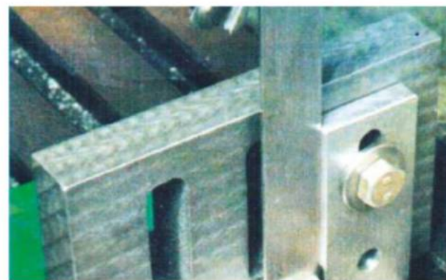
Setting up a support for machining the side arms.
