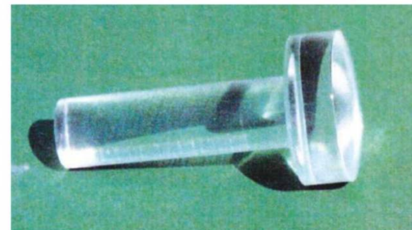
The magnifying lens for the tool. Made from acrylic, it is a simple turning exercise; shank must be a good sliding fit in the body and the large diameter rounded at the end to provide magnification.
