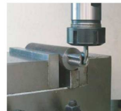
Milling the slot in the tool holder.
