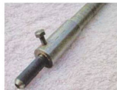
A sharpened tool from silver steel.
