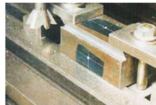
Cutting the dovetails in the lower slide.
