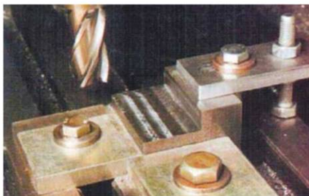
Machining the lower arm spacer. With only one clamp being used the supports are essential for added security whilst machining.
