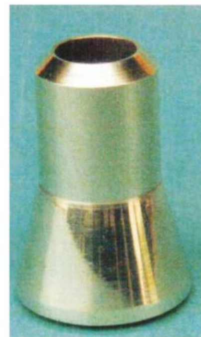
The body of the optical centre punch; this one is from aluminium but almost any material will do.
