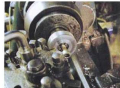
The spigot located on an expanding mandrel.
