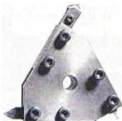
Another similar toolpost loaded with zero-rake tools for cast iron and brass.
