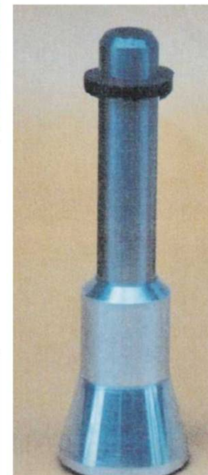
When the body is in the correct position the magnifier is removed and replaced by the centre punch.
