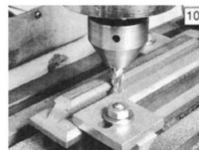
Machining width of top to final dimensions.
