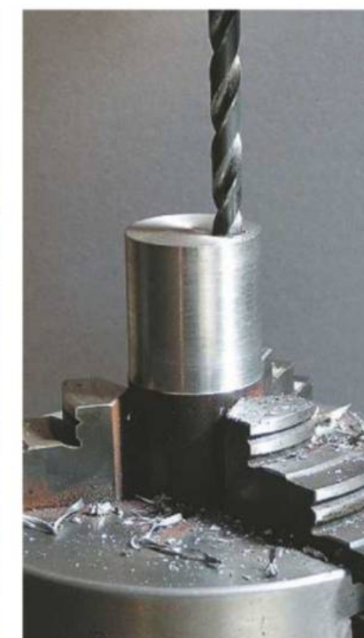
Drilling and tapping the offset hole.
