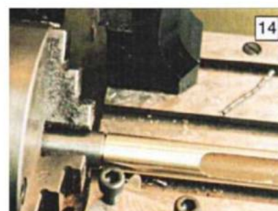
The vial tube mounted on a tapered stub mandrel.
