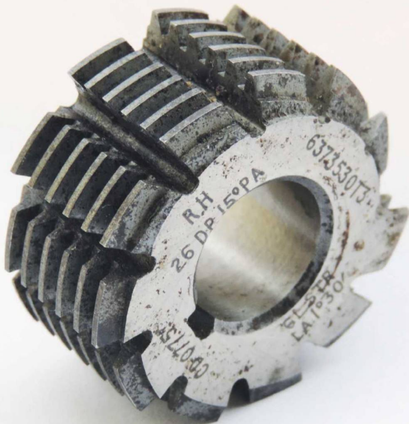
This hob is 26DP, but has the rather unusual pressure angle of 15 degrees, rather than the more usual 14.5 degrees.
