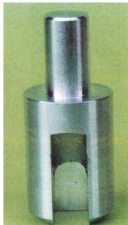
This frontal view of the body shows the two angles required accurately to position the lens. The angle value of the body itself is not critical, provided, of course, that it is matched precisely by that of the lens.
