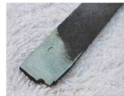
A form tool made from gauge plate.
