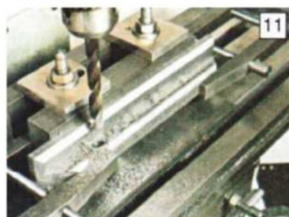
Drilling holes in central web after first positioning them with a centre drill.
