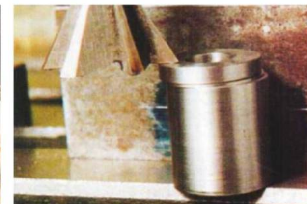
Setting the depth of dovetail using distance pieces.
