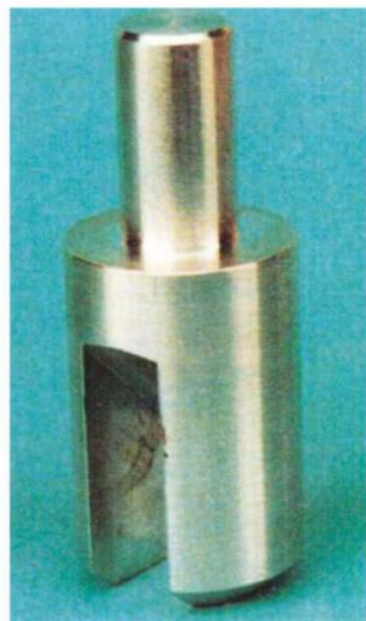
The body of the centre-finder showing how the slot has been milled out to accept the lens.
