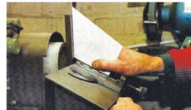
2. Setting the tip angle by tilting the table.
