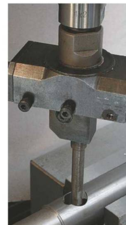
Boring the hole for the tool holder.
