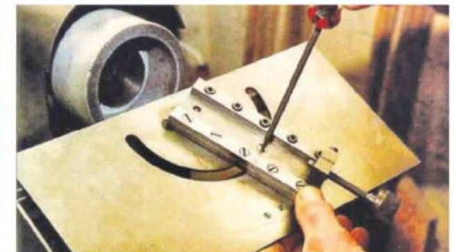
3. The angle of the slide creates the clearance.
