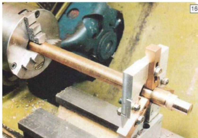
Making the vial tube ends; the fixed steady is being used to minimise scrap.
