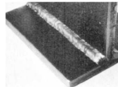
Above A typical example of a good quality weld where the electrode has made a single pass.
