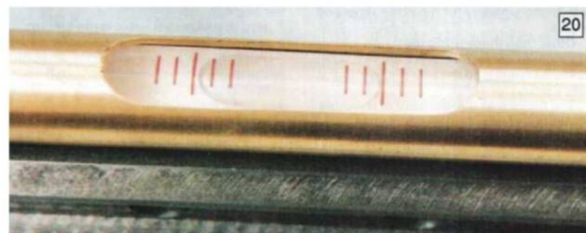
The vial calibration; each line is about 2mm apart.
