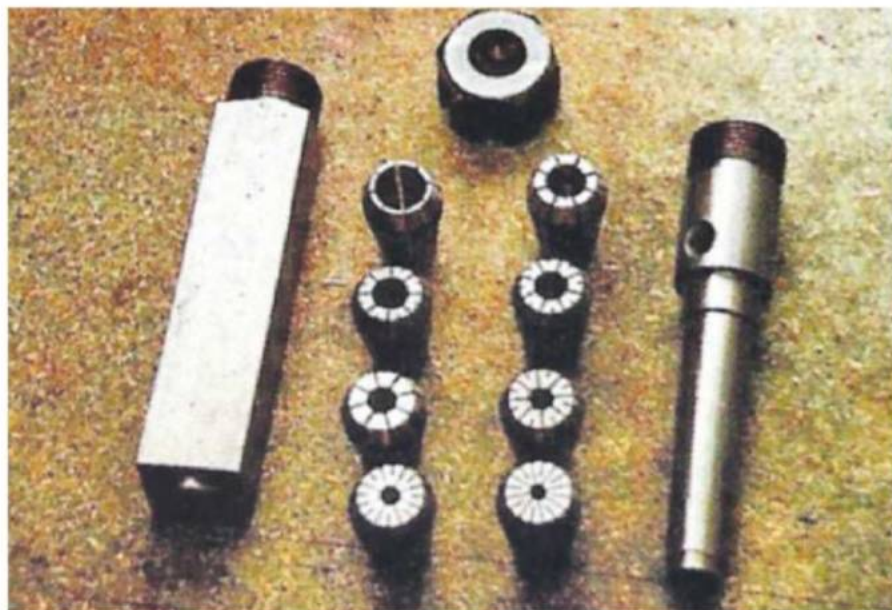
Right 1. ER20 spring collets, normally used in the Morse taper chuck (right) can be fitted to the square holder (left) and used to hold a wide range of drill diameters.
