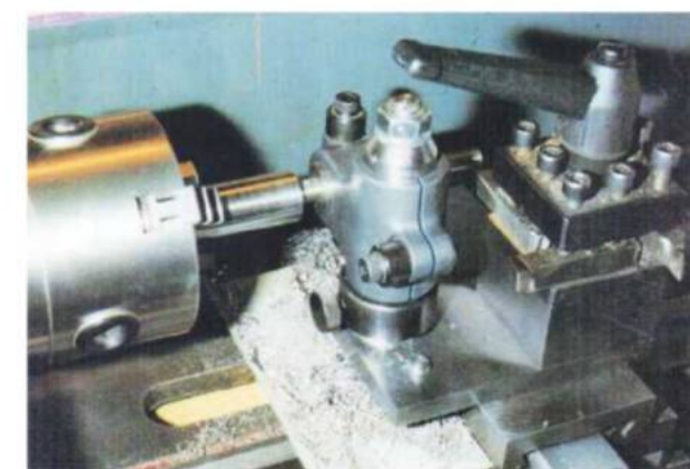
Showing the fixture rotated 180 degrees to present the boring bar.
