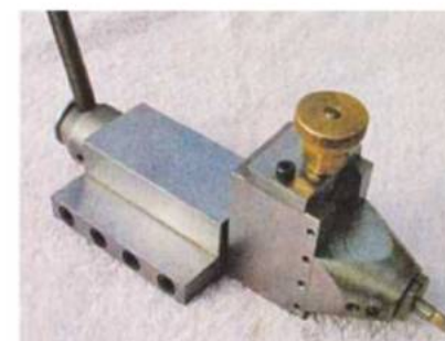
A ball turning tool based on that marketed by Hemingway kits.
