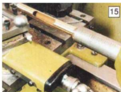
Machining the vial tube; note how this is supported between stub mandrel and tailstock centre.
