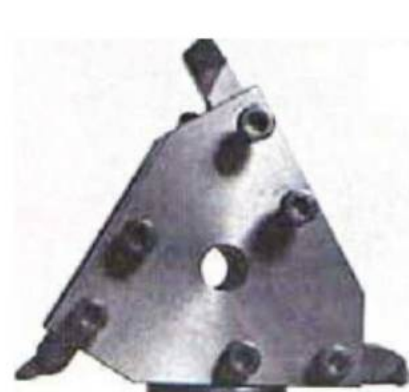
This version is loaded with a set of tools for right hand cutting.
