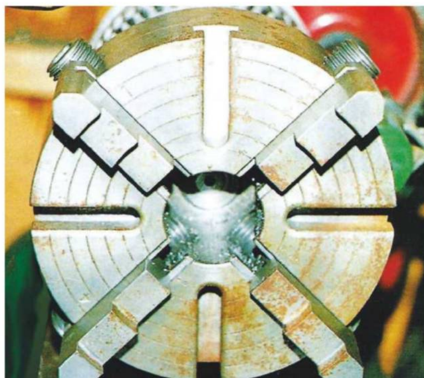
Jaw and screw started in body.
