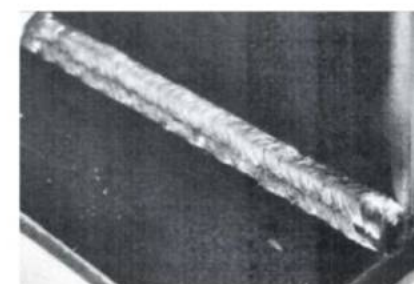
Above A typical weld with three passes of the electrode.
