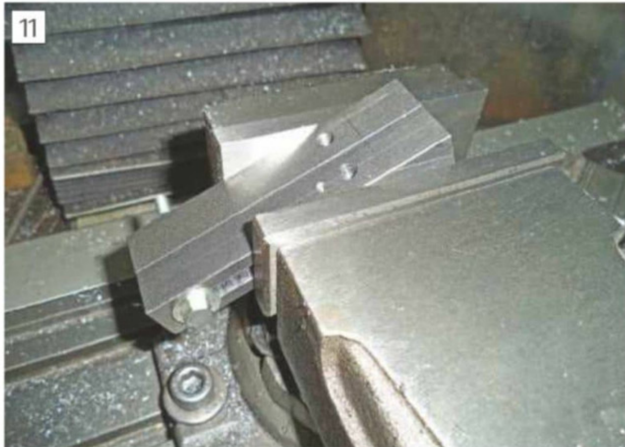
Milling the chamfer on the jaws
