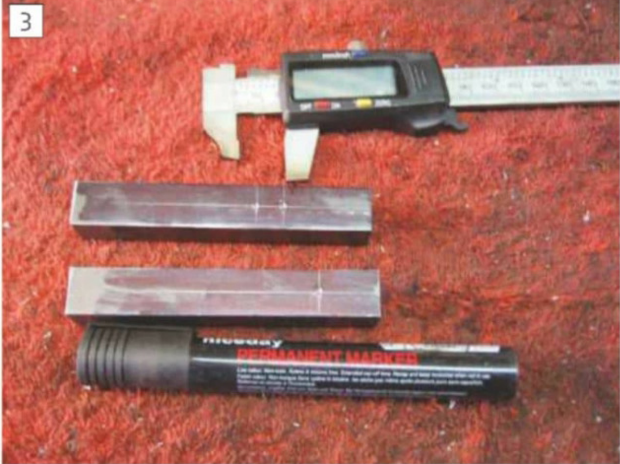
Marking out using odd leg digital calipers
