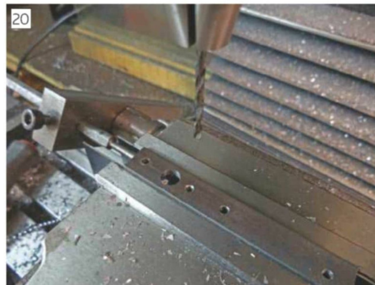
Drilling the keep
