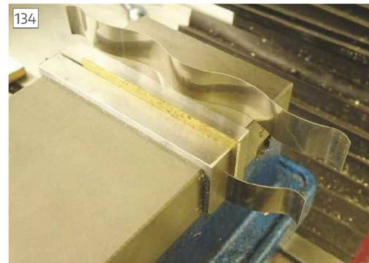
Wavy parallel supporting thin work piece
