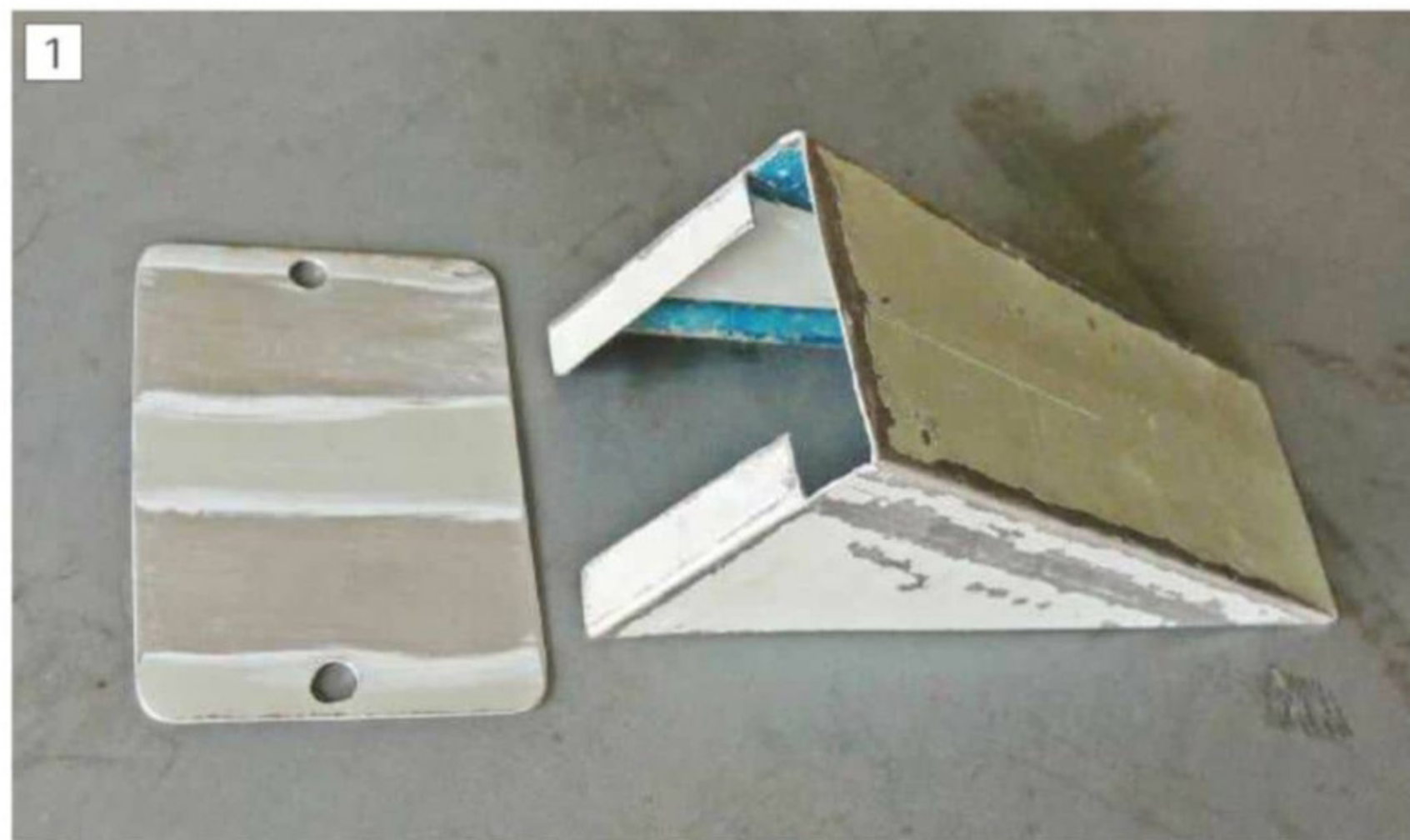
Bracket parts ready for welding.
