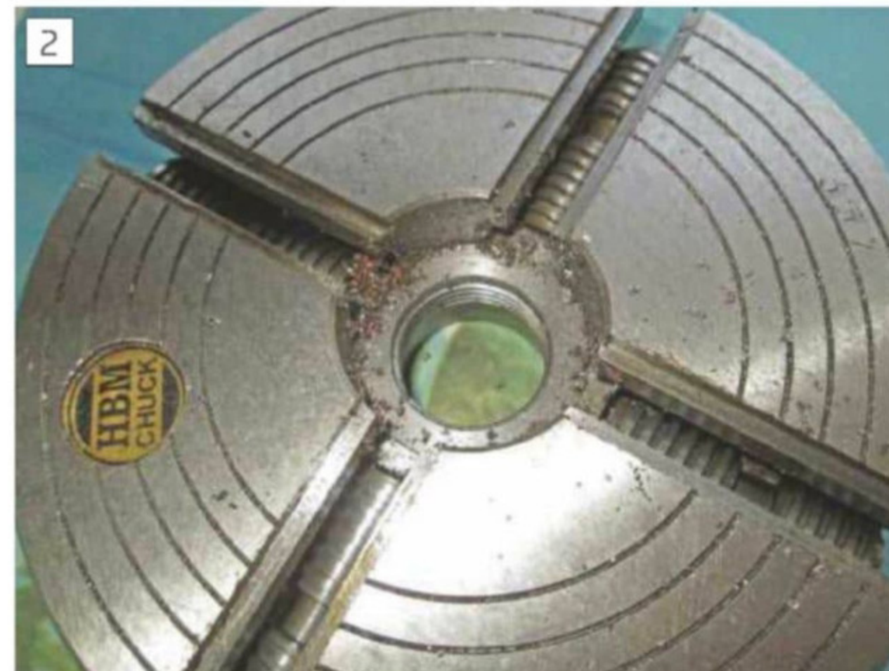
Swarf after removal of the jaws
