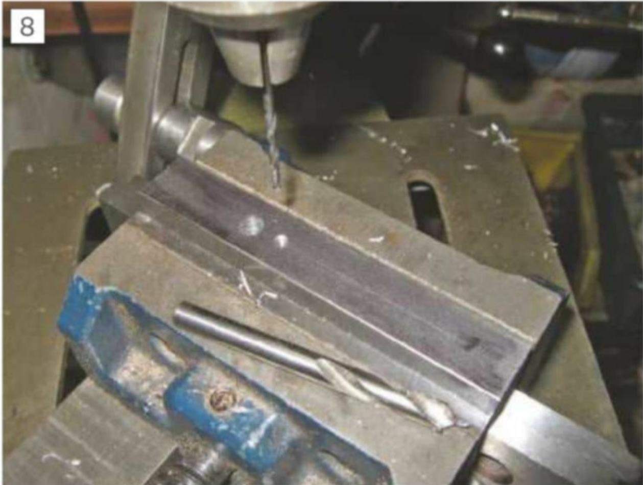
Drilling M2.5 tapping
