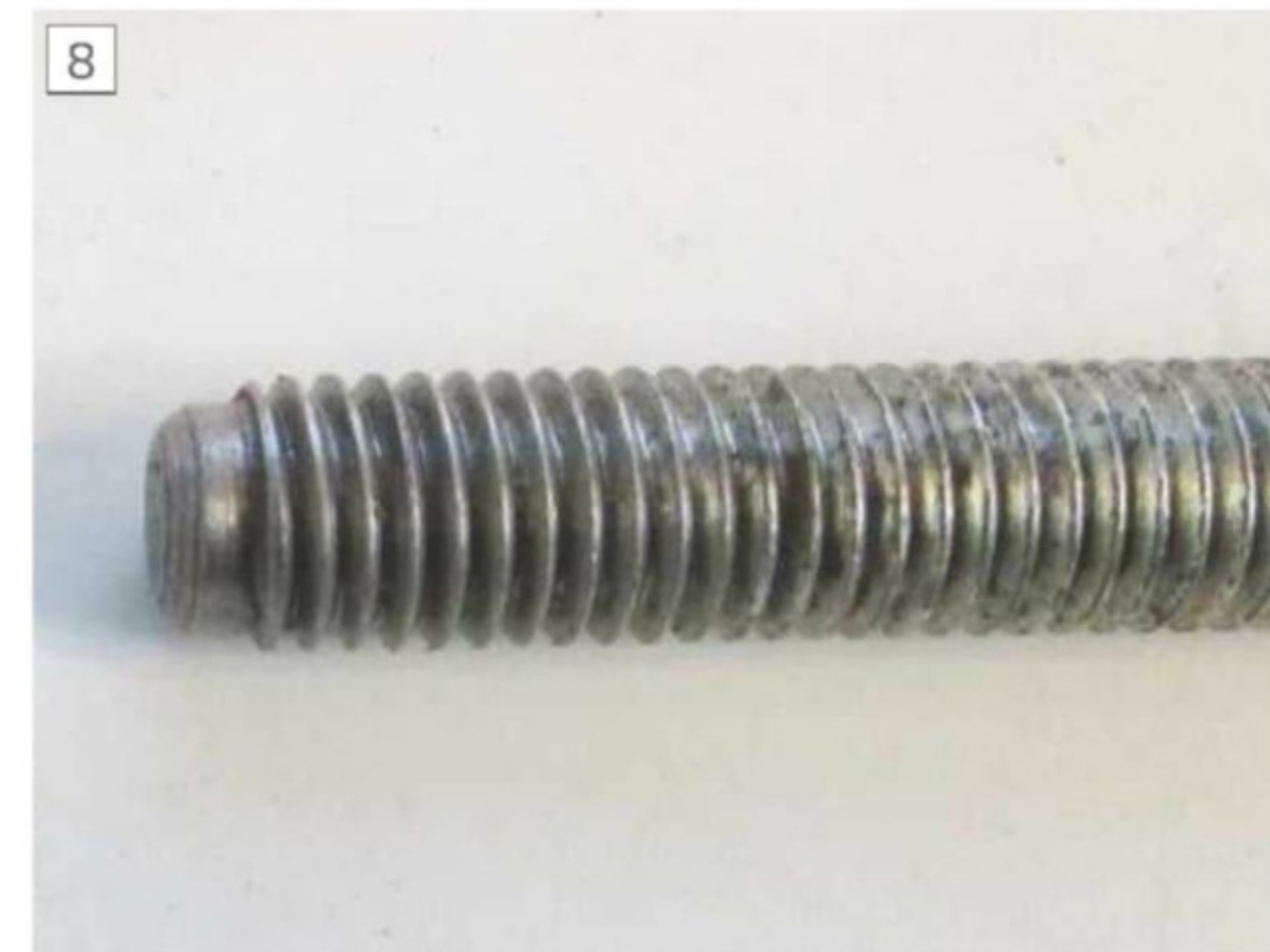
Machined drawbar end to assist location in chuck arbour
