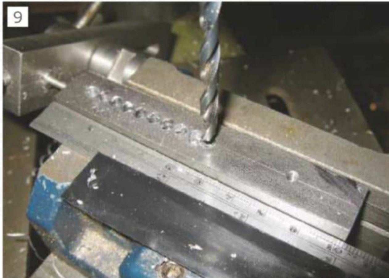
Chain drilling 6mm holes for slot
