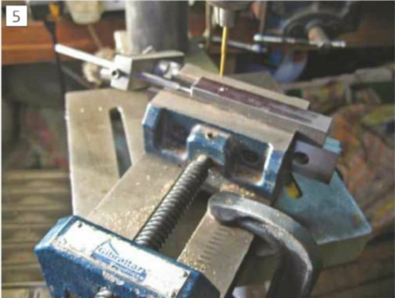
Vice firmly clamped to drill table
