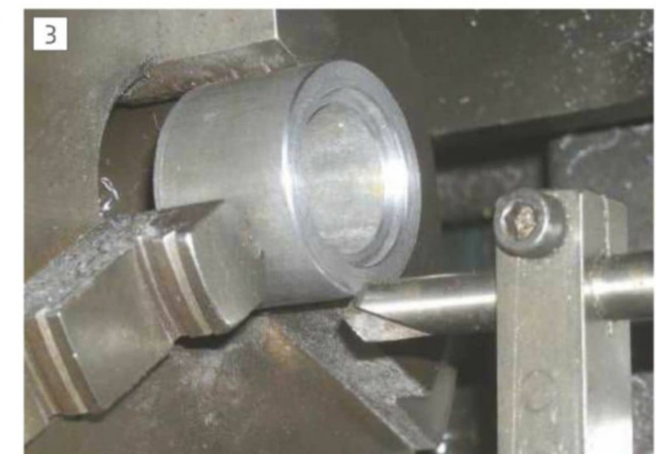
External chamfering with lathe running in reverse
