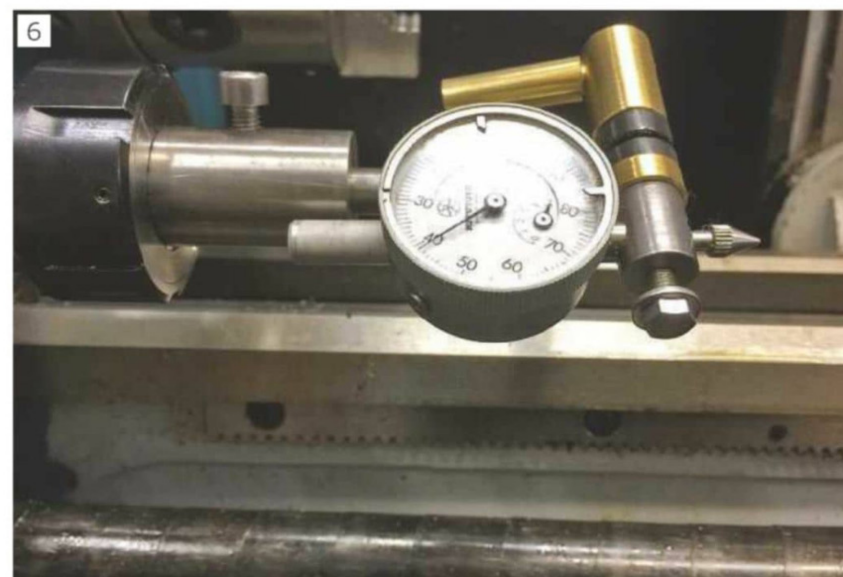
Using a DTI to set the stop.
