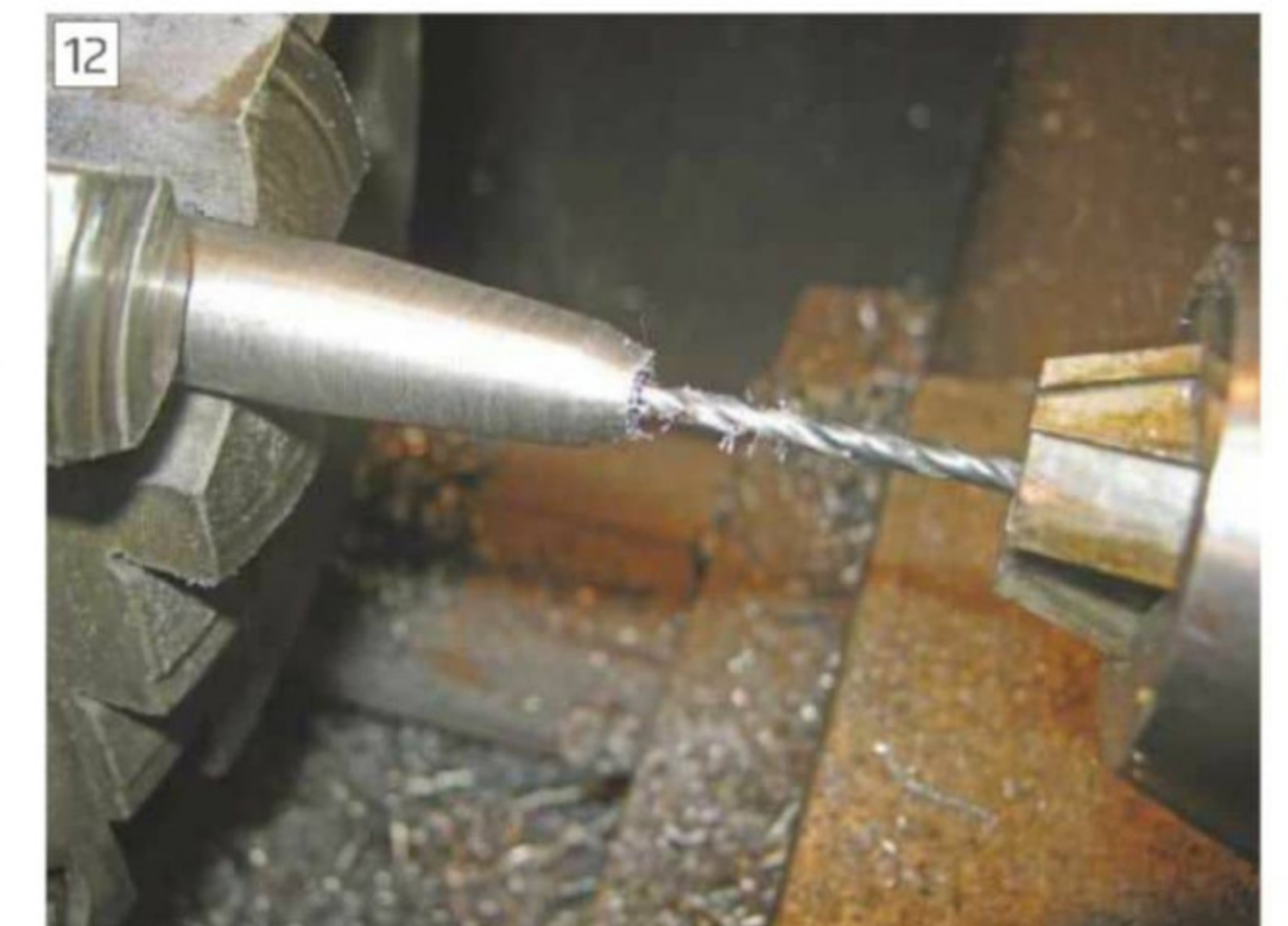
Drilling the punch
