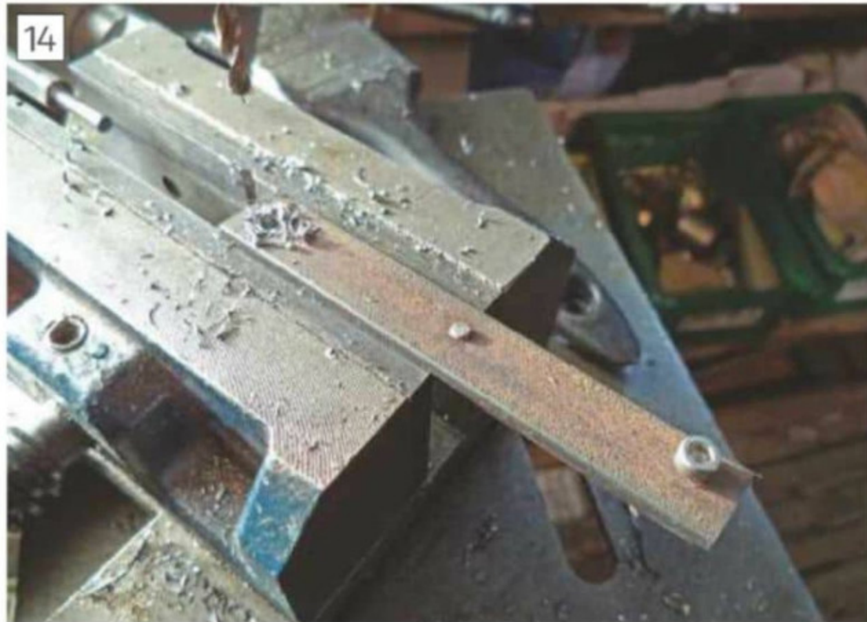
Pivot around the middle hole to drill the rest
