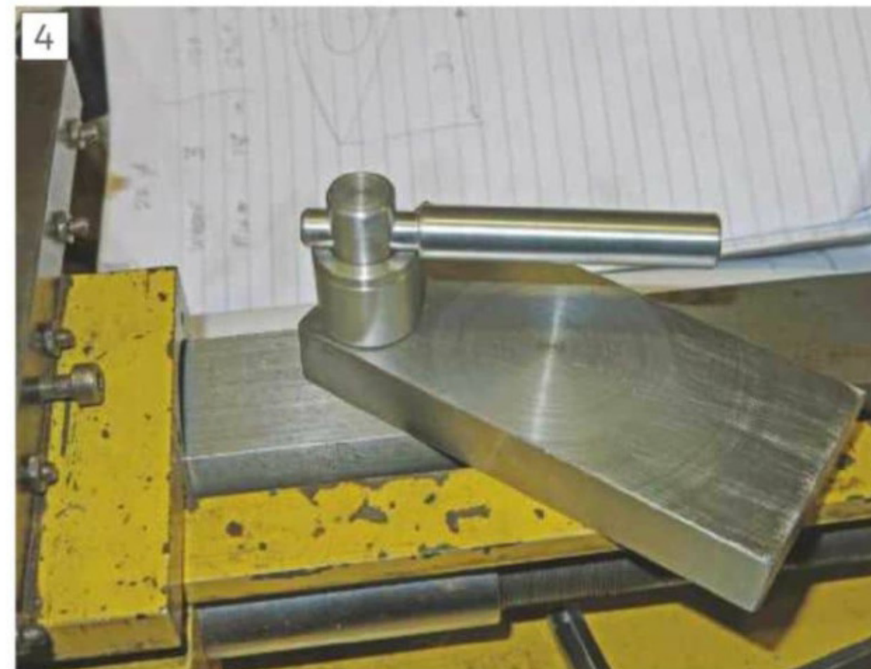
Pillar assembled to block
