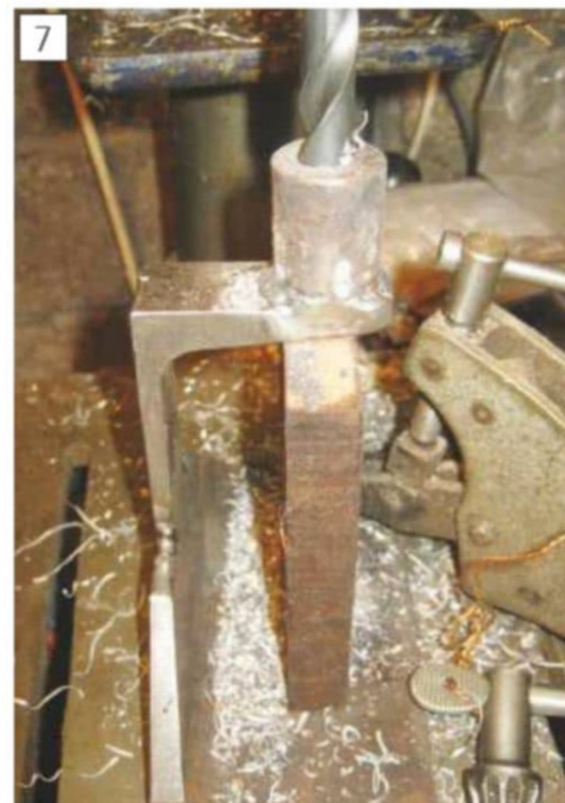
Drilling the guide
