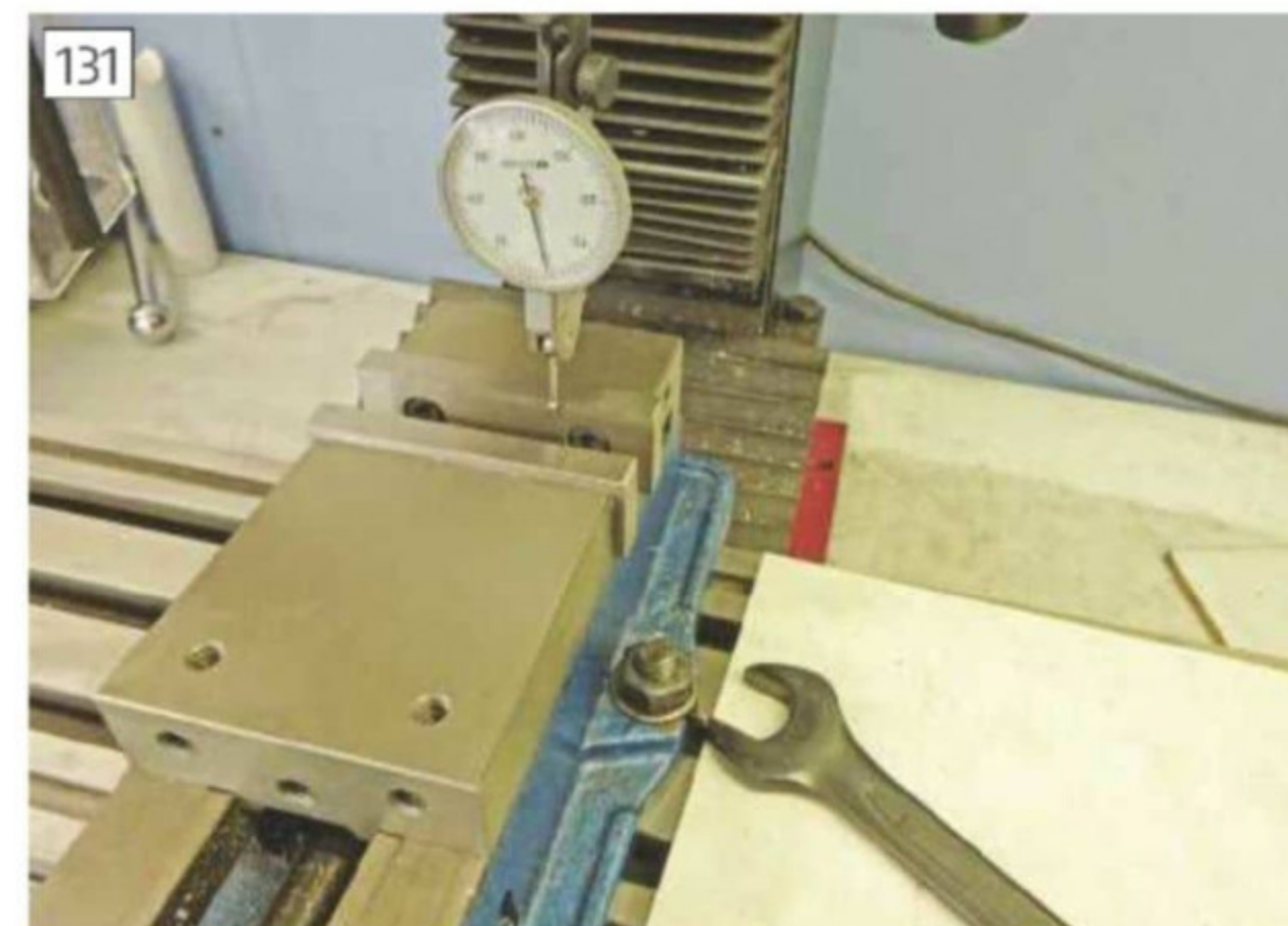
Setting to X-Axis using Dti against fixed jaw
