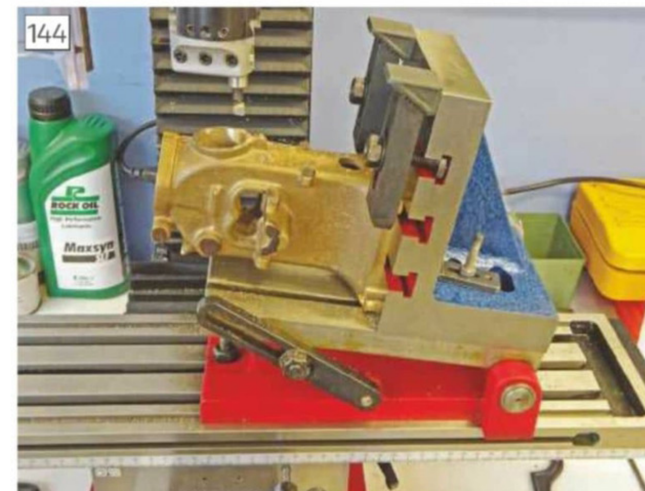
Combining tilting table and angle plate to achieve desired angle
