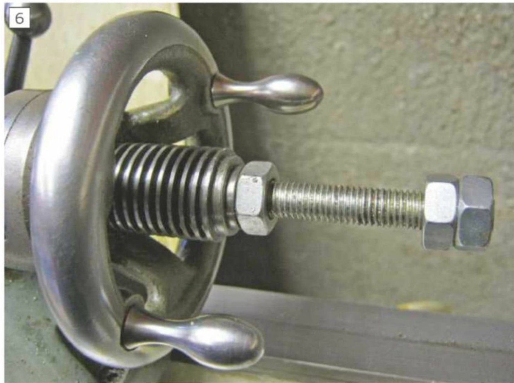
Drawbar for tailstock chuck
