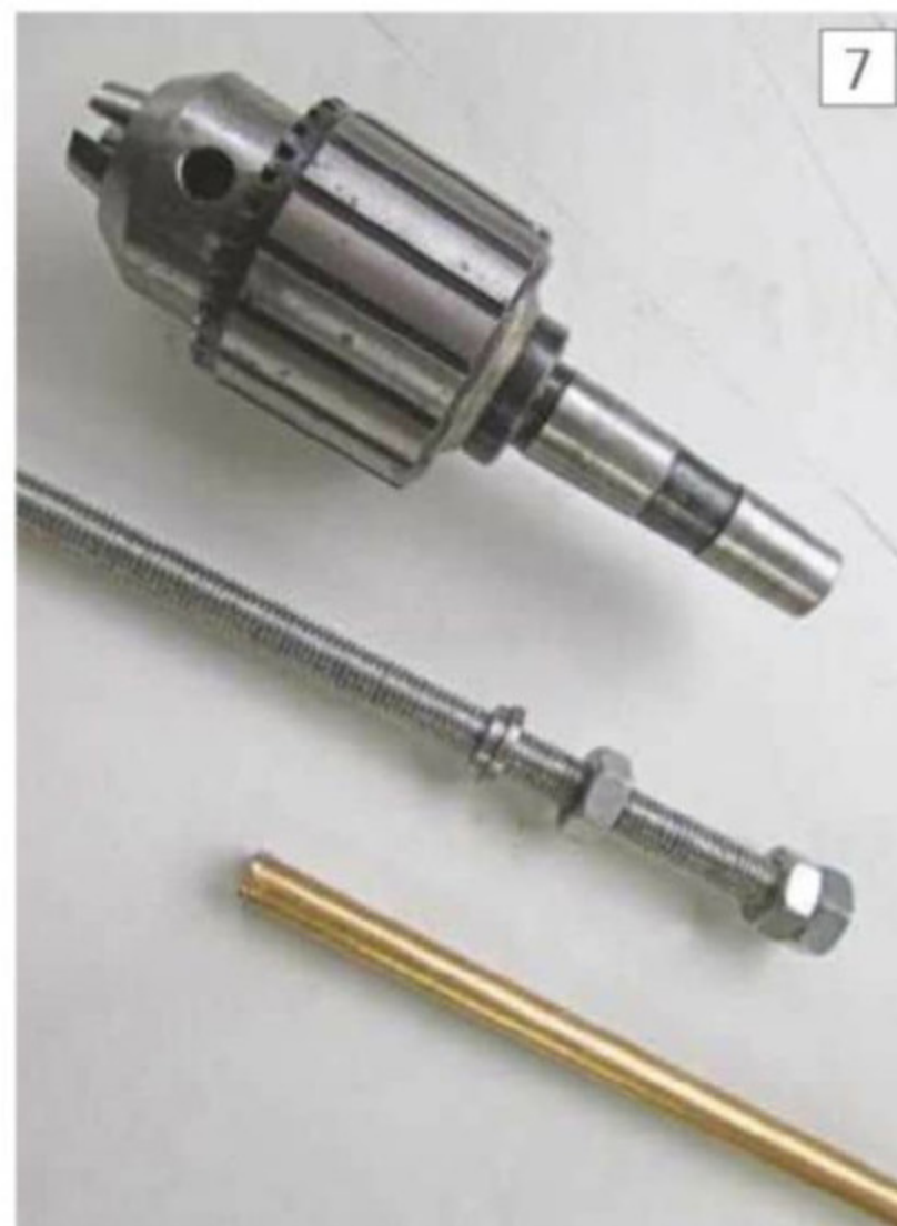
Drawbar components for tailstock chuck and dolly/drift for chuck removal
