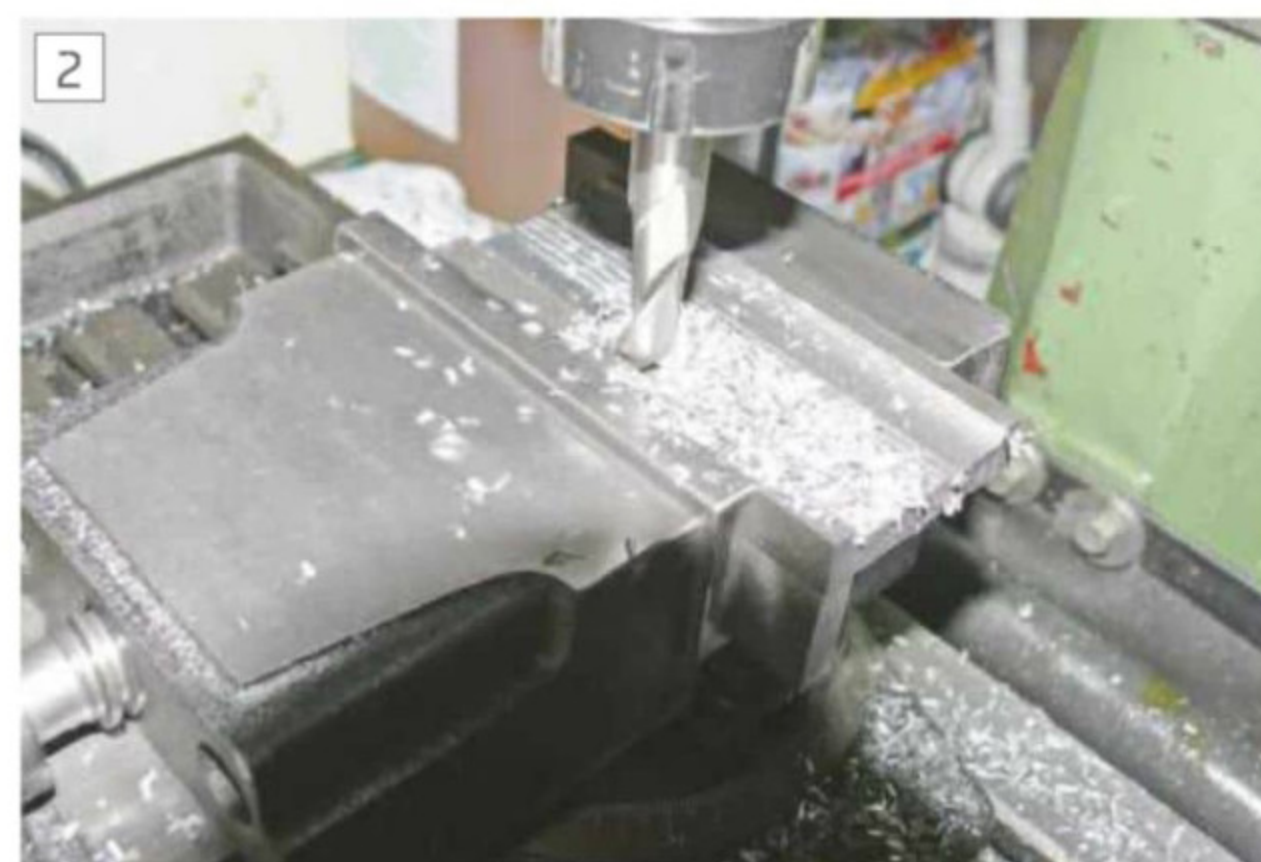
Milling a slot for the laser.
