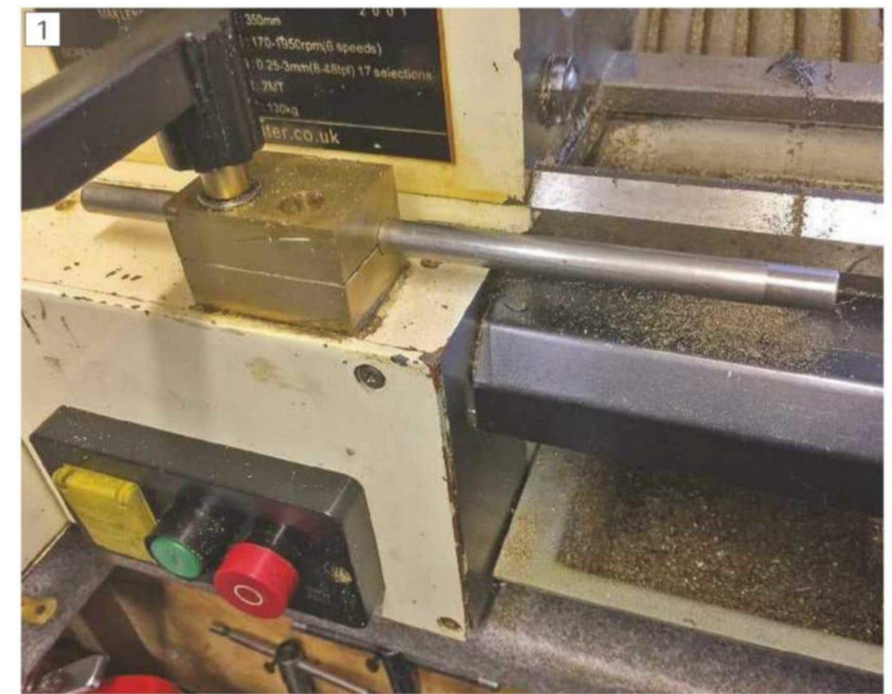
The conventional saddle stop on my first lathe
