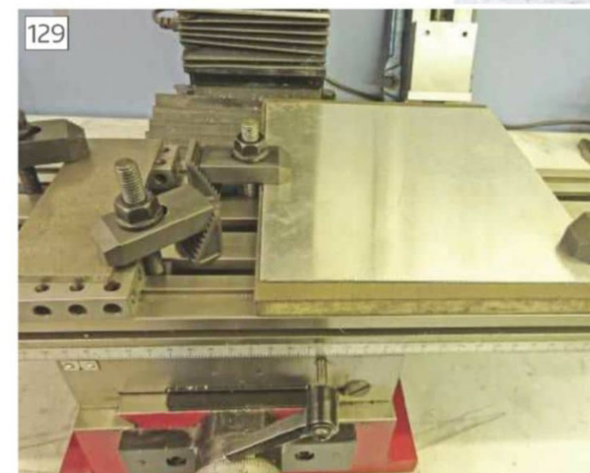
Clamping of plate and sheet materials to protect table
