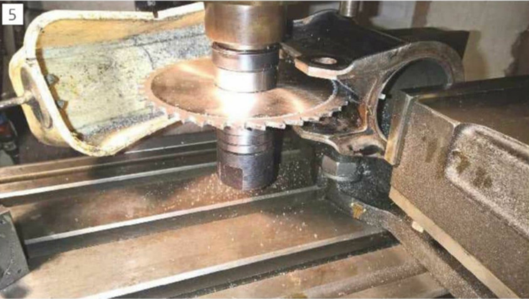
Slitting between the strut mounting bolts
