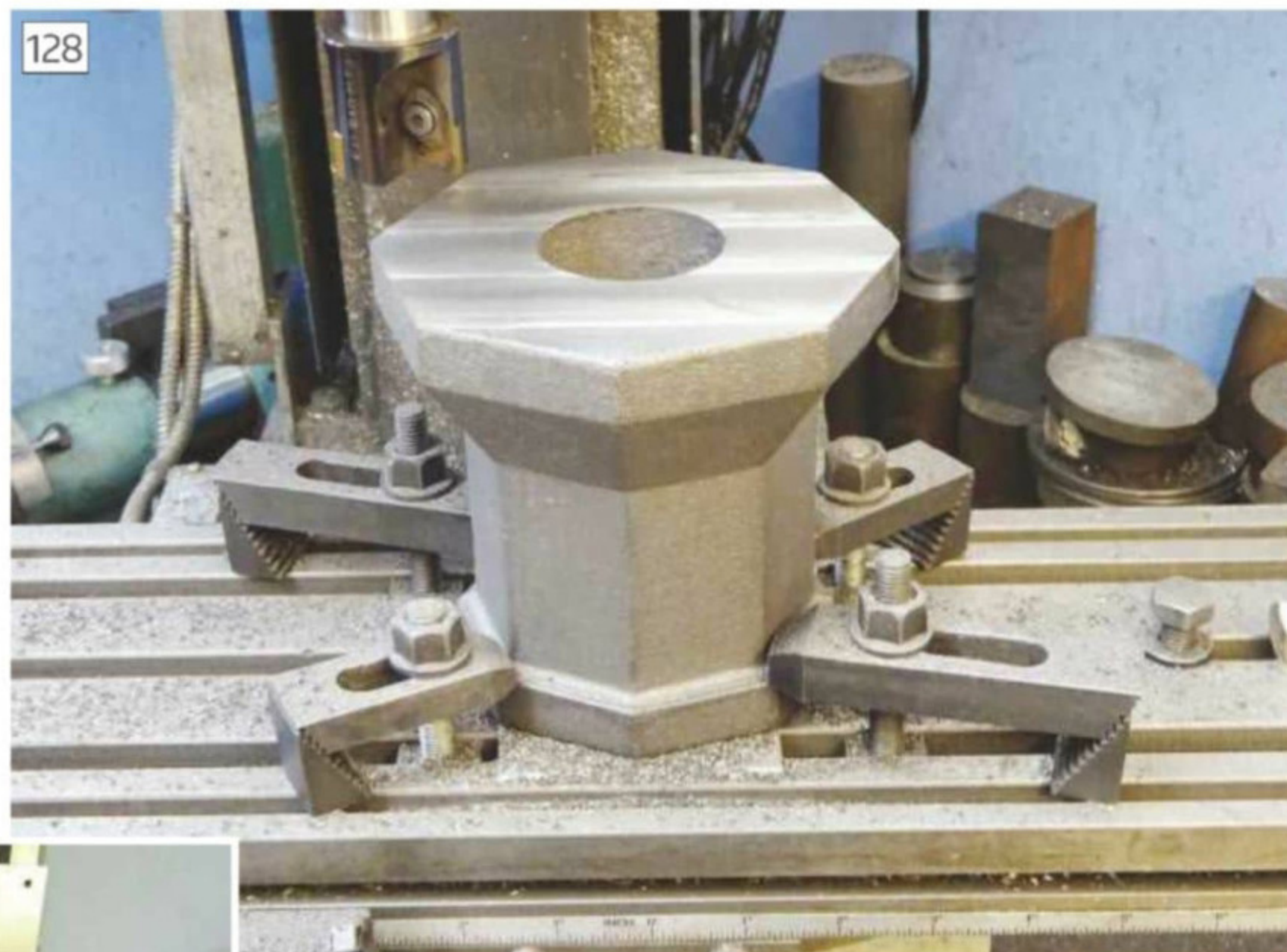
Correct placement of clamps.
