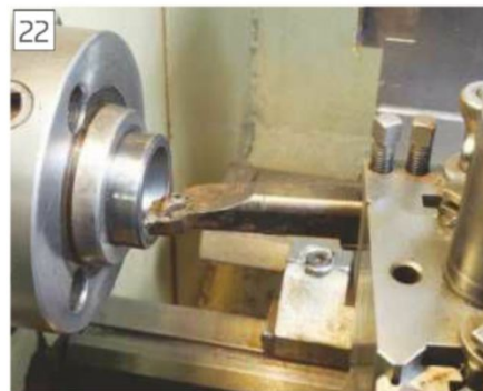
Machining the bore
