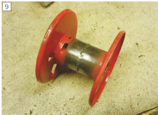
Modified hoist drum
