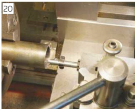
Screw cutting the collet adaptor
