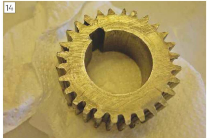
Detail showing the swaging over of gear teeth
