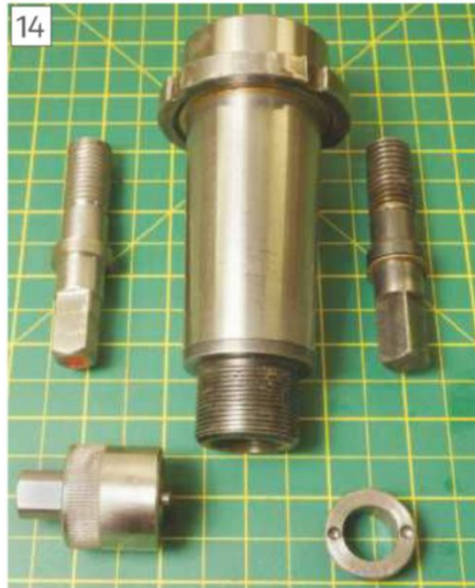
Collet and carbide tool with 20mm shank
