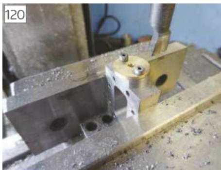
Shaping an oval boss with an external cuts
