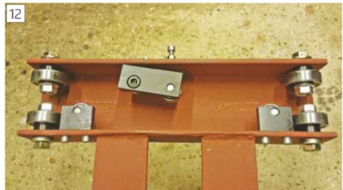
Rollers with side adjustment on one side only
