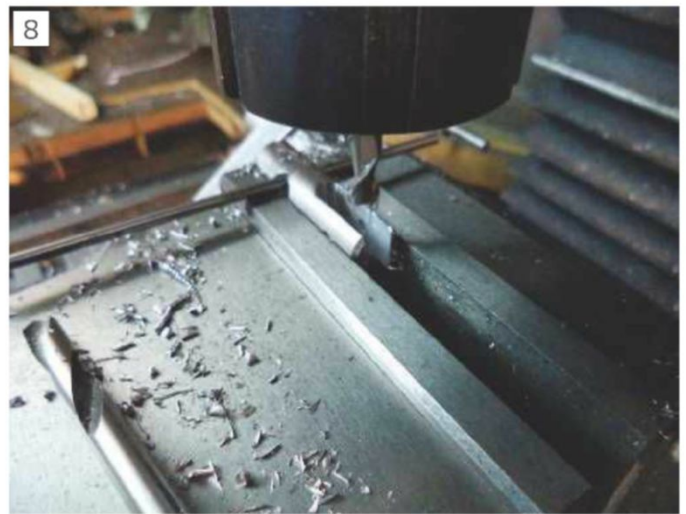
Mill or file to finish the slot
