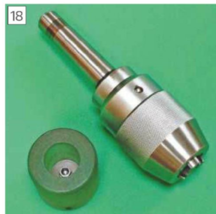
Handle for use with keyless chuck
