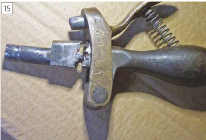
Fractured weld on the cast iron selector handle
