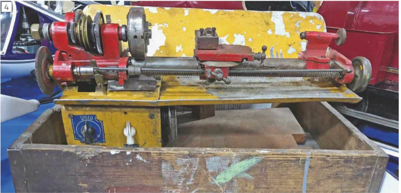
WWII Lathe made from a gunsight.
