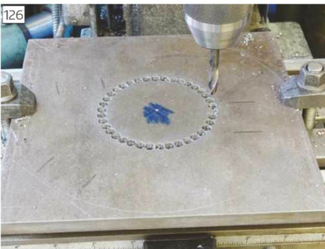
Stitch drilling out circular waste
