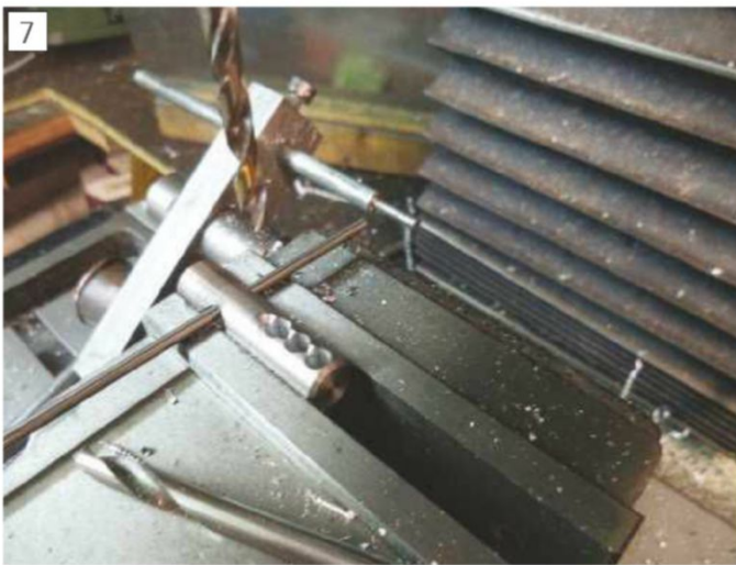
Preparing slot by drilling
