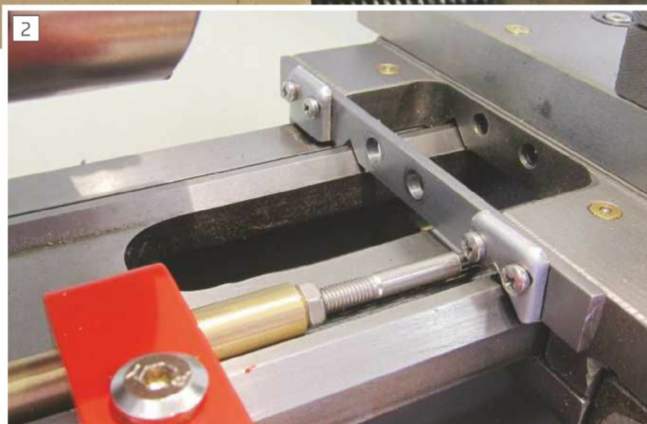
Tapped holes for steady, cross bar and depth stop.
