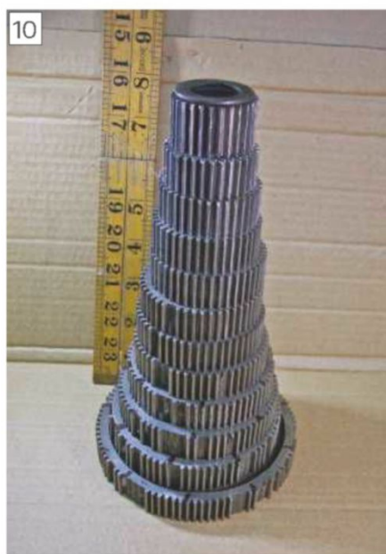
The damaged cone gears
