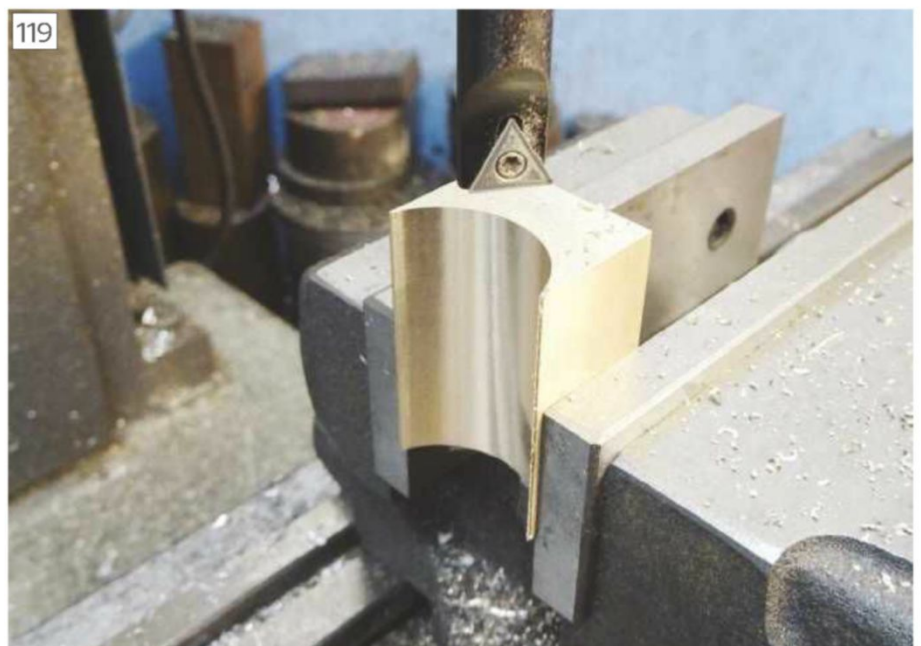
Machining a concave surface
