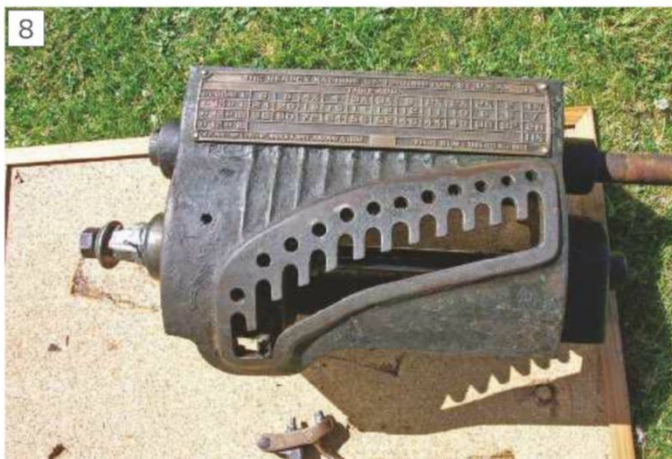
The gearbox after removal from the lathe
