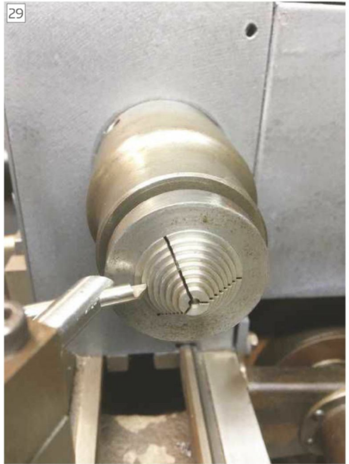
Dial indicator used to depth the steps accurately.
