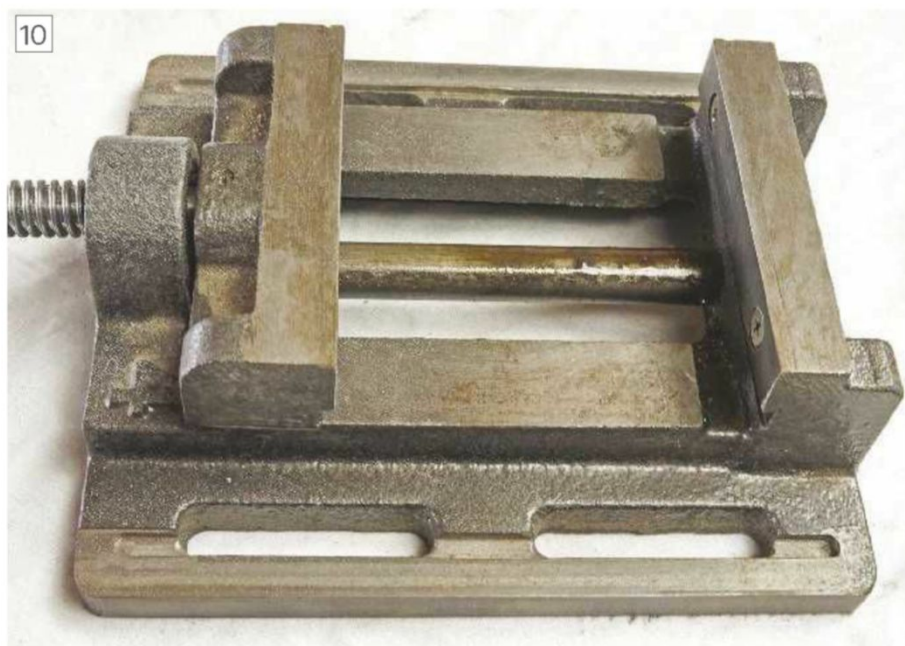
The vice as machined for the version 2 clamps – note the milled groove, and the faced top and sides of the flange
