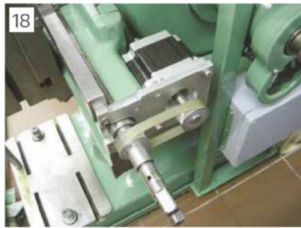
Drive arrangement with cover removed
