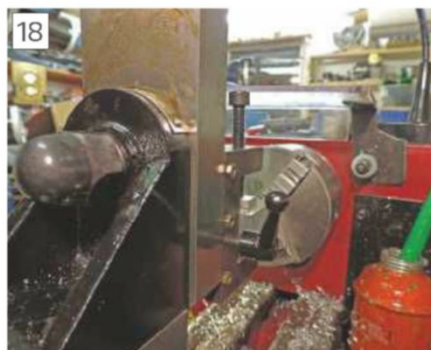
Vertical slide locking lever and gib adjusters.
