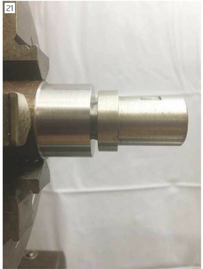
Checking Collet seating depth.
