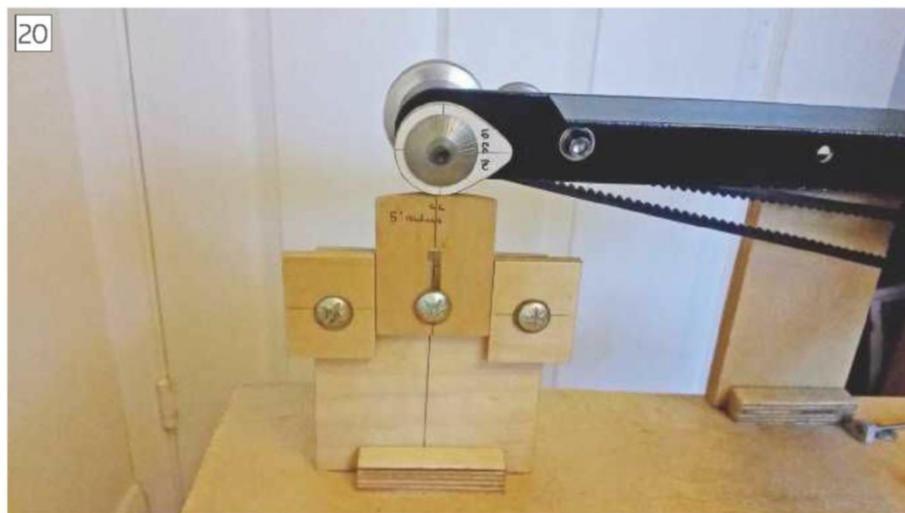
The height-adjustable cam rest.
