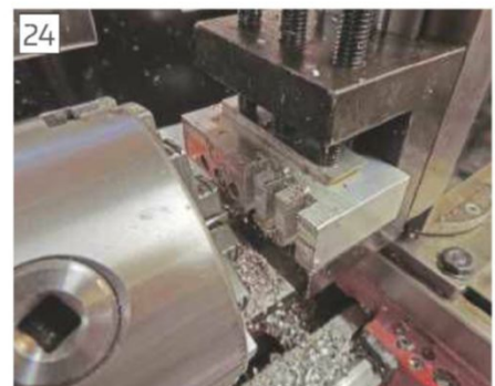
24 First three slots, note increasing depth.
