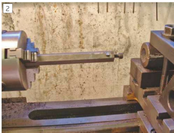
Boring the body of a casting clamped to the cross slide.
