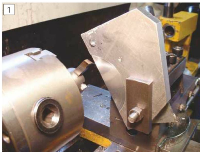
Flycutting work held in the toolpost of my mini lathe.
