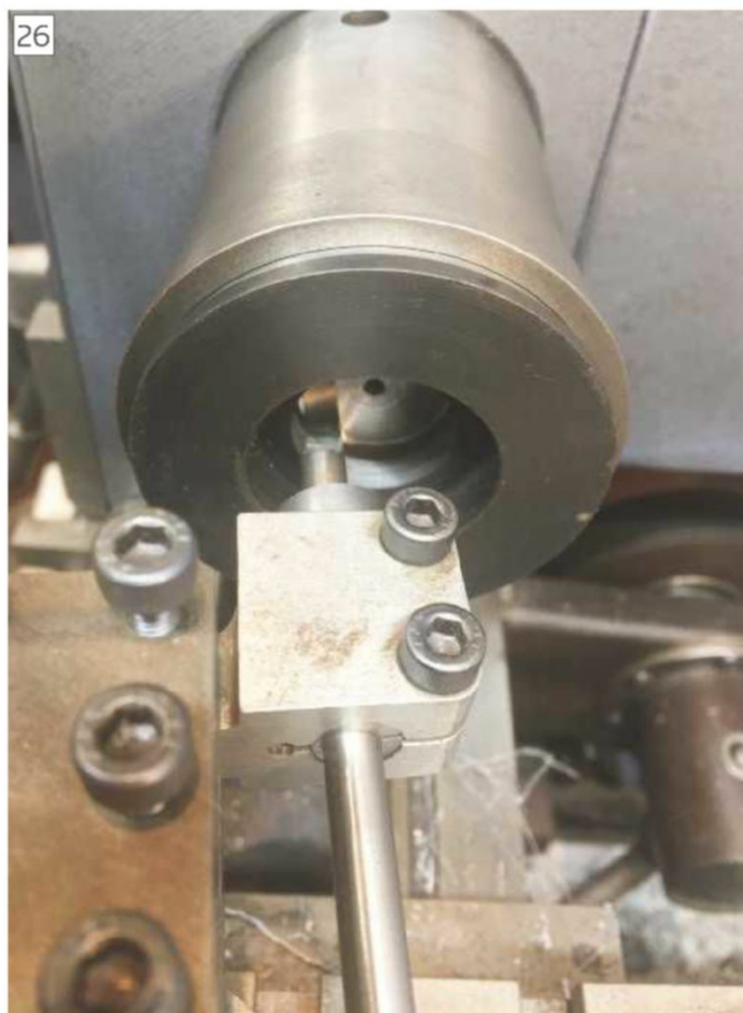
Rough machining collet steps.
