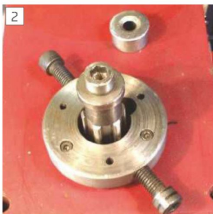
Locking ring on spindle top
