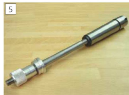
Weldon-style cutter holder with drawbar.
