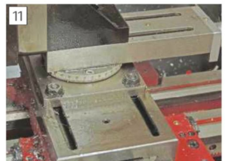
The top slide can be moved along the cross slide to a more convenient position.
