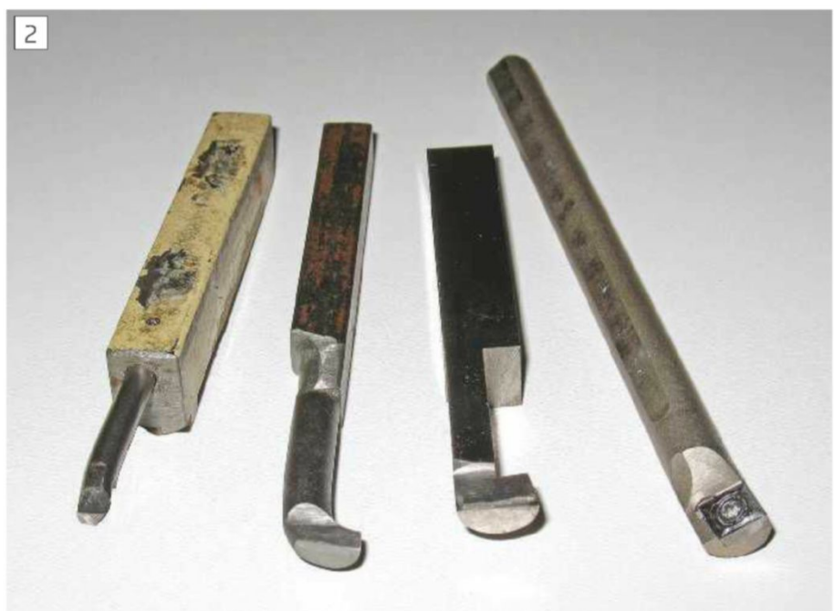
Boring Tools. Three HSS tools & a carbide Insert.
