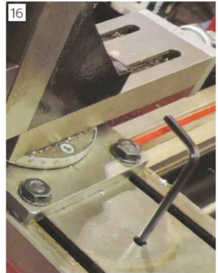
Cross slide clamp screw, this must only be tightened gently!
