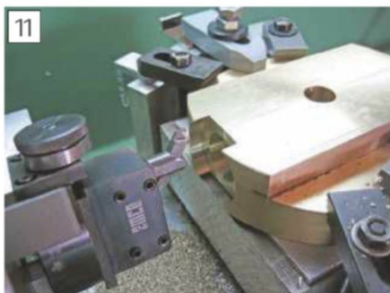
Boring for ball nut
