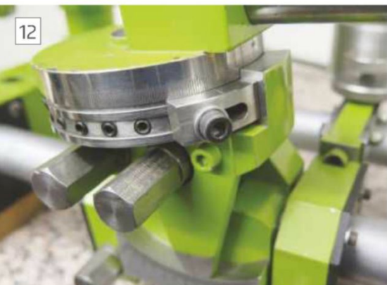
Setting Dish Angle and Stop 1 to 2 Degrees
