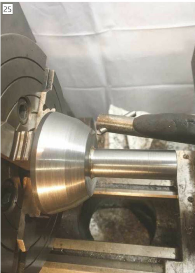
Machining Secondary chamfer.
