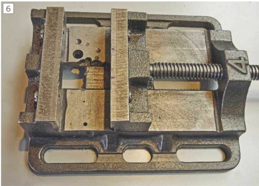
The vice showing the groove milled in the flange
