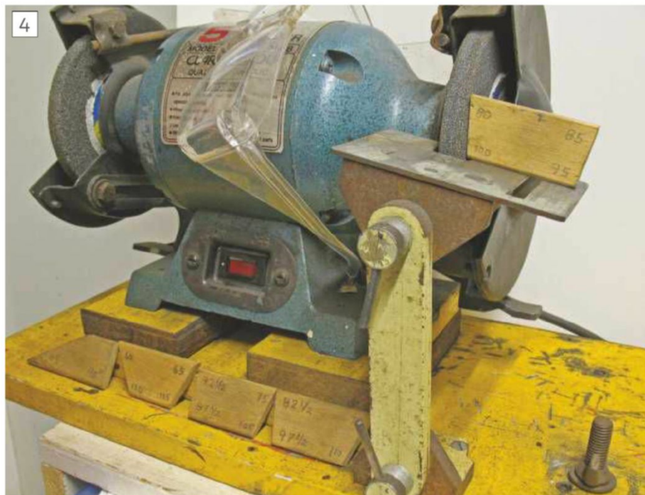
Grinder. Note the safety eye shields kept ready for use on the grinder body, and the wood templates for setting various angles.
