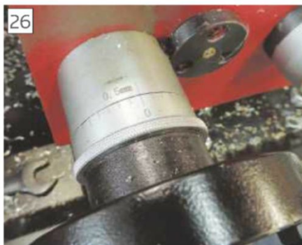
Handwheel dial, marked in 0.5mm divisions.
