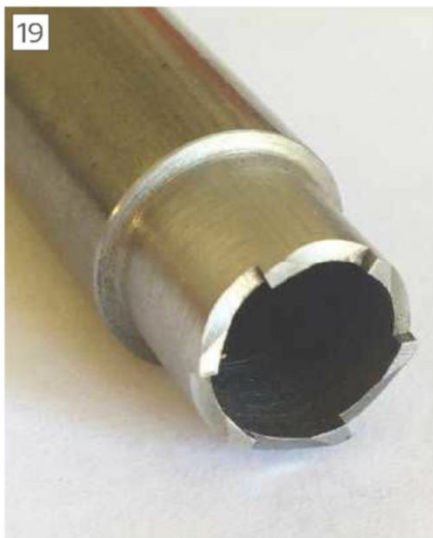
Small holesaw cutter 8.5mm ID x 11mm OD.
