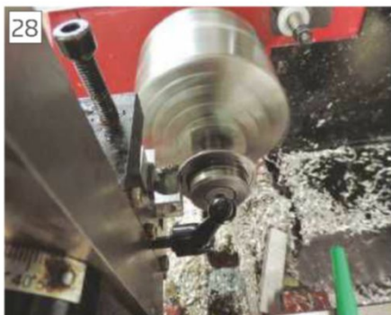
The slitting saw is held in a sprung holder that adapts to different diameters.
