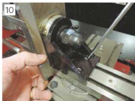
Attaching the vertical slide – take care not to bottom out the screws.
