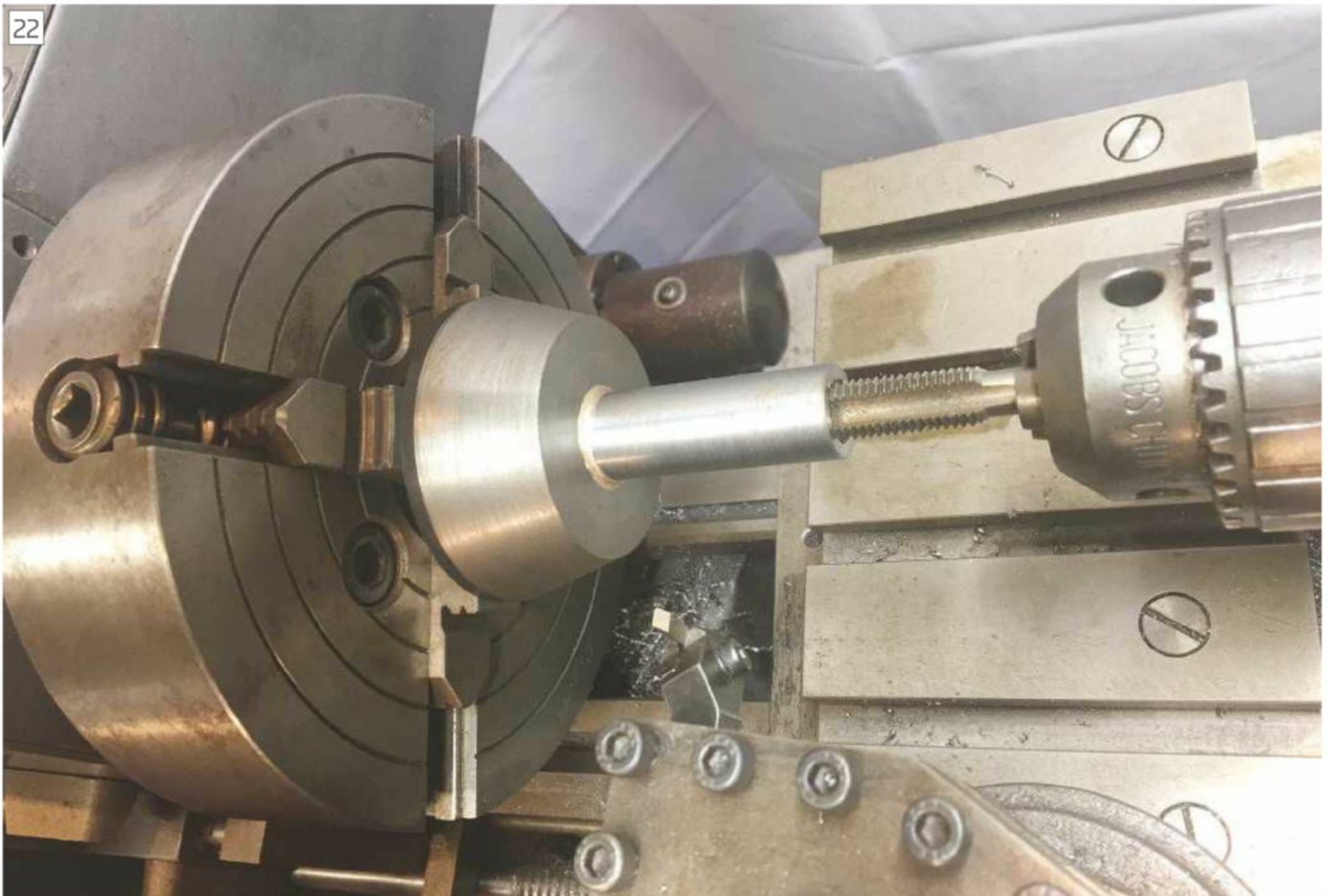
Tapping Drawbar Thread.
