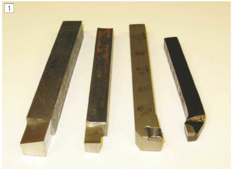
Knife Tools. From L-R: Carbon Steel, HSS, carbide Insert, TCT (Left Hand).
