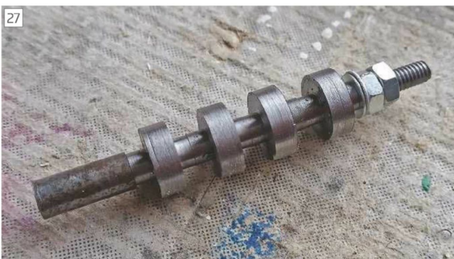
Four cam blanks mounted on the mandrel ready for grinding.
