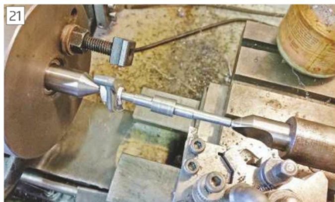
Machining the grinding head spindle between centres.
