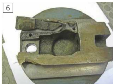
Smashed dovetails on the vertical slide
