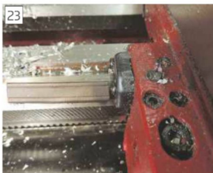
23 Magnetic strip used as a temporary depth mark.
