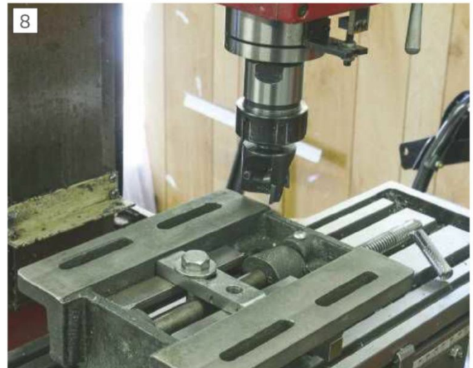
Milling the base of the vice parallel to the jaw sliding surfaces
