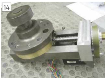
Restored ram head
