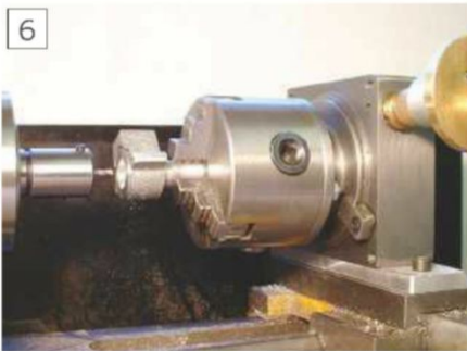
Milling with a cross-slide mounted rotary table.
