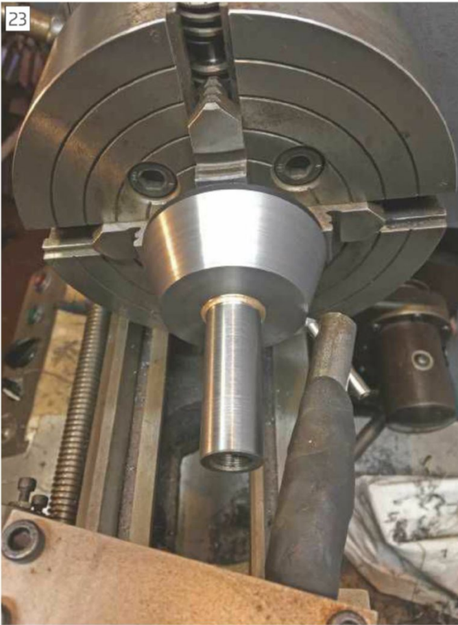
Machining the closing taper on an internal collet.
