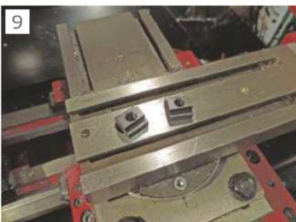
M6 the nuts fit the slots in the SC4's slides.
