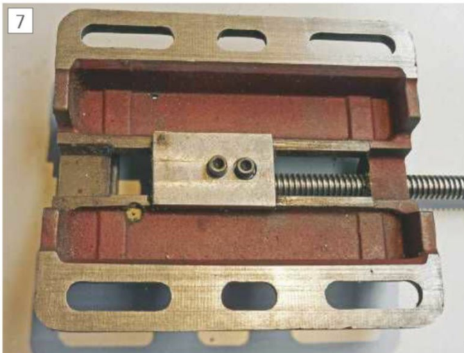
The stronger keep plate fitted to the vice – a few attacks by the tin moths evident
