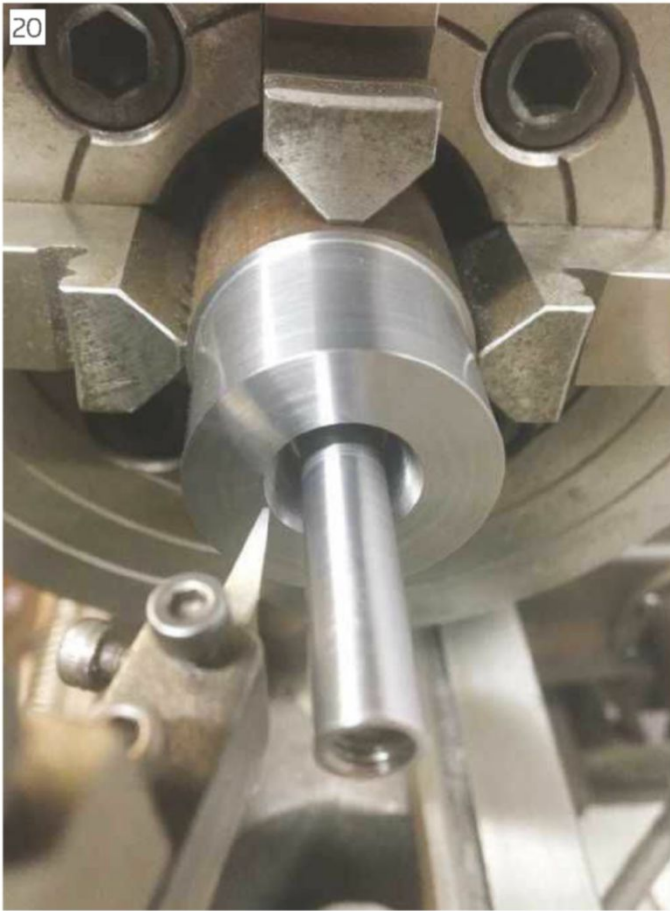
Machining external collet expanding taper.
