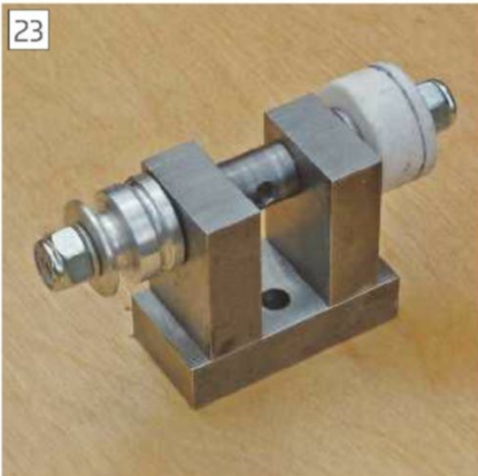
The completed grinding head. A larger grinding wheel than that shown was used.
