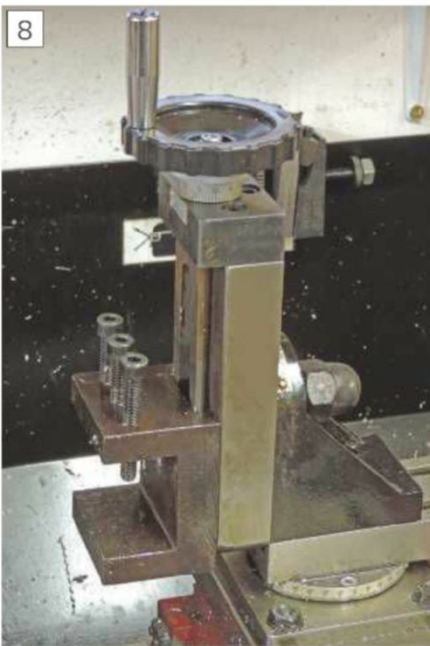
'New' style vertical slide with clamp style carriage.
