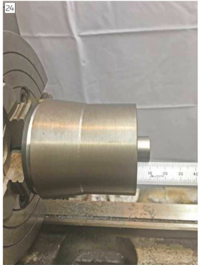
Using Collet Chuck to check seating depth.
