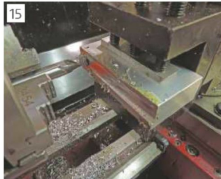
Surfacing the aluminium block with an uncoated carbide slot drill
