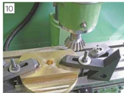
Dovetailing replacement block
