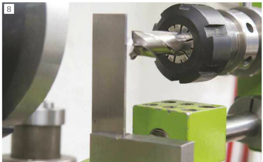
Setting Cutter Tips Upright and Square
