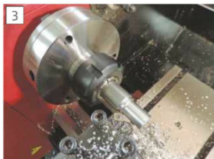
Direct mounted ER32 chuck on the SC4.
