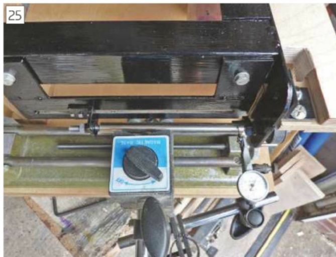
Locking the centre alignment using a test bar.
