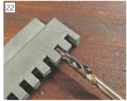
22 Using tape as a depth stop.
