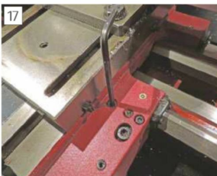
Carriage clamp screw, do not overtighten, it will not lock the slide solid.
