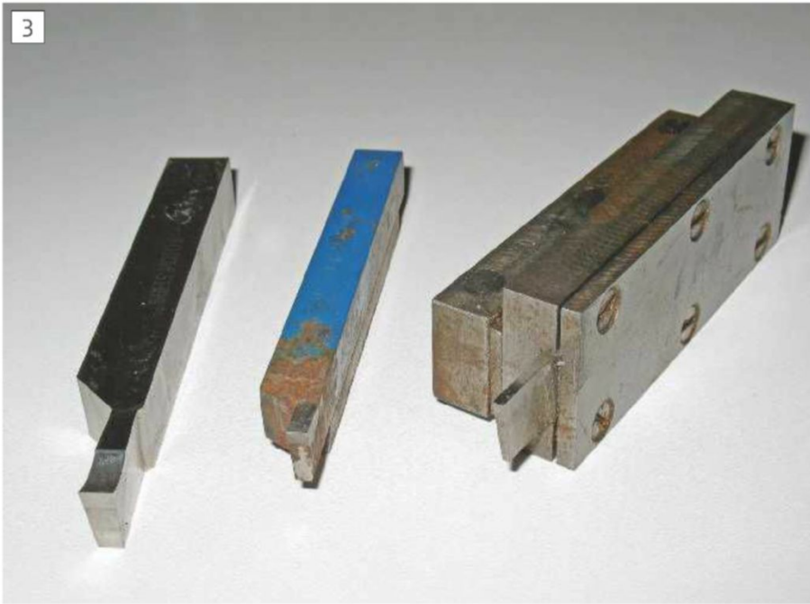
Parting Off Tools. From L-R: 5mm HSS, 3mm TCT, & 1.84mm carbon steel.
