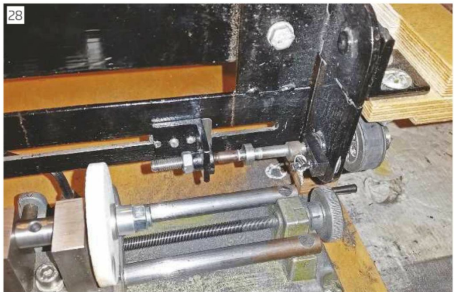
A single cam ready to be ground.
