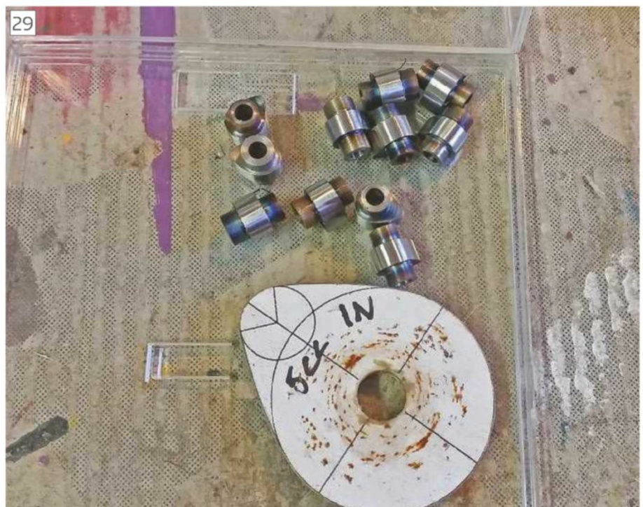
Finished cams, polished and ready for case hardening.
