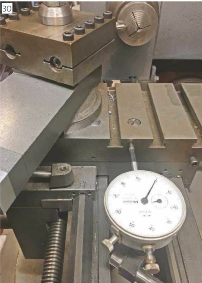
Finish machining an external collet.
