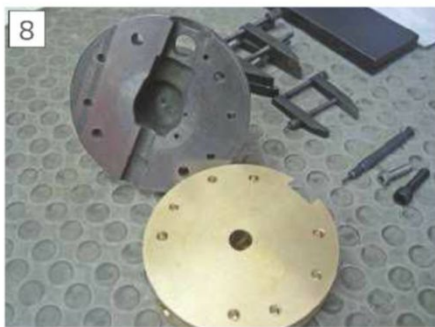
Mating surface milled to a good finish
