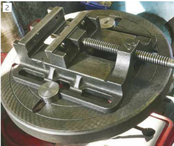
The vice clamps in position on the machine
