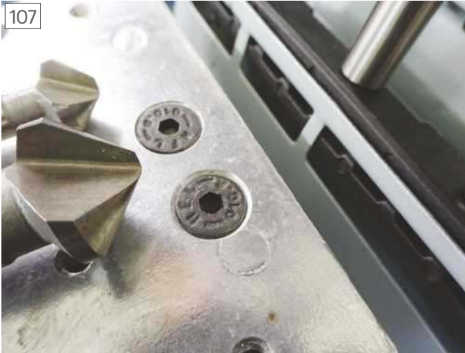
Holes from different size countersinks
