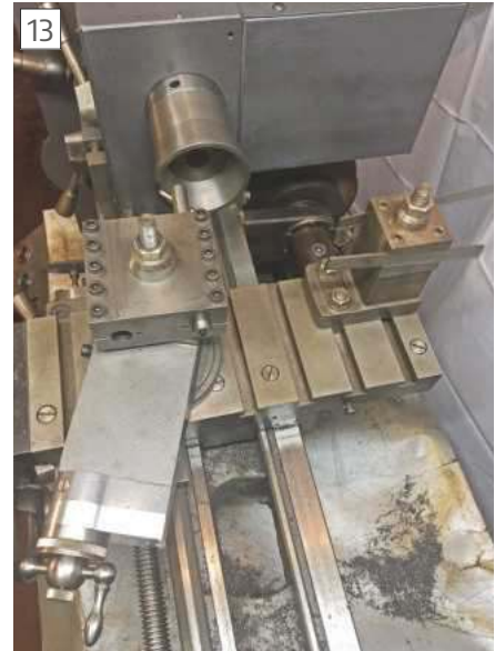
Topslide set up to machine closing taper.
