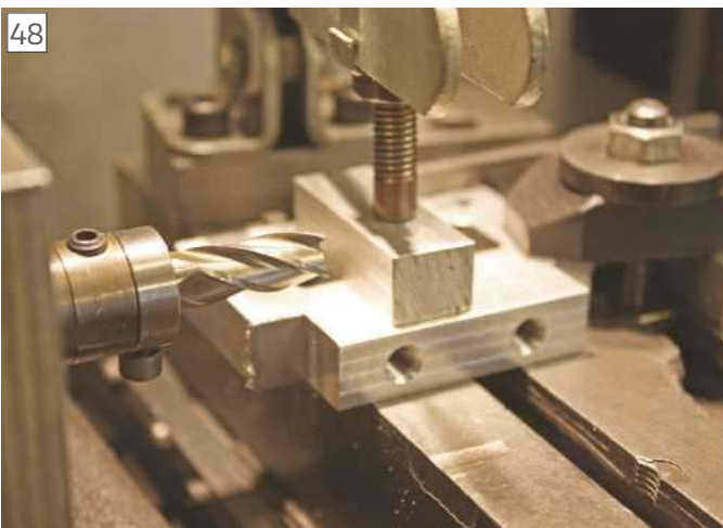
Milling bevel box supports.
