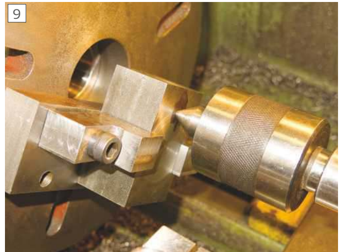
Block clamped by tailstock
