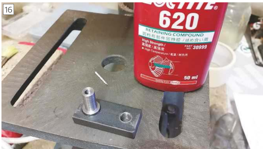
Fixing the idler axle to the swing arm with Loctite. A high temperature grade was used as I had it in stock, but a low temperature grade will be fine for this application.
