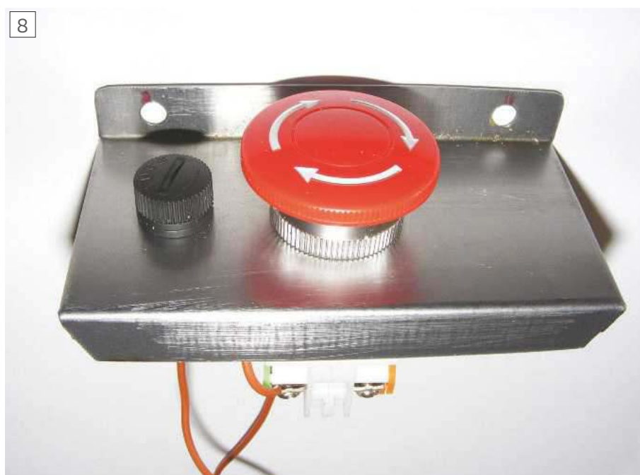
The top of the case with the e-stop and fuse holder mounted.
