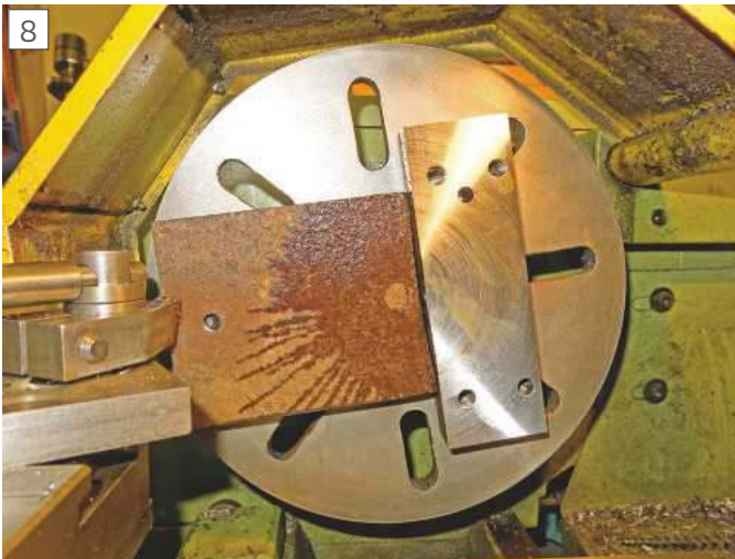
Setup after skimming to give a true surface
