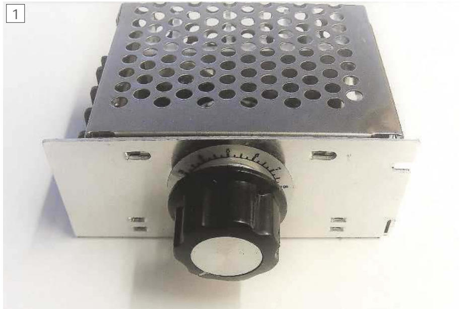
The 4kW motor speed controller.
