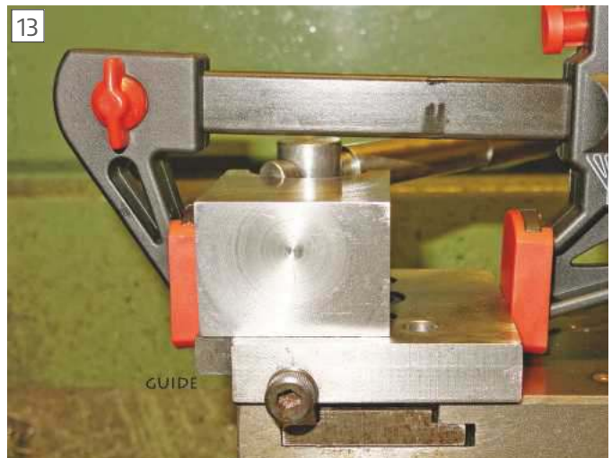
Guide lightly clamped to block
