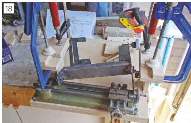
Building the base around the Unimat and frame. The base was made to fit these components and was not built to a plan.
