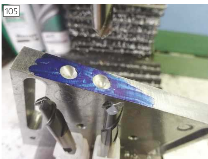
Starting a drill on an angled surface
