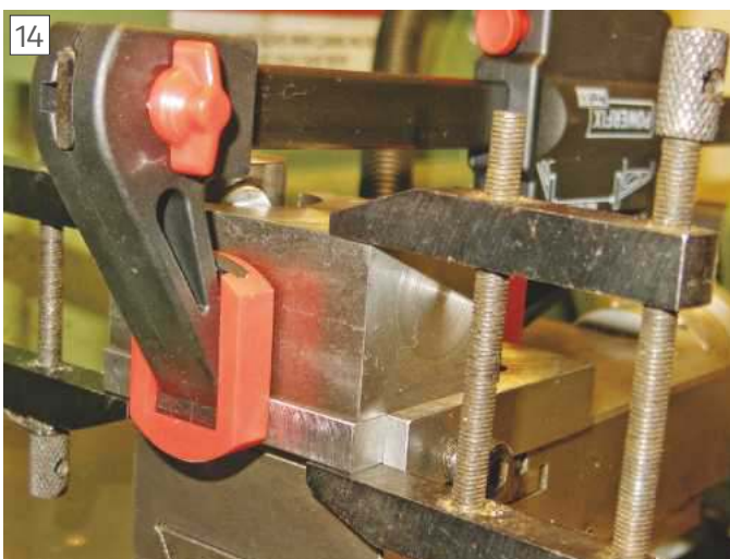
Guide secured with toolmaker's clamps
