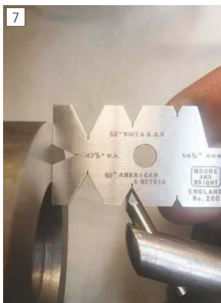
Setting toolbit square using Screw cutting Gauge.
