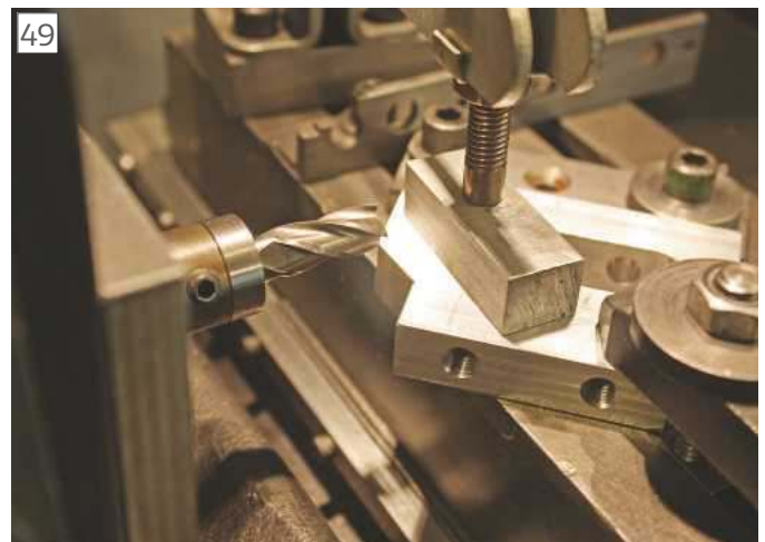
Milling angle on bevel box supports.
