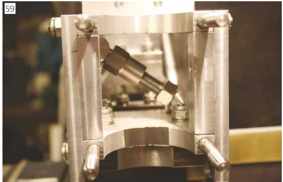
Shows the spreader mounted in the attachment.
