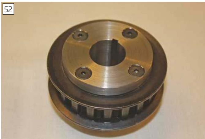
Assembly of rear pulley and spacer.
