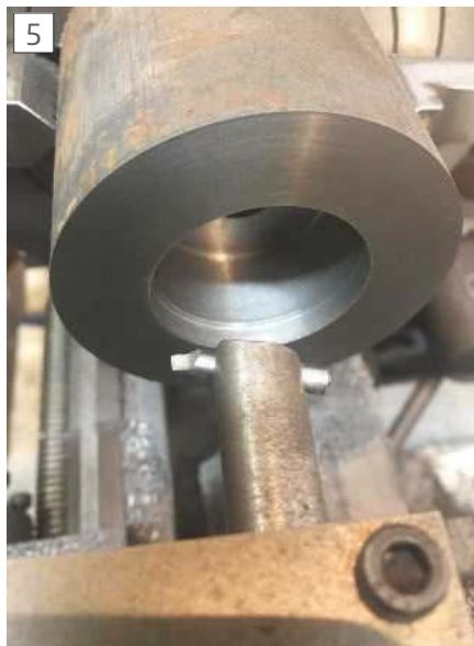
Toolbit to machine the runout groove.
