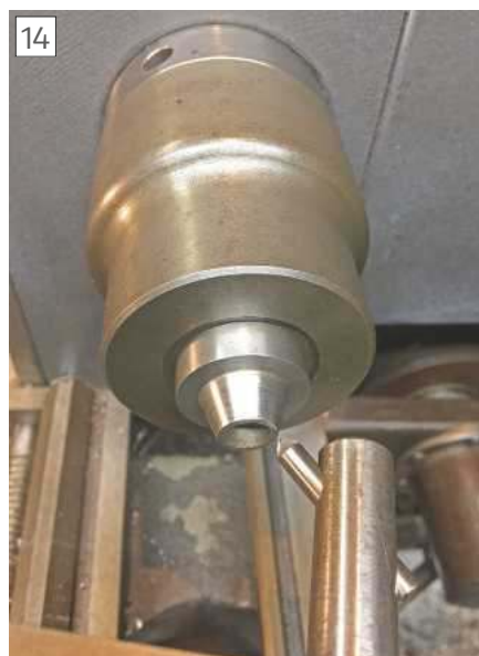
Machining External collet expanding taper.
