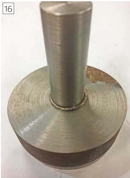
Components trial assembled without flux.
