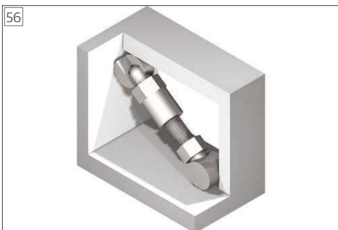
Computer-generated view showing how spreader fits.
