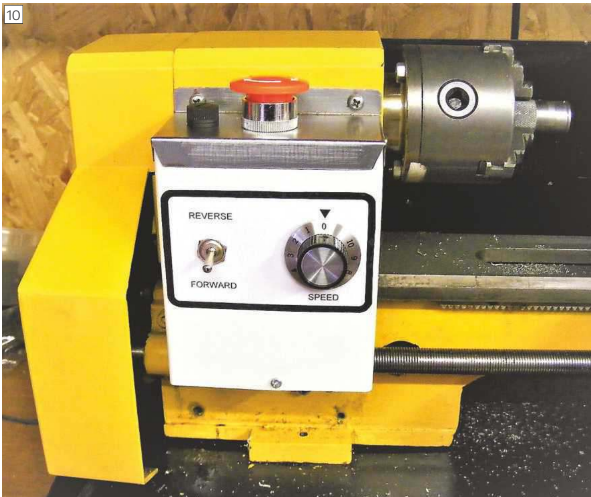
The completed controller mounted on the headstock.
