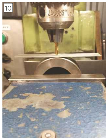
Centering workpiece under drill spindle.
