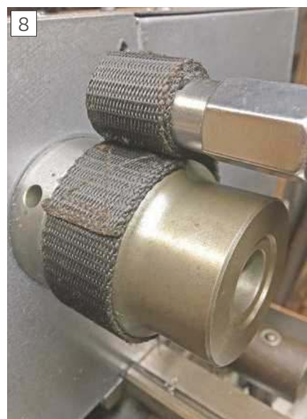
Strap wrench removing Master Chuck.
