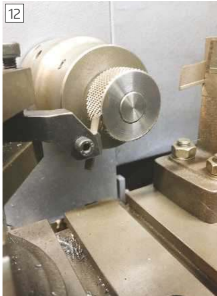
Threaded Knurled Component being machined using a threaded slave.
