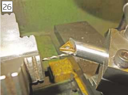
Drilling angle hole to meet blind lengthways hole
