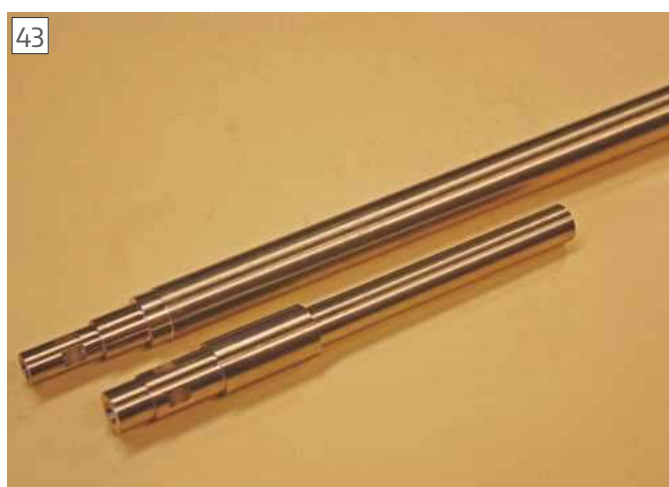
The countershaft and vertical shaft.
