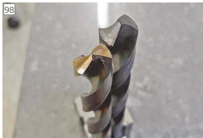
Split-point and standard drill bit ends
