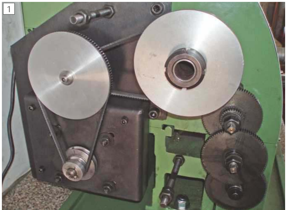
Modified for two-stage speed reduction
