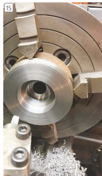
Machining chucking recesses in large collet head.
