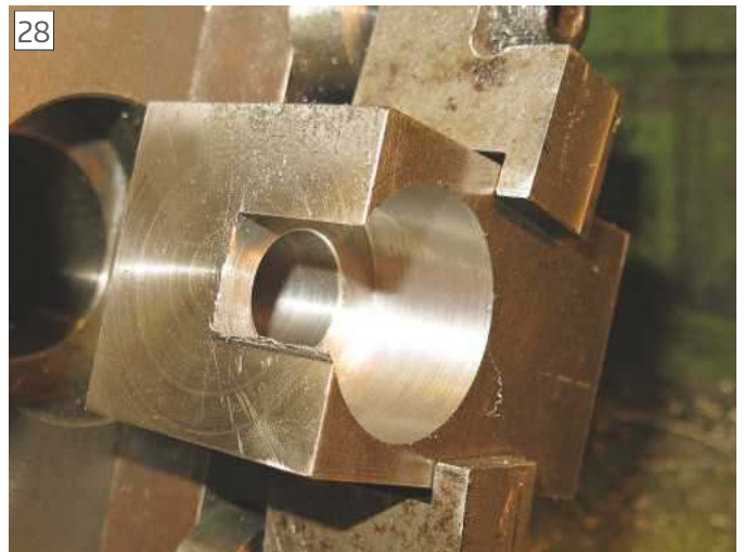
Example bore cut with the tool
