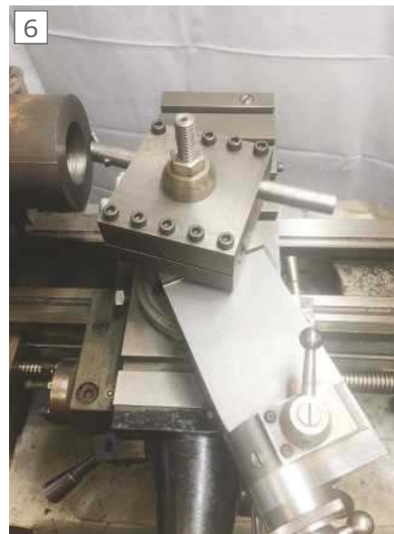
Retracting topslide set up for screwcutting the thread.
