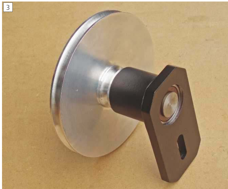
Intermediate pulley and bracket assembly
