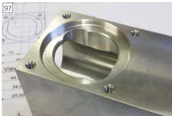
Clean edge around subsequently tapped holes
