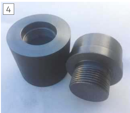
Dummy Spindle and Threaded Chuck Body.
