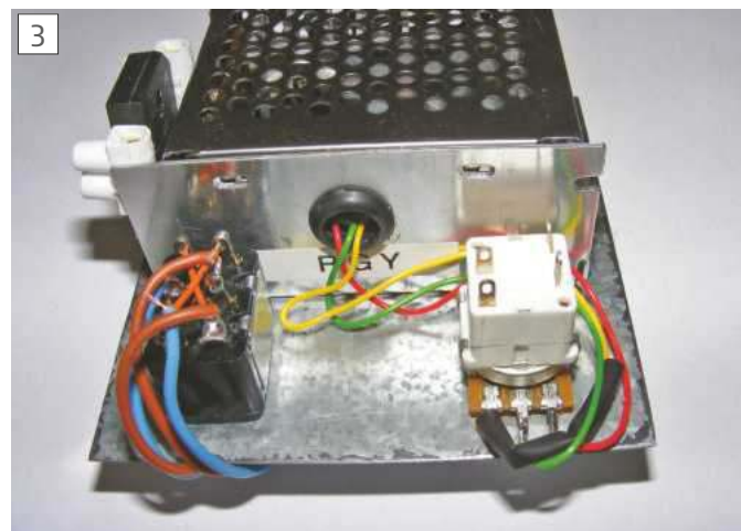
The controller panel. Note the flying leads to the new potentiometer.
