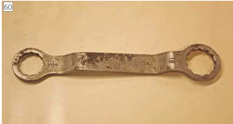
The spanner used to adjust the spreader before modification.
