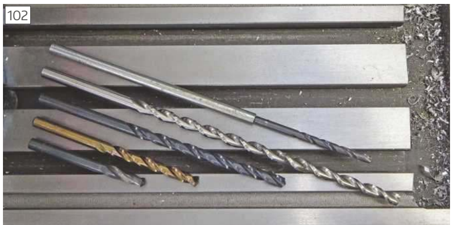
Stub, Standard, Long and Extra Long bits and an extended drill
