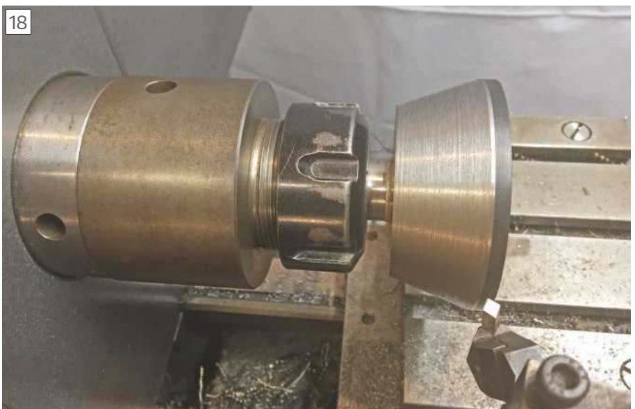
Rough machining of large collet taper.
