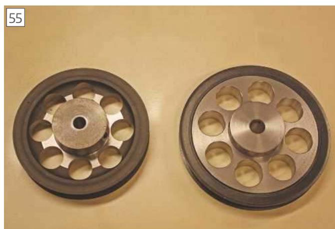
The two larger pulleys with lightening holes.
