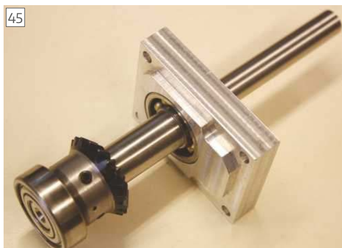
The vertical shaft with bevel gear and bearings mounted in the box top.
