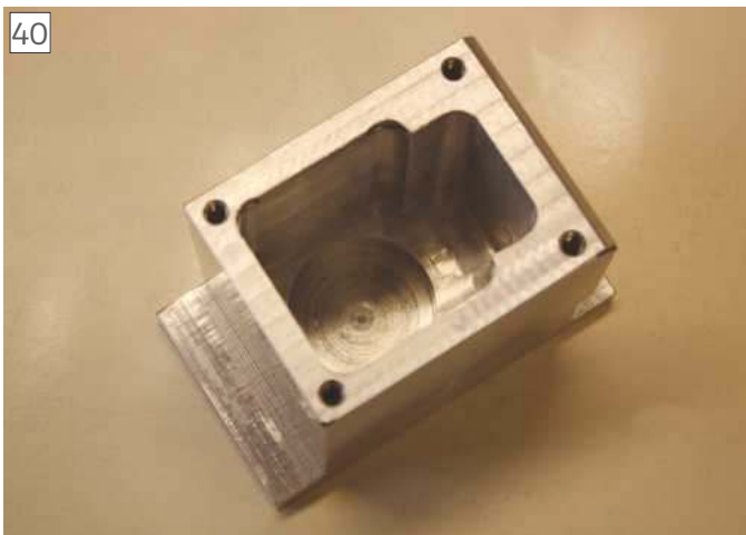
Inside shape of the bevel box complete.
