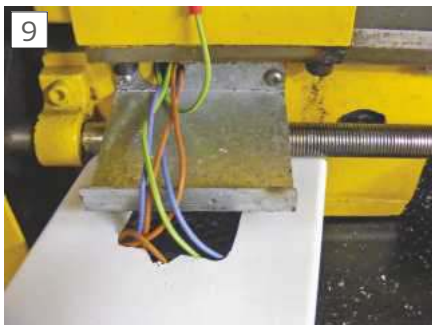
The bottom bracket fixed to the headstock.
