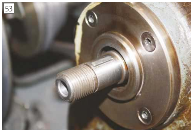
Rear of horizontal spindle showing woodruff keyway.
