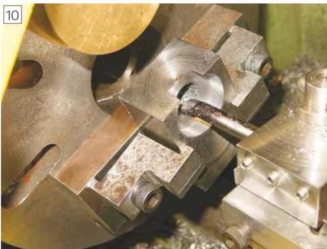
Boring in progress
