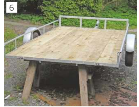
The new floor from pressure treated planks.
