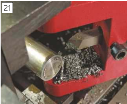
First cut just takes the corner off.
