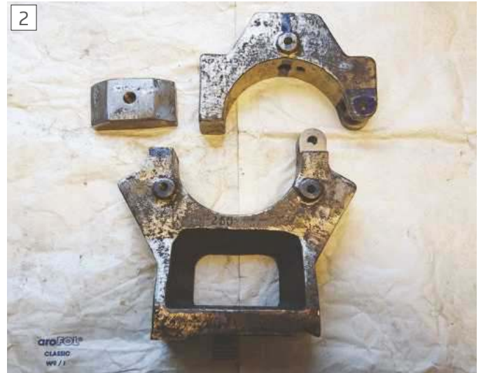
The original parts of the casting, after cleaning up and starting work
