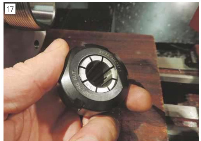
How a fitted collet should appear.
