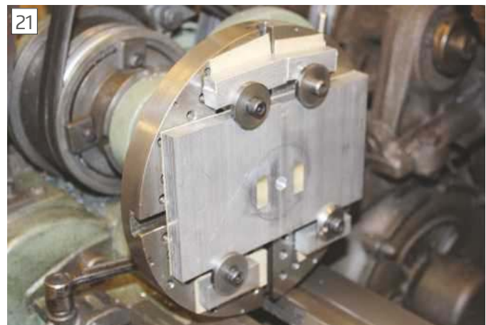
Two Aluminium plates clamped to the faceplate on the lathe.
