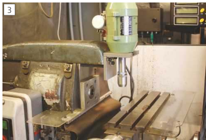
The bench grinder mounted on the support arm via a piece of angle iron.
