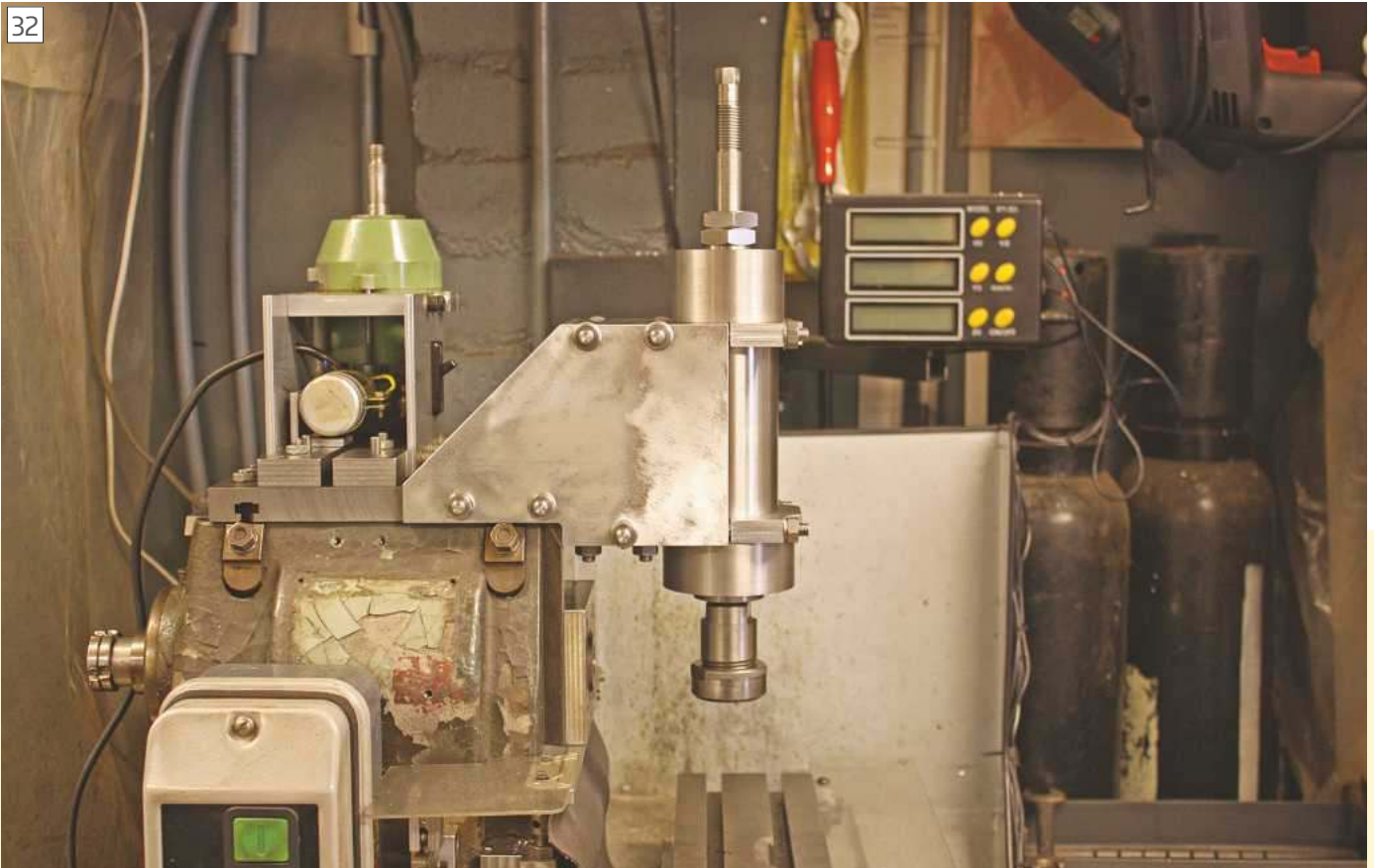
Vertical spindle assembled with Mk 1 attempt mounted on the rear.
