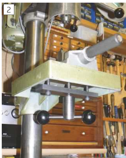
The Clamp in place on the drilling machine
