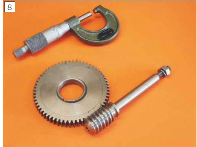
Worm's Acme thread was screwcut thinner than normal to allow it to twist into straight alignment with the gear.
