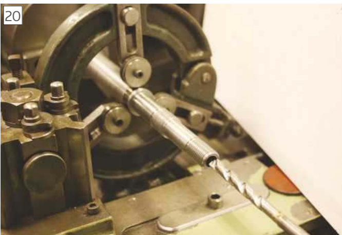
Drilling the 5/16" diameter hole through the spindle.
