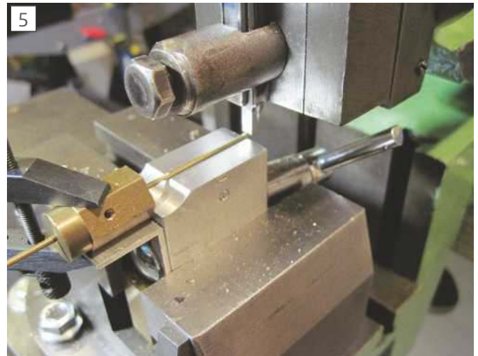
A jig for machining fine scale Hex Material
