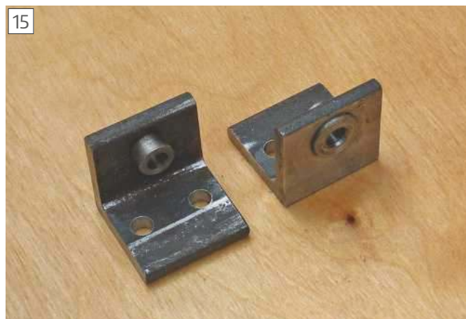
Completed pivot brackets.
