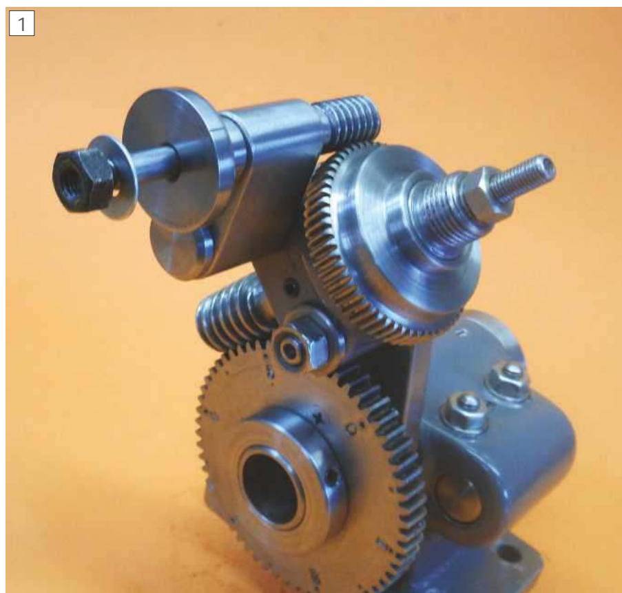
The semi-completed VDH shows the main gear made from a Myford change wheel and the upper gear specially cut "straight at an angle".
