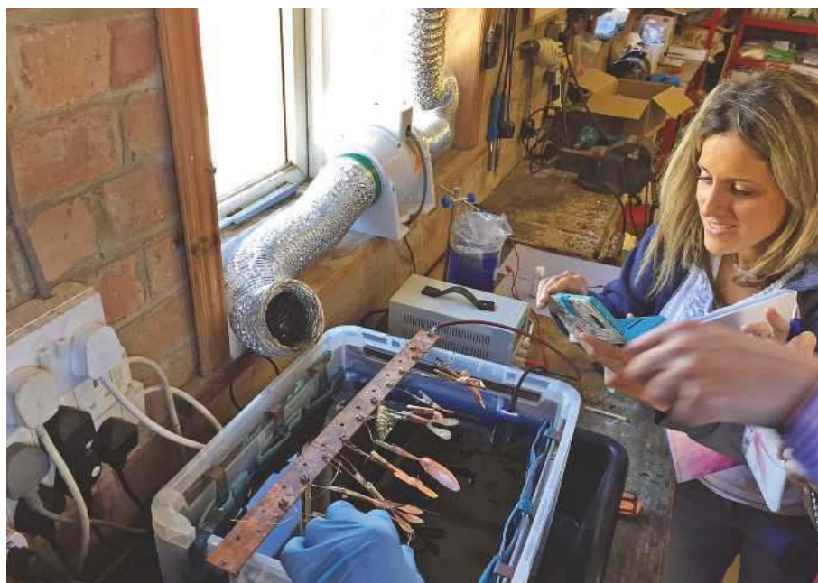
Setting up a plating tank
