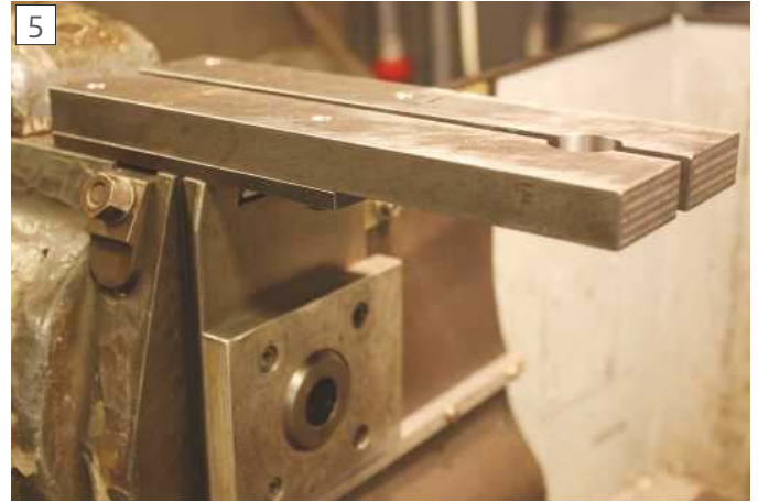
The two rectangular base bars mounted in the dovetail slot.
