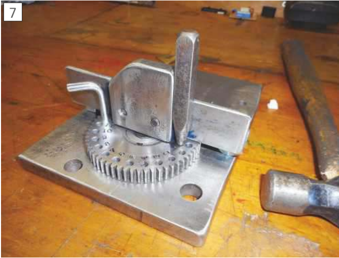
Scrap-box jig was used to stamp numbers on the modified gear.
