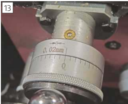
Set the cross slide index to zero.
