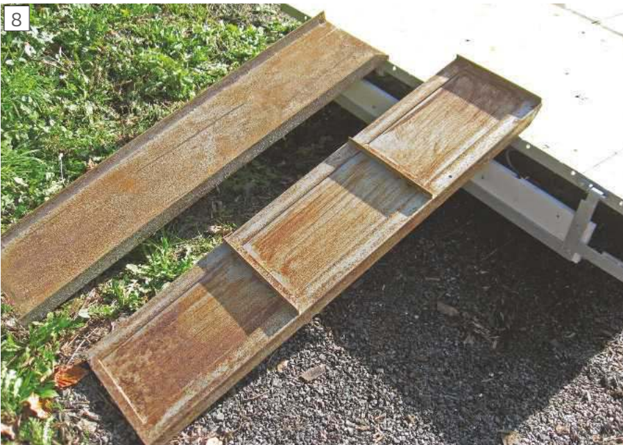
Reinforcement for the loading ramps.
