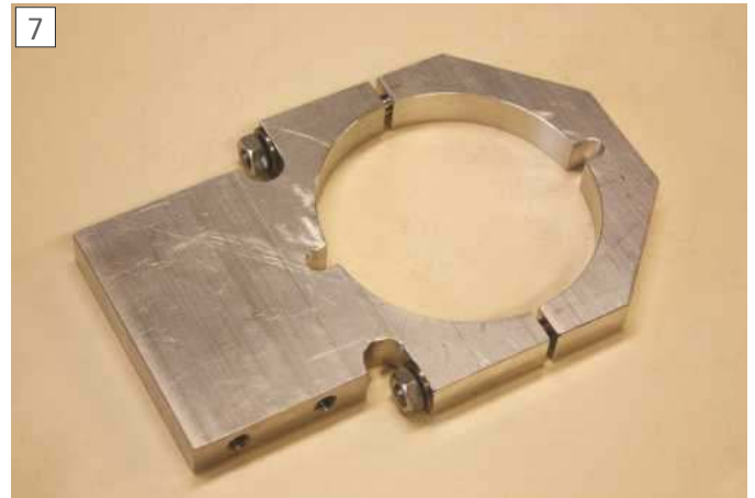
Upper clamp to support the bench grinder.
