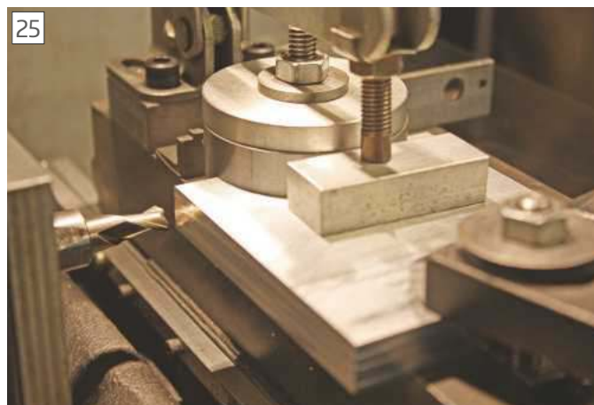
Milling tube clamps to size.
