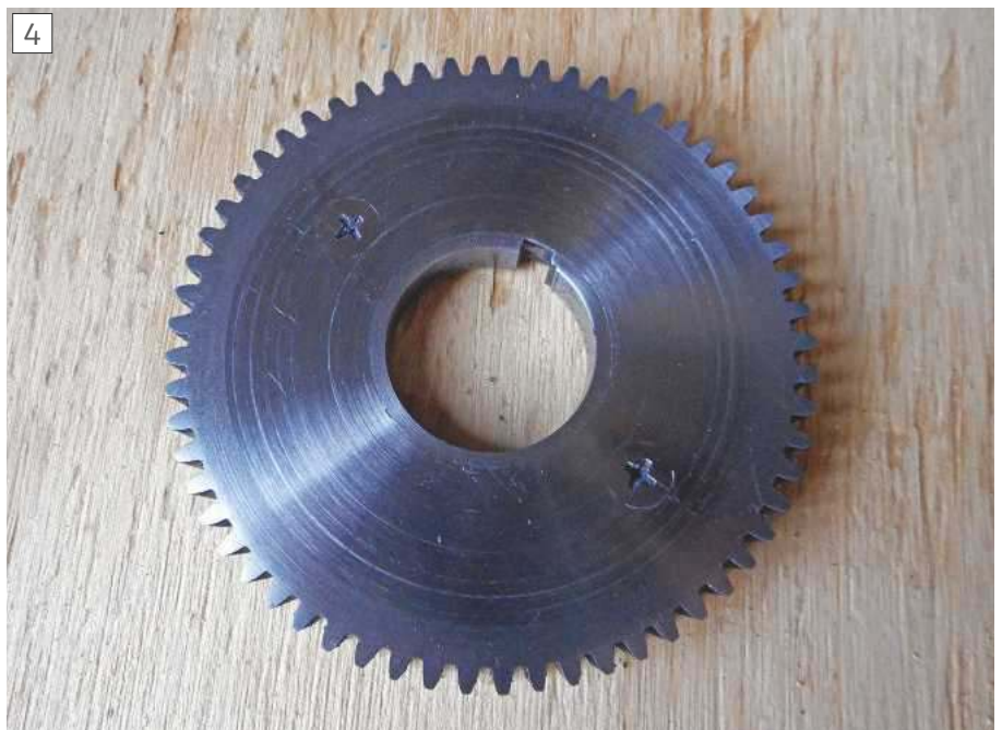
The gear after the recesses were machined out and filled with steel discs screwed and Loctited into permanent position.
