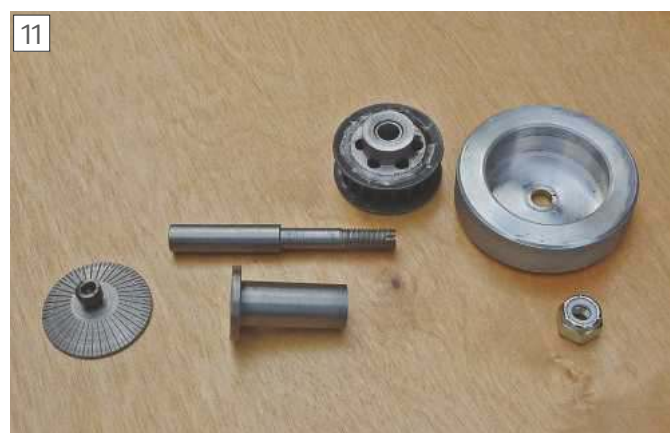
The master cam assembly components. The outer sleeve has already been fixed to the frame.
