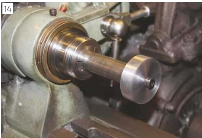
Main body tube internal support.
