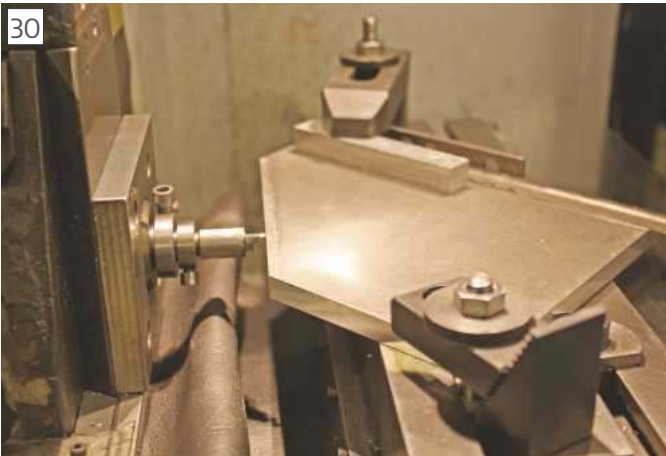
Milling side plates to shape and size.
