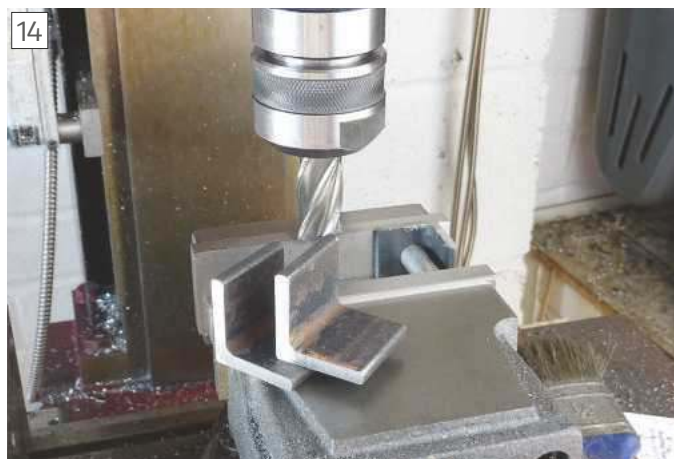
Machining the pivot brackets and tailstock angle square.
