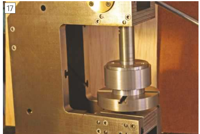
Pressing the taper roller outer rings into their housings.
