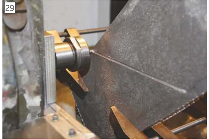
Cutting Aluminium plate for side plates with 1/8" diameter slot drill.
