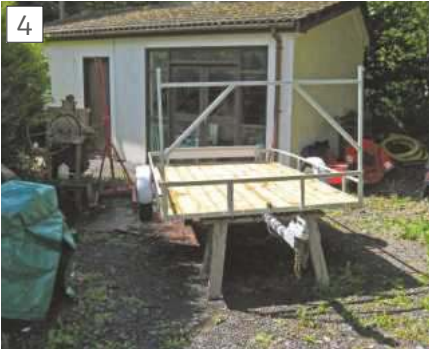
The ladder rack was reinforced with diagonal stays.
