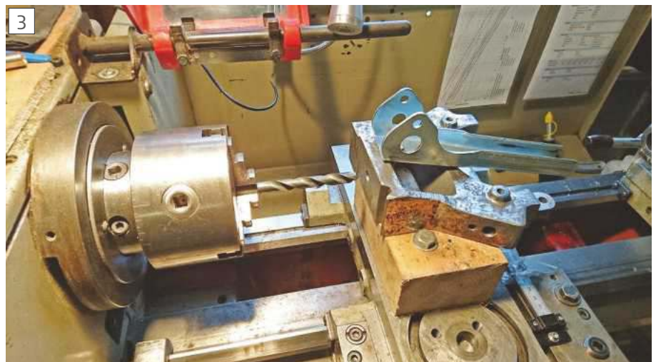
Holding the casting for drilling (staged photo)
