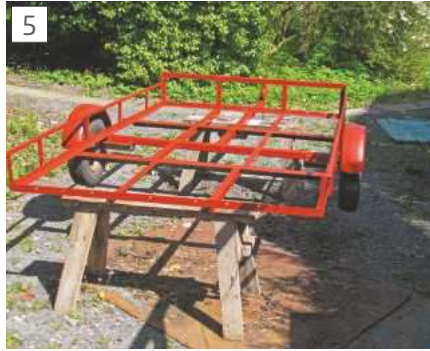
The chassis was cleaned and red oxide primed.
