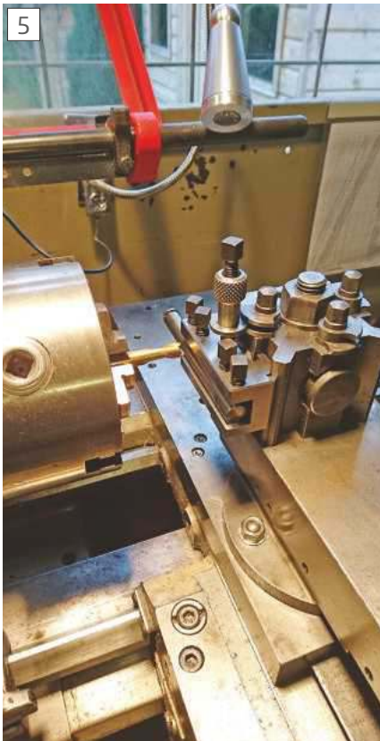
Starting to mill the flat on the fingers
