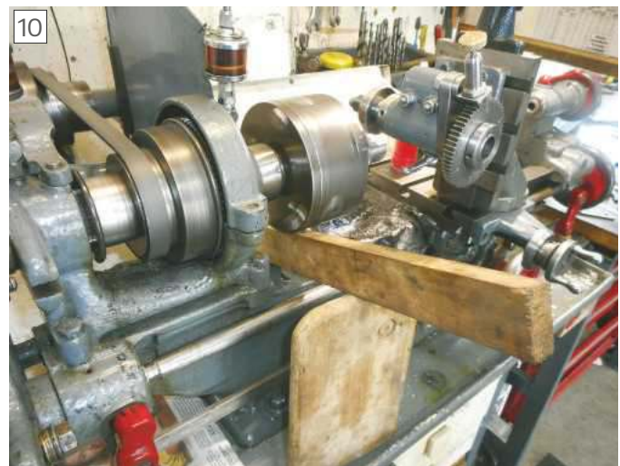
Old school wooden shock absorber smooths chuck rotation under interrupted cuts such as when milling gears. Belt guard for display only, not recommended practice.
