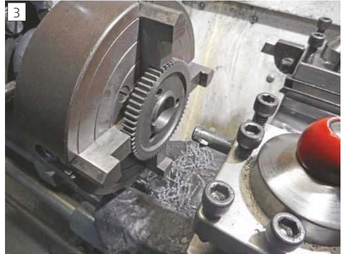
Cutting the keyway in the cast iron gear with a boring bar, using the lathe carriage as a slotting tool.
