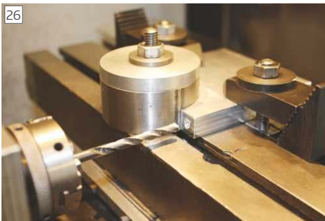
Drilling holes in clamps to accept studs.
