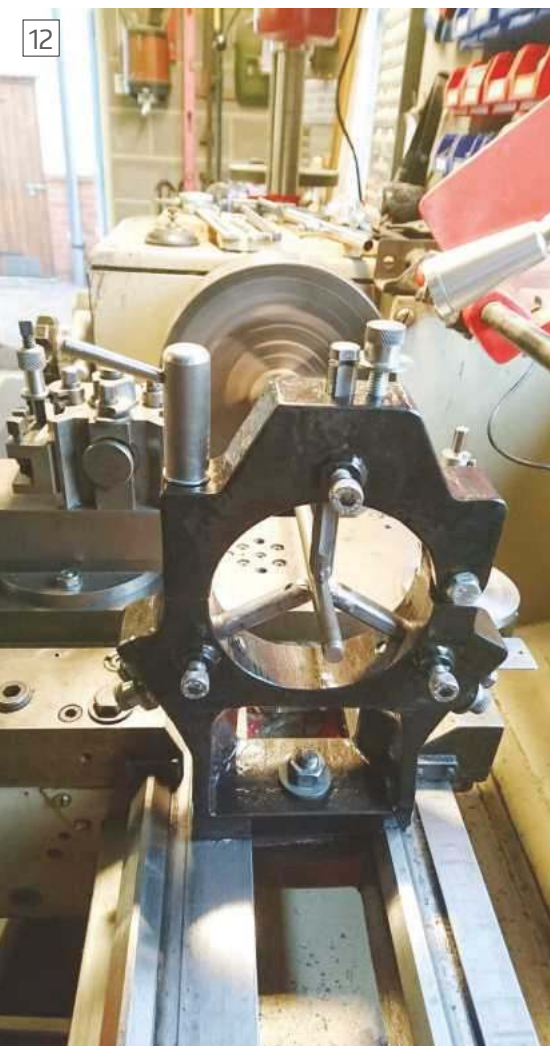
The completed steady in use
