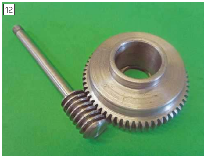
Result is a worm spindle that runs straight in line with the gear, just like on a proper worm wheel.
