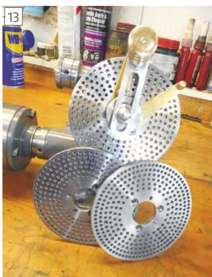
Gears proved highly accurate within one thou when drilling 814 indexing holes in the three index plates.
