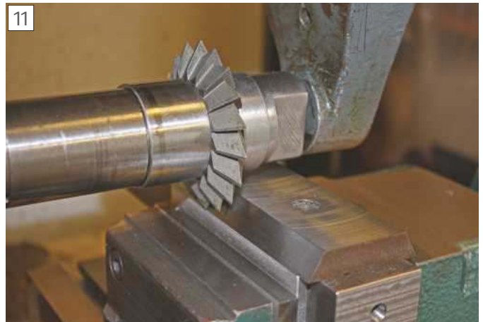
Cutting the angle on the clamp plate in attempt 2.
