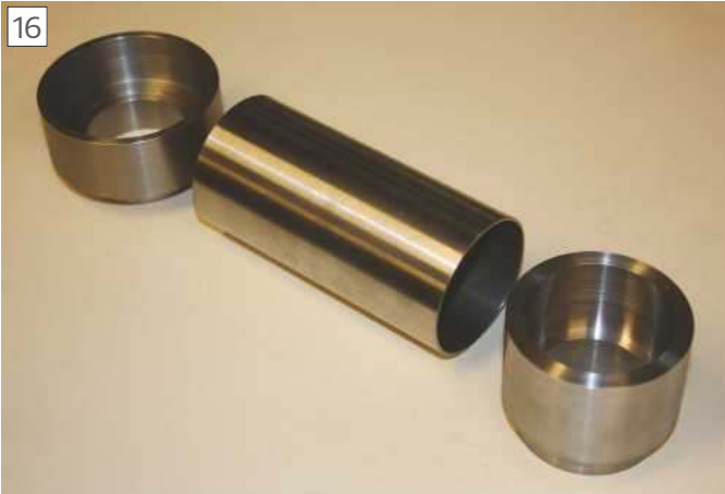
Main body tube with 2 bearing housings.
