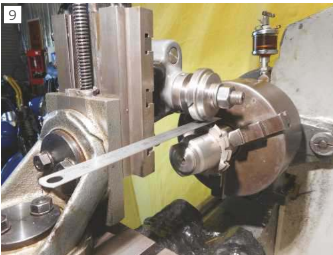
Centring cutter by the steel ruler method. Note borderline high position of vertical slide in this set up.
