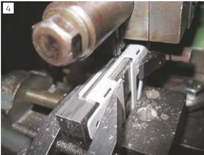
Holding G3 Axle Guards against a supporting block
