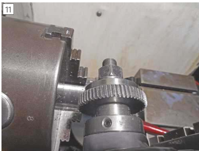
Gear teeth are straight but cut at a 4.2 degree angle to match worm thread helix angle.
