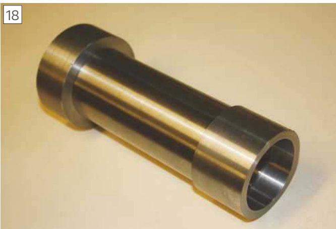
The bearing housings pressed into the main body tube.
