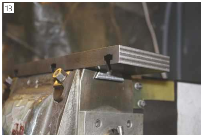
Base plate and clamp plate in the dovetail slot of the machine.
