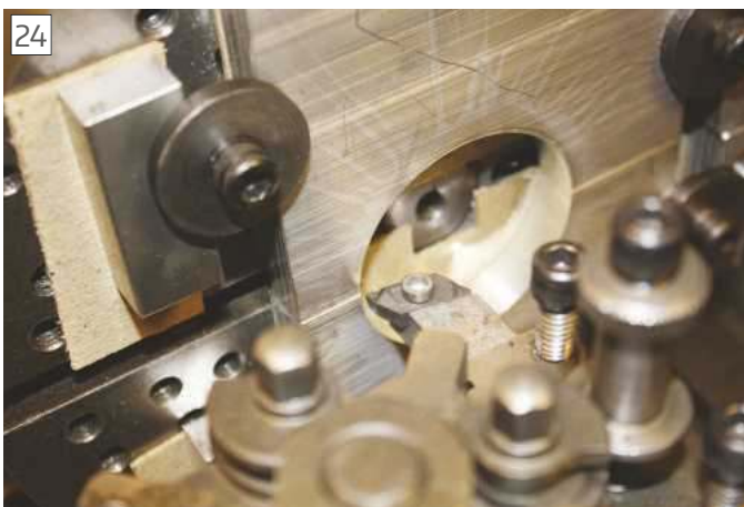
Finish boring hole in tube clamps.
