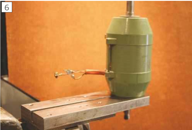
The bench grinder mounted on the base bars.
