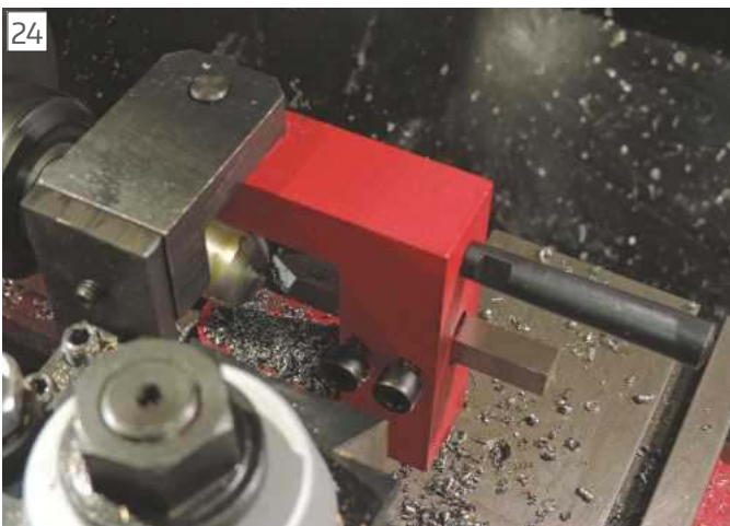
Do not take the tool past this position or you will 'dimple' the ball.
