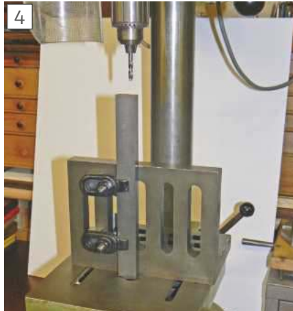
Posed photo showing the Clamp securing a large angle plate to the drilling machine to allow drilling into the end of a long bar - and allowing for adjustment of the angle plate to centre the drill.
