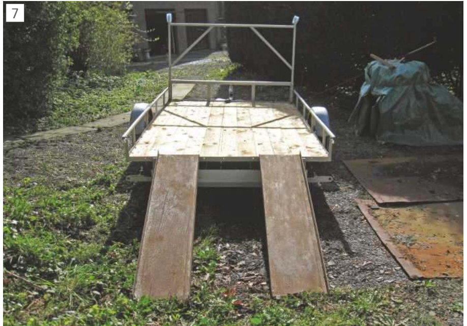
The loading ramps.
