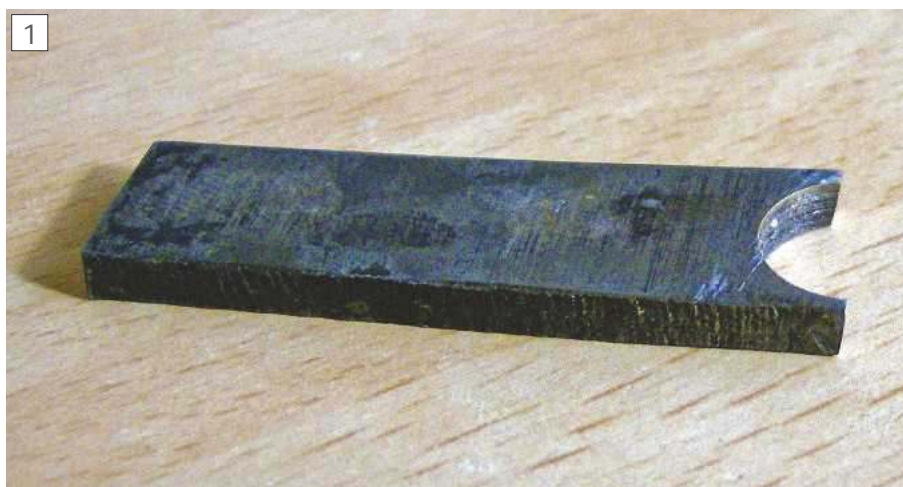
Simple form tool from gauge plate.
