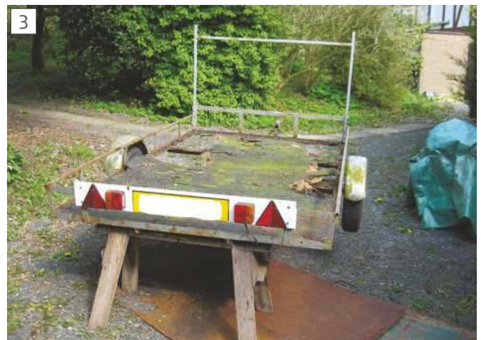
The trailer was raised to a comfortable working height on trestles.
