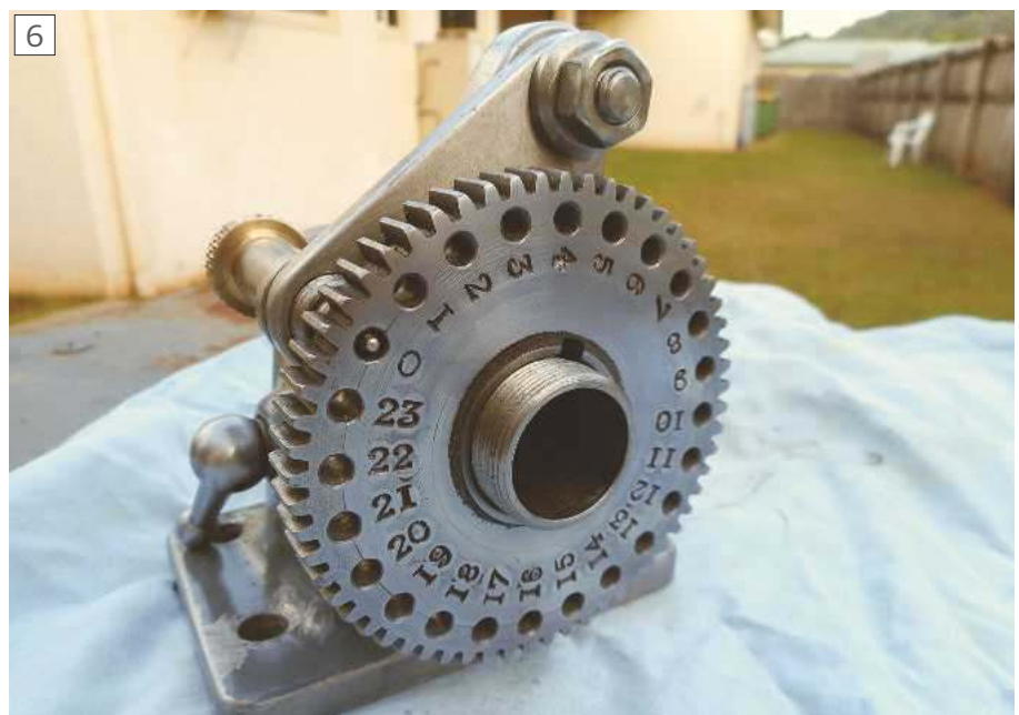
Steel plates remained intact during drilling of 24 holes and stamping of numbers on the modified gear.
