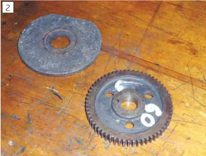
The 60T 20DP Myford change gear before modification, with one of the washers used to fill in the recesses.
