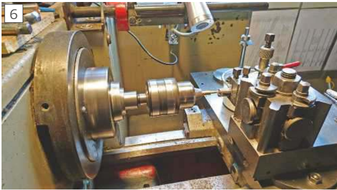
Milling the slot for the bearing
