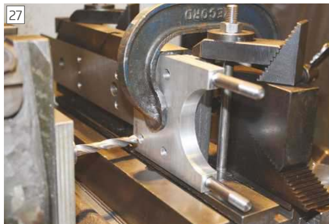
Drilling 4 holes in lower clamp for bolting to base plate.
