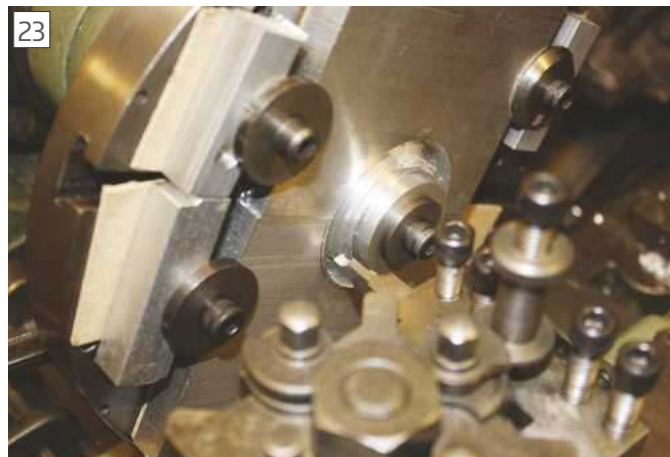
Trepanning hole in main tube clamps.
