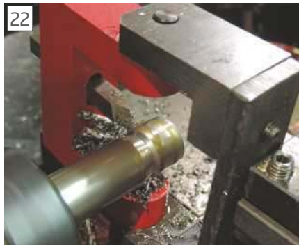
If a stalk has not been machined the tool will cut a rather long tapered shoulder.
