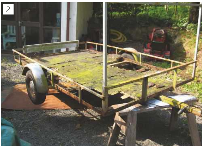
The floor of the trailer showed signs of rot...
