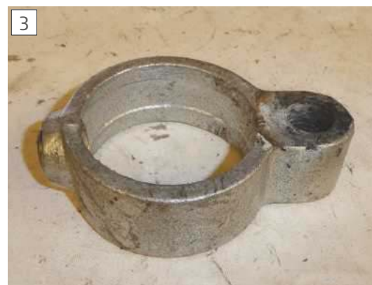
Scaffold gate hinge
