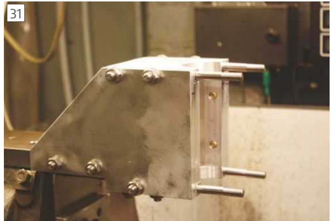
Clamp plates and side plates assembled on the base plate.
