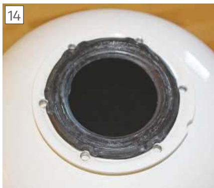
Gasket created by removing and trimming the rubber bladder from the expansion vessel.
