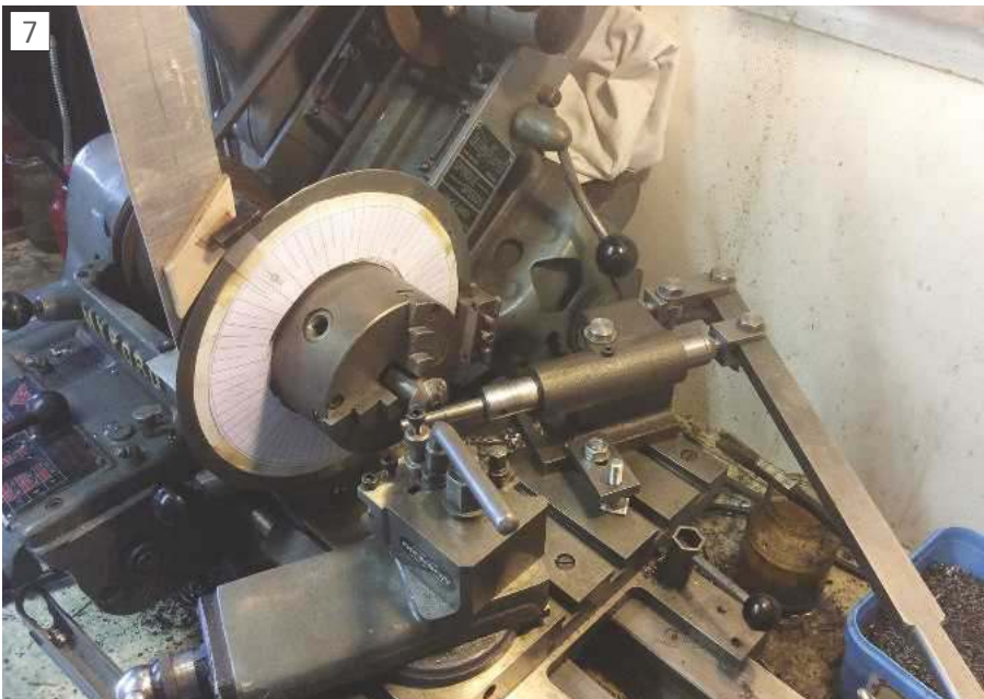
The set up used to cut the graduations on the protractor.
