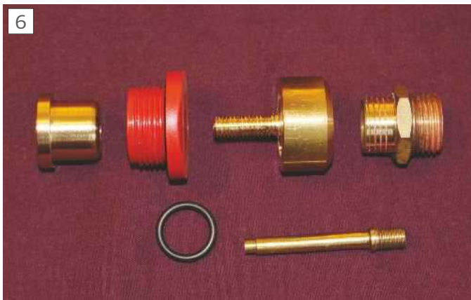
Brass parts, O-ring and core of the Schrader valve that were used to adapt the Primus bottle screw cap (red).
