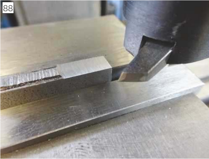
Small fly cutter in use on narrow work
