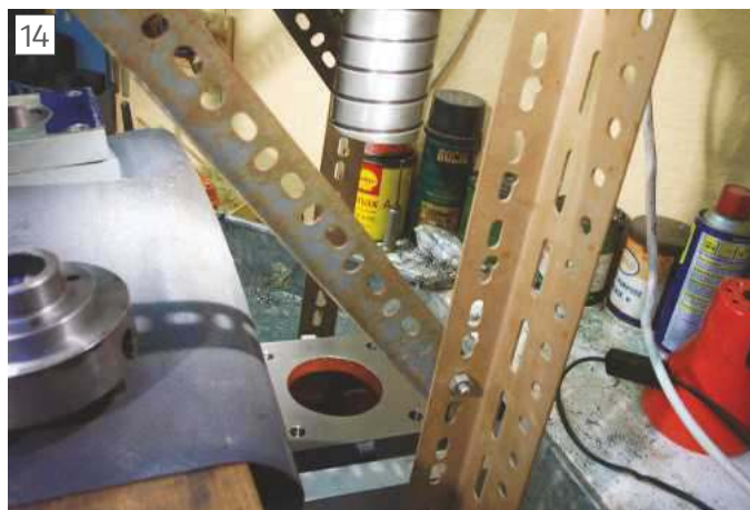
Mill work head supported on Dexion frame
