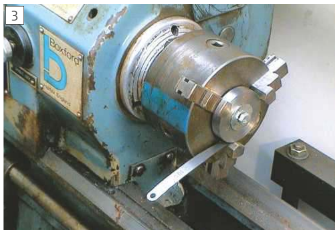
Checking for gaps with a feeler gauge
