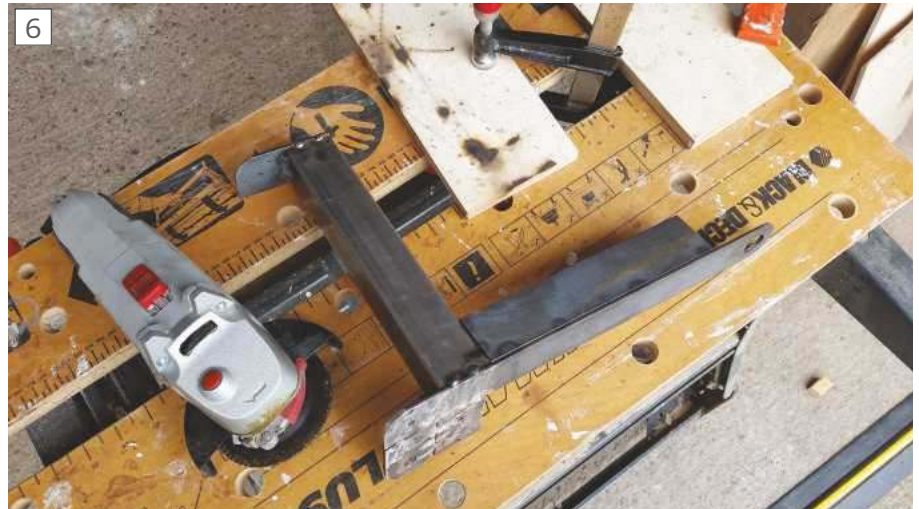
Grinding weld beads flat.
