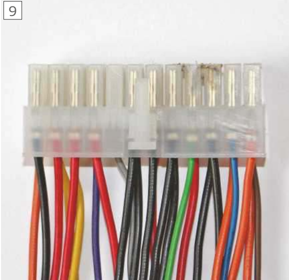
24 pin ATX connector. Connect the green wire to one of the black wires (0V) to switch on the supply. 12V will then appear on the yellow wires when the mains is switched on.
