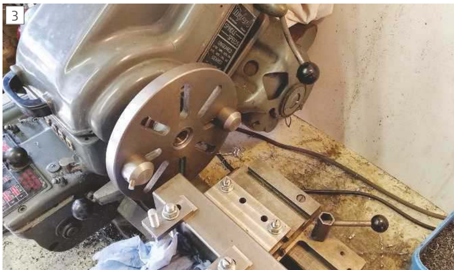
Machining the ends of the tube square in the lathe using a faceplate fly cutter.
