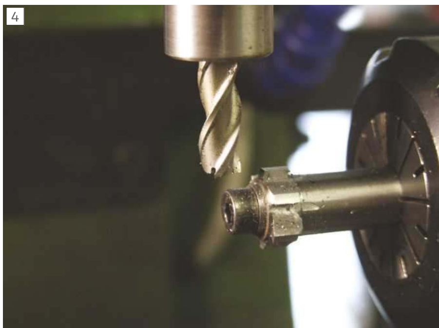
Milling the primary clearance angle (10 degrees)
