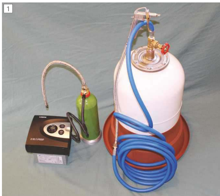
The completed mini air duster, left, and the maxi air duster, right. The Wolf compressor is shown fitted to the ATX power supply.
