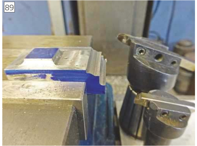
Profiles produced with single point fly cutters
