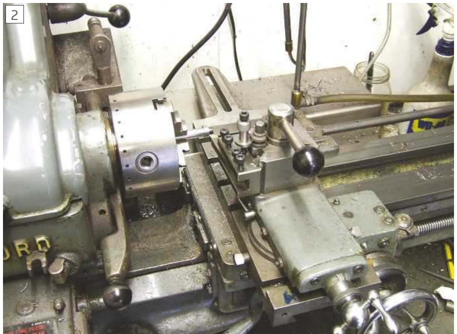
Machining the cutter to width and creating the 2 degree side clearance angle
