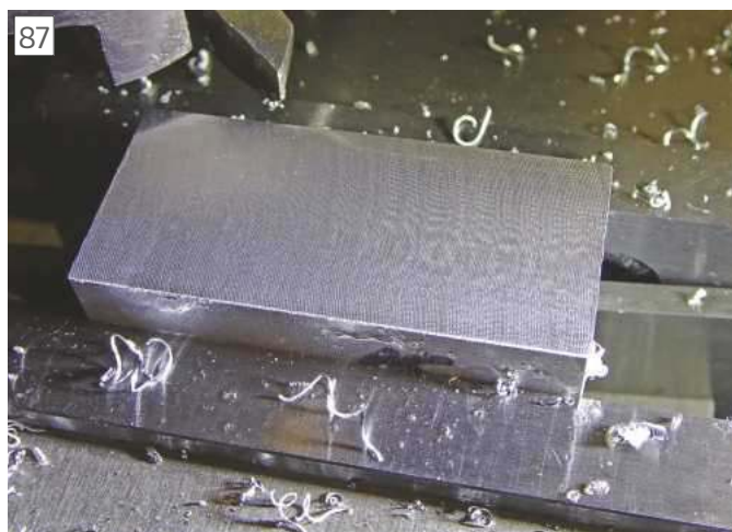
Double cut "trammed" finish
