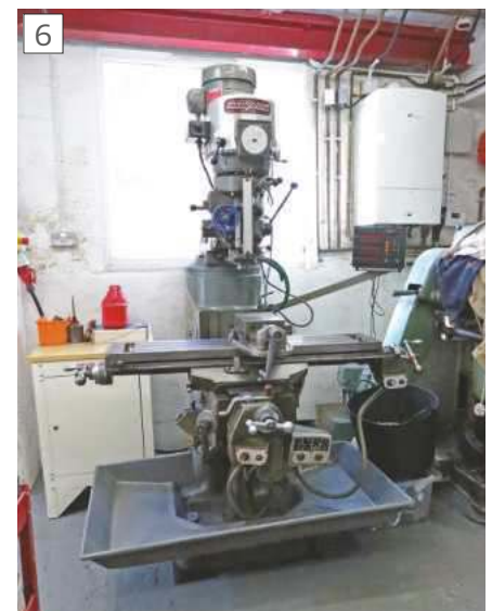
Bridgeport vertical milling machine in the workshop, one of several millers (Mike Chrisp).
