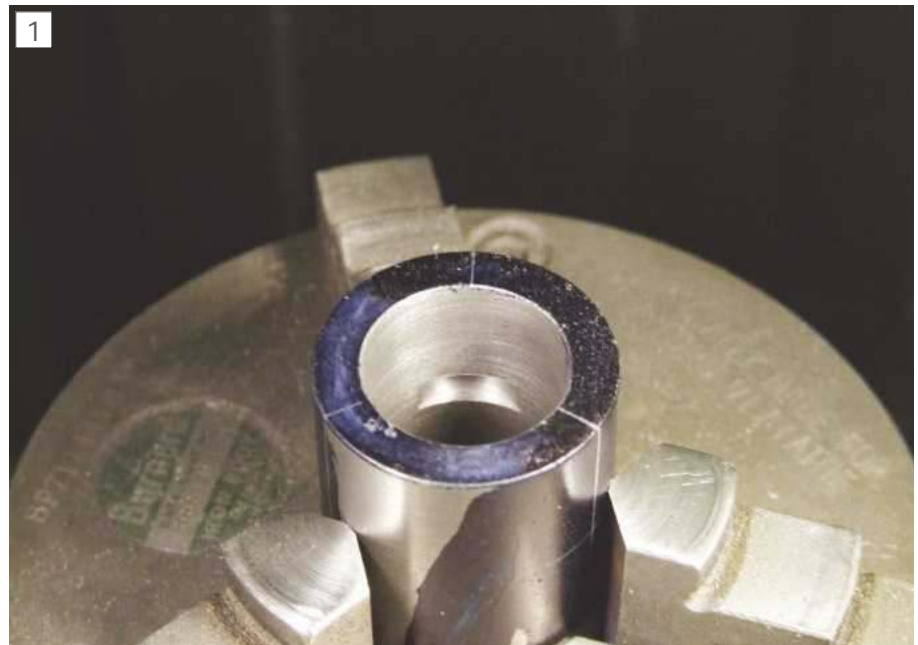
The challenge was to machine the pockets in the bore of this component
