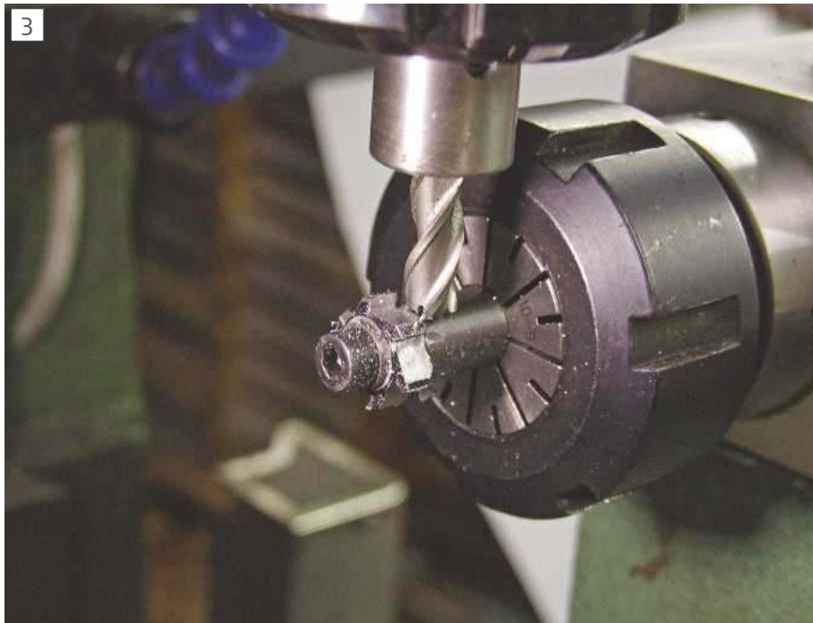
Milling the radial rake angle (5 degrees)
