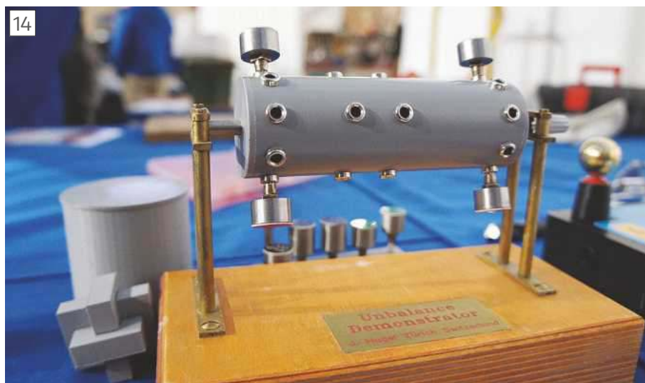
14 An unbalance demonstrator created by Professor Joerg Hugel of Switzerland, one of many items of experimental and demonstration equipment built by members.
