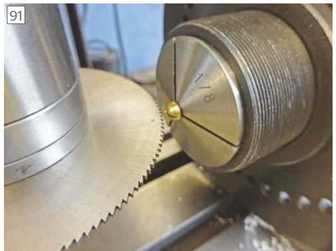
Slitting a screw head with a fine toothed blade
