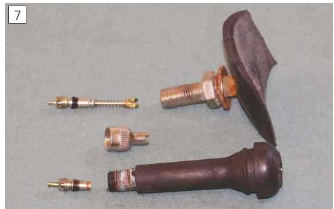
Different types of Schrader valve: tubed, top and tubeless, bottom.
