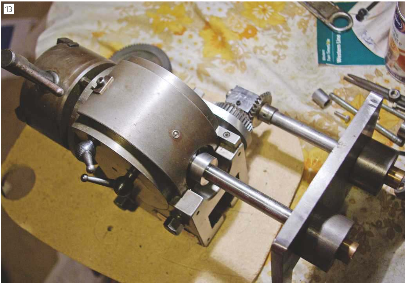
The backing plate is being fitted onto the two shafts.
