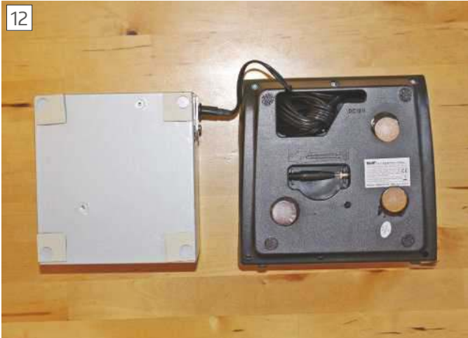
Three low-profile rare earth magnets and four corner sockets glued to the ATX case comprise a simple detachable coupling between the pump and power supply.
