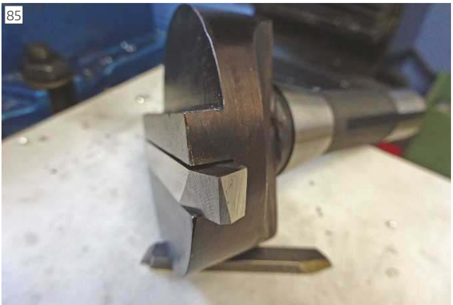
Suitably ground toolbit mounted in flycutter
