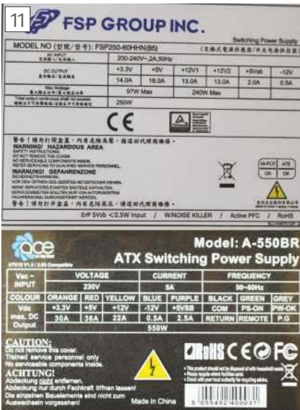
Top: older type of ATX power supply that lists the two separate 12V1 and 12V2 outputs. Bottom: more recent supply that outputs only one 12V line.
