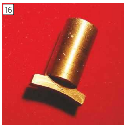
The cracked key
