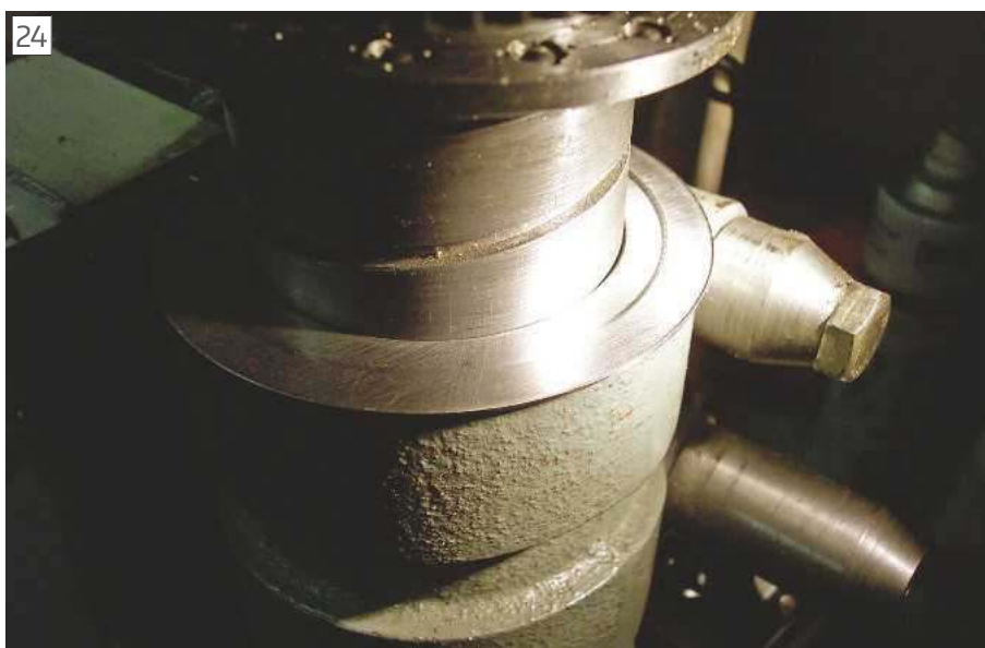
Rolling track marks on thrust bearing washer
