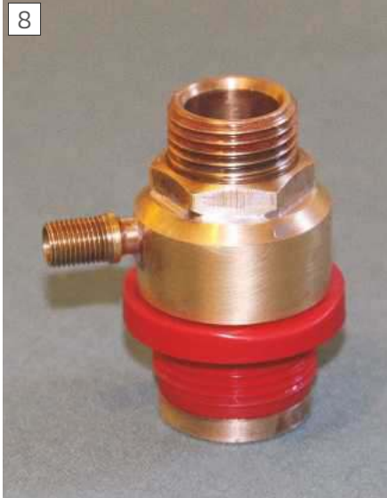
Modified Primus bottle cap, showing Schrader inflation valve and BSP union that connects to the braided tail.
