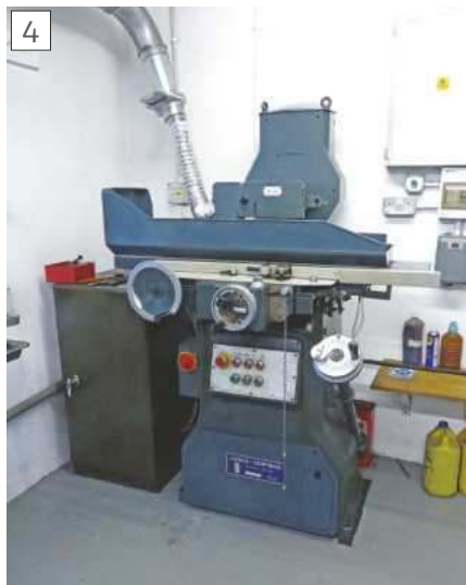
Jones and Shipman surface grinder with dust extraction equipment in a room devoted to grinding equipment (Mike Chrisp).
