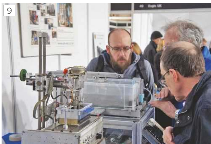
9 Demonstrating the SMEE wire eroder at an exhibition. This was a group project by the Digital Group. An earlier plunger (or single access) spark eroder stands in front.
