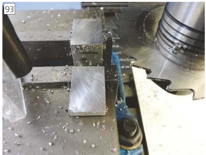
Finish left on parts after completing the cut
