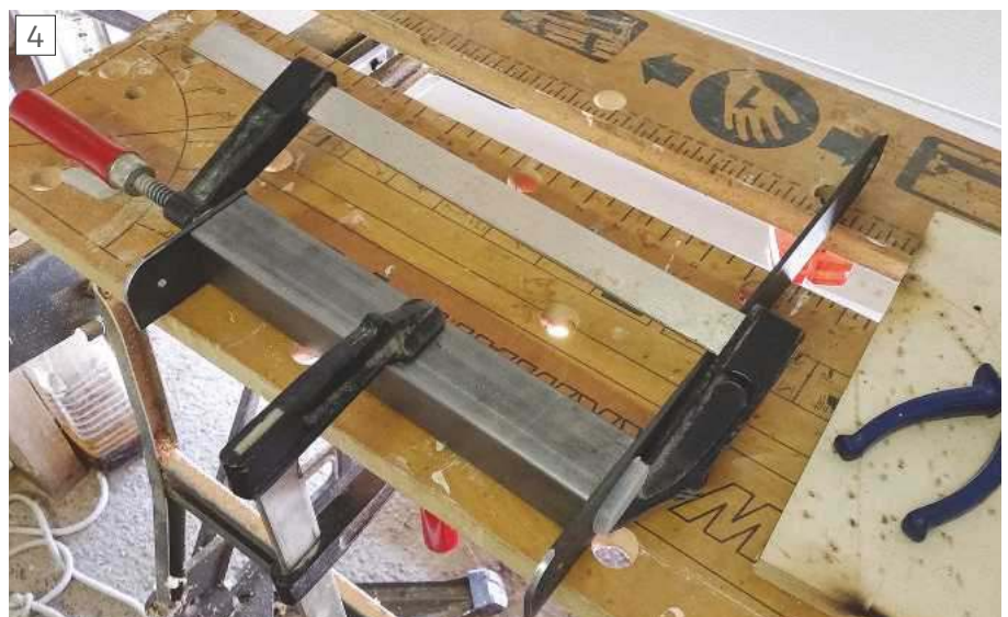
Clamping frame components together ready for welding.
