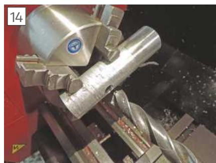
Using a 4-jaw chuck to hold a tube centred across the axis of the lathe.
