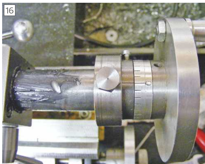
The extra collar with the fiducial mark.
