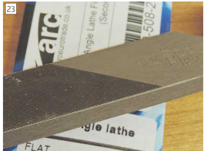
A close up of the file's cut showing a 'safe' edge.
