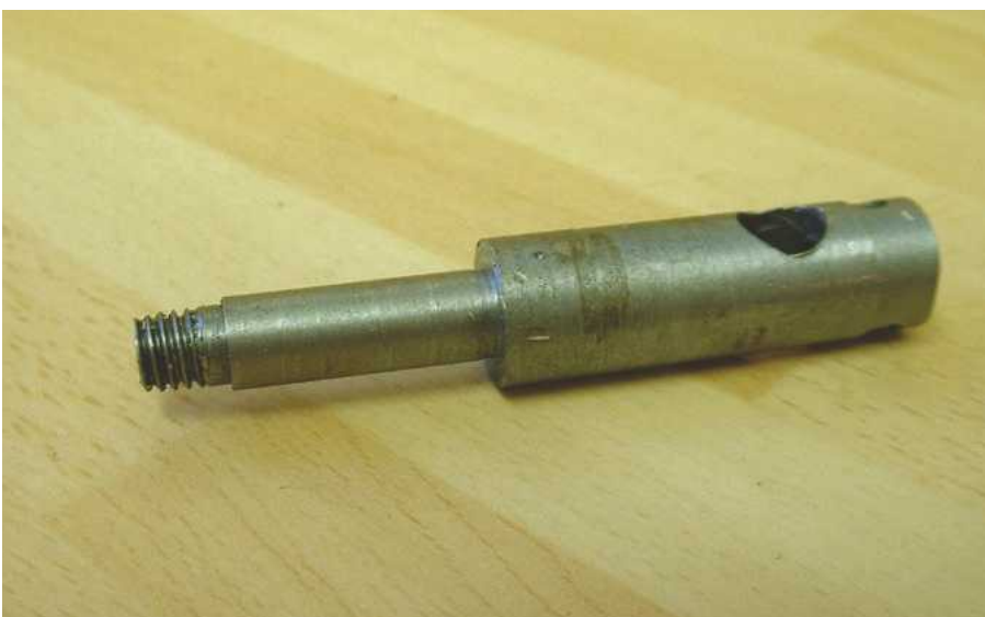
A basic screwed mandrel, use it and recycle it!
