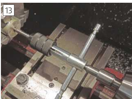
Tapping complete, note how the pump centre has extended.
