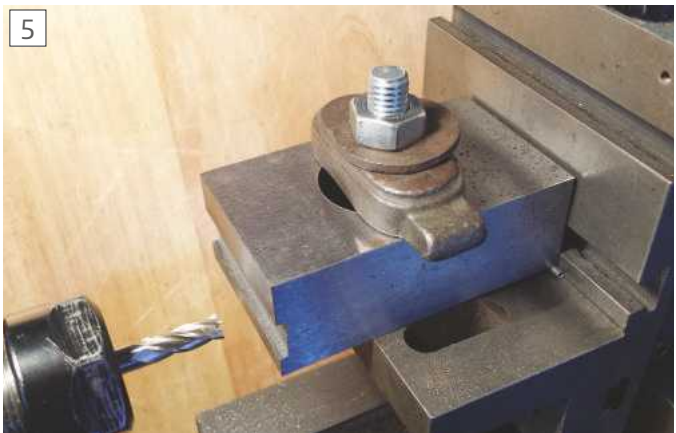
Milling the slot for the parting blade.
