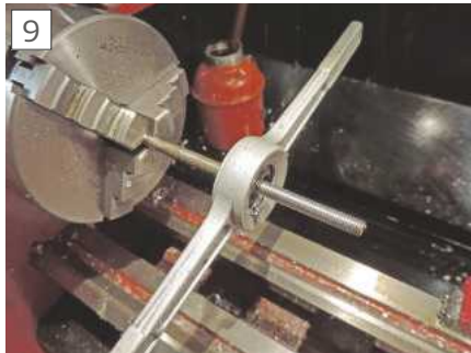
9 The thread was finished by running a die along the thread.
