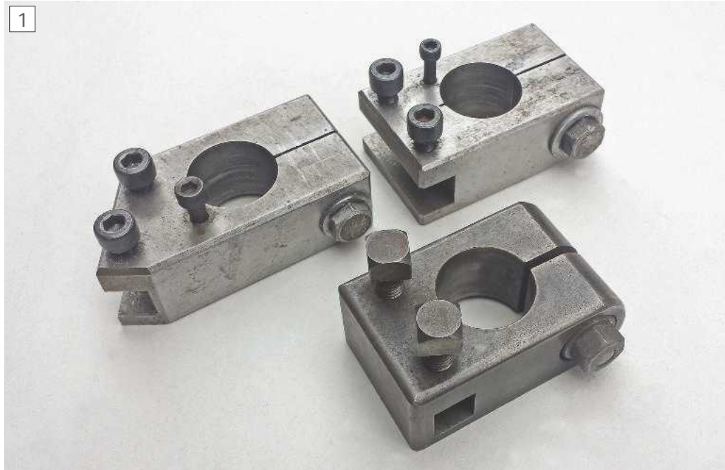
The standard Drummond tool holder with two home made variants.
