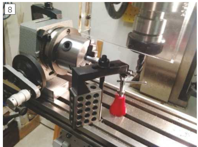
Supporting the spindle to allow milling the outboard end
