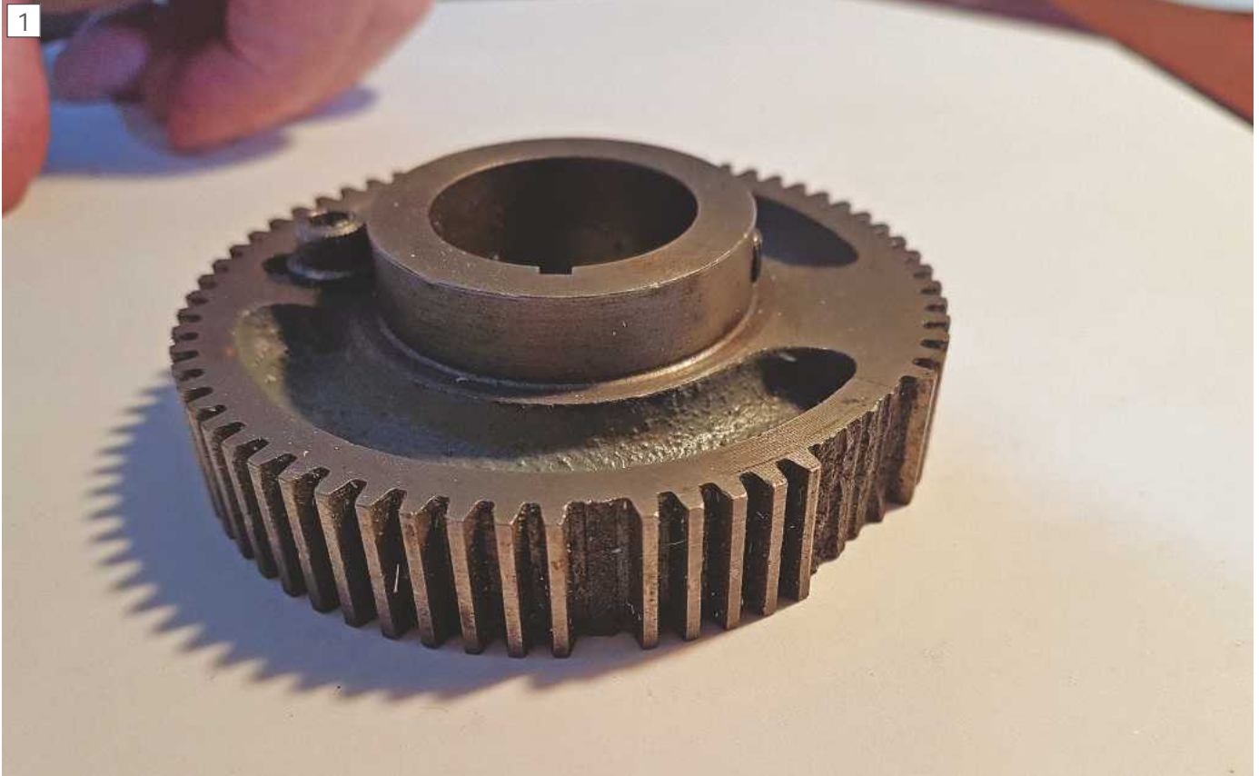
The broken back gear
