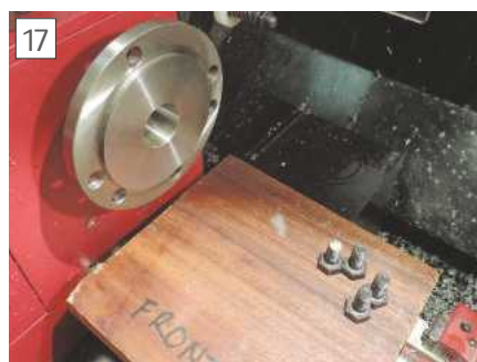
The SC4 spindle flange, note the fixing bolts with low-profile heads.
