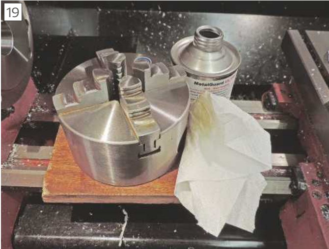
The 4-jaw chuck treated with MetalGuard.
