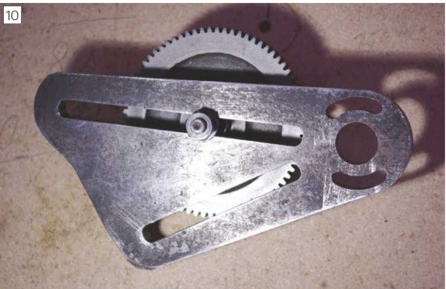
Change wheel quadrant with a pin fitted in the slot.
