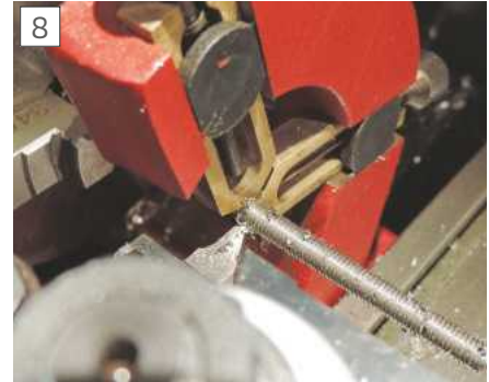
8 Taking a second cut, the steady happily works on the top of the emerging thread.
