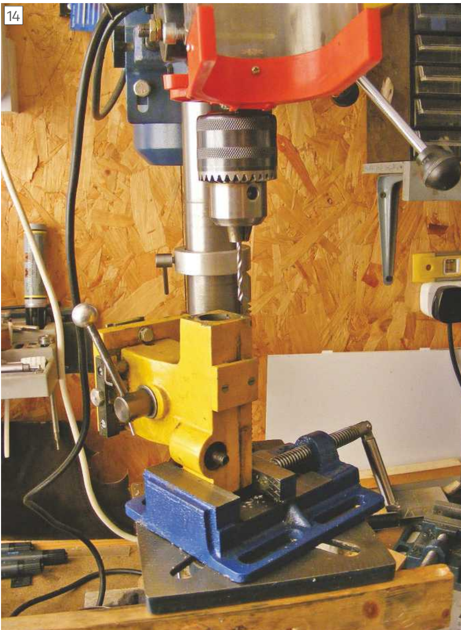
Drilling the tailstock.
