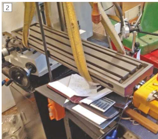
Assembling a long bed to the mill
