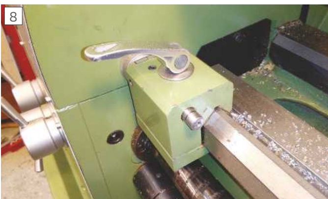
The cycle wheel lock used as a saddle stop lock
