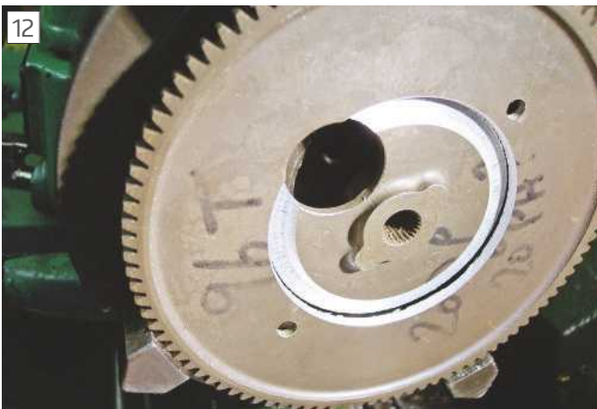
Gear centre being trepanned out
