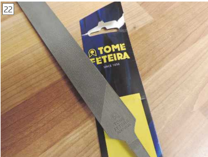
A proper lathe file.
