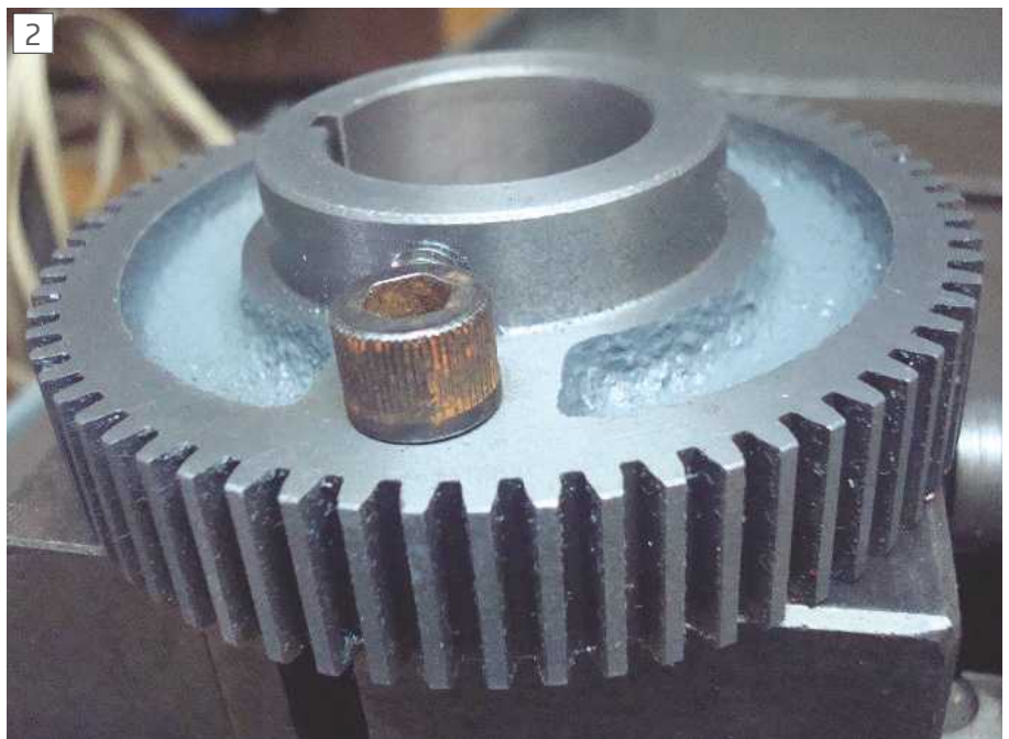
The cap screw in place, you could use M8 instead of 5/16" UNC.
