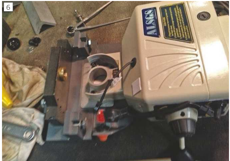
The feed pinion is just visible near the wire emerging from the unit
