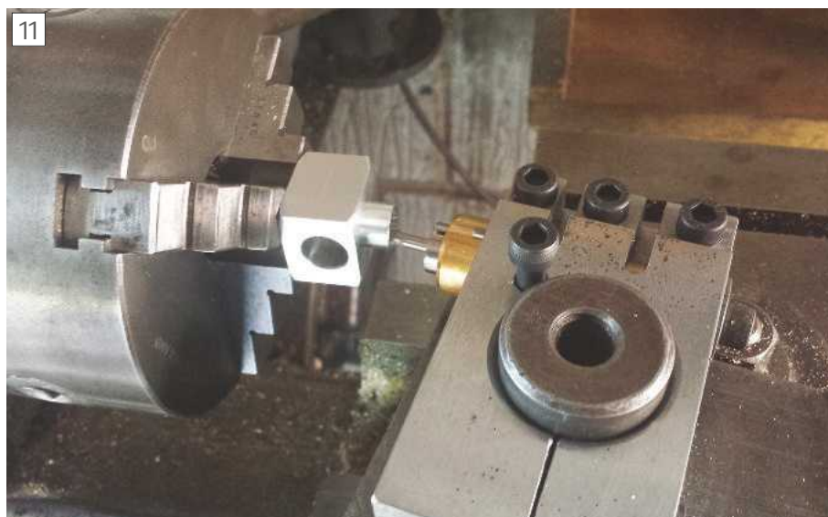
Boring the air intake taper on a small carburettor.
