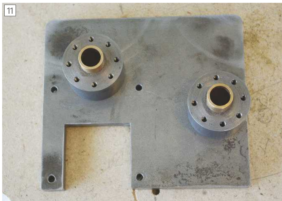
Back plate with bosses fitted. The main shaft boss remains fixed but the bevel shaft boss needs to allow for adjusting the mesh on assembly.
