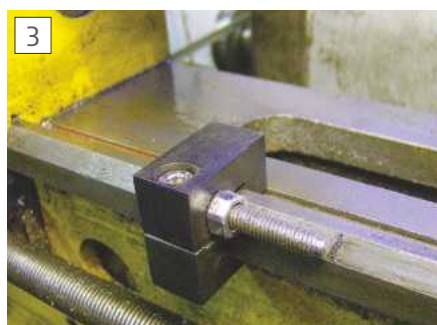
A simple shop-made bed stop.
