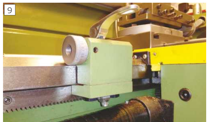
Another view showing the fixing underneath the saddle stop block
