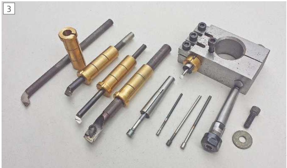
The new boring bar holder and accessories.
