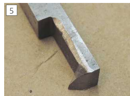
This stock HSS threading tool has had extra clearance ground below its tip.
