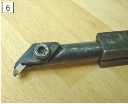
6 A 3/8" (~10mm) shank boring bar with a 1/8" (3.2mm) inserted tool ground for cutting a fine thread up to an internal shoulder.
