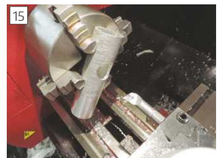
The boring tool has an angled tip which needs to be set at centre height for best results.
