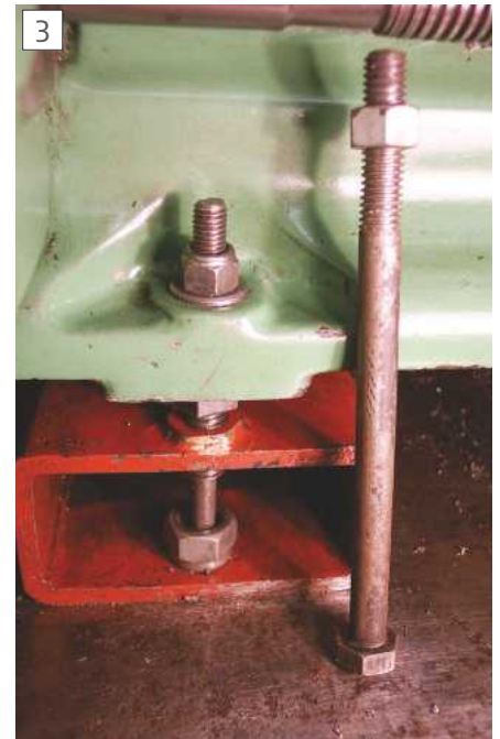
Lock nut released and similar long bolt shown
