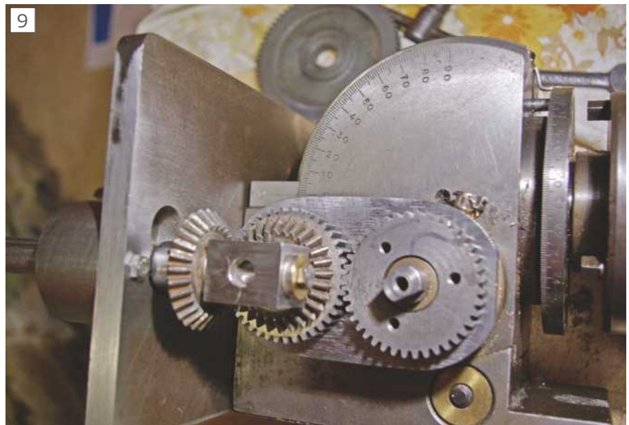
Bevel plate attached. Screws should not be fully tightened yet.
