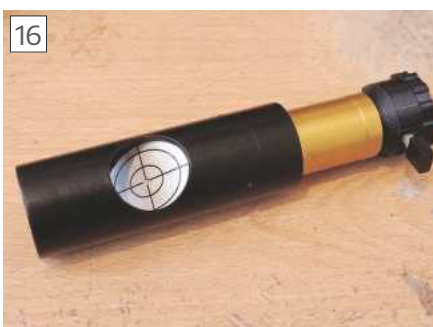
This laser collimator was made with the same technique, but with an independent 4-jaw chuck.
