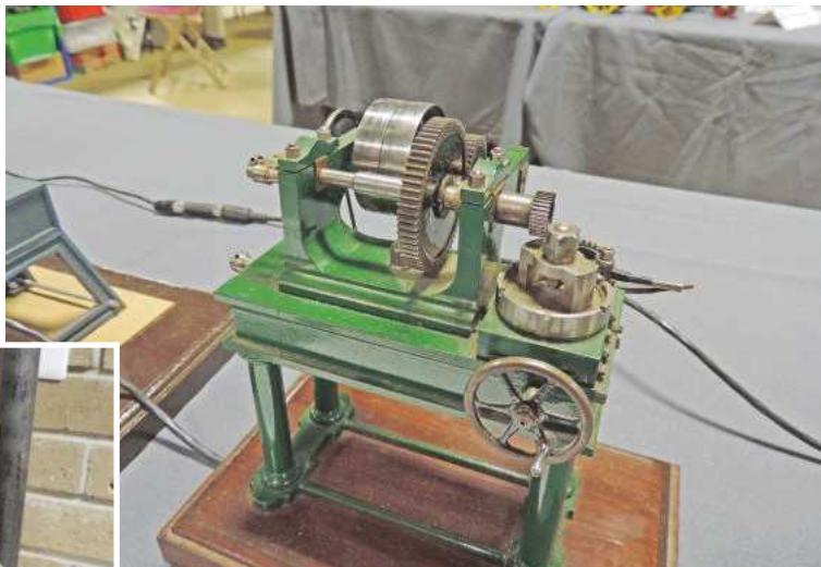
Maurice Turnbull exhibited several of his wonderful models of Victorian machine tools. This model is Archibald Milnes' nut cutting machine of 1840. Early milling cutters often had very large numbers of teeth compared to modern ones.
