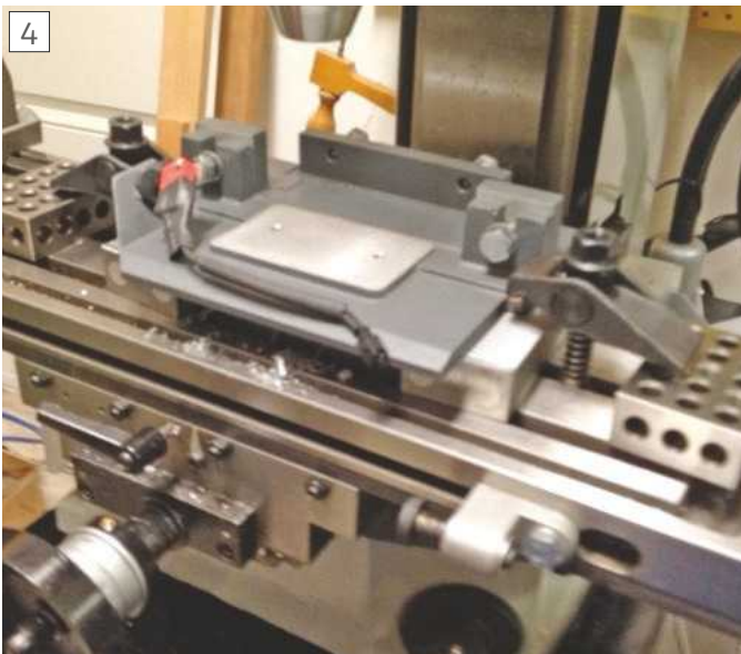
Milling off excess material from the adaptor casting
