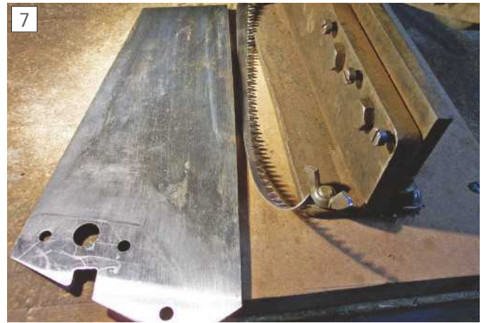
Teeth sheared off wood saw
