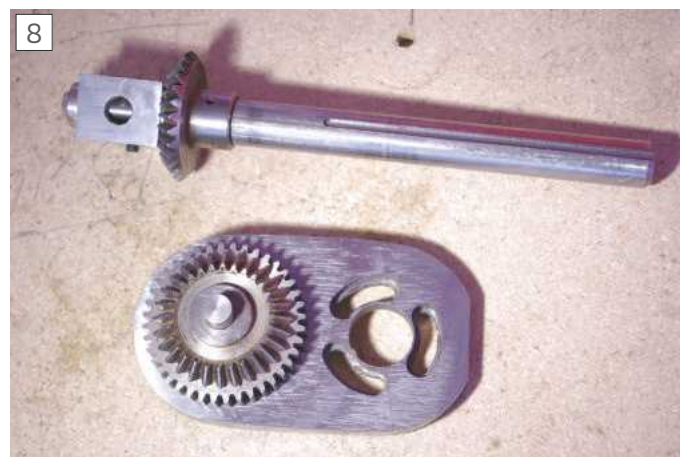
Bevel shaft with bevel block attached above. Bevel plate with bevel gear and forty tooth gear on pin below.
