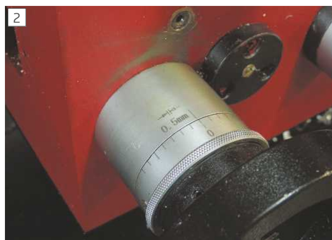
The handwheel dial on the SC4 reads to 0.5mm, but you can easily stop the lathe within 0.1mm.
