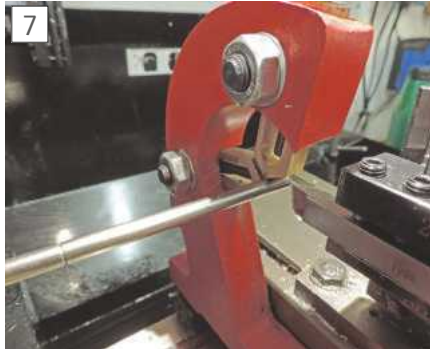
7 Using a steady to support a long workpiece for threading.
