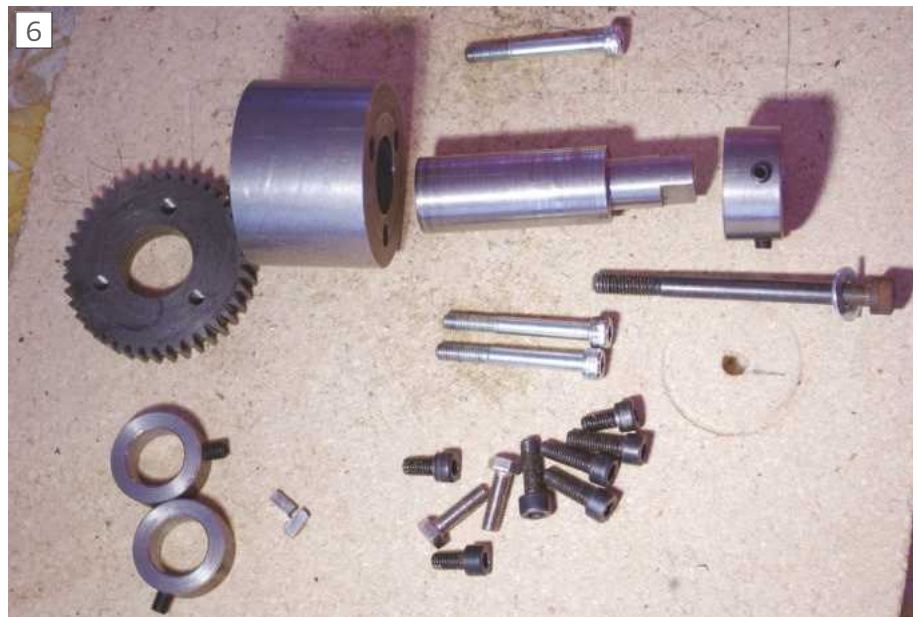
Left to right above are the 40 tooth gear, the spacer, the input shaft extension, and the collar to retain the dividing arms. The three plated Allen screws fasten the dividing plate and spacer to the gear. Collars for the change wheels to the left below with two keys. M5 fasteners for assembly.
