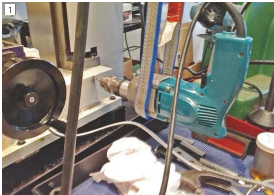
Using a sling to support a power drill
