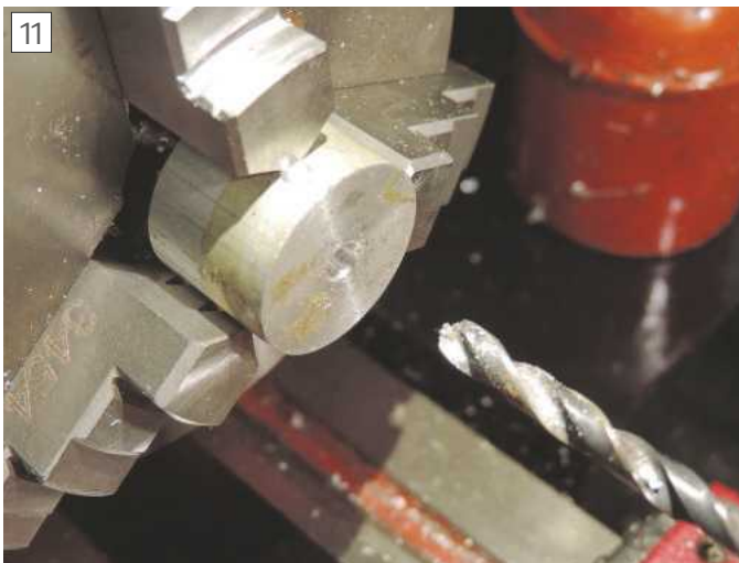
Hole prepared to tap M6.
