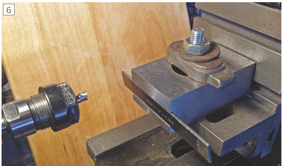
The fly cutter for the slot and the parting blade in place.
