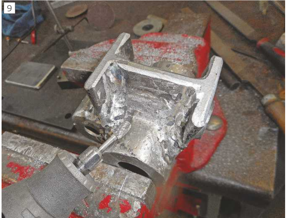
The welds on the stand webs are ground smooth before welding on the base plate. This allows much easier access for the grinder.
