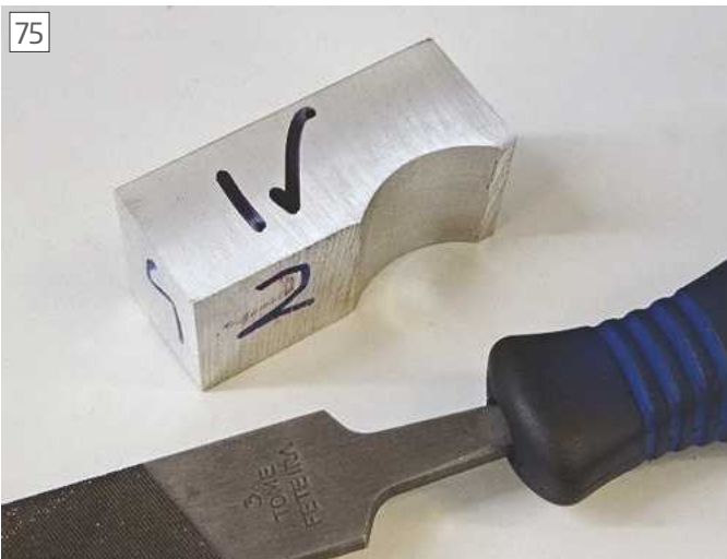
Face 1 after machining and De-burring with File
