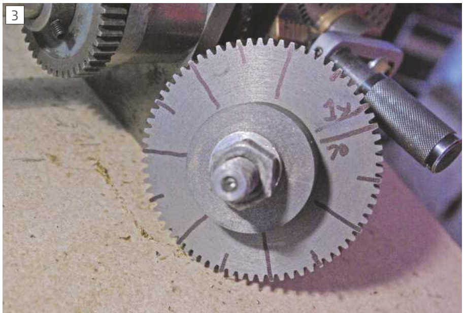
Proof of the pudding, a gear with 71 teeth.
