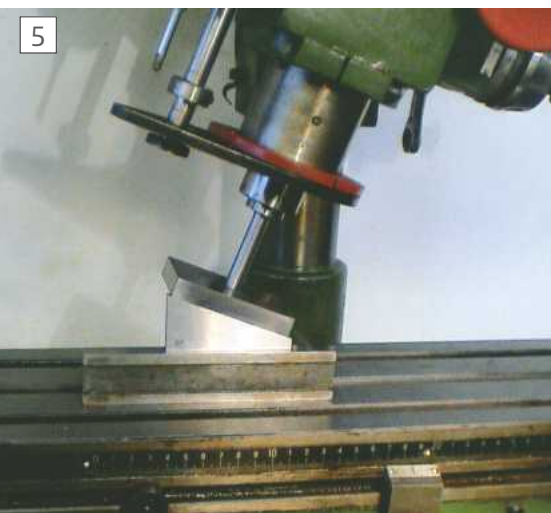
Using the platform with an angle gauge
