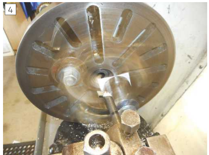
The offset job rotates around the boring bar as the scallop is machined. Ensure there is enough clearance before starting lathe.
