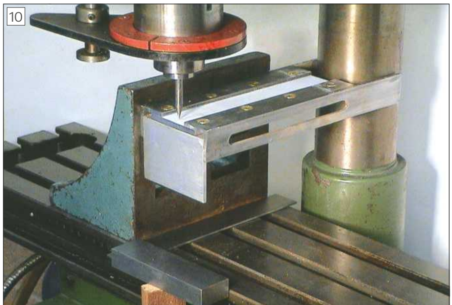
The indicator fits around the column
