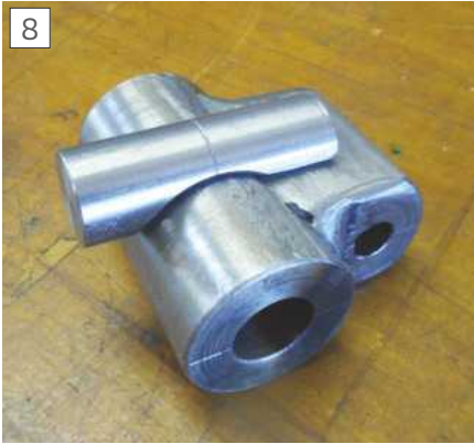
The main spindle lock barrel has the scallop turned in the lathe, then is positioned ready for clamping and welding.
