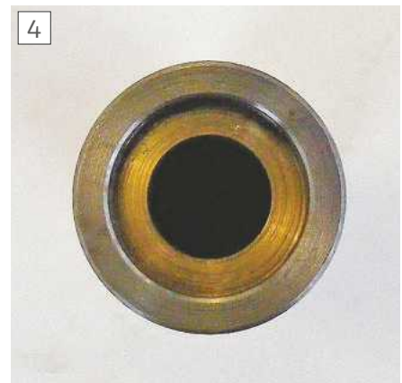
The auxiliary sleeve showing the recessed bush
