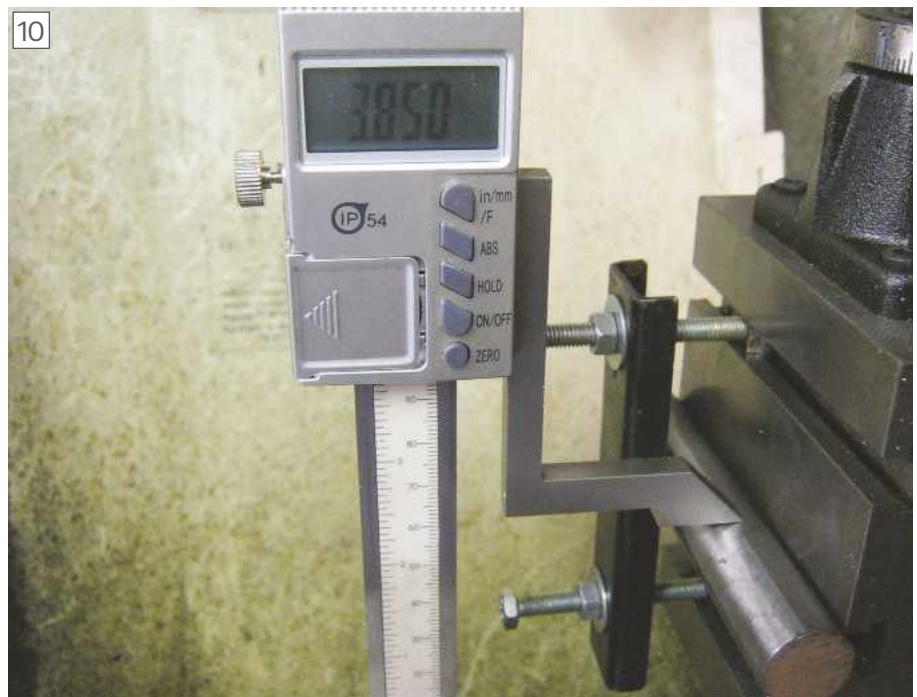
Setting a work piece mounted on a vertical slide to lathe centre height.
