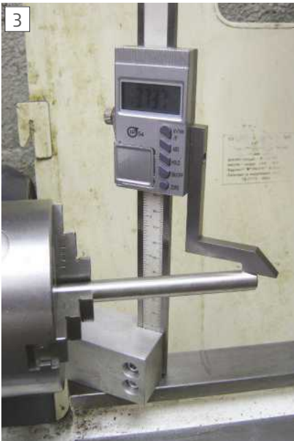
Using a piece of silver steel and a Digital Height Gauge to calculate centre height
