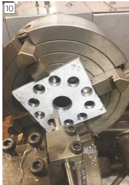
Boring the index Plate.
