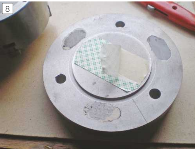
Holes filled with epoxy steel.
