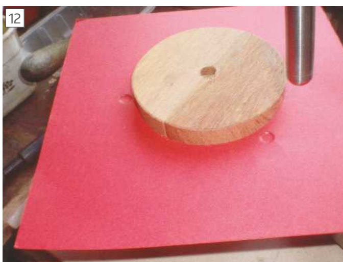
Marking out the hole locations.
