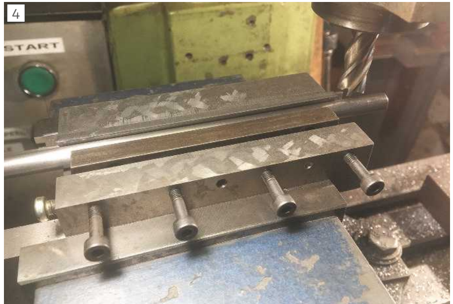
Machining new Gib Strip.
