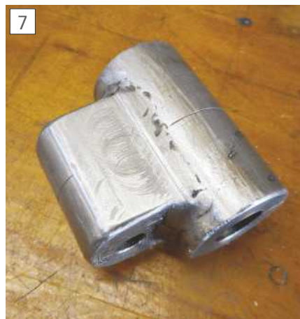
The top and bottom of the smaller tailstock clamp barrel are milled flat and blended to the main body with files and rotary grinder.
