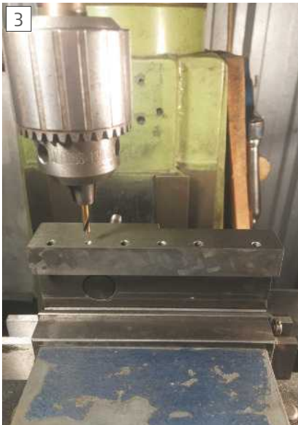
Drilling addition screw and dowel holes in slide.
