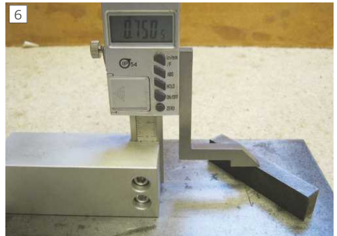
Measuring the thickness of a block prior to scribing a centre line along it
