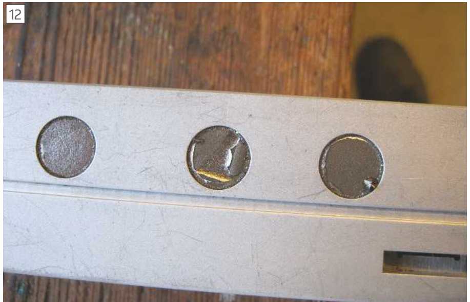
Plating coming off and swarf stuck to the magnets on the base of the Digital Height Gauge
