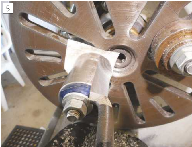
By taking light cuts, the boring bar is brought out to meet the marked out radius line for the scallop. Piece of paper provides extra grip.
