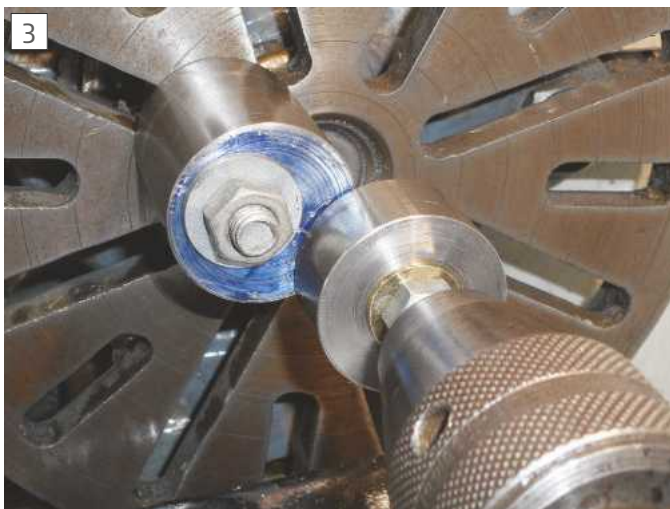
A slice of 1 5/8" bar held in the tailstock is used to position the marked out scallop ready for boring to the correct radius.
