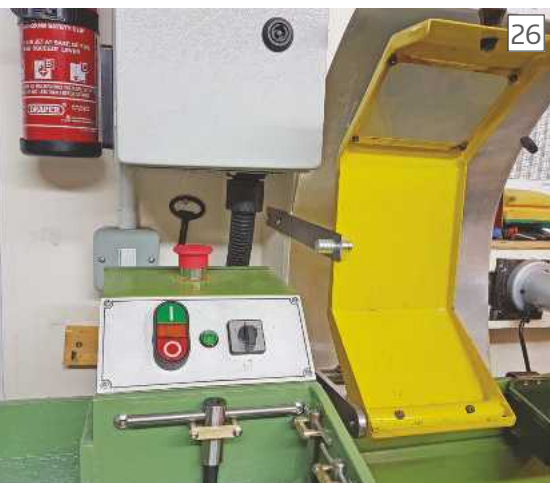
Chuck Safety Cover restrained clear of the chuck
