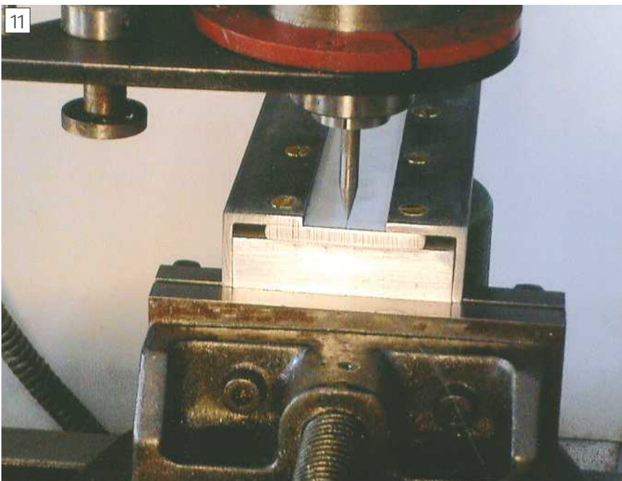
Using the indicator to check vice jaws
