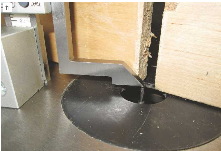
Setting depth of cut on a router table
