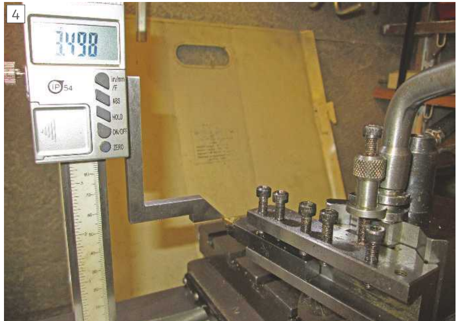
Using the calculated centre height to set the tool height
