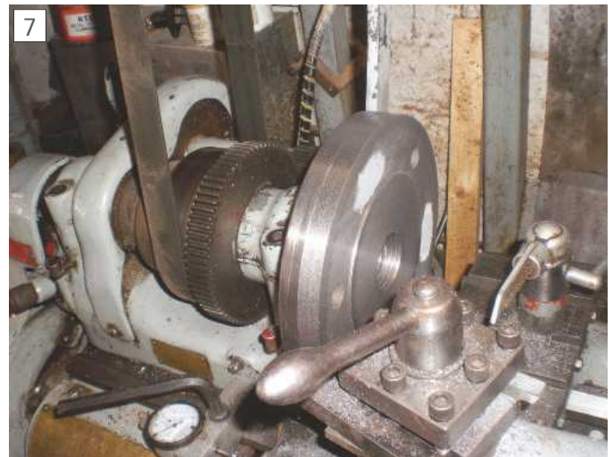
Skimming the mounting face.
