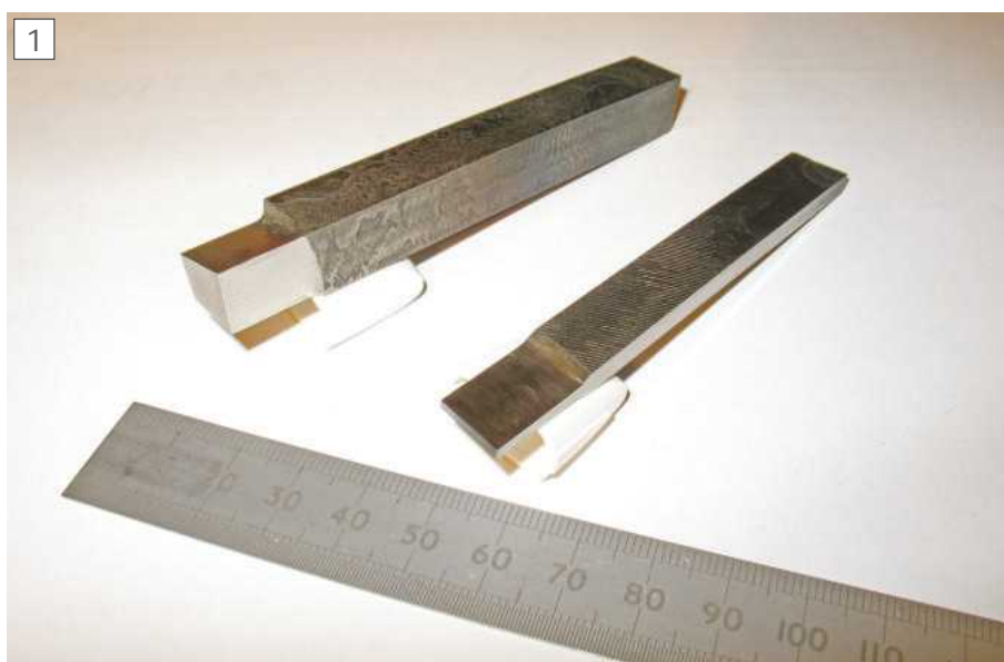
The two tools mentioned in the text. Note the grain swelling on the knife tool caused by overheating, the rough surface from the milling tool, and the tempering colours.
