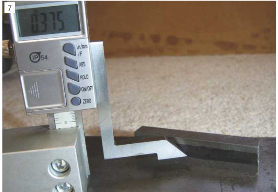
Scribing a centre line on a block using the Digital Height Gauge
