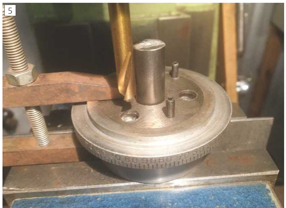
Transferring holes to the shank.
