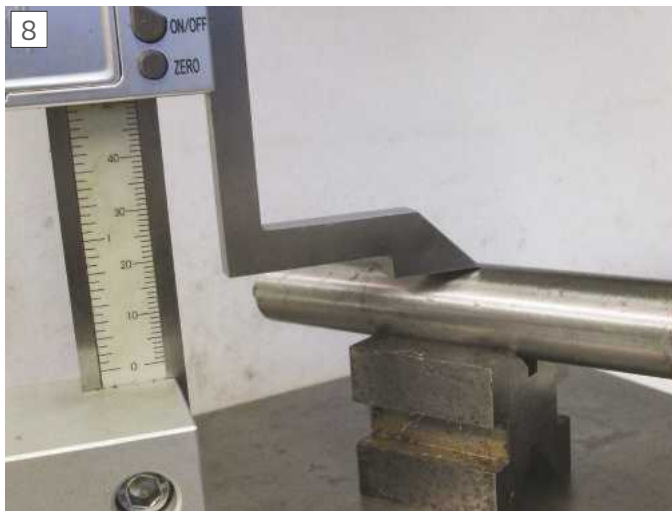
Measuring the overall height of "v" bloc mounted cylindrical work
