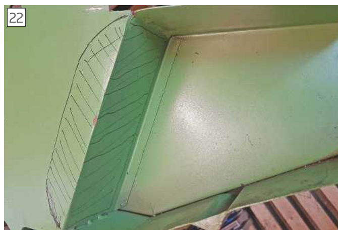
Splash Back Panel areas marked for material removal
