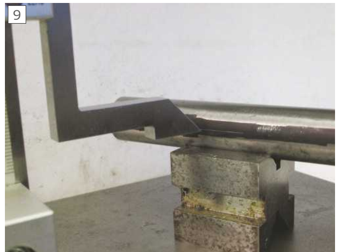
Marking the centre line on cylindrical work
