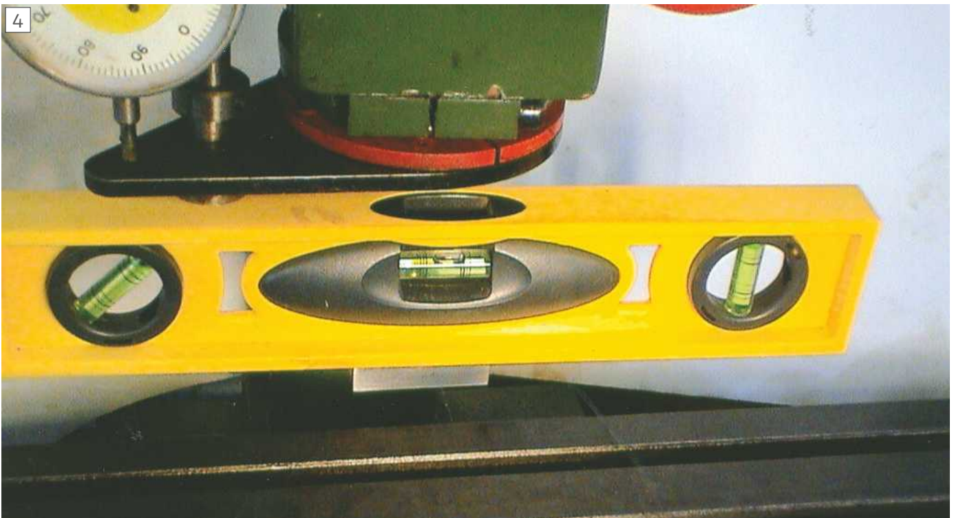
Using the spirit level to align the plate and mill
