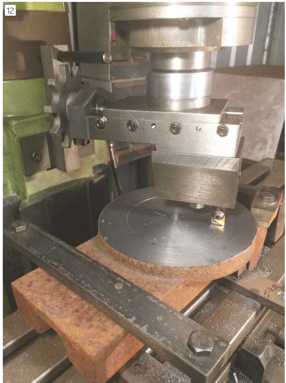
Machining the shaper Vice body.
