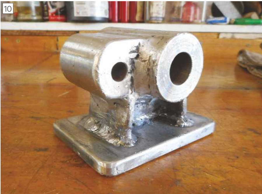
With the base plate welded in place and ready for final clean up, the job is now looking like a versatile dividing head body.
