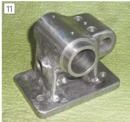
Body is finish machined following G.H. Thomas's original methods, just the same as a casting.
