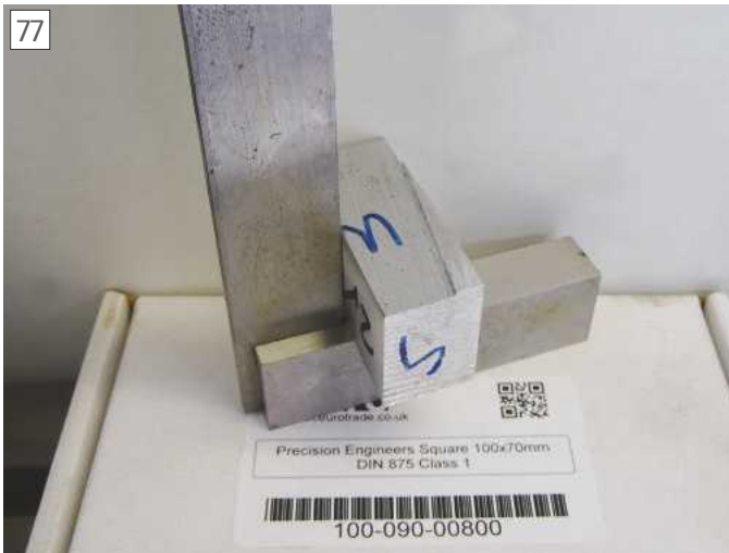
Checking face 1 is square to face 2
