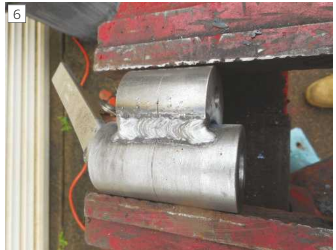
The two main barrels are held in the vice, tacked in two places each side, then welded together.
