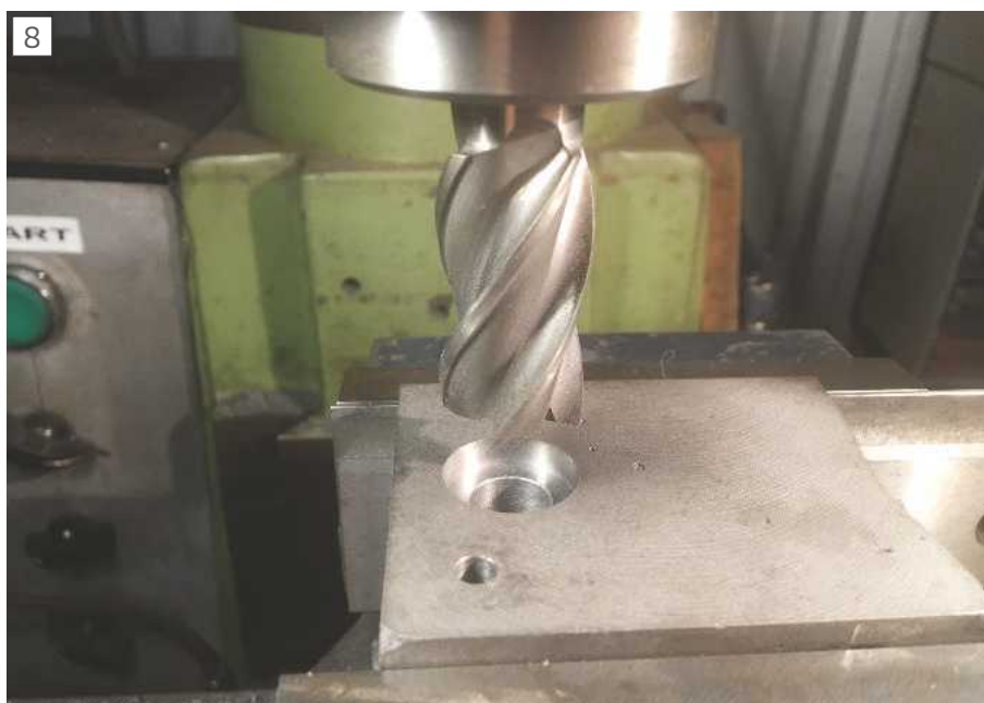
Machining recess for feedscrew.
