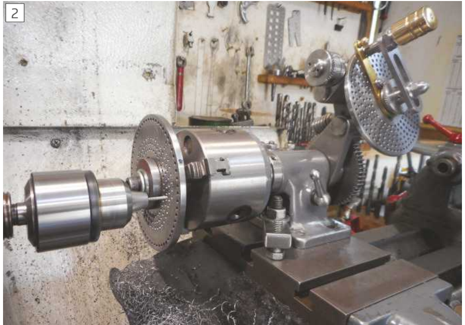
The almost completed unit in use on the lathe drilling its own index plates.
