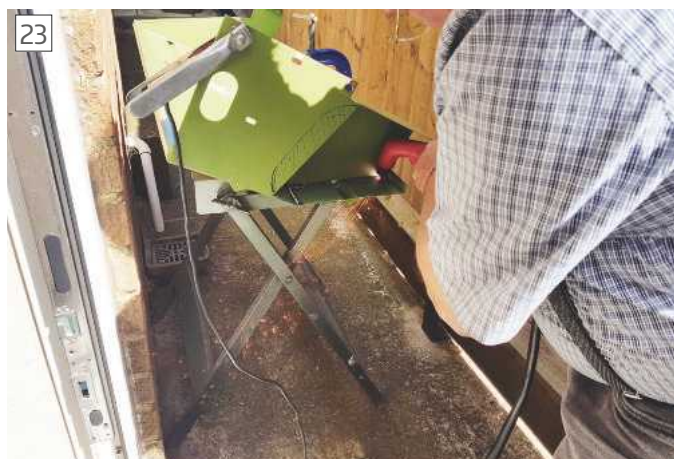
Merfyn making first cuts with his plasma cutter
