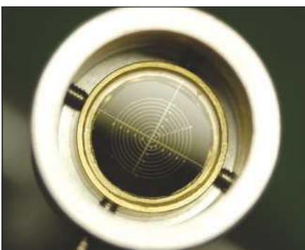
Paul Buckley makes an Optical Centre Finder from microscope parts.
