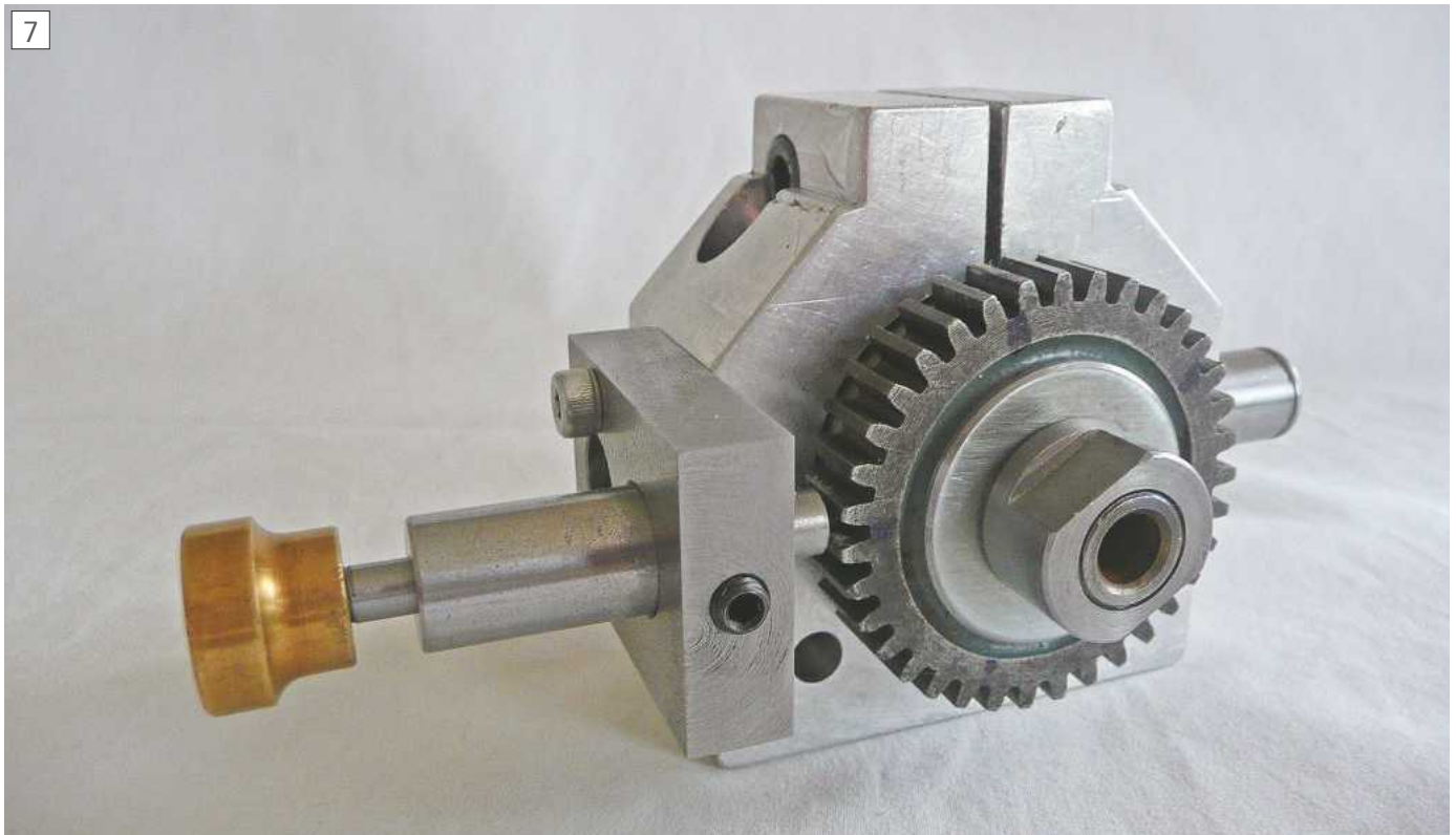
Using a change wheel for indexing
