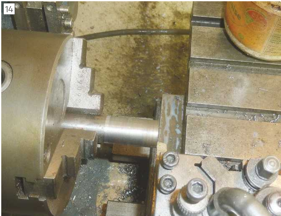
Using the knife tool as an end stop. The tool is positioned by the carriage multi-stop.
