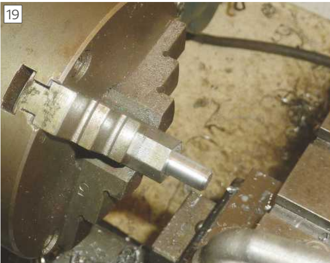
Outside diameter machined on component in example 3.
