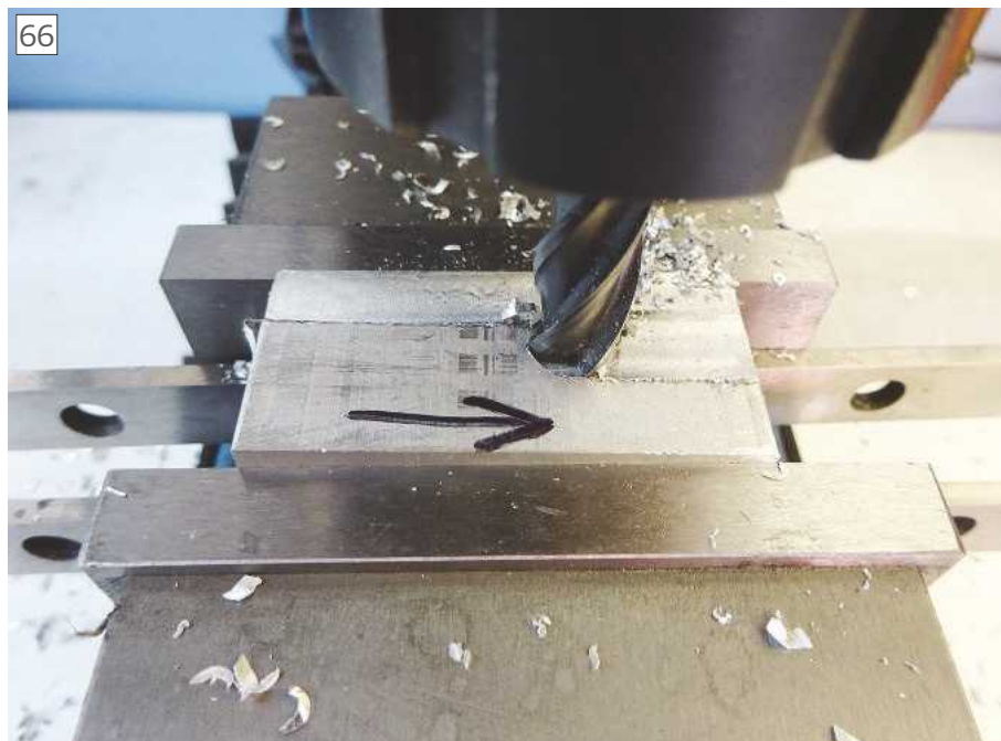
Mid way through the second pass of a facing cut
