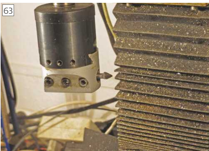
Timing belt cutter mounted in a boring head for convenience
