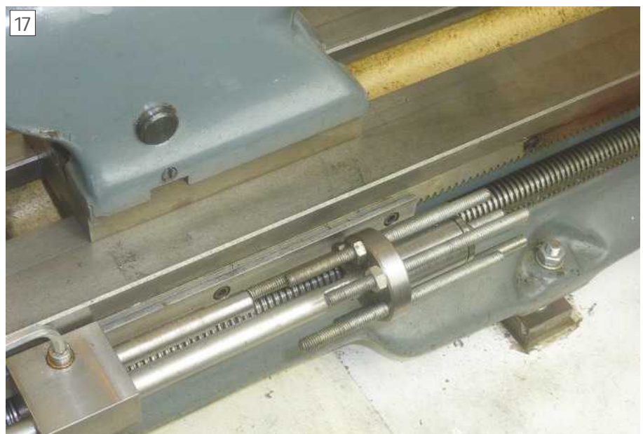
The multi stop with all six positions set.
