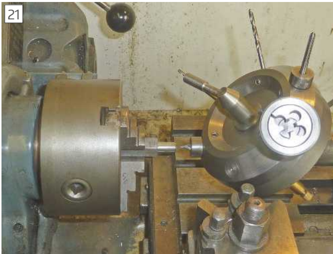
Centring the end of the part.
