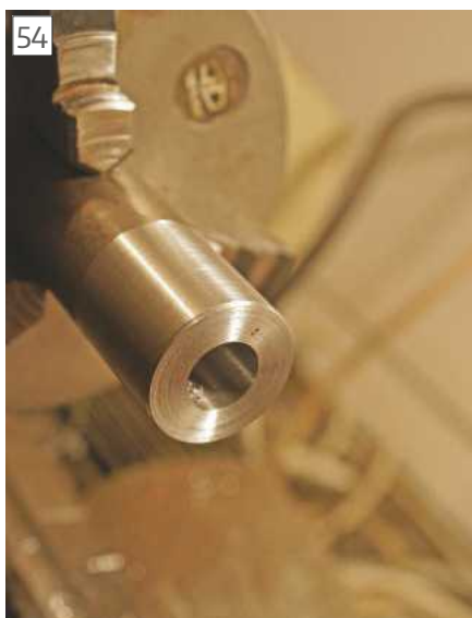
Steel casing for the nut
