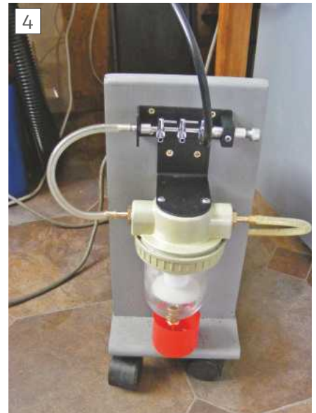
The front of the trolley showing the trap and manifold.
