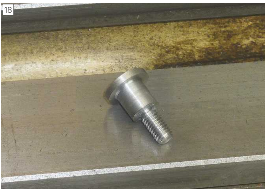
The component parted off ready for cutting the slot on the milling machine.
