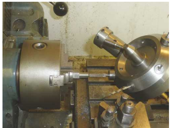
Tapping the bore, turning the lathe spindle by hand.
