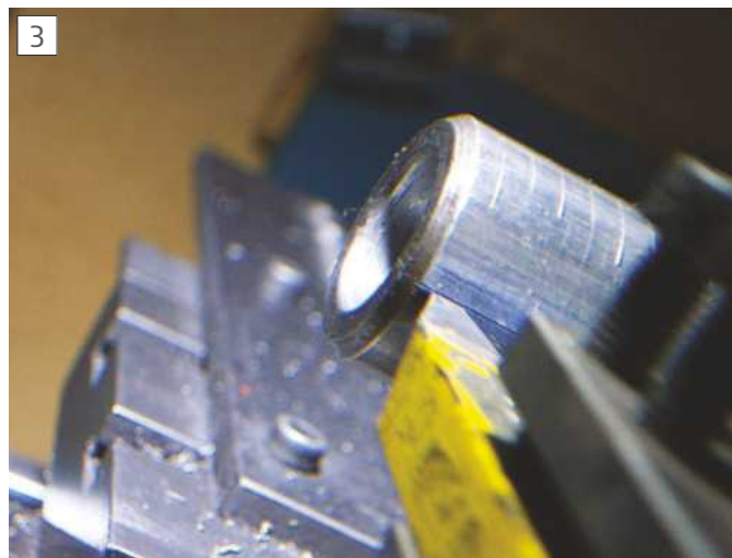
An ACME type tool set up ready for work
