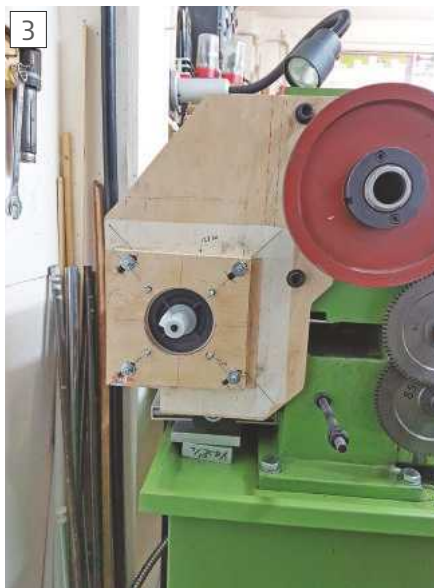
Ply backplate bolted to headstock, motor on blocks
