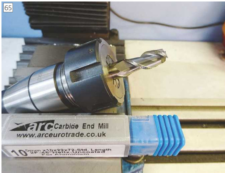
Correct cutter projection
