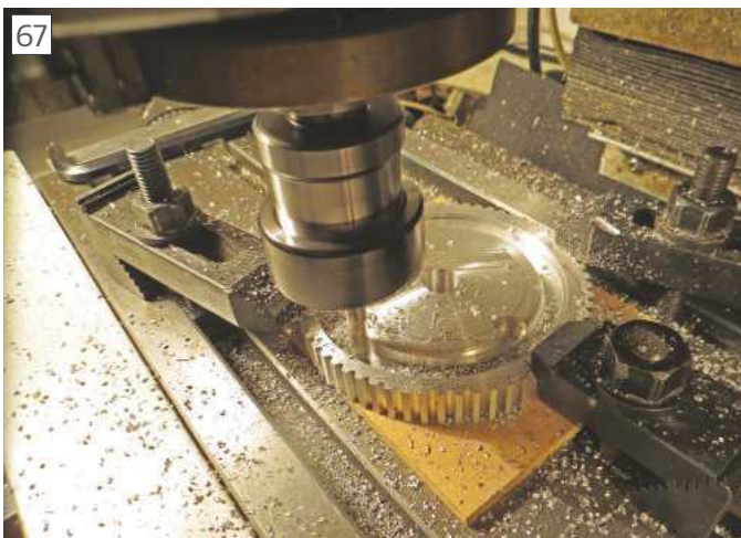
67 Roughing cut to remove the centre. Note the delicately placed clamps and the MDF sheet to protect the mill table
