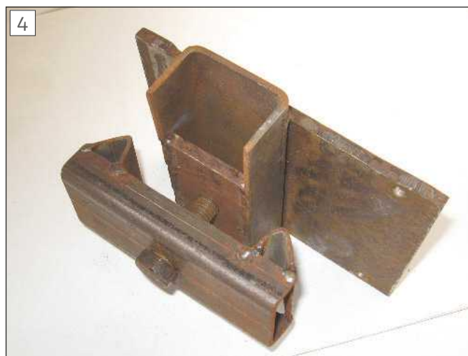
The base clamping system fits the lathe bed
