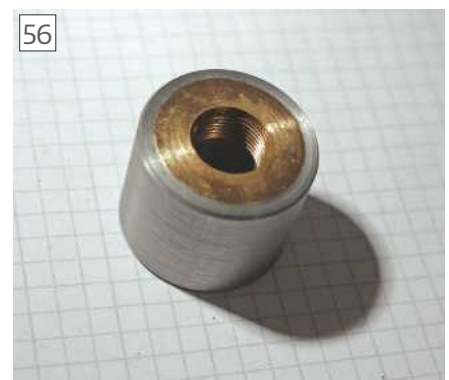
Nut Loctited firmly into the casing
