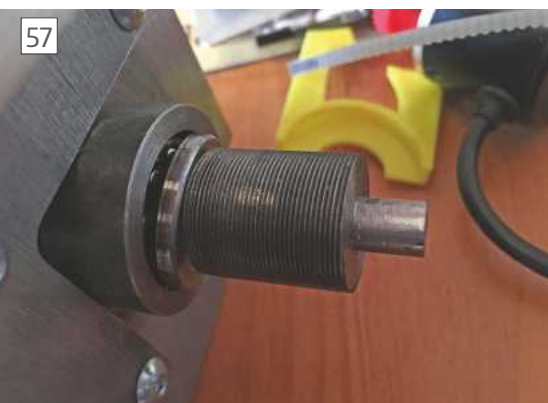
Through bolt being machined
