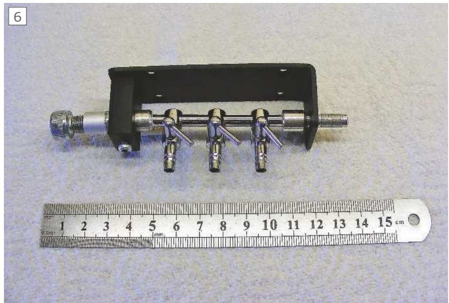
The manifold with the tubing connector and pressure relief valve mounted in the bracket.
