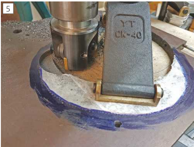
Removing material from backplate
