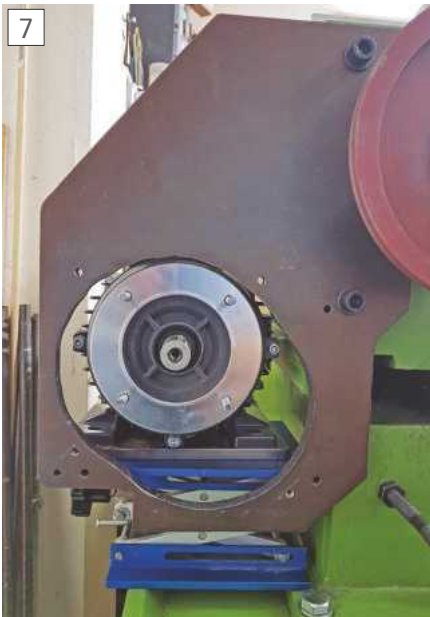
Motor supported in backplate – final check prior to fitting motor plate
