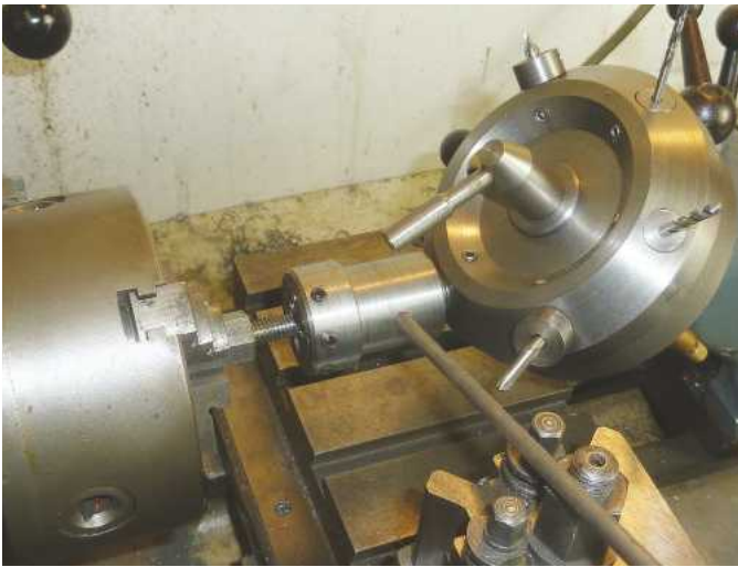
Cutting the external thread, turning the spindle by hand or using the back gear if available.
