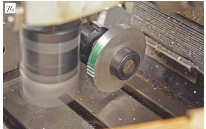
74 Enough confidence this time around to cut immediately to full depth
