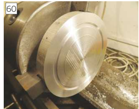
Initial trepanning mark indicating where it will need to be cut later
