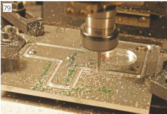
Profiling the stepper mount plate - note the hold down bolts
