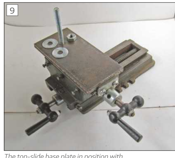
The top-slide base plate in position with toolpost removed
