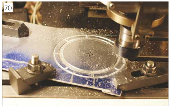
70 Milling out the index disk. The aluminium is glued to an MDF backing sheet
