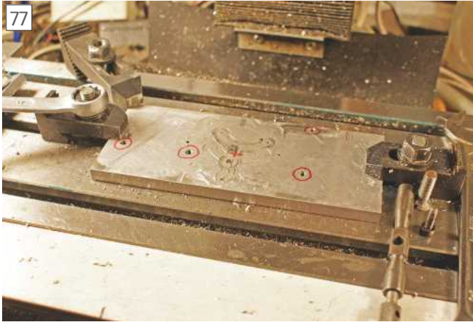
Sacrificial plate predrilled for hold down bolts
