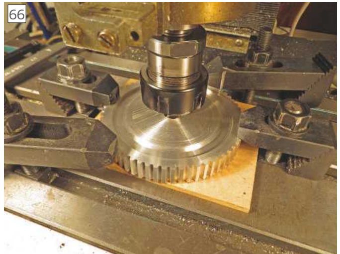
66 Centred on the table using a suitable shaft mounted in the mill ER25 collet
