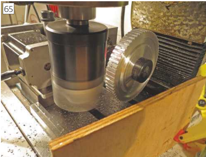
65 Cutting to full depth on this pass
