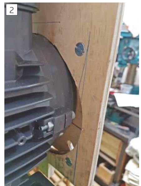
Checking for 2mm minimum clearance from ply backplate
