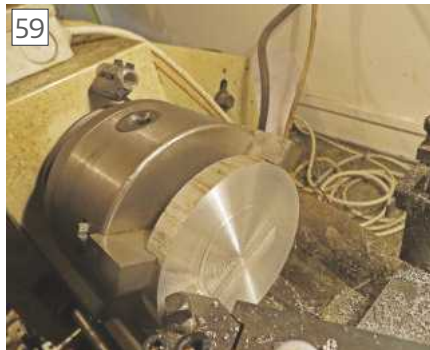
Big slice of aluminium being faced for the toolholder plate timing gear
