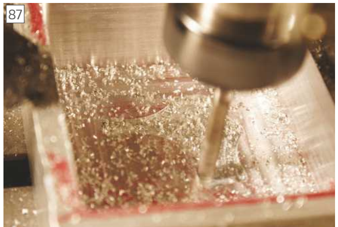
Milling out the base leaving 4 mount points for the Arduino
