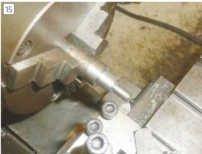
The part in example 2 with all diameters machined, ready for threading before parting off.
