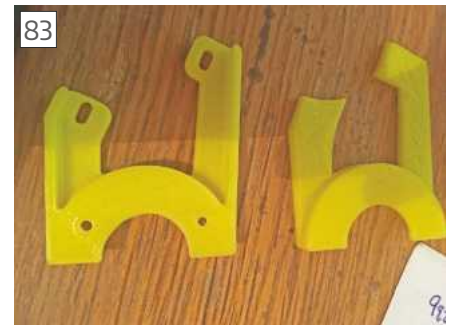
Version 2 alongside V1, note holes, bracing to the arms and a generally better finish
