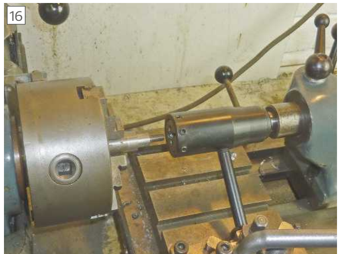
Cutting the screw thread using a tailstock die holder.
