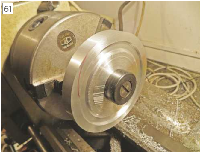
Bored and mounted on a mandrel for machining to diameter. Note use of ER25 collet
