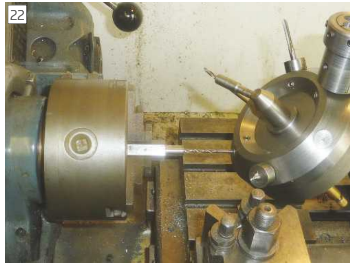
Drilling the smaller bore.
