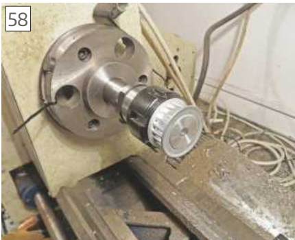
Commercial timing gear being bored for 1/4"
