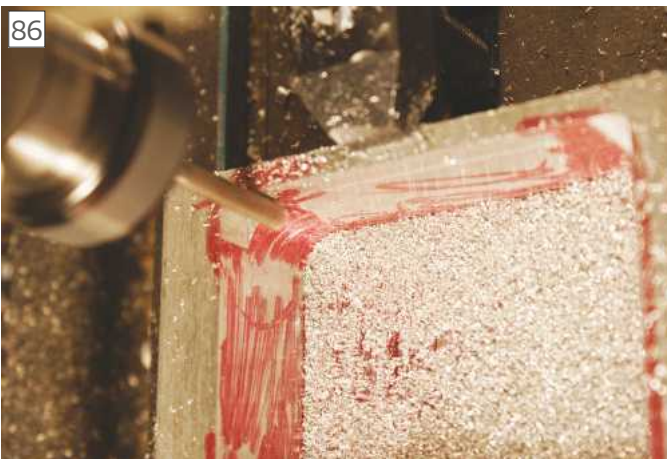
Smaller end mill cleaning the corners and applying a final finish internally
