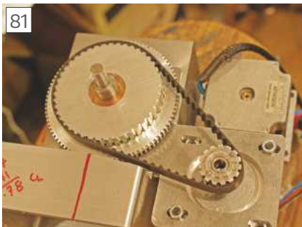
Stepper installed in the mount plate. Note the oval holes allowing some L6R movement
