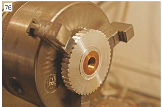
76 Bronze nut installed, awaiting a final cleaning cut
