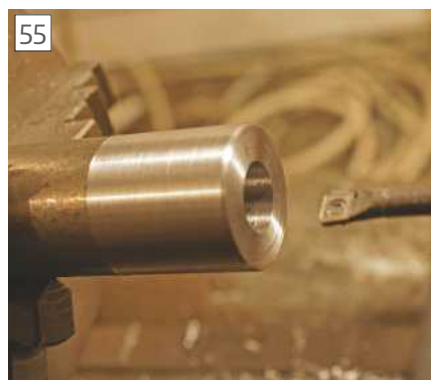
Boring taking place
