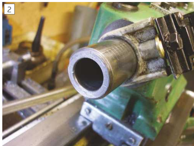
Mark extended across the nose of the barrel
