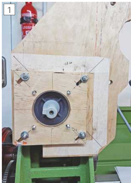
Initial clearance checks between motor and ply backplate
