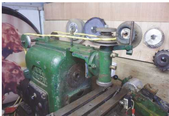
Testing belt length for the simple but effective vertical attachment. Custom collets are needed.
