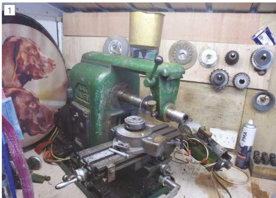
The Ajax horizontal and vertical milling machine is small but made of robust castings.
