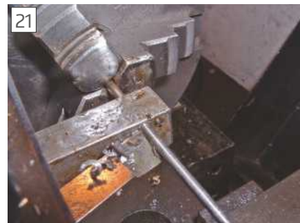
Running down a TIG welding stick with an improvised steady.
