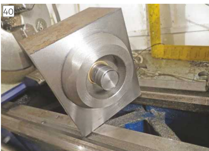
Bush in place with press tool inserted. Several attempts were needed to get the fit right
