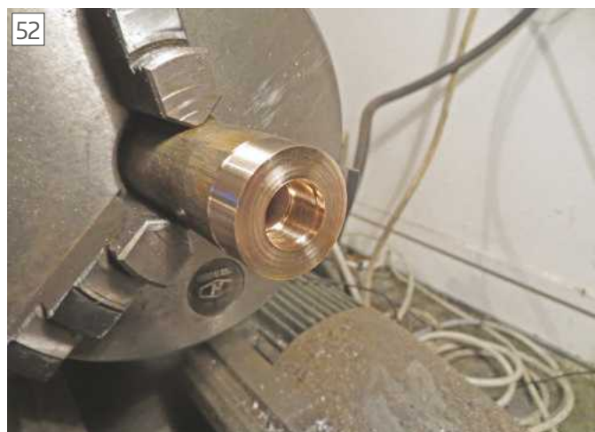
52 Cleaned and bored to size
