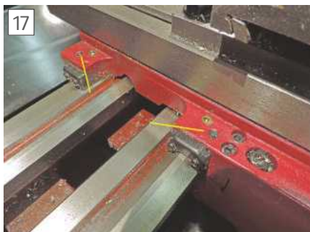
Fixing points for the SC4 fixed steady.
