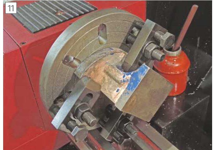
Care is needed to ensure balance and avoid clashes with the lathe bed.
