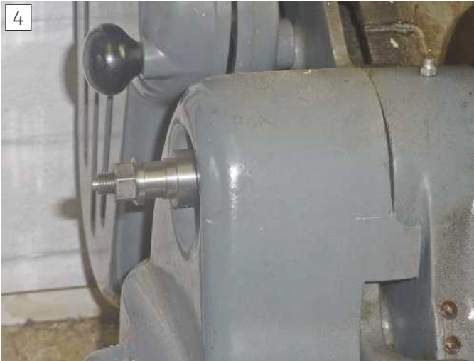
The mandrel backstop fitted to the outer end of the lathe spindle.
