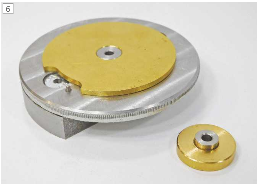
The inside former, the pin for the click spring, and the outer roller
