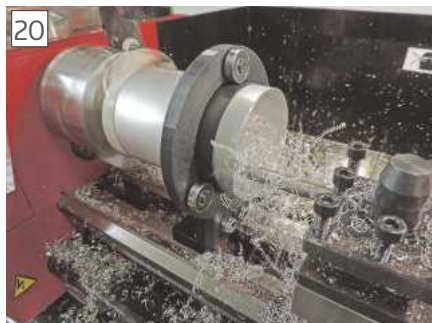
This 3D printed device was a solution to a one-off job too big for a standard steady.
