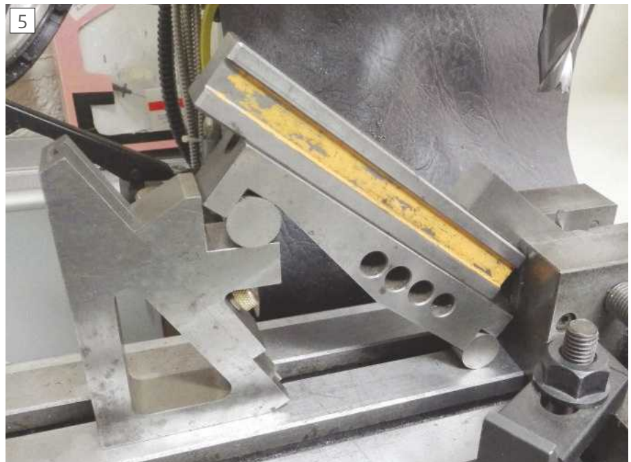
Using an additional parallel to transfer an angle to a block in the milling vice
