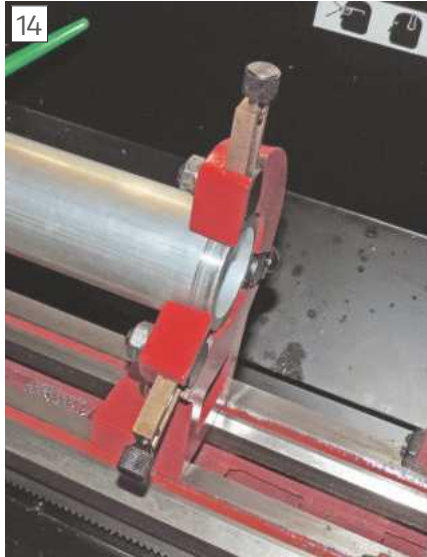
A typical use of a fixed steady.
