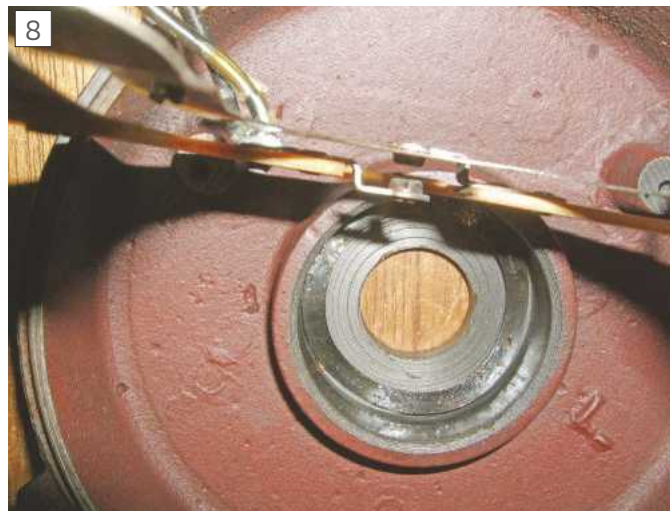
Contacts showing the normally open state
