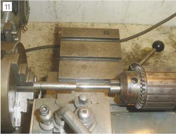
Parting off the blanks slightly over length using a stop set in the tailstock.
