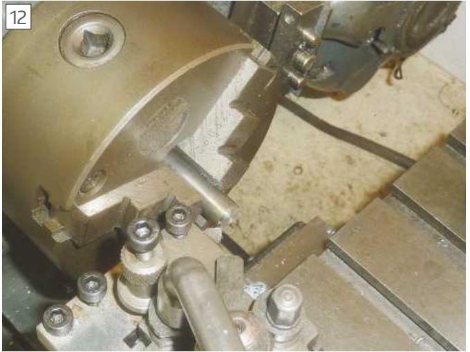
Facing and chamfering one end of the blank, which has been positioned against the mandrel backstop.
