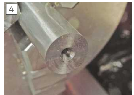
The centre, note the central hole inside the cone.
