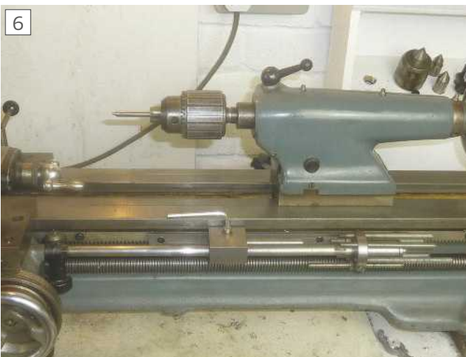
Carriage multi stop fitted to the lathe.
