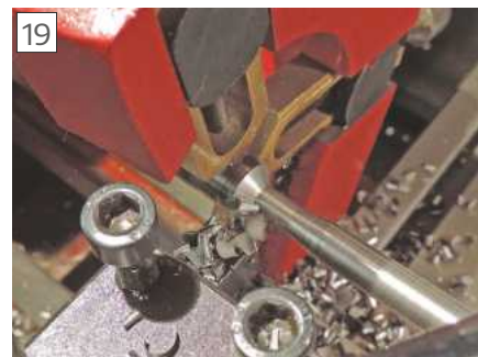
The steady allows a 3mm deep cut on an overhung, thin bar.
