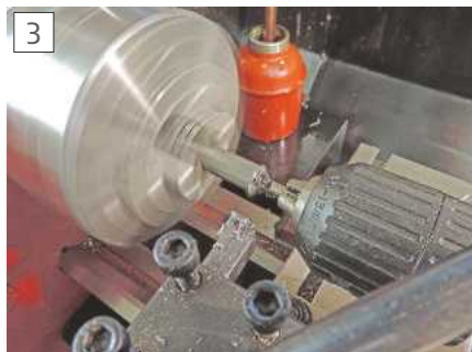
Preparing a bar by facing and centring.
