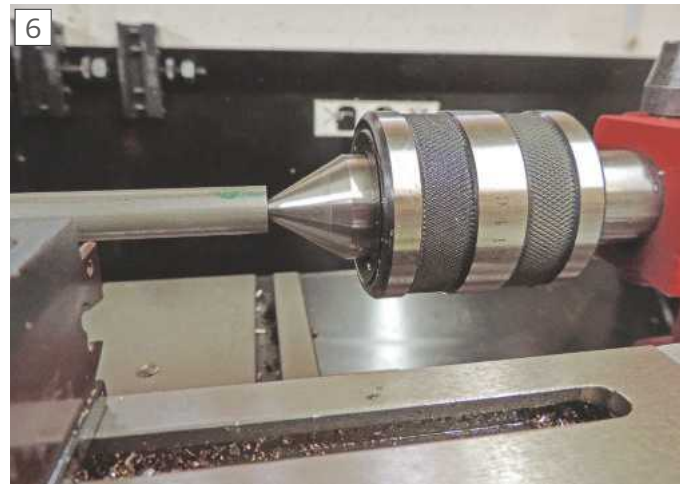
Rolling centre in the tail of the work.
