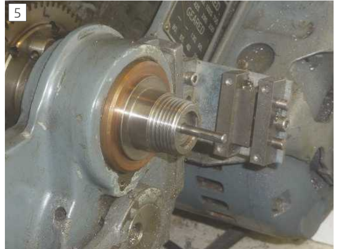
The inner end of the mandrel backstop with chuck removed.
