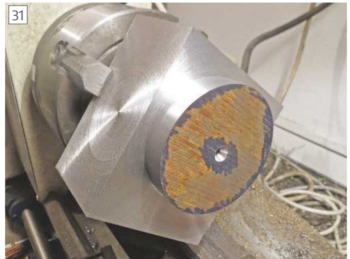
Lots of hot swarf later, the block is ready for the cone
