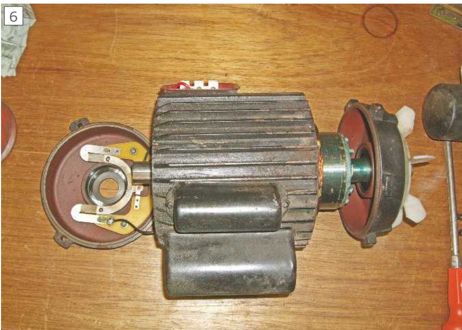
The motor dismantled to show the centrifugal switch
