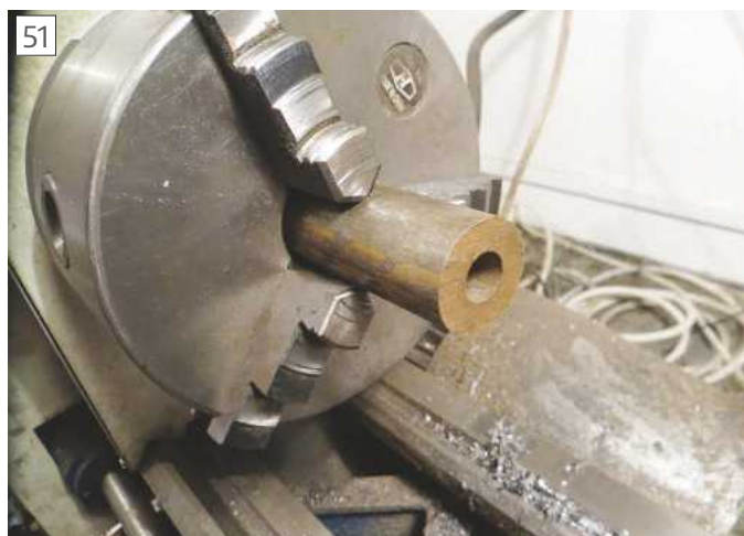
51 Cored bronze rod for the locking nut
