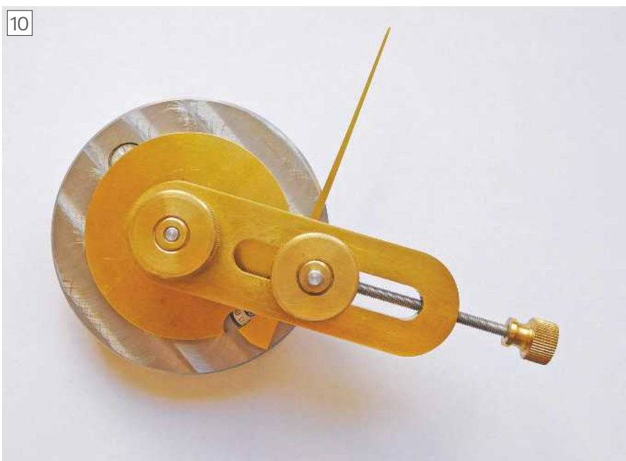
The tool ready to bend the click spring
