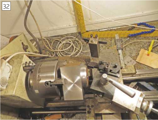
Topslide still in the same position as for the plate cone, note the inverted tool cutting on the far side of the block
