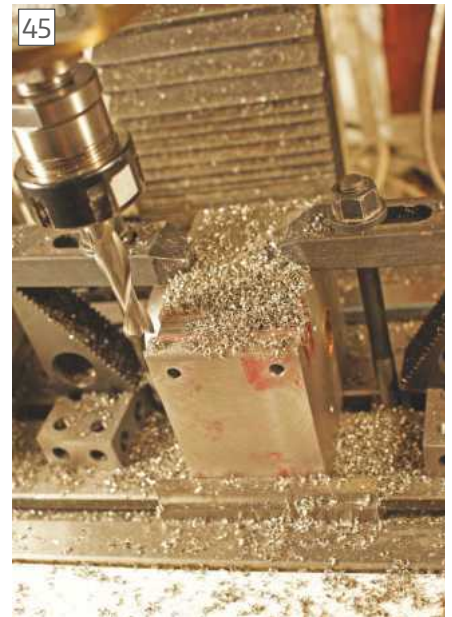
The block gets some slots to access the hold down bolts
