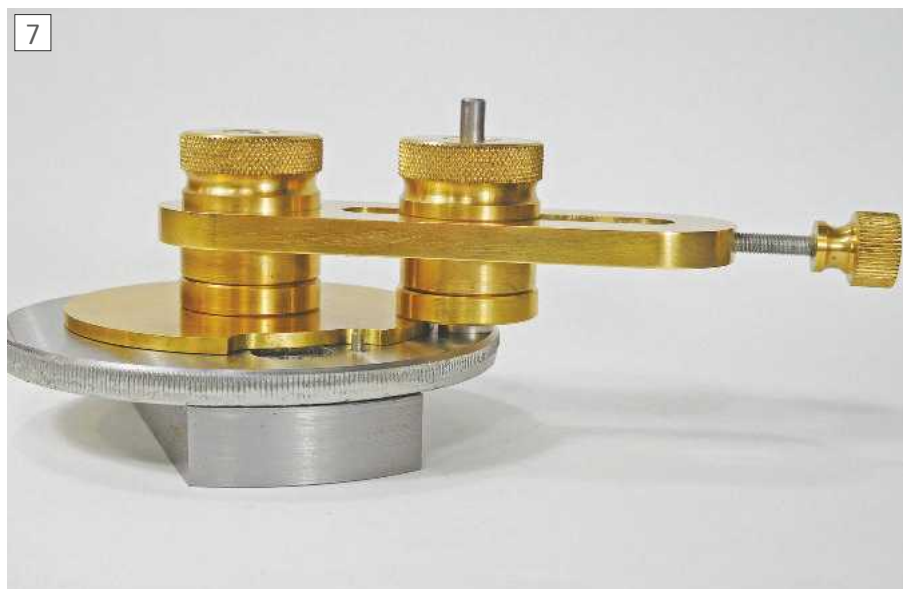
With the depthing tool upside down, we can bend click springs
