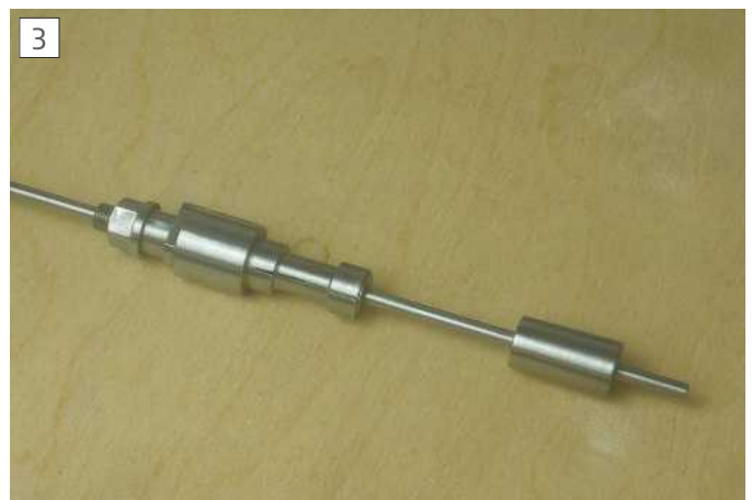
The parts of a mandrel backstop.
