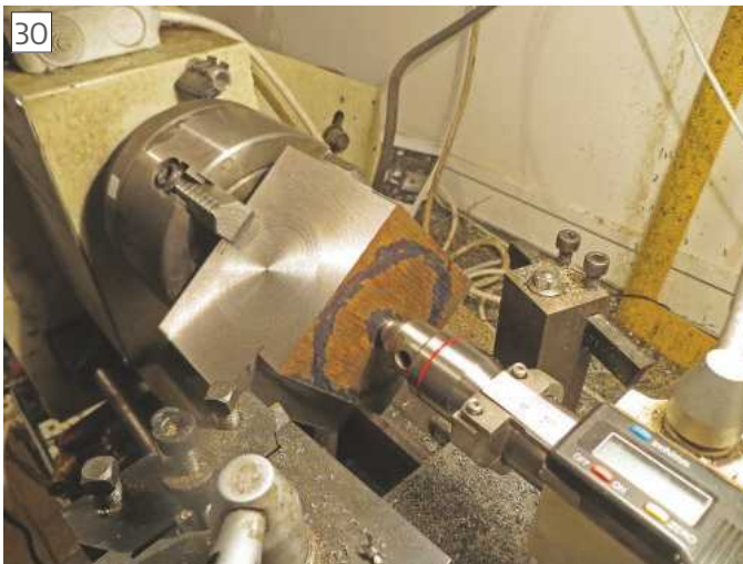
Starting to machine down the block ready for cutting the cone surface
