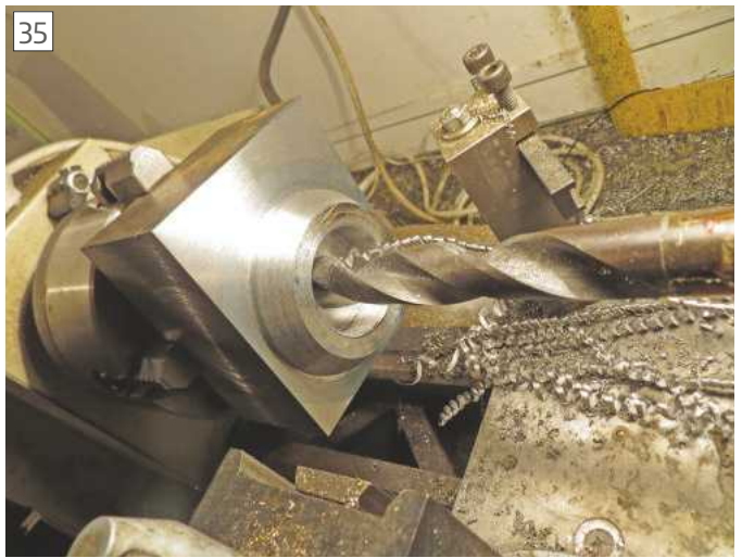
Start the process with a 25mm drill
