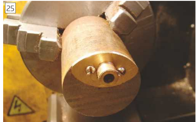
This simple jig is for turning elliptical glands.
