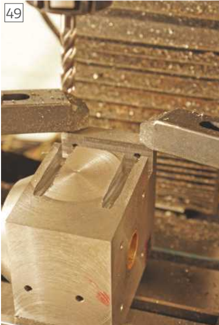
49 The finished access channels for ball head hex keys
