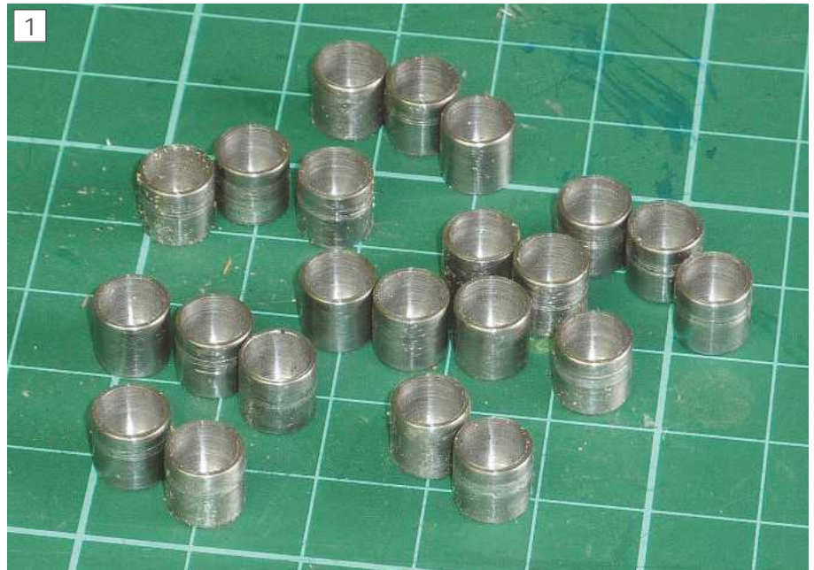
A production run of bucket tappets for miniature IC engines.
