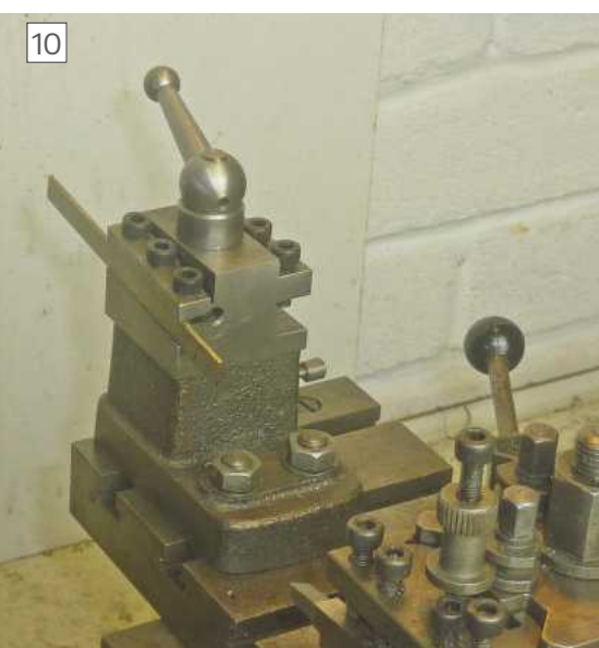
A rear tool post with parting-off tool.
