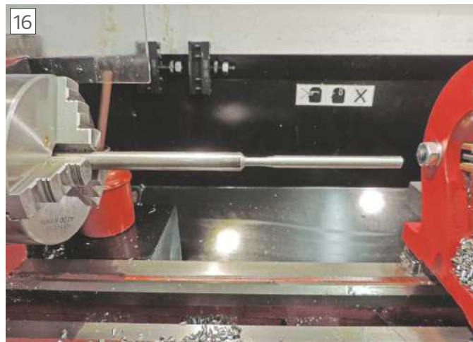
A machining challenge, with huge overhang.
