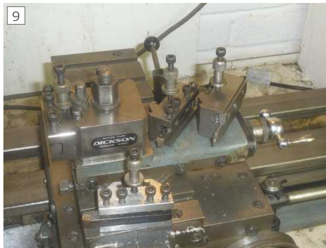
A quick change tool post with a selection of tool holders.
