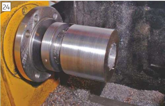
This large cylinder is screwed on to an arbour fitted to the lathe.
