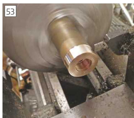
53 Parting off - 0.7mm pitch thread visible
