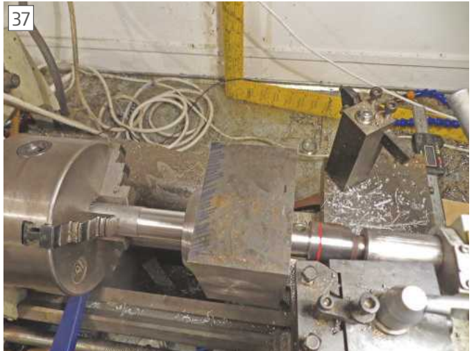
Scary stuff to clean the face - taper bar supported between centres
