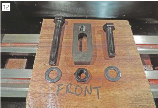
One of four clamps in the standard SC4 set, these should always be set up so they are angled down to the 'toe' that grips the work.
