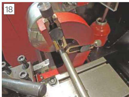
Setting the steady close to the chuck.
