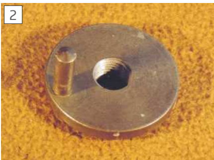
The catchplate from an old Super Adept lathe.
