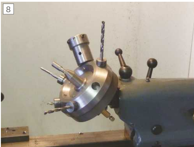
Tailstock turret fitted to the lathe.
