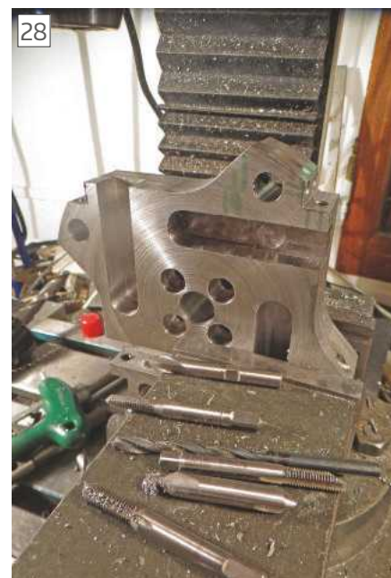
Drilling and tapping the tool fixing bolt holes - not the very 2nd hand tap awaiting disposal
