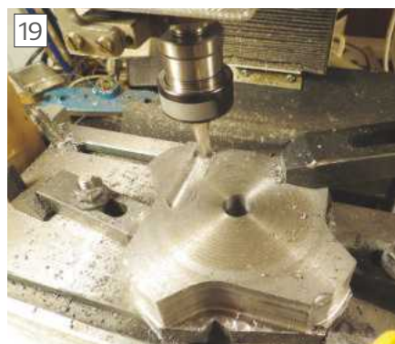
19 First tool slot being cut - note the additional hold down clamp
