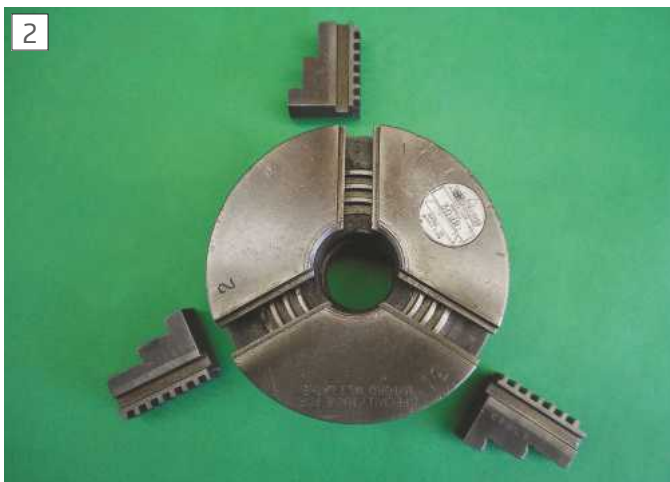
Jaws removed, revealing the spiral scroll inside the body and the meshing teeth on the jaws.
