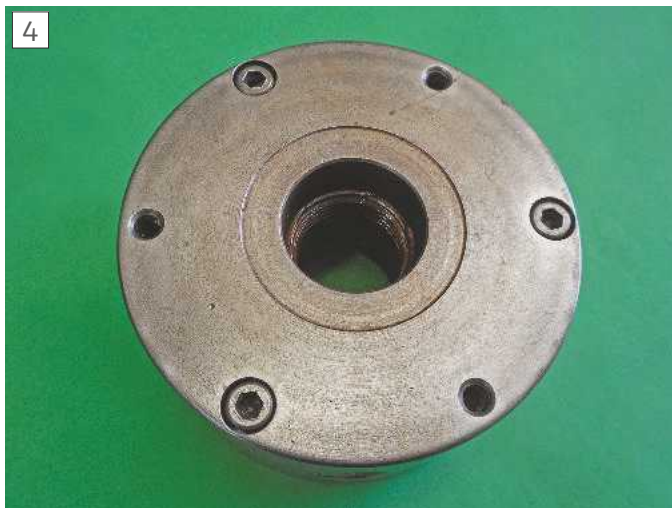
Three Allen-head screws retain the backplate. Three threaded jacking holes lie in between.
