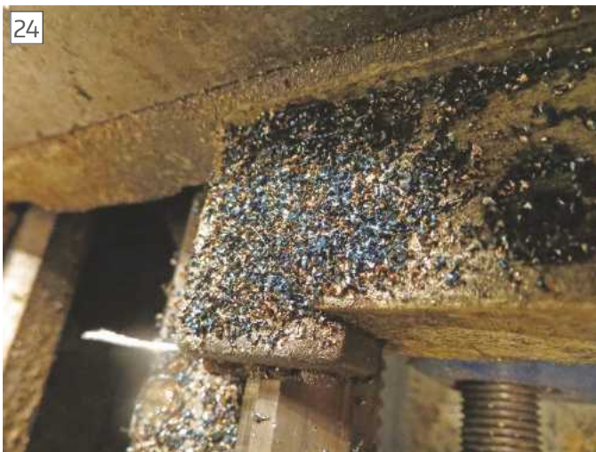
Seriously hot swarf once I had the courage to push the carbide tools and lathe far beyond what I thought was reasonable. I had to install serious shields to stop being assaulted by this stuff
