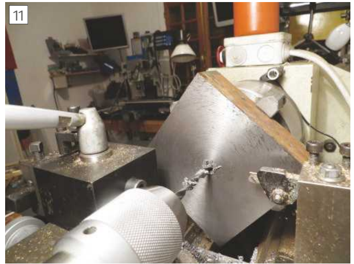
Toolholder plate faced and then drilled through
