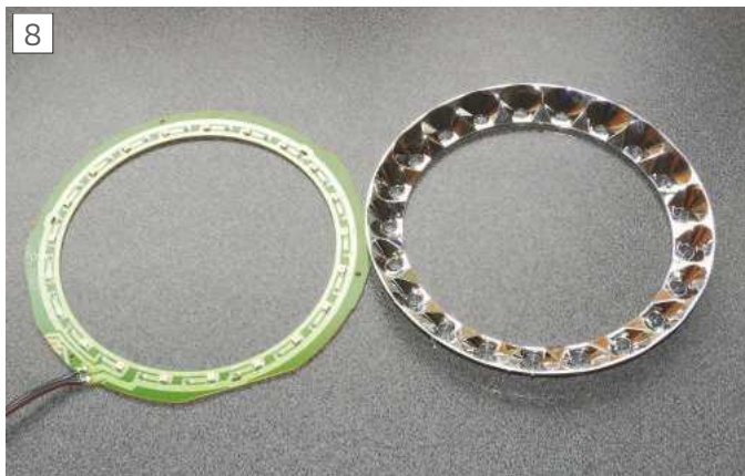
The Two Parts of the LED Array
