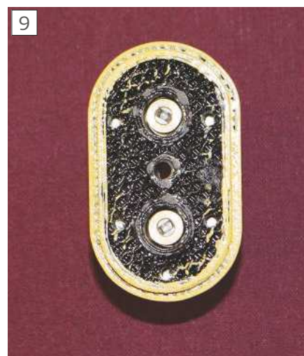
Slotted inserts in the shafts of the 3D printed shaver unit.
