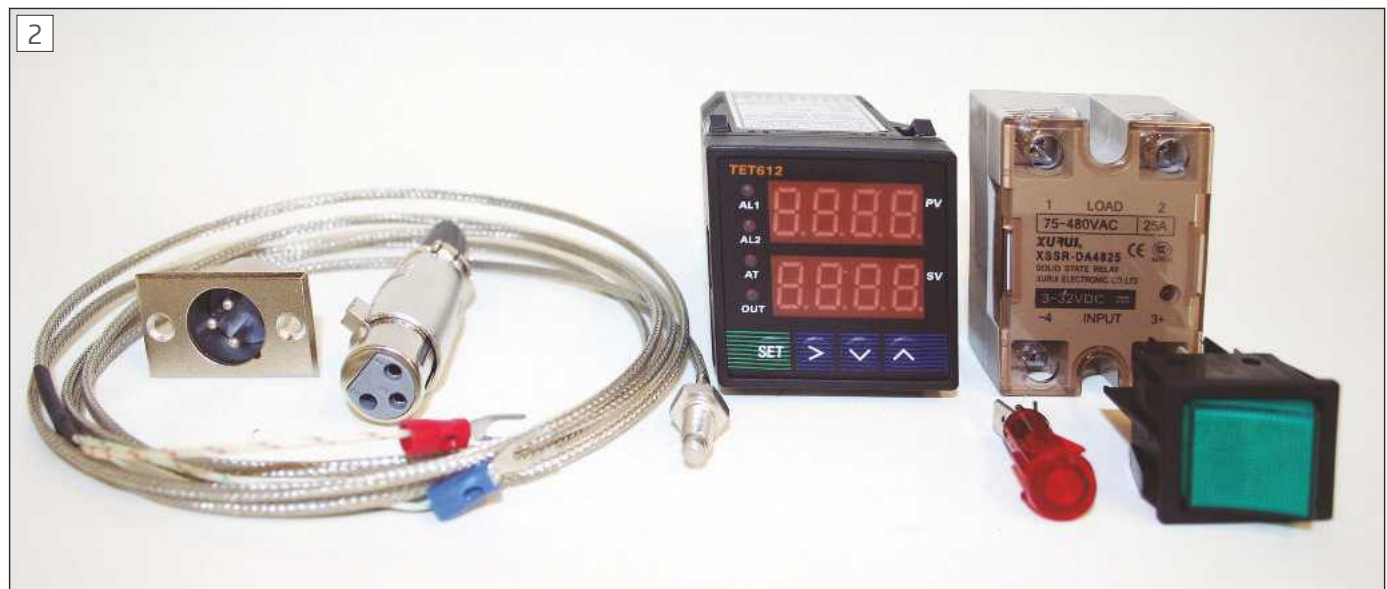
Controller Components: Thermocouple and connector, controller, and Solid State Relay
