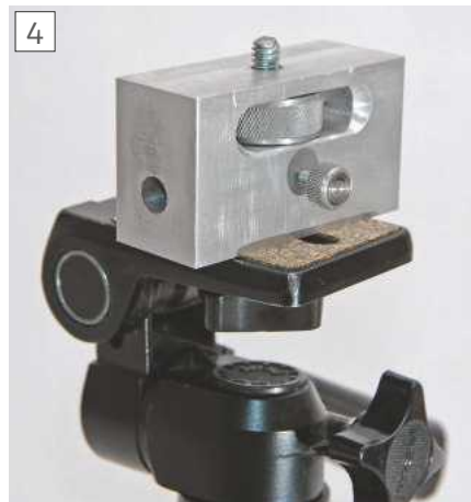
An Adapter for Coupling a Flash to an Umbrella
