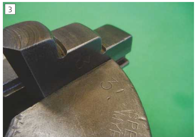
Burnerd chuck comes with jaw and slot stamped as matching pairs, some others may not.
