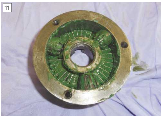
Pack gear teeth with grease but no need to fill the whole cavity.
