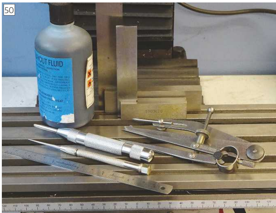
Selection of marking out tools, Rule, Scriber, Auto Punch, Square, Dividers and odd leg callipers
