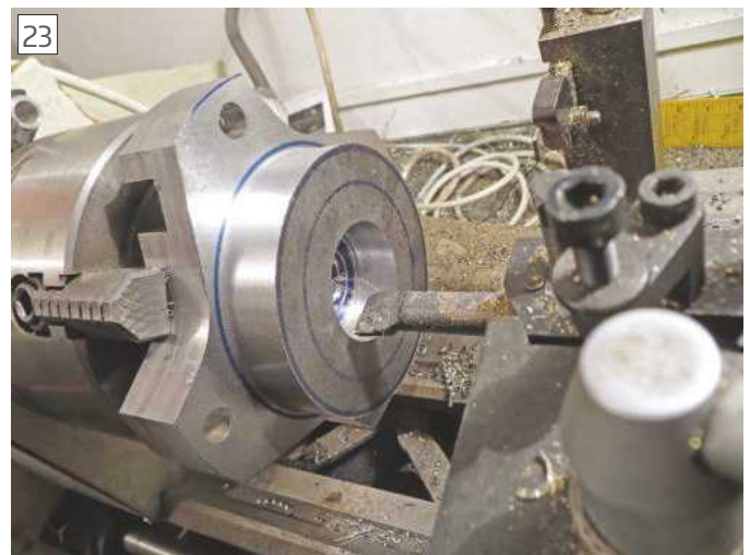
Boring the centre hole ready for the cone which will be machined between the two lines on the unmachined face
