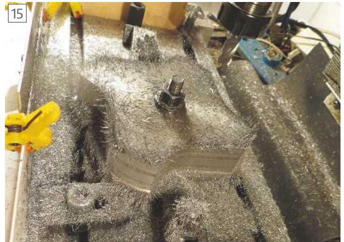
Hairy look caused by using a magnet on the plate to limit swarf distribution
