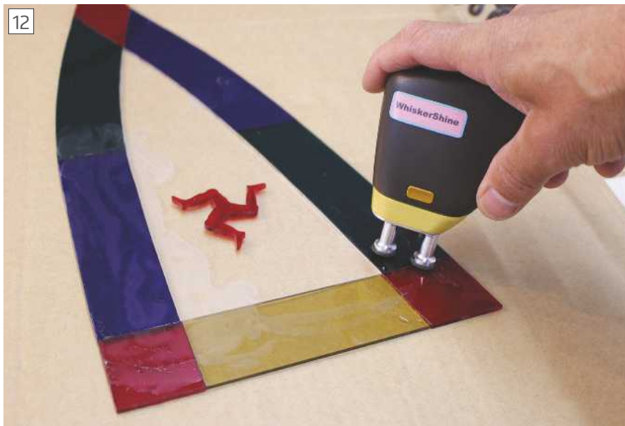
The WhiskerShine removing blemishes from an acrylic window.
