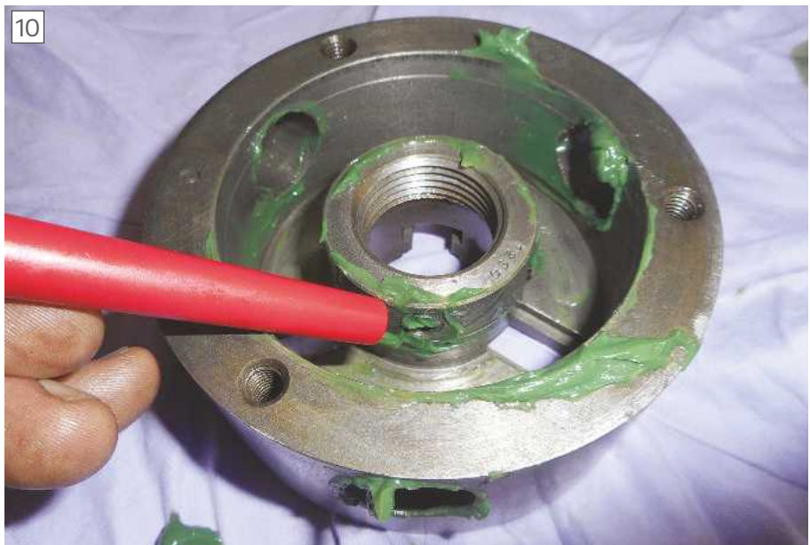
Grease interior of chuck body and the small holes for the pinion shafts.
