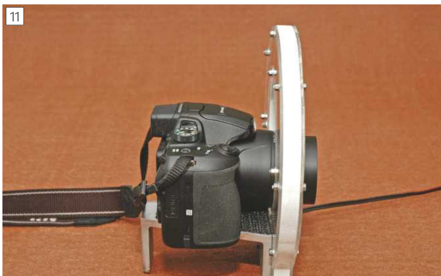
The Camera Mounted on the Ring Light
