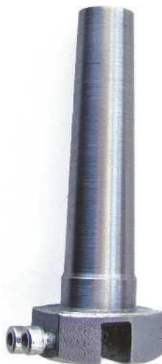
The flycutter showing the tool slot and clamp screws
