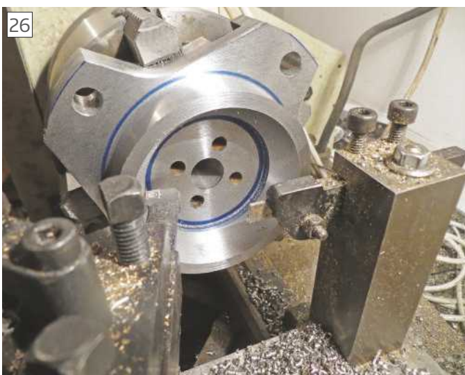
Cone cut although the surface finish leaves something to be desired
