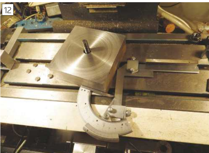
Plate mounted skew on the mill to minimise waste
