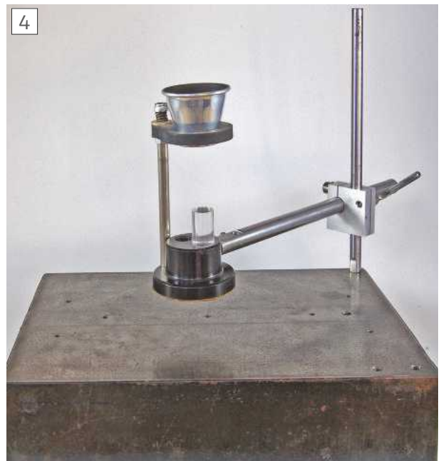
The punch and loupe assembly fitted to the pillar and base
