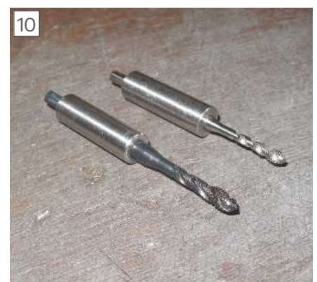
M4 & M3 taps bonded in silver steel sliders.
