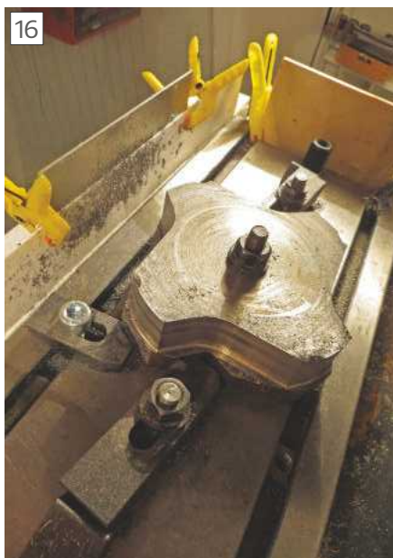
16 Cleaned up and ready for the slots to be cut. Note the position of the clamps
