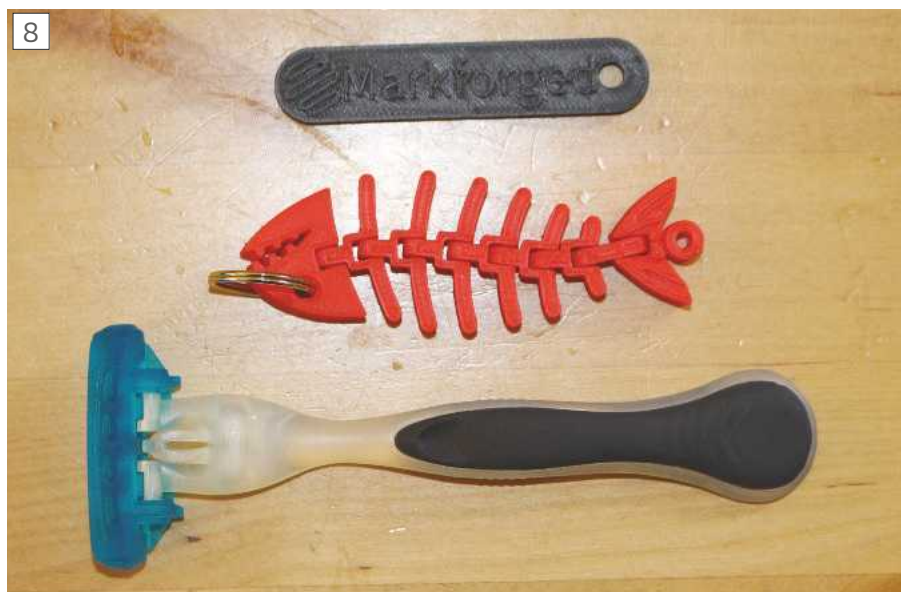
From the goody bag: top carbon fibre reinforced name tag from the Markforged; centre articulated key ring printed by FDM; bottom shaver prototype composed of three resins made in SLA.
