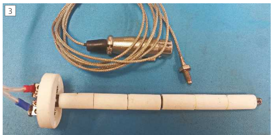
Medium and high temperature K type thermocouples
