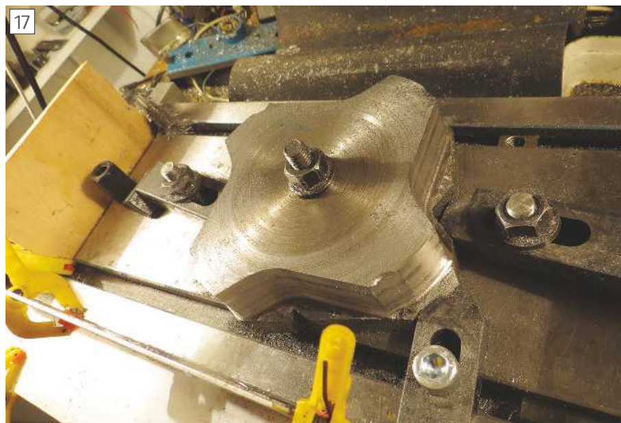
17 Another view of the part finished plate - the reason for angling the part on the bed is clearer now
