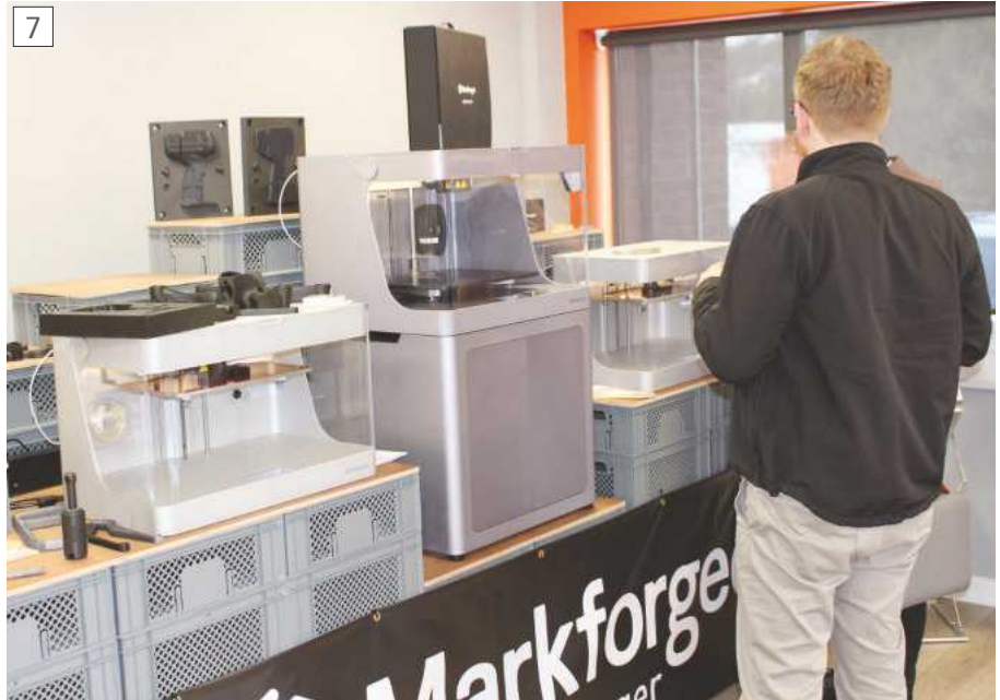
Markforged 3D printers which can extrude composite material.
