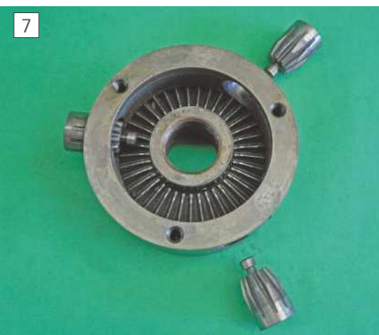
Barrels pull straight out on the Burnerd. Others may have retaining screws or pins to be removed.
