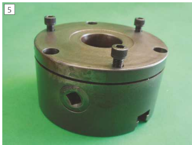
Gently ease the backplate off using the three jacking screws evenly.
