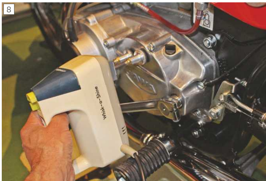
The Whisk-a-Shine buffing up a motorcycle engine.
