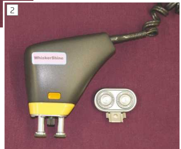
Philips electric shaver converted to become a light polishing machine.
