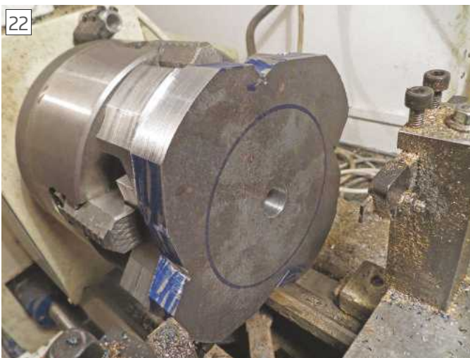
Part way through machining - the blue line is the target point - roughly
