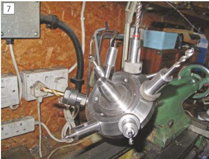
Tail stock turret with M8, M6 & M4 taps in tool holders.
