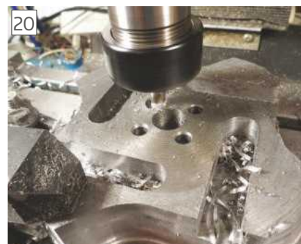
20 Slots finished and just the bolt holes for securing the plate to the main shaft to go. Note this is a CNC bore routine rather than drilling with the final size drill
