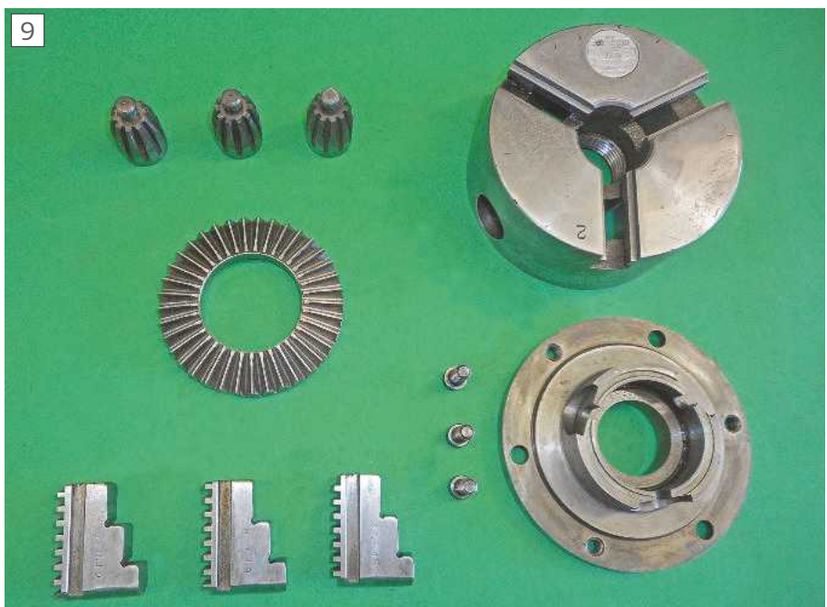
Cleaned chuck parts laid out for reassembly.
