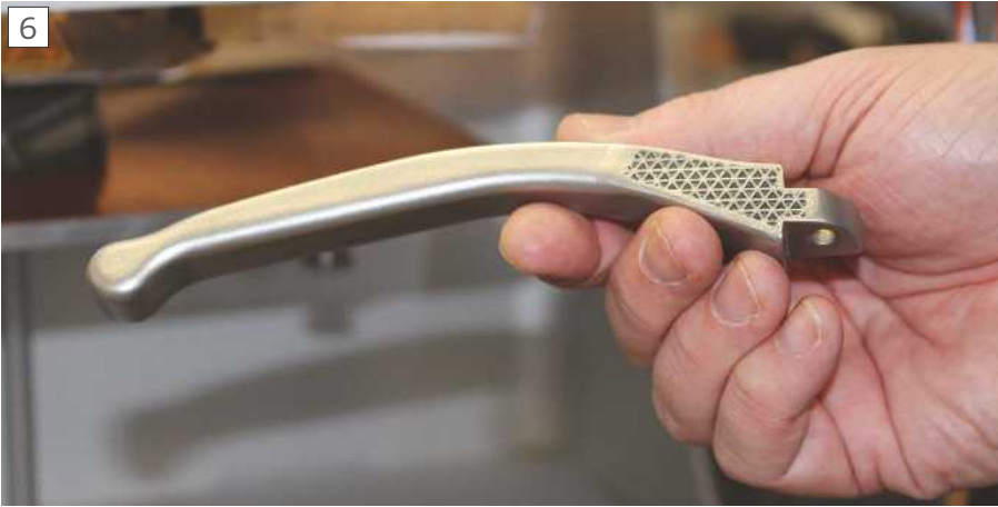
Motorcycle handlebar lever in stainless steel created by one of the new generation of metal printing machines.
