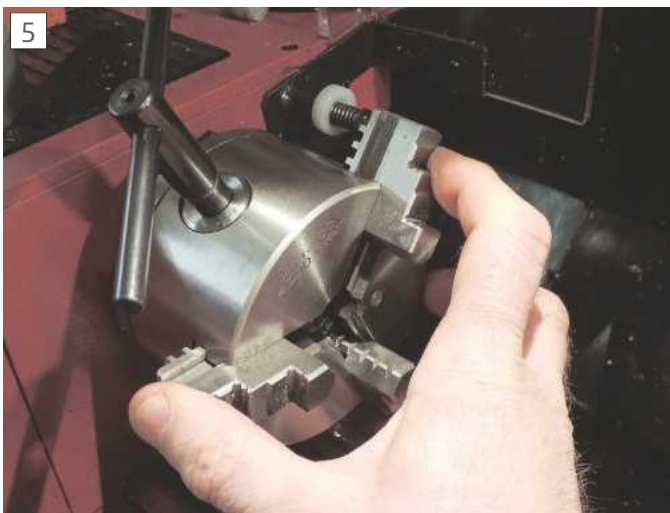
Using finger pressure to ensure all three jaws are equally engaged with the scroll.
