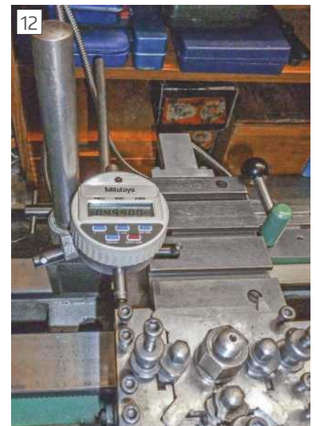
Sensitive dti to compare output with that of M-DRO
