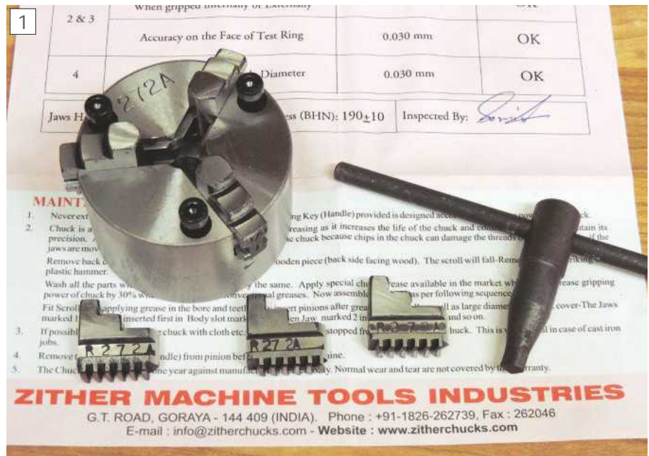
A 100mm (4") 3-jaw self centring chuck by Zither, with its alternative jaws, key and test sheet. This chuck has proved very accurate in use.
