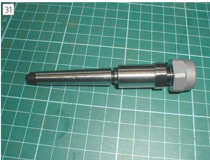
Taper and collet holder as bought
