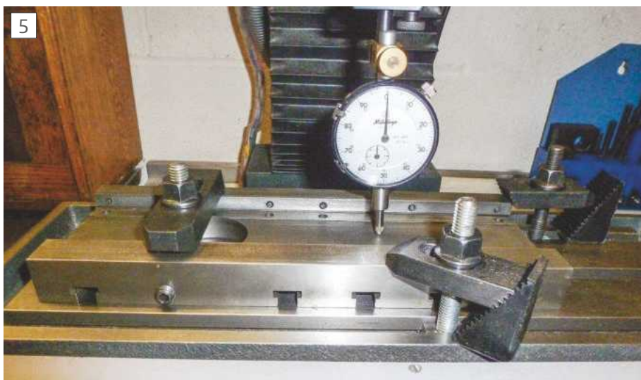
Checking flatness of cross slide
