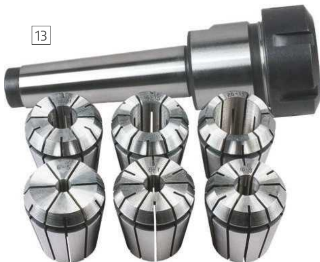
This ER collet chuck is chiefly intended for holding milling cutters, but it can also be used in a lathe with a matching taper.
