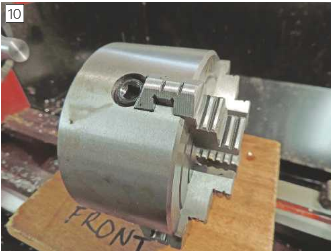
The independent 4-jaw chuck has a separate adjuster for each jaw.
