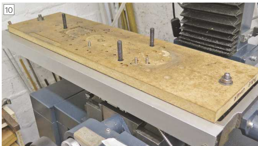
Location Dowels and Clamp Studs in Place
