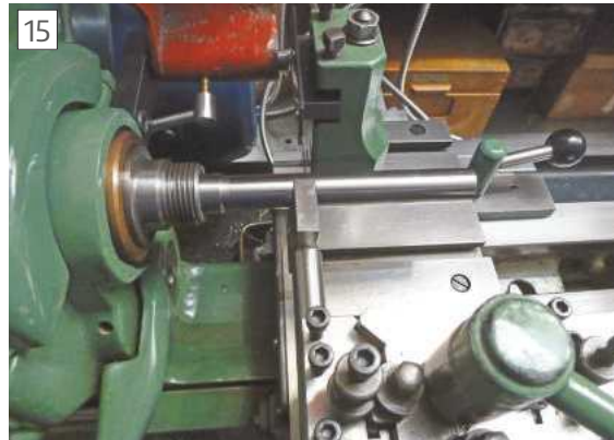
The 1 inch slip to check cross slide movement
