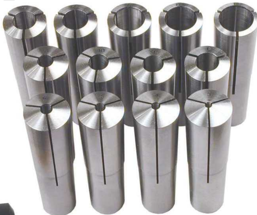
A set of MT3 collets, these metric collets have an M12 drawbar thread at the back.
