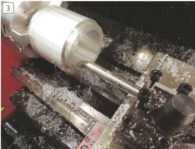
Large diameter work held on the step of internal jaws, the large overhang means only light cuts can be taken.
