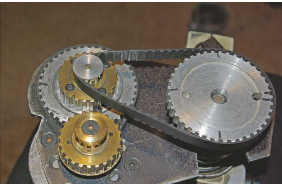
A view of the drive from below showing the thin flange fitted to the larger wheel on the motor shaft. This should almost touch the 40 tooth wheel on the countershaft.
