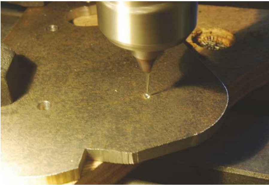
Picking up a centre punch mark using a sticky pin. Note that the position of the punch mark had to be adjusted.
