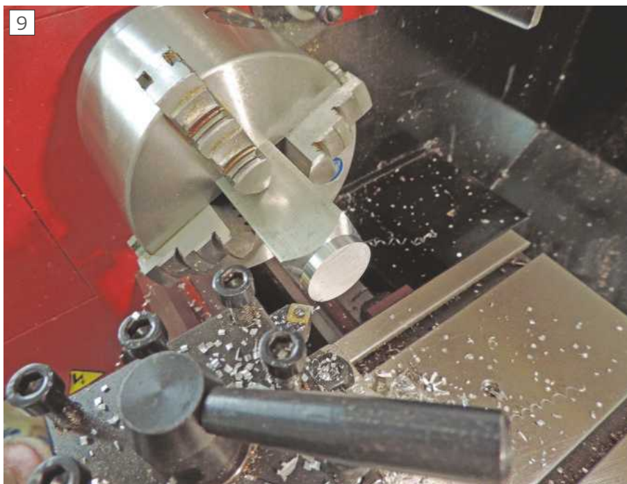
This self-centring 4-jaw chuck makes a task like putting a concentric spigot on square stock simplicity itself.
