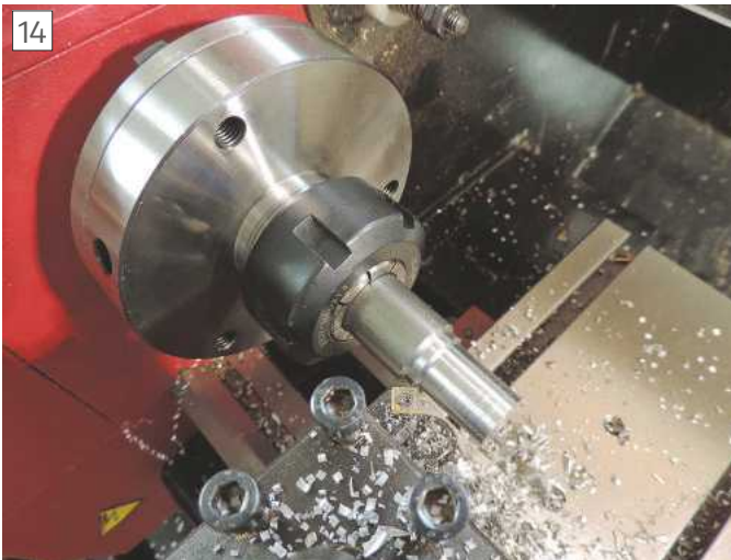
The ideal solution for a lathe is a flange mounted collet chuck, like this ER32 example fitted to the SC4.
