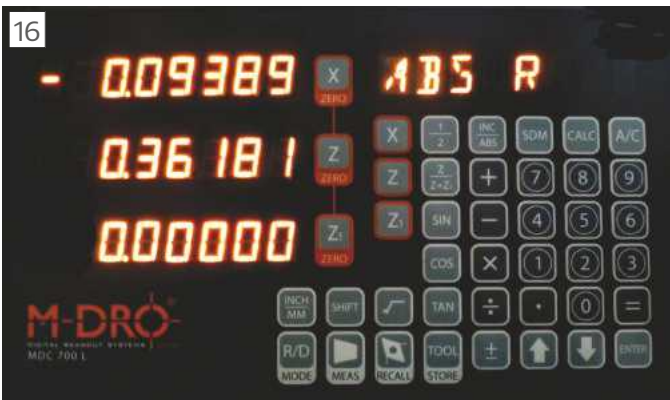
M-DRO showing new 0.36181" diameter
