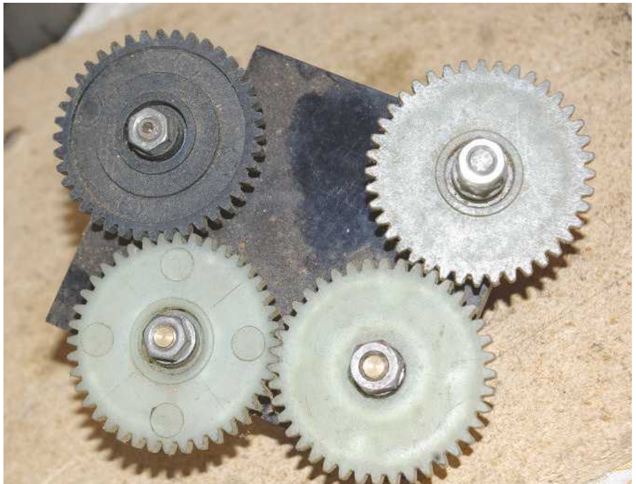
A simple thread cutting attachment for the Unimat. One gear has a short shaft with a fork to match the lead-screw end, the other has an expanding mandrel to go into the end of the spindle.
