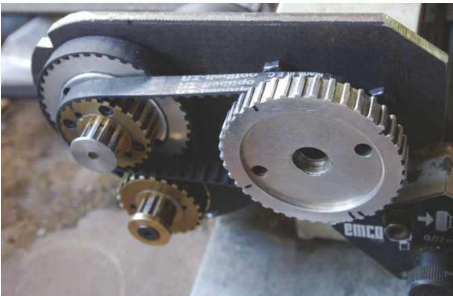
The new 6mm plate fitted to the lathe, before drilling for the guard. The less than perfect spacing of the teeth on the large wheel is noticeable.
