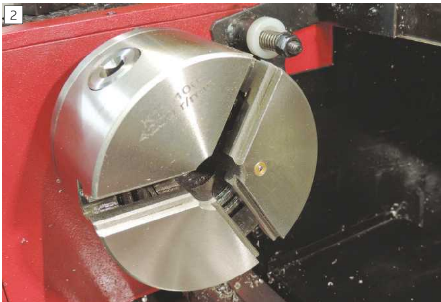
The standard 3-jaw sc chuck supplied with the Arc SC4-500 lathe, without jaws fitted. You can see the scroll, key socket, front oiling point and the maximum speed (4,200 rpm) marked on the body.
