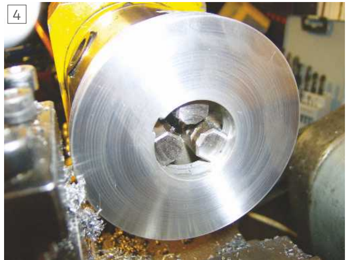
How internal jaws can be used to hold a hollow disc – this is a blank for a poly-vee pulley.
