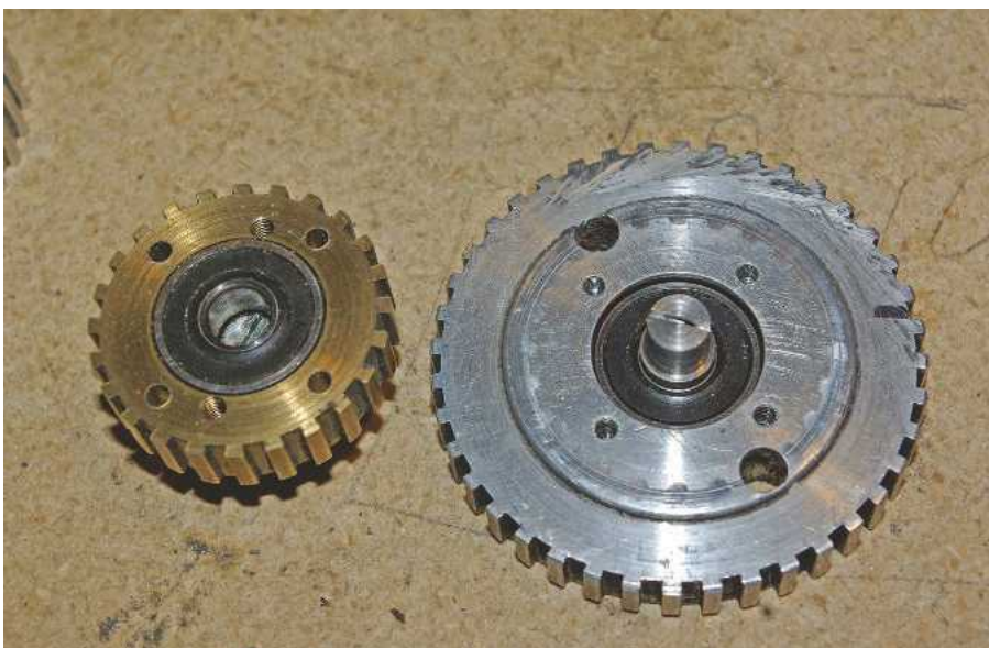
The two large wheels for the countershaft. These screw together trapping the bearings inside.
