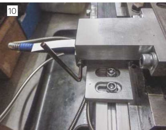
Adjusting gap between encoder and mag strip cover
