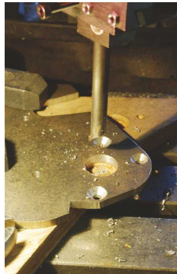
Boring a hole for the motor on the new 6mm plate.
