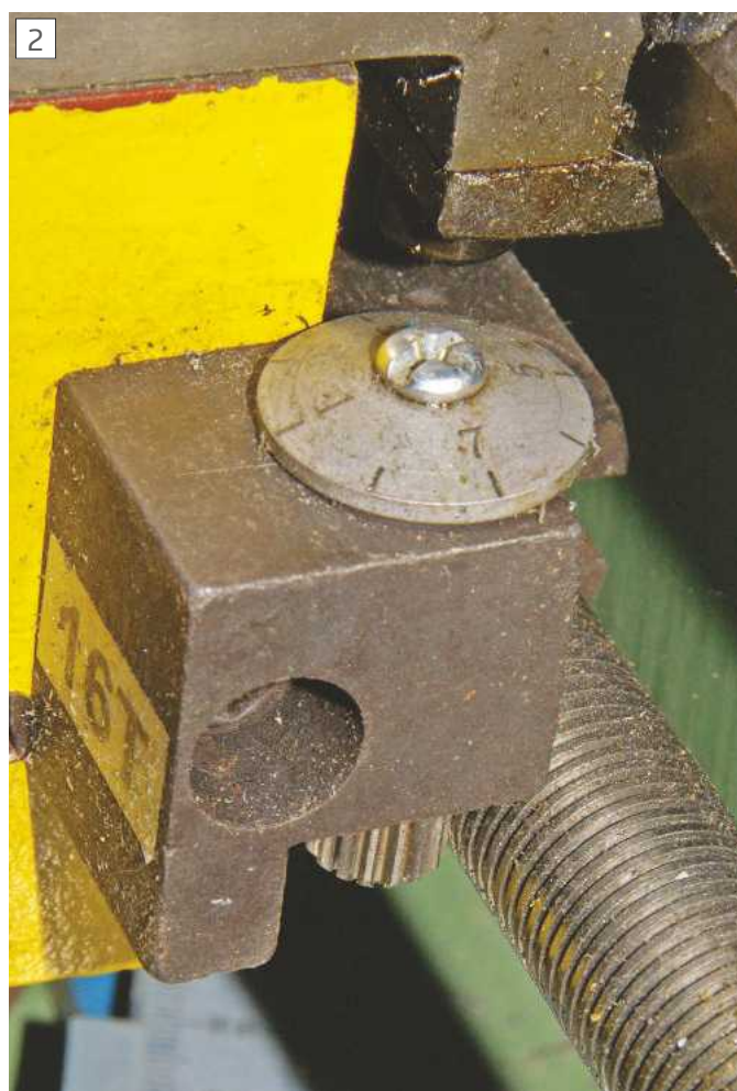
A Mini-lathe thread indicator, engaged with the leadscrew.
