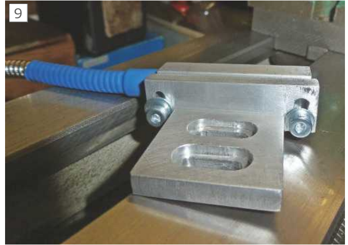
Encoder on new bracket
