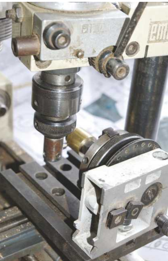
A posed photograph showing the kind of set-up needed to mill the wheels using the Unimat. Note that when set up in this way the dividing attachment only has one screw clamping it to the table, see text for a suggestion.
