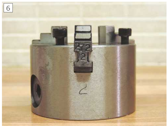
Many chucks have the jaw slots numbered.
