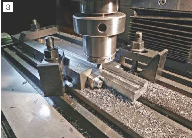
Milling slot to full depth with bracket fixed in place
