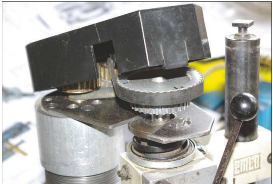
The original plate, set up on the milling attachment and showing that there is room for the cover to close over all the works.
