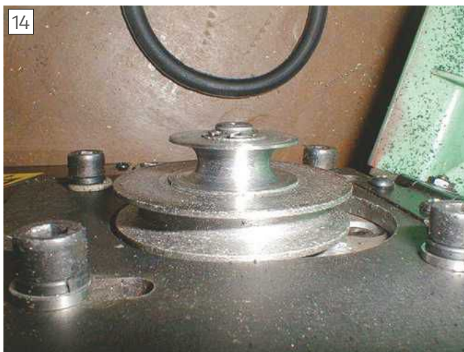
14 New pulley fitted.
