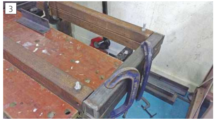
Ordinary g-clamps used to hold tubes in place
