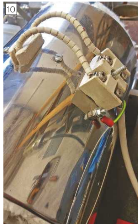
The ceramic connection block and ground connection
