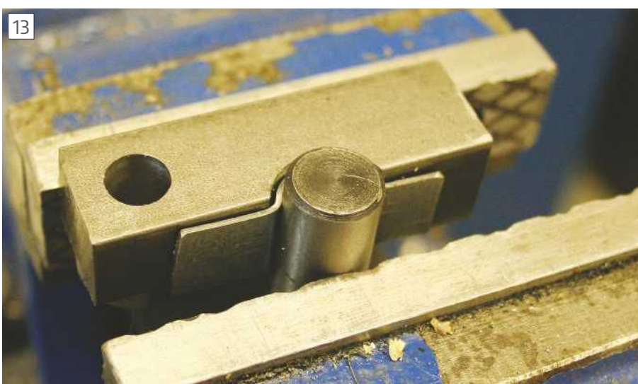
Body Clips are pressed in a simple jig.
