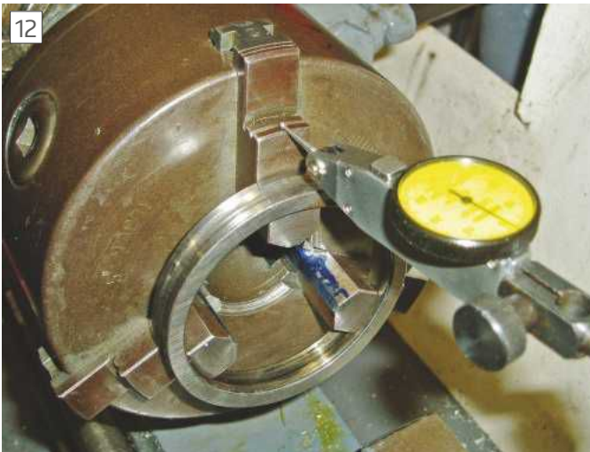
12 A ring is used to tension jaws for any checking or grinding of outside jaw steps.
