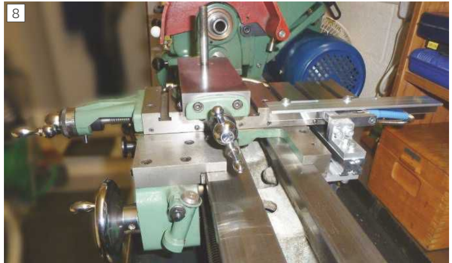
Cross slide encoder and strip fitted.
