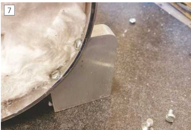
Legs are fastened with M5 x 8mm long screws
