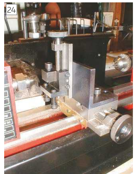
Toolpost vice used as a vertical slide.
