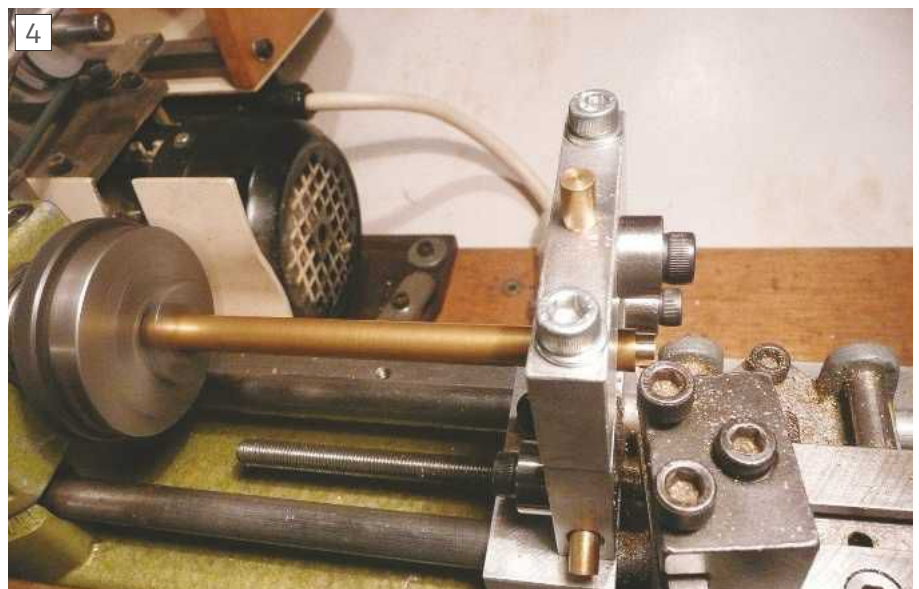
The assembled steady fitted to the lathe
