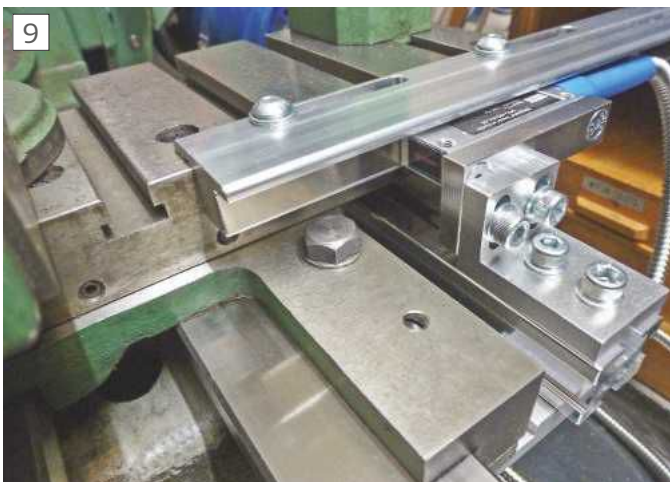
Forgot to reinstall the original Myford saddle clamp before fitting the encoder unit, fortunately there was just sufficient room!
