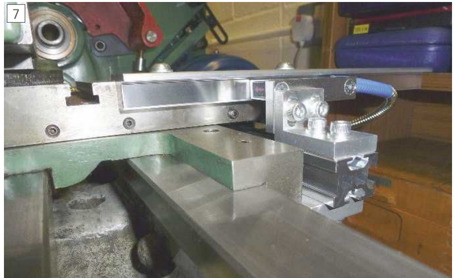
Shows the gap which has to be gauged with a piece of card between 0.25 & 0.5mm for both the carriage and cross slide.
