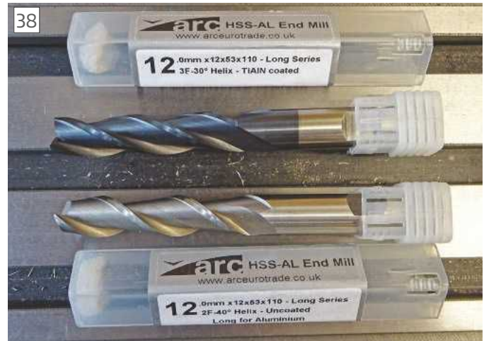
Different helix angles to suit material
