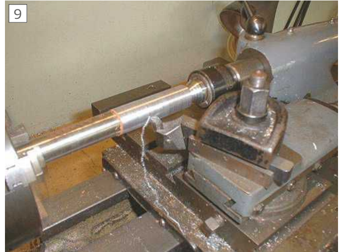
Sleeve mounted on shellac mandrel.
