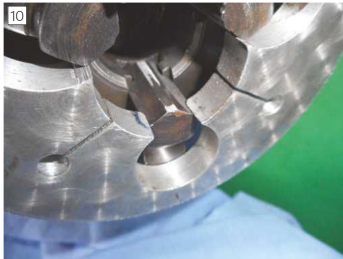
Shiny areas show high spots being removed.
