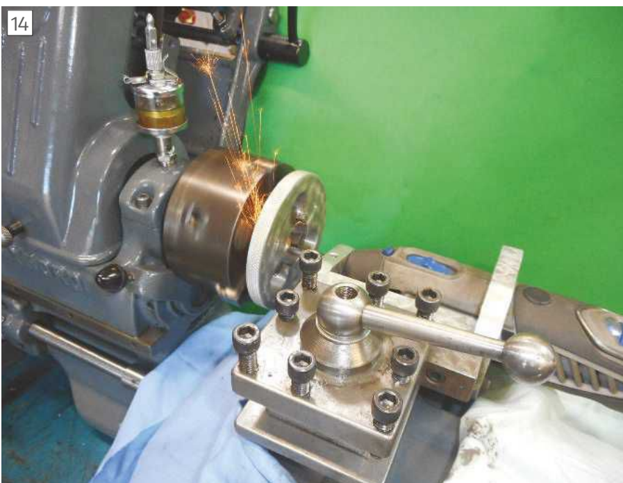
14 Chuck grinding requires only simple shopmade equipment.
