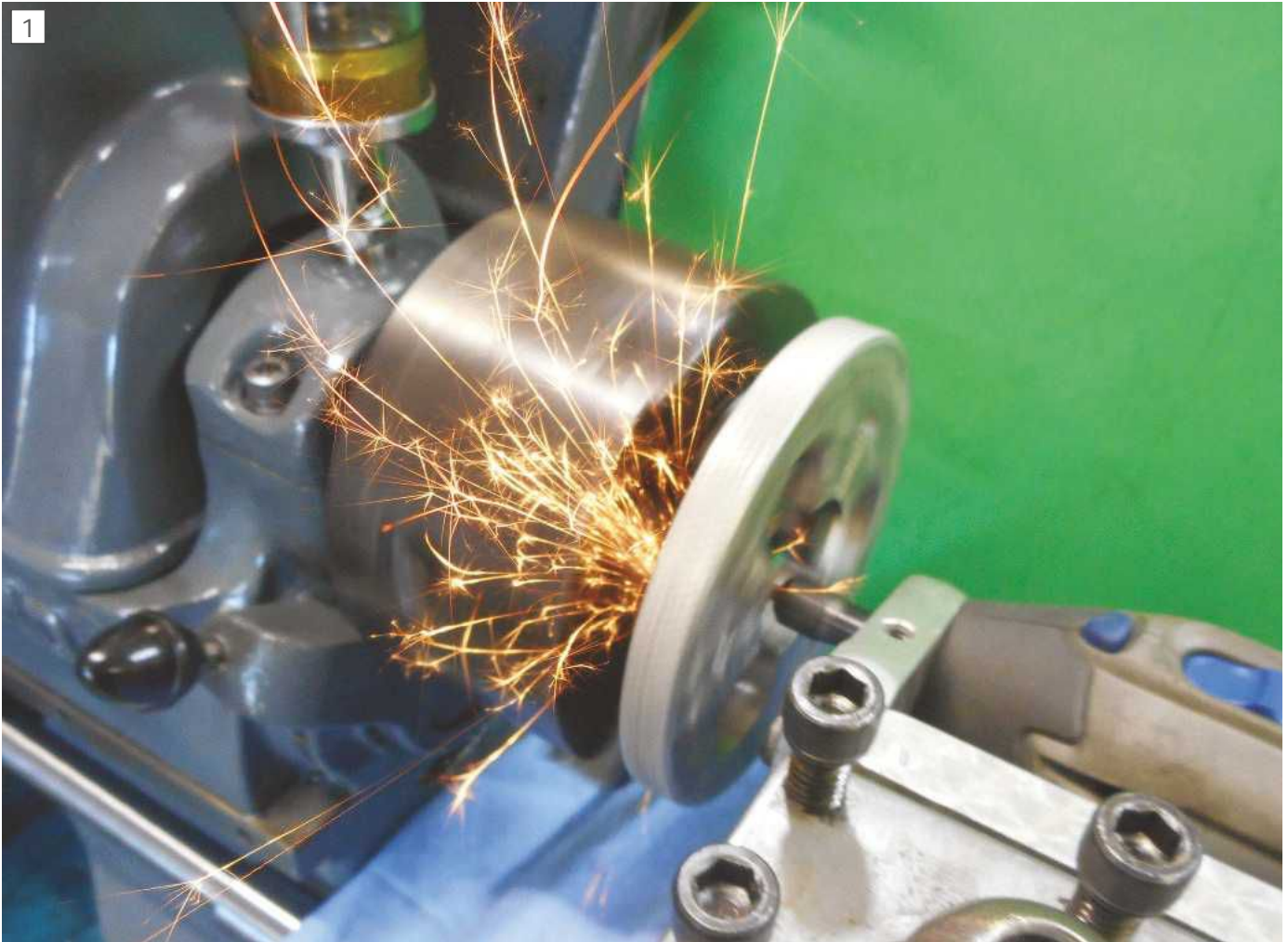
Sparks fly as the bell-mouthed chuck jaws are brought back parallel with a toolpost-mounted hand grinder.
