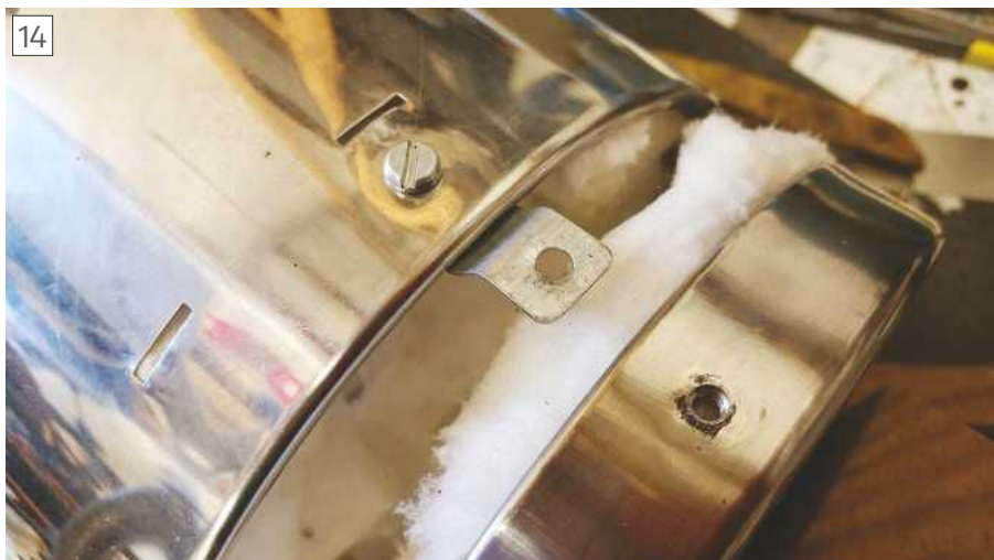
Clips are held in place with screws or self-tappers.
