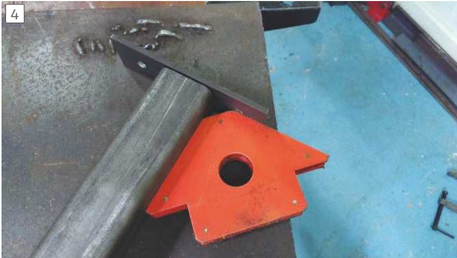
Magnetic clamp to get a 90-degree angle
