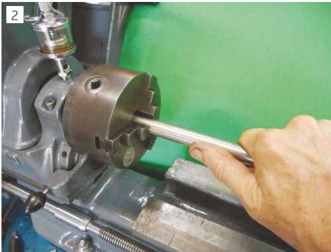
Distorted chuck allows noticeable movement of a test bar lightly gripped in the jaws.
