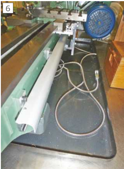
Carriage encoder, strip and cover fitted.
