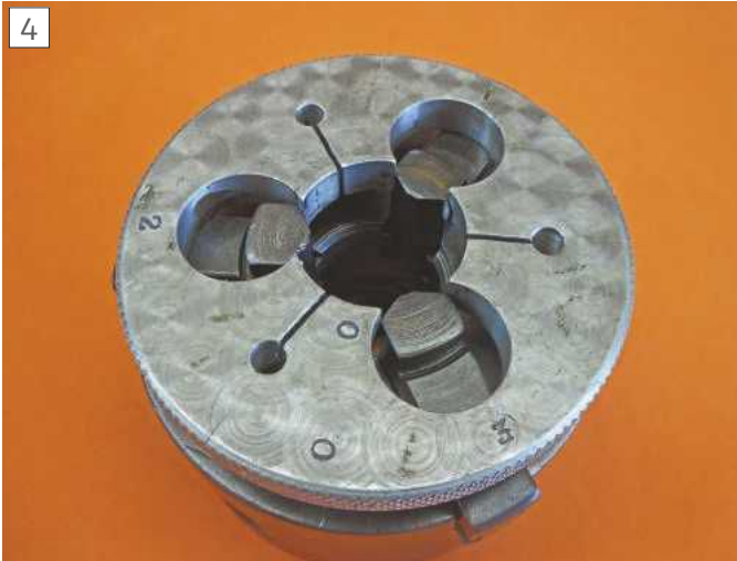
Central hole in plate is about same size as hole in chuck.
