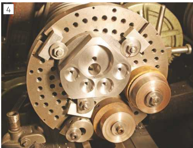
The fixture fixed to the faceplate with balance weights
