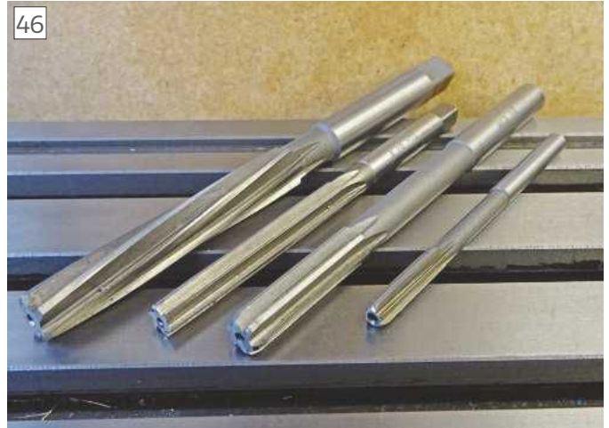
Hand and machine Reamers
