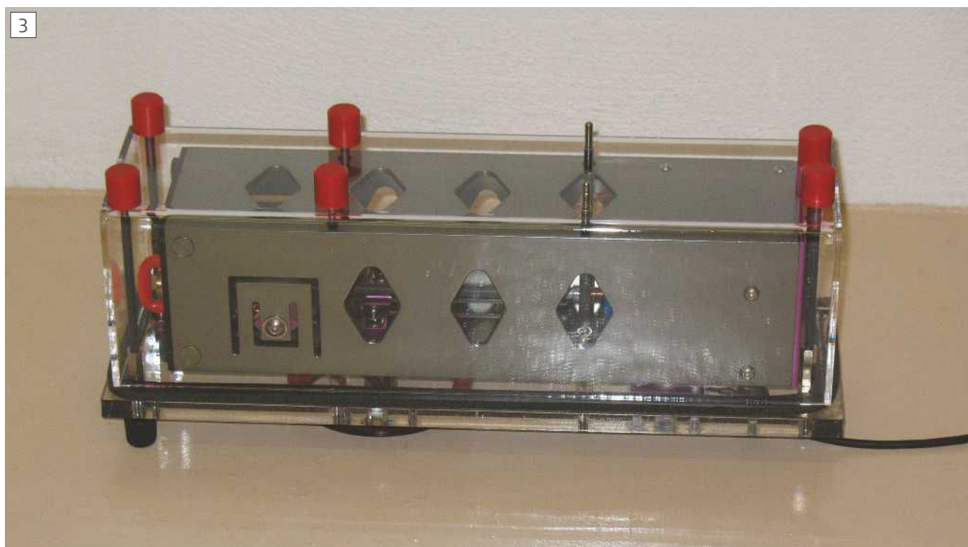
My homemade VS1 vertical-motion seismometer.
