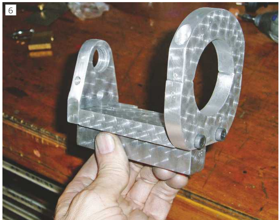
Toolpost hand-grinder mounting bracket is cut from aluminium plate and screwed together.
