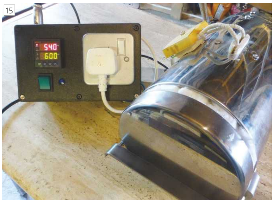
Digital Controller enables exact temperature selection.
