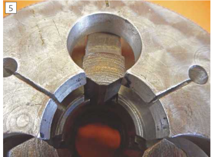
The three holes allow jaws to protrude for grinding.
