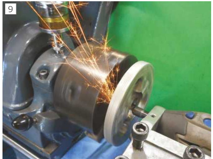
Grinding stone just kisses the high-spots on jaw at start of grinding.
