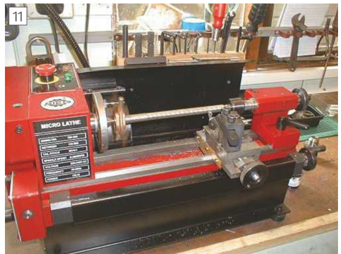
Turning test bar.
