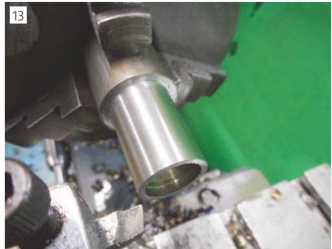
13 Result: A .100" deep cut produces no chatter now the chuck grips firmly with no bell-mouthing.
