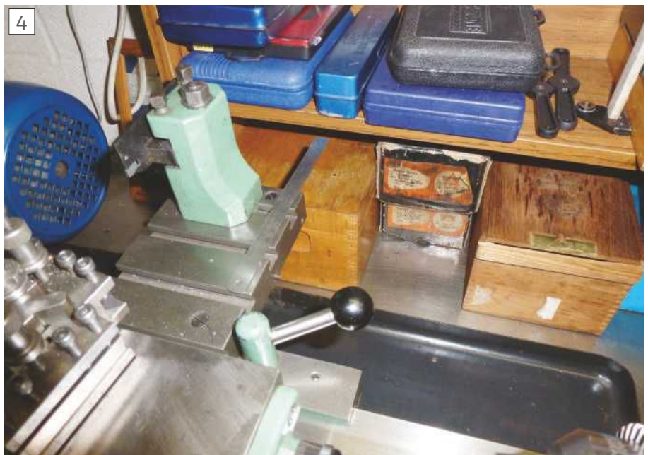
Checking for clearance beyond cross slide.
