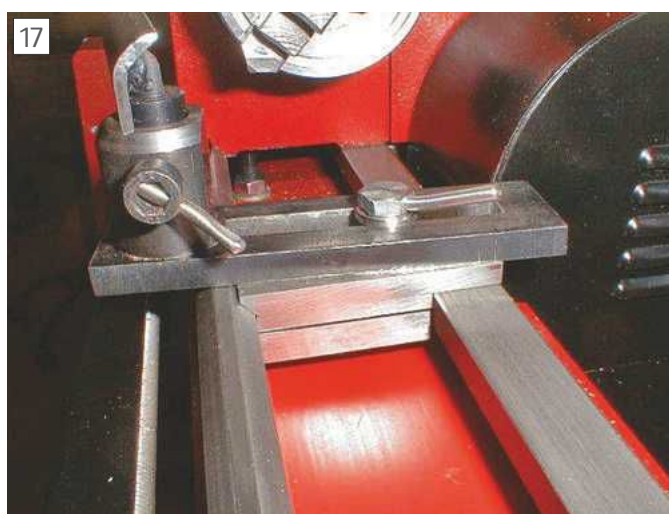
17 New base for t-rest.
