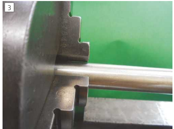
Bell-mouth at right-hand end of jaws is visible and measurable with feeler gauges.
