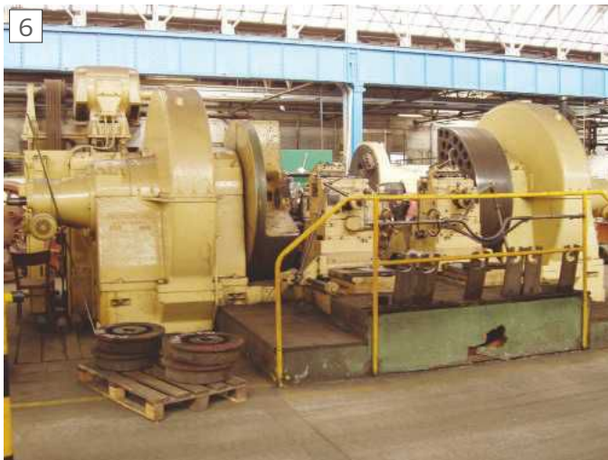
I don't suggest you need a wheel lathe, but a smaller centre lathe is essential
