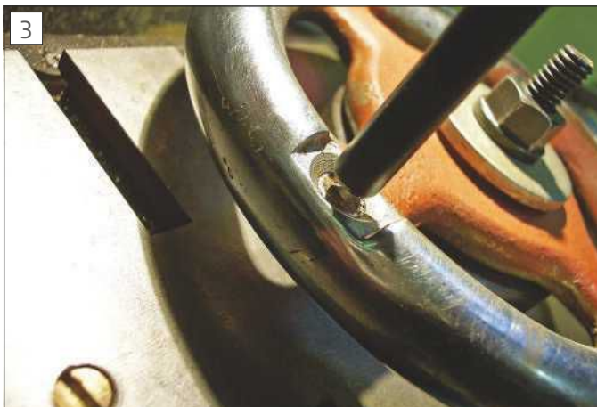
Finding the centre on the broken thread
