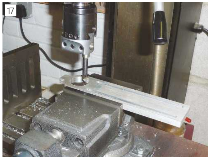
Boring the banjo to a sliding fit on the rear bearing.
