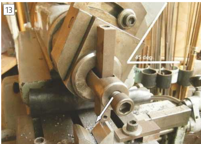
Note the drilled hole which give the tool somewhere to run out at the base of the vee
