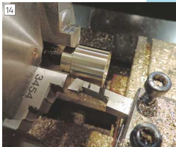
Using a mark of the tool shank to judge the depth of a hole. The top slide has been swung over to create a tapered hole.
