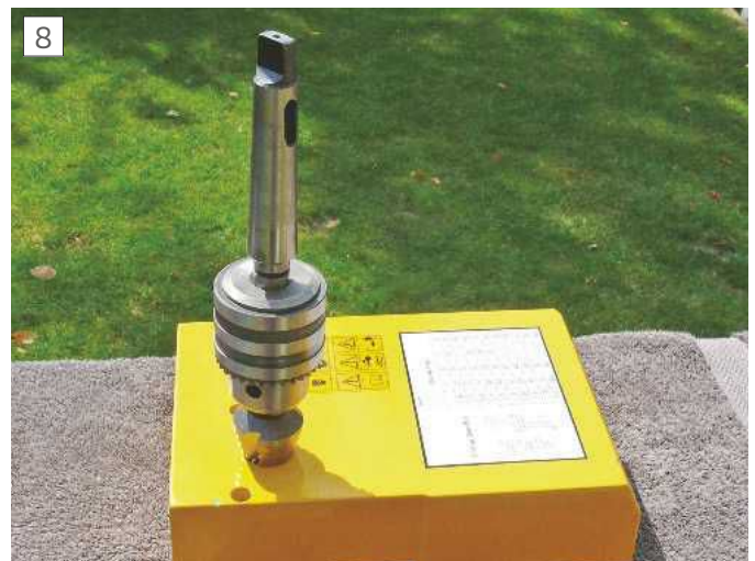
Enlarging cover hole with hand-held chuck and step drill
