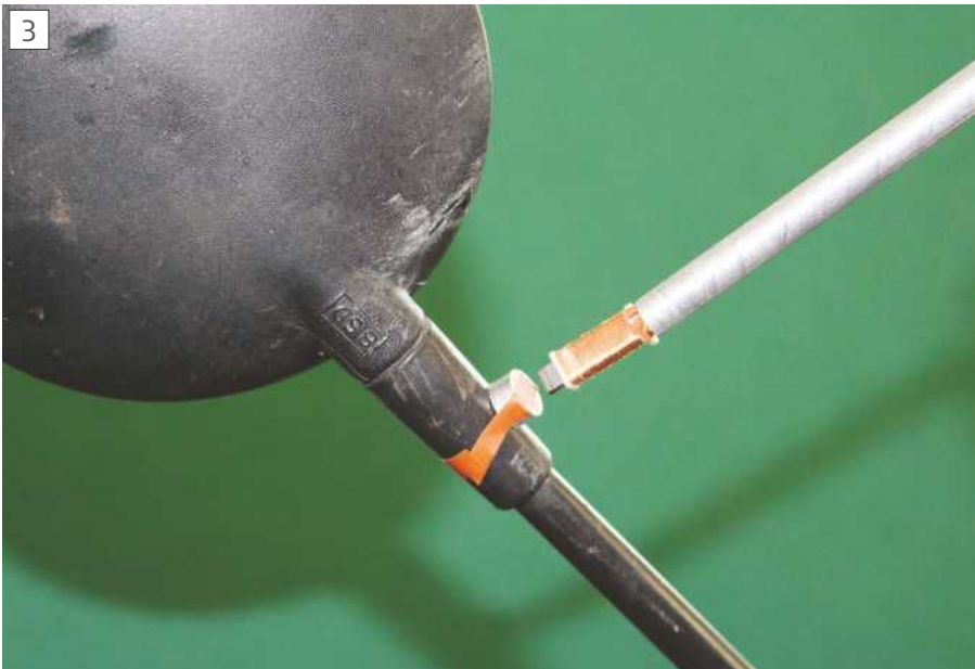
Arrangement of coil and magnet used to measure the mirror's vibration frequency.
