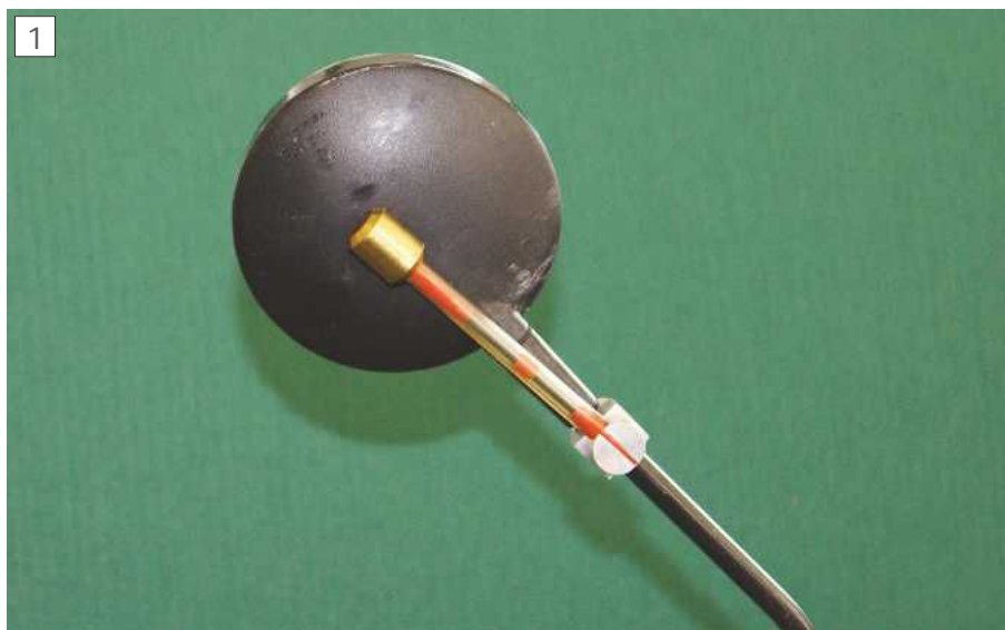
Tuned mass damper fitted to my motorcycle's mirror.
