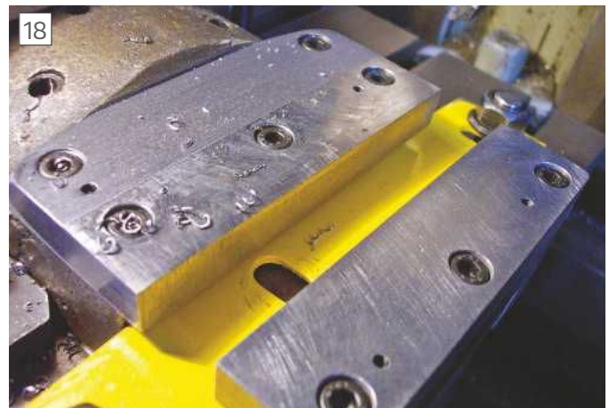
Finishing cuts on the shaper
