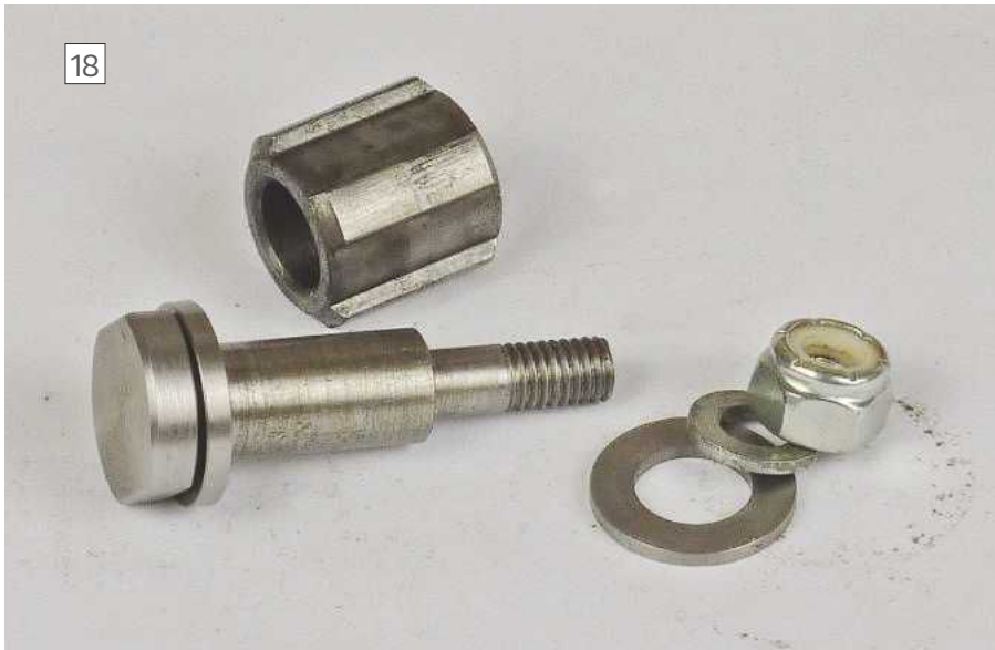
18 Gear axle showing longer splined bush for fitting two gears side by side and preventing relative rotation between the gears.
