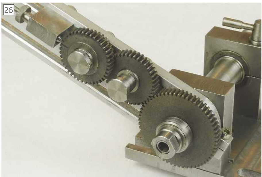
An intermediate gear being used to prevent clearance problems. The size of this gear does not affect the gear ratios.
