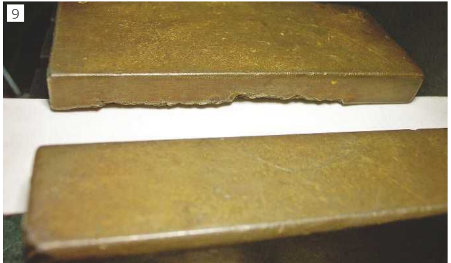
Crumbling on the underside of the tool post slot
