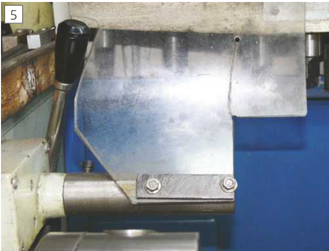
Modification to prevent fouling tension lever
