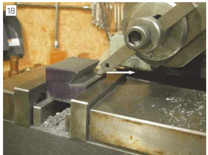
Finishing the horizontal surface
