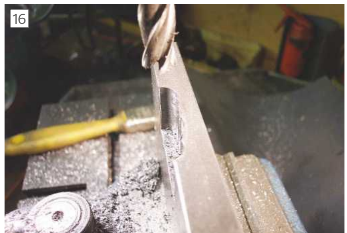
Restoring the feed nut pocket height
