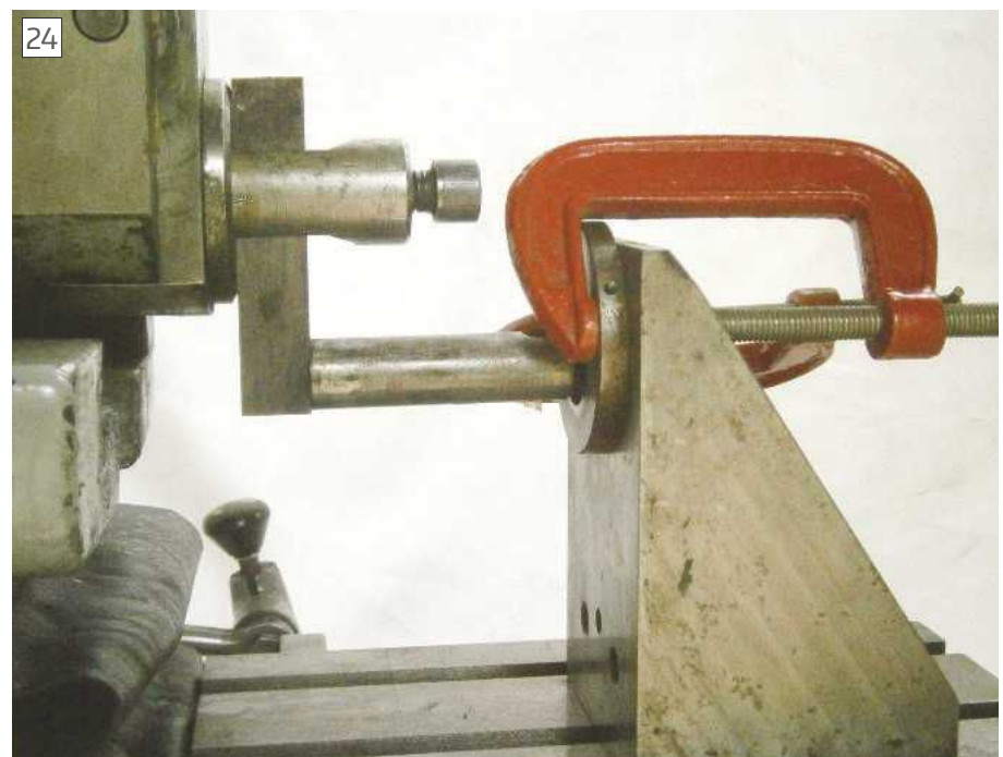
Setup for an internal keyway, the angle plate has a hole and the clapper box is locked
