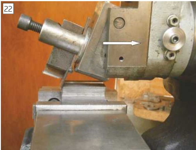
Hinge lifts cutter clear of work on return
