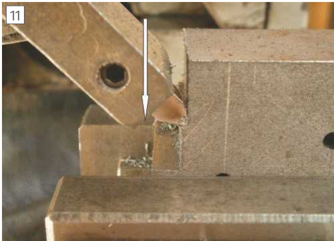
Generating a vertical surface
