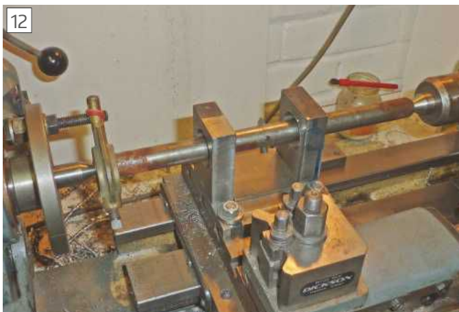
Line boring the bearing housings using a boring bar between centres on the lathe.
