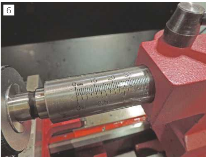
A clearly graduated tailstock barrel is a great asset on any lathe.
