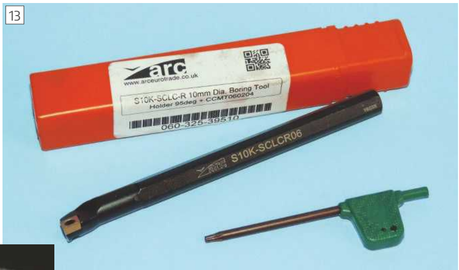
A boring bar fitted with a tungsten carbide insert.
