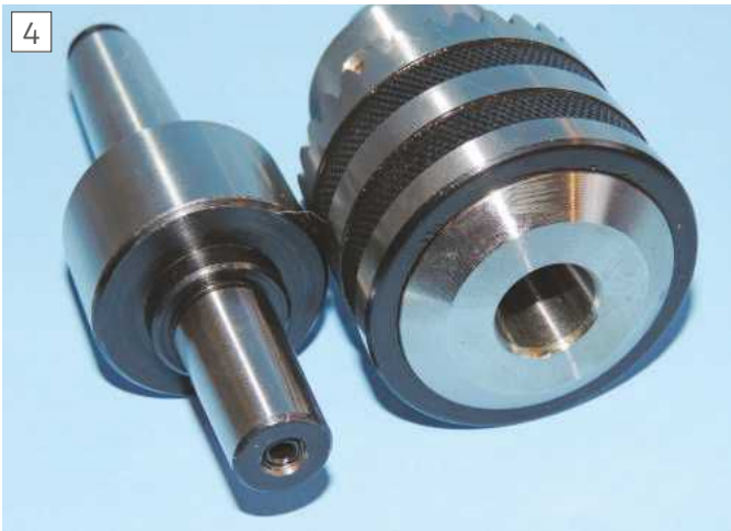
B16 taper and matching socket on a chuck and a rolling centre.
