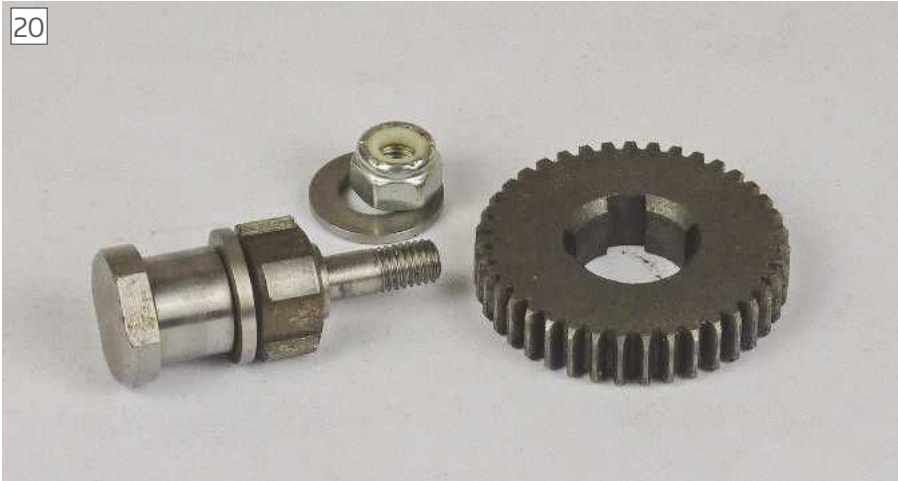
View of gear axle with fittings assembled. The gear slides onto the splined bush.
