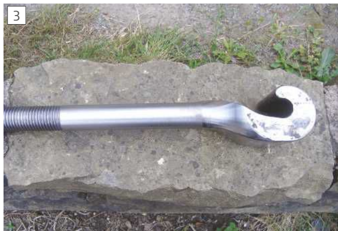
A component that would have traditionally been forged, made with a combination of flame cutting and cnc turning
