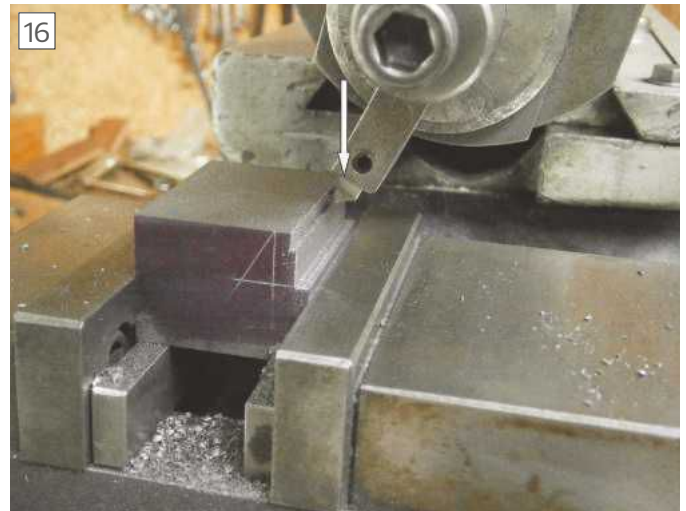
Initial cut for edge of dovetail
