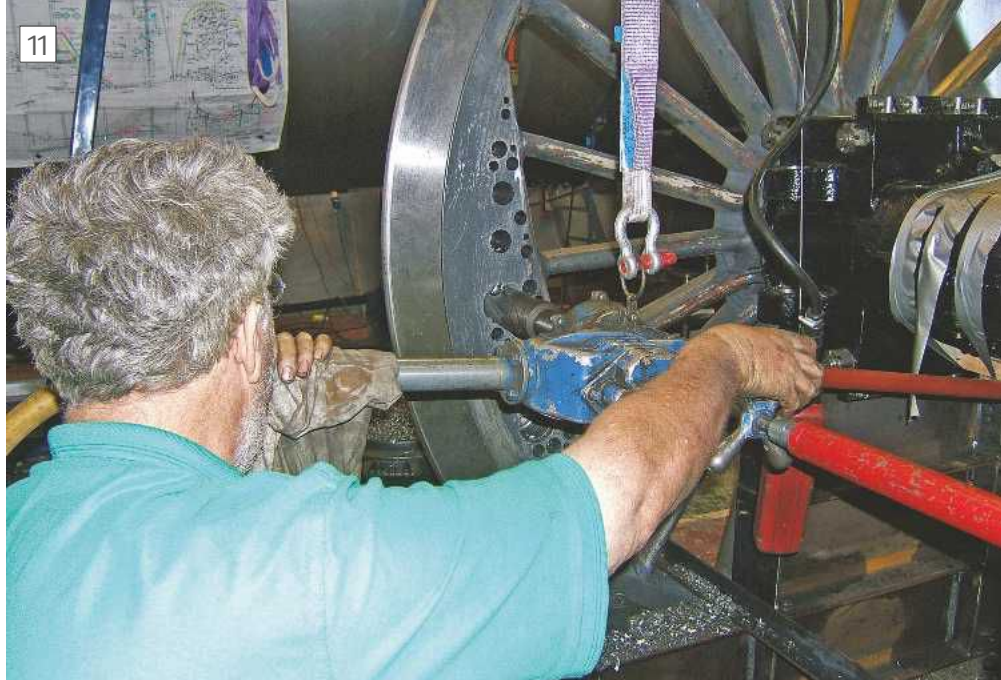
A windy drill in use drilling balancing holes in driving wheels. Otherwise a job requiring an expensive boring machine with a right angle head.
