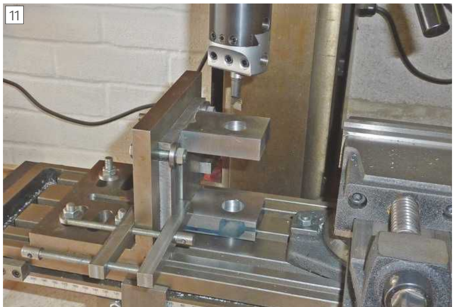
Boring the bearing housings undersize with a boring head.
