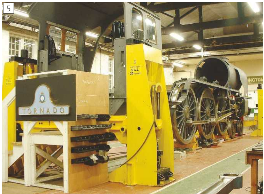
A set of synchronized lifting jacks makes the wheeling easy
