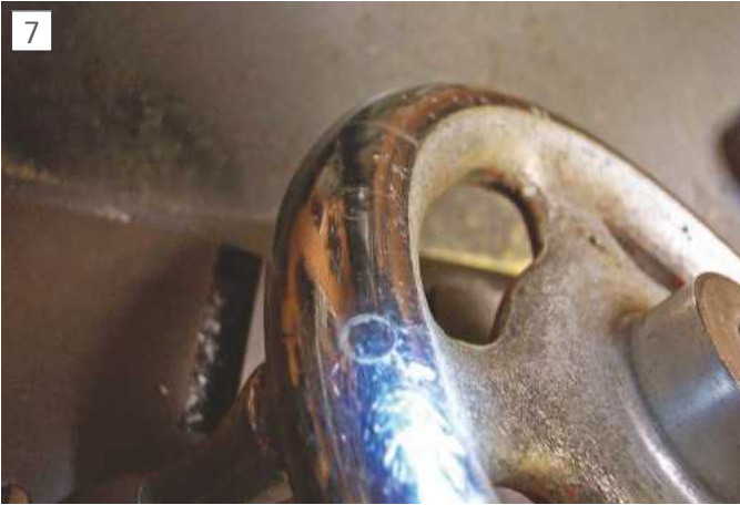
The cross pin glued back in place
