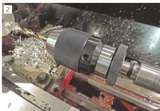
This 13mm capacity keyless chuck is a pleasure to use and has excellent grip.
