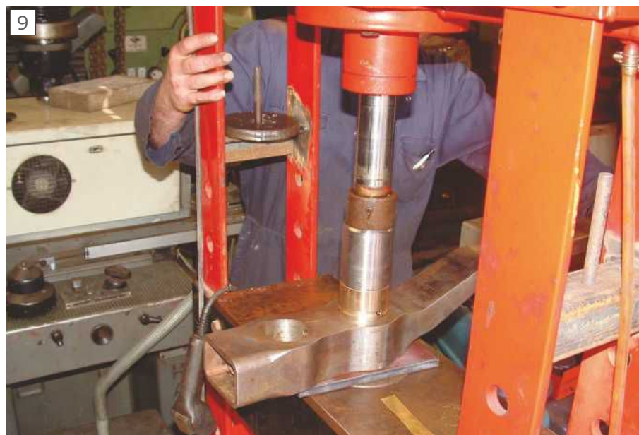
A small hydraulic press, pressing in a bush in a combination lever
