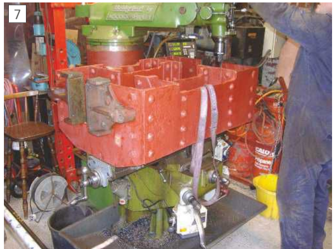
A 2ft gauge pony truck, showing the versatility of a Bridgeport
