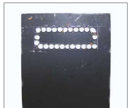
Mike Cox's Chain Drilling Jig
