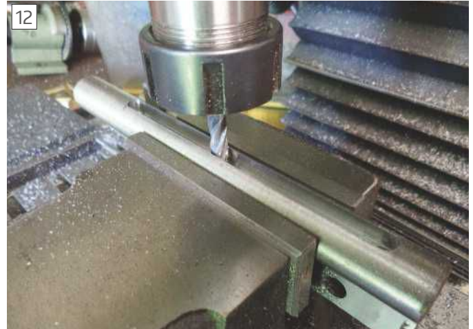
Cutting the Key way with a slot drill
