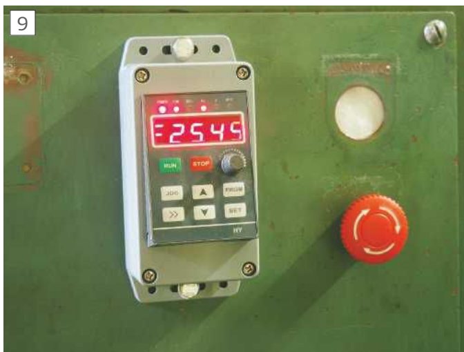
A neat feature of the VFD allows the control panel to be mounted remotely.
