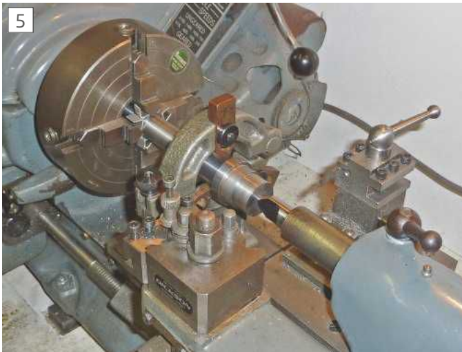
Setting up the part-finished spindle in the four-jaw chuck and fixed steady ready to machine the spindle nose details.
