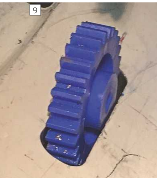
The proposed gear in place for a trial fit.
