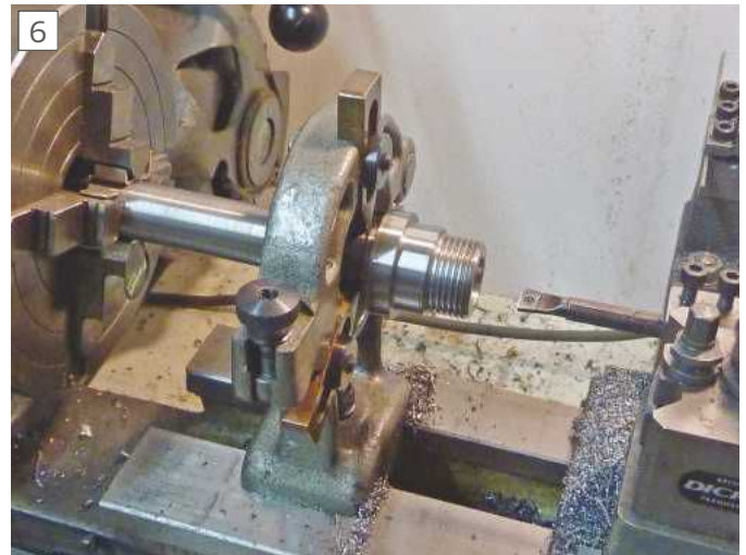
Making the tapered spindle bore.
