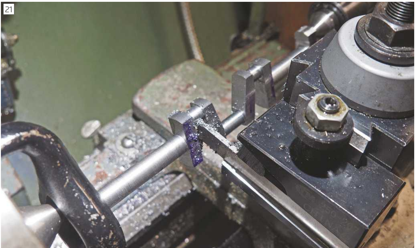
Turning a crankshaft between centres.
