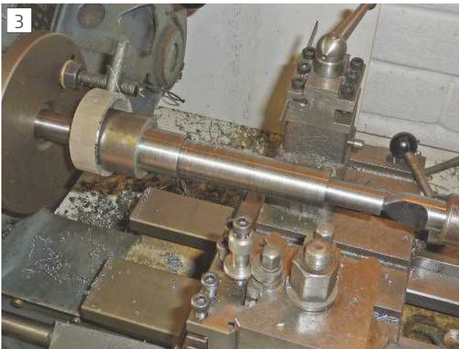
Roughing out the spindle between centres on the lathe.
