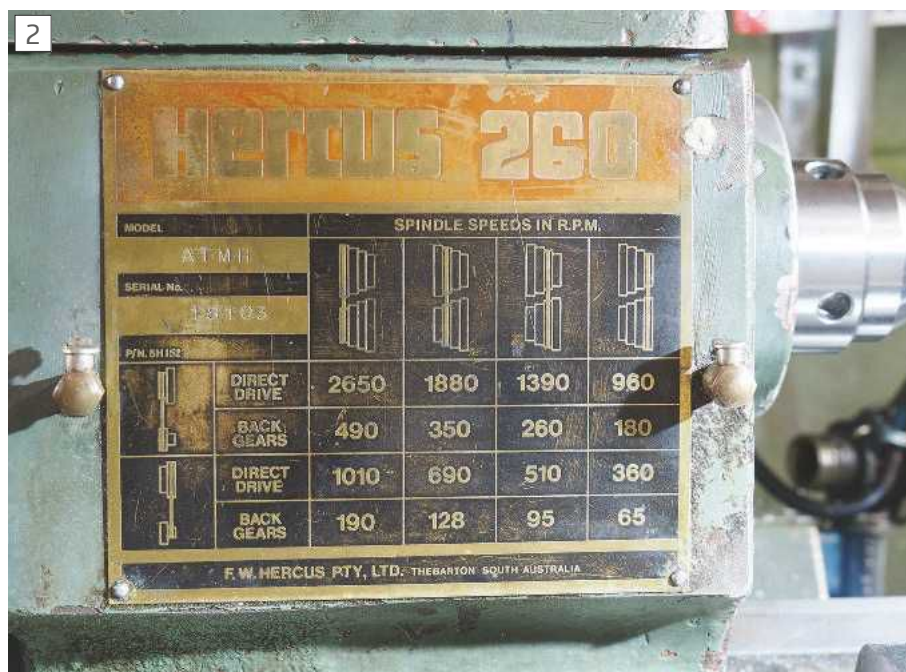
Spindle speeds on the headstock. The serial number indicates a machine from about 1983.
