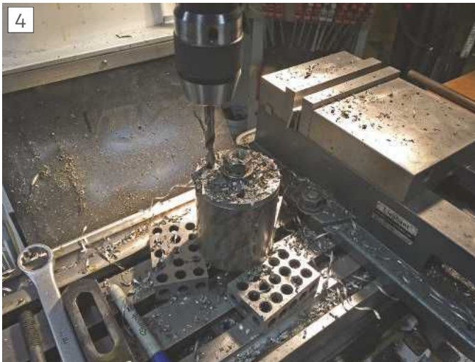
Extension piece bolted to the quill and machined to matching diameter.
