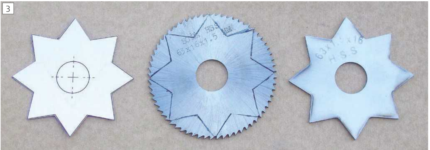
Making the 'star system' parting blade
