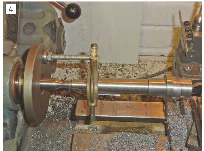
Continuing roughing out operations on the spindle.
