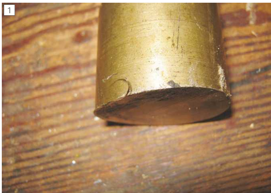
Saw cut run off
