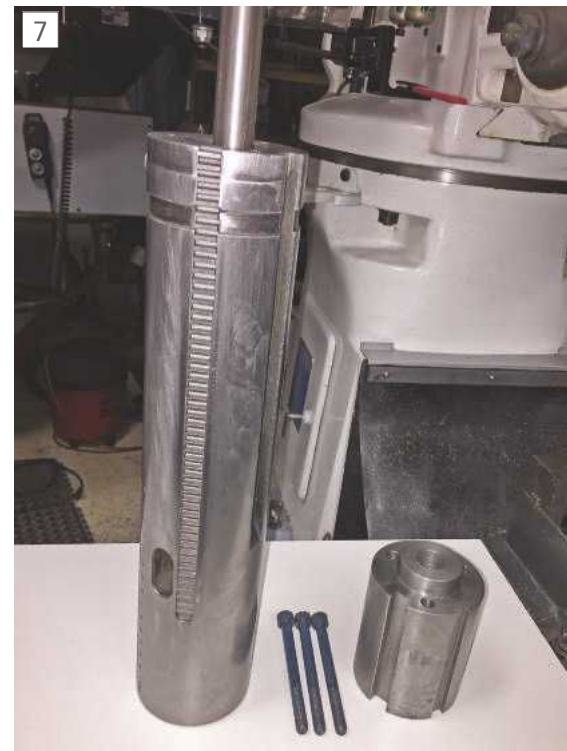
Component parts of the quill extension showing position of gear rack.
