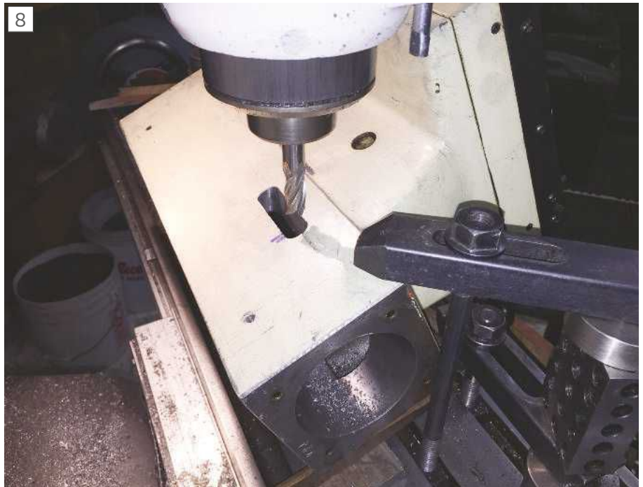
The tailstock set at 25 degrees and the gear access hole milled.
