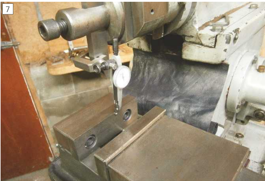
Aligning fixed jaw with the ram
