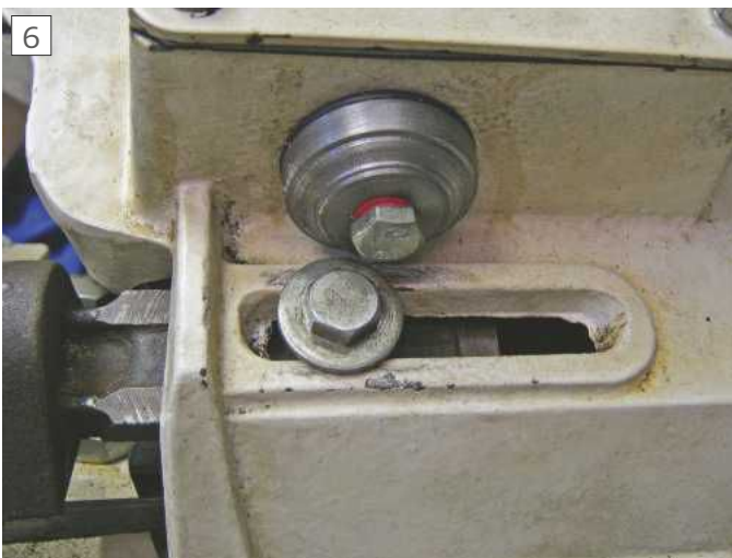
New hole closure piece showing "o" ring seal
