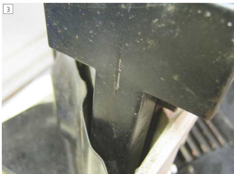
Blade wear mark on blade guide
