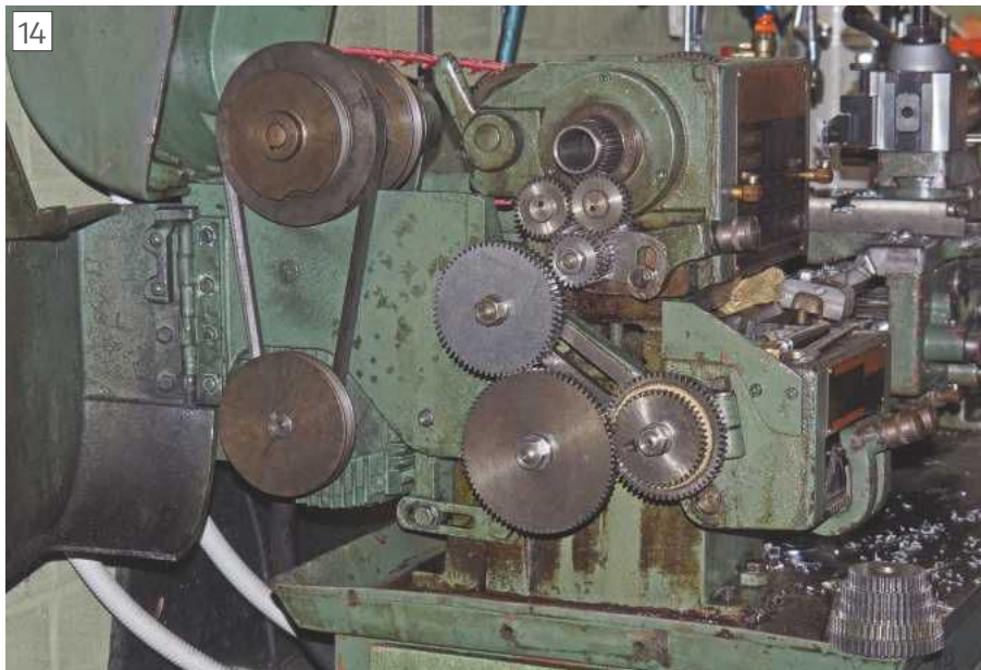
Set up for cutting Imperial threads. The chunk out of the countershaft pulley flange causes vibration at high speed and will have to be repaired or the pulley replaced eventually.
