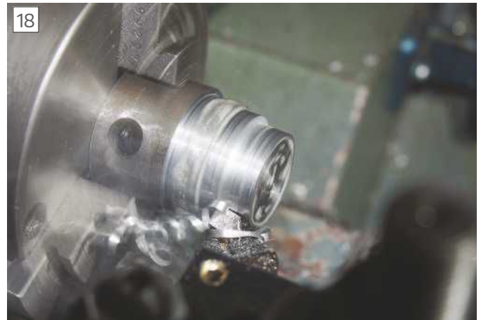
A 2 mm cut in mild steel with an "Eccentric Engineering" tangential tool.
