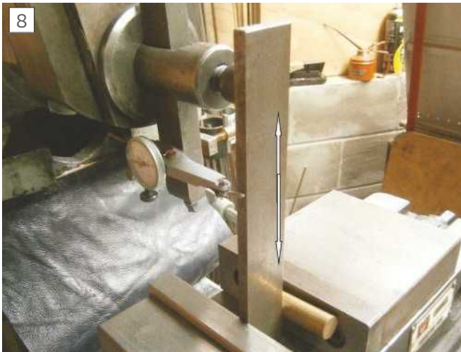
Checking the fixed jaw is vertical
