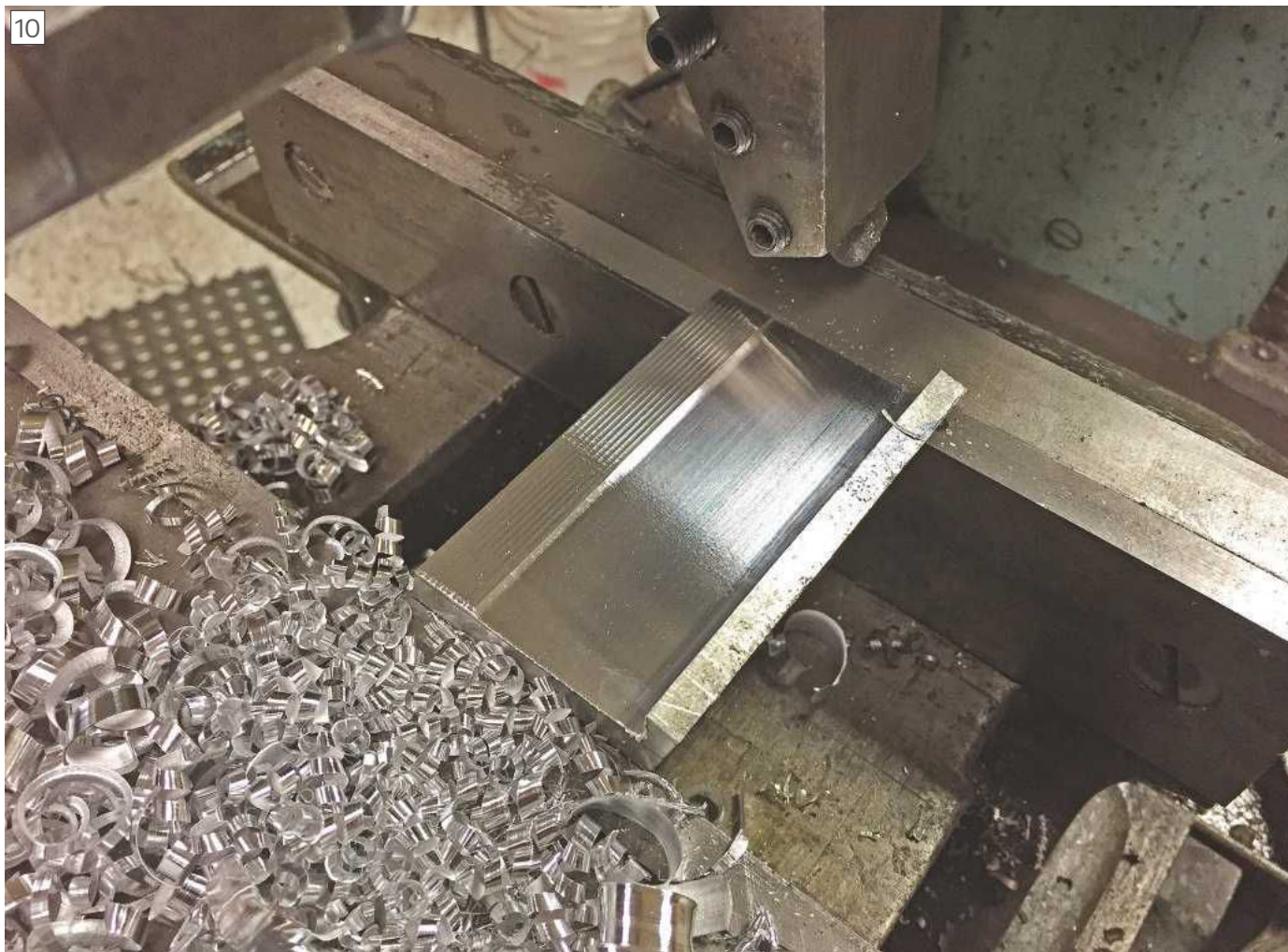
The housing being roughed out under the shaper.
