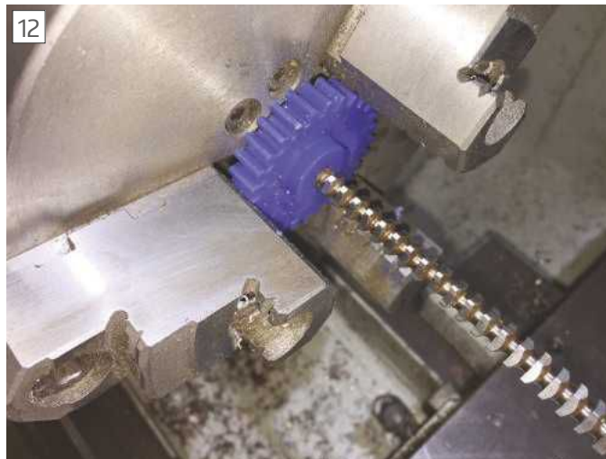
Broaching a 1/4" square hole in the gear.
