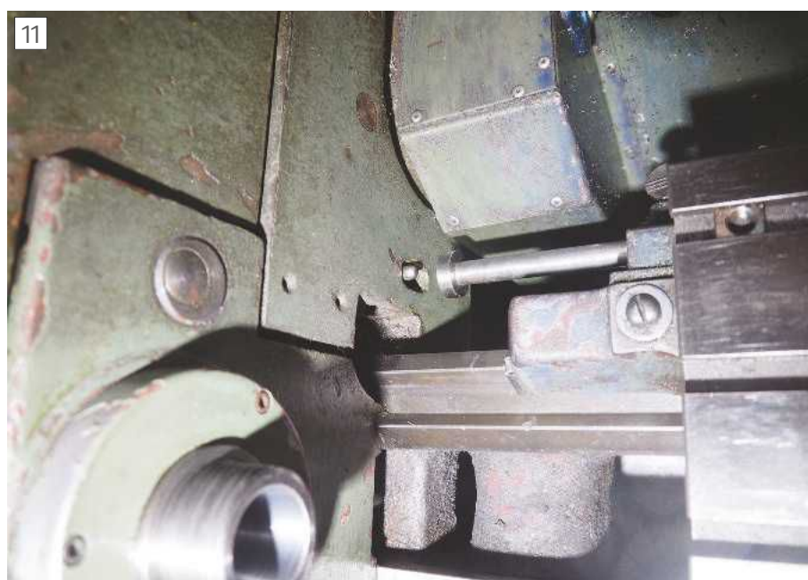
The automatic saddle stop operates the headstock cover interlock switch via a separate lever.
