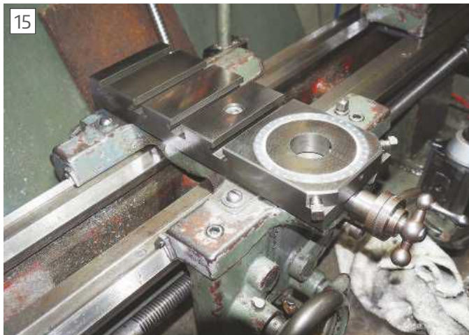
New production T-slotted cross slide. The round head screws fasten the travelling steady.
