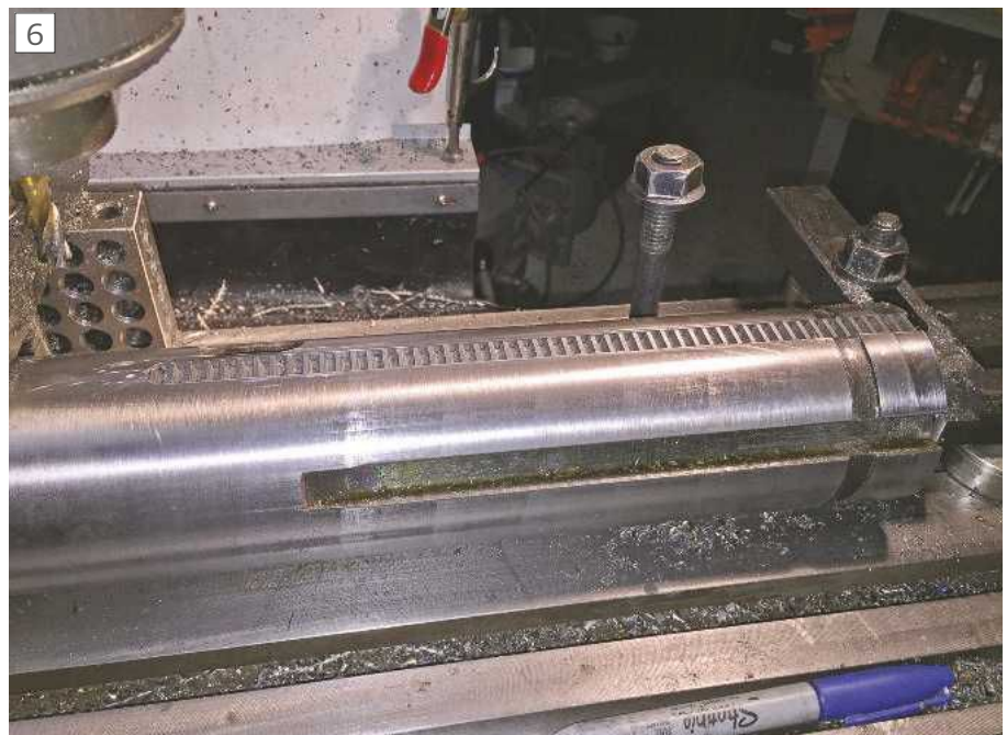
Assembled extension showing keyway slot in foreground and recessed rack.
