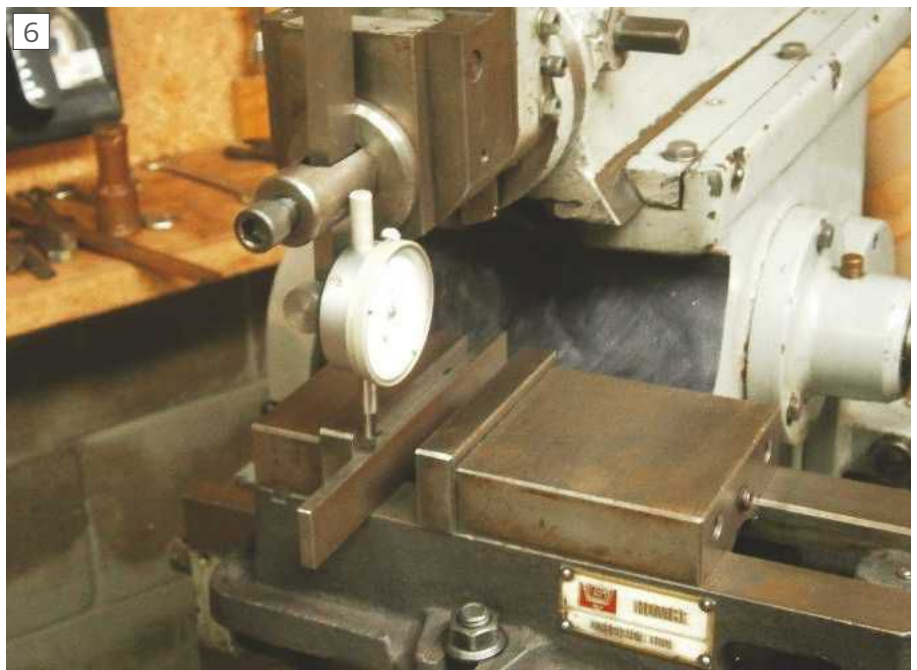
Checking vice base is horizontal
