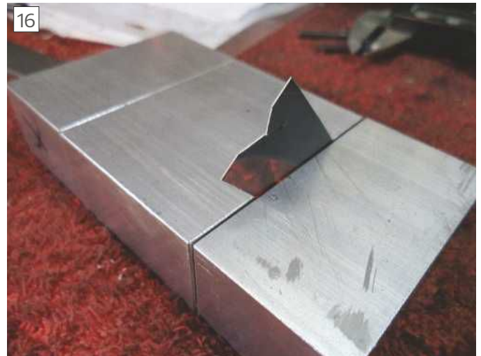
Card placed in the joint to give pinch
