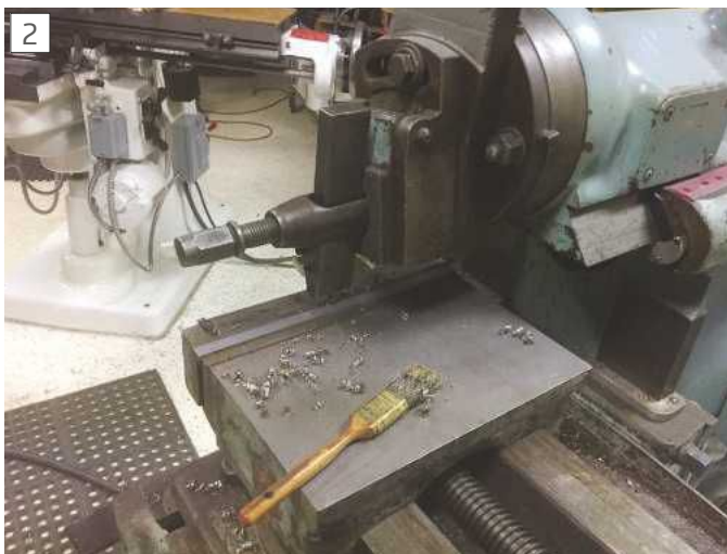
Turning a spigot on the extension piece to match the existing quill.
