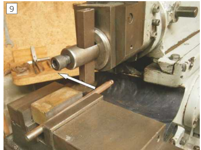
Round bar ensures the work is aligned with the fixed jaw
