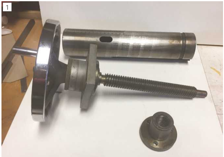
Disassembled original quill, LH acme shaft and bearings and nut.
