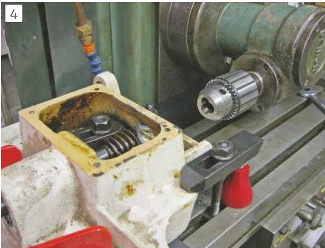
Main bandsaw casting clamped in line with swung vertical head
