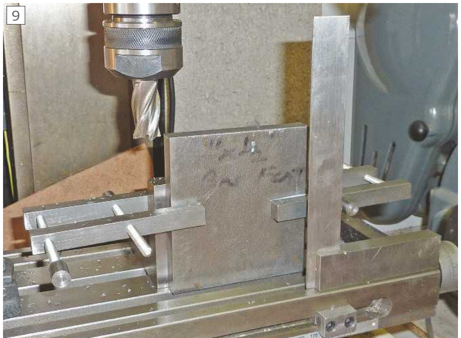
Machining the first baseplate edge.
