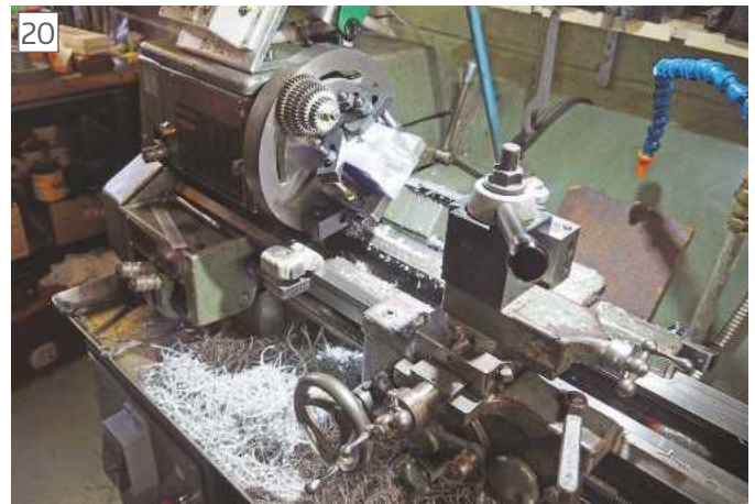
Boring a "Mastiff" crankcase from the solid on the faceplate makes a lot of swarf.
