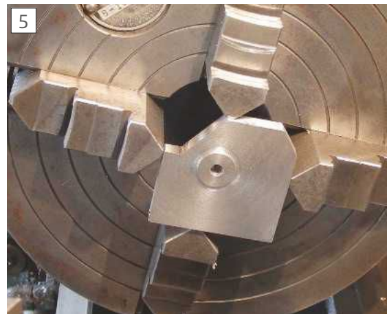
Turning the boss on part ST1.
