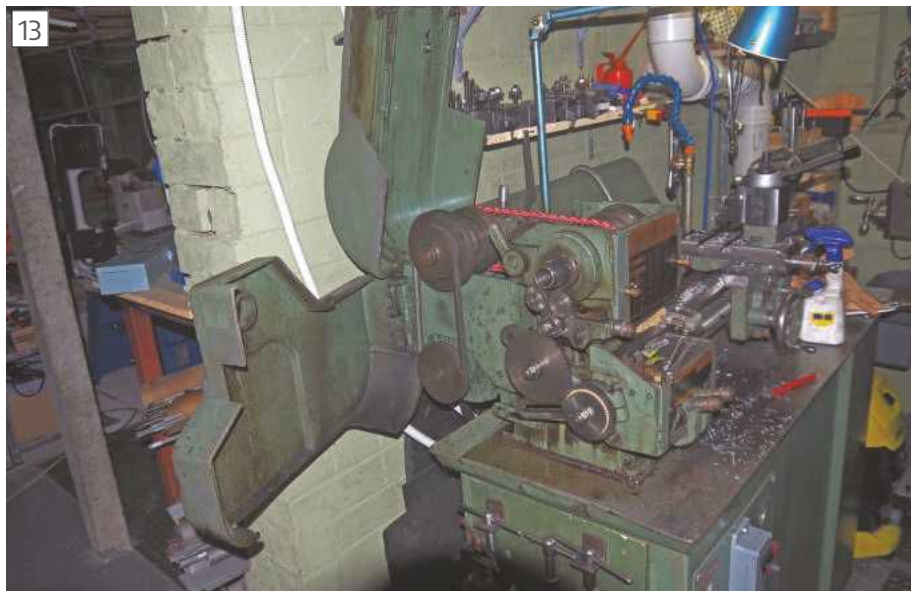
Motor drive belt in high speed. Projections on the covers are just visible close to the hinges. These form a mechanical interlock to prevent the gear cover being opened unless the top is first lifted to operate the safety micro-switch.
