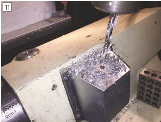
Tailstock in second setup to pilot drill the housing.
