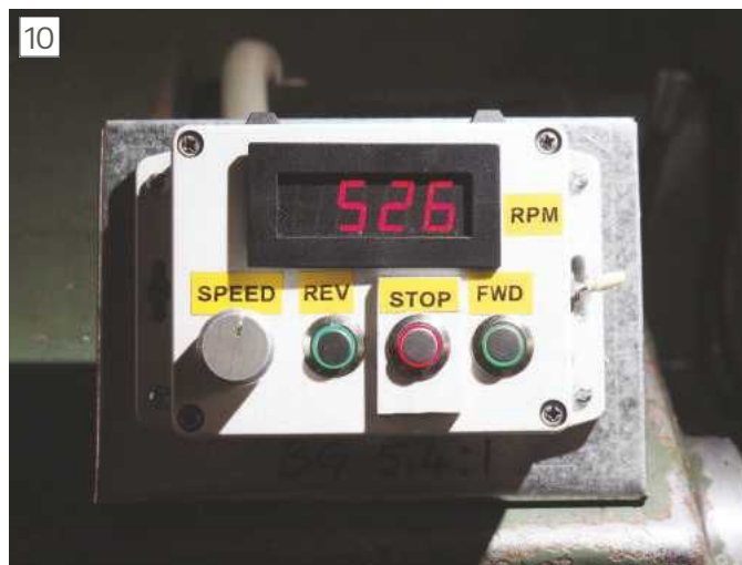
The basic controls are mounted on top of the headstock cover.
