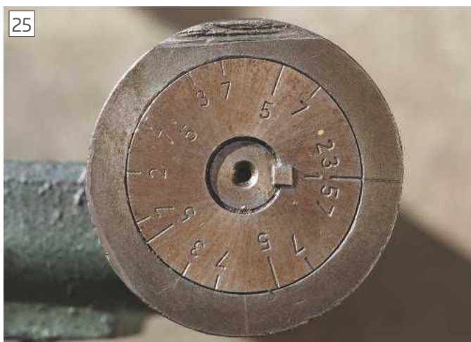
I'm sure you would eventually get used to reading the dial and re-engaging the half-nuts correctly but using the VFD makes it unnecessary.
