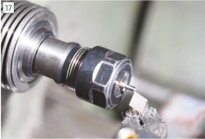
ER16 collets will grip down to 1 mm stock. High speeds and very sharp tools allow it to be machined easily.
