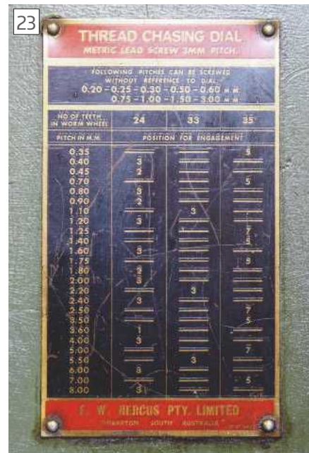
Thread chasing dial information. The camera didn't move, the embossing and printing aren't registered. This is the only sloppy work anywhere on the machine.
