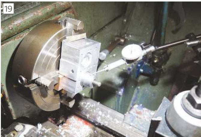
Setting up a part finished "Mastiff" cylinder block in the four-jaw chuck. Internally threaded chuck bodies give minimum overhang.
