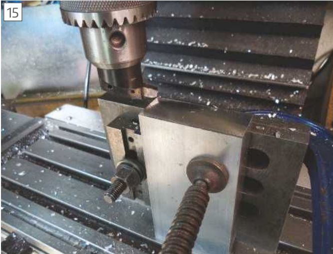
Fly cutting the material for three way clamp square
