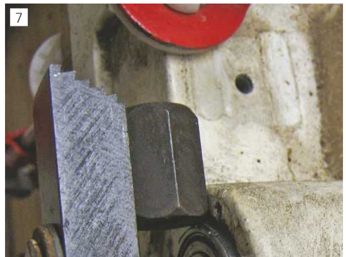
Drawing the bearings out using a piece of studbar
