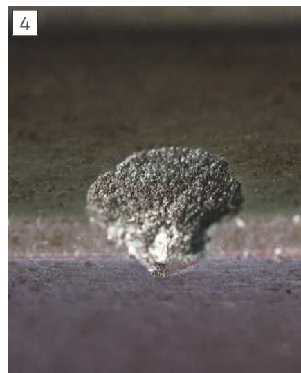
Hardened beds don't distort when things are dropped on them, they chip.
