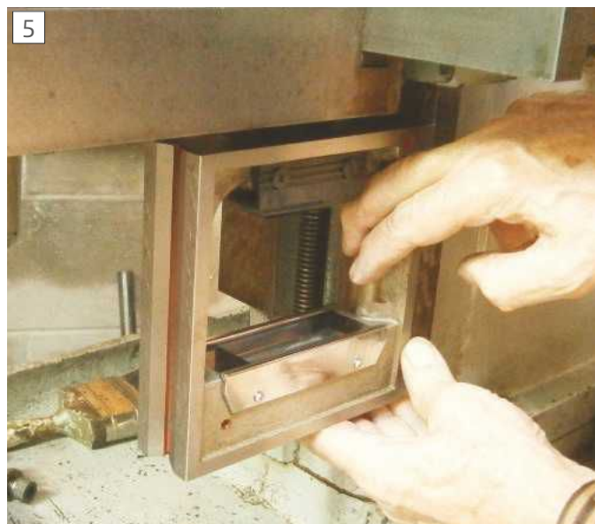
Face of vertical ways vertical.
