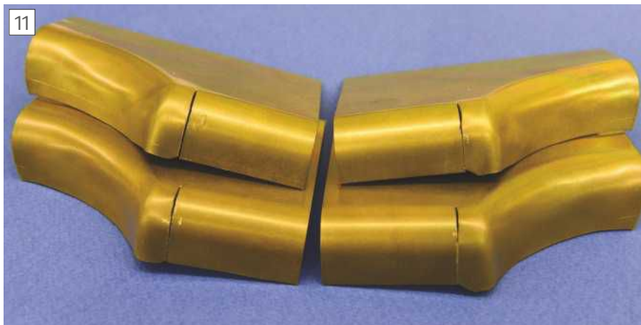
Nearly finished, but the saw cuts look too open
