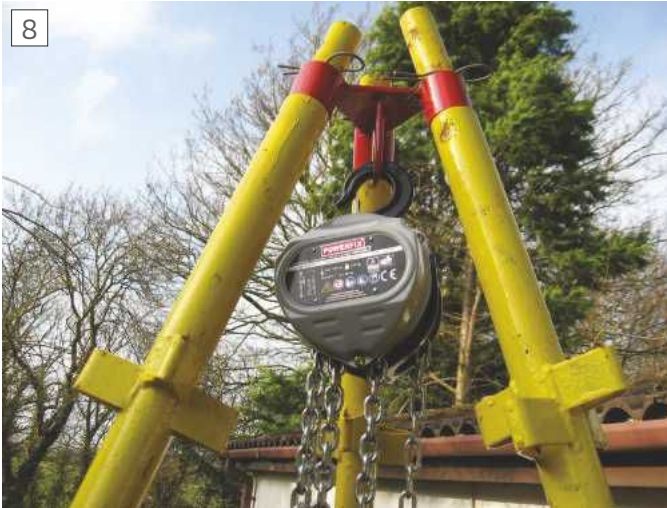
The chain hoist is hooked to the eye, supporting the chains reduces the weight you need to lift
