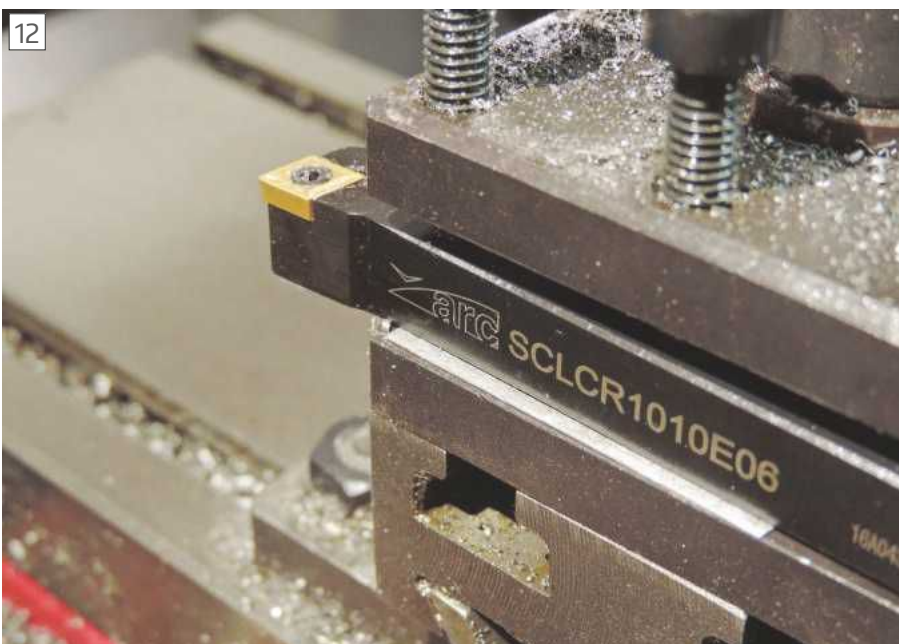
12 10mm shank tools suit the SC4-510 lathe, but as inserts can vary in thickness you may need to use packing with the standard toolpost.
