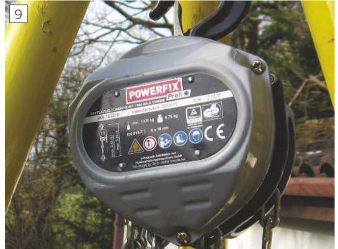
The chain hoist used was a Powerfix unit with 1000kg swl.
