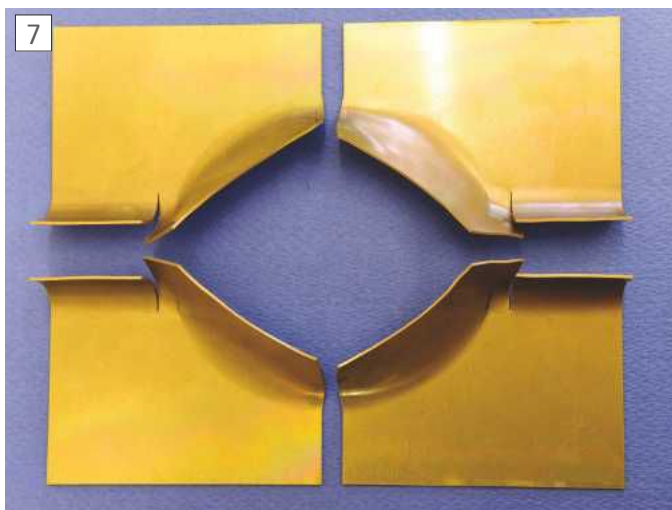
Further shaping after making two saw cuts
