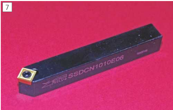
This 'neutral' tool is for chamfering and roughing.
