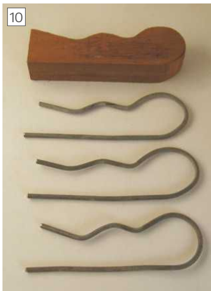
Shop-made clevis pins shaped around a wooden former
