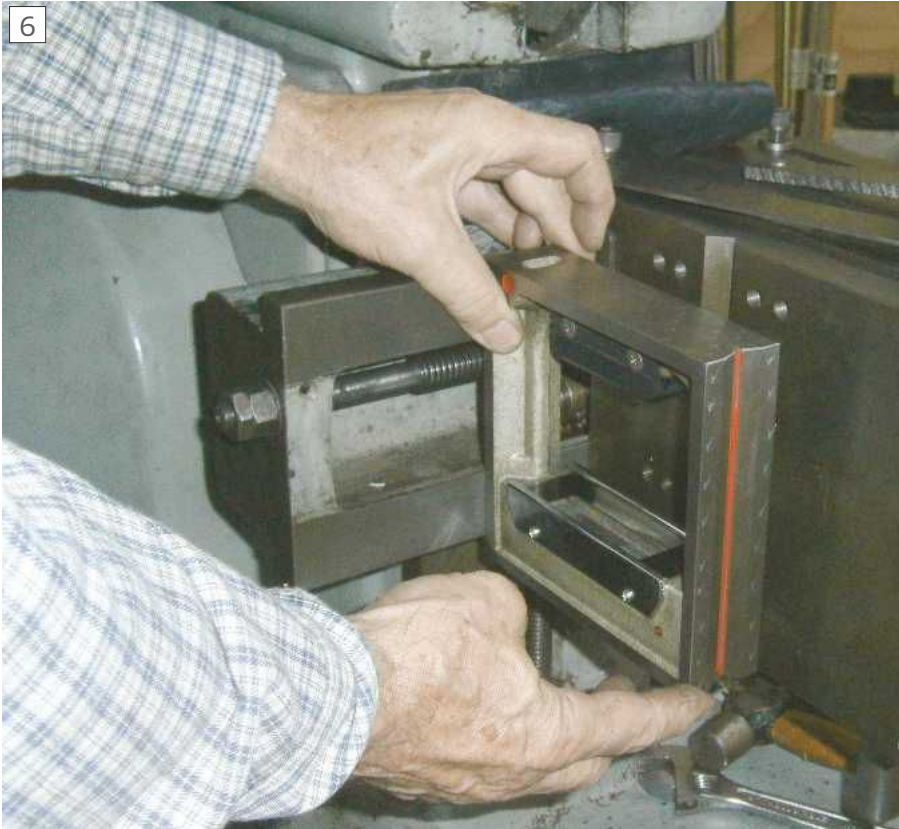
Face of cross rail vertical.
