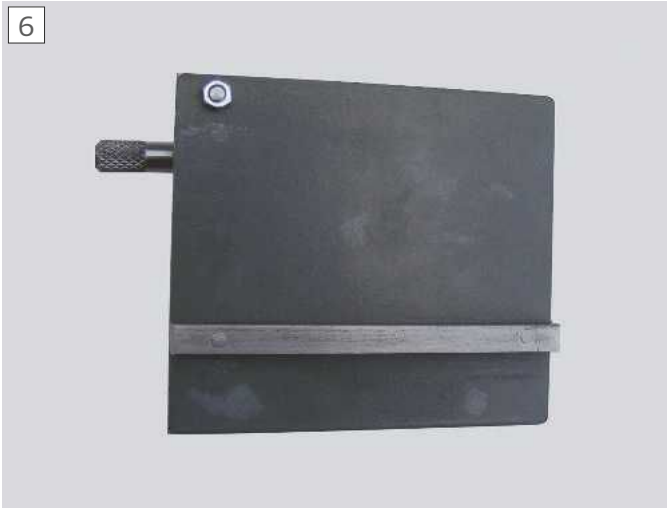
The underside of the sub table with guide bar
