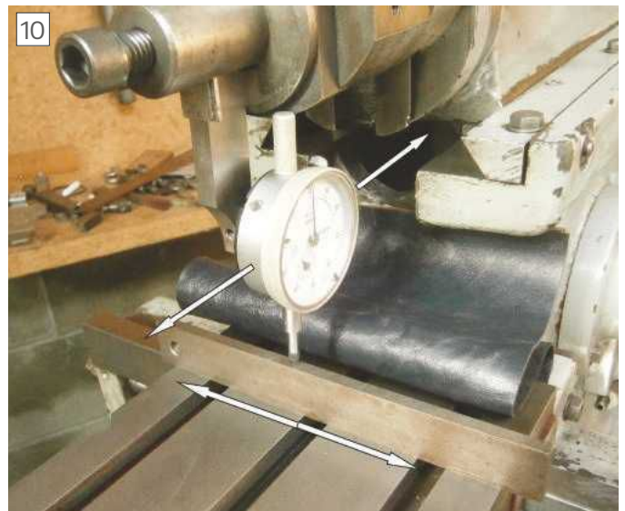
Top of table parallel with movements.
