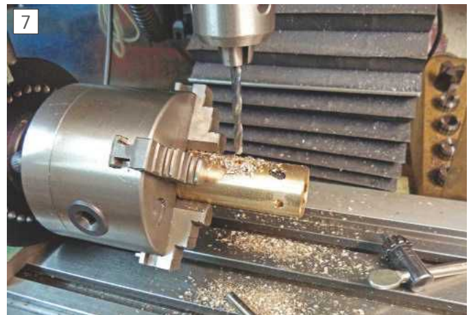
Using the spin indexer to drill holes for spigots
