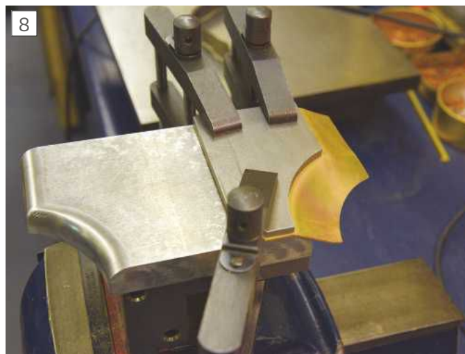
Initial work was done with the former horizontal
