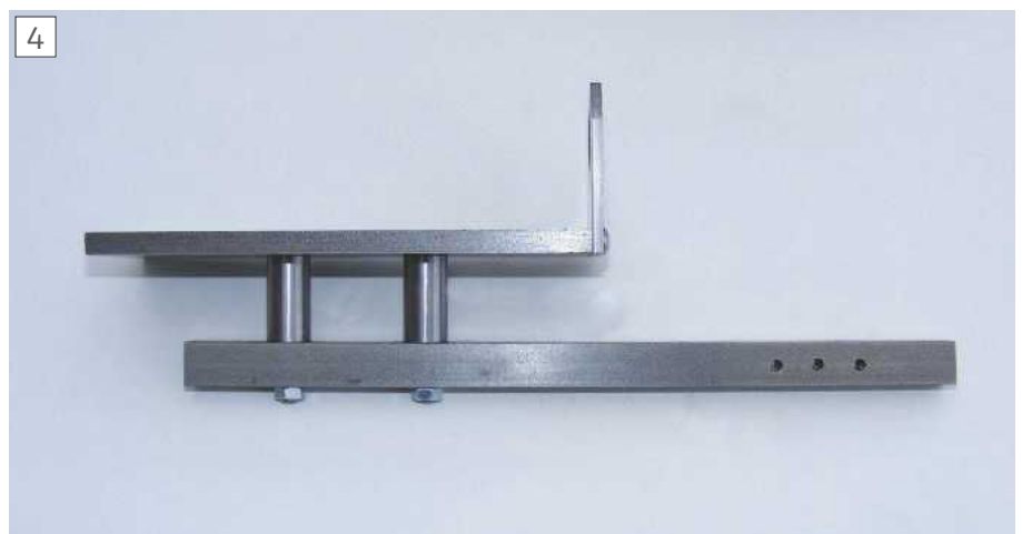
Bracket assembled to support barw
