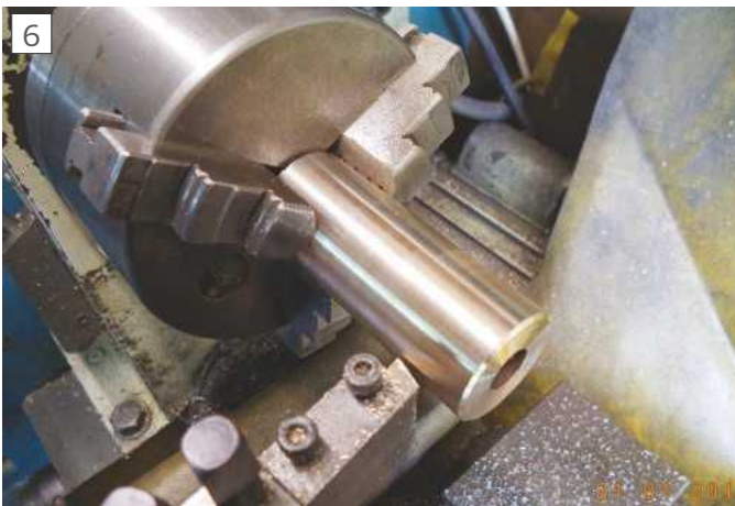
Roughing out the slide bush
