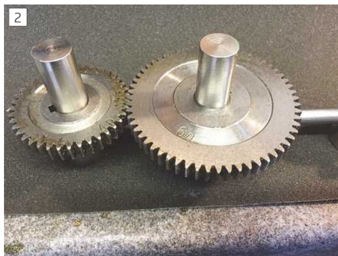
Meshing the lead screw gear and its driver
