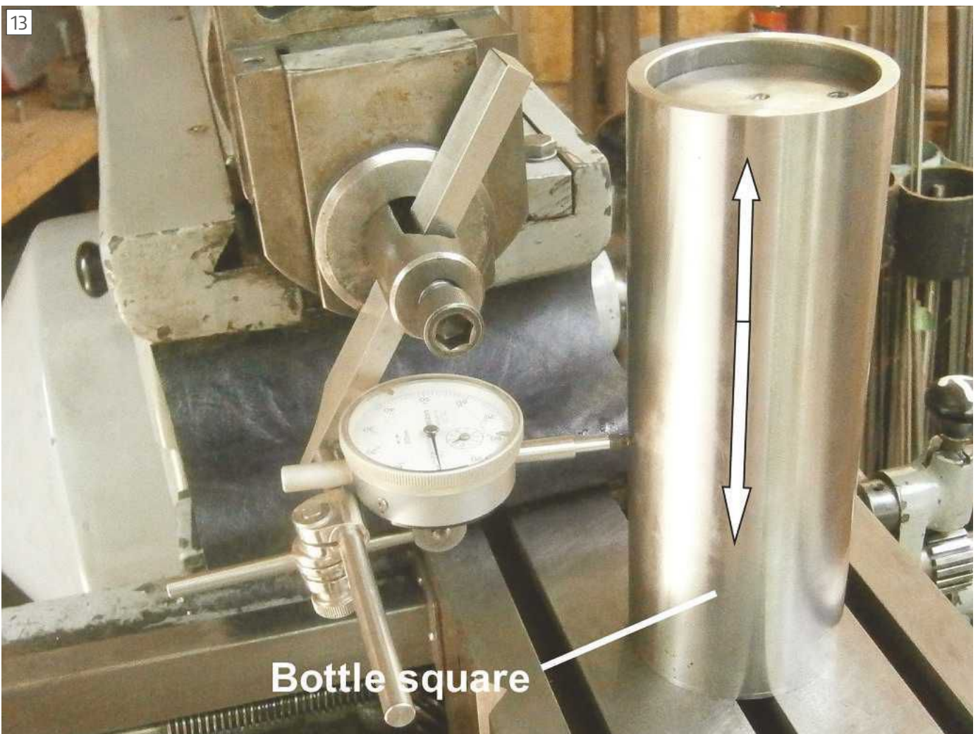
Vertical movement of table square to its top.
