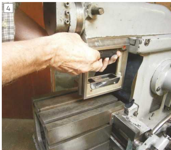
Ram guiding surface horizontal.
