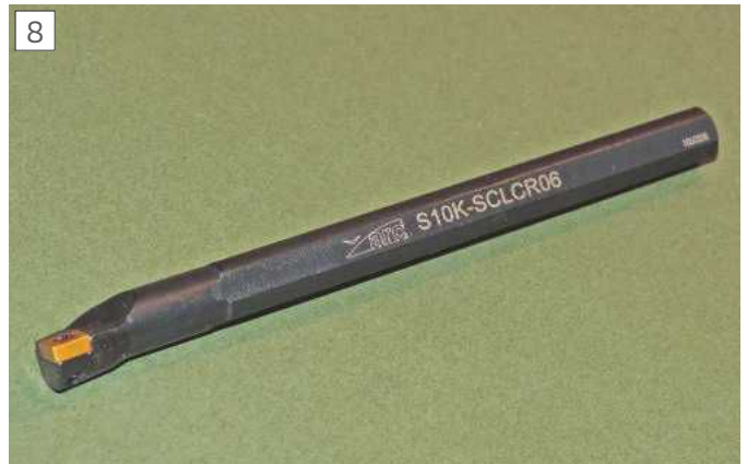
Indexable boring bars can be used in surprisingly small holes.
