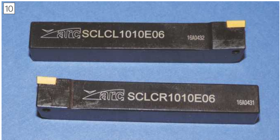
10 Helpfully, many toolholders have their codes etched or stamped on them, making it easy to order suitable inserts.
