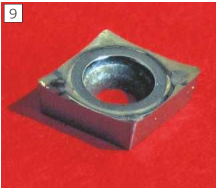
9 This sharp-edged uncoated CCGT insert is meant for non-ferrous metals, but some people report they work well on steel if used with care.
