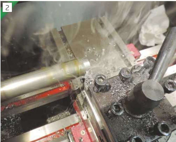
The 'chamfer' tool works well for roughing cuts, the chip breaker groove promotes short swarf rather than long ribbons.
