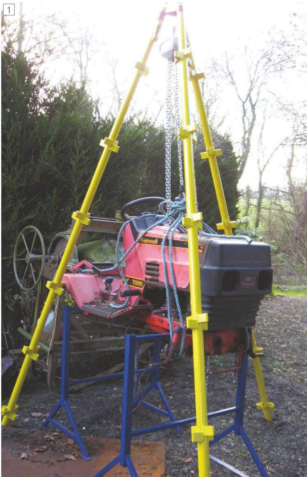
The hoist lifting the lawn tractor
