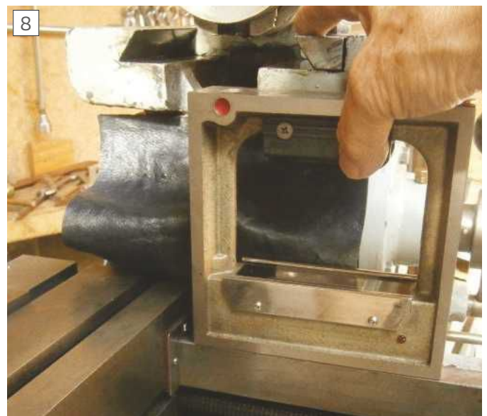
Top of cross rail horizontal.
