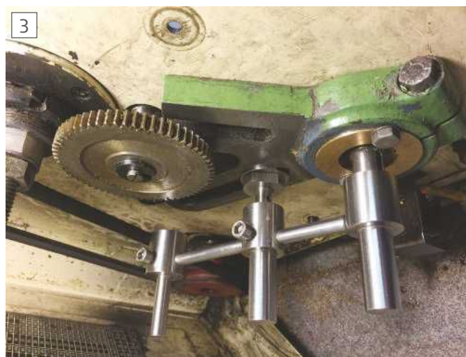
Using the jig to position the banjo correctly
