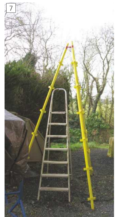
Using a stepladder makes assembly easier and safer
