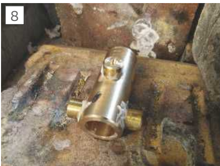
Bush fluxed for soldering
