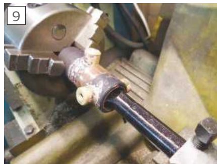
Finishing off the bore
