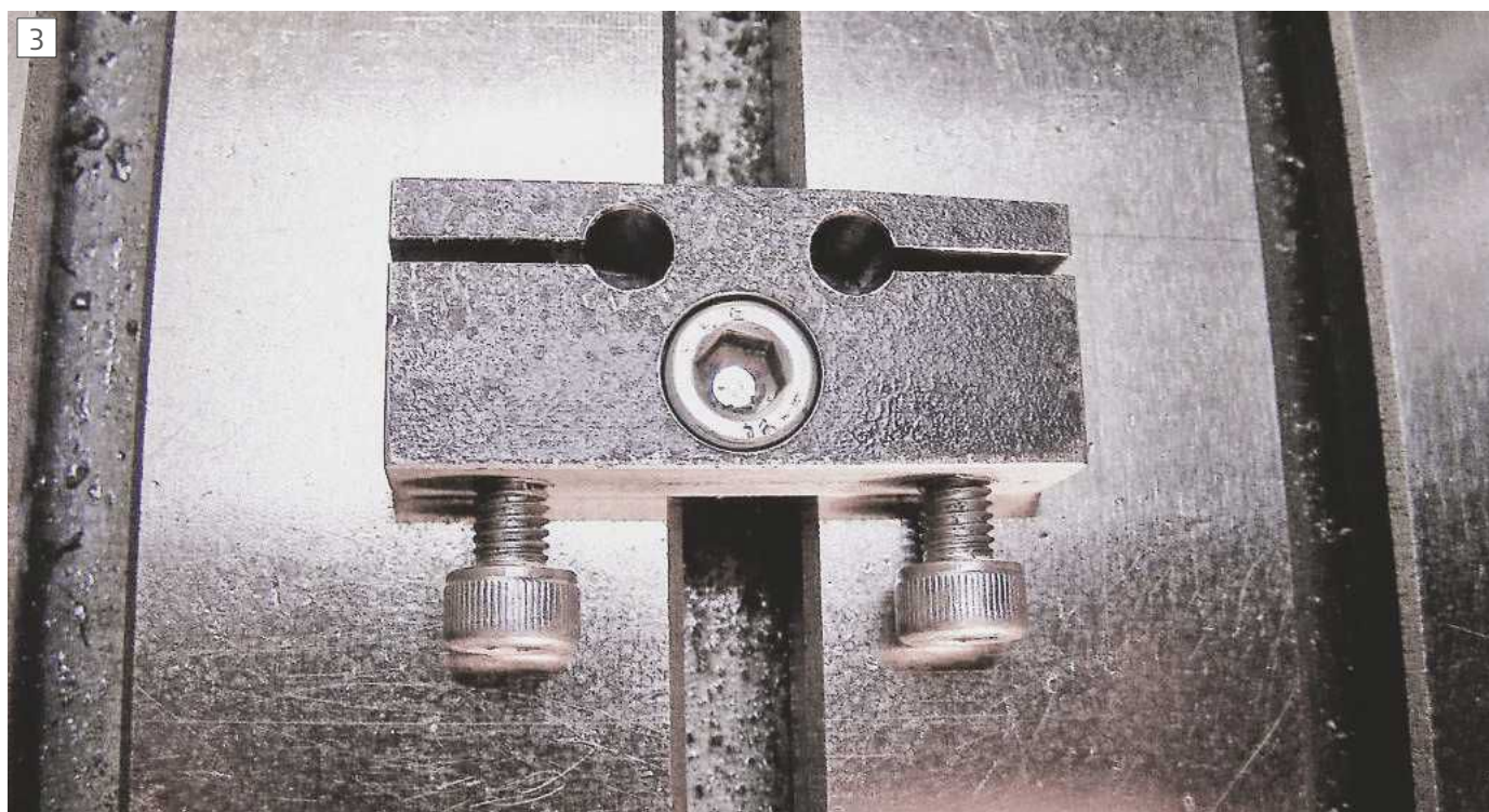
A clamp with a recessed securing screw.
