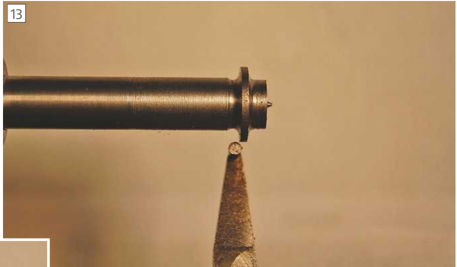
Cut for final tooth height
