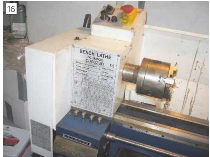
Headstock of the lathe showing gearbox ratios
