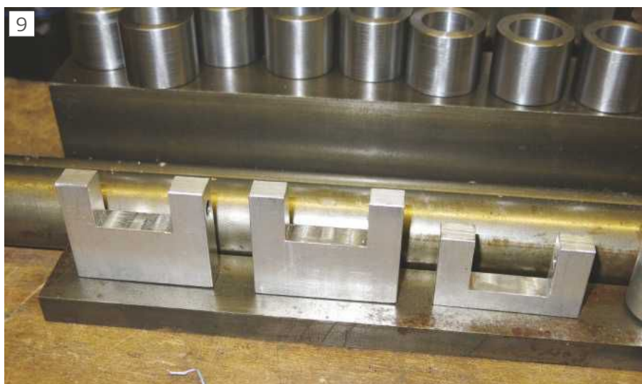
Soft jaws for four jaw chuck
