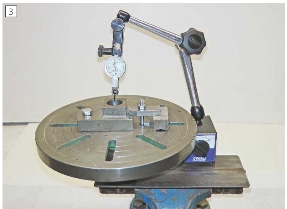
Centring an item using a dial gauge
