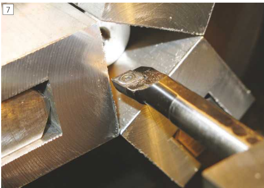
Trialling boring bar depth
