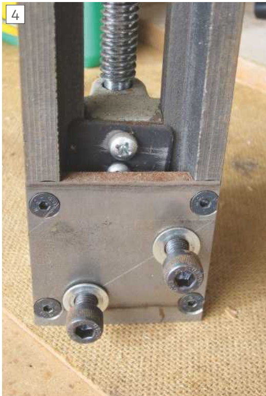
Screws fitted to sub-vice
