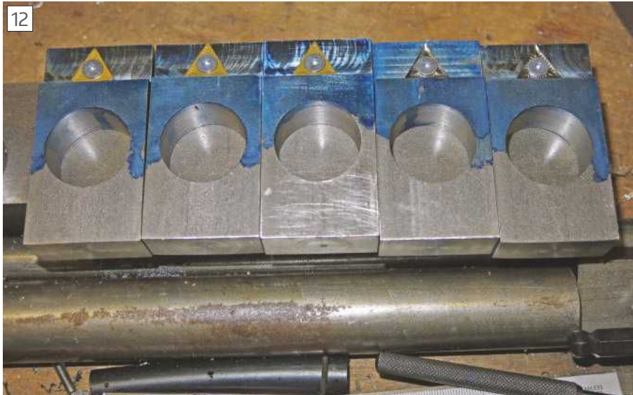
Matching blanks with inserts fitted
