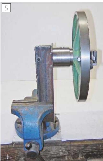
Setting up for balancing the faceplate
