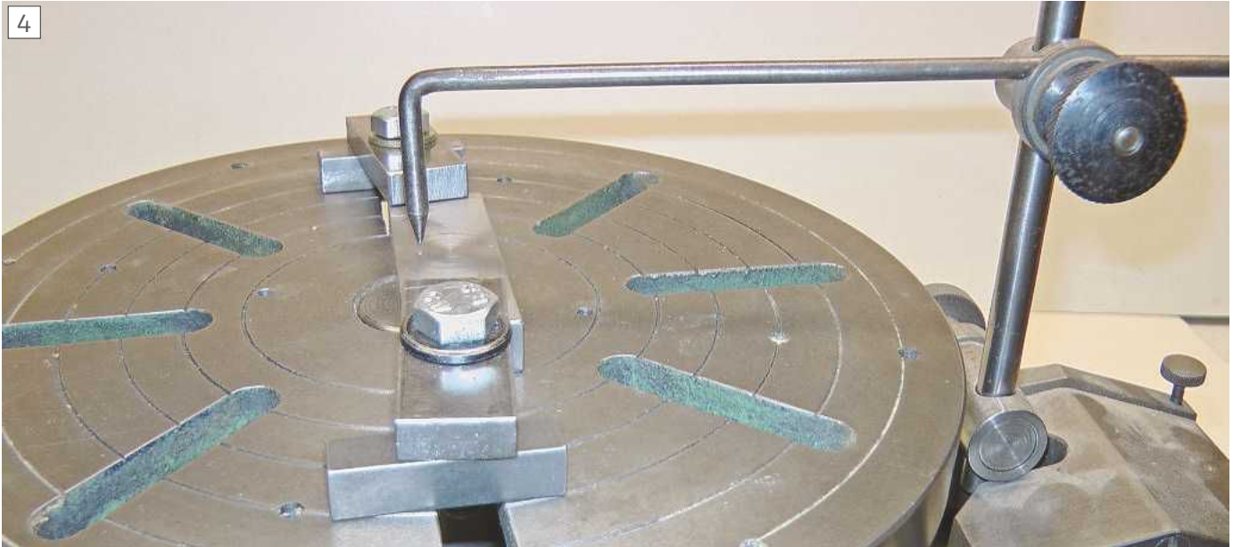
Centring to a centre pop mark with a scribing block
