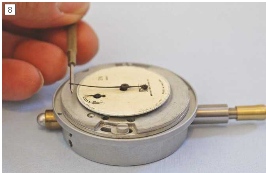
Bending up the main hand to restore its shape and prevent scuffing.
