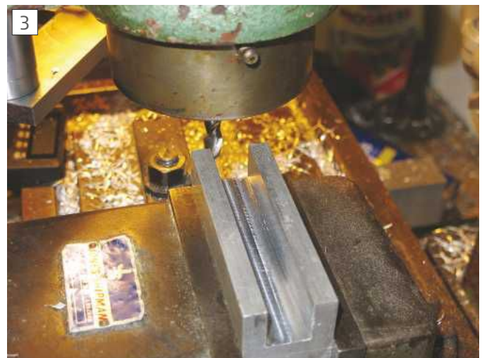
Grooving the soft jaw material
