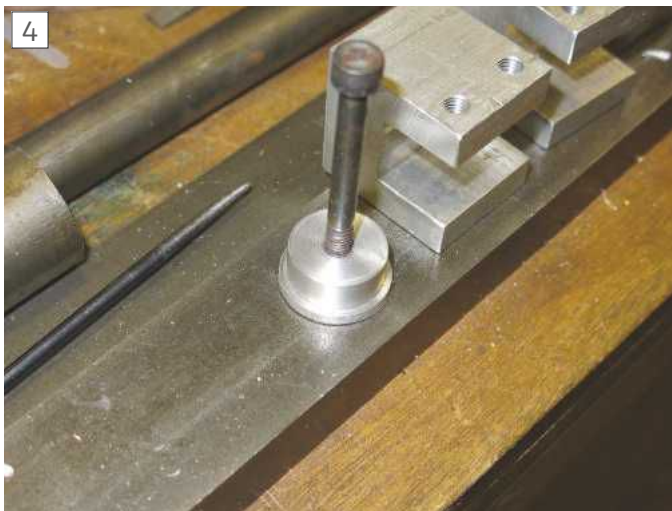
Temporary stop, to be used to set jaws
