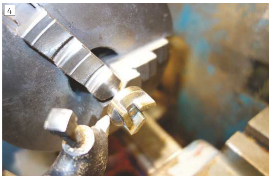
Finishing impeller to size
