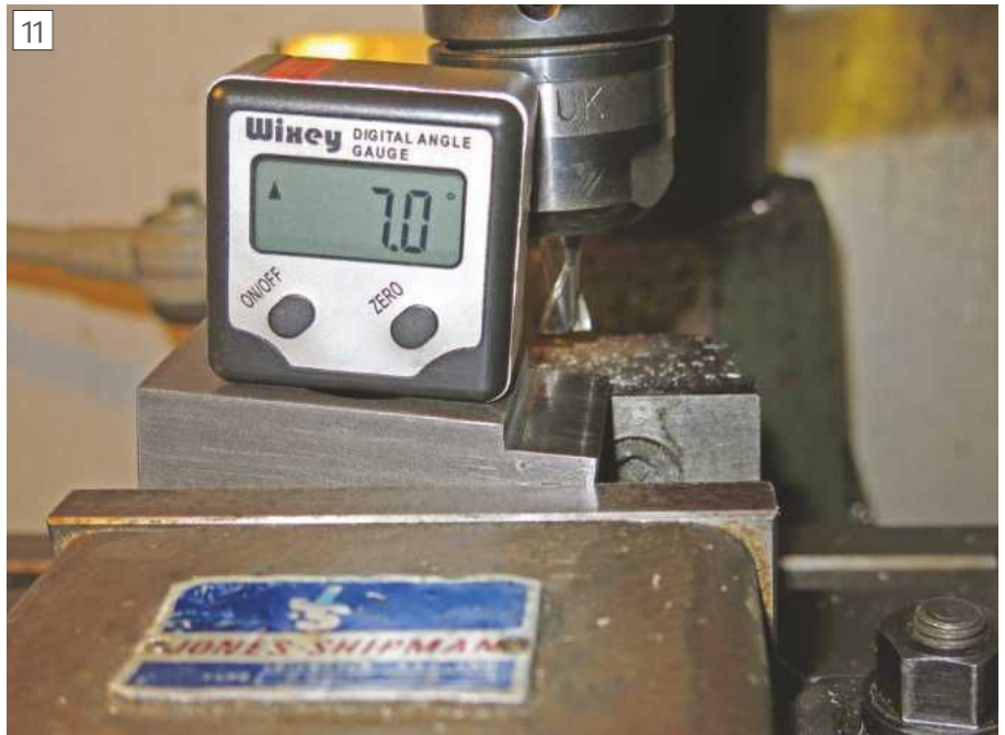
Setting angle of blank in vice
