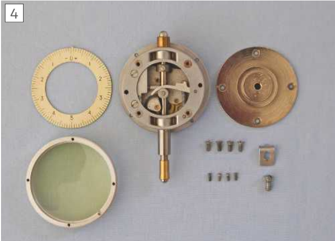
The case opened, showing the clockwork mechanism.
