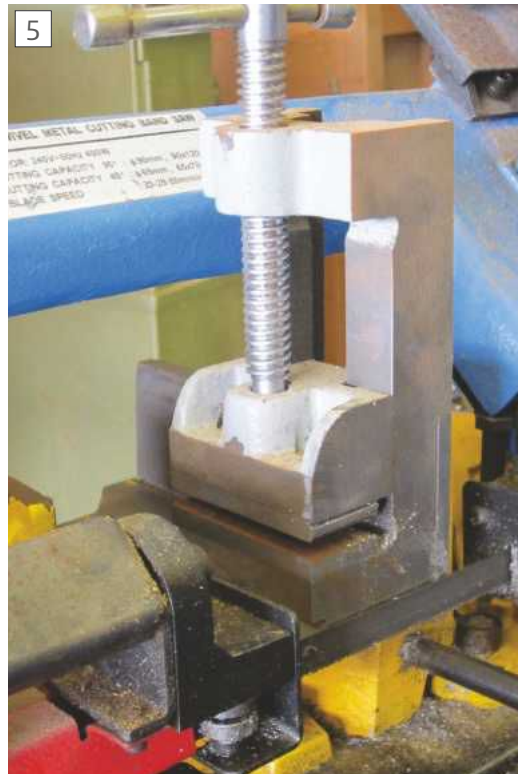
The new sub-vice mounted and ready for use
