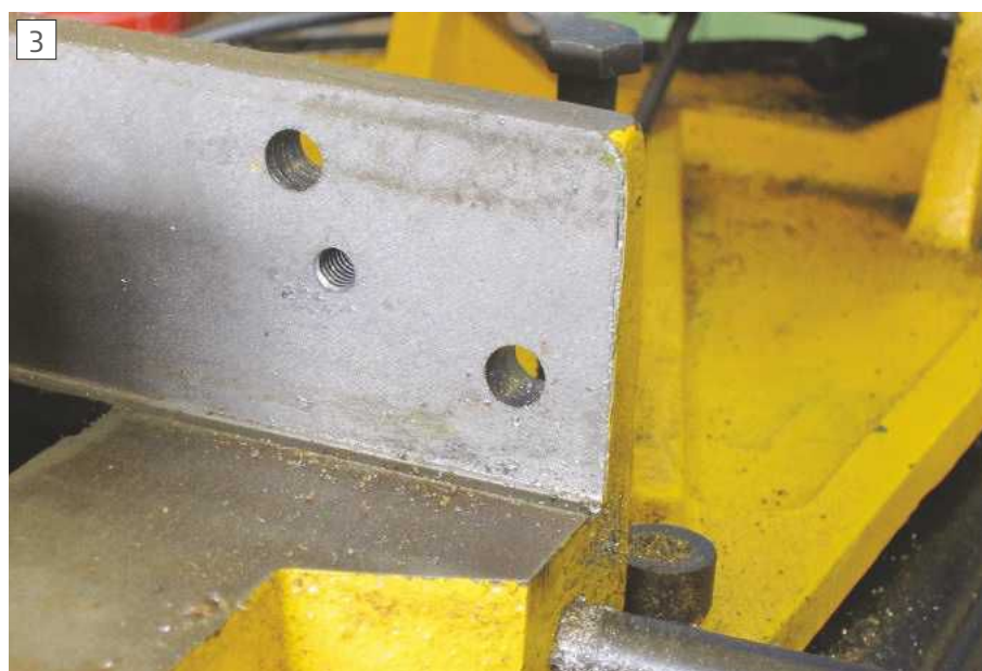
The bandsaw vice rear jaw after removal of the jaw plate and drilling for sub-vice mounting
