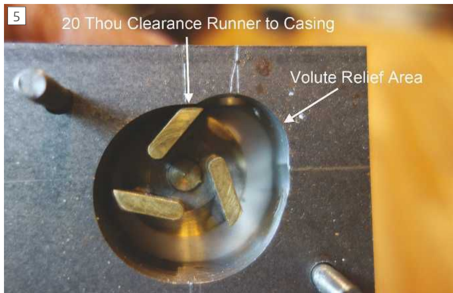
Details of the impeller in situ
