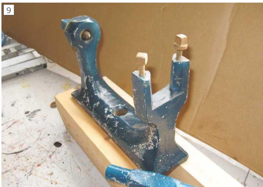
Arrangement for headstock nose bearing adjustment
