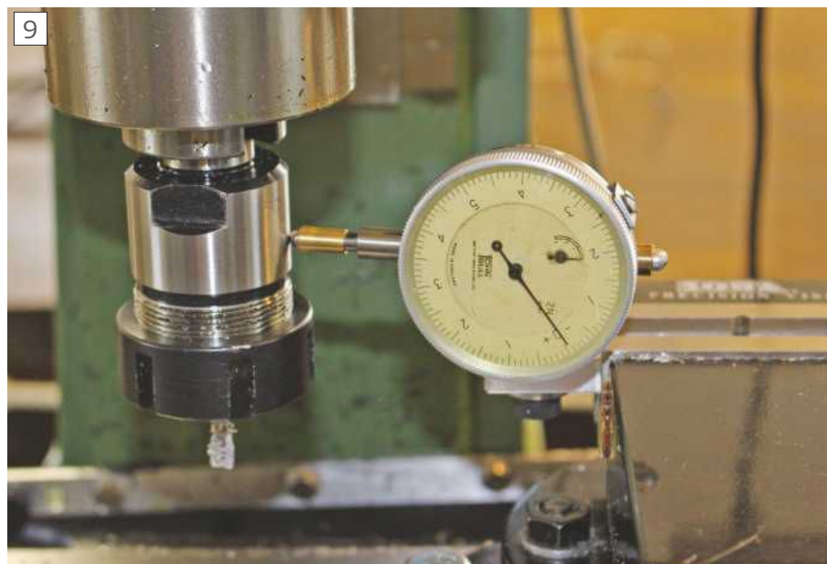
Restored John Bull DTI testing runout on a milling machine spindle.
