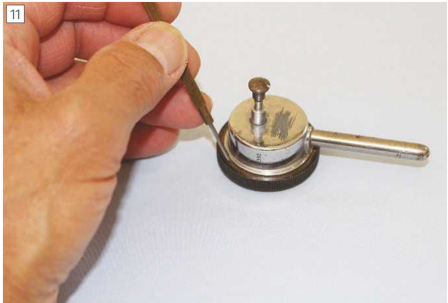
Levering out the circlip on the Baty DTI to release the front bezel.
