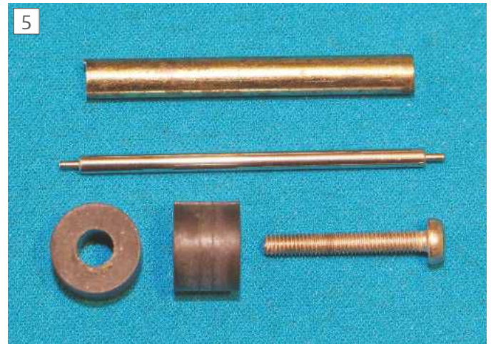
Parts that make up the home-made hand puller.
