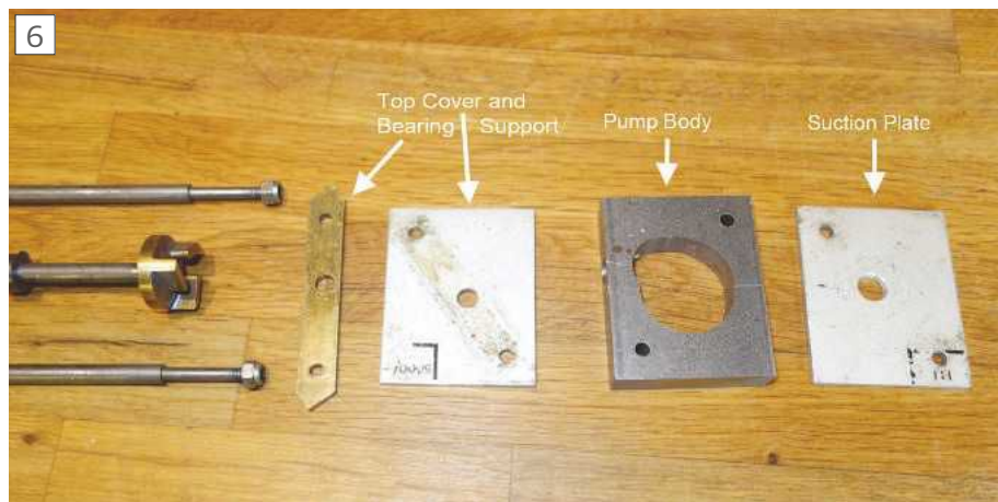
Top cover, pump casing and bottom cover parts
