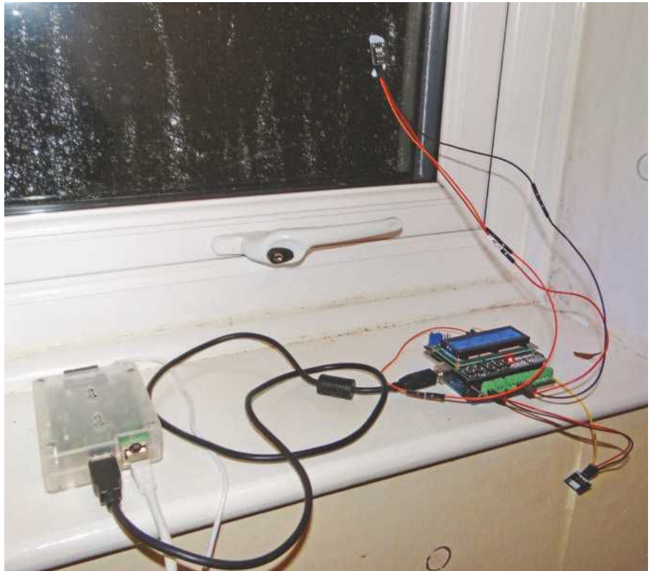
RaspberryPi Data Logging the Arduino in a Damp Hallway
