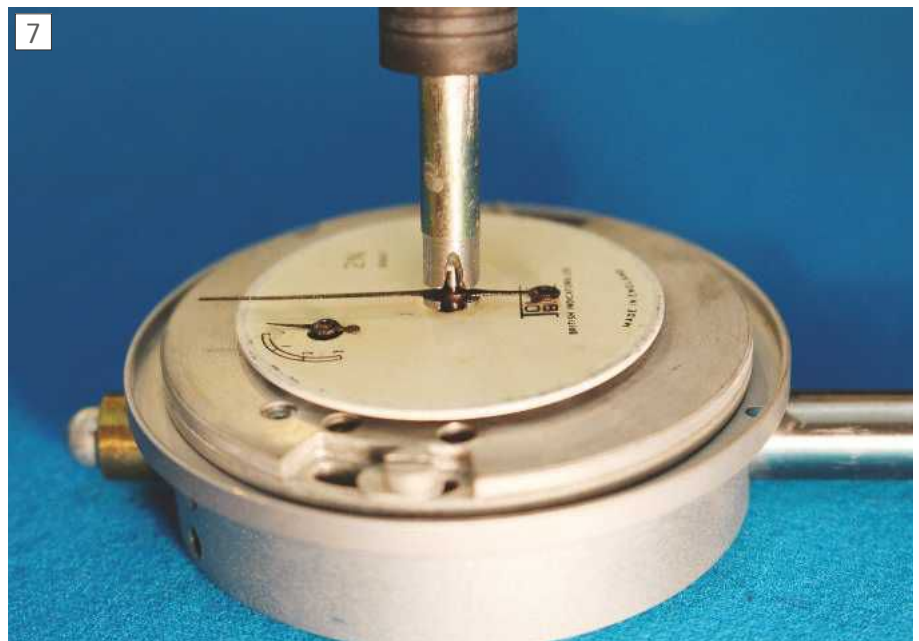
Removing the DTI main pointer with the hand puller.
