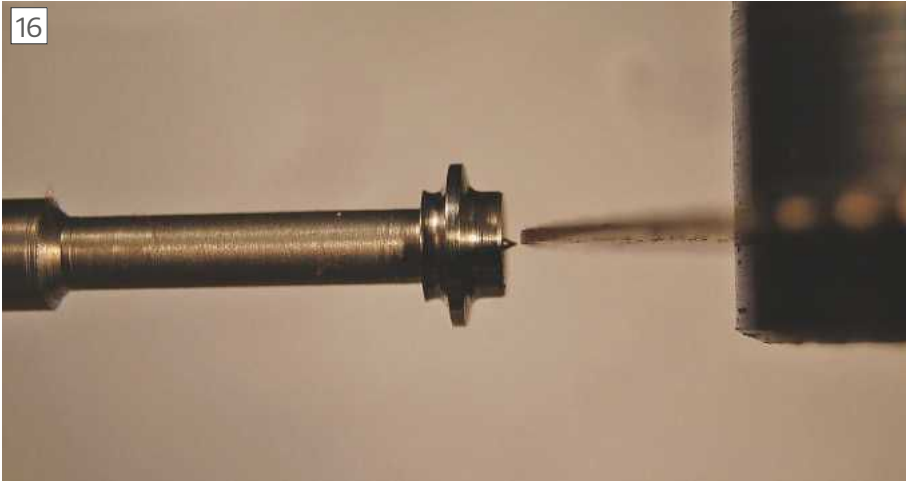
Saw blade on centre height
