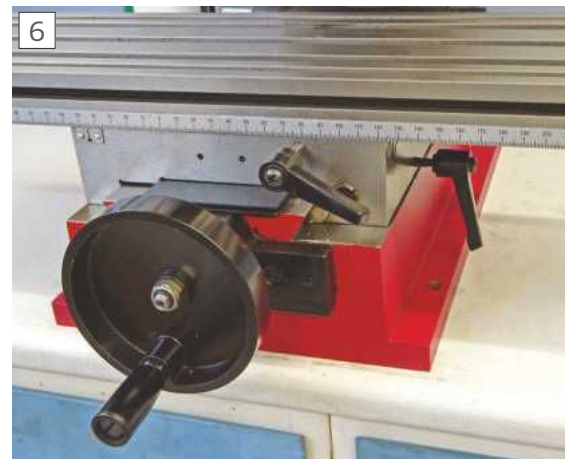
Y-axis hand wheel and locking levers
