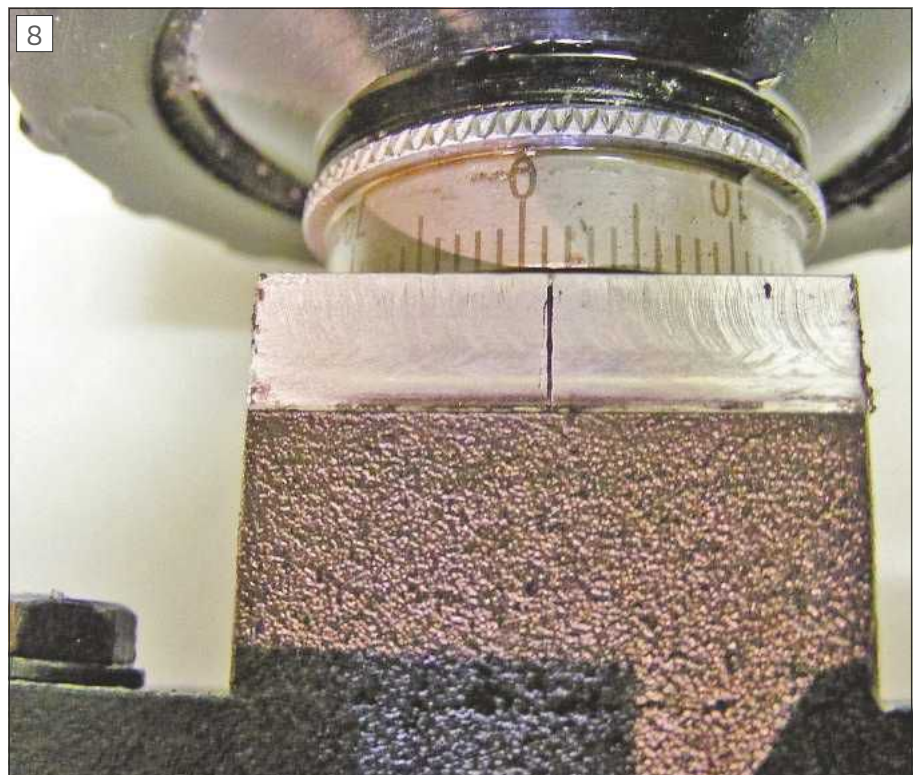
The milled strip with the fiducial line.
