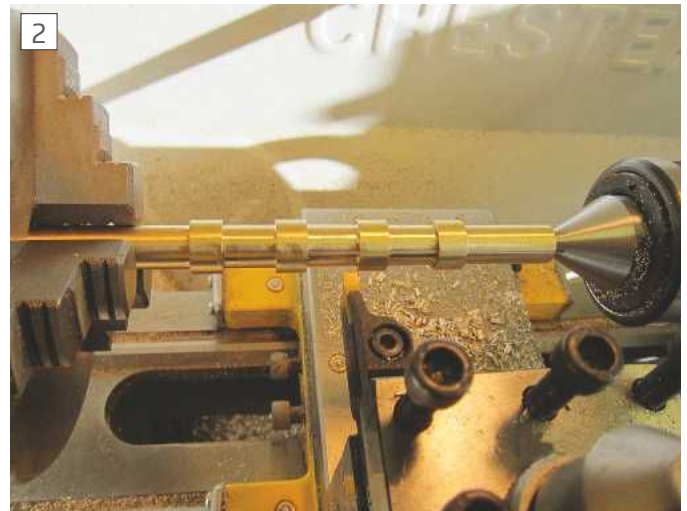
2 Turning a 20t blank in the lathe using a parting/grooving tool.
