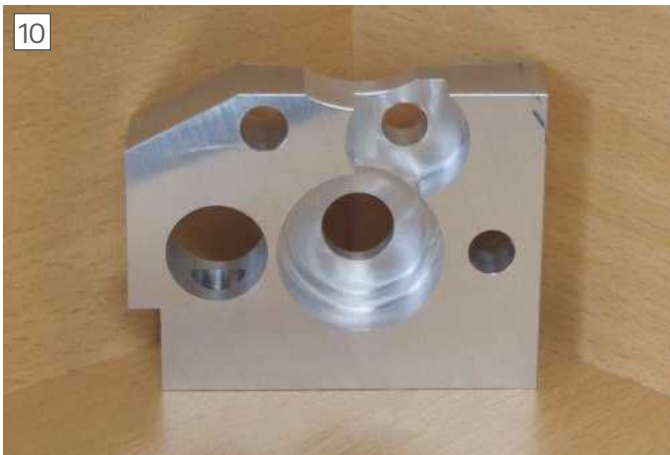
Front view of ML 7 Screwcutting clutch body
