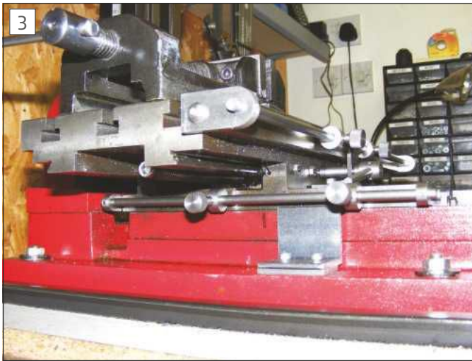
Left side view showing the y axis stops.
