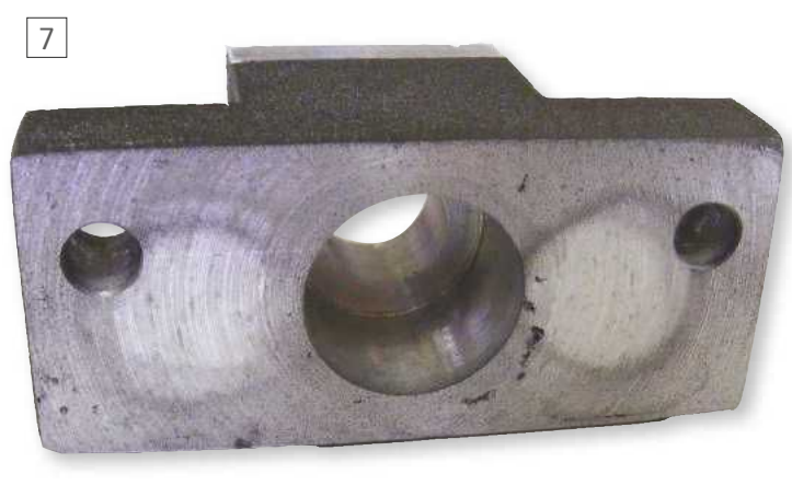
The flange bearing recess.
