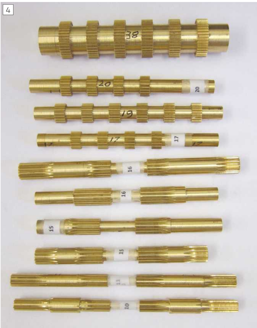
4 A selection of blanks after the teeth had been cut.
