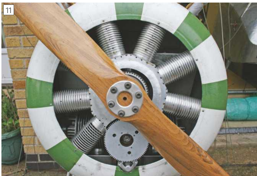
Dummy engine fitted over the JPX and prop.
