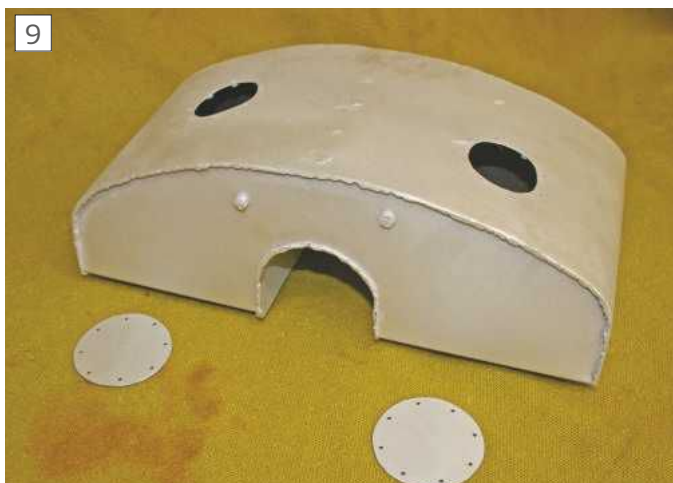
Top of the completed silencer
