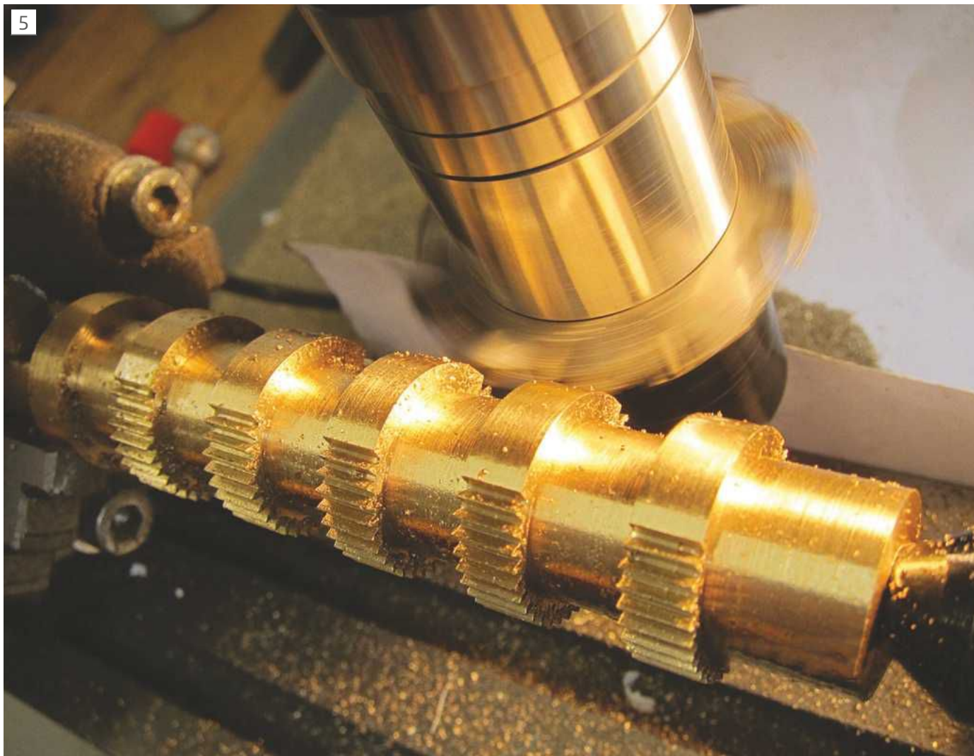
Cutting 5 gears on a 45t blank, the sixth was cut after reversing the blank.
