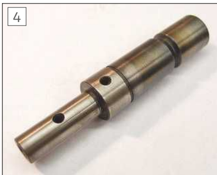
S7 Screwcutting Clutch shaft, note angled undercut, courtesy of Phil Proctor
