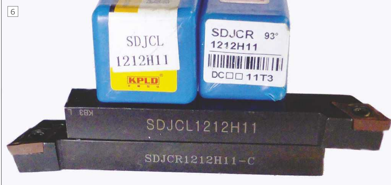
SDJ lathe tool holders, left and right.
