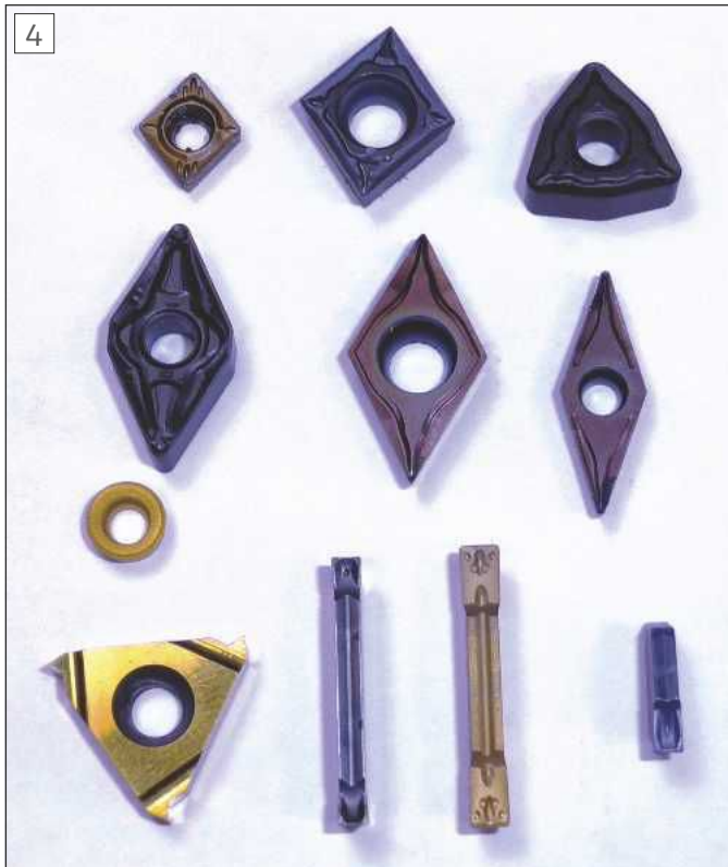
Carbide lathe tool inserts I currently use.
