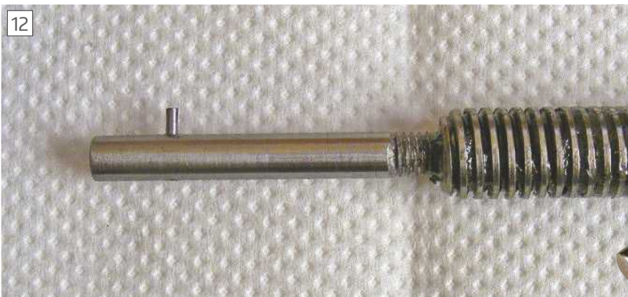
The end of the feed-screw showing the extension.
