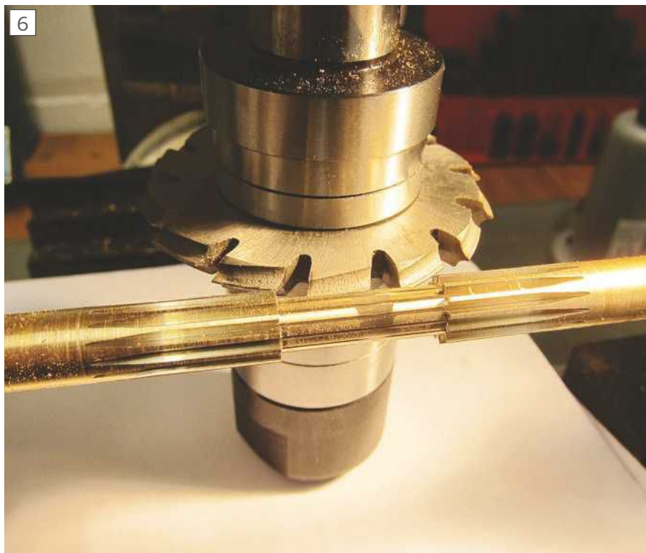
Cutting the teeth on a 15t blank from the centre outwards in both directions.
