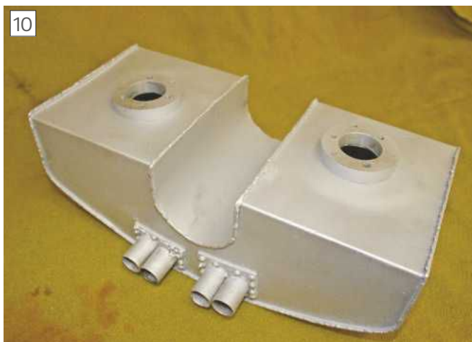
Underside of the silencer.
