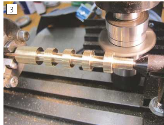
3 Cutting the teeth on a 26t blank
