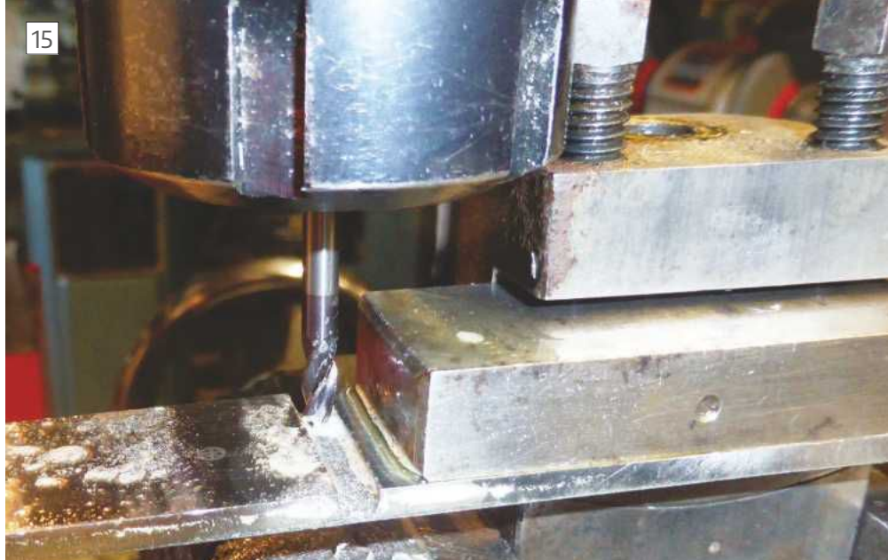
Milling hardened High Speed Steel.
