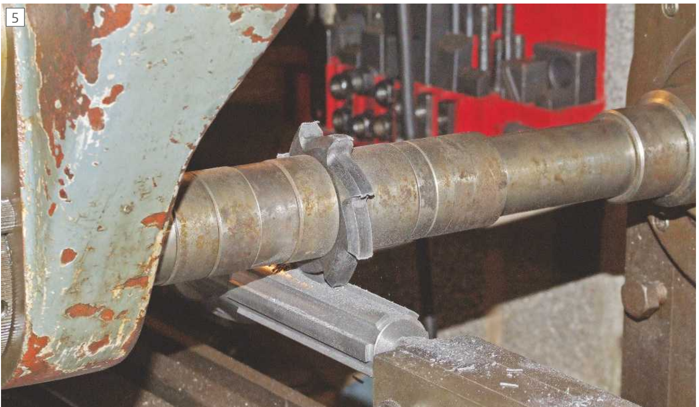
Cutting the External Splines
