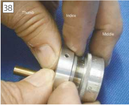
Inserting thimble frictions spring
