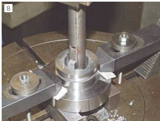
Cutting the Internal Splines
