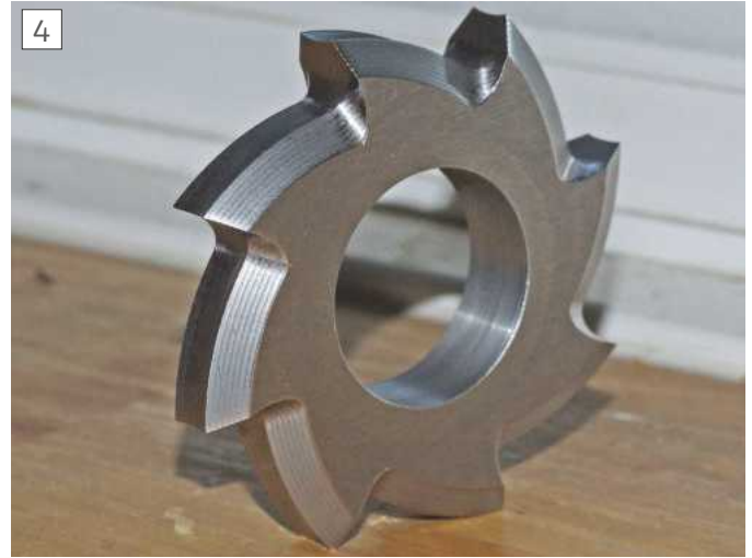
Finished Spline Cutter
