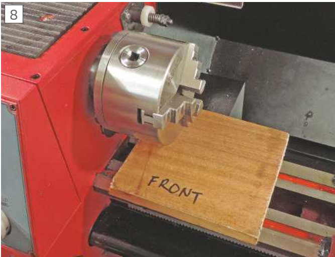
A simple protector for the bed.
