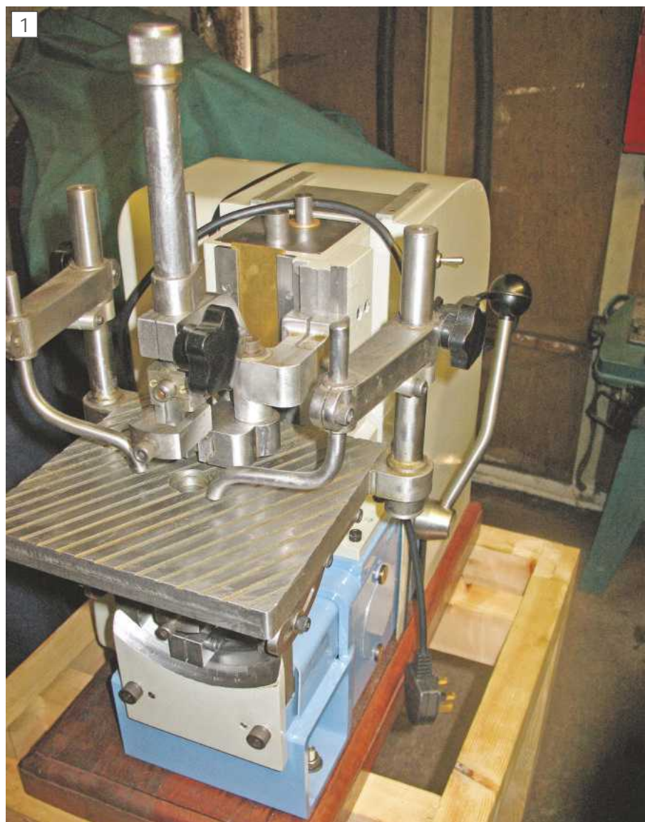
Assembled machine from right hand side, large lever to rear tensions drive belt.
