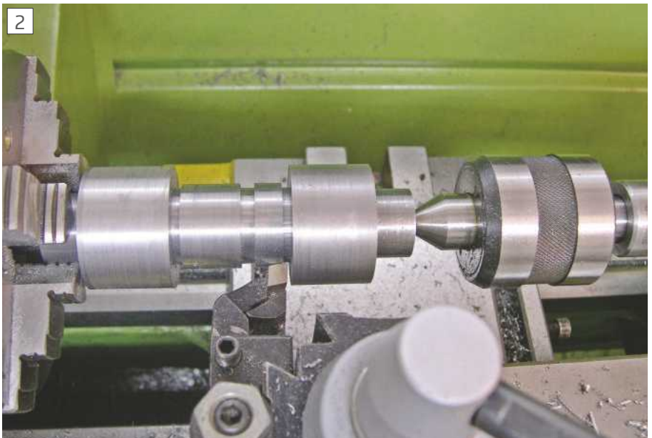
Outer diameter reduced to 43mm, inner to 30mm
