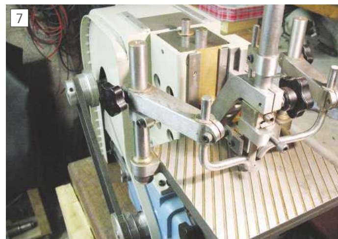
General view showing the two drive rods protruding from the top of the tower, also visible is the two piece brass swarf shield that slides up and down with the arms
