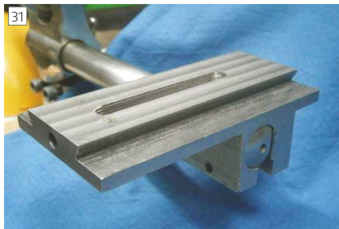
Finished saddle on bed
