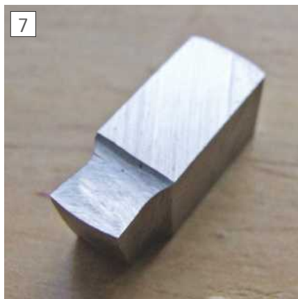
Finished Internal Spline Cutter
