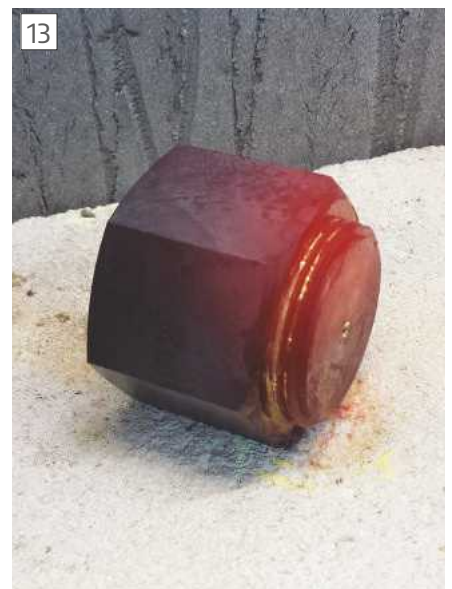
Heat source removed post silver soldering
