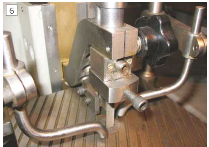
Work table and top arm, just visible are some of the weight reducing holes.
