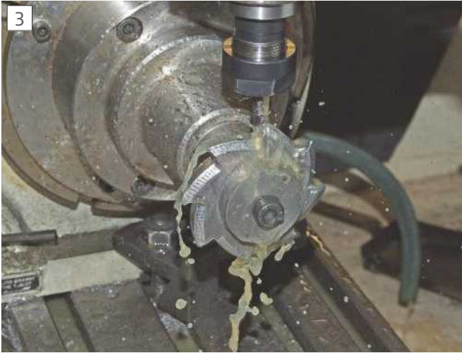
Spline Cutter – Finishing Cut
