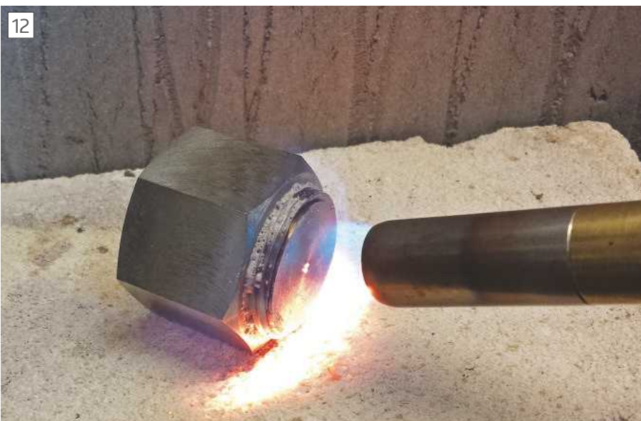
Assembly being heated on fire brick
