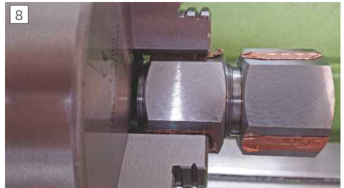
Mating check to prove internal thread
