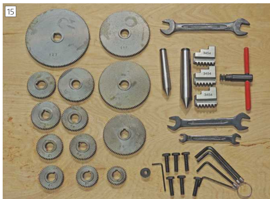
The accessories supplied with the lathe. Another four change gears are fitted in the gearbox, and there is the three-jaw chuck.
