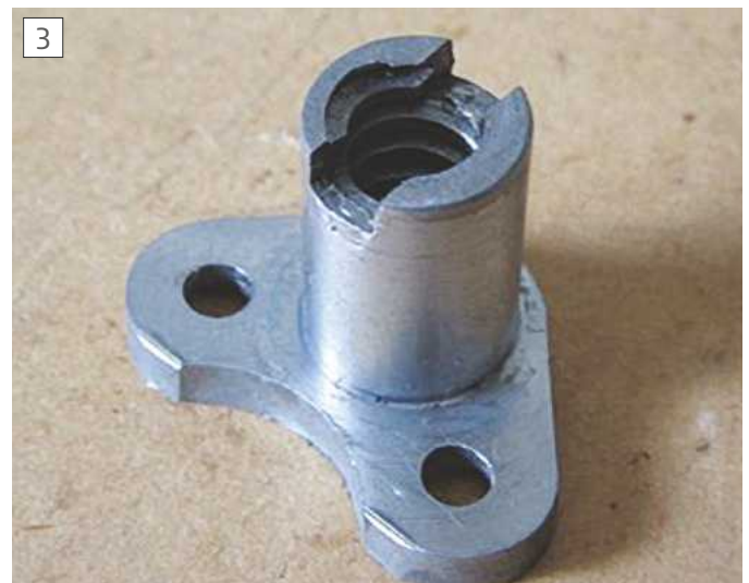
Slot in feed nut
