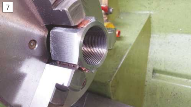
Part C threaded internally
