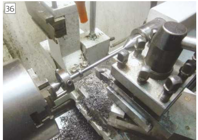
Turning leadscrew blank
