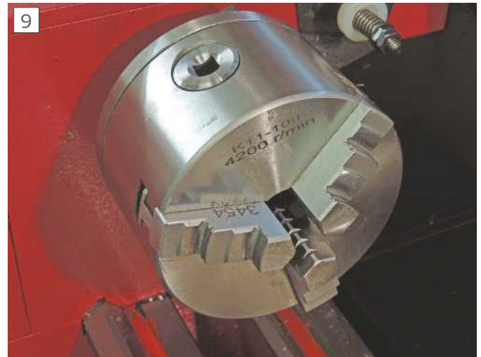
The three-jaw chuck, 4,200 is the maximum safe speed.
