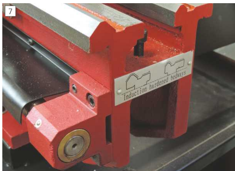
The prismatic bed of the Arc SC4-510
