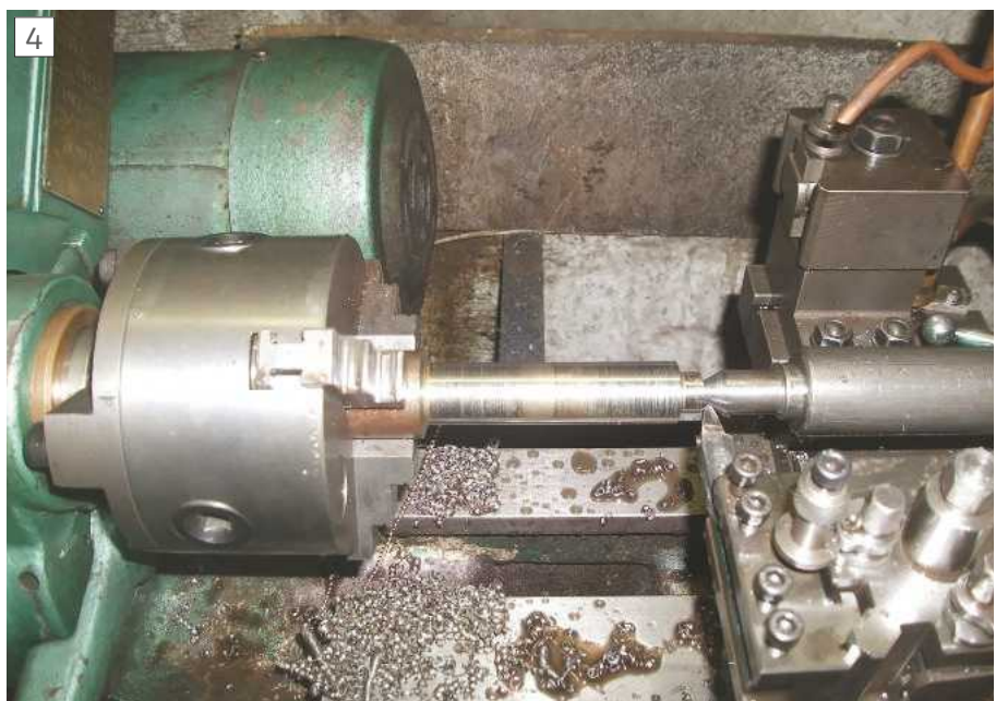
Roughed out arbor ready for the final taper machining.
