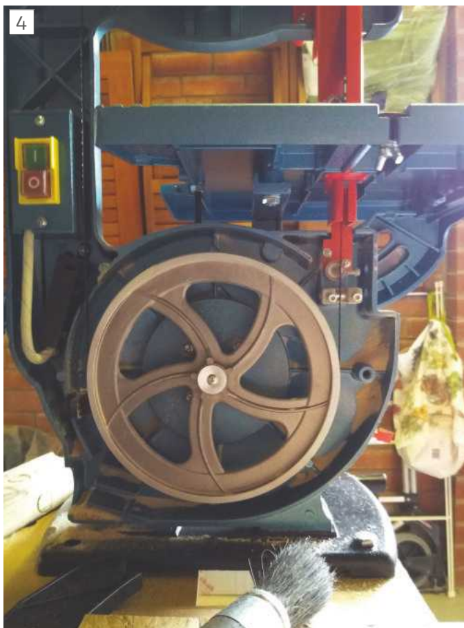
Fitting the coarser toothed blade.
