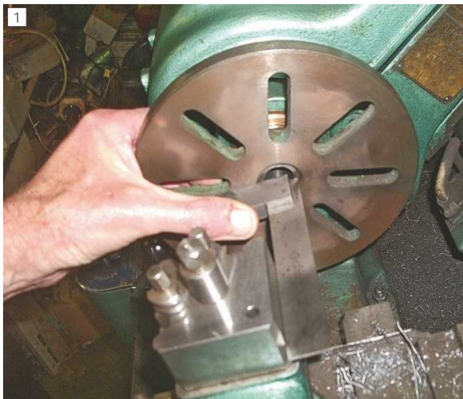
Setting the tool-post body square to the lathe spindle
