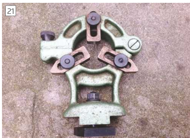
21 The standard Myford steady has no fine adjustment.
