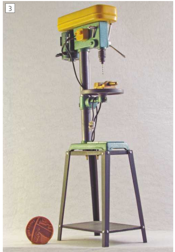
Note the 0.3mm drill bit, made from a piece of fine wire, flattened and then twisted.
