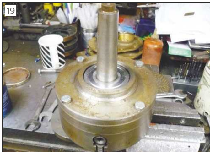
19 Rotating chuck mounted on MT arbor.
