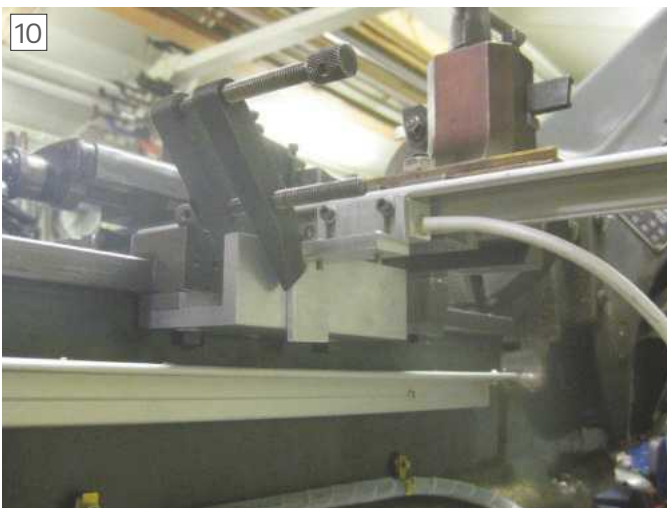
Aligning scale with cross-slide.
