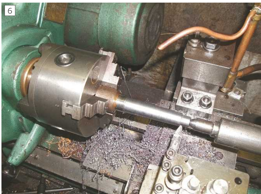
Finished taper before polishing
