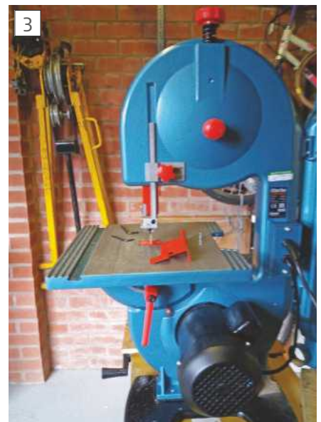
You can see the table clamping arrangement in this image.
