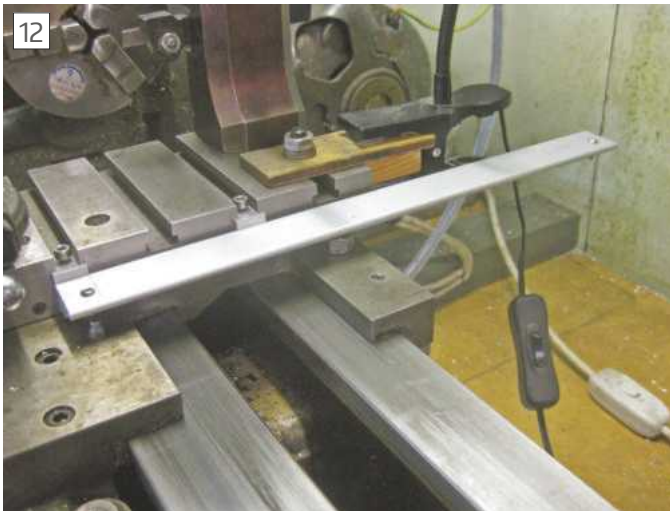
Scale secured using aluminium blocks in t-slots.
