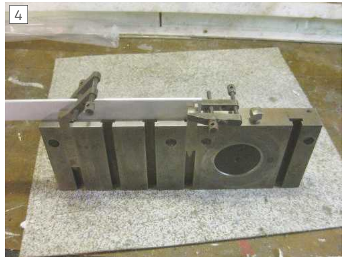
Clamping the scale for drilling.
