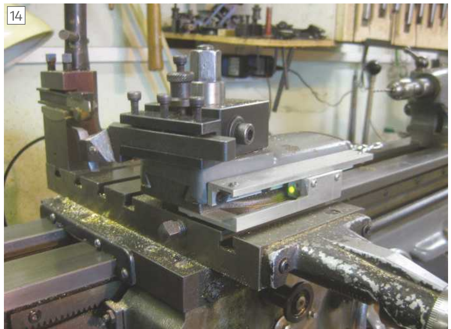
Top slide scale fitted.
