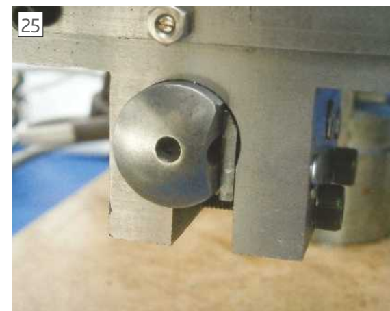
Saddle fitted to bed
