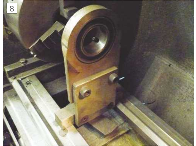
Reverse of the cathead steady, note the large diameter ball race.
