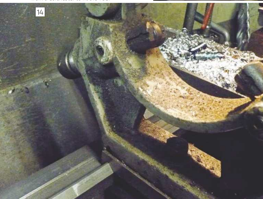
Close up showing how it was converted from a Colchester to fit the TOS.
