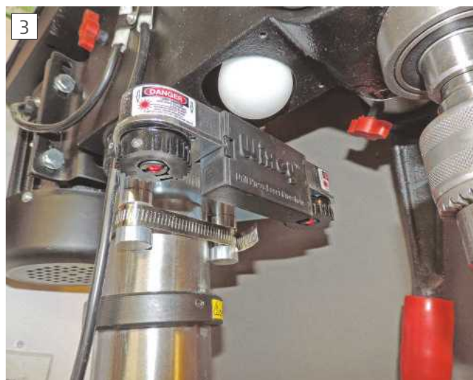
Laser unit fitted to pillar.
