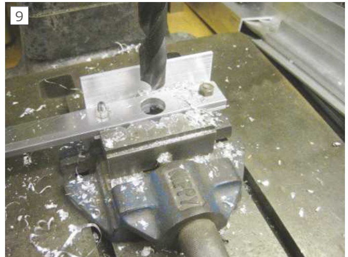
Using saddle keep as a drilling jig.
