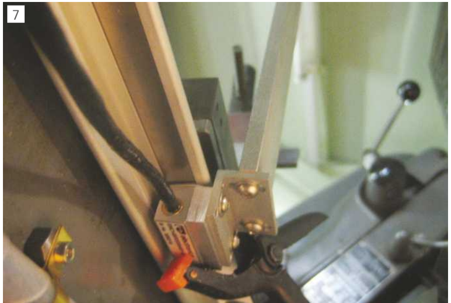
Encoder offered up to the scale.
