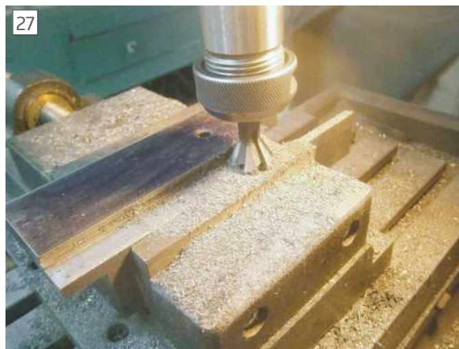
Finishing saddle dovetail
