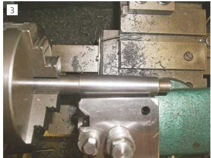
Top-slide swung so the tool-post body touches the taper all along its length
