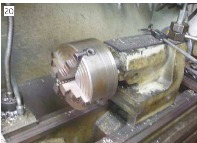
20 The rotating chuck in lathe tailstock.
