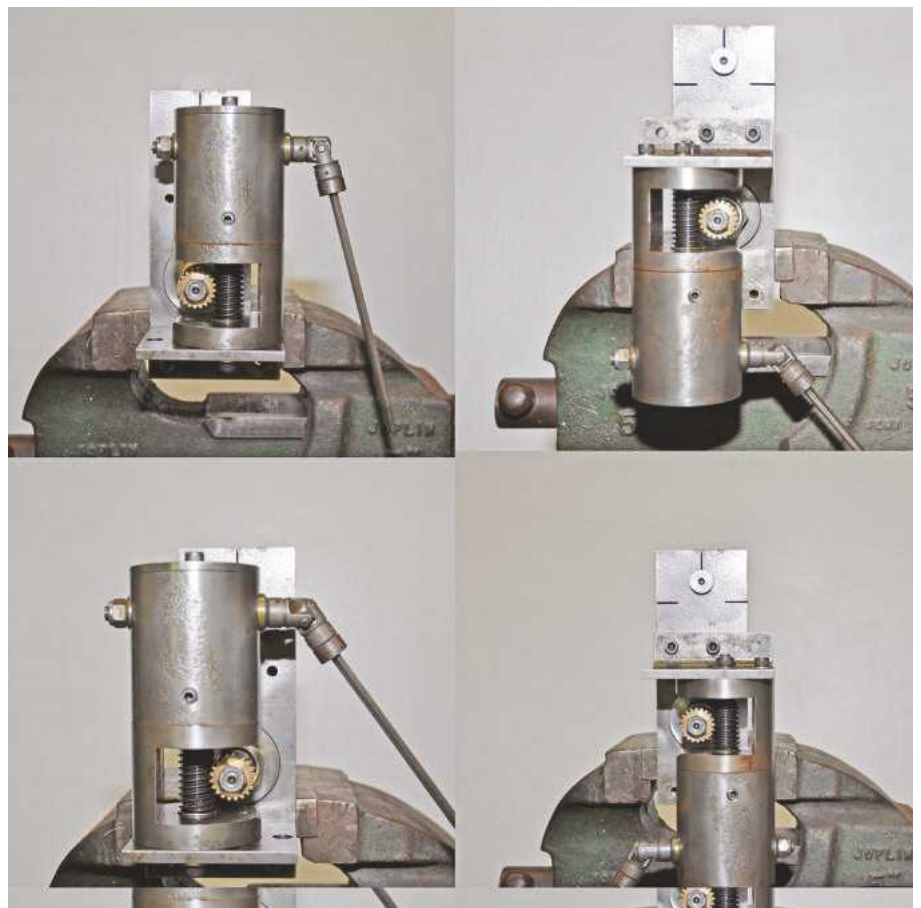
Mounting options for the Swivelling Mitre-Gear Worm-Drive.
