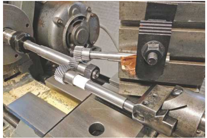
Two 25tooth, 32DP, 25deg LH & RH helical gears, and one 22tooth, 32DP spur gear all in mesh.
