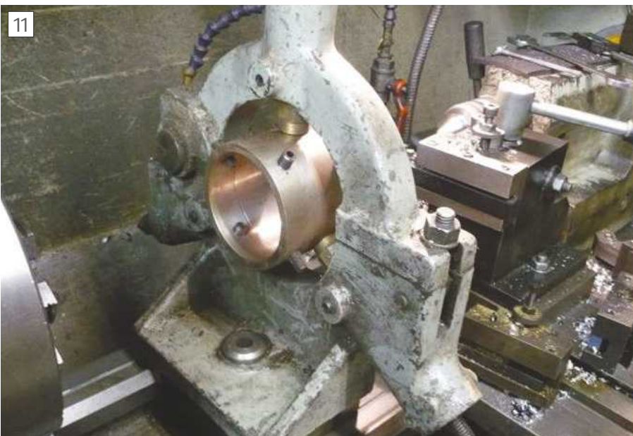
Use of the loose cathead with a normal steady.
