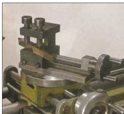
Terr Gorin fits a Top Slide to a Unimat SL.
