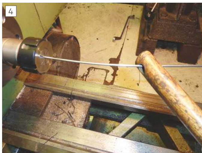
Tube straightening. The rotating tube is firmly stroked from left to right while maintaining a marked curve just within its elastic limit.
