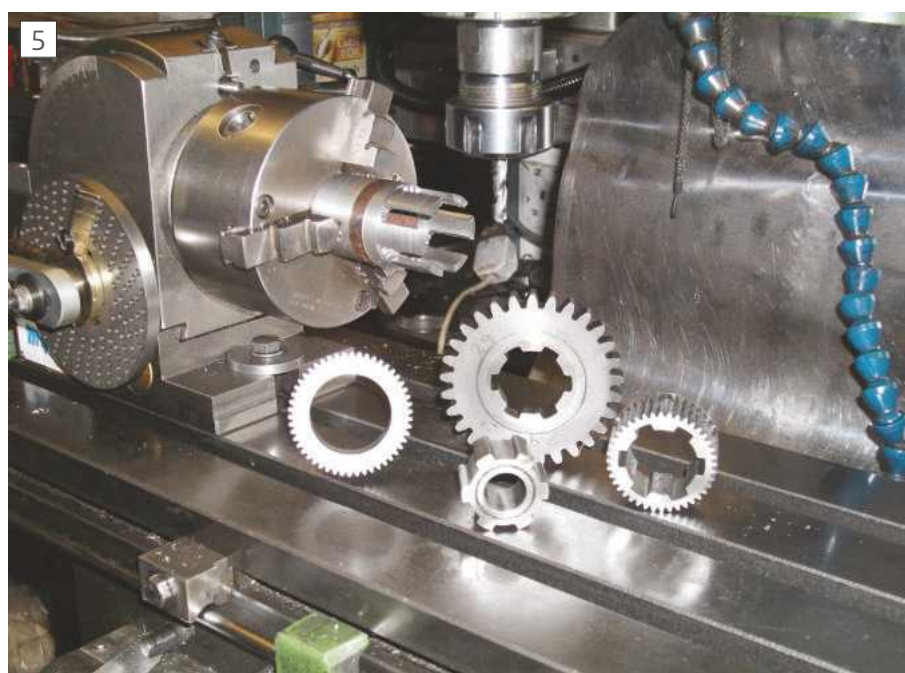
Machining the inner spline hub.
