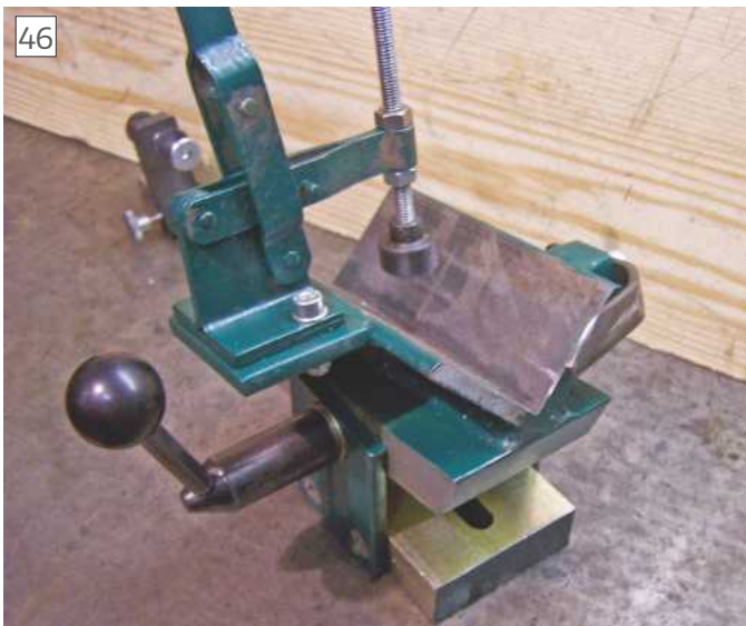
The painted and blackened jig showing new 8mm slot
