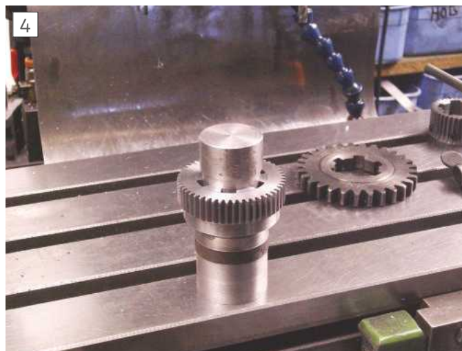
The 50 tooth gear with the splines loctited in.
