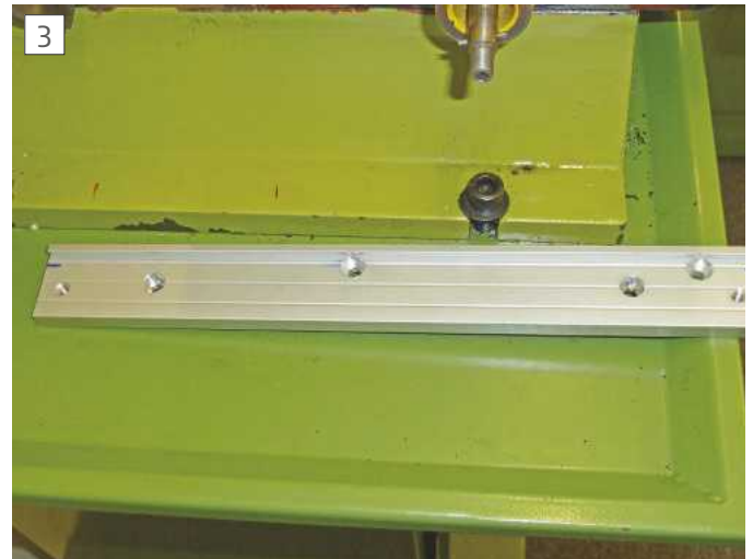
Drilling mounting plate
