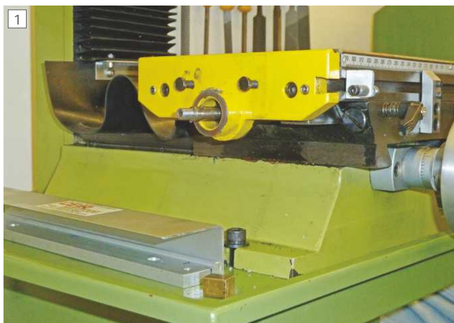
Choosing a mounting point for the y-axis
