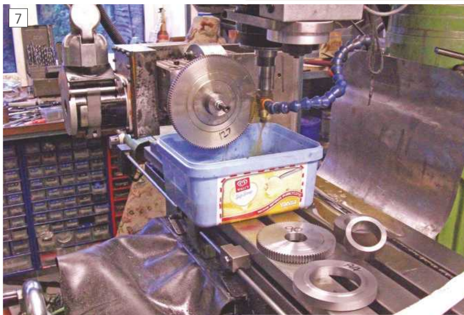
The 127 tooth gear being hobbled and the other gears and blanks.
