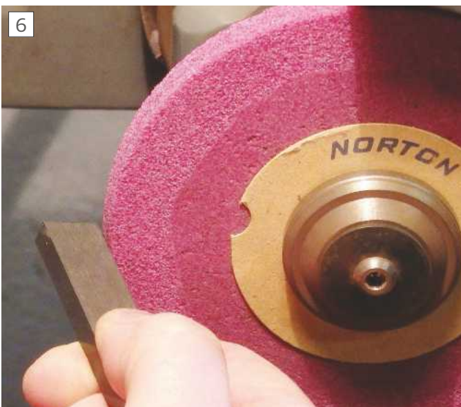
Refreshing the wheel with a boron carbide stick
