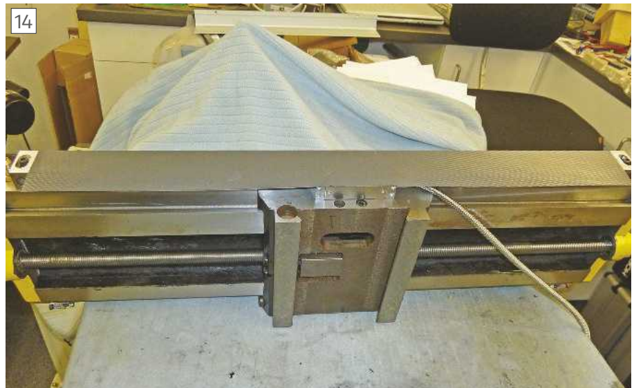
DC flap added to help keep coolant out
