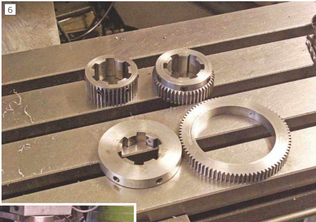
Only three new spline parts were required.
