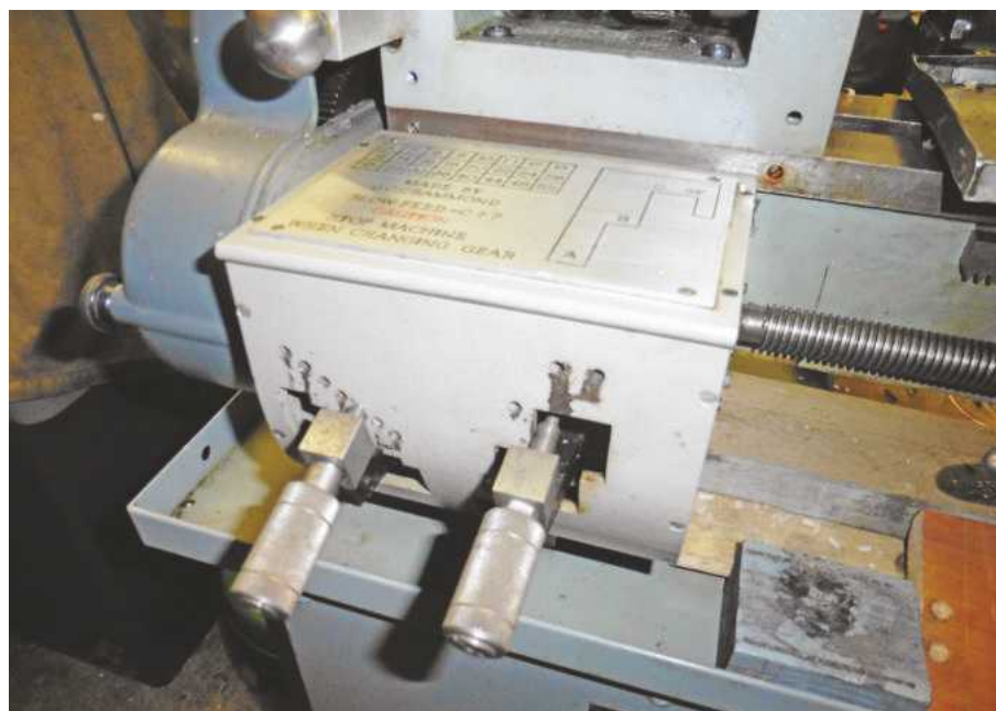
Gearbox fitted to the 'Crammond' lathe
