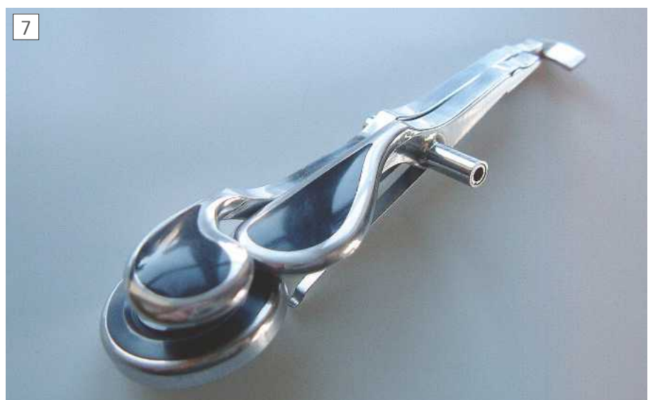
The construction and installation of the left hand thumb key cluster. The key is kept open by 2 flat springs screwed to the underside of each lever.
