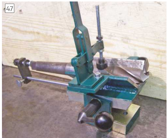
Drill set up and clamped in the jig
