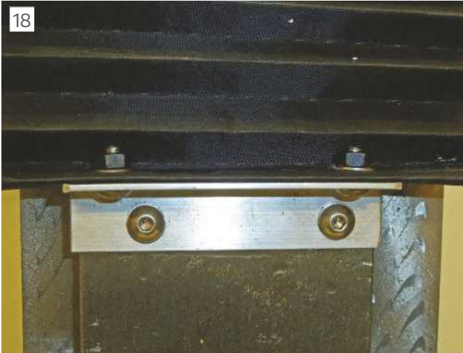
Button head screws maximise travel
