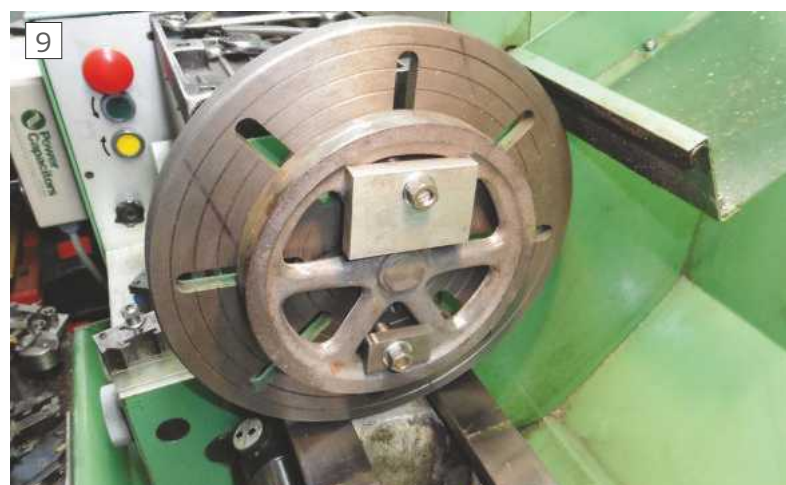
Flywheel mounted on faceplate
