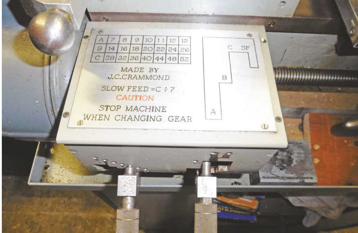
Information plate engraved on home-made pantograph
