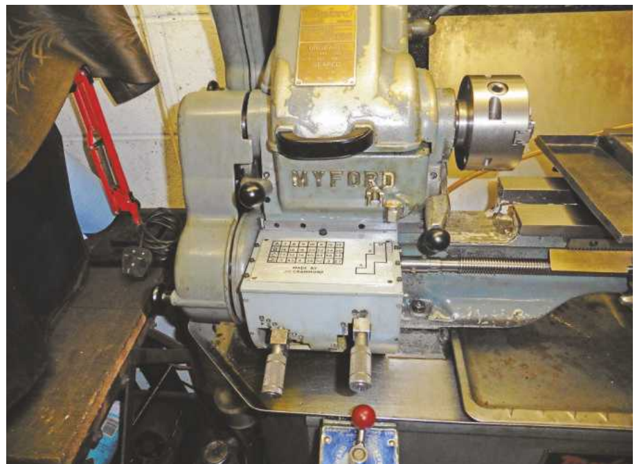
Gearbox fitted to Super 7
