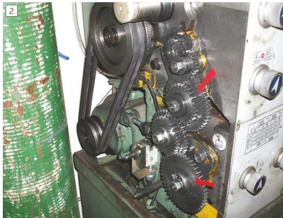
The changewheels on the rear of the Warco headstock.
