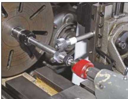
Jeff Thyer adapts his Myford lathe for hobbing helical gears.
