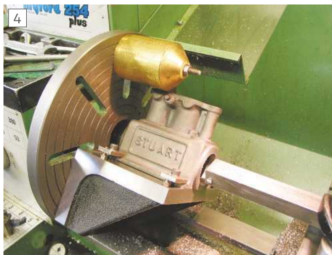
Line boring the Sirius crankcase
