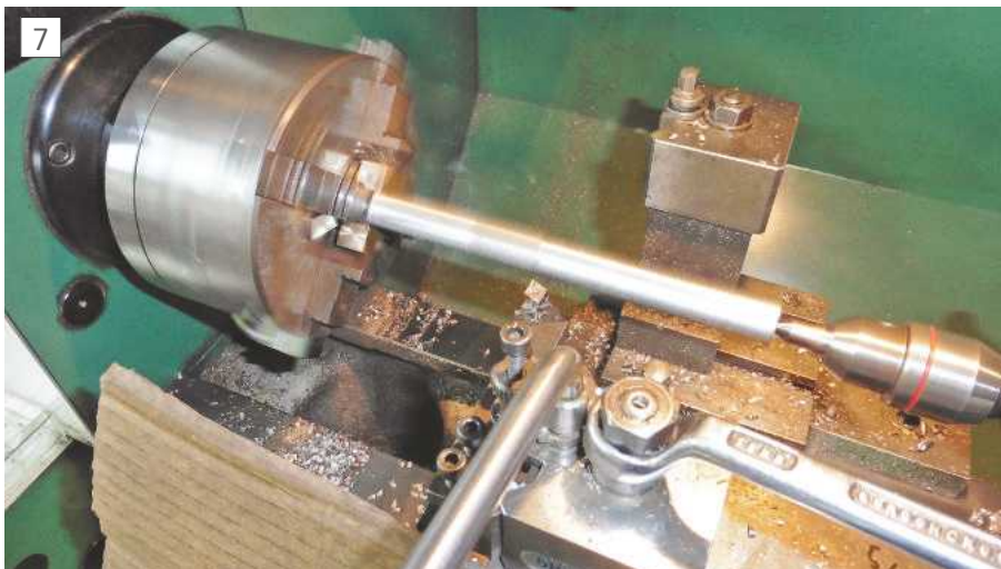
Machining cylinder support for Stuart Number 1
