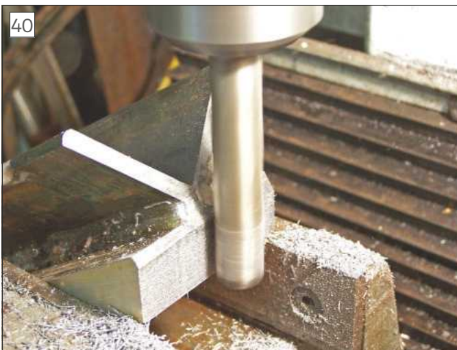
Machining the front face of the jig
