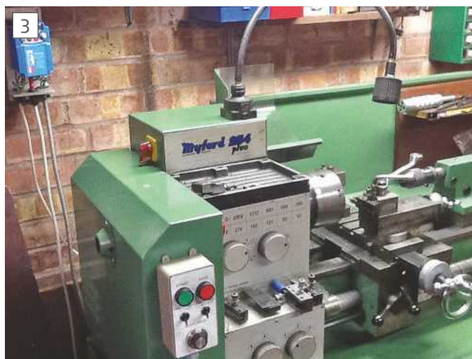
The business end of the Myford 254, note the wall mounted inverter
