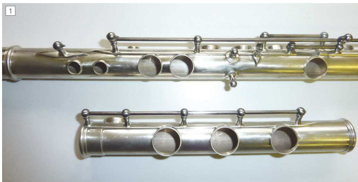
Stainless key posts silver soldered to straps which are then soft soldered to body tube. Good alignment is vital.
