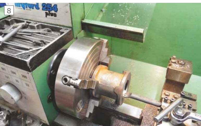
Boring cylinder in four-jaw
