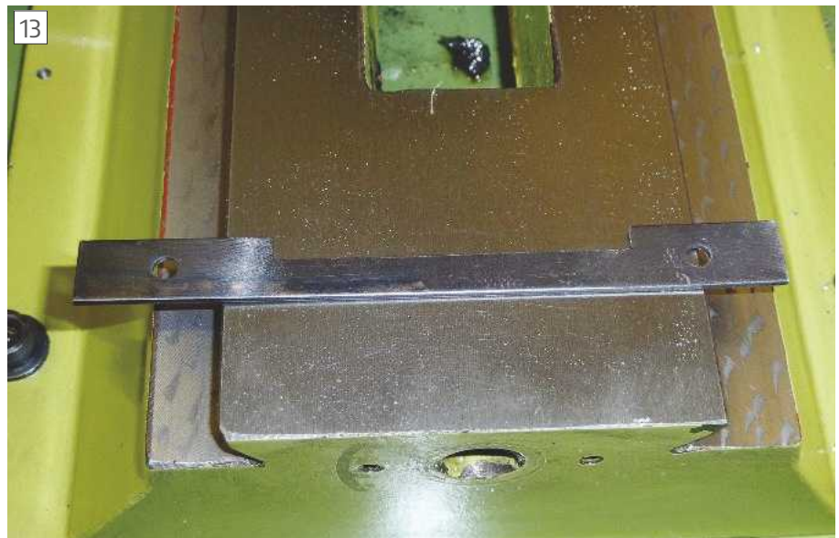
Modifying the clamp for the rubber shield
