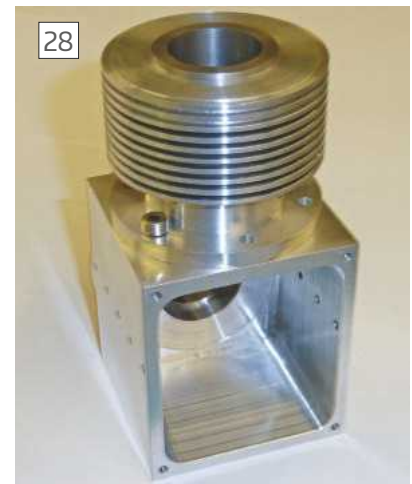
The crankcase was milled out on the WM16
