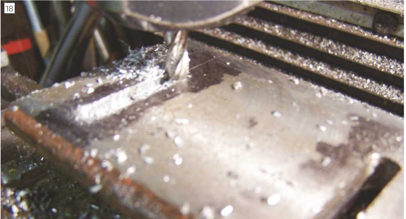
Machining the slots in the angle base
