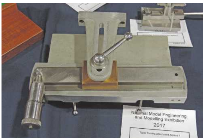
Myford taper turning attachment by Steve Tracey, who also exhibited several other beautifully finished tools, including a mirror-polished cast iron boring head.
