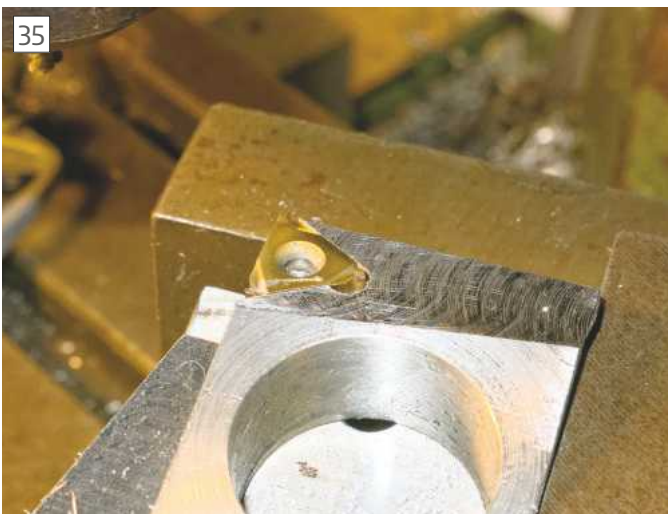
Insert in place
