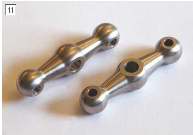
Finished Valve Rod Couplers
