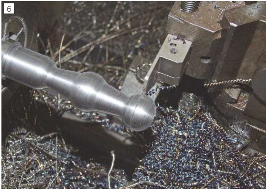
Close up of Profiling Operation
