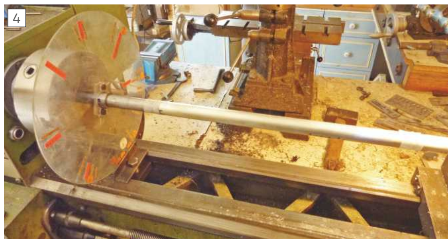
Marking out tone hole positions. The disc shows all the angular data and the piece of angle clamped to the lathe bed carries an index mark.
