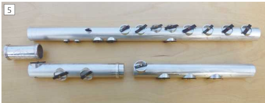
All saddles clamped in place ready for soldering. Two foot joints are shown (see text) and a head socket.
