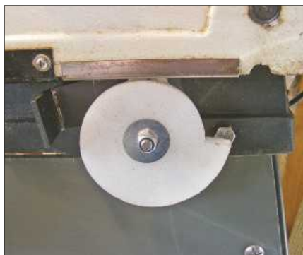
Another visit to Mike's Workshop, where he shows us how to make and fit an adjustable bandsaw stop.
