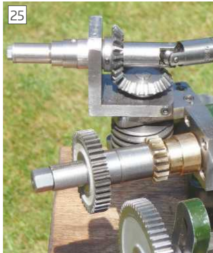
16:1 bevel and worm index drive
