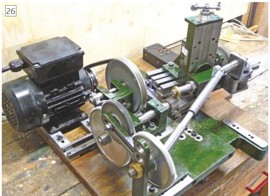
Setup for hobbing a 5T 27DP 780 HA LH gear
