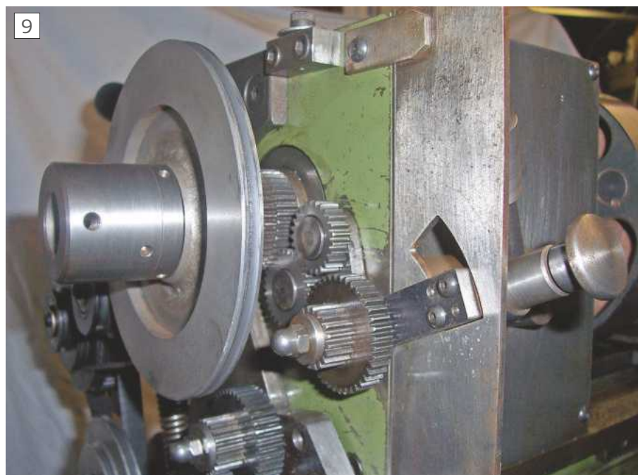
Tumbler reverse and the rear spindle steady.
