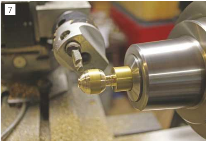
Ball creation and closeup of cutter tip
