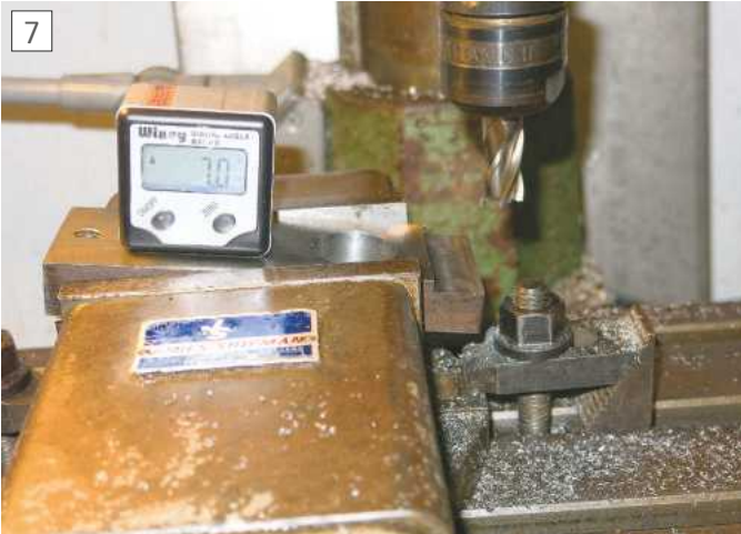
Setting a blank at an angle
