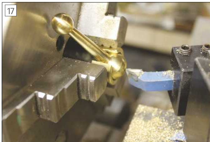
Setup to flatten one side of ball
