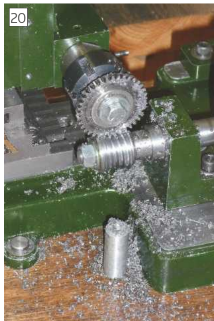
Cutting the double enveloping worm
