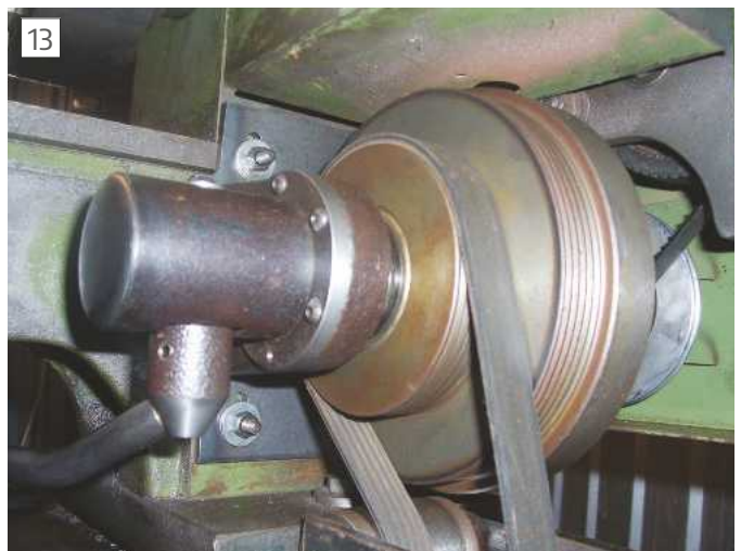
Clutch unit fitted to rear of lathe.
