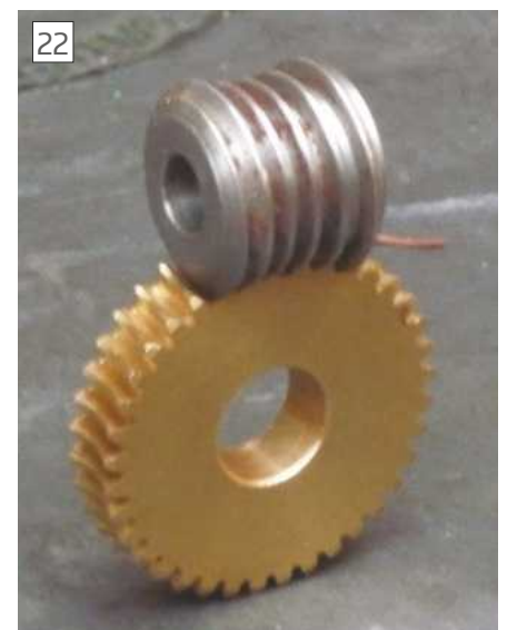
Double enveloping worm and wormwheel
