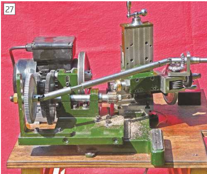
Setup for hobbing a 7T 22DP 730 HA RH gear
