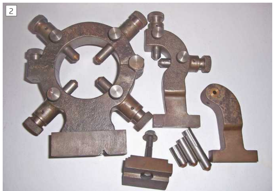
Fixed and Travelling Steadies including Travelling steady for small diameter work.
