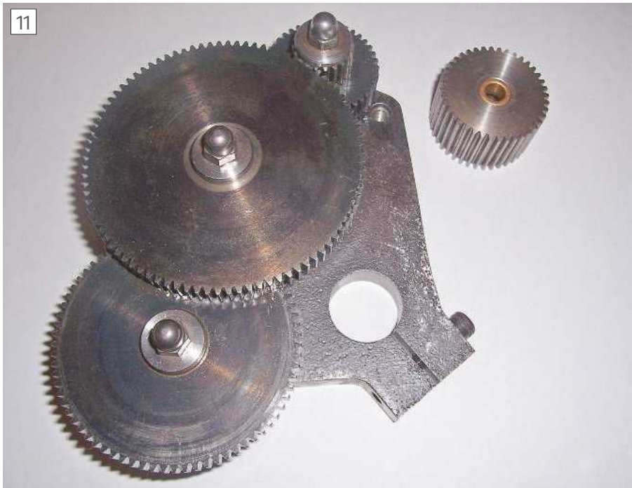
Fine feed attachment, used with a 100T gear on the Leadscrew.
