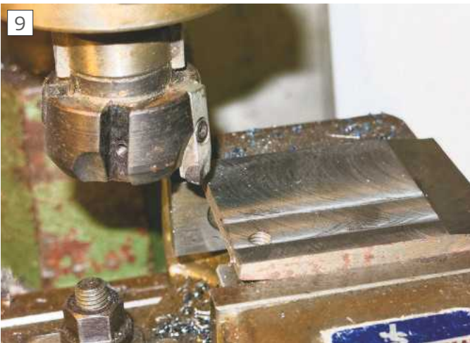
Facing with a cutter with only one insert fitted.
