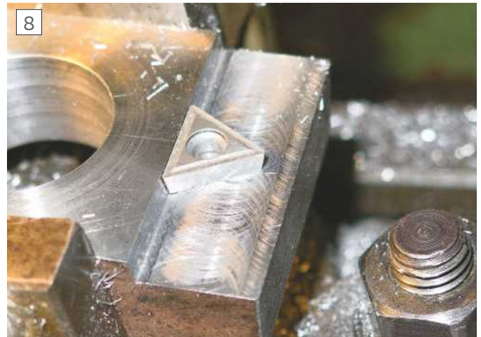
Using an insert to gauge hole position
