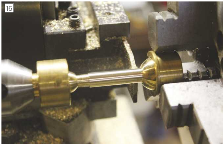
Ready for shaft tapering
