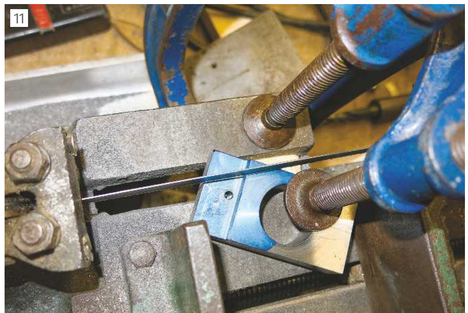
Cutting the point angle
