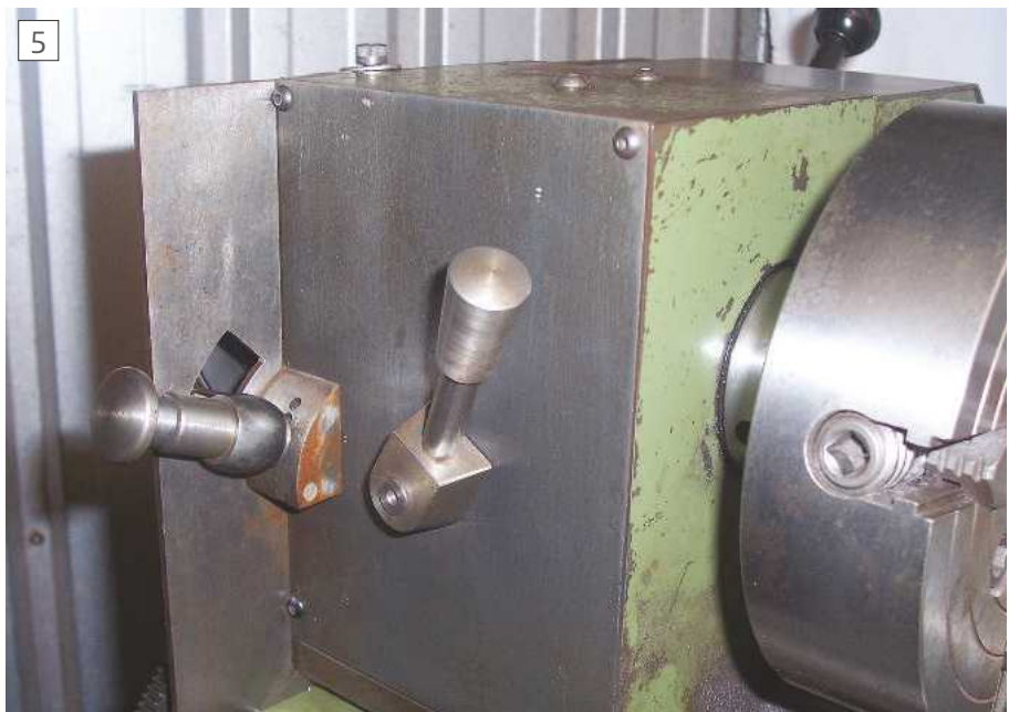
Headstock showing the spindle lock handle in the clamped position and the tumbler reverse lever.
