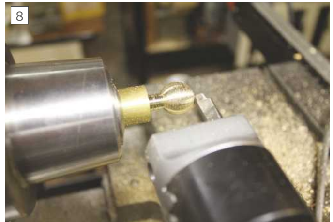
Front view of partially completed ball
