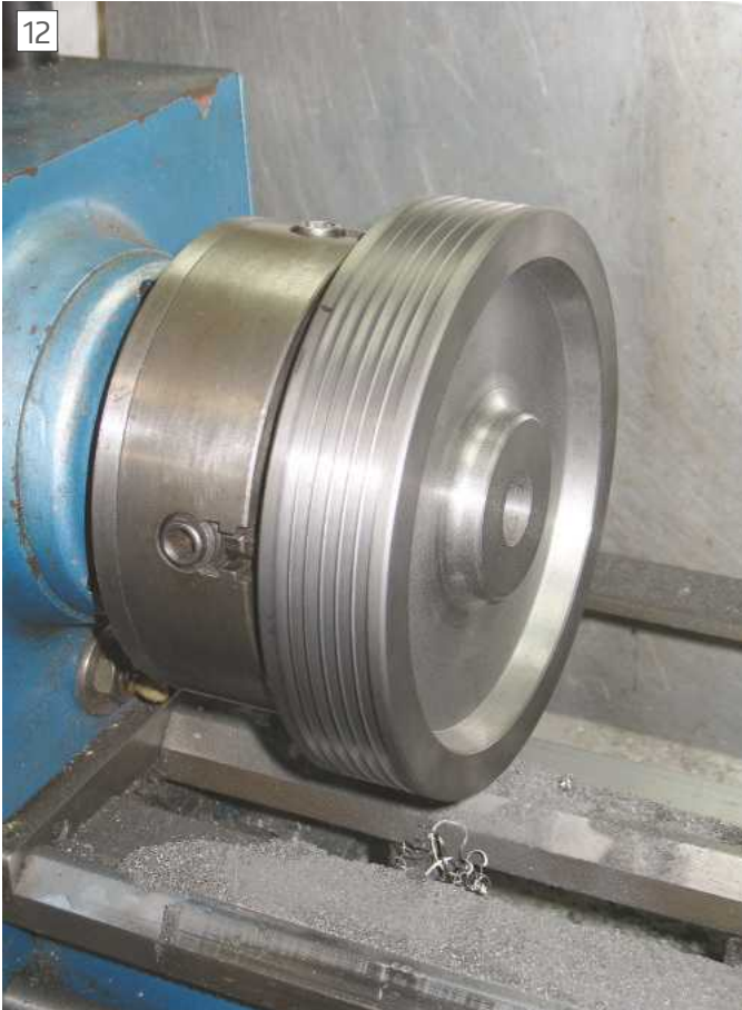
The pulley finished turning and ready for the cutting of the keyway
