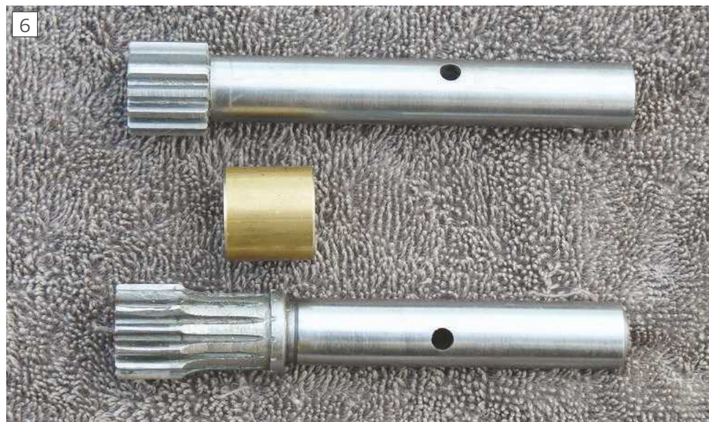
New gear and shaft (top) compare with the bent original
