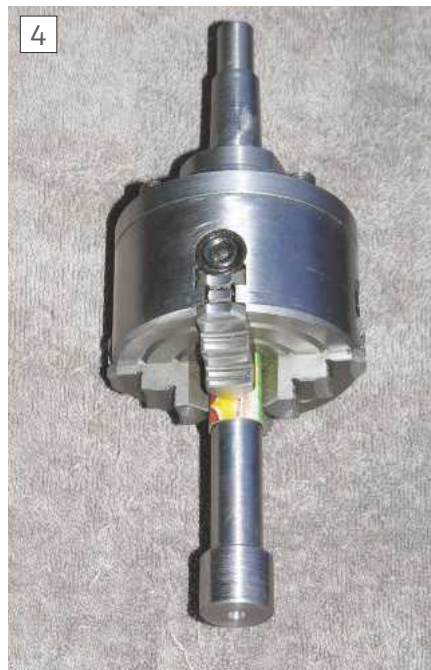
Fitting the gear blank to the new shaft
