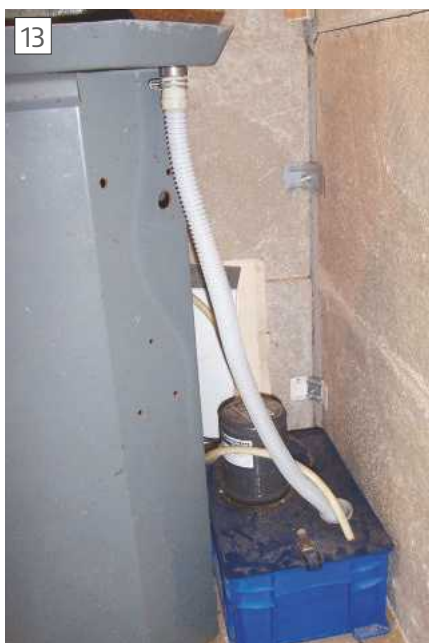
Position of coolant system
