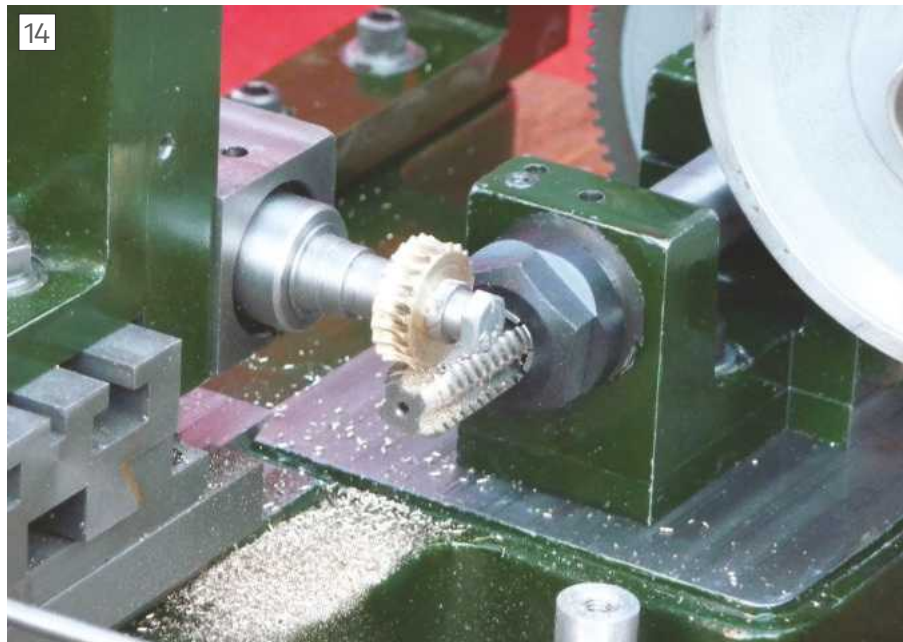
Cutting a 22 tooth wormwheel with a 5/8" x 8 tpi RH ACME tap
