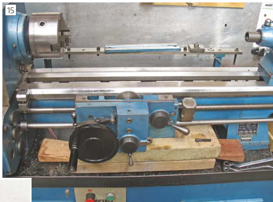
On completion, the lathe was stripped down to clean away iron dust
