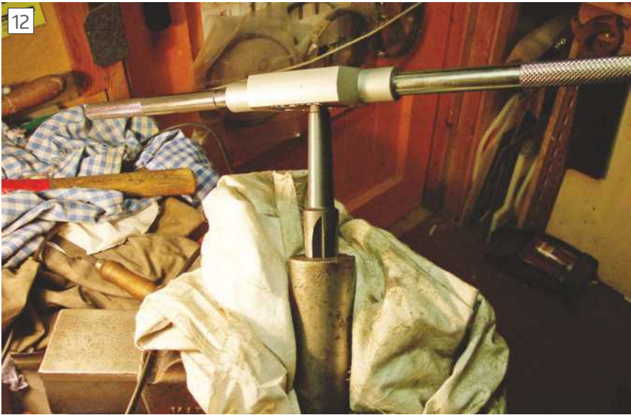
Hand reaming with the 3 MT reamer to clean up the worst of the damage
