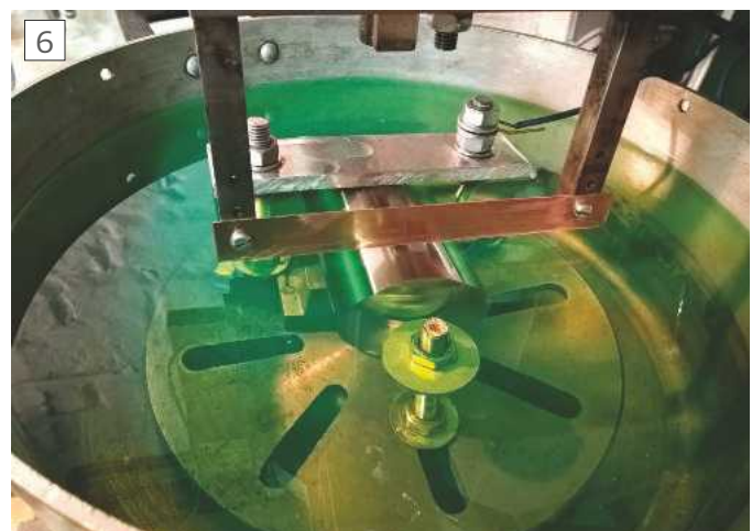
The electrode for parting-off, on the machine, liquid partly drained
