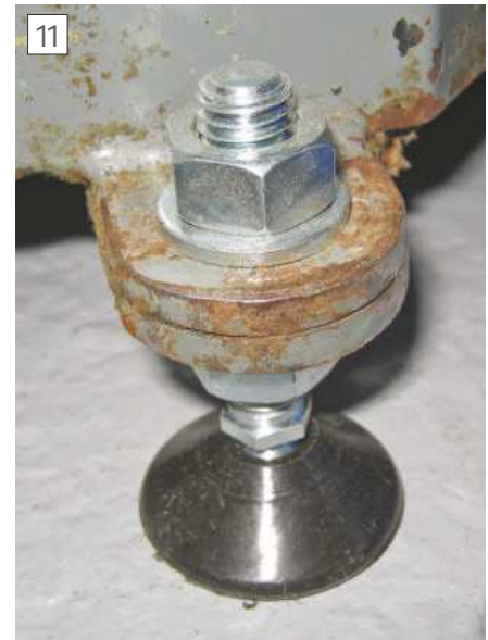
Fitted lathe stand adjustable foot
