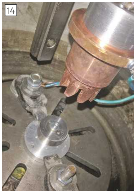
The EDM set-up for vane-cutting, prior to filling with liquid
