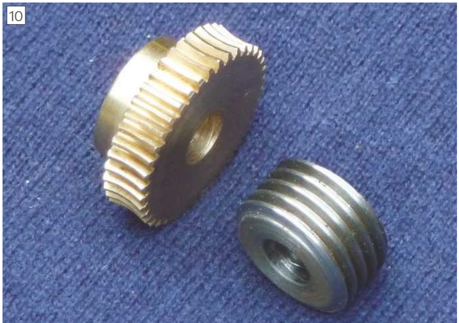
Finished Mod 0.8 LH worm and 39 tooth wormwheel
