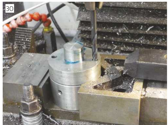
Drilling Through Register Pin Holes into Die Holder Body
