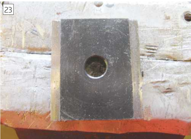
Clearing swarf and cleaning up the tailstock clamp plate
