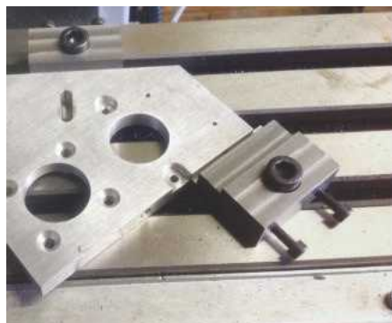
John Hinkley shows how to make some useful milling clamps.
