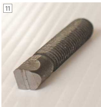
A cutting tool made from a bolt to round the tips of the pulley vees
