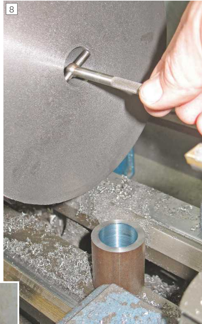
Using the Telescoping gauge to compare the prototype bore with the pulley bore diameter
