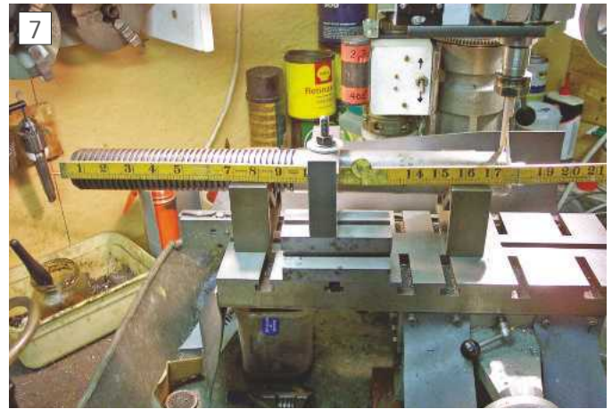
Barrel clamped on Vee blocks on the mill table. Note the size and overhang
