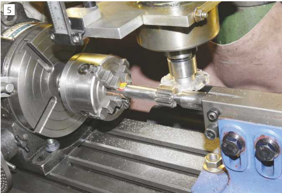
Making one of several 13 tooth gears!
