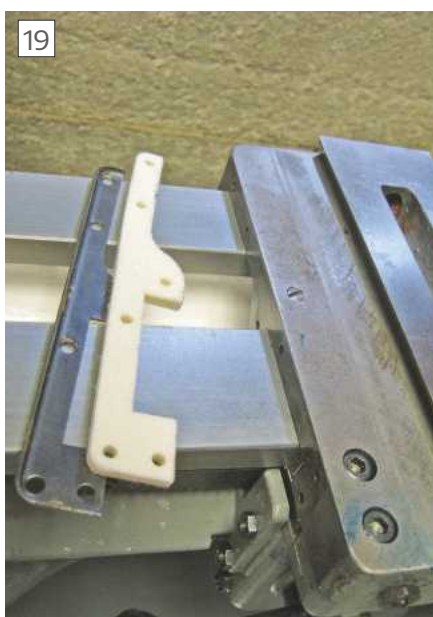
Lathe bed felt wiper awaiting fitting
