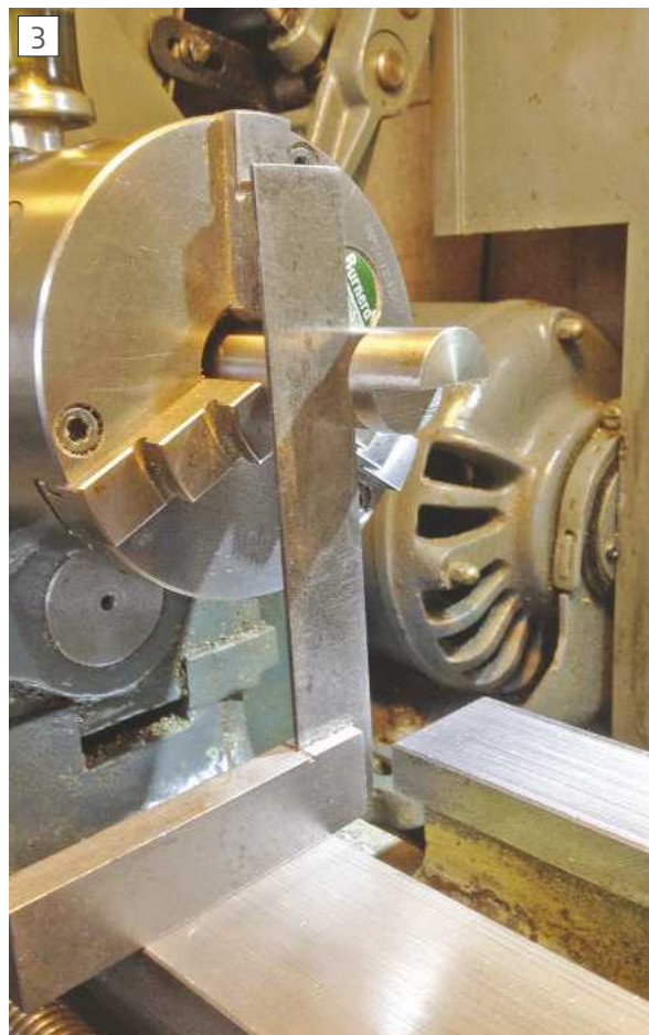
Setting the gauge with an engineer's square
