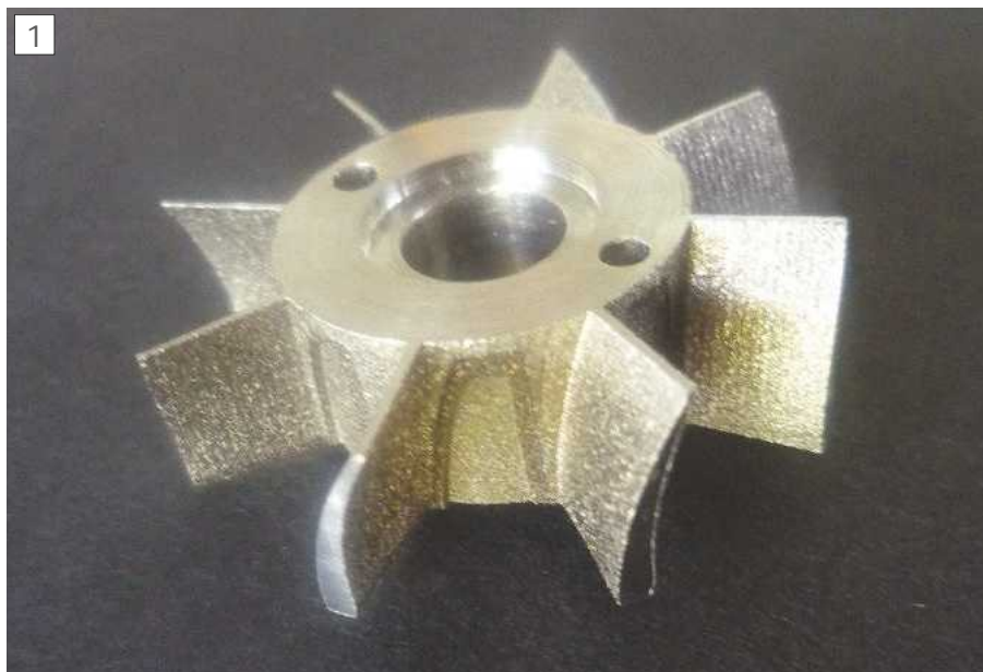
The work-piece, an exit-vane section of a turbine wheel in Inconel 718
