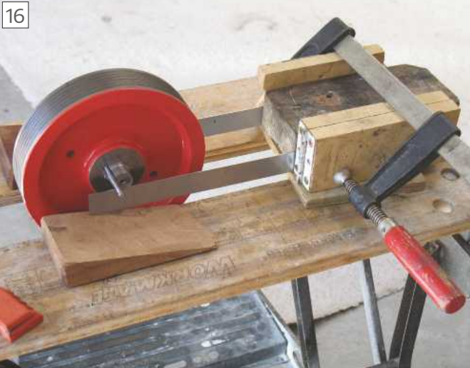
A couple of rulers used to improvise a crude but effective balancer
