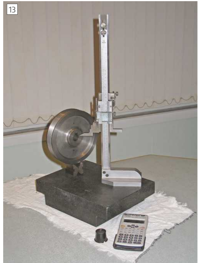
The pulley rested on a Vee block while the keyway was marked
