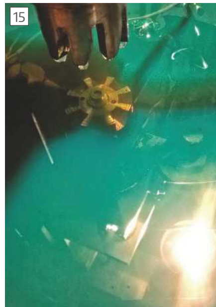
The EDM in the middle of the job, immersed in the liquid
