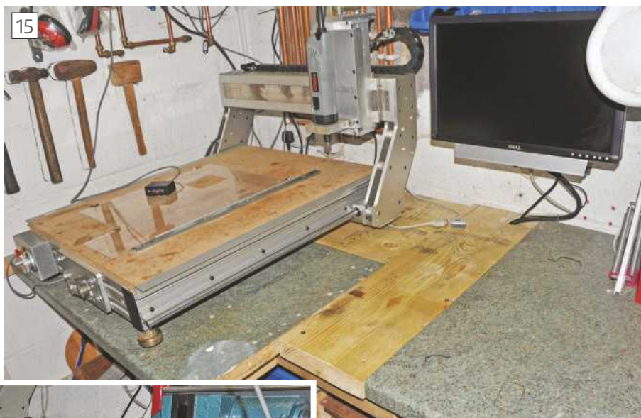
Work top made out of scaffold boards.
