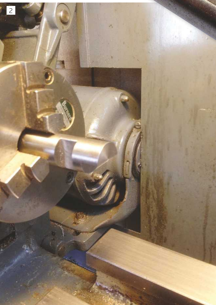
If well made, the gauge is as accurate as the 3-jaw chuck it is held in.
