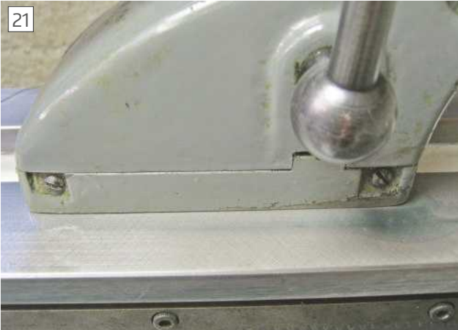
Position of adjusting screws on tailstock.
