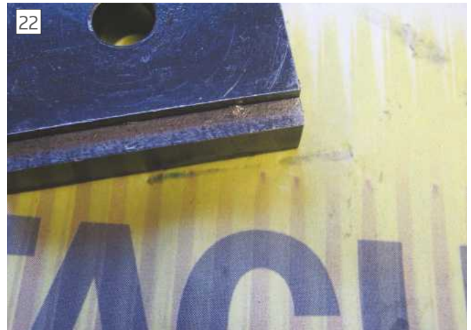
Swarf embedded in the tailstock clamp plate
