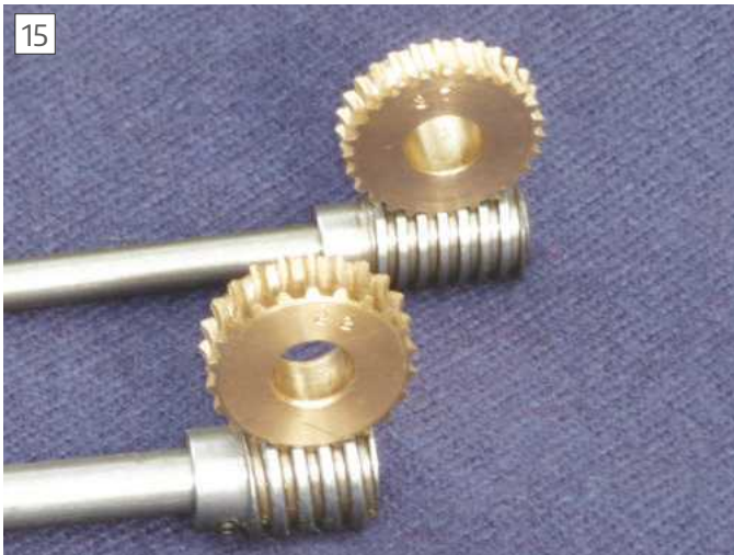
Completed 22T x 8 tpi RH and 27T x 10 tpi LH worms and wheels
