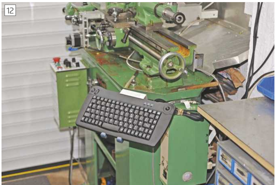
Keyboard in position ready for use with CNC controller on the lathe.
