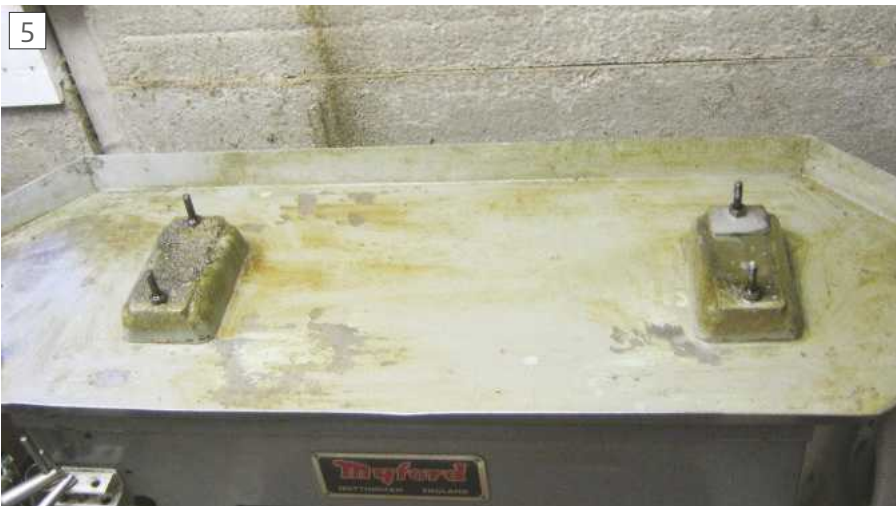
Lathe bed removed showing state of paintwork on tray
