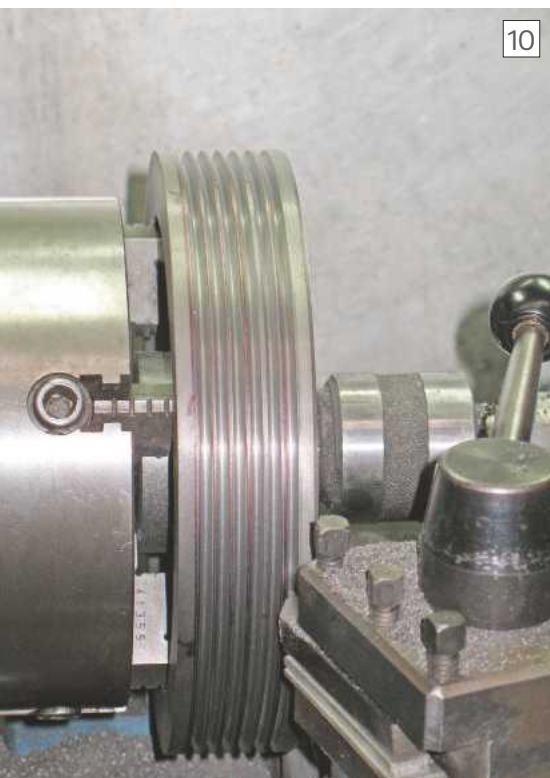
Set up for cutting the vees on the pulley
