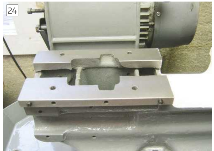
Position of adjusting screws on the headstock
