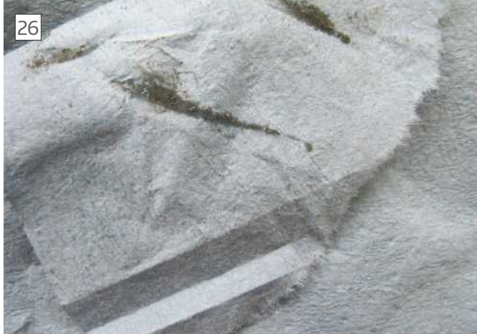
Debris removed by reamer from headstock bore
