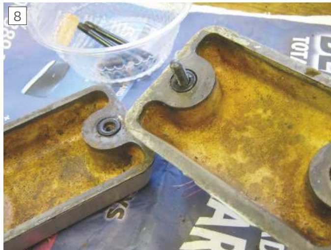
Underside of mounting blocks showing "creeping" paint and tray sealing washer.
