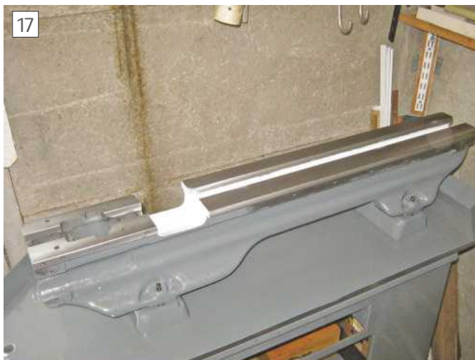
Reground lathe bed back on the stand
