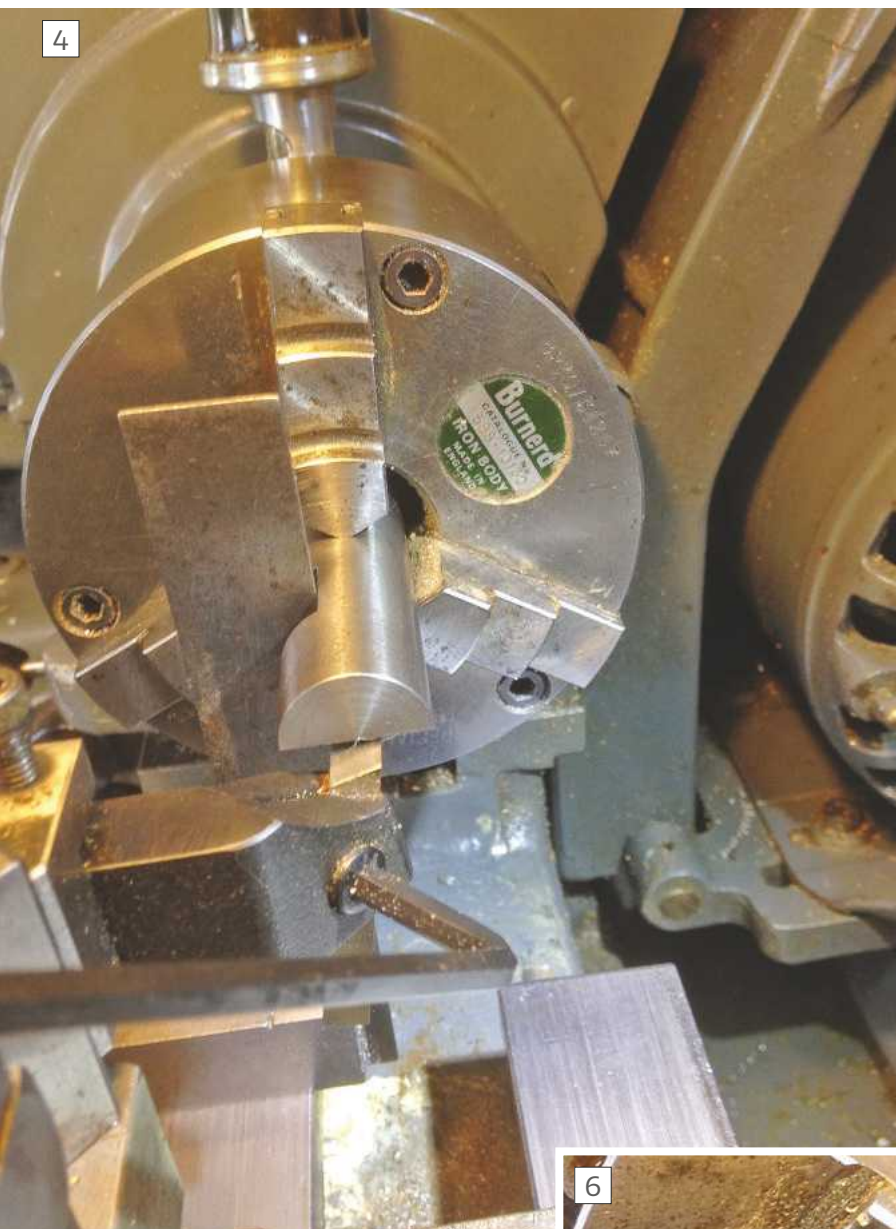
Setting a tool to the gauge
