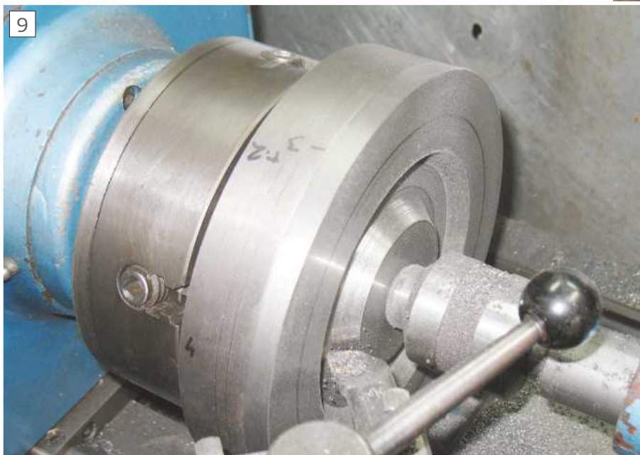
The jaws of the 4-jaw chuck expand to clamp on a recess cut on the back of the pulley
