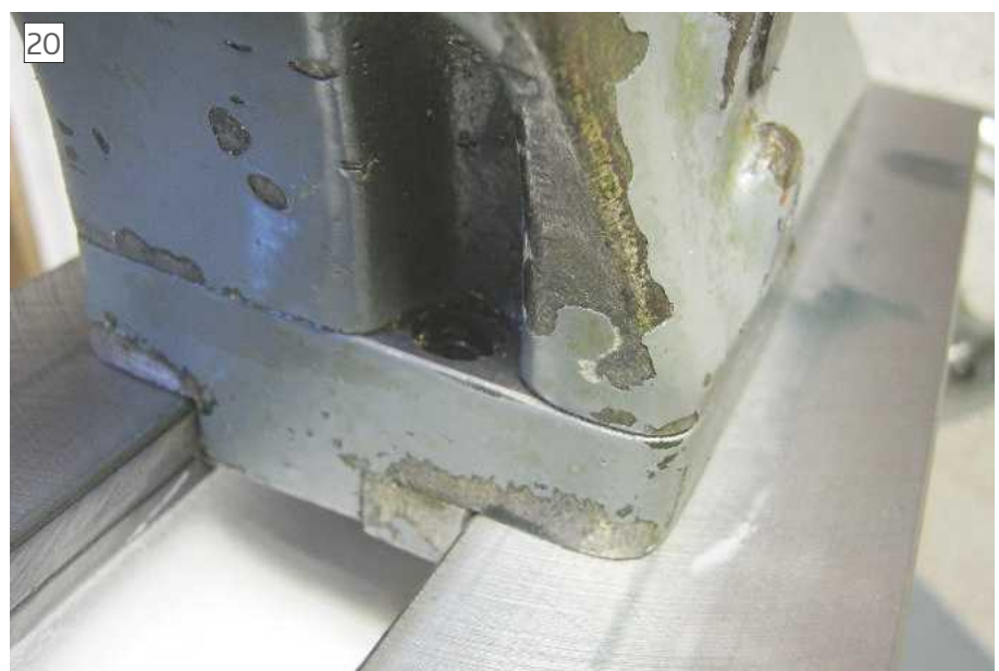
Tailstock adjustable strip and securing bolt
