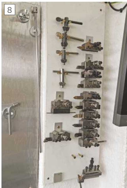
Tools mounted above lathe on improvised tool holders
