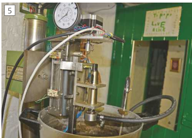
The EDM slide with stepper drive and electrode holder
