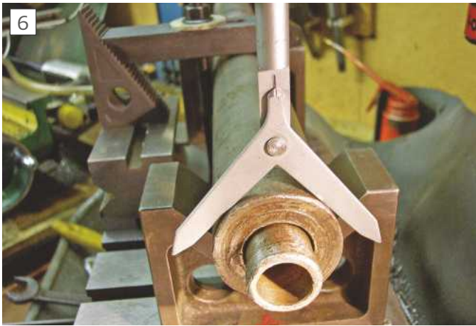
Barrel centred under the milling machine quill
