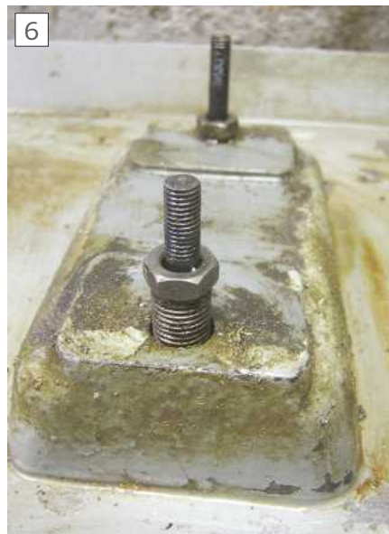
Lathe bed mounting block adjustment components
