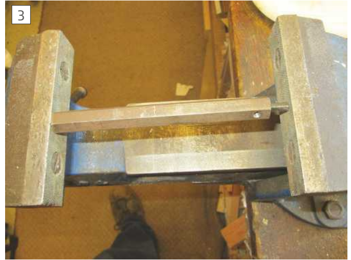
Driving the piece of Allen key into hex bar using a vice
