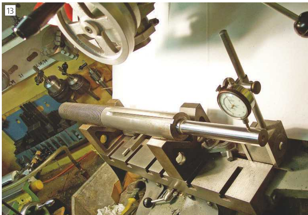
Checking socket truth and alignment
