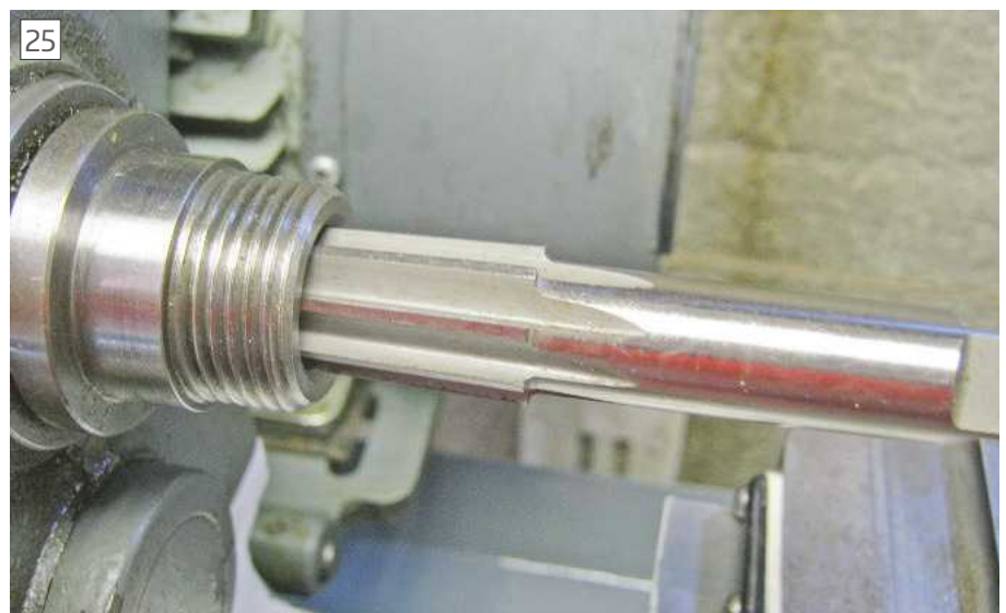
Using a No 2 Morse taper reamer to clean headstock bore
