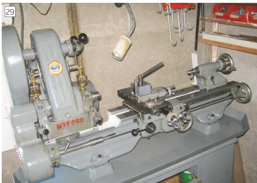
Rebuilt lathe after the bed regrind.
