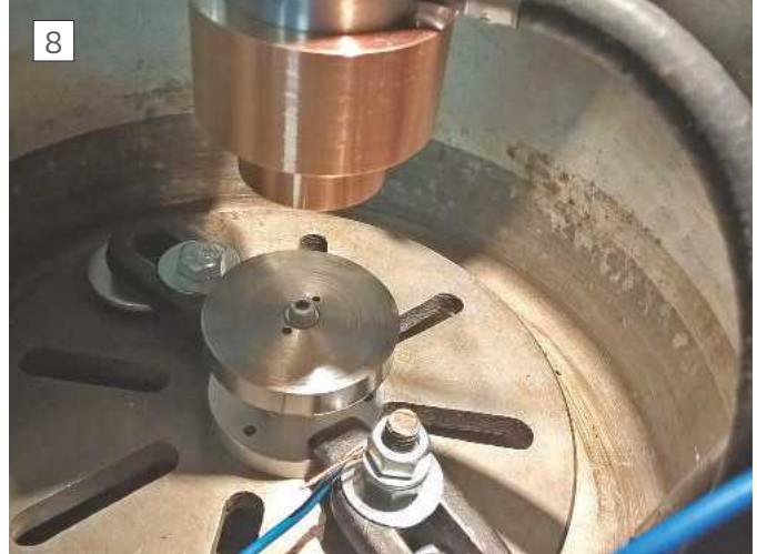
The electrode and blank, for reduction of diameter
