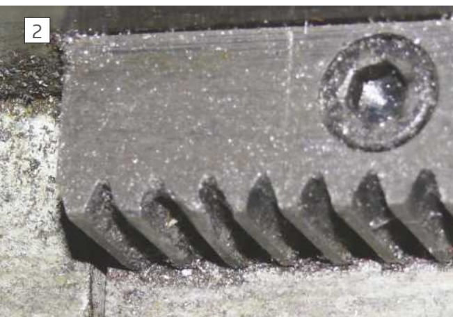
Damage to the rack
