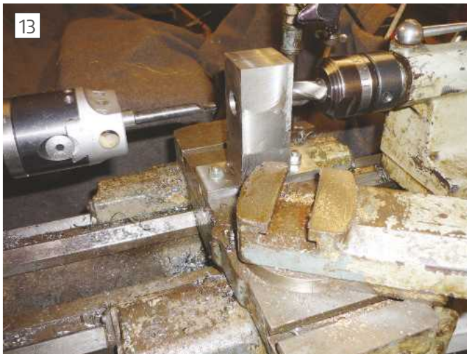
Aligning Guide Hole Ready for Boring
