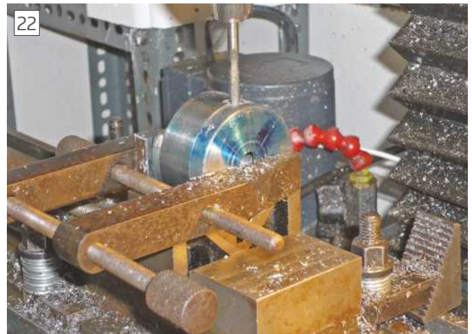
Aligning Die Screw Positions for Drilling
