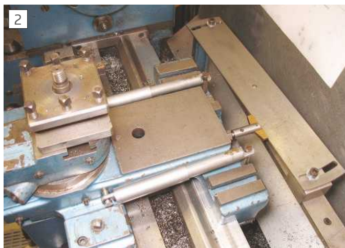
The factory taper attachment uses springs to pull the cross slide onto the straight edge
