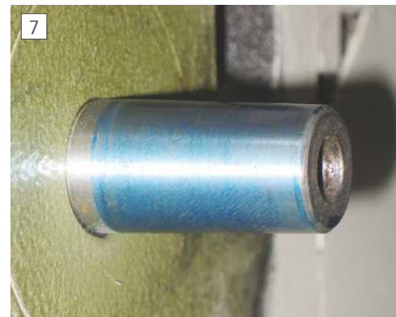
An even rub of blue transferred from the prototype bore proves a good fit
