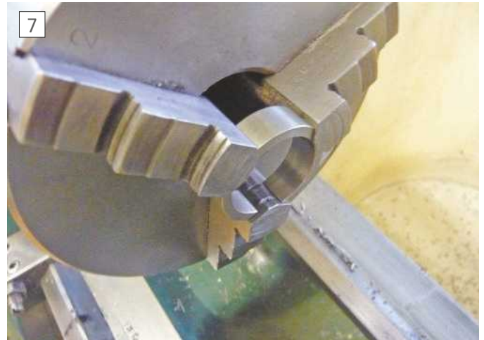
Grinding spacers fitted between jaws
