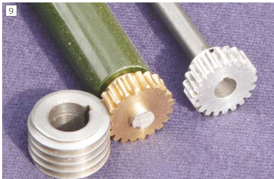
20 DP RH worm, 20 tooth wormwheel and temporary 20T helical gear
