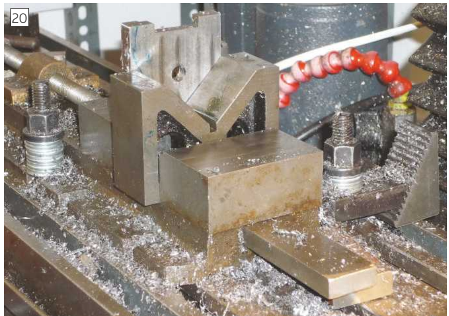
Set-up for Drilling Die Screw Holes
