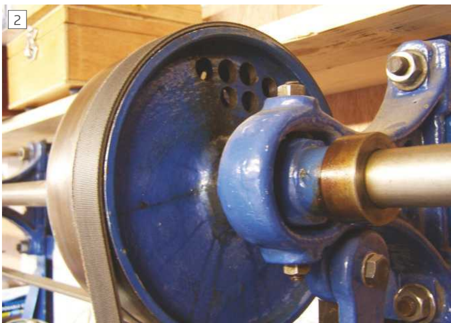
The balancing holes in the pulley
