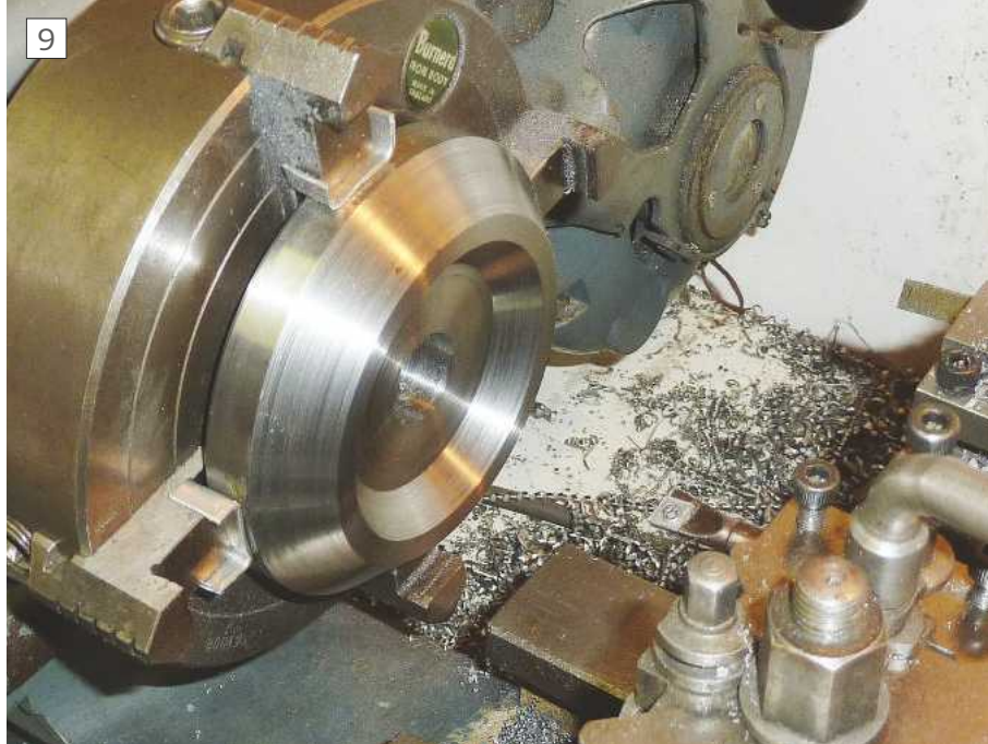
Turning operations on the turret completed.
