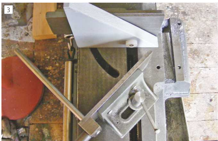
How the anti-slip disc lines up with the slot.
