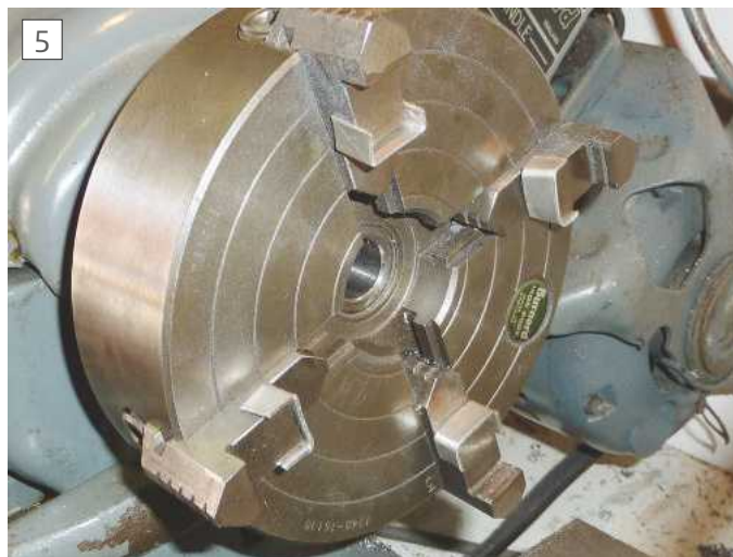
Setting up the four-jaw chuck with jaws reversed. Aluminium pads have been fitted to protect the finish on the work.
