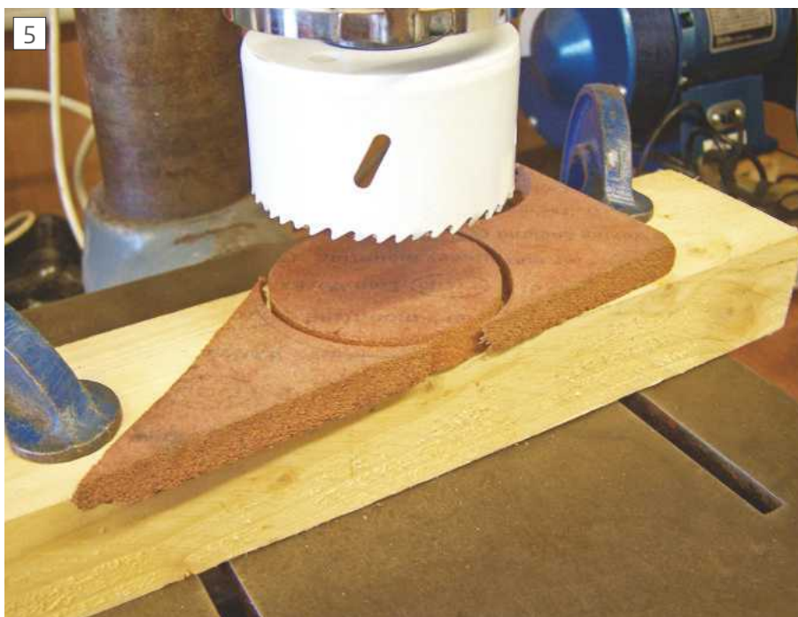
The set-up for cutting the circular pads without a pilot hole
