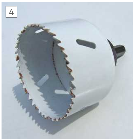
The hole saw used to cut the pads
