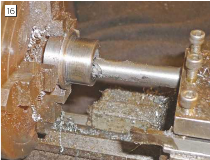
Boring to Fit Guide Tube
