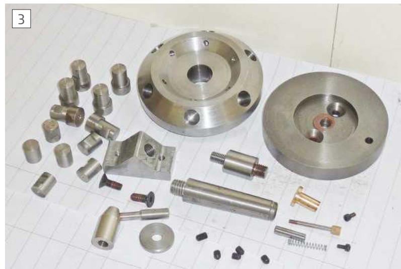
Turret dismantled to show all the parts required.
