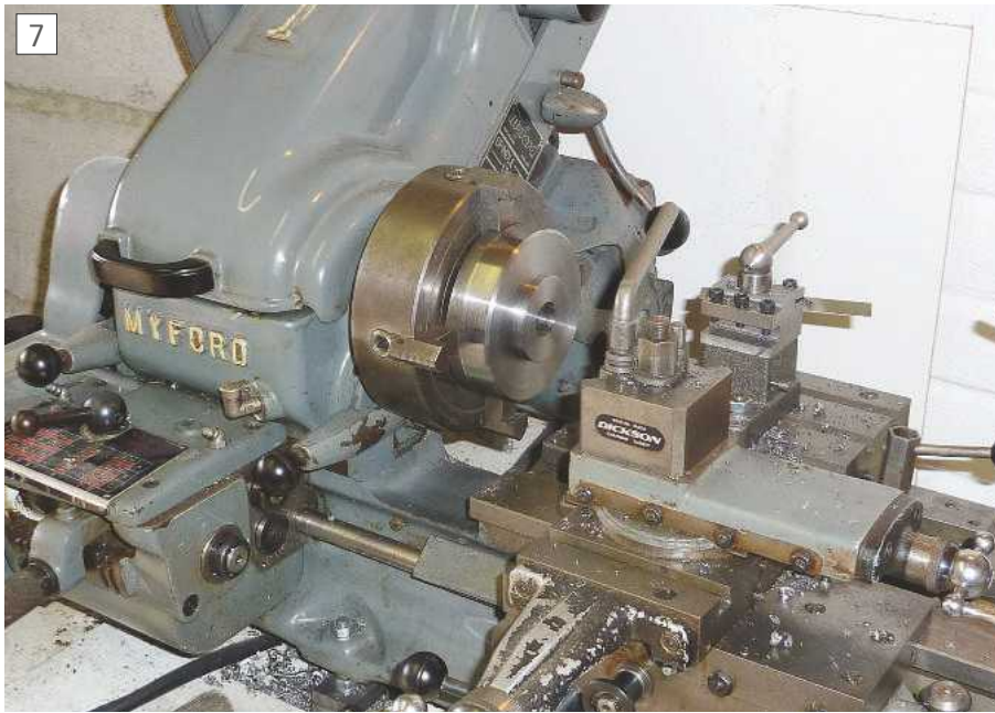
Finish-turning operations on the turret.
