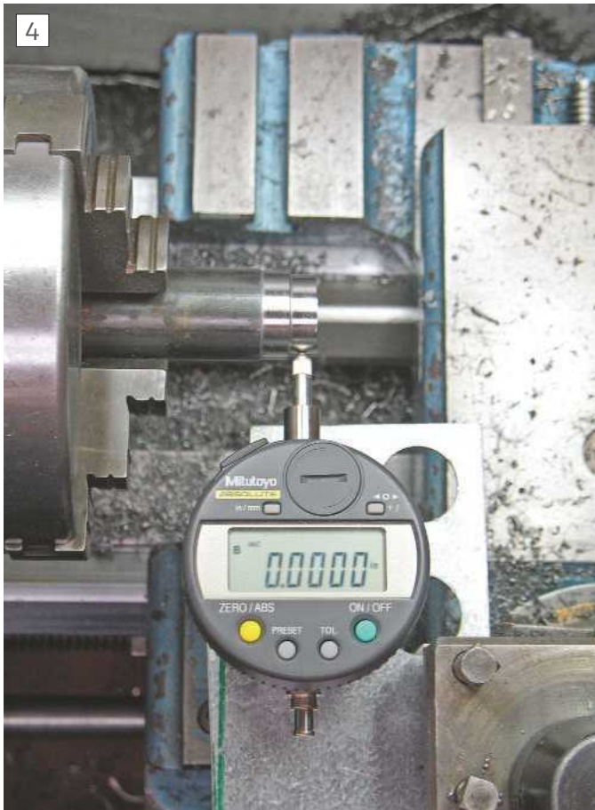
The top slide is moved to zero the gauge
