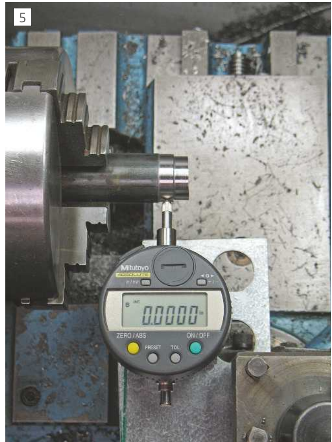
The gauge zeroed on the other step with the top slide moved
