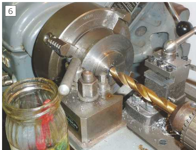
Drilling the hole in the turret before boring.
