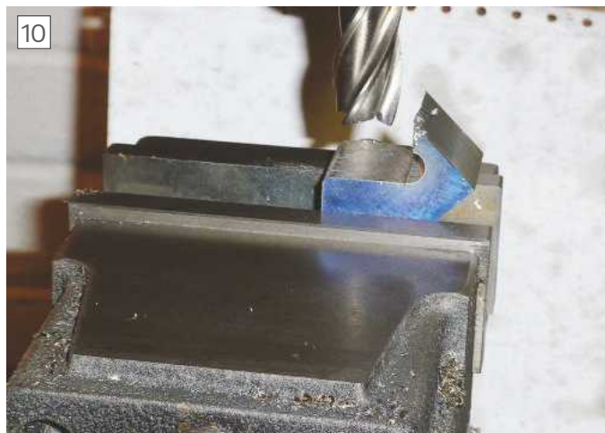
Milling operations on the angle piece.
