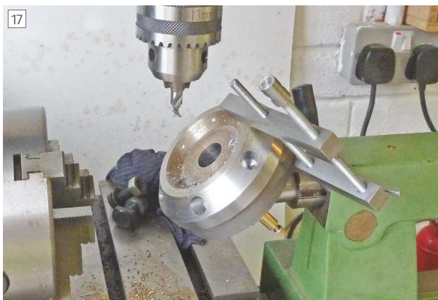
Drilling the holes for the tool station locking screws.
