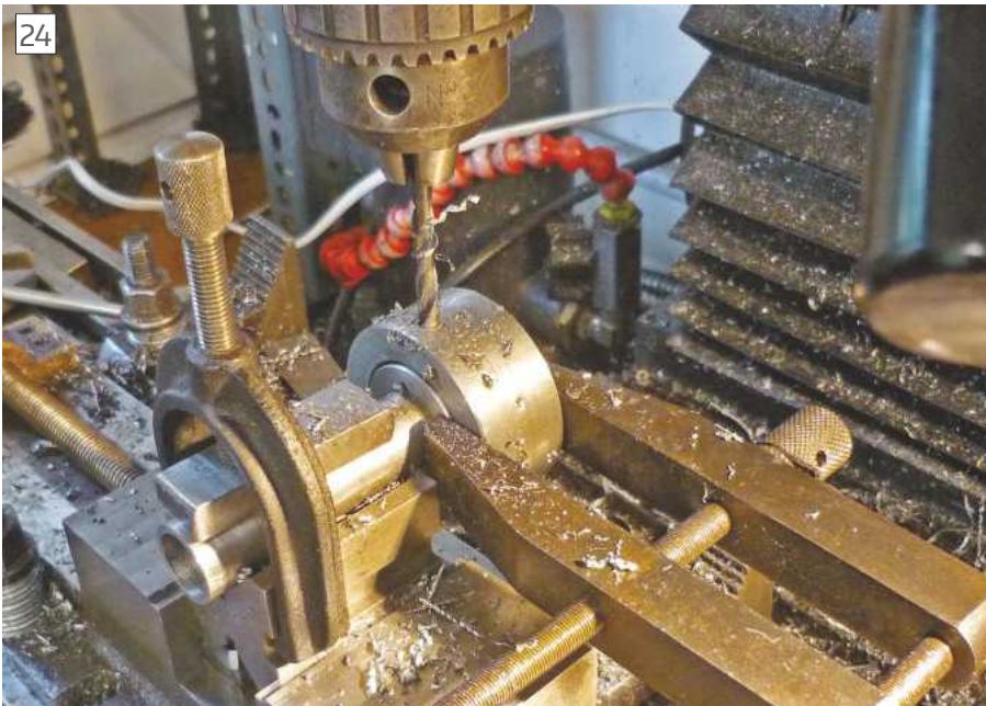
Drilling Die Holder Securing Screw Hole
