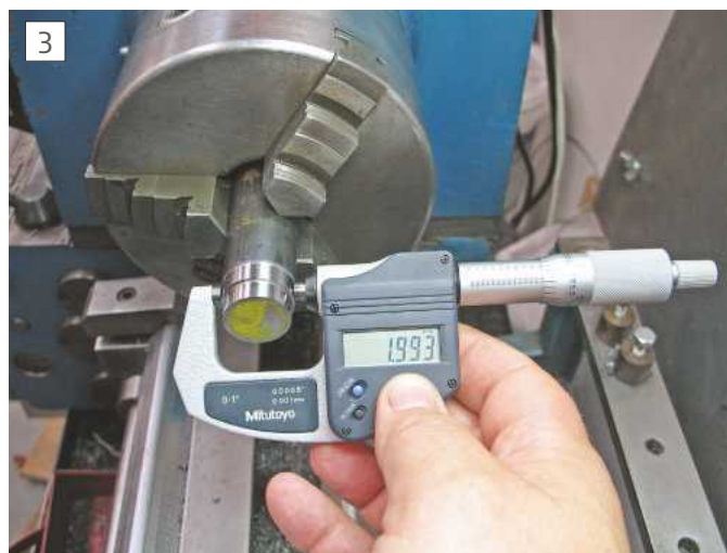
Measuring the difference between the steps on the bar
