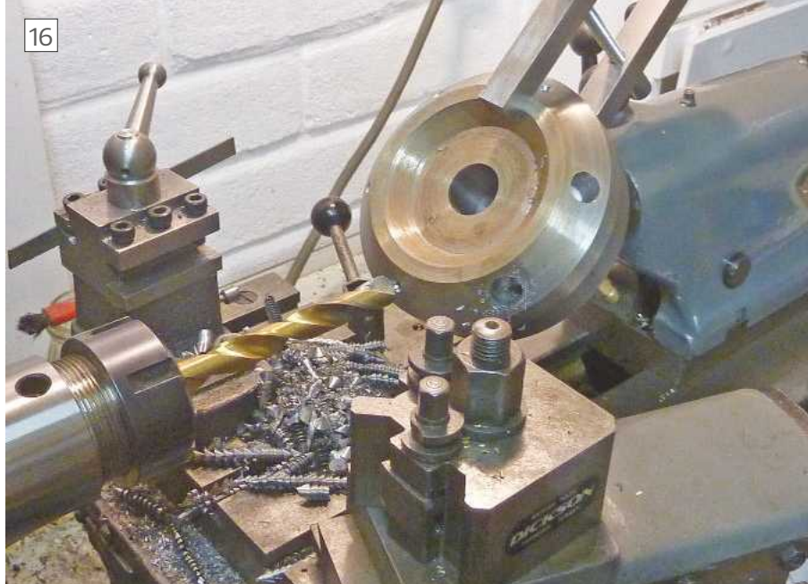
Drilling the tool station holes from the headstock.
