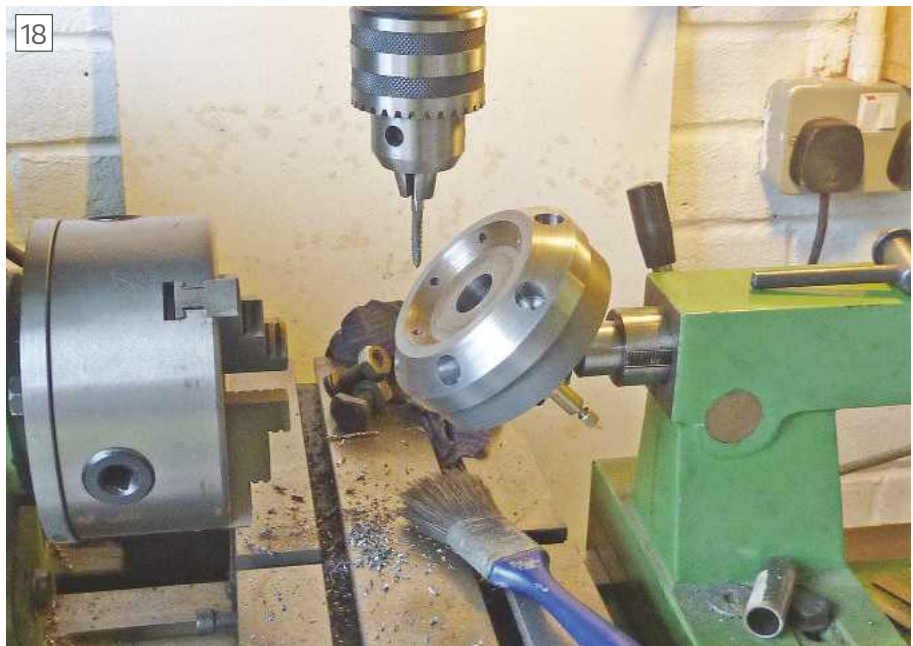
Tapping the holes for the tool station locking screws. The drill spindle is rotated by hand having isolated the machine from the mains.
