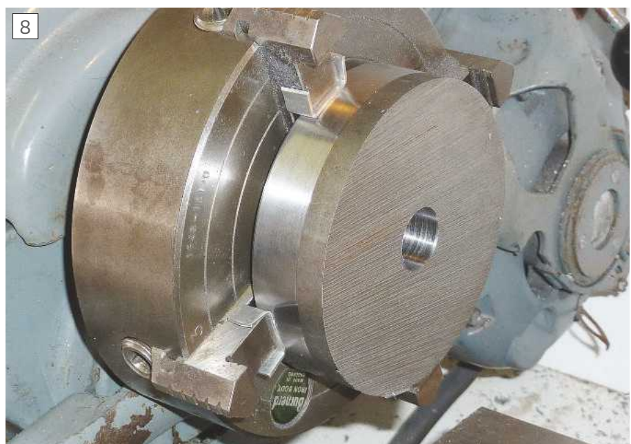
The turret reversed in the chuck ready for machining the remaining surfaces.
