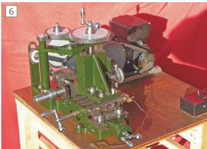
Set up for hobbing a wormwheel with plunge feed
