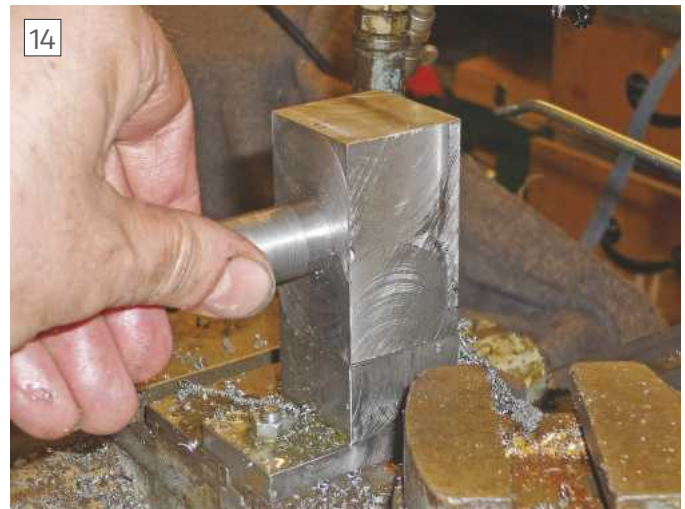
Testing Bore Size Using a Plug Gauge
