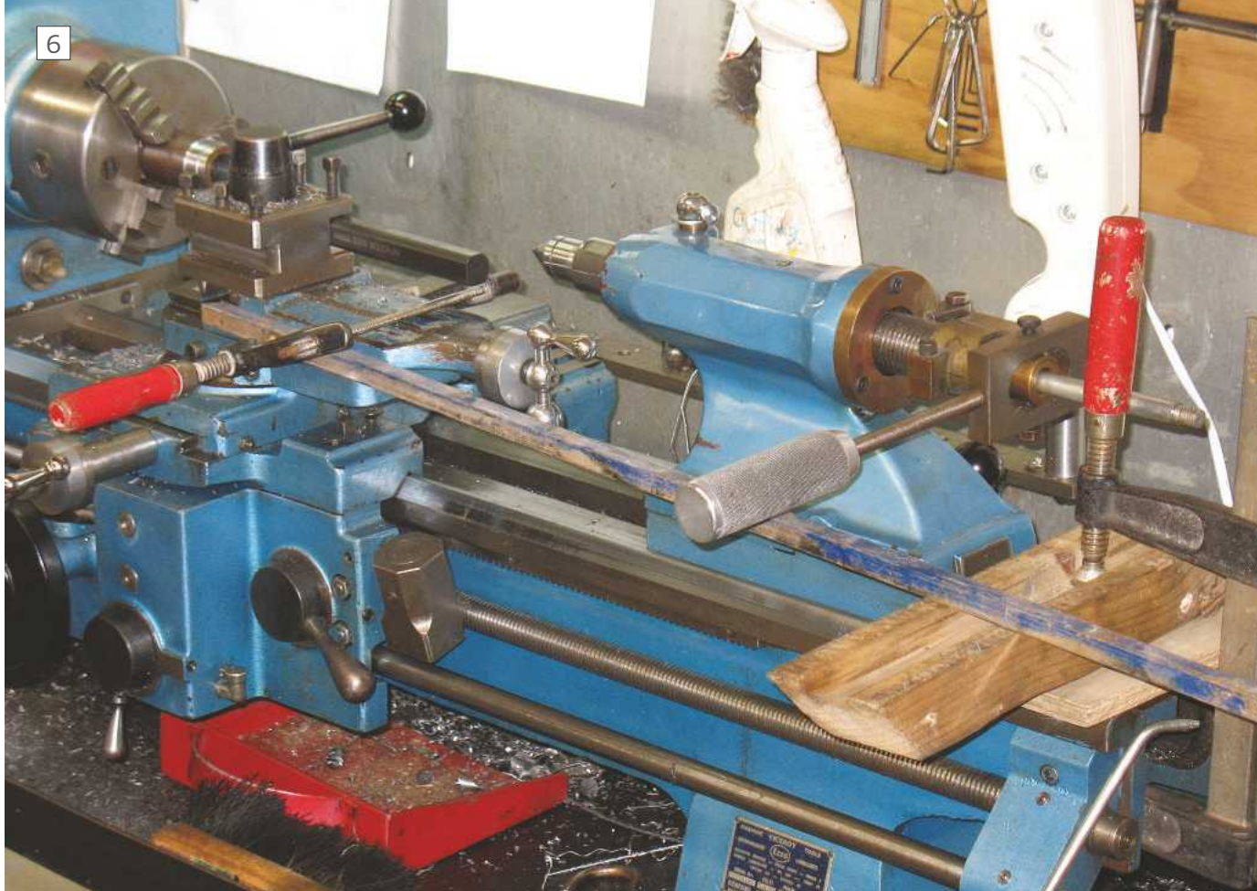
Key steel clamped to the top slide allowed fine adjustments to angle
