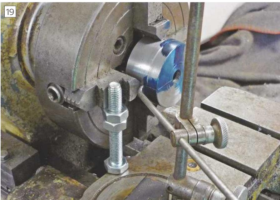
Marking Out the Die Screw Positions
