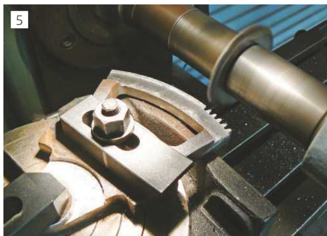
Cutting the switch gear quadrant
