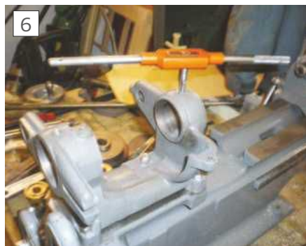
Headstock fitted to the bed
