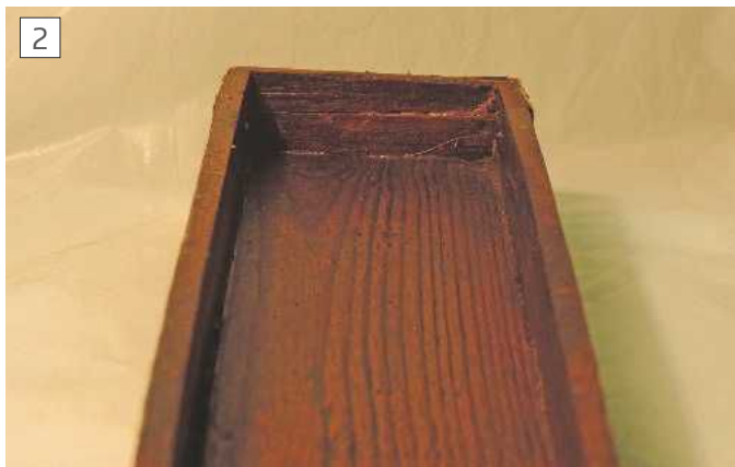
This was the end where the wood had split leaving the joint weakened
