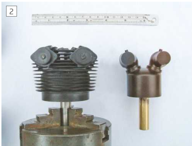
Completed exterior and core patterns. Note Milliput fillets between each fin.
