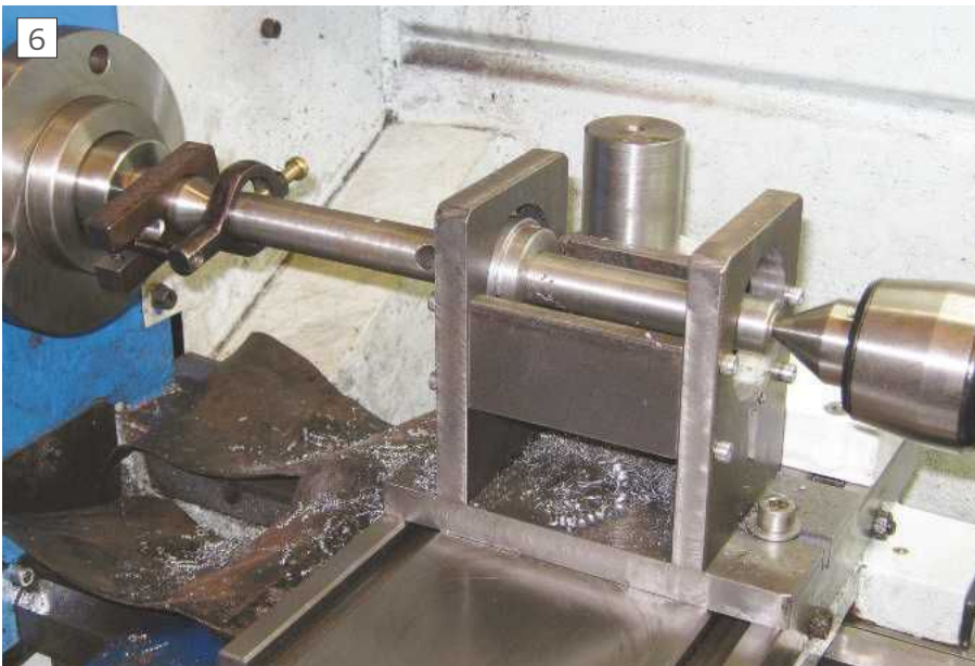
Using a between centres boring bar for finishing the bores in the uprights
