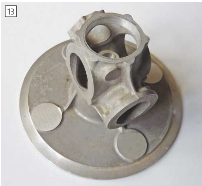
Partly machined rear cover casting.
