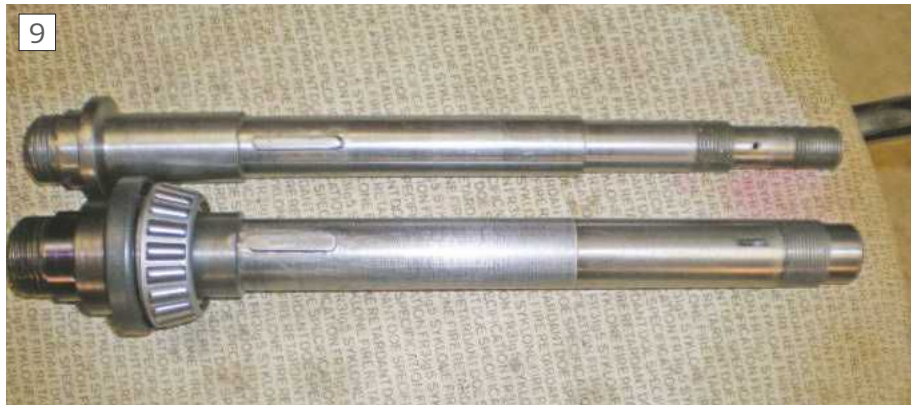
Original Drummond spindle and remachined Myford spindle compared
