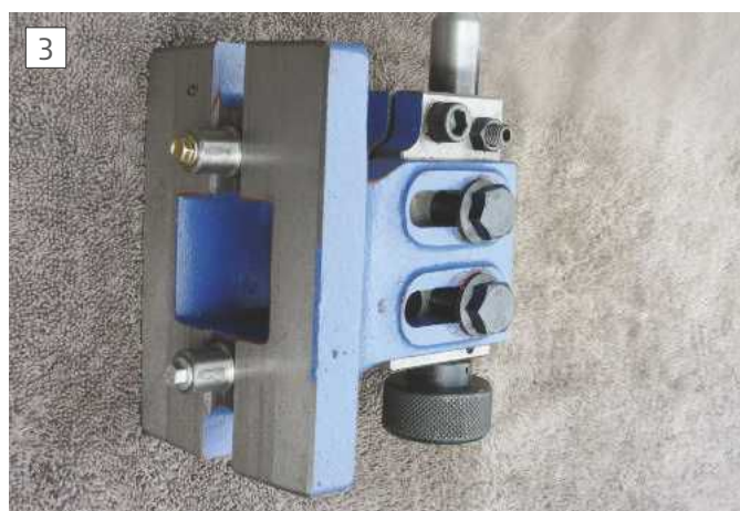
Dowels fitted in the keyway
