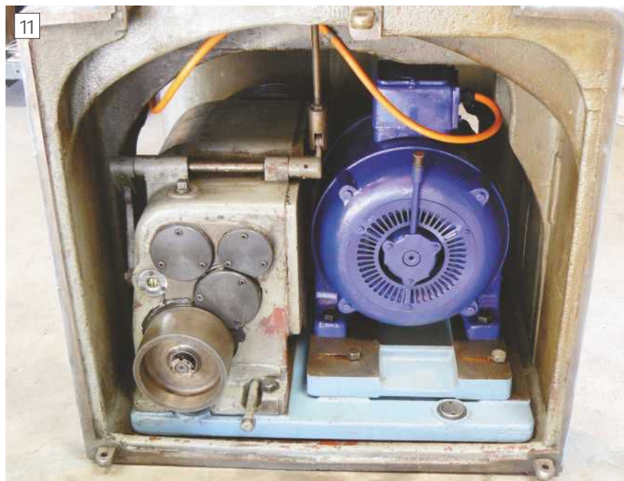
Motor and gear box on rubber mounted sub frame
