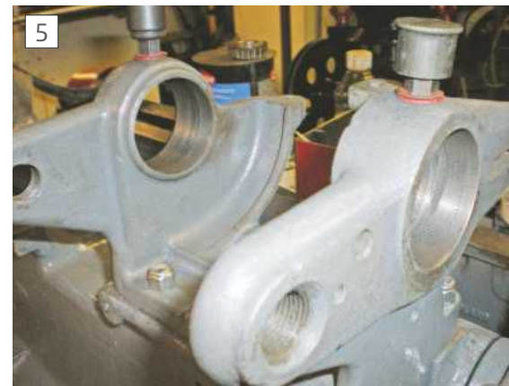
Headstock bored for taper roller bearings
