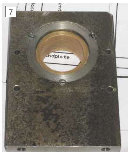
Using "French keys" to fix the rear bearing housing to the rear upright
