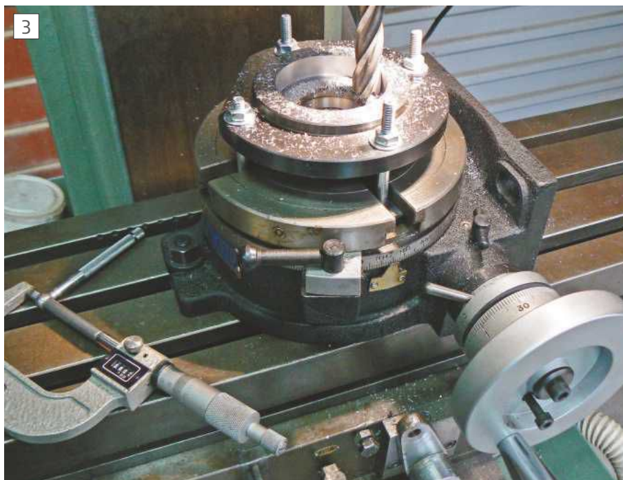
Enlarging the seal housing with rotary milling
