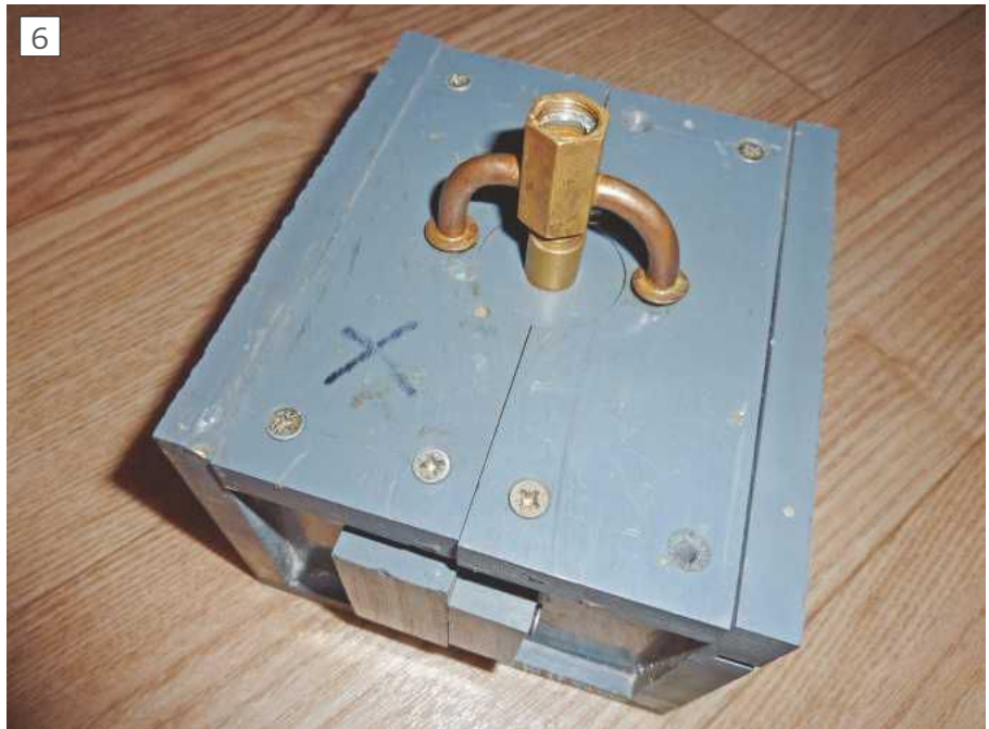
Box ready for wax injection.
