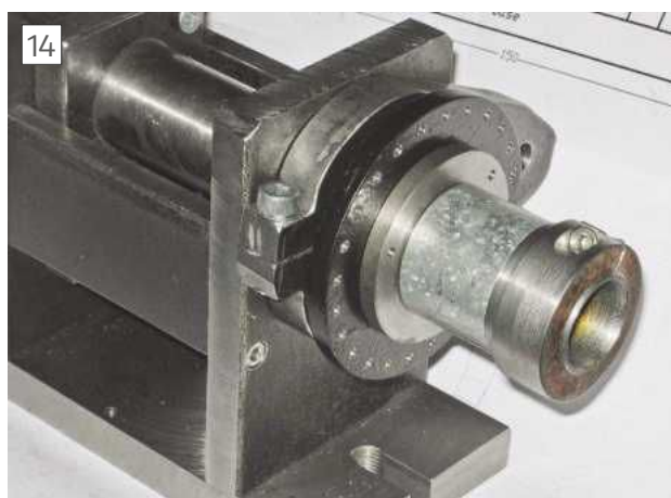
Banjo arm, hub with hole plate, spacer and spindle nut
