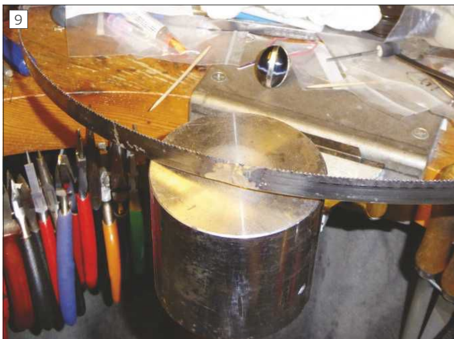
After cleaning the joint up, the blade is ready to fit into the saw – see photo 9 .
