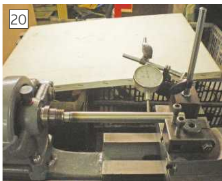
Testing horizontal alignment
