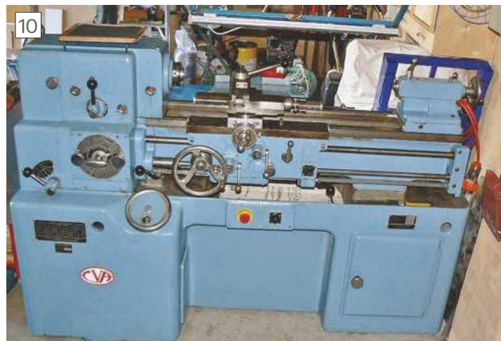
Lathe after cleaning and painting
