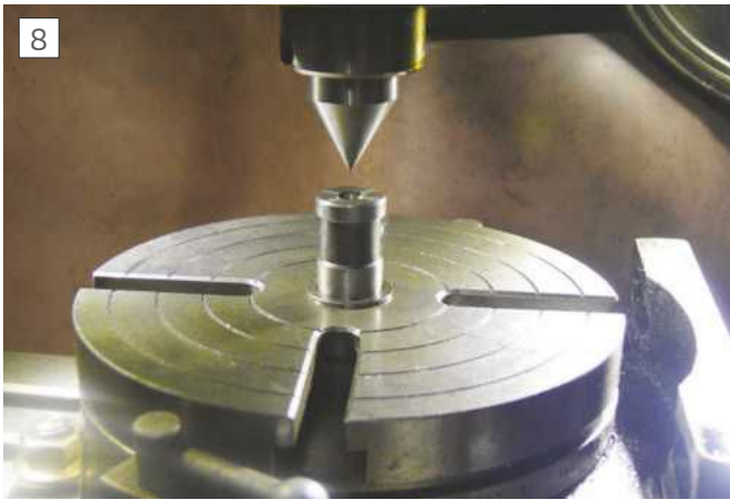
Aligning using the arbor and one of the plugs
