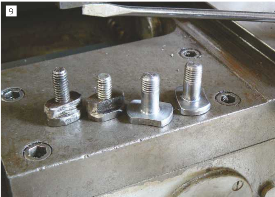
Compound nuts (as found on the left; replacements on the right)
