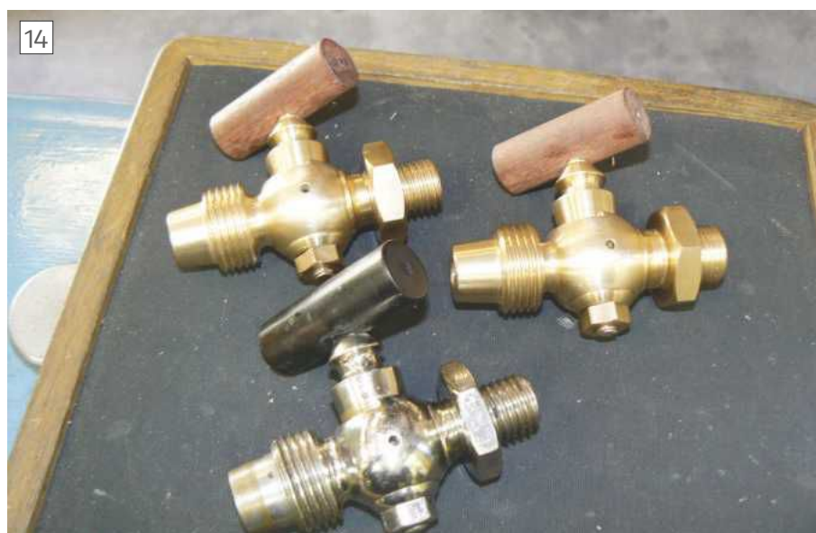
Gunmetal valves for a steam indicator
