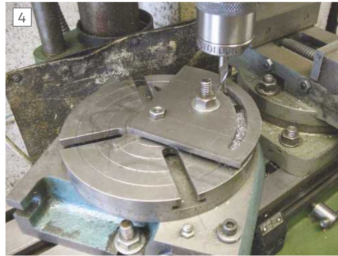
Milling the radius slot for the hinges
