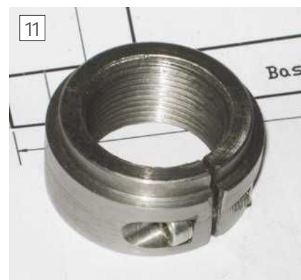
Split spindle nut for adjusting axial play
