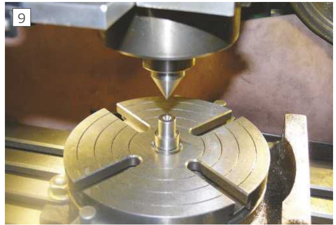
Using a centre-drilled arbor
