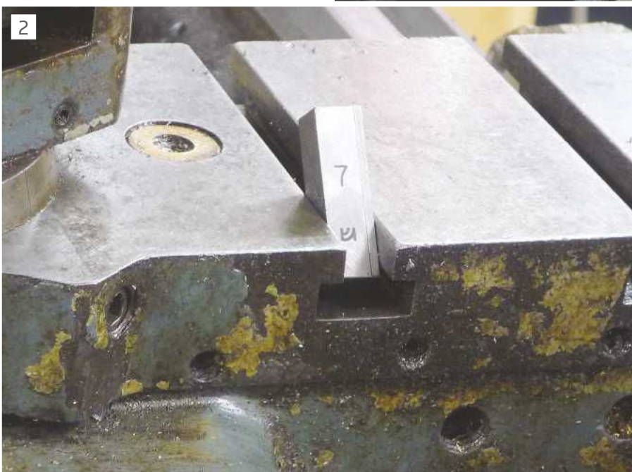
Measuring Cross-Slide Slot Width Using Slip Gauges
