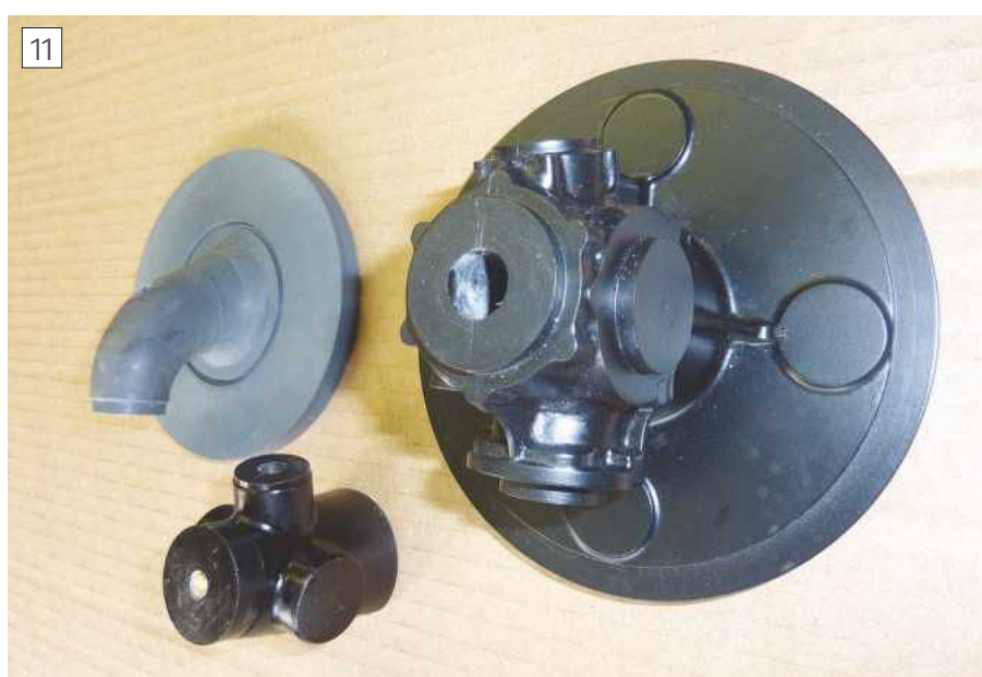
Master pattern and 2 cores for rear cover plate.
