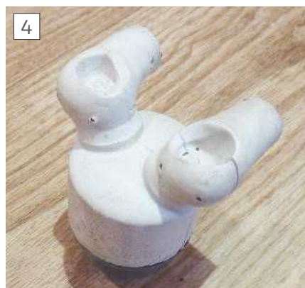
Soft rubber core cut into 3 parts. Made from Shore A 25 hardness silicone.
