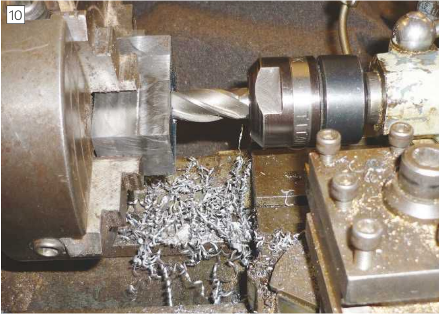
Opening out Guide Hole Using an End Mill
