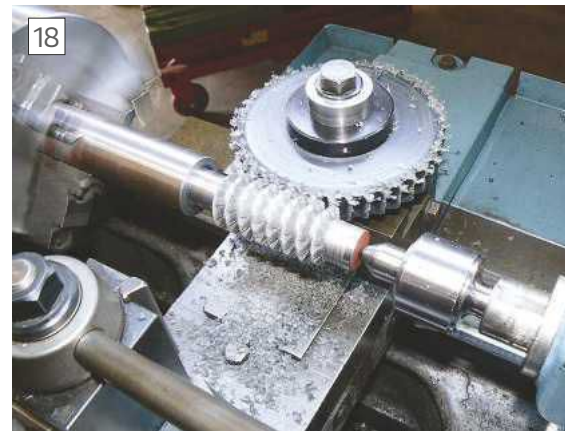
Hobbing a replacement worm gear for a bandsaw gear box
