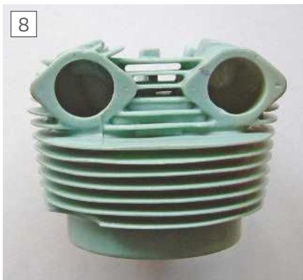
Typical wax casting. Note air bubble at lower left.
