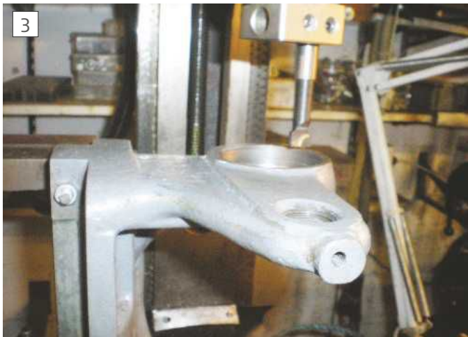
Starting the boring operation
