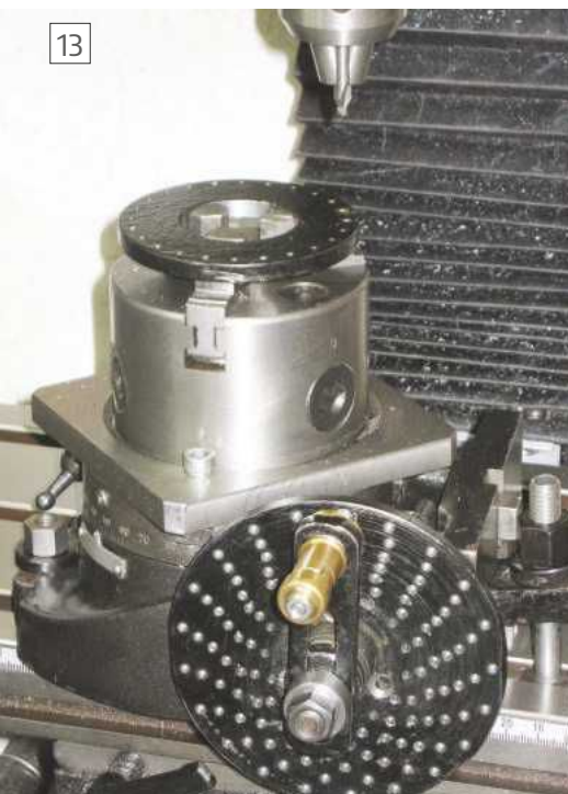
Drilling the 24 hole indexing plate
