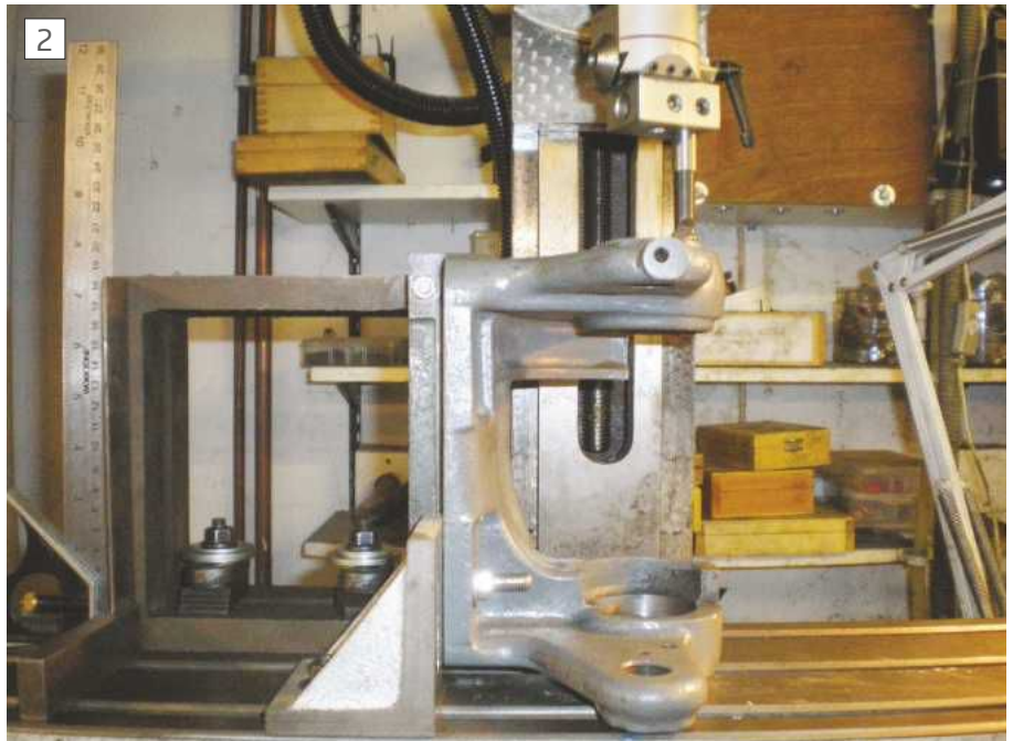
Set up for boring headstock
