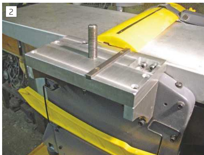
The base plate with pocket for attachment screws
