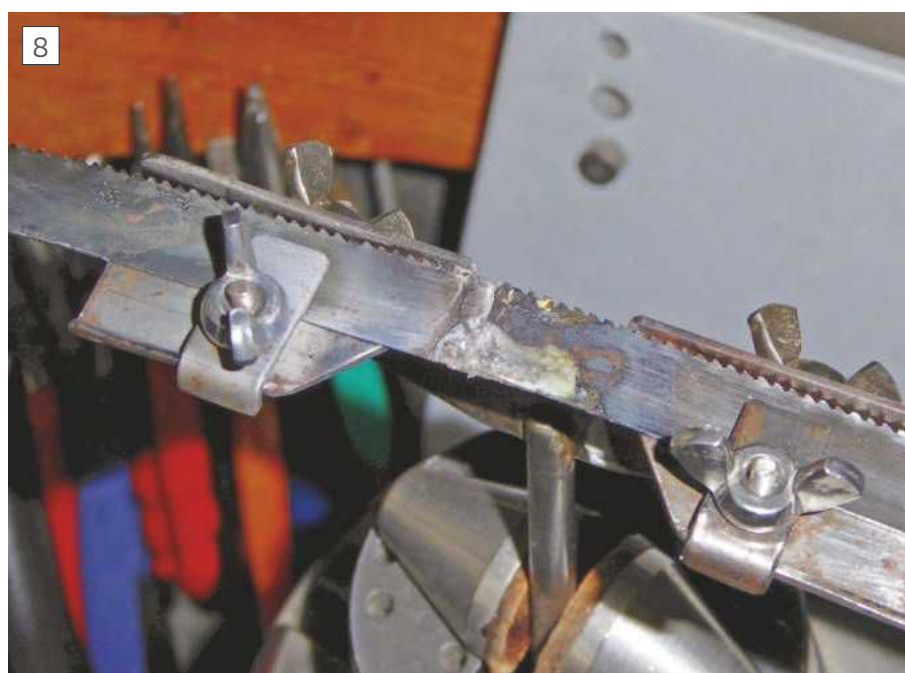
Insert a small piece of silver solder between the blade ends as shown in photo 7 . (I used a little rectangular piece of sheet solder.)
