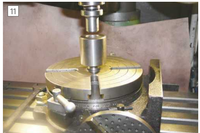
Making use of the vertical alignment fixture in horizontal mode
