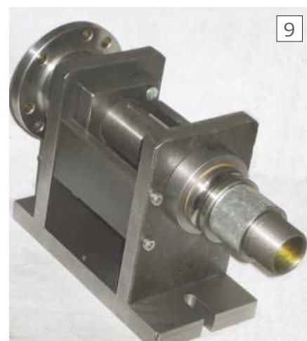
Spindle brake mounted, and a piece of tube as a spacer
