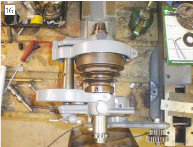
Cast iron guards fitted
