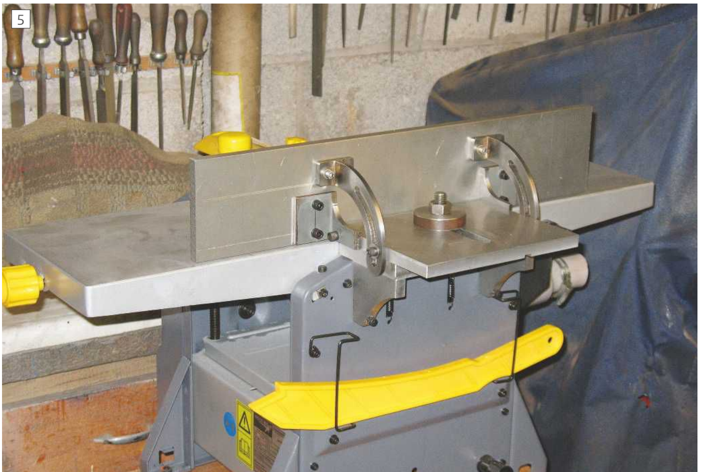
A rear view of the assemble fence
