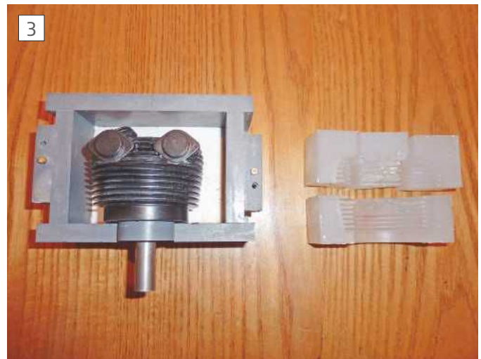
Left – ready for first rubber pour. Right – the result cut into 4 chunks. Rubber could have been saved by blocking out the box corners.
