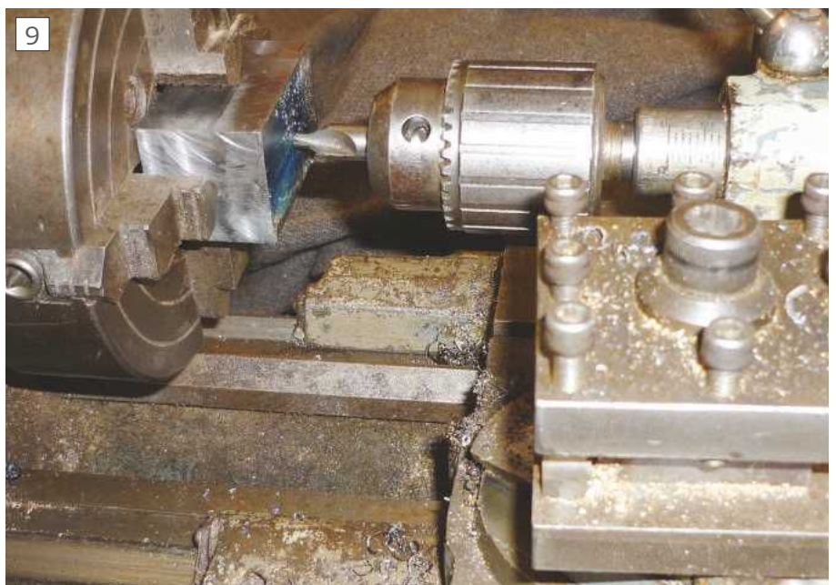
Drilling the Guide Hole
