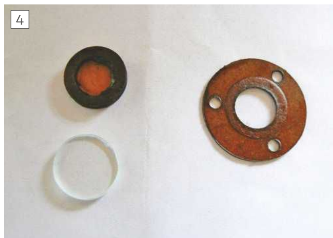
Gearbox sight glasses – old (top) and new (btm)
