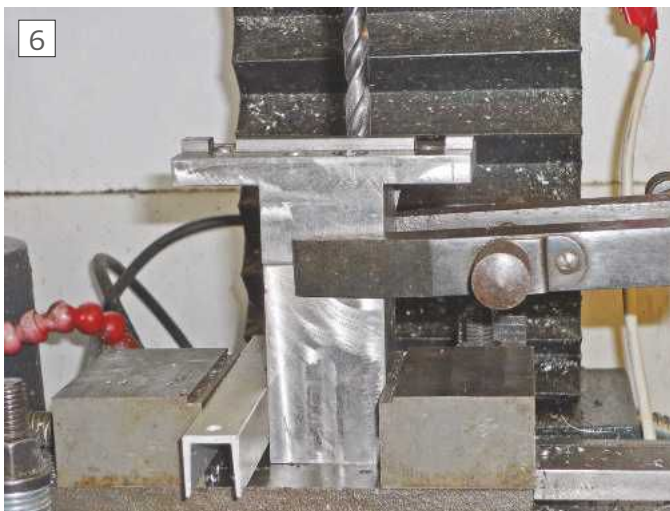
Spotting Base Holes into Column
