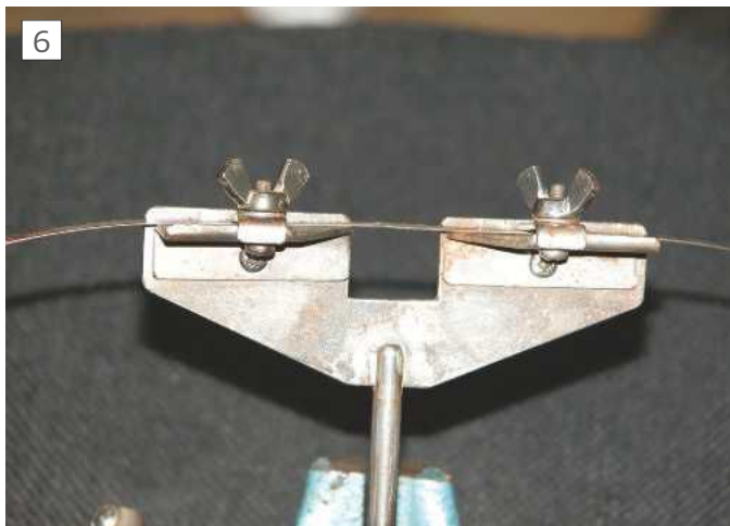
Adjust the clamps until the scarf joint fits nicely under a little tension, as shown in photo 6 .
