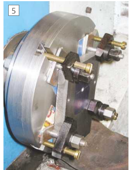
Rough boring the uprights
