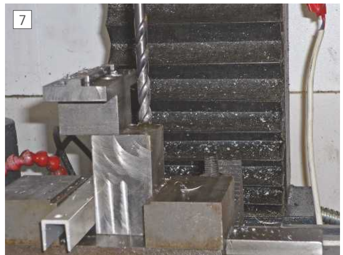
Drilling Out Spotted Hole
