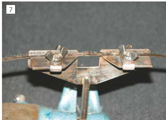
Insert a small piece of silver solder between the blade ends as shown in photo 7 . (I used a little rectangular piece of sheet solder.)
