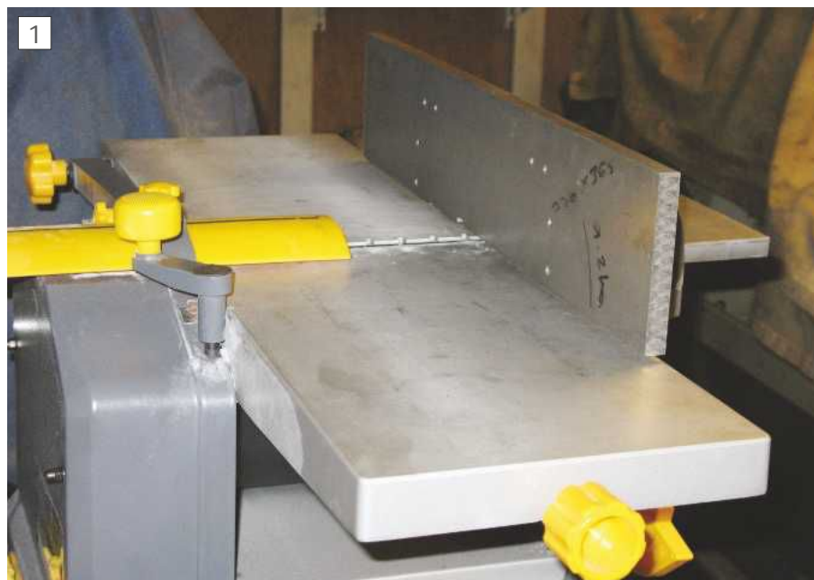
The new fence in position on the table
