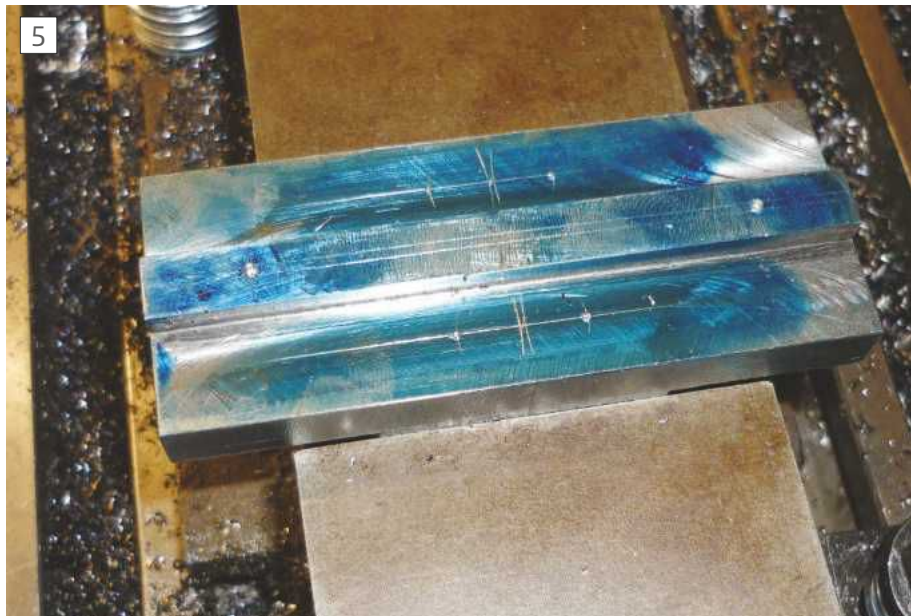
Base Holes Marked Out
