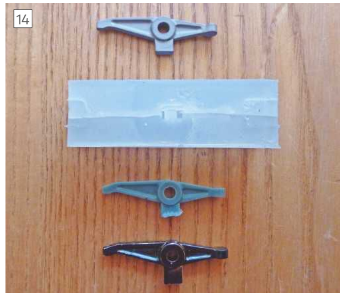
Valve rocker. Master pattern at bottom with a wax above. Split rubber mould. High tensile stainless steel casting at top.
