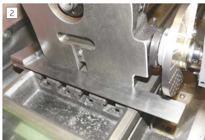
Aligning using a square
