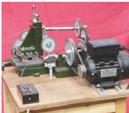
Christopher Robinson explains the use of a Jacobs-type gear hobber
