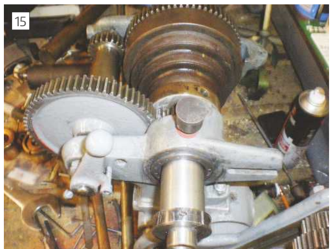
Back gears and pulley in situ
