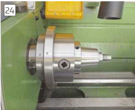
Lining up the line-up marks
