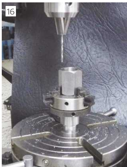
Drilling tapping size for the Thread Adaptor mounting holes
