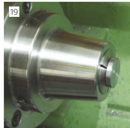
Adaptor reversed and faced off
