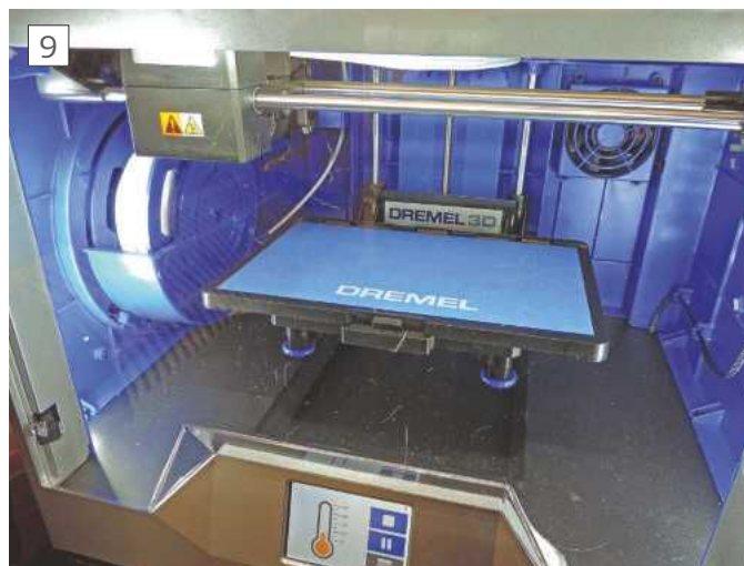
The printer warms up, note that a sheet of build tape has been applied
