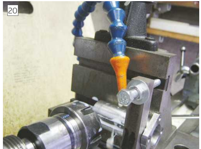
Grooving the sleeve on the lathe to take the key
