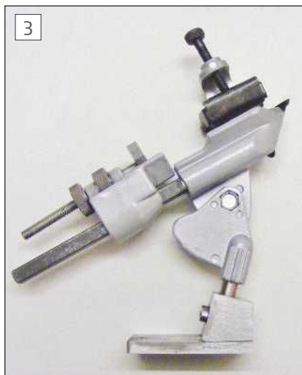
The drill grinding jig with the base modified
