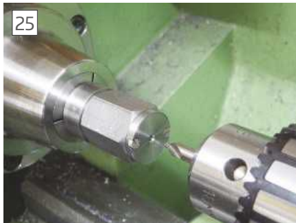
Machining the centre for accurately positioning the desired thread core size drill
