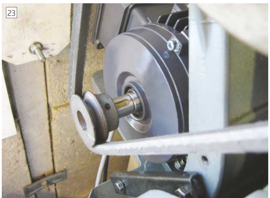
New motor mounted on the lathe motor platform
