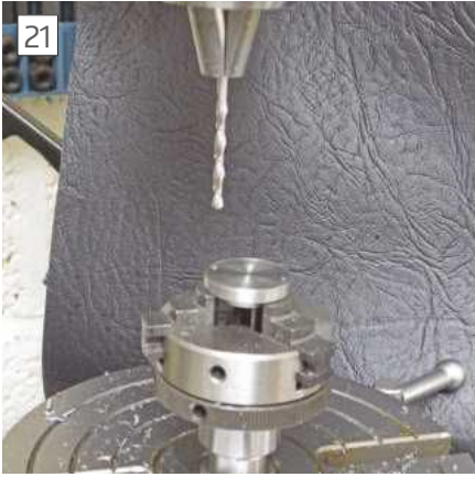
Drilling the Thread Adaptor mounting holes
