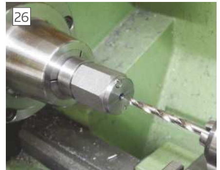
Machining the core size of the desired thread
