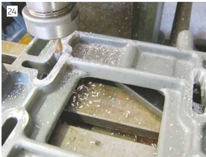
Extending the lathe motor support platform slots
