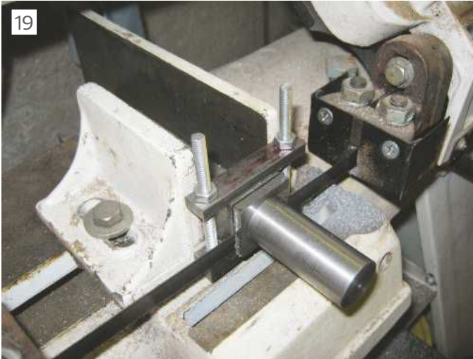
Unbored sleeve being parted from the excess stock
