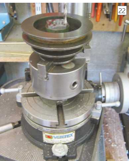
Drilling the sleeve flange for bolting onto the pulley
