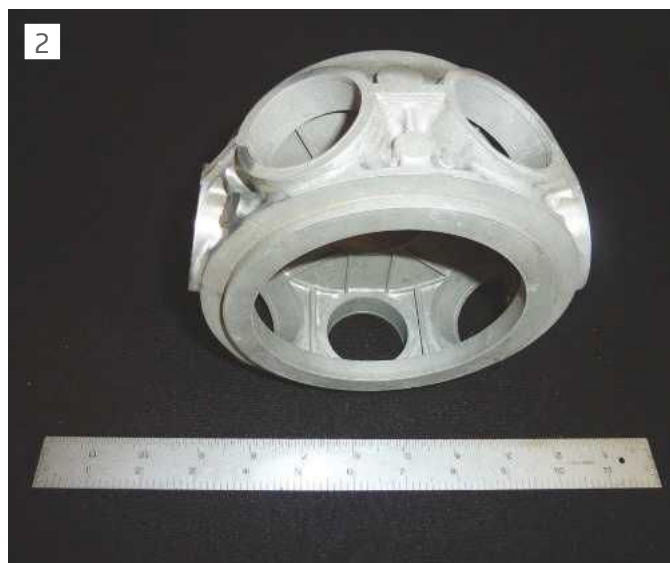
The crankcase from rear. Notice the various stiffening ribs.
