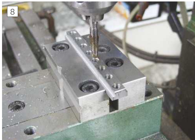
Before removing the tee-nut from the vice it is best to tap the thread for the stud so that it is square to the working face - example only
