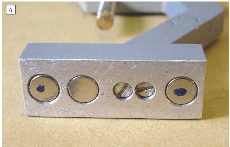
The base, showing the magnets.
