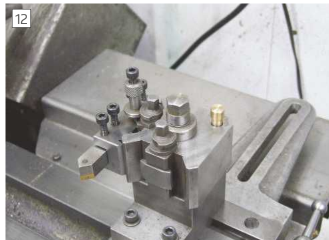
A chamfer tool set in a standard toolholder
