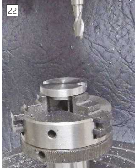
Counterboring the Thread Adaptor mounting holes
