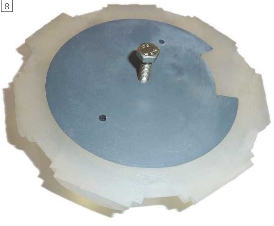
A finished positive ready for the foundry. The kernels have a taper to make withdrawal easy and saved about £40 in total!
