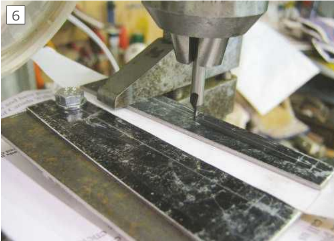
Set up for drilling rivet holes
