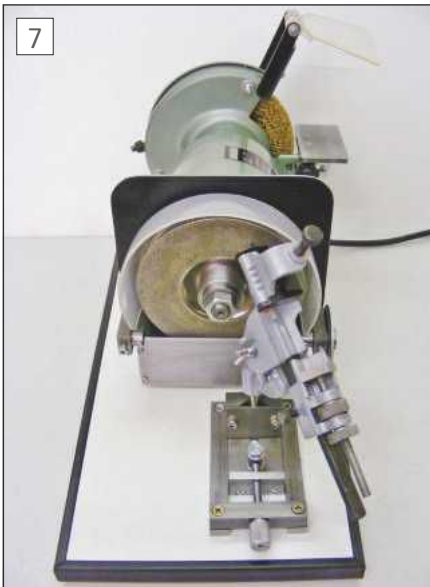
This shows the grinder set up for drill sharpening
