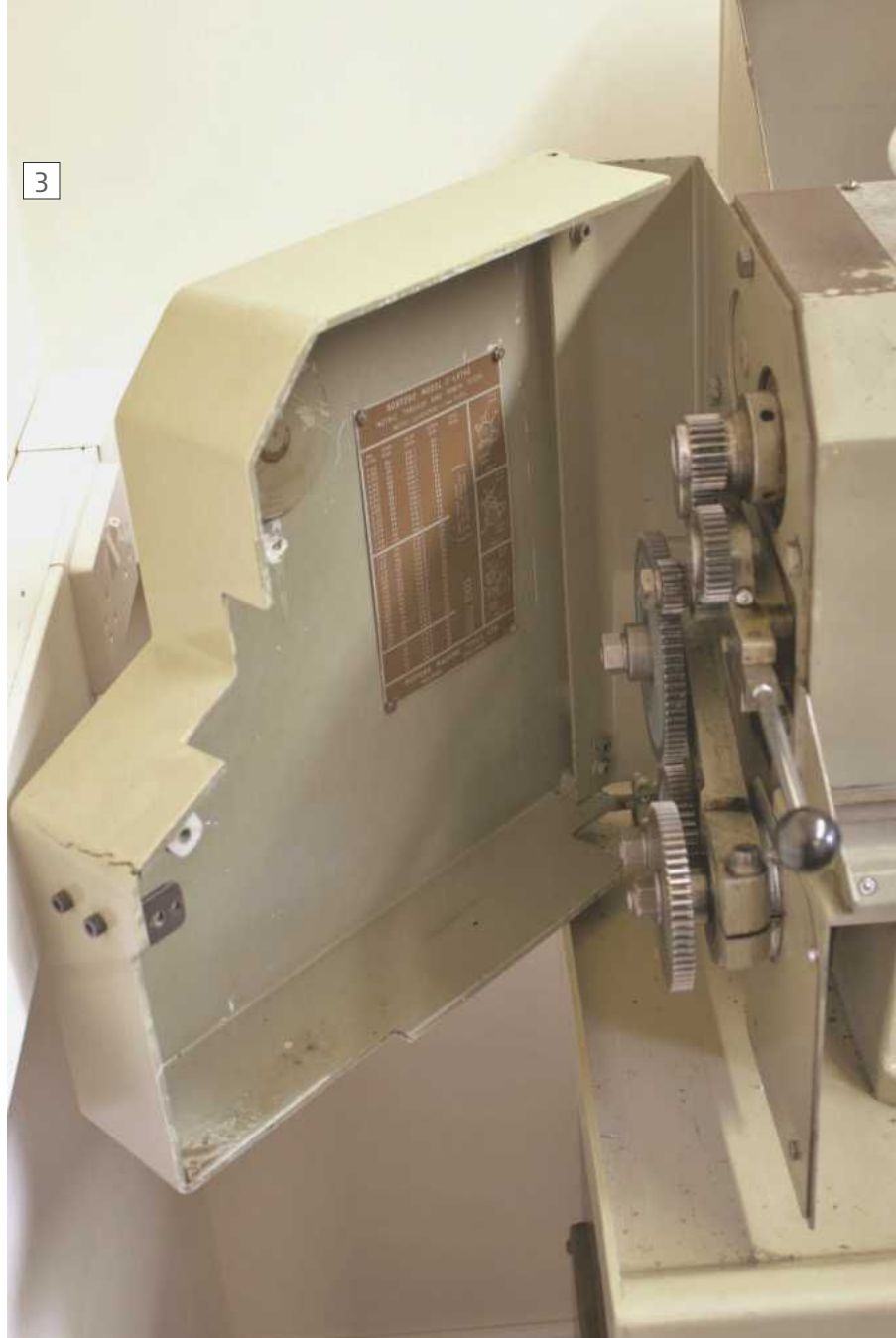
Change gear cover open to show gears
