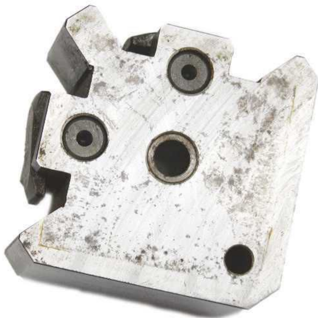
The bushing fitted into the toolpost
