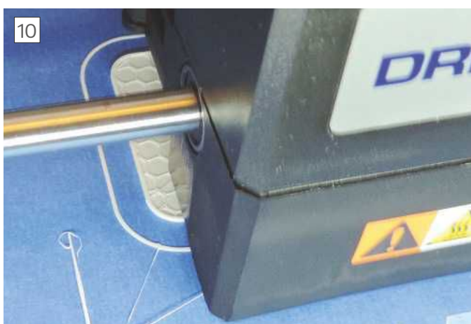
The printer starts up- by drawing a 'skirt' around the part, then building the part up in layers. The loose material at bottom left is some I should have removed from the extruder after I set up the printer
