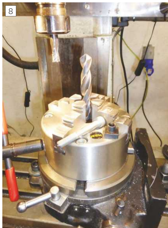
125mm chuck mounted on 6 inch rotary table
