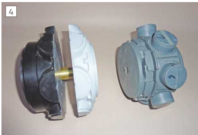
Main pattern on left, core pattern on right. Both are in two sections needing radial registration.
