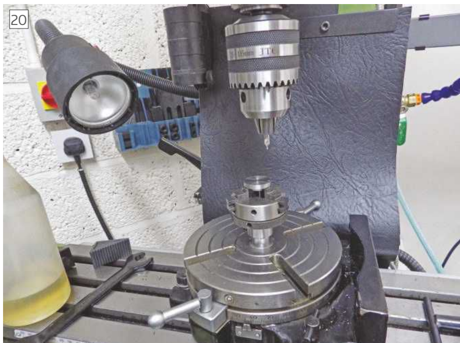
Centring the Thread Adaptor mounting holes
