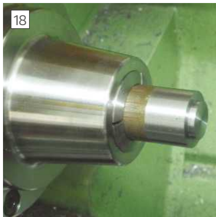
Early stage in machining the adaptor
