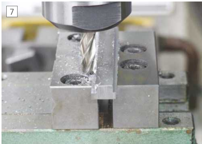
Finish machining the shoulders on a tee-nut to the same 'depth' on each side - example only
