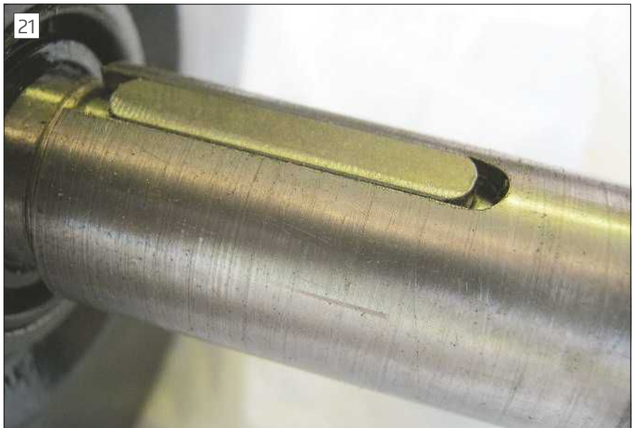
Sleeve in place on the motor shaft with key inserted in keyway
