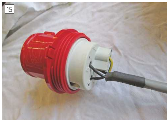
15 Use of heat shrink sleeving
