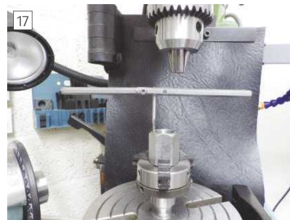
Tapping the Thread Adaptor mounting holes
