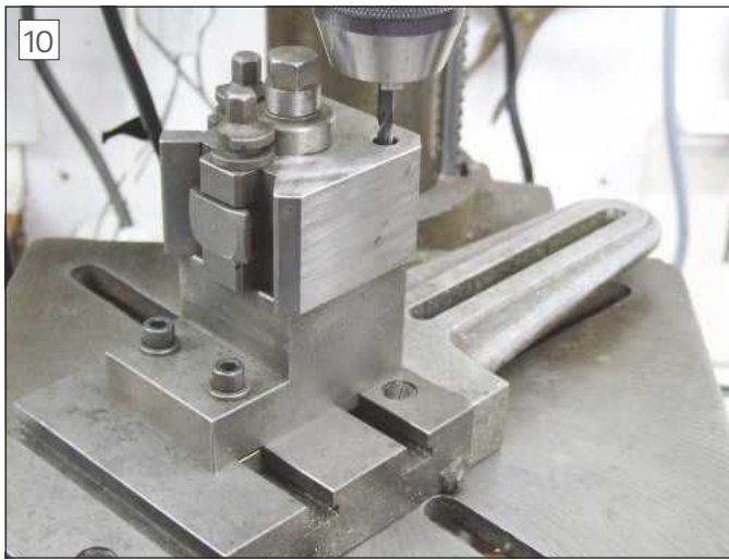
Drilling for the setting pin (posed photo)
