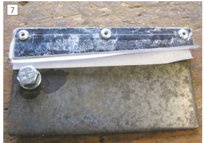
One side of mounting bracket riveted up
