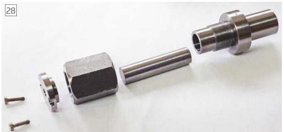
Component parts of a standard Universal Screw Modification Fixture ready for assembly
