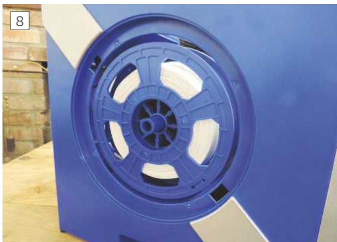
Dremel's 500-gram reels of PLA fit into the side of the machine, behind a twist off cover
