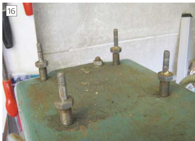
16 Original mill mounting studs
