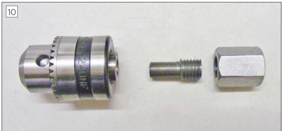
The chuck, threaded adaptor and shortened connector nut
