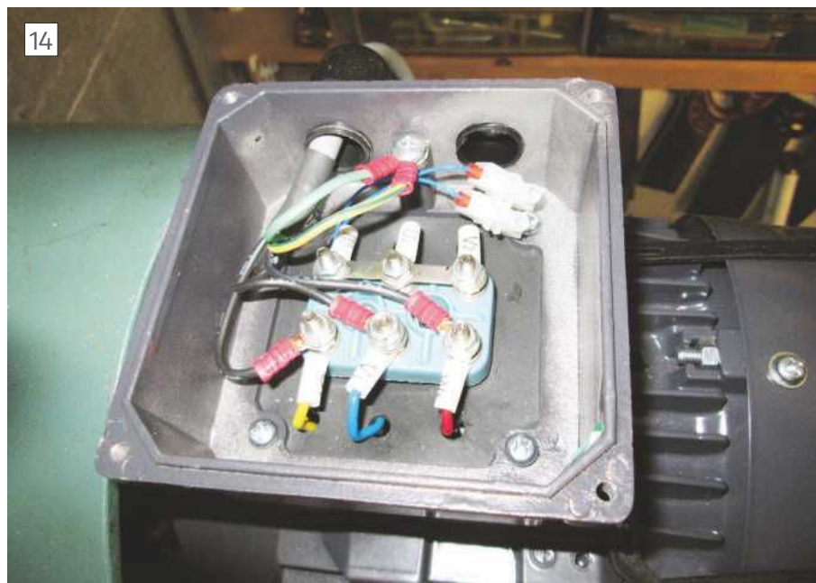
14 Screen and earth connected to earth
