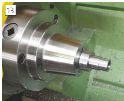
Housing mounted in a collet chuck
