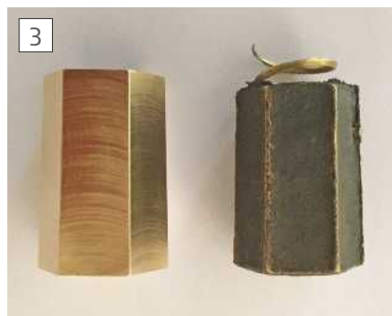
The old and new 'nuts' side by side.
