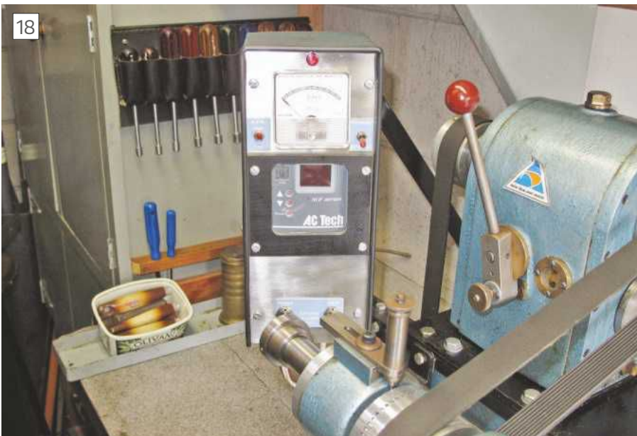
VFD drive control system for lathe G
