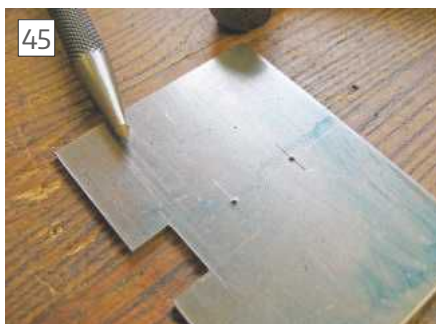
Next the two counter sunk 3.2mm holes were marked and centre punched, photo 45 .
