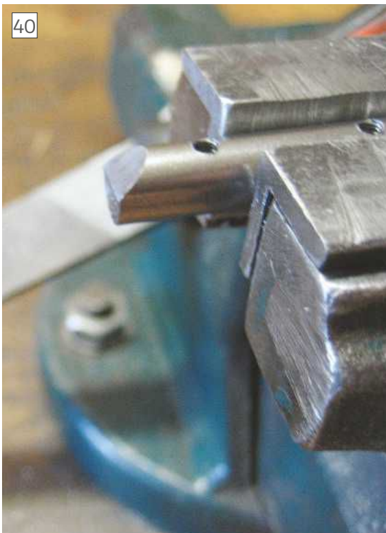
Finally, the 4 x 45° chamfer in one end was filed, photo 40 .
