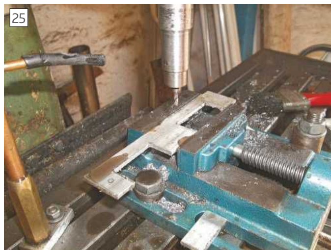
Profiling the new wiper plate
