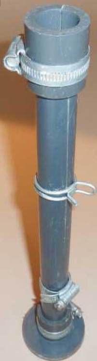
Core box assembled with hose clips ready for sand.
