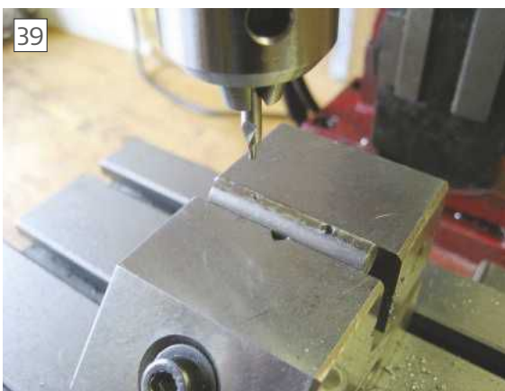
The two M3 tapped holes were drilled and tapped, photo 39 .
