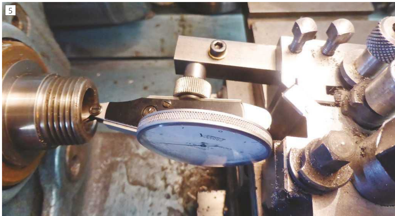
Indicator mounting for Myford MT2 runout
