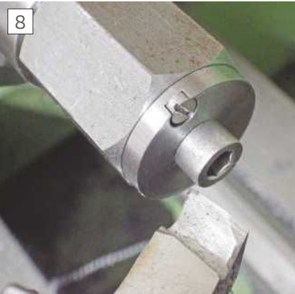
Facing off a Screw Head perpendicular to the screw axis
