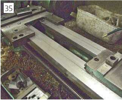
35 Tailstock wiper producing a ploughed clear area
