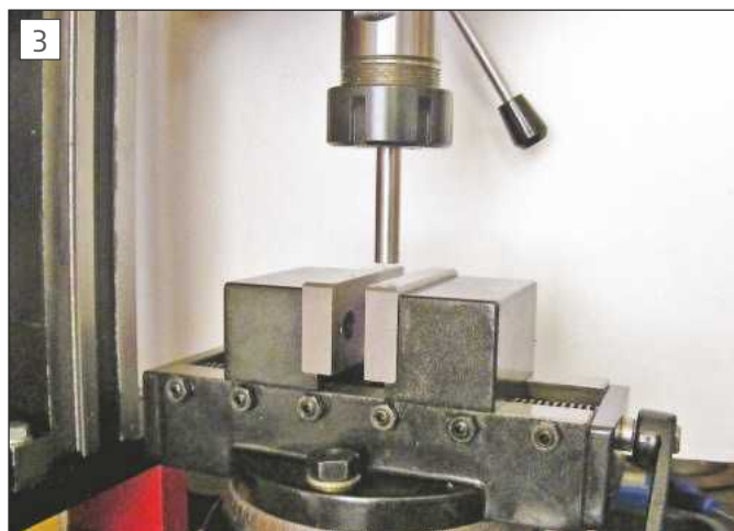
The vice clamped around the silver steel rod.
