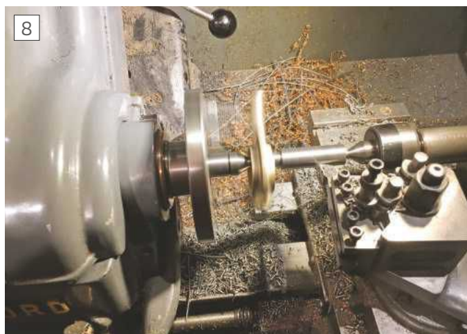
Finish turning a 'long stud' between centres.
