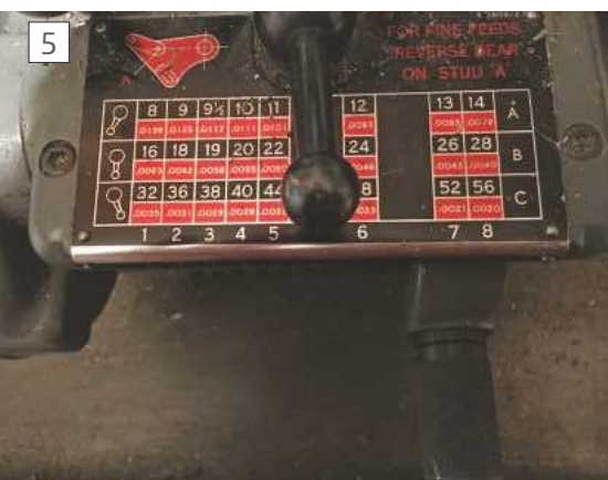
The Myford Gear Box selector plate.
