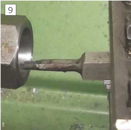
Counterboring the nut
