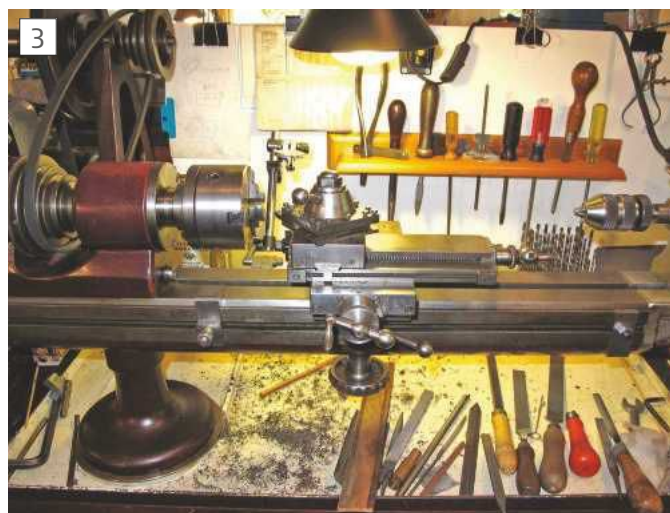
Carriage of lathe A, note the cantilever bed design
