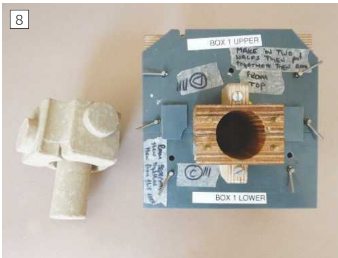
The two halves put together for a final ram. Notice the founder's notes to herself!
