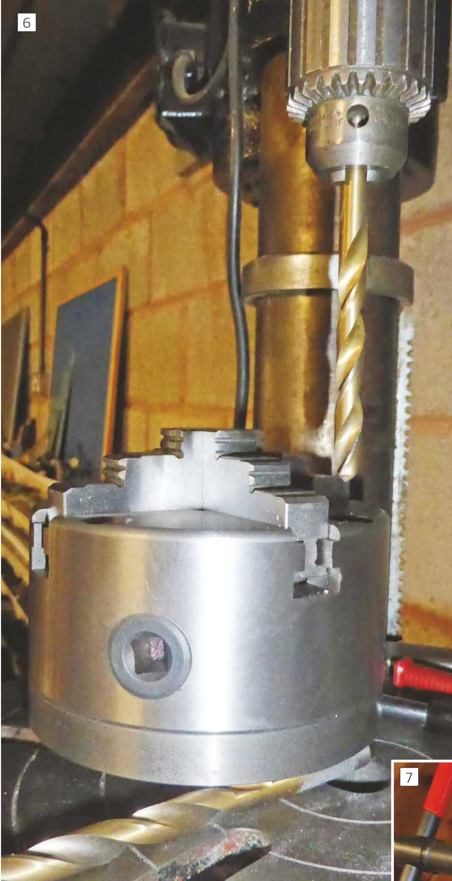
Spotting through chuck onto backplate
