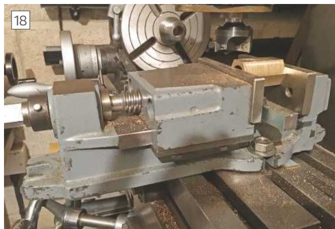
Packing under the front of the vice to generate the necessary taper.
