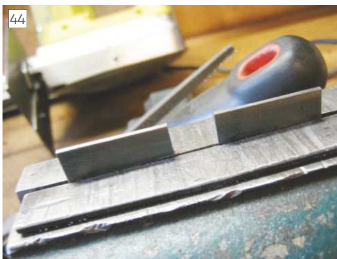
And the final outer shape was finished using appropriate files, photo 44 .
