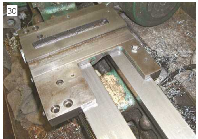
Rear of carriage showing area for new wiper
