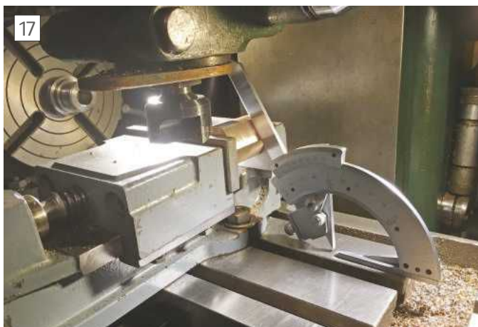
Milling a parallel hexagonal side and setting the angle for the next side.
