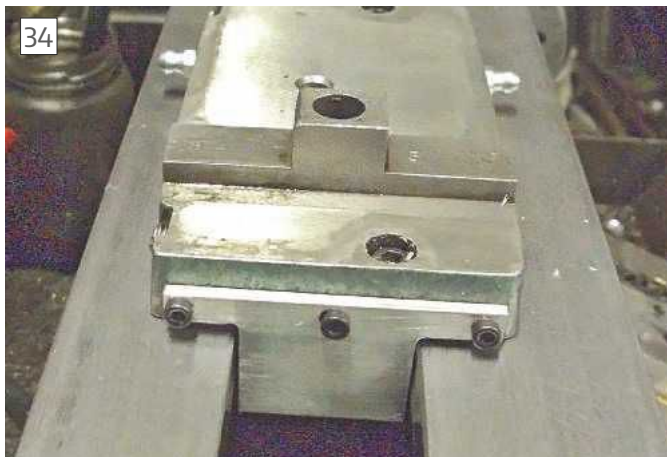
Tailstock wiper in place
