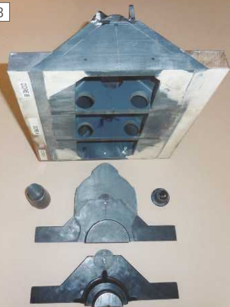
Another view. The wood side blocks form prints for the external bracket cores.
