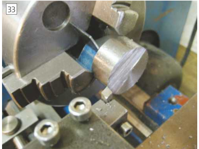
Next the part was cut a little oversize with a hacksaw and the part was faced off to a final dimension of 12mm in width, photo 33 .
