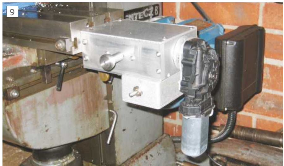
Finished power feed
