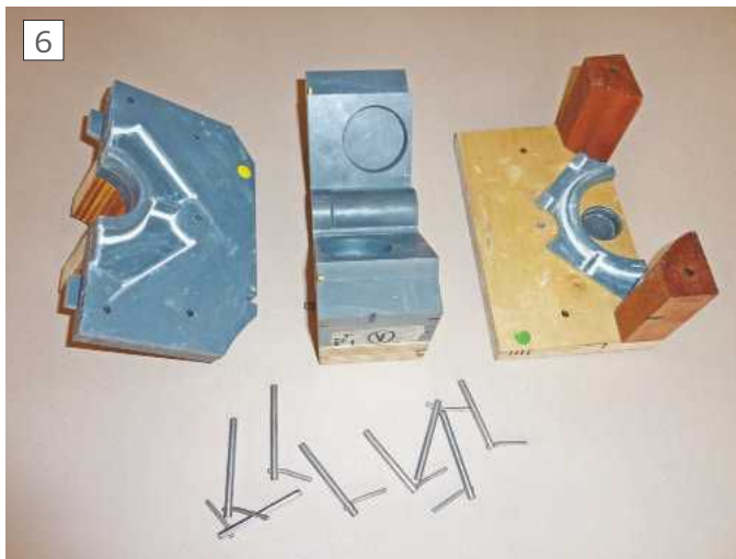
One of the main core boxes. This one is in two halves to make ramming easier.
