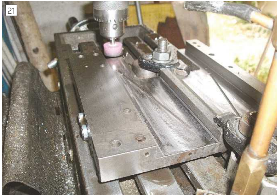
Finish ground carriage
