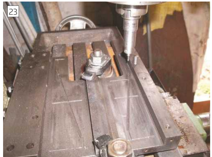
New oil grooves cut in carriage
