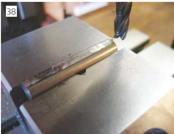
This bar was made from 8mm free machining steel. After cutting off the bar a little over size according to the measure in the drawing and faced off to final length in the lathe, the part was taken to the mill and the upper face was milled, photo 38 .
