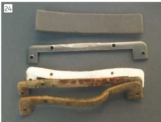
Carriage front felt wipers and cover
