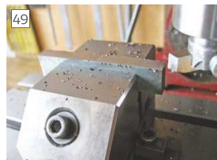
After a rough cut out, the part was milled to correct outer measurements according to the drawing, photo 49 .
