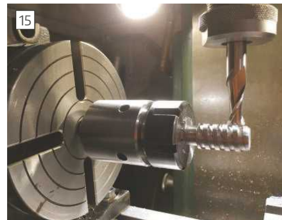
Milling the teeth into the tap.
