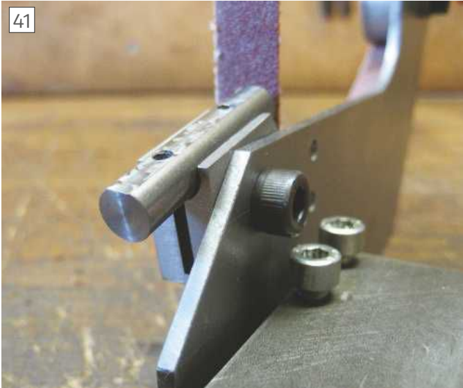
The bar was mounted in the grinding plate bracket and the adjusting and locking function could be tested, photo 41 .
