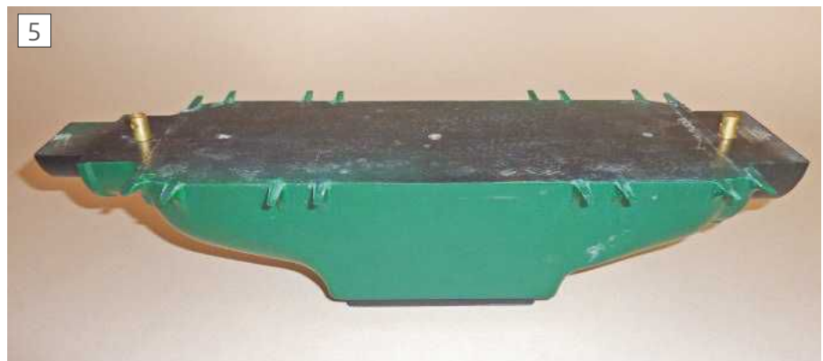
Lower half of pattern. Made chiefly of wood laminations with PVC core prints at each end. The 16 little buttresses are also plastic. Each one is given draft.
