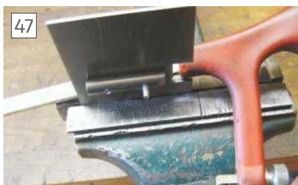
Finally, the grinding plate was assembled with the adjusting bar and the counter sunk screws were cut and filed off, this to make sure they weren't protruding from the adjusting bar, this way the bar would slide smoothly in the adjusting bracket, photo 47 .
