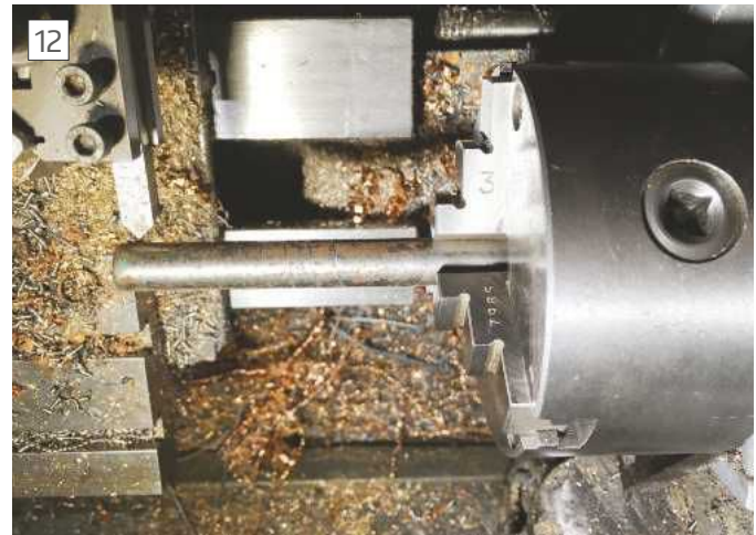
The test piece confirming 4tpi.
