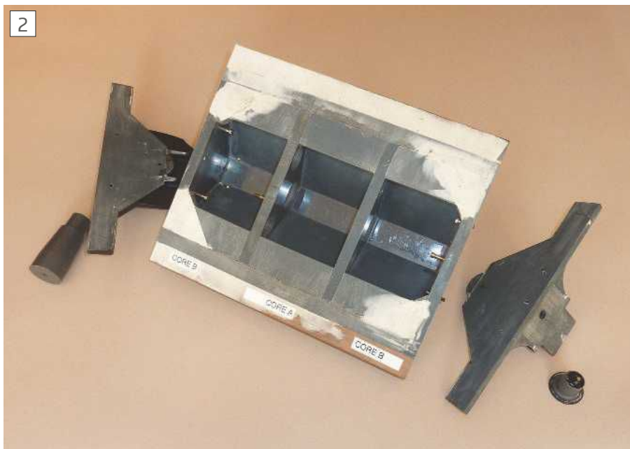
The 5 parts of the upper half of the pattern. Constructed mainly from 12mm PVC plate.
