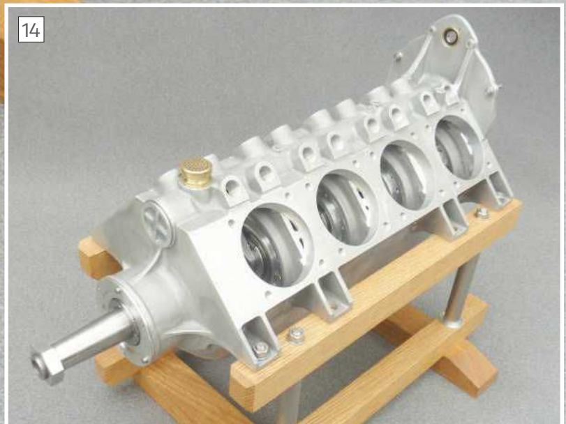
The ENV engine crankcase finished.
