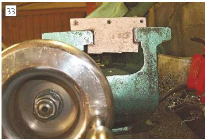
Tailstock wiper in end of bed to check the fit
