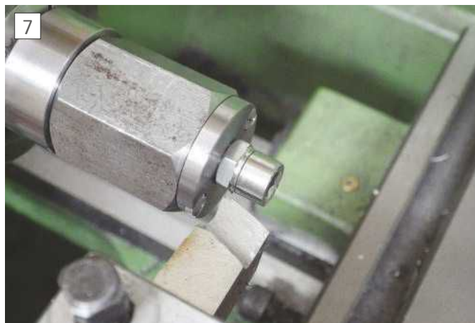
Set-up showing the modification of a screw Head together with a Nut being modified with a washer face
