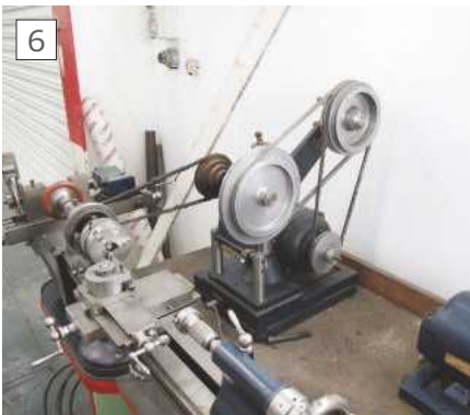
Drive arrangements for lathe D
