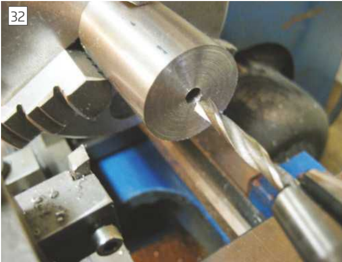
This part was made from 30mm diameter free machining steel. First, the M6 tapped hole was drilled and tapped in the lathe and the 6.5 clearance hole was drilled, photo 32 .
