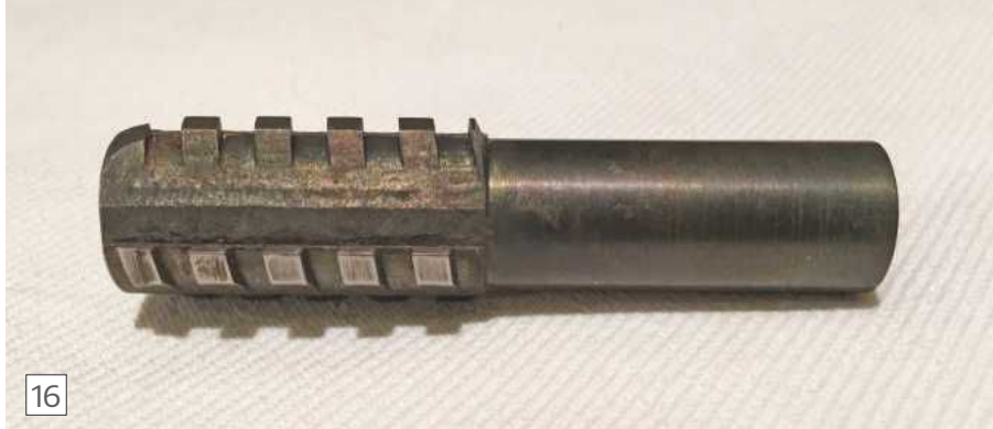
The finished tap after hardening and tempering.
