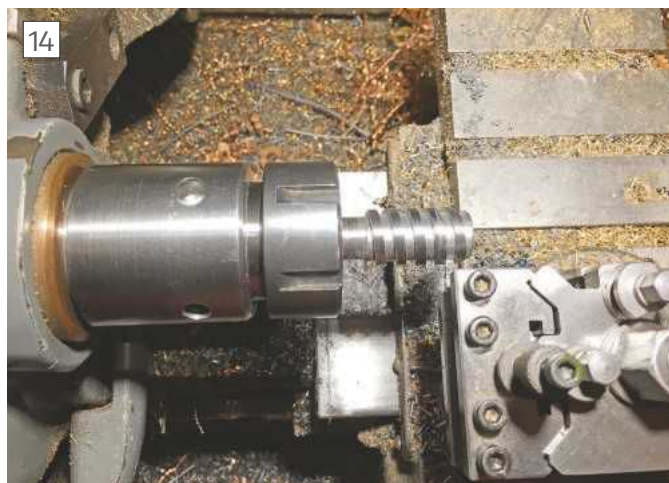
Screw cutting the 4tpi tap.
