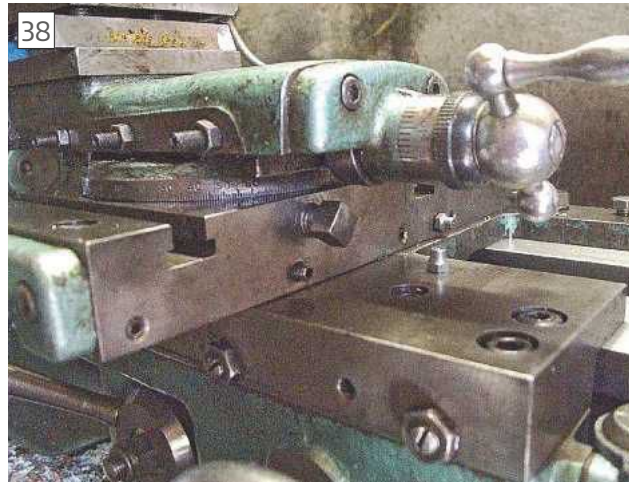
38 Cross slide front locking screw
