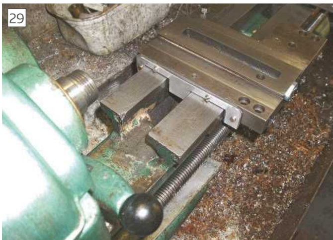
New wiper fitted to carriage front
