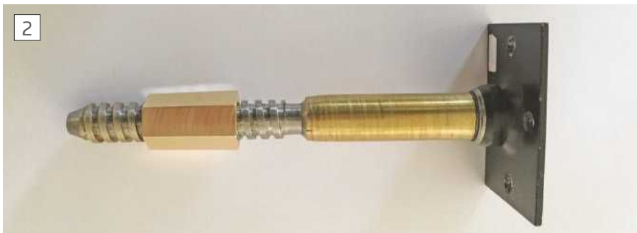
The 'Leadscrew' with the new 'nut' finished and fitted.
