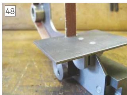
The grinding plate was mounted to the grinding tool and the function of adjusting the plate in accordance to the grinding belt could be tested, photo 48 .
