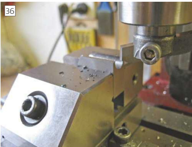
The part was turned over in the mill vice and the next face was milled according to the drawing, photo 36 .
