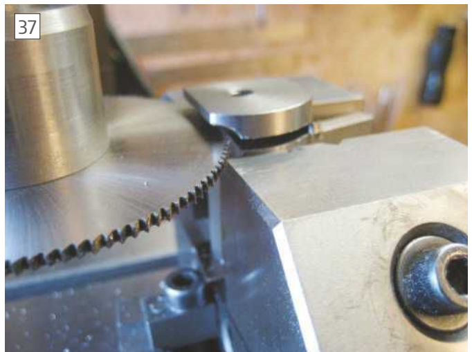
Final job on this part was to mill out a 2.0mm wide slot, this slot would enable me to lock the grinding plate in any wanted position when using the tool, photo 37 .
