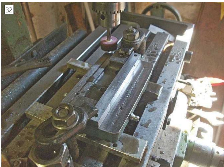
Grinding tailstock base plate
