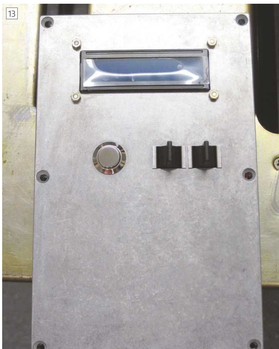
Front panel of control unit showing LCD, paddle switches for menu navigation and select button.
