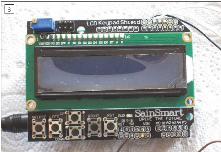
Arduino compatible LCD and Keypad shield.
