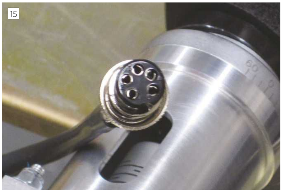
Multi pin locking plug connected to stepper motor.
