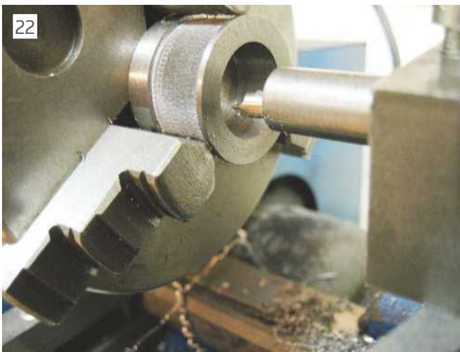
Then the ring was bored to final inner diameter and depth using a boring bar in the lathe. Again I aimed for a diameter 0.02mm under nominal measure to obtain a light press fit with the ball bearing, photo 22 .
