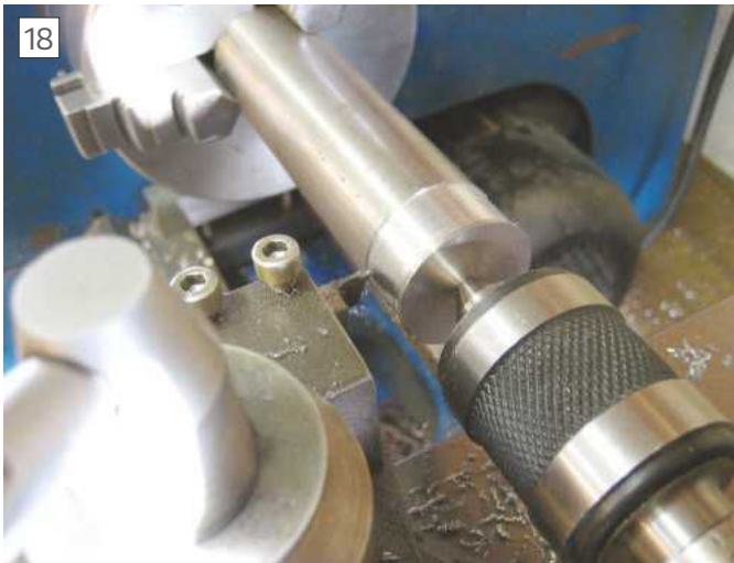
This wheel was made from 30mm free machining steel. First job was to face off the steel bar, make a centre hole, and changed to a special narrow grinded toolbit, so I could turn the 28mm section, photo 18 .
