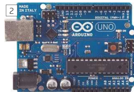
Arduino Uno microcontroller board. Note USB programming connector and I/O port headers.
