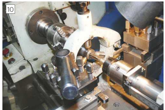
Using a home made floating reamer holder
