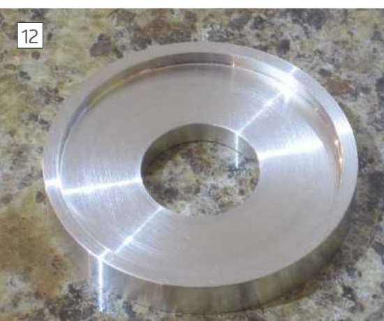
Round portion of mount showing register bore for rotary table mounting and counterbore to suit cylindrical section.
