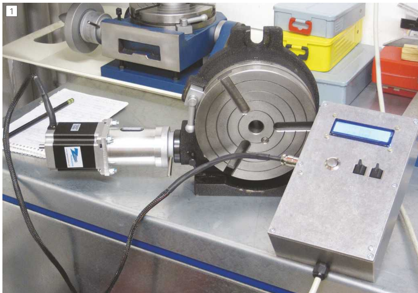
Completed Arduino Indexer showing control unit and motorised rotary table.
