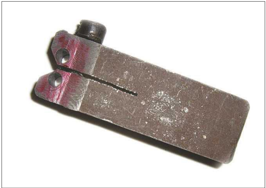
Form tool shank, with adjusting screw
