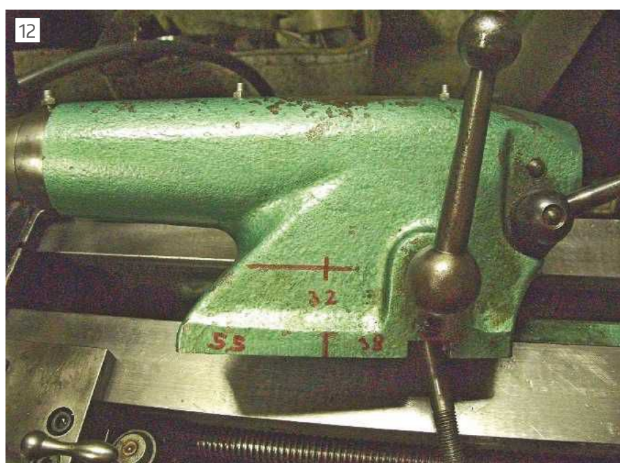
Top casting marked for clamping mechanism
