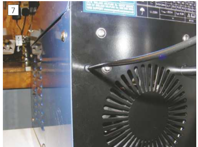
The gas tube emerges from a grommetted hole at the rear of the welder.
