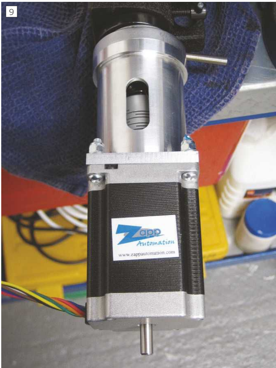
Completed motor mount attached to rotary table.
