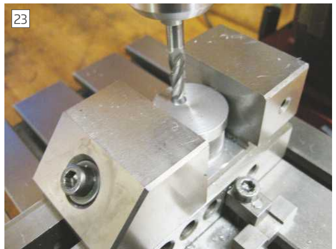
Next the part was placed onto the bed of my bench mill, and the 8mm hole was drilled with an end mill, photo 23 .
