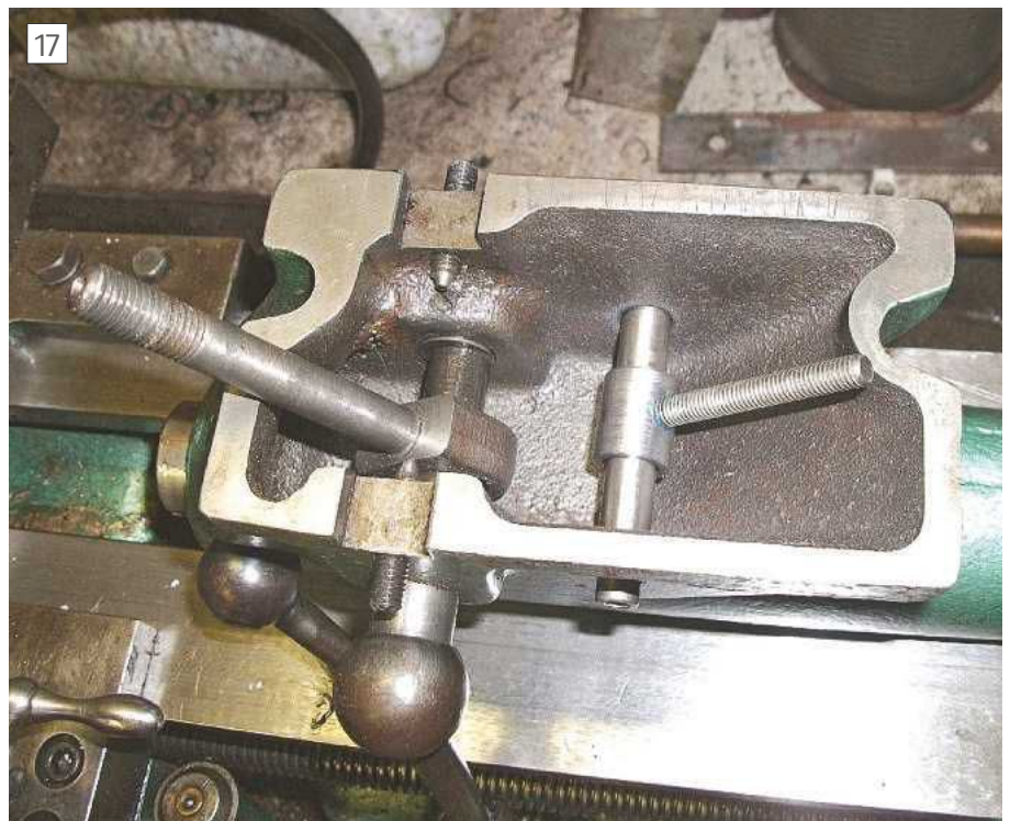
Modified internal clamping mechanism
