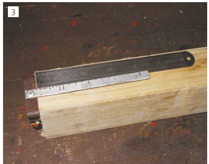
How to set the zero point for graduating
