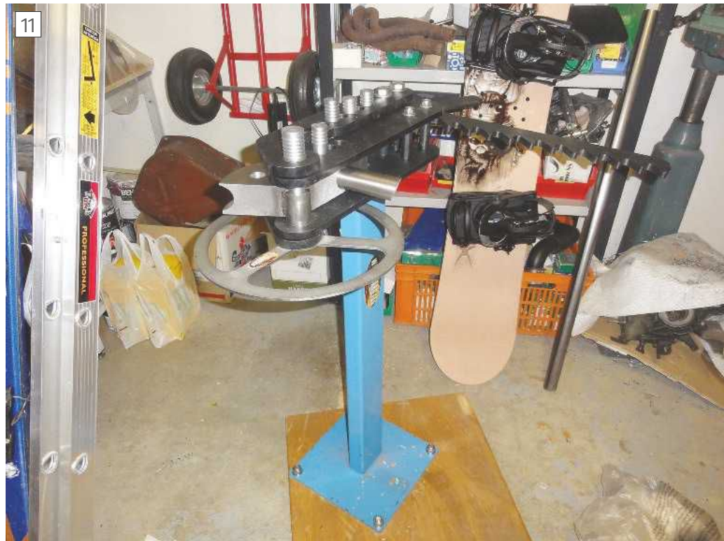
Pipe bending jig
