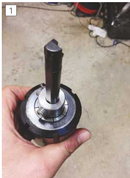
Boring bar in eccentric hole
