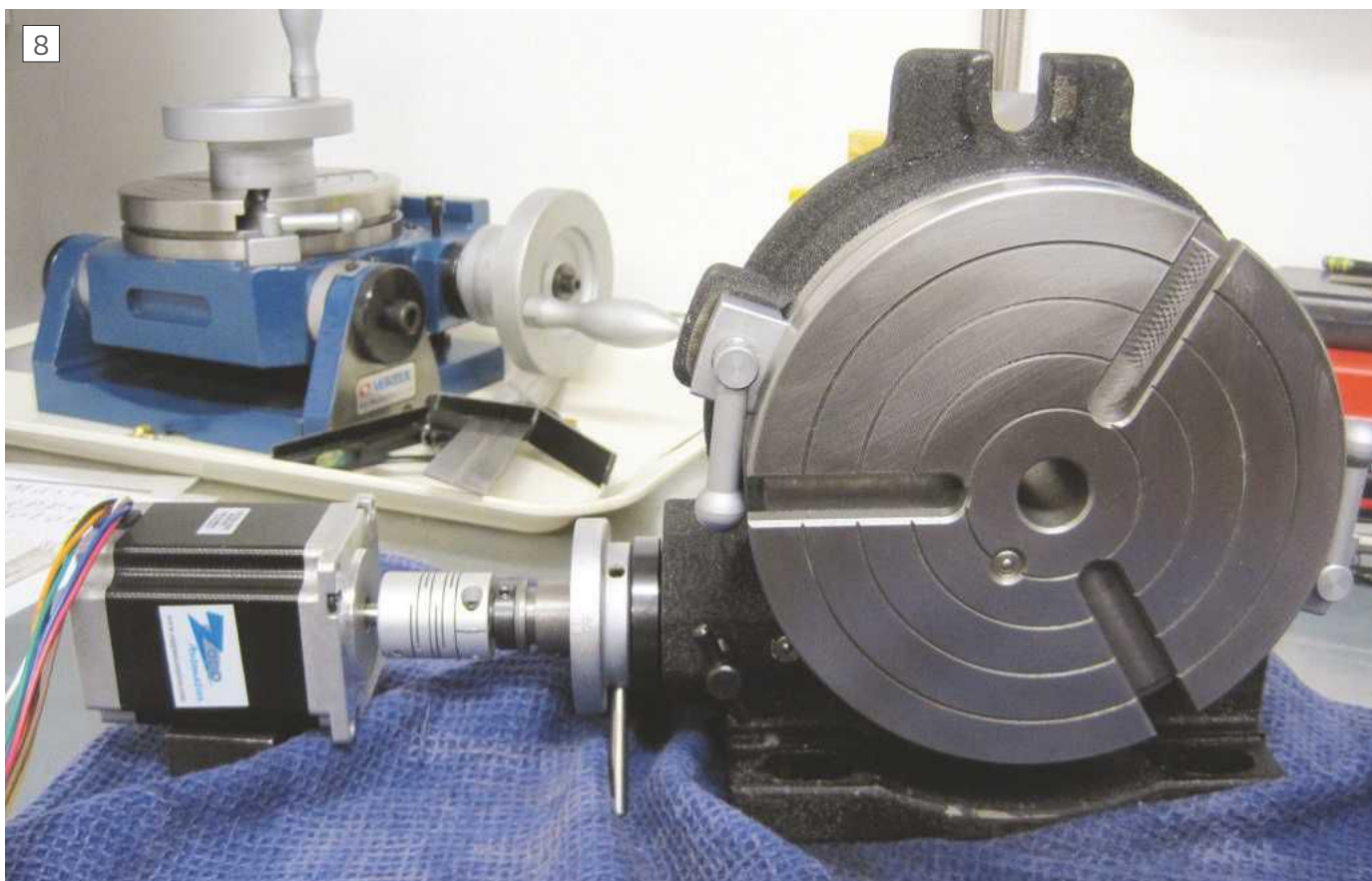
Stepper motor and rotary table connected up with bellows coupling for initial trial.
