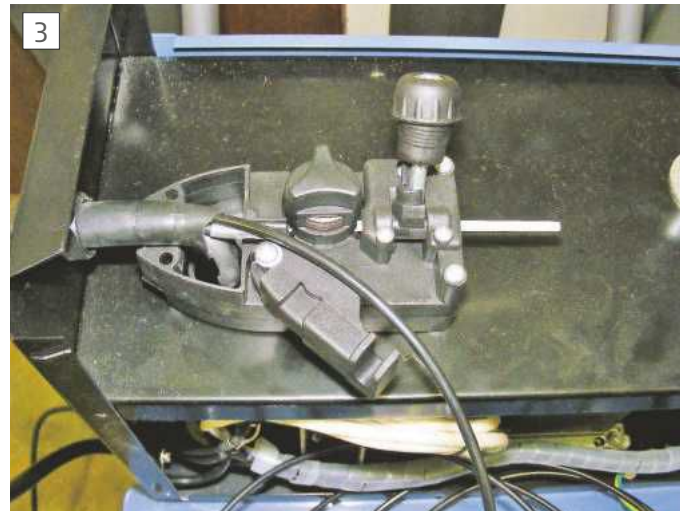
Feeding the gas tube into the sleeve.
