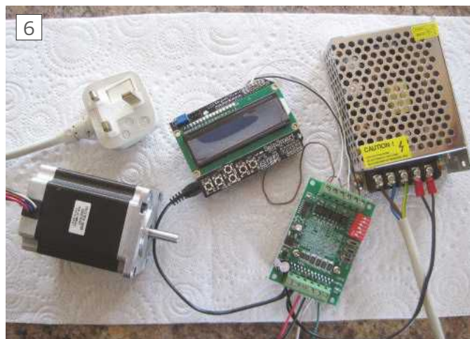
The components connected, the PSU must be fitted in an earthed case before connecting to the mains.
