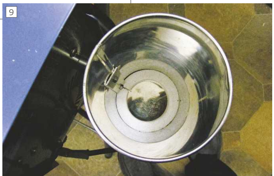
The polystyrene ring to support the bottom end of the cylinder.
