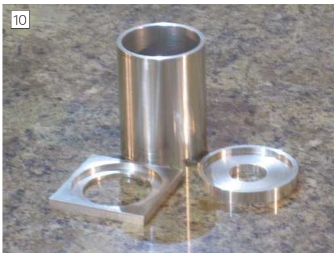
Motor mount components, taken before mounting holes drilled in round portion.
