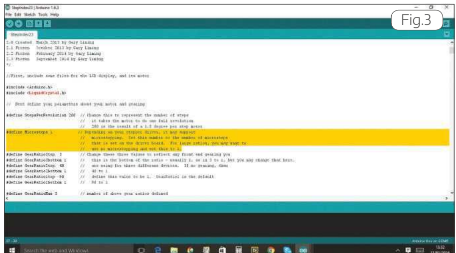
Screen shot of Arduino IDE showing Gary Liming's step index software. Highlighted portion shows constant controlling multi-stepping.
