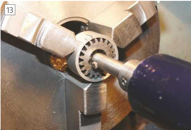
Cutting the keyway in a gear
