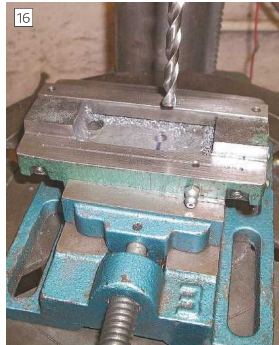
Clamping bolt hole location
