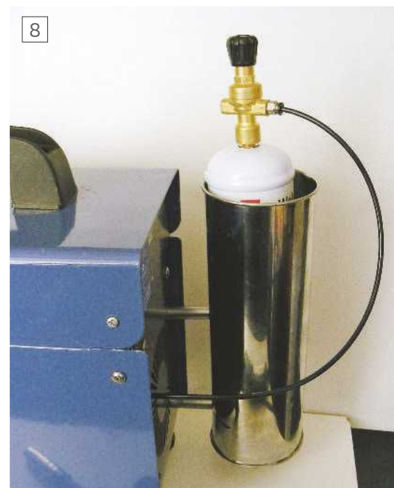
The support for the gas cylinder.
