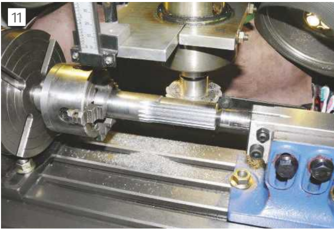
Cutting the gears as a 'stick'
