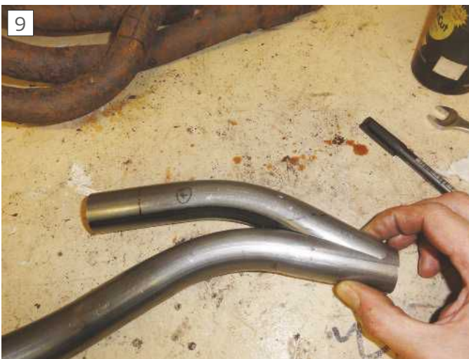
Two pipes joined
