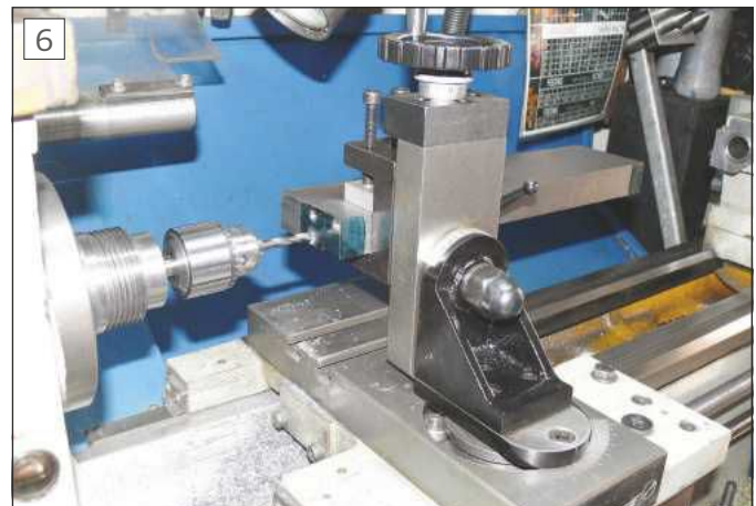
Drilling a hole for a dowel
