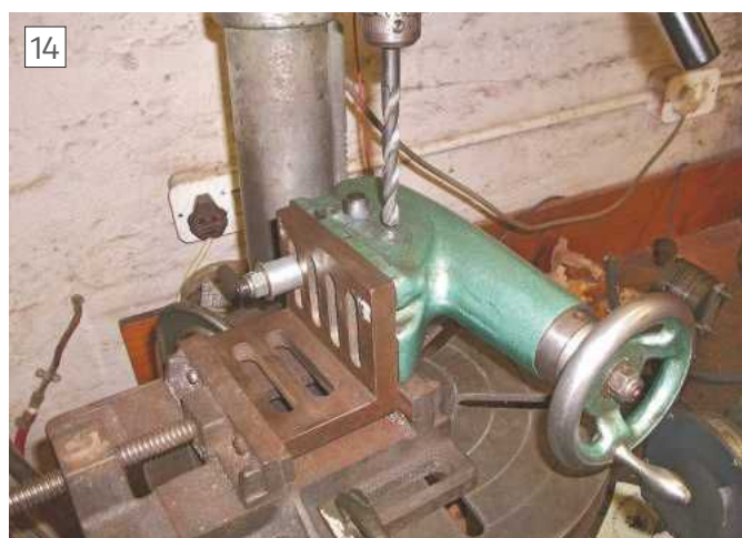
Drilling the clamping rod hole in the tailstock casting
