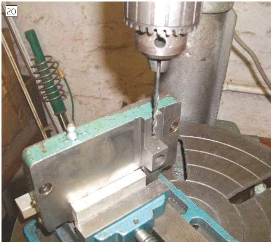
Centre drilling pusher screws position
