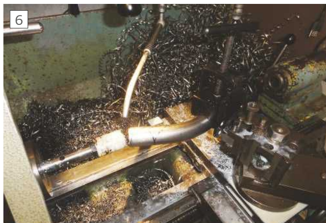
Set-up for notching
