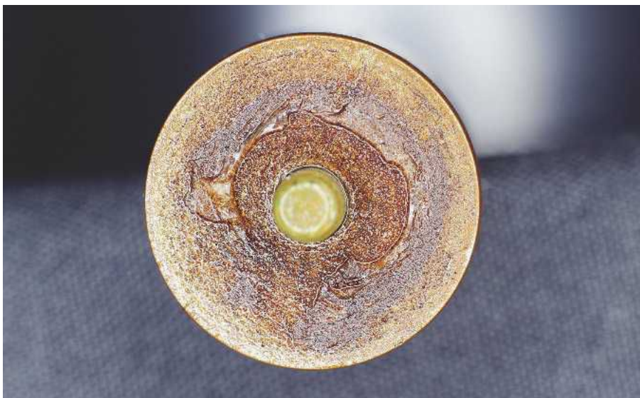
Acid Damaged Piston
