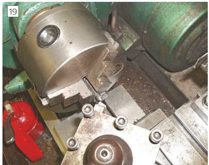
Machining tailstock alignment screws
