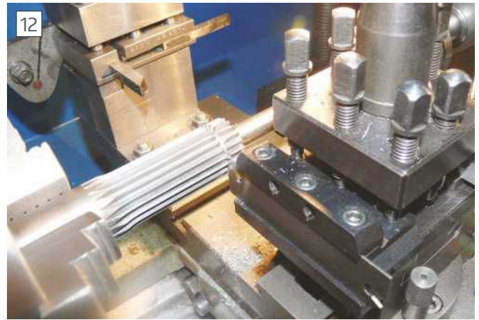
Parting off the gears
