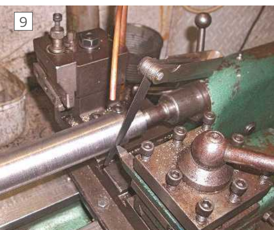
Checking clearance with a feeler gauge
