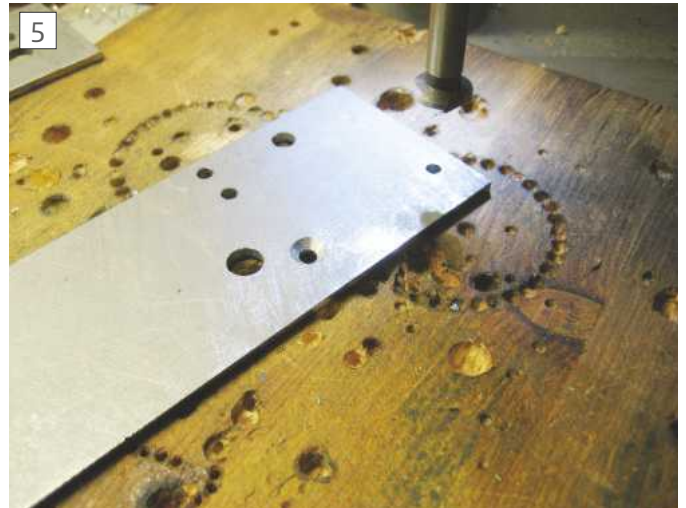
Next the frame was taken to the drill press and the two 4mm holes were counter sunk, photo 5 .
