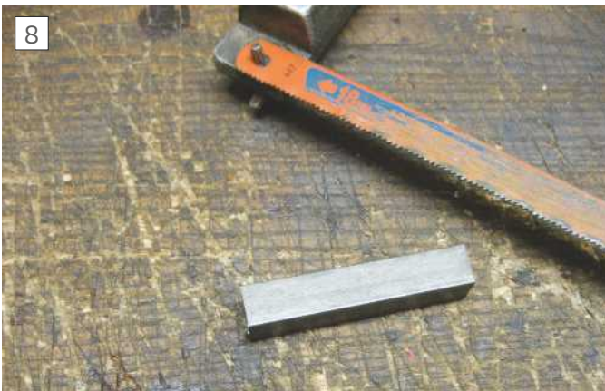
This part was made from a 10x10mm cold rolled steel. I cut the piece a little over size, photo 8 .
