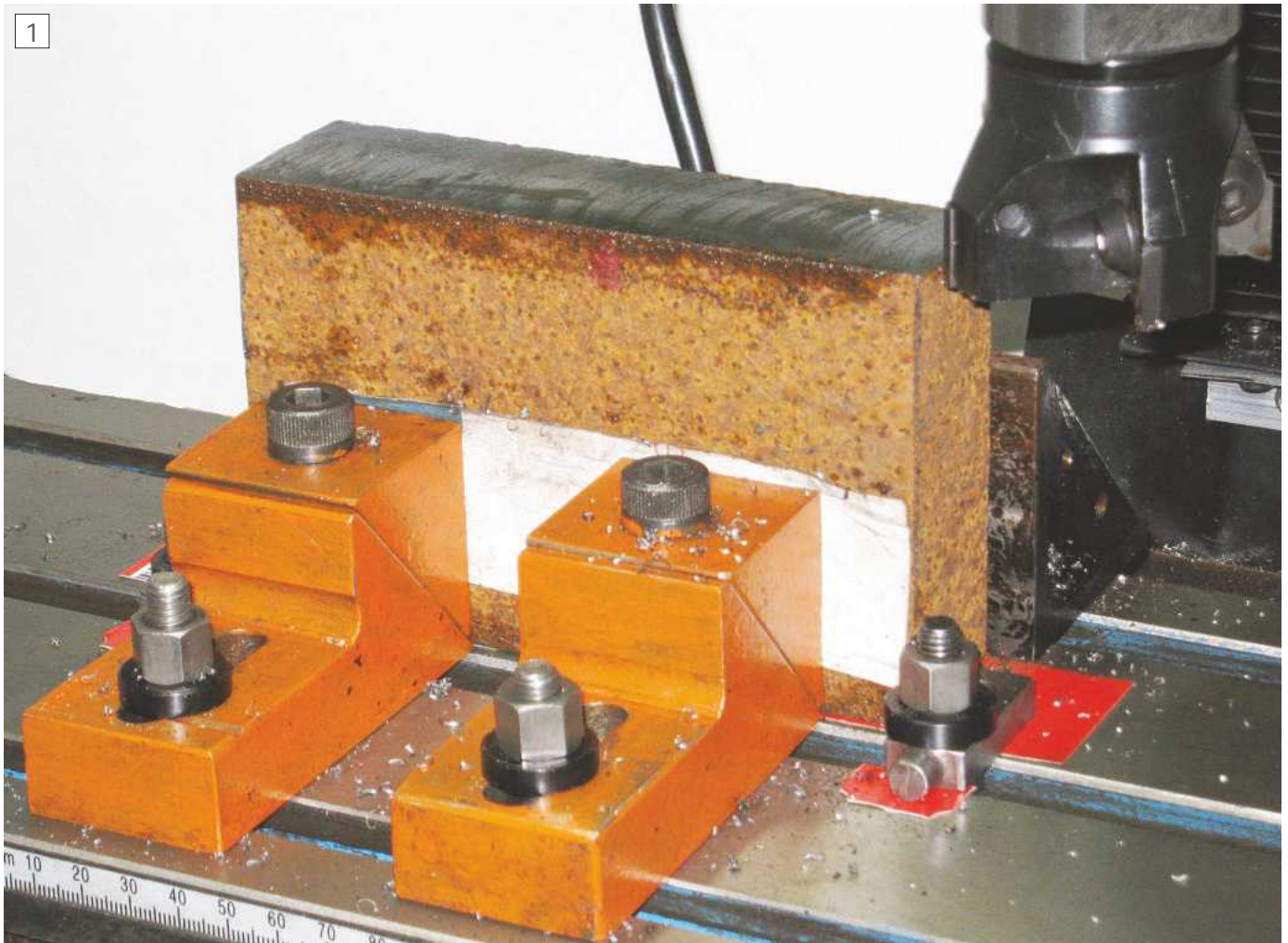
Clamps in use together with angle plates
