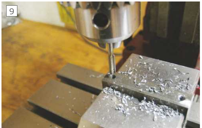
The part was placed in the bench mill, and after locating the zero point, the tapped holes were drilled and tapped, photo 9 .
