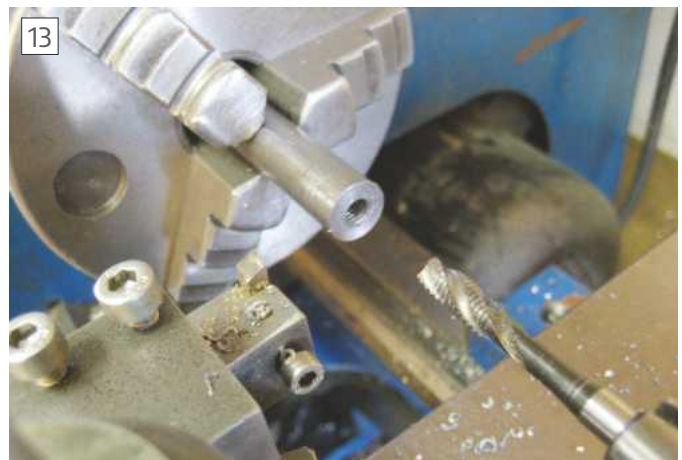
The shafts were made from 12 free machining steel. First job was to drill and tap the M6 tapped hole, photo 13 .
