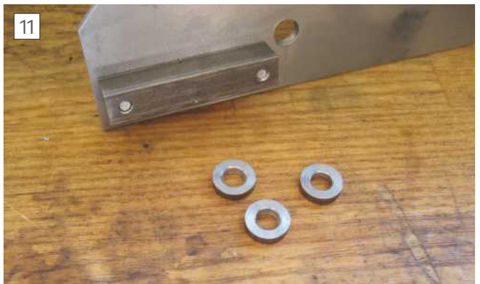
The washers were made from 12mm free machining steel and their job is supporting the shaft for the driving wheel and the two belt wheels, photo 11 .
