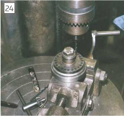
Using a hardened jig to guide drilling of holes in a cutter blank
