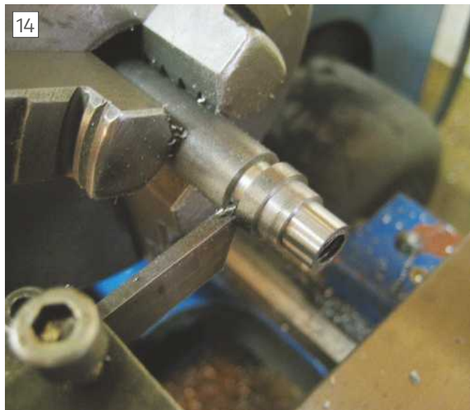
After turning down the shaft according to the drawing, I paid special attention to the nominal 8mm diameter, photo 14 .
