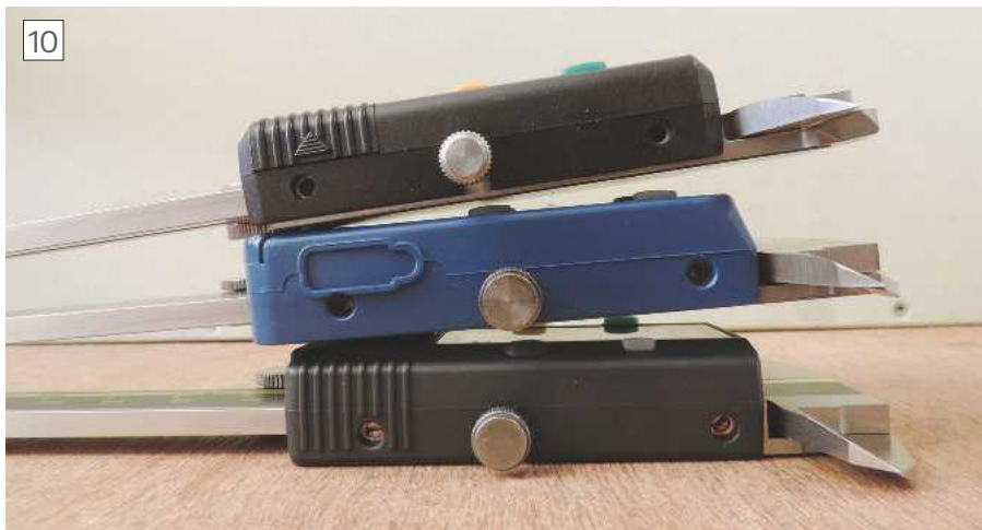
The three calipers all have reasonably sized gib screws, making adjustment easier.
