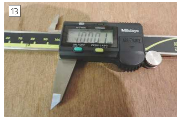
A seventeen-degree temperature change did not affect the Mitutoyo's reading – the M&W caliper was also rock solid.
