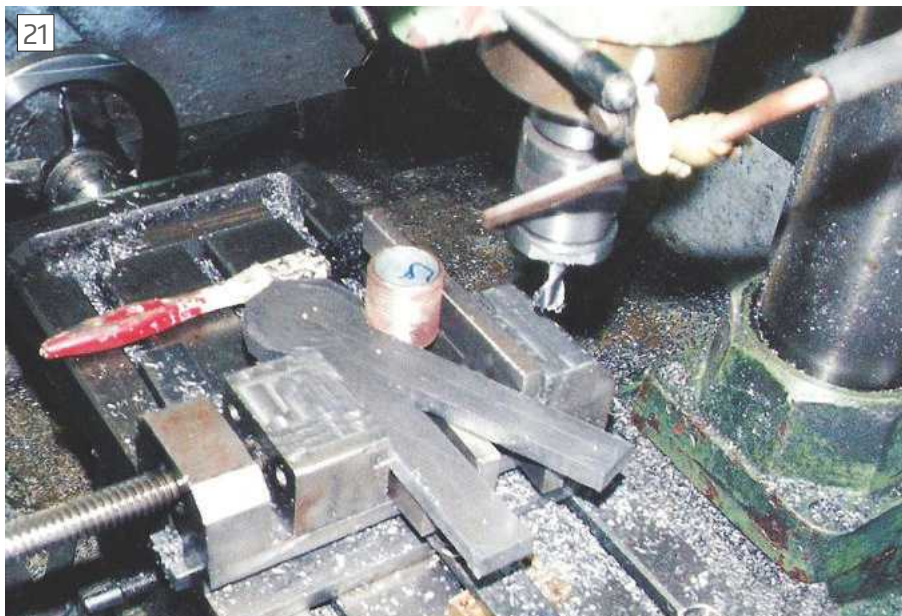
Milling the auxiliary drive arms
