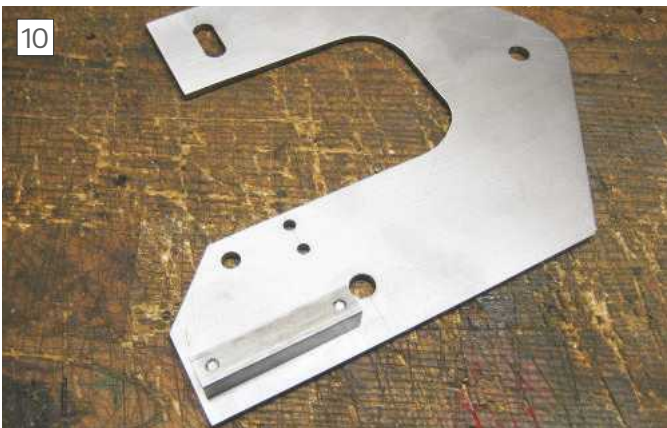
The tool holding bracket was mounted to the main frame, photo 10 , and I was ready to go on to next set of parts.
