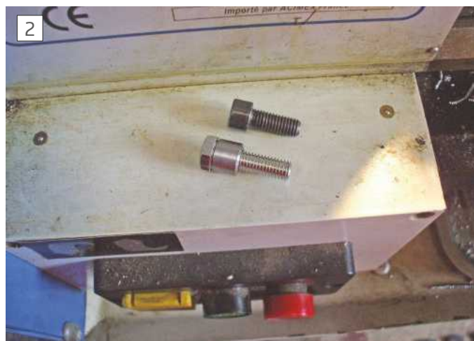
Comparison between the original Allen screw and the replacement one.
