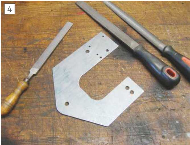
After the rough cut out, the outline was finished using appropriate files, photo 4 .
