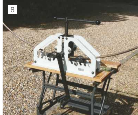
Bending half-tubing with a ring roller
