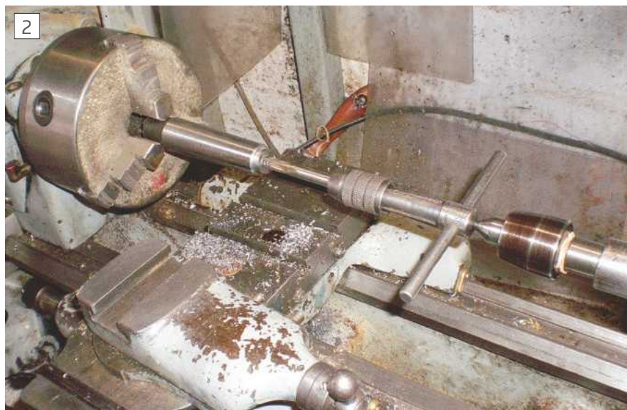
Tapping for a drawbar thread
