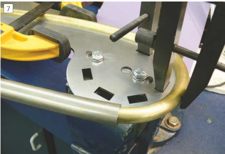
The bending jig in use
