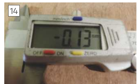
The Workzone caliper was most affected by changing temperatures, drifting about 0.007mm per degree, enough to cause material errors in the average workshop.
