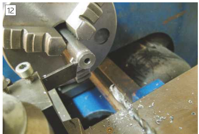
Making these washers was a simple drill and cutoff operation on the lathe, photo 12 .
