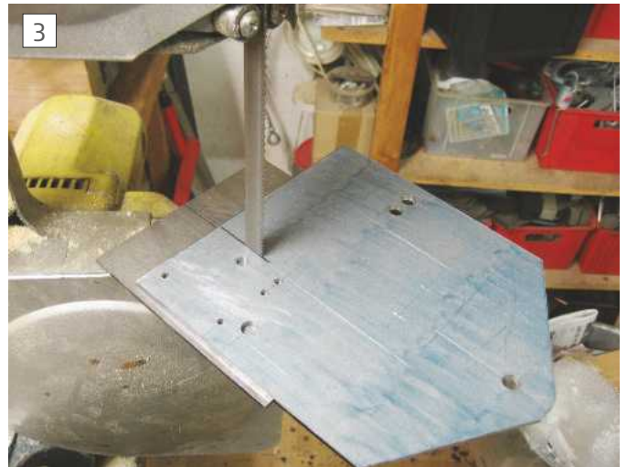
After deburring all holes, the next job was to cut out the contour of the frame plate this was done using my band saw, photo 3 .
