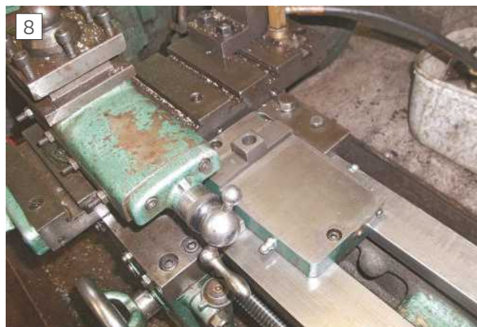
Modified base plate showing adequate clearance of oil nipples from carriage
