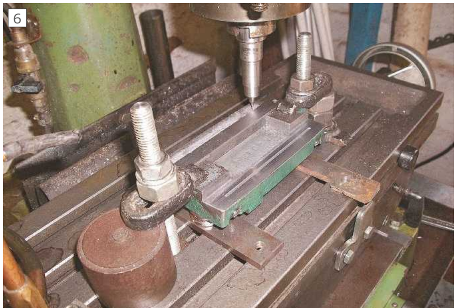
Machining oil grooves on tailstock base plate casting
