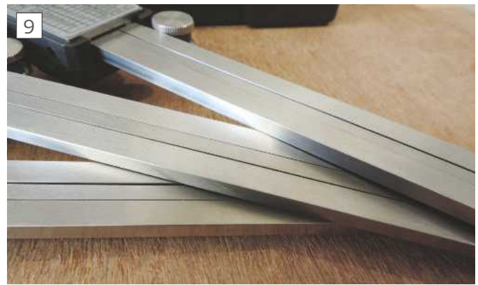
From the top, M-DRO, M&W then Mitutoyo at the bottom, if this prints well, you will be able to see how the finish improves as you go down the pile.
