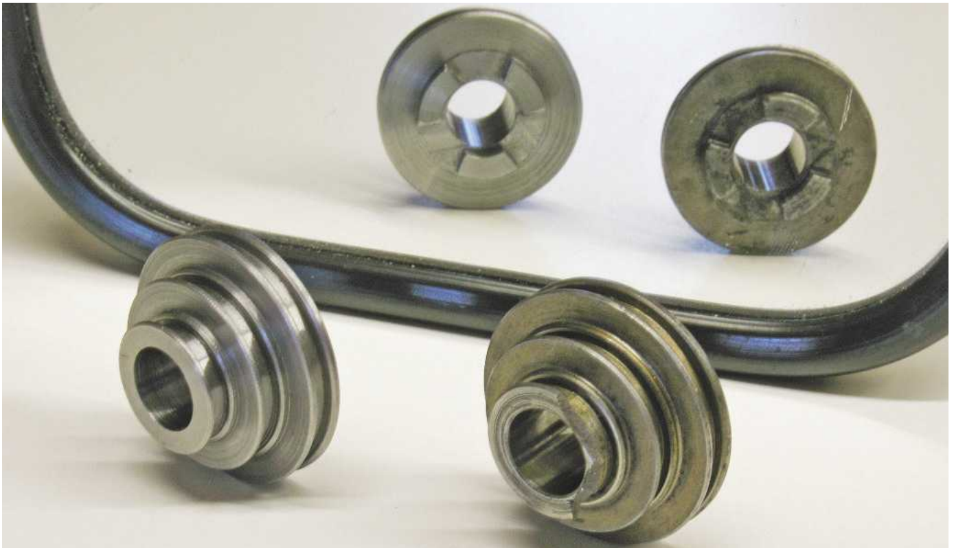
Showing damaged and replacement item. Front view shows grooves and broken flange whilst the view in the mirror shows the driving lugs at the rear.
