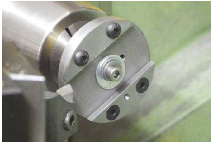
Machining outer diameter of workhead
