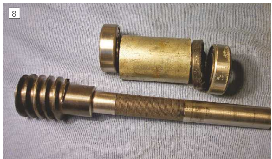
Worm shaft bearings and oil seal fitment
