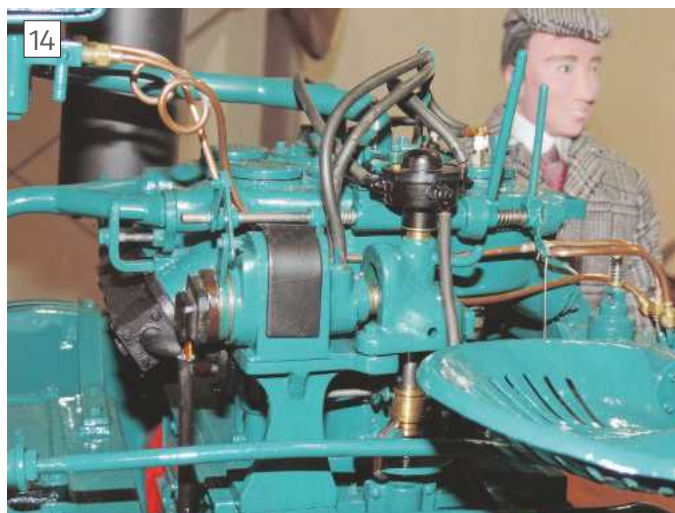
A close up of the fully working control gear
