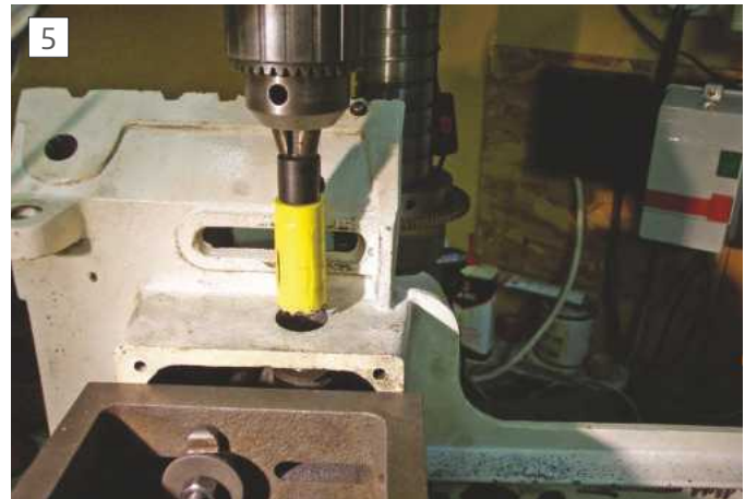
Enlarging hole with hole saw
