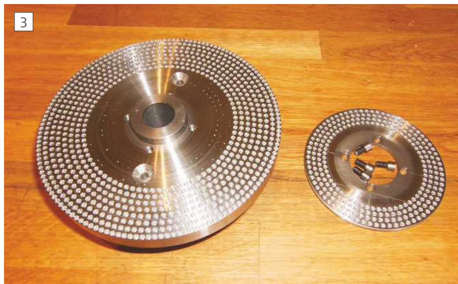
Both Division Plates as machined
