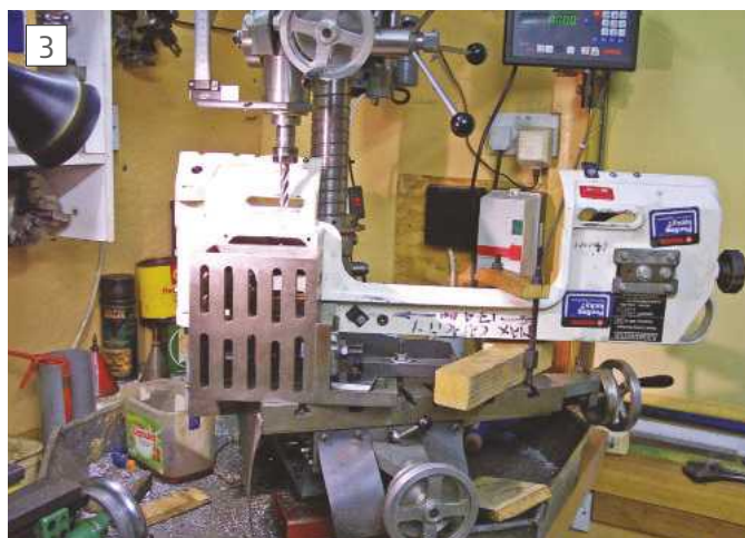
Frame mounted on mill table
