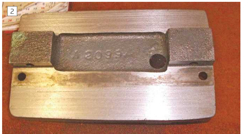
Scoring on underside of tailstock
