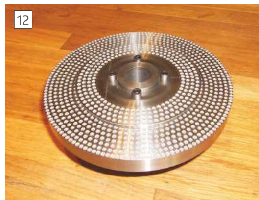
Completed Clock Wheel Division Plates
