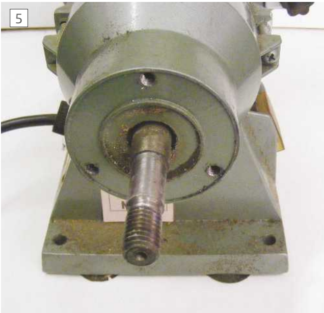
The fully stripped down grinder.
