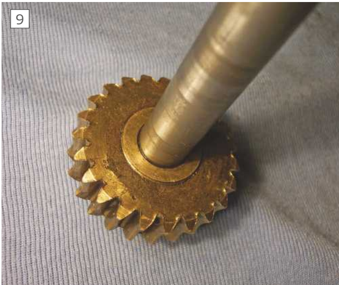
Rough surface on worm wheel
