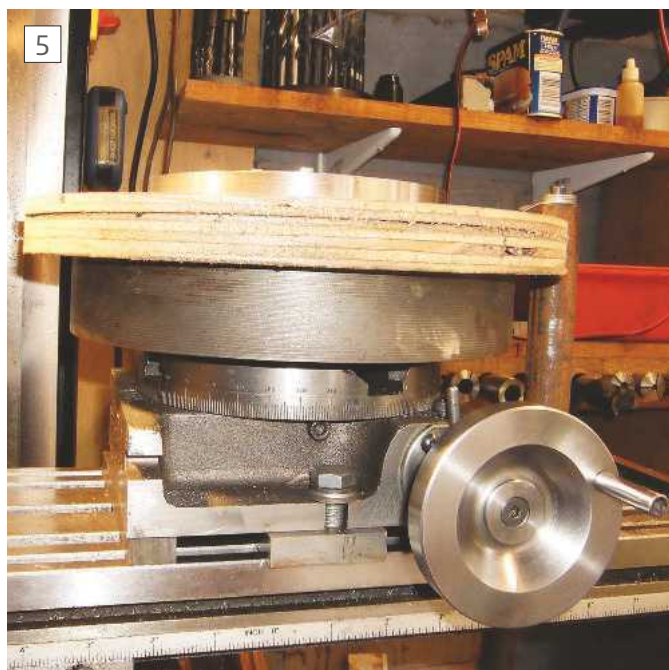
Wood Faceplate mounted on Dividing Head, fastened down to Milling Machine bed.
