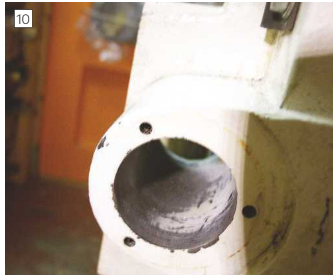
Paint in one of the shaft bores
