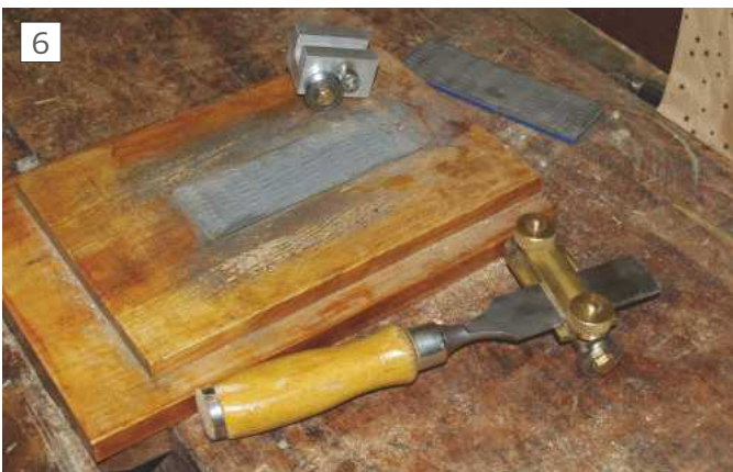
Here you see the wooden mount on the woodworker's bench. If your eyes are sharp enough, you can see two black lines to indicate the angles (The one on the left, more visible, is for chisels and plane irons; the other one is for box-chisels; being much thicker they must project further to get the correct angle)
