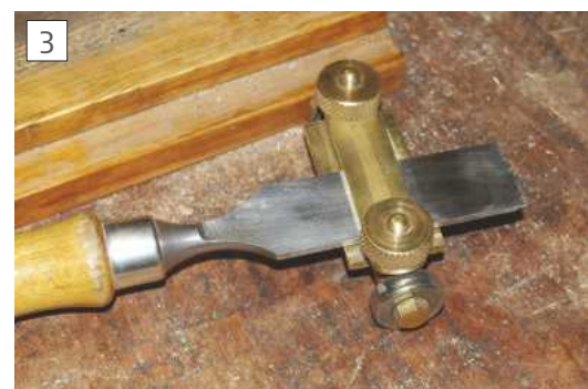
On the right-hand side you see a piece of brass, milled in place, to ensure the chisel is positioned correctly
