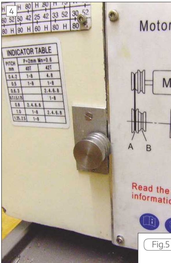
View on outer casing showing the control knob and front plate
