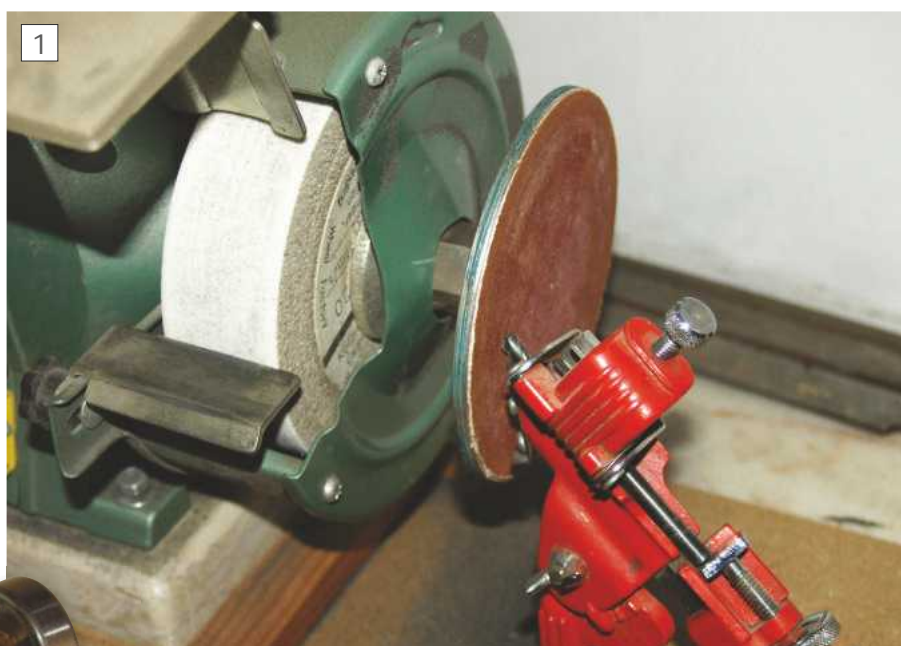
The faceplate and jig ready to sharpen a drill
