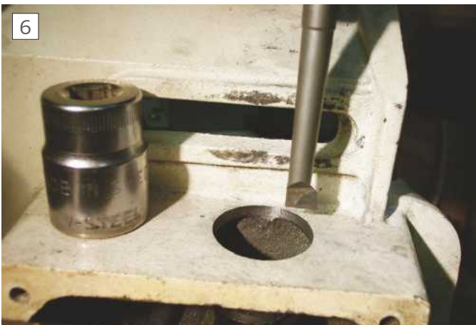
Enlarging hole with boring head
