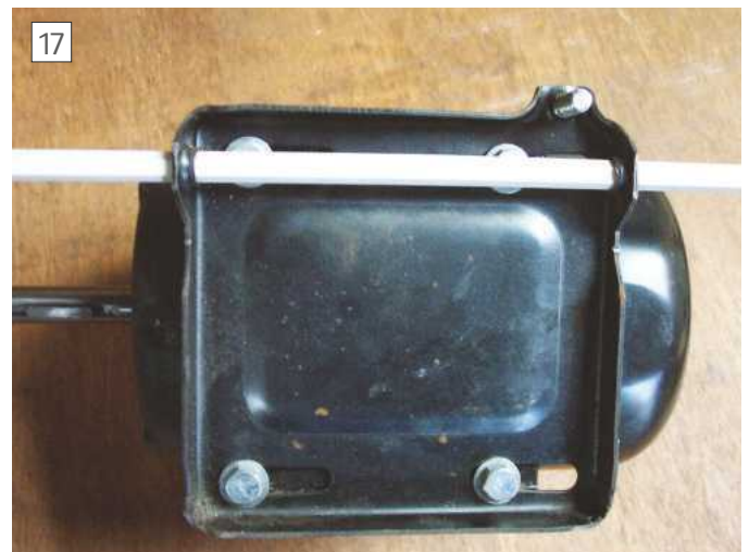
Motor platform pivot axis
