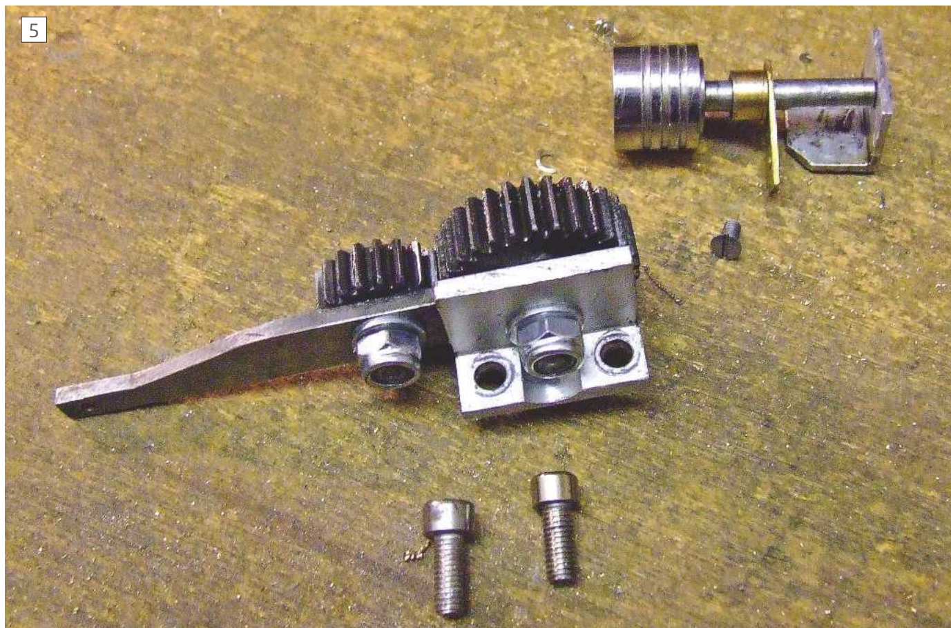
Disengagement and control actuator assemblies
