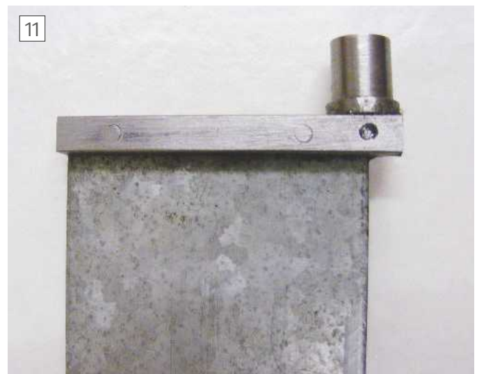
The underside of the rest. Note the support bars.
