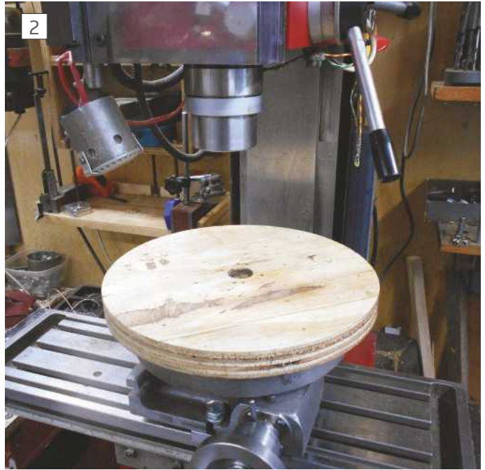
CES Dividing Head fitted with Wood Faceplate
