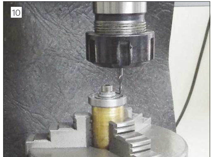
Machining o-ring grooves
