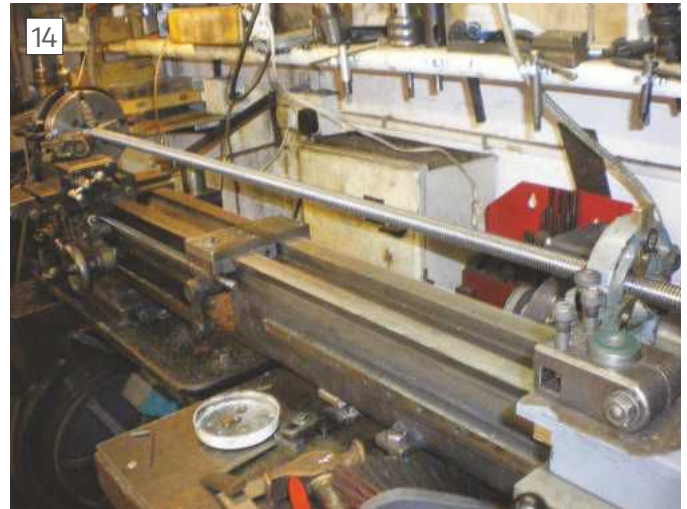
Set up for machining the ends of the leadscrew
