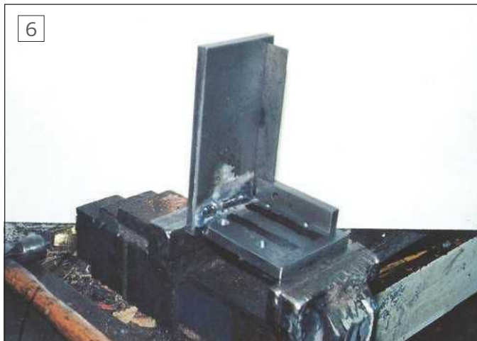
Checking alignment after initial weld
