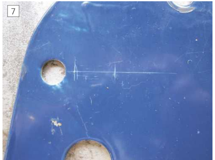
7 Marking the side plate for machining the slot
