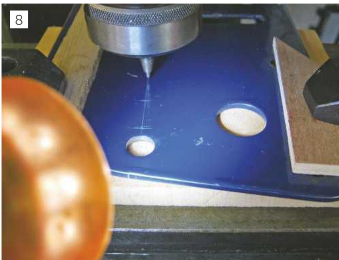
8 Setting milling machine to cut slot
