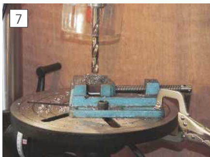
Drilling a 13mm hole in cast iron
