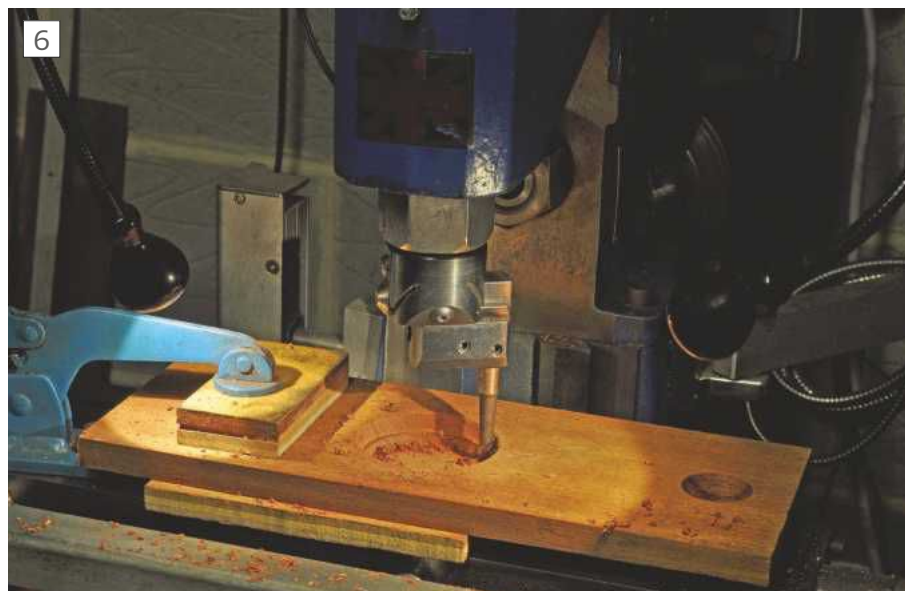
Boring the hole for the weights
