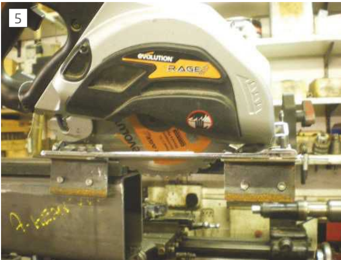
Cutting the shear with an Evolution Rage saw
