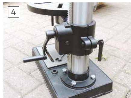
The robust table mounting arrangement
