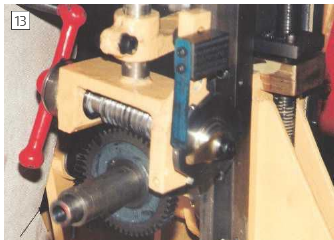
Ratchet arrangement for worm and wheel.
