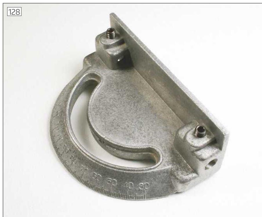
An angle-setting accessory for a bench grinder
