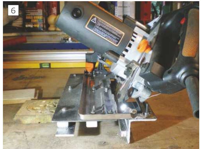
End view of the cutting jig
