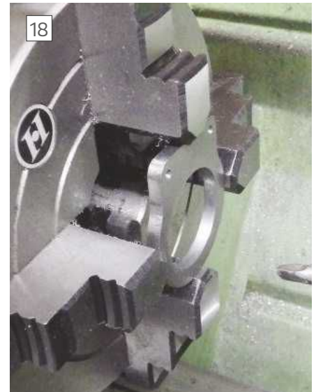
Boring work head base
