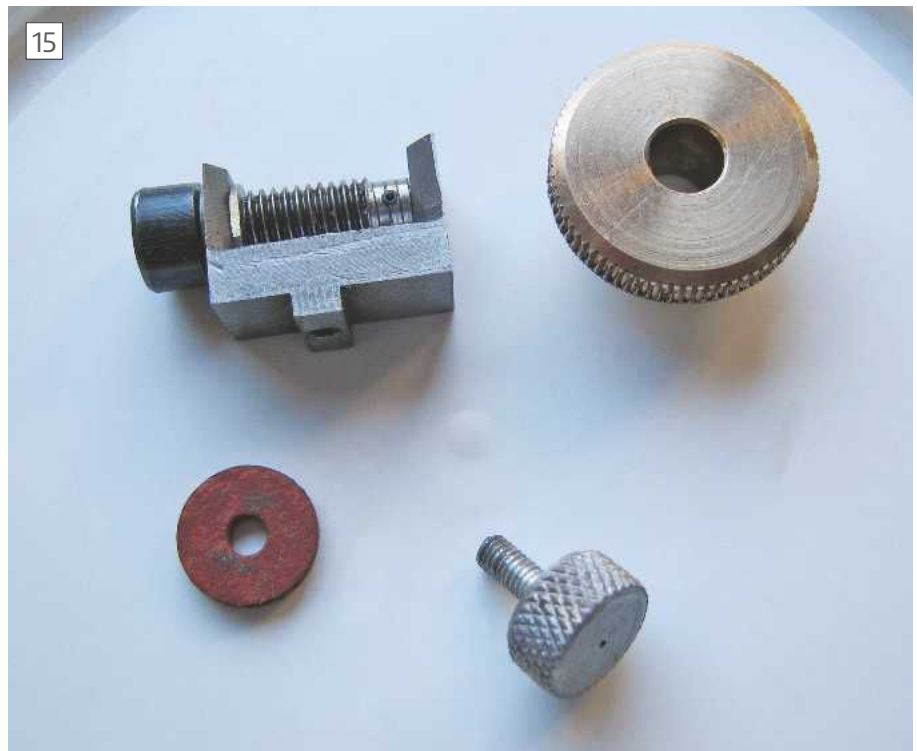
Manufactured parts for the worm and wheel addition
