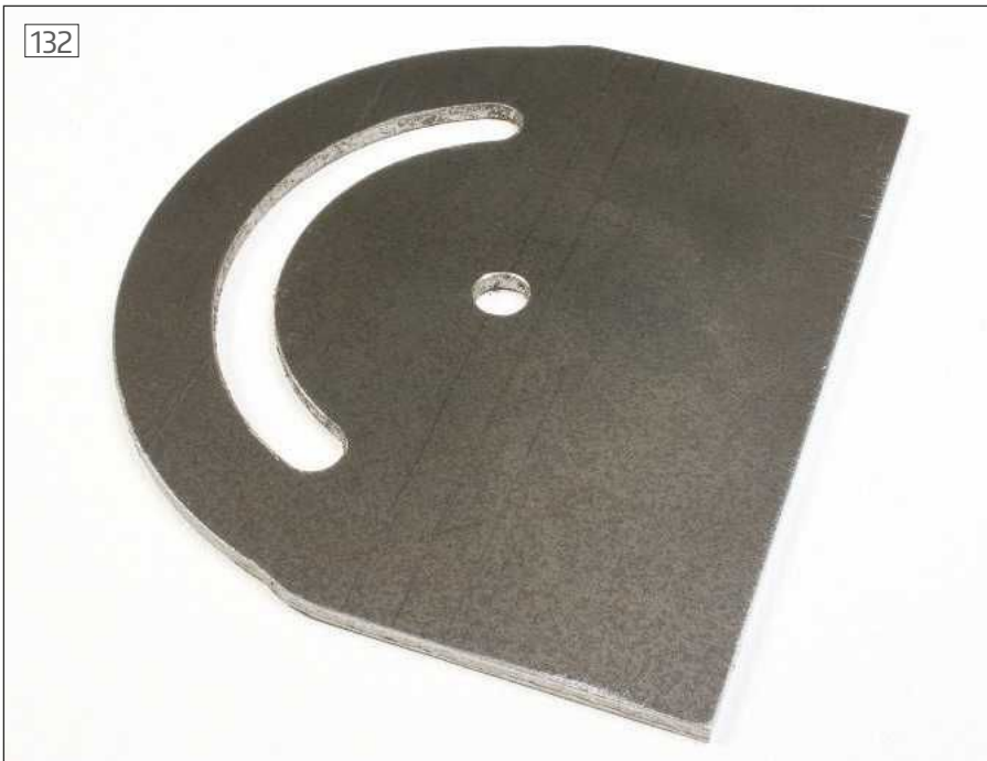
The completed soleplate
