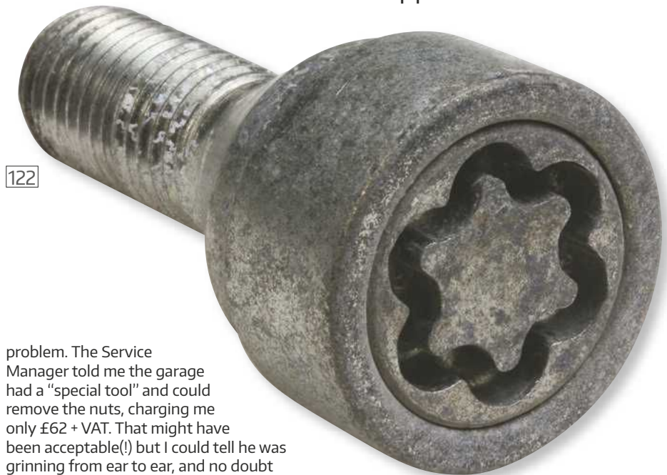
A locking wheel nut. The key has a projecting ridge which matches the groove in the nut.
