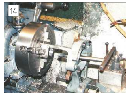
Boring the small bearing housing
