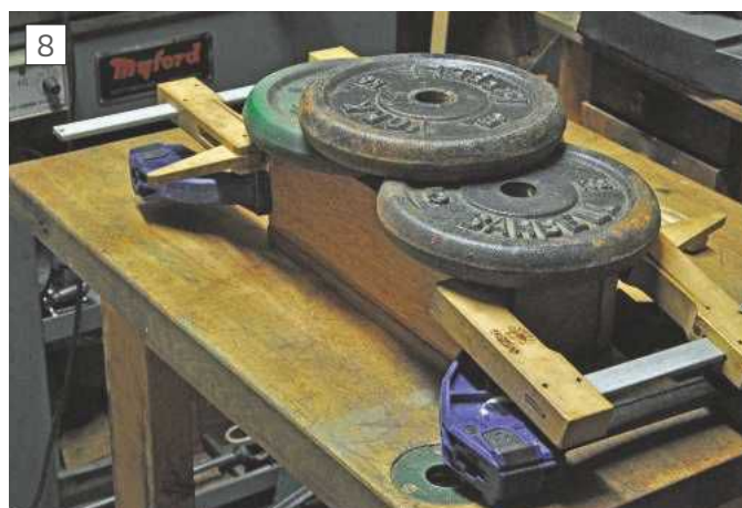
Base frame glued to top
