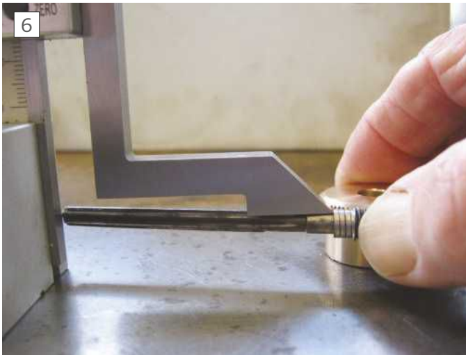
6 Checking worm wheel dimensions
