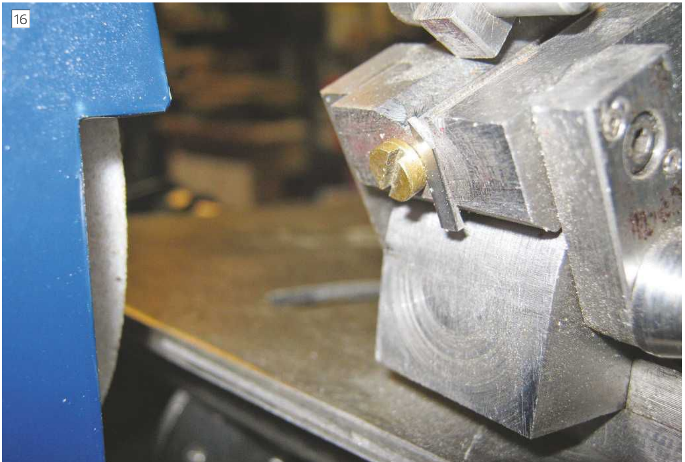
Modified drill stop on four facet jig
