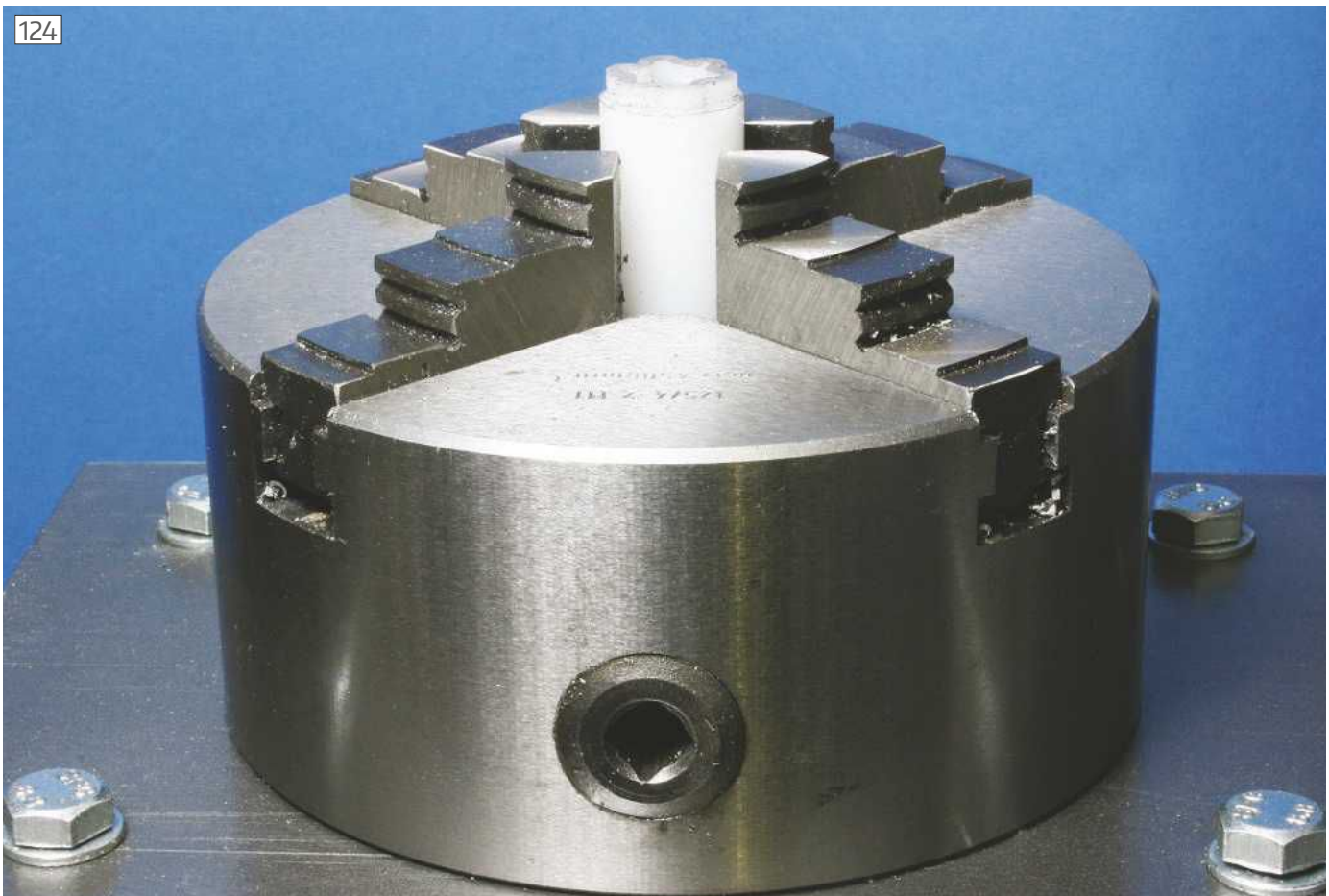
A test piece was cut in Acetal gripped in an upward-facing chuck bolted to the mill sub-table
