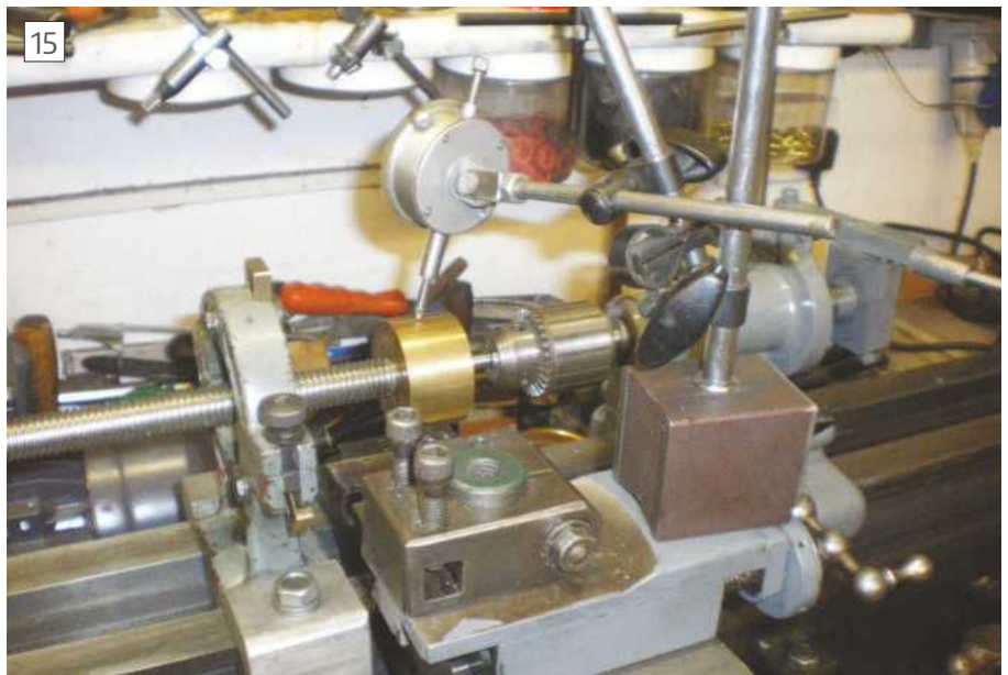
Using the matching nut as an aid to alignment
