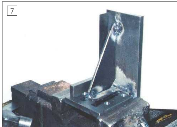
Bracing piece tacked in place
