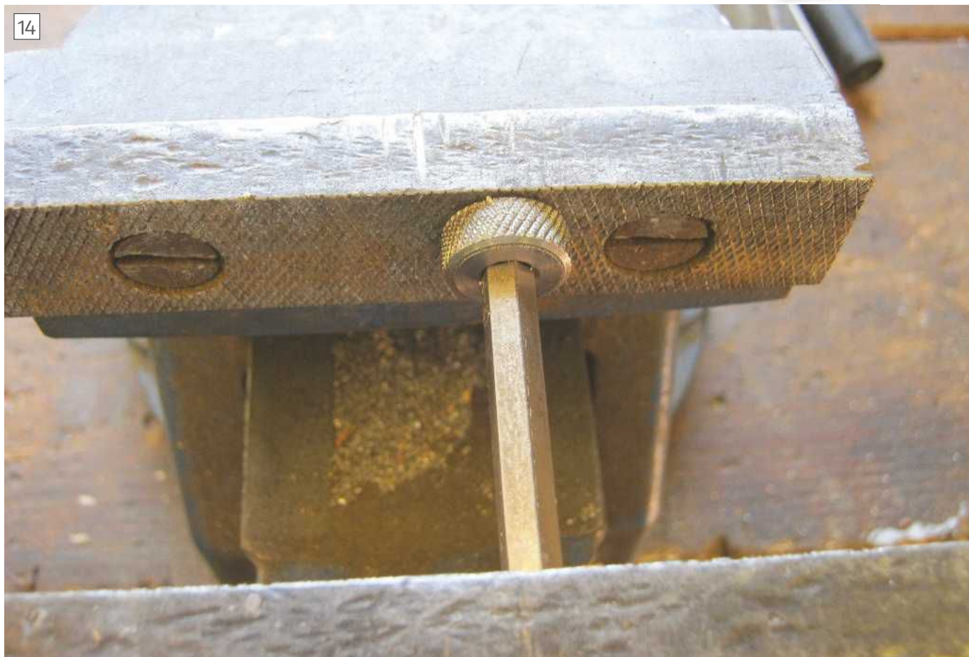
Using a vice to force the knob onto its Allen key shaft
