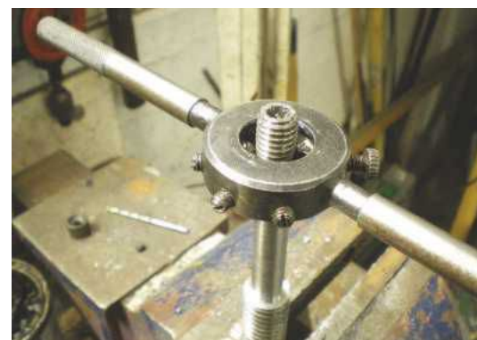
Threading the end of the leadscrew for a handwheel.
