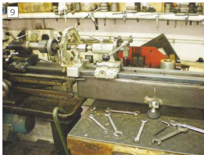
Using engineer's blue to guide scraping of the shears
