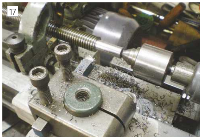
Machining the journal for the joint end
