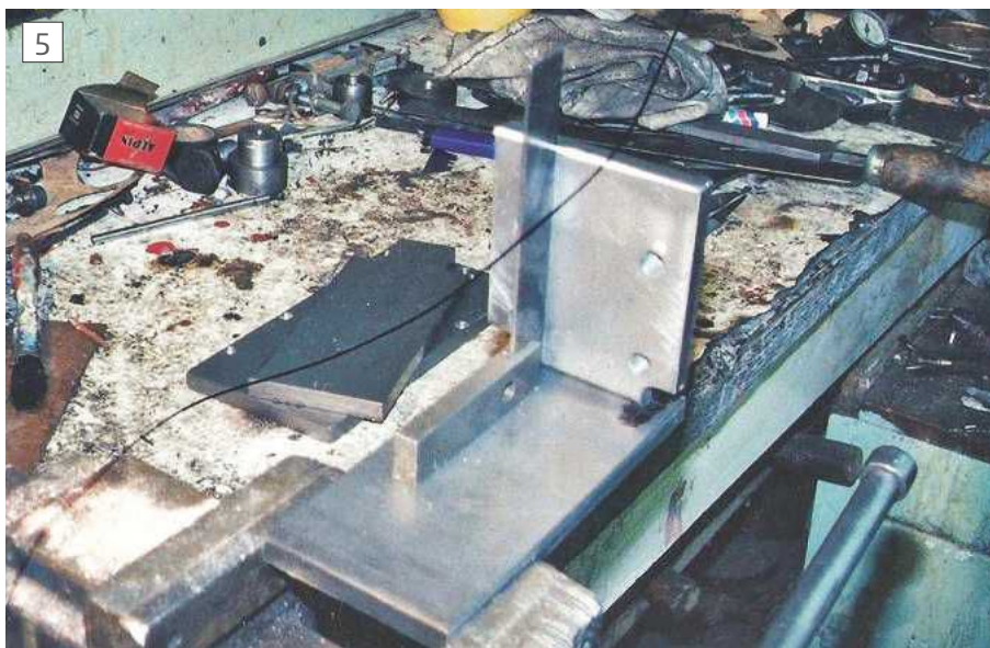
Setting the parts of the angle square
