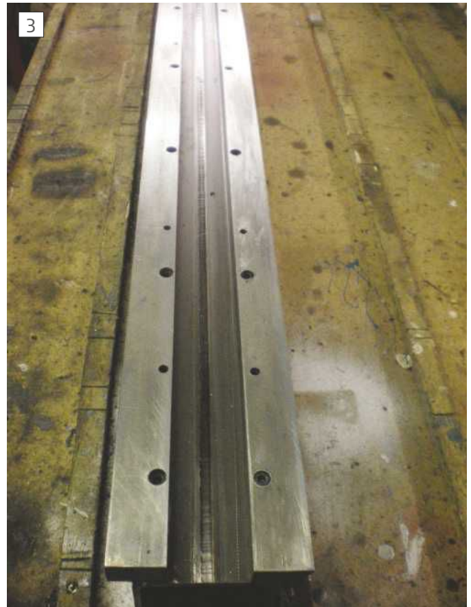
Locations of the fixing screws
