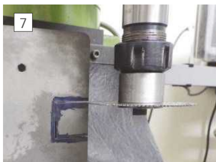
Slitting saw set up
