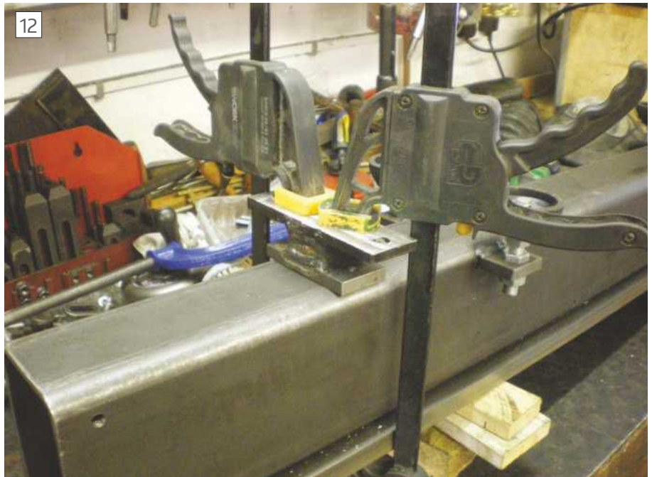
Positioning the permanent feet
