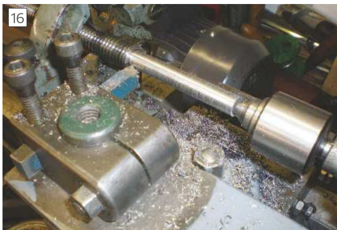
Machining the leadscrew to fit a Myford journal on the tailstock end
