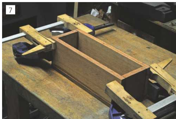
Base sides clamped to end pieces
