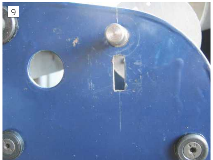
9 Slot cut, ends squared
