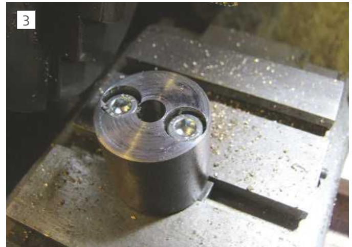
Fixture to carry the worm wheel whilst hobbing
