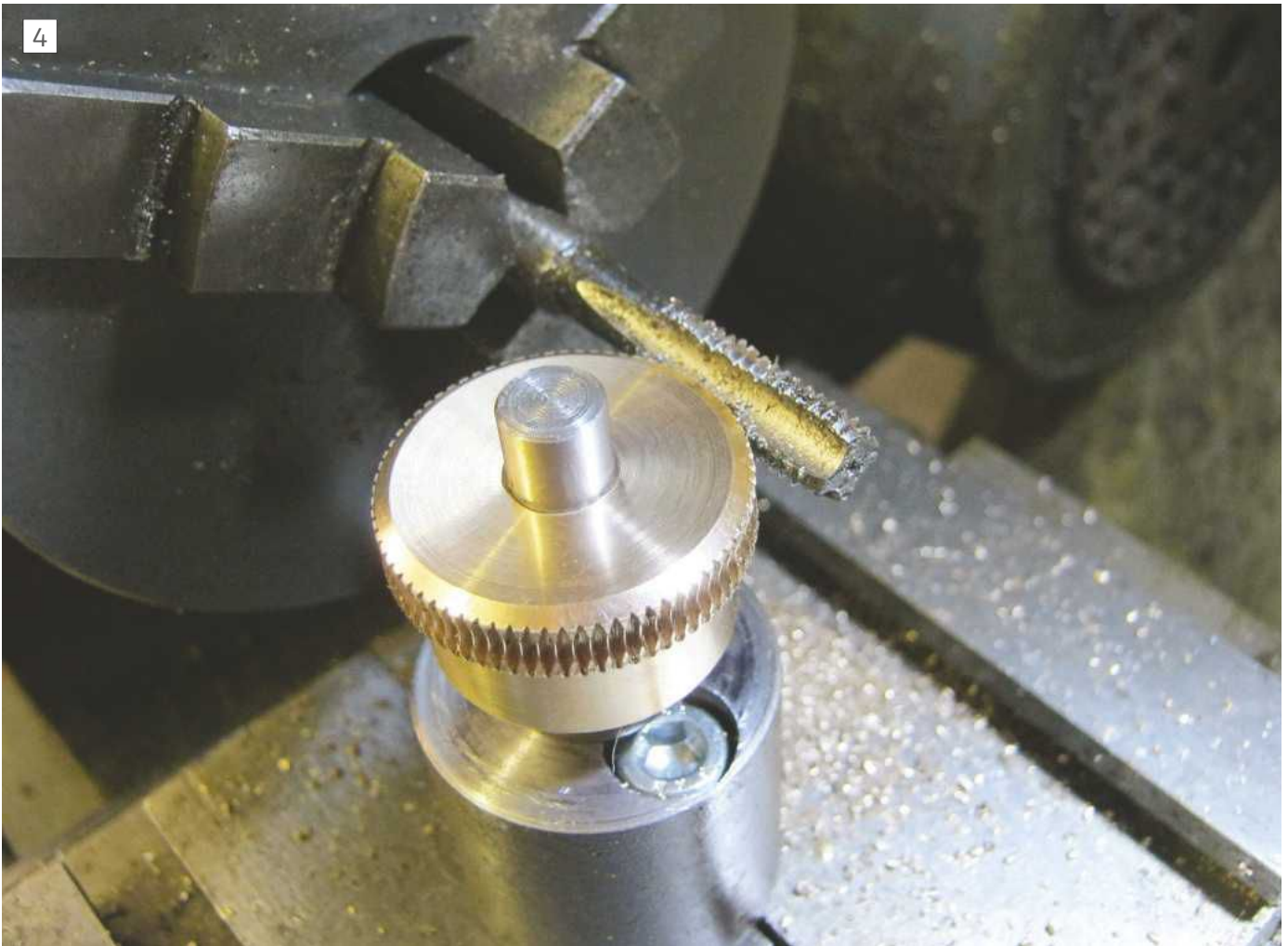
Worm wheel hobbing in progress
