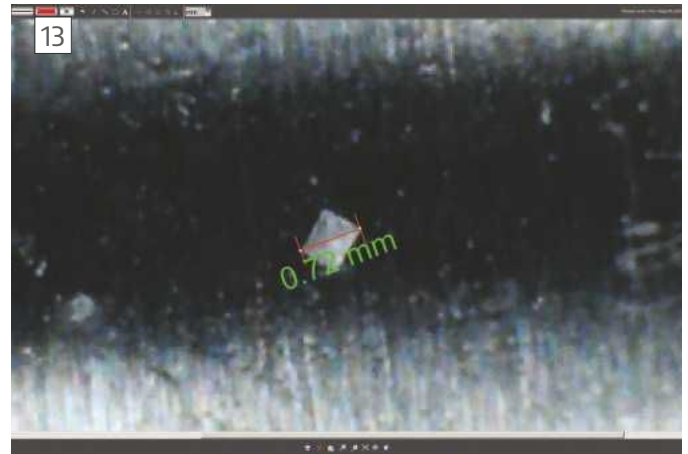
Indent measurement with the USB microscope
