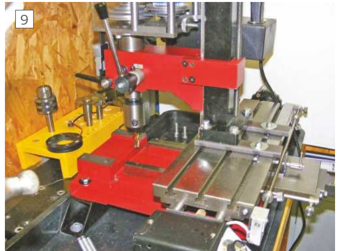
The mill column mounted on the milling table for truing up the base pads.
