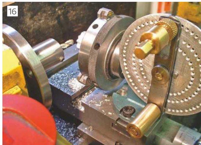
Fluting an aluminium knob
