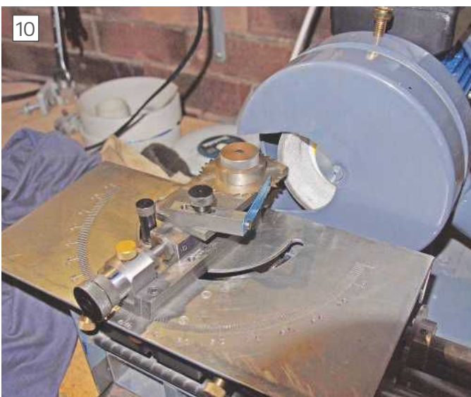
In use with the Worden slitting saw sharpening attachment.
