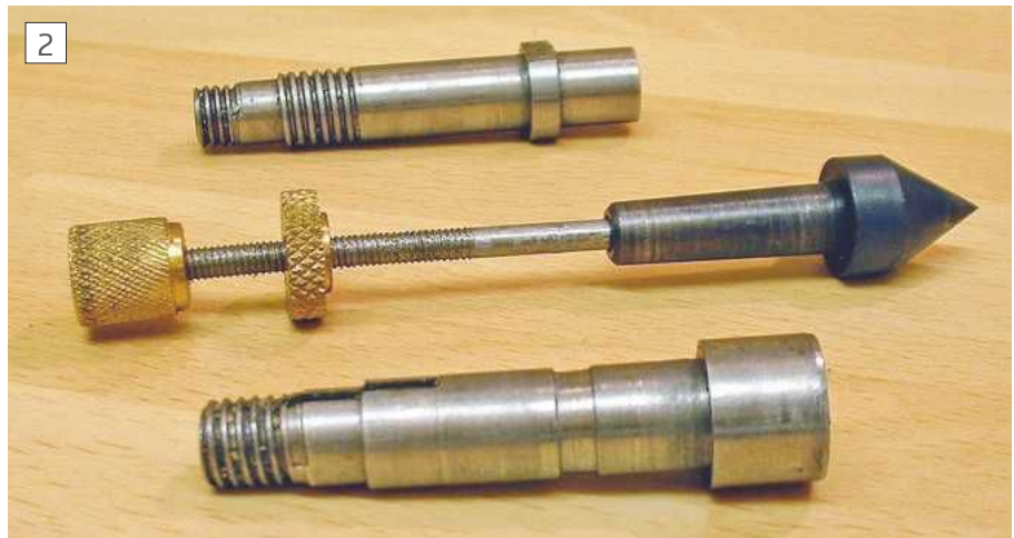
Spindles, drawbar and centre for the original light dividing device
