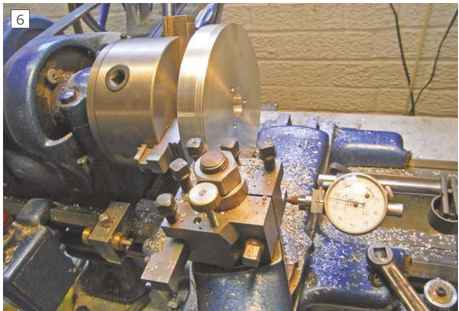
Machining the v-grooves
