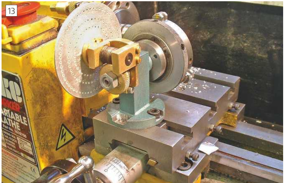
The dividing device attached to the lathe
