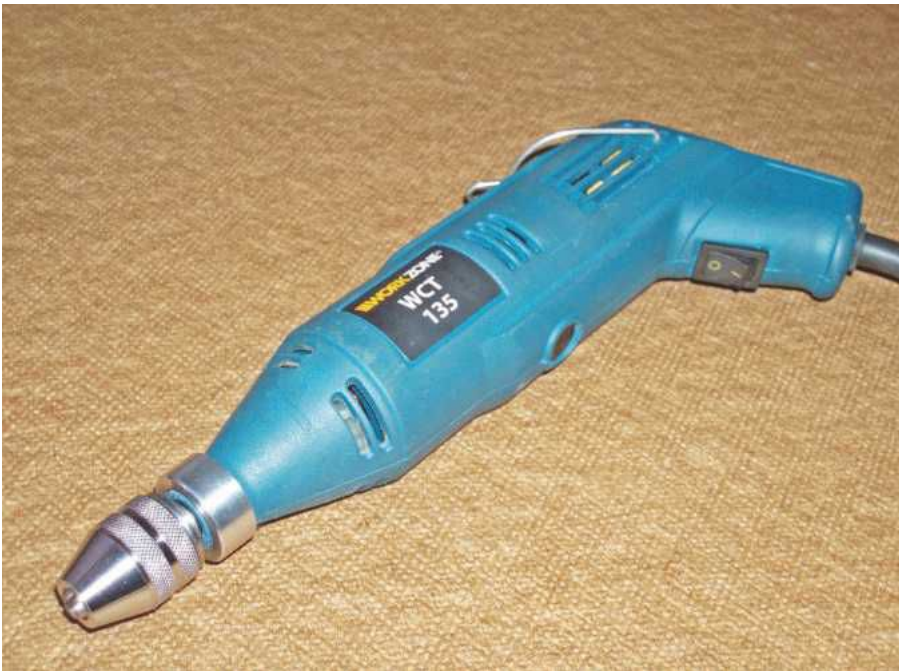
The new chuck fitted to the drill
