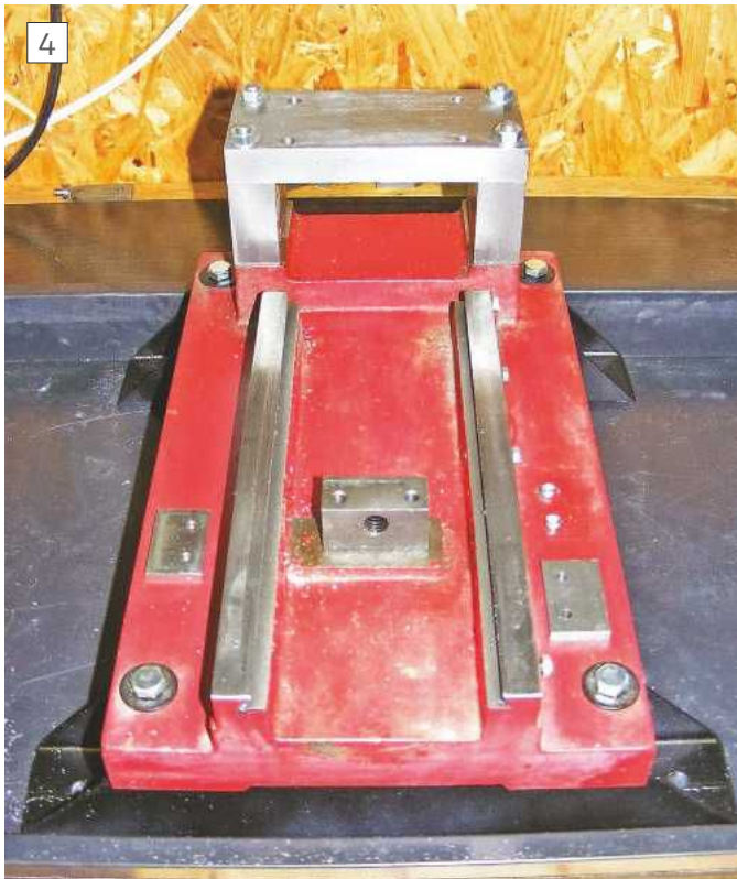
The base of the mill with the riser blocks and support plate.
