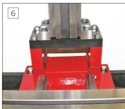
The new column fixed to the support plate and riser blocks.
