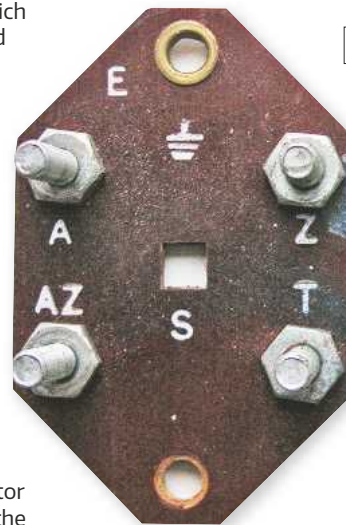
A pair of motor terminal boards, showing their markings
