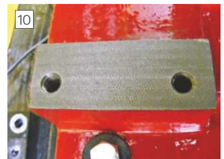
The left hand base pad after milling.
