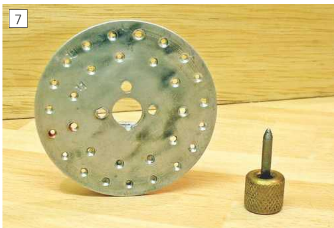
One of the index plates with the original, unsprung, detent
