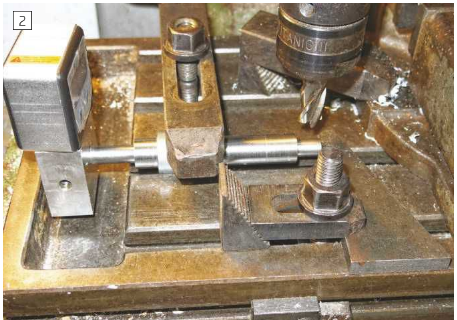
Setting up with the angle gauge
