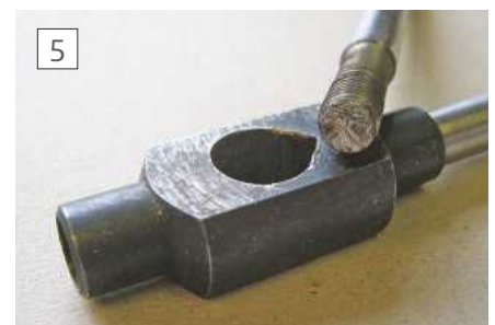
Wear on the end of tap wrench screw
