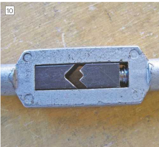
Jaw arrangement of another design of tap wrench
