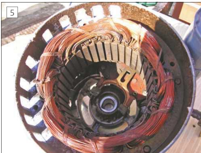
The windings of a typical motor
