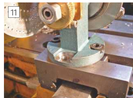
Attachment points allow mounting across or along the lathe axis
