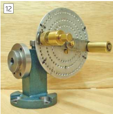
This view shows the chuck backplate
