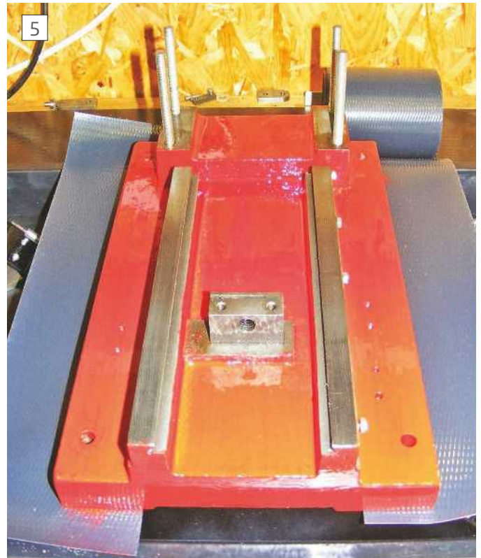
The base after cleaning up and painting.
