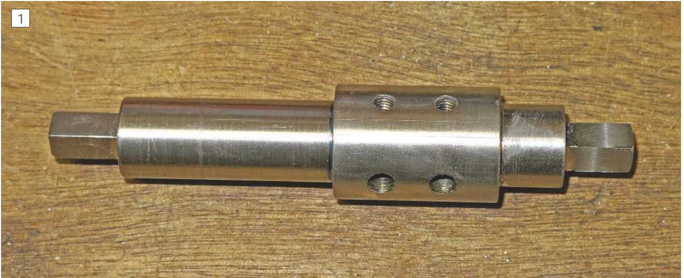
The shaft with a square at each end
