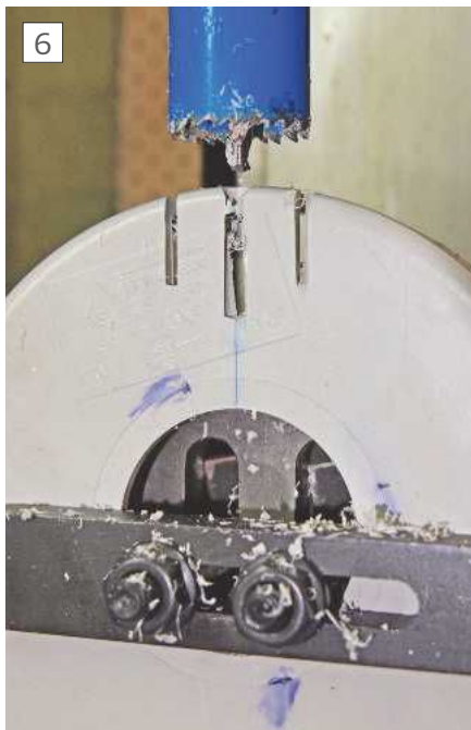
A hole-saw again, this time roughing out the duct exit.
