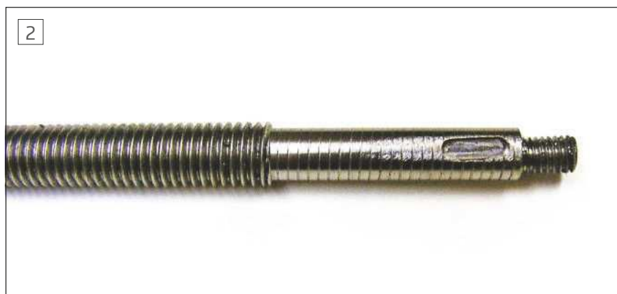
The end of the extended leadscrew after machining.
