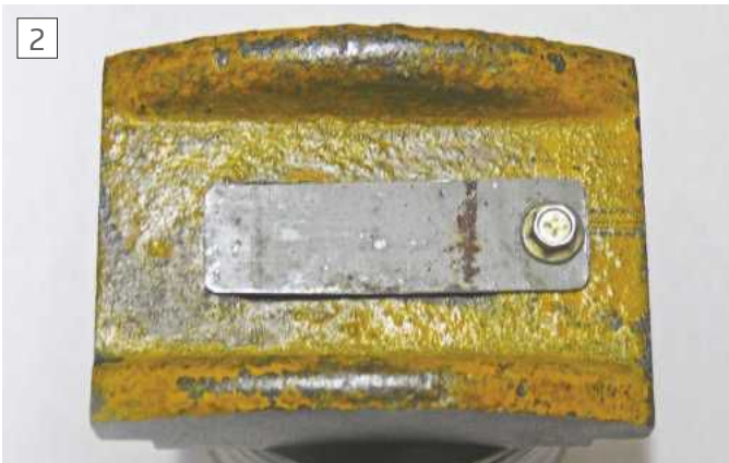
Recess for the bolt head
