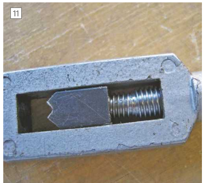
Fixed jaw removed to show double adjusting screw
