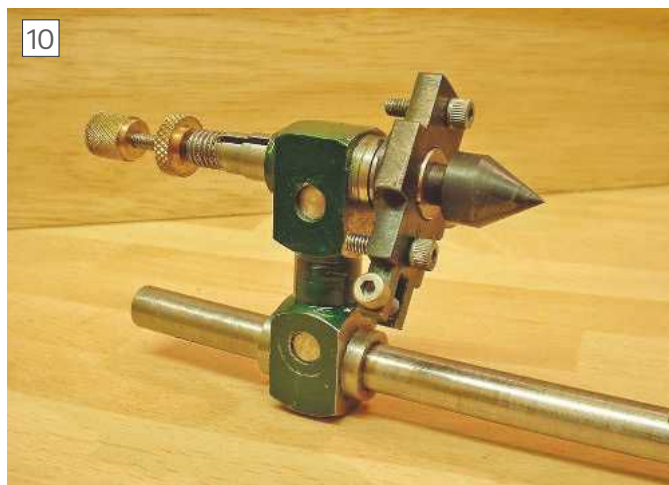
The original tailstock, showing the driving plate
