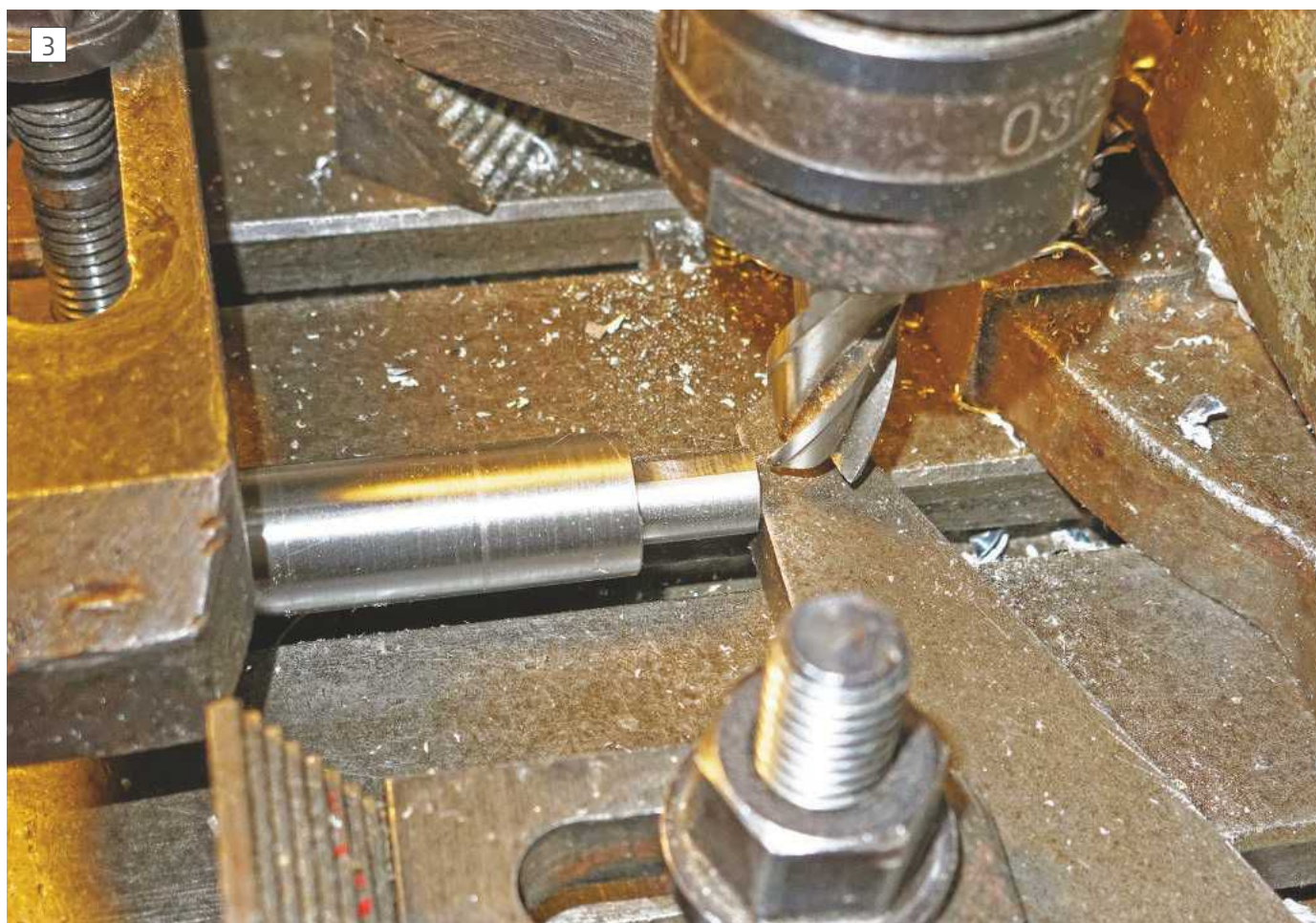
Machining the first square...
