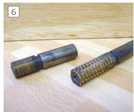
The original 20 tpi hob compared with a 10 tpi version
