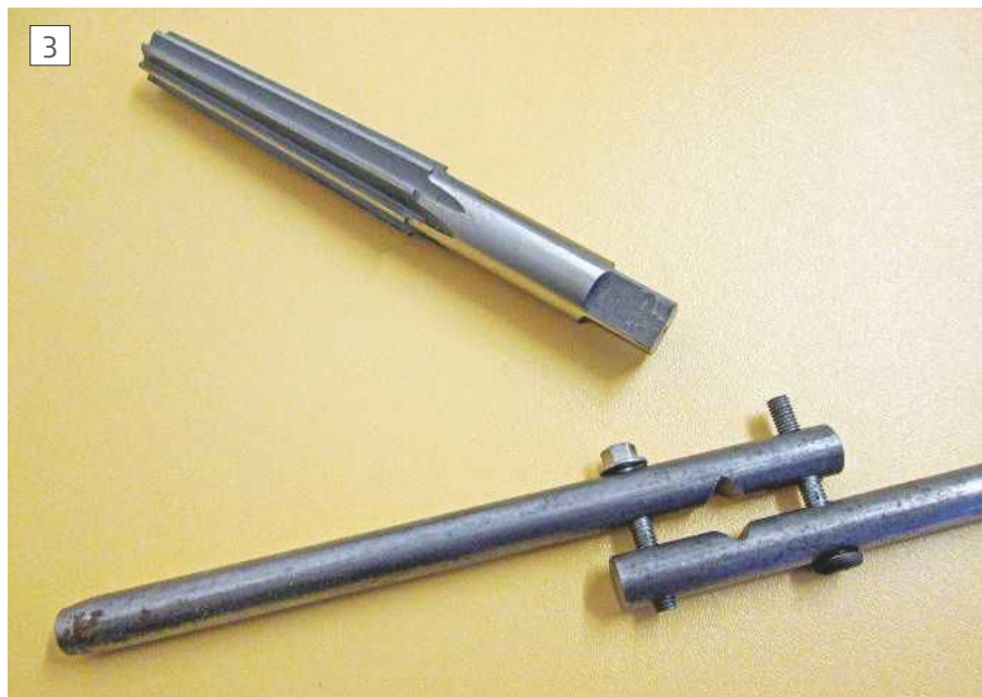
Tap wrench made to turn a Morse 2 taper tap
