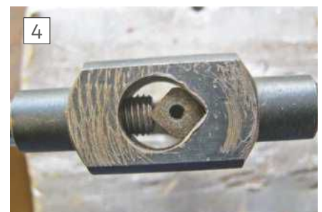
Wrench from kit gripping a tap
