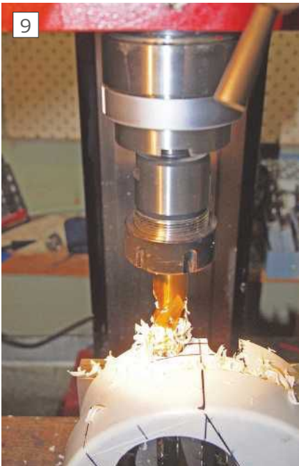
Milling the duct clearance in the front cover.
