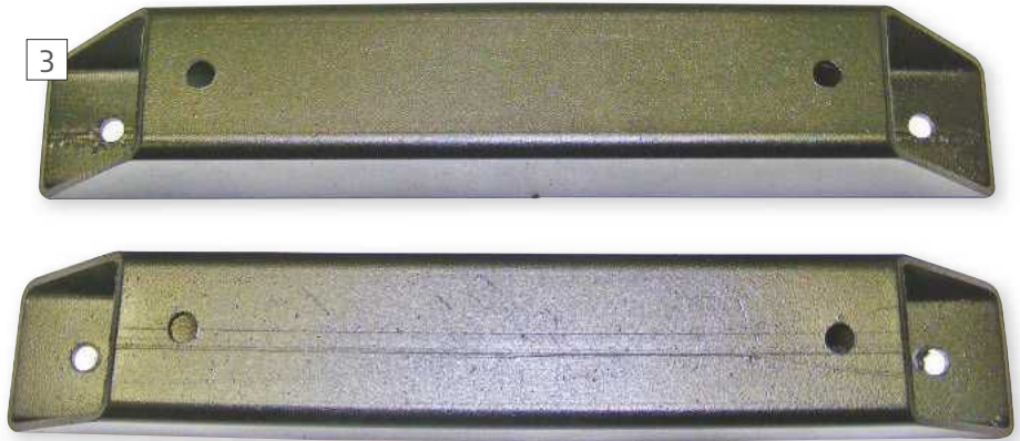
The finished mill riser blocks.
