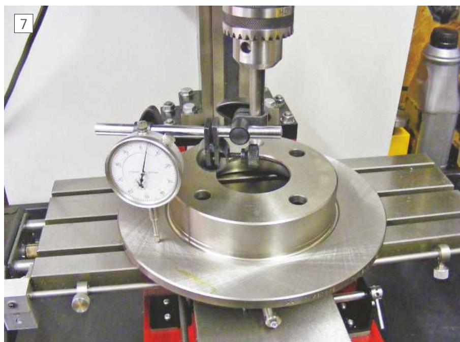
The set up for trammings the mill.
