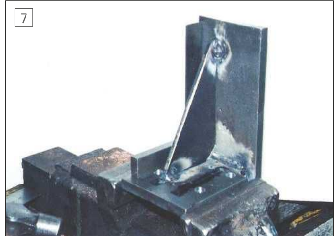
Bracing piece tacked in place
