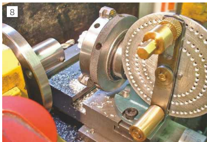
The new, sprung, detent and handle
