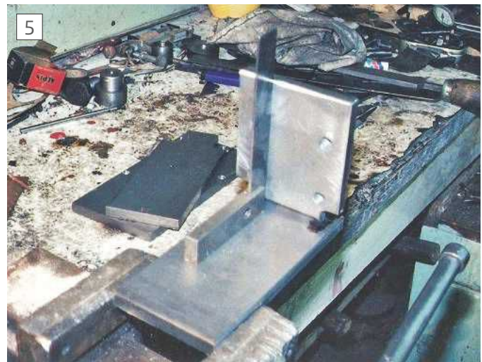
Setting the parts of the angle square
