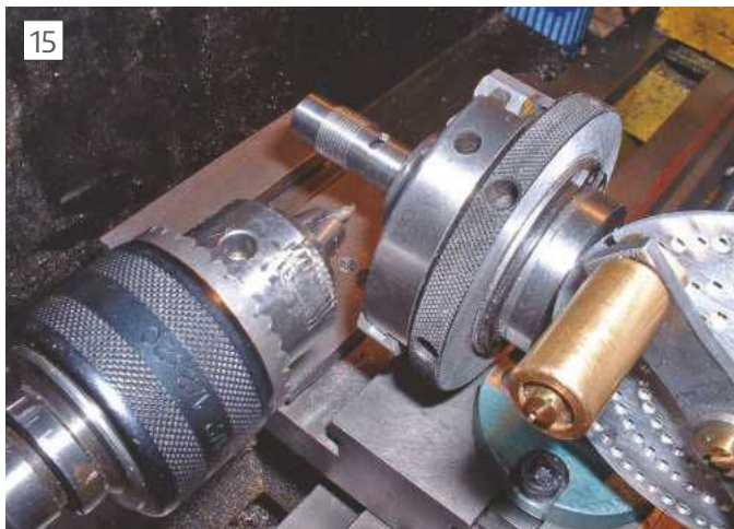
Drilling an inlet port for a small IC engine
