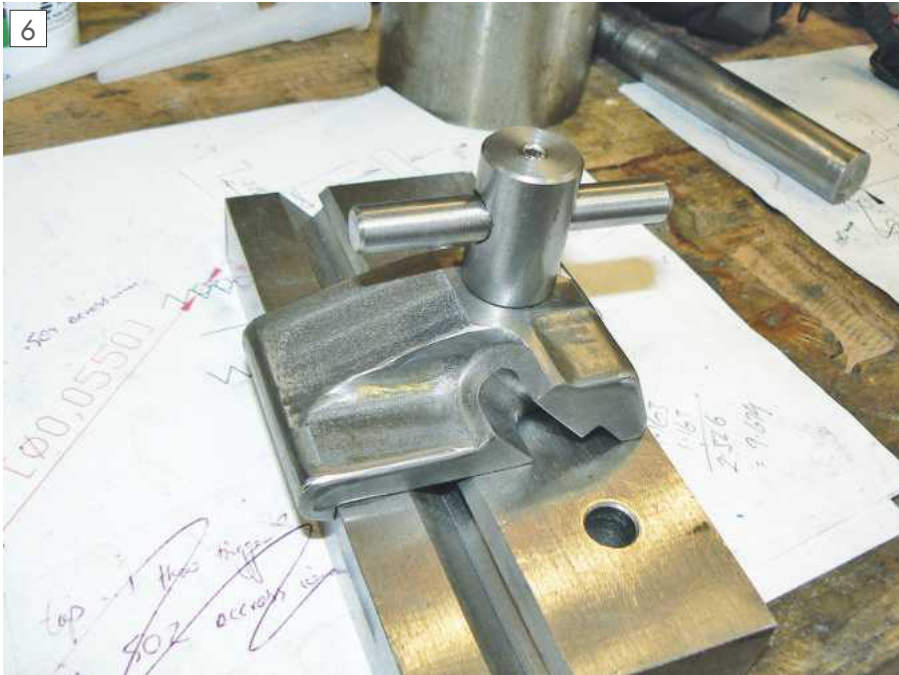
Radiused corners in a pocket.
