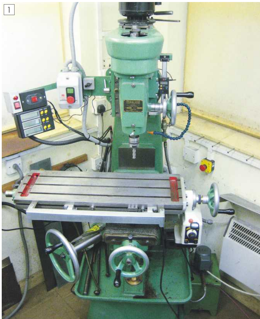
The milling machine showing power feed unit in place.
