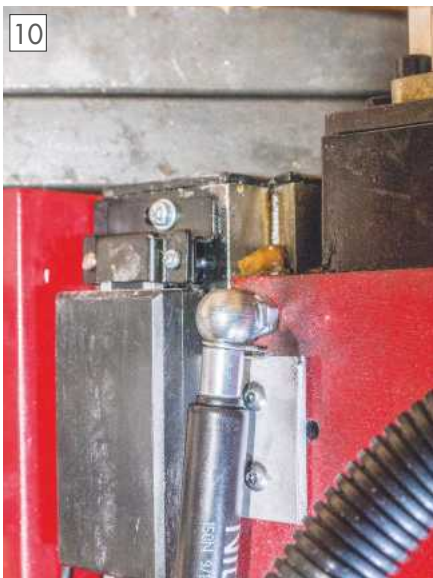
Top of Z axis scale with read head at maximum.
