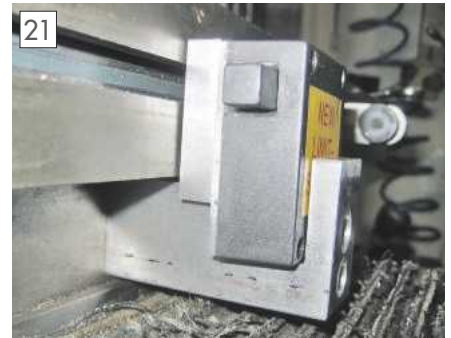
The fabricated bracket with the limit switch attached.
