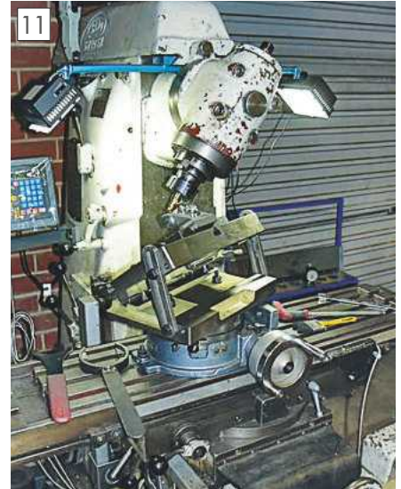
Setup for the intersection of two surfaces.
