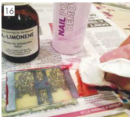
When you are satisfied that the process has completed, remove the toner resist. A combination of nail varnish and solvent, in this case Di-Limonene, is very effective but MUST be carried out preferably out of doors, or at the very least where an adequate supply of fresh air is available AND use an effective respirator to avoid breathing the fumes that the process gives off. Both acetone (nail varnish) and Di-Limonene fumes are dangerous by themselves. When used together, they are even more so. After all, if they can dissolve solid toner, think what they might be doing to you if unprotected.
