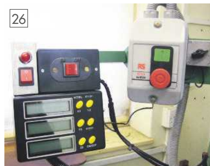
The remote switch and indicator at top left. The DRO display is also seen with its various control switches, along with the machine on-off switch.
