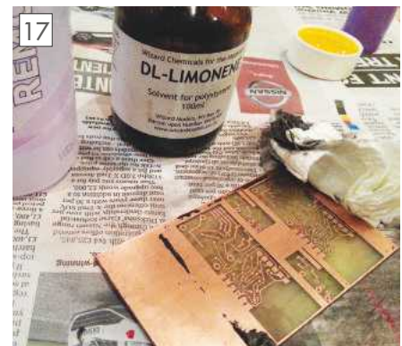
When you are satisfied that the process has completed, remove the toner resist. A combination of nail varnish and solvent, in this case Di-Limonene, is very effective but MUST be carried out preferably out of doors, or at the very least where an adequate supply of fresh air is available AND use an effective respirator to avoid breathing the fumes that the process gives off. Both acetone (nail varnish) and Di-Limonene fumes are dangerous by themselves. When used together, they are even more so. After all, if they can dissolve solid toner, think what they might be doing to you if unprotected.
