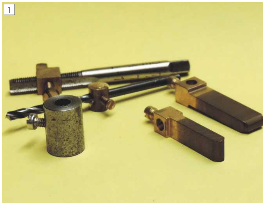
A selection of stops and pegs. The one on the drill is in fact from a round pin plug, the rectangular one on the tap shows its origins; while the other pegs await conversion. The round one in the foreground was made to suit a larger drill, and retained for future use.
