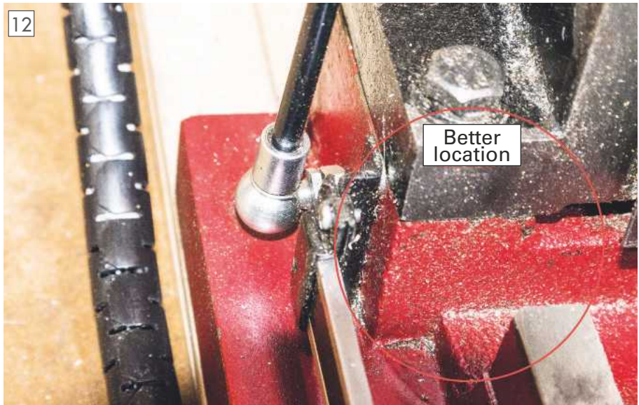
Gas strut bottom fixing, circled in red is a better area to place this end but is harder to access for drilling and tapping.
