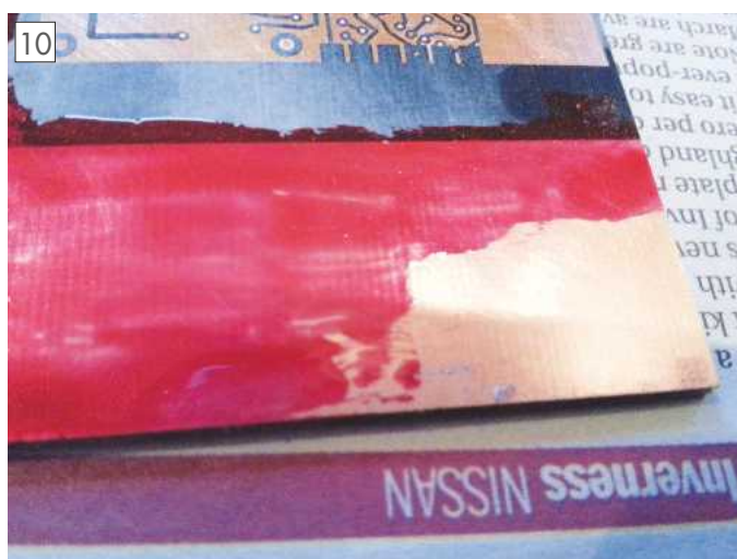
The work will be held in the etchant by a plastic clamp, and to prevent unwanted wastage of the etchant, paint over this area with nail varnish (shown red, the copper corner is as yet unpainted).
