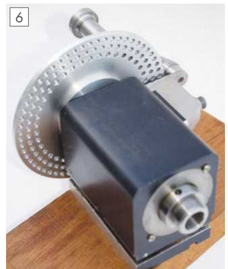
Dividing head made using a Sherline headstock.
