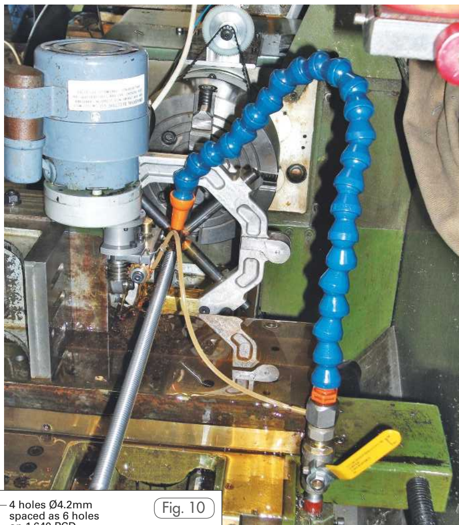
Set-up for Milling leadscrews.
