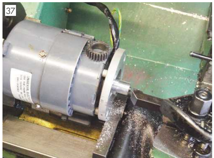
Turning the gear hub in situ on the drive motor.
