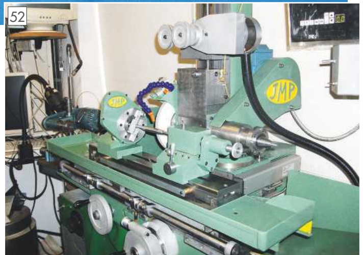
The 10 tpi screws used for down and crossfeed on Universal grinding machine.
