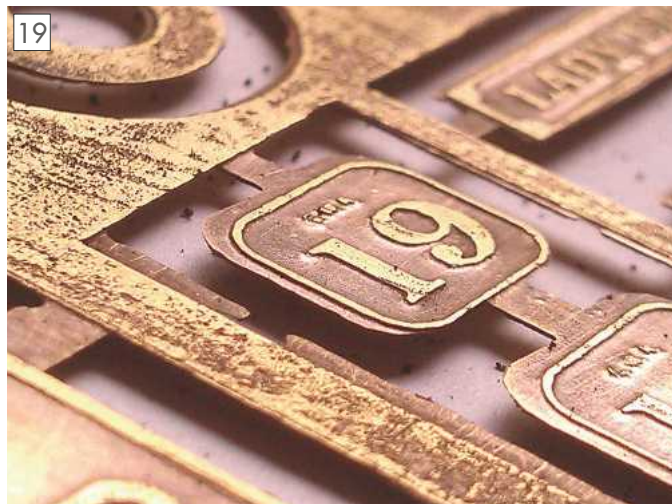
A few strokes of a needle file results in an acceptable set of plates.
