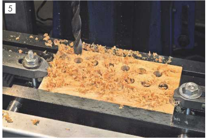
Drilling collet recess.
