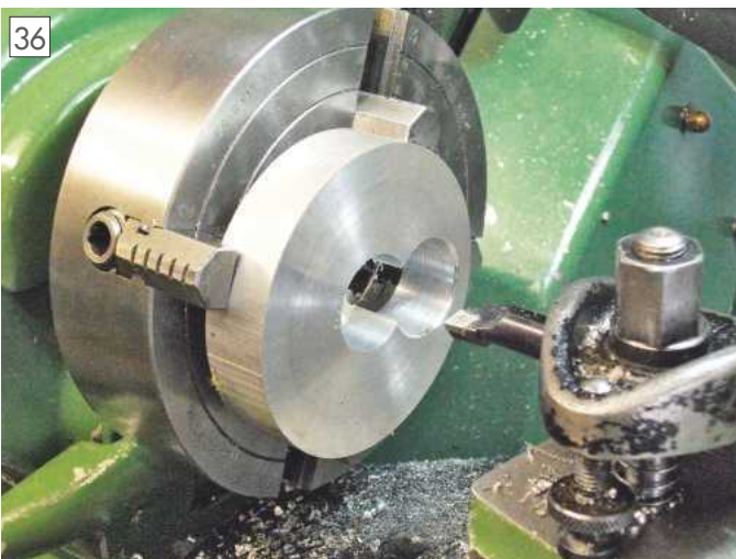
Boring the hole through the mounting plate.
