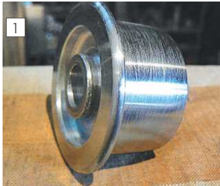
Small pulley showing radii and draft.
