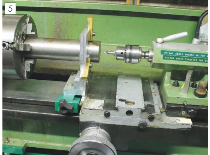
...centre drilling the bar end...
