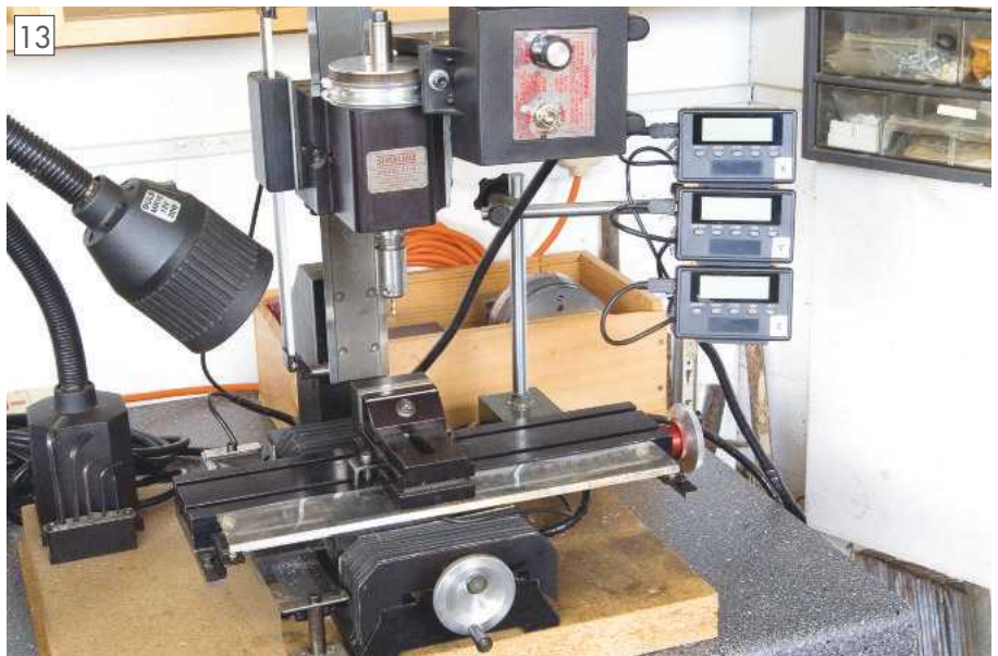
Sherline mill, now fitted with DROs and protective bellows.
