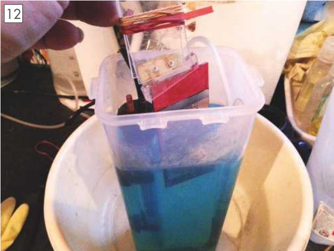
When the etchant is up to temperature pour it into the bath and, with the work clamped using a plastic menu holder or some other arrangement, lower the work into the etchant. Cover the bath to stop splashes when the aerator is turned on!
