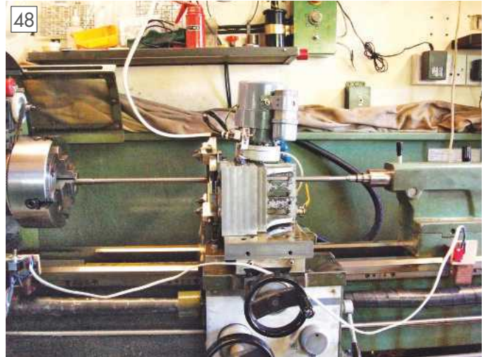
Milling a left hand 1/2 inch 10 tpi lead screw.
