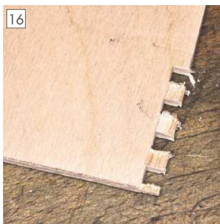
Trial cut shows breakout problems.
