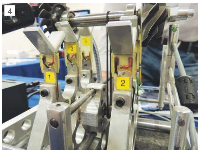
Strain gauges from piezo sounders!
