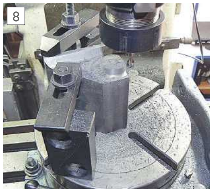
Boss parallel to parting plane.
