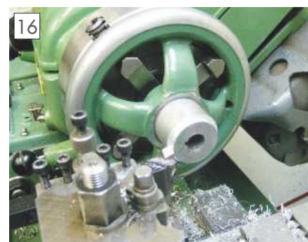
Shortening the handle so it will fit onto the end of the feed screw.
