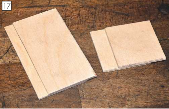
The box sides cut from 3mm birch ply.
