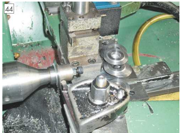
Rough cutting the form on cutter.
