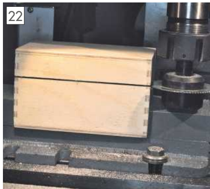
Cutting off the lid with a slitting saw.
