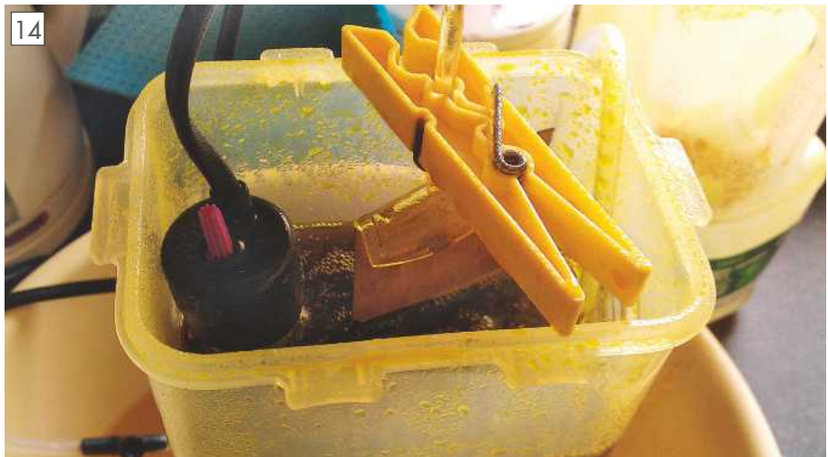
This shows an earlier process using ferric chloride and how much more difficult it is to see the work in progress.
