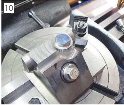
Blending a circular boss into a surface.
