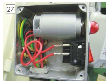
The inside of the remote switch box, showing the small transformer at the top. The small bulb screws directly into it, as does the lens assembly.
