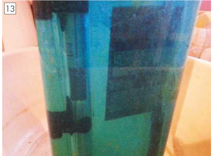
The great advantage of using sodium persulfate is that it is very transparent, until you turn on the aerator when the bubbles obscure the work! You can see the progress of the etching which accelerates towards the end of the process.
