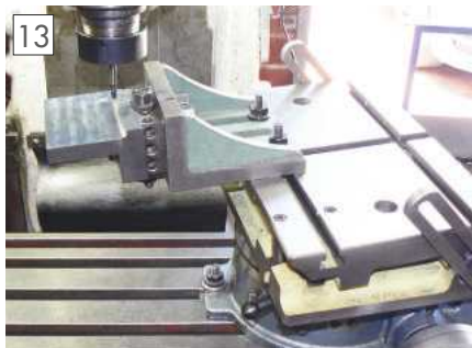
Creating a curved surface with draft.
