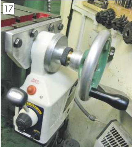
The complete drive unit in place.
