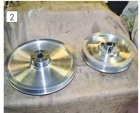
Large pulleys relieved for more uniform thickness.
