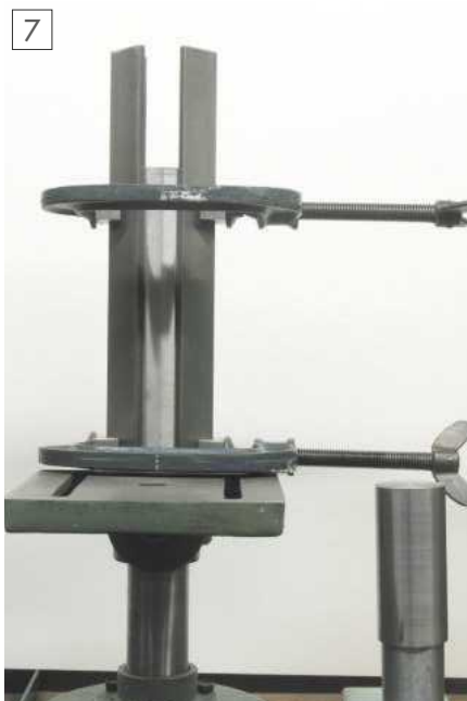
Angle, clamps & original column.
