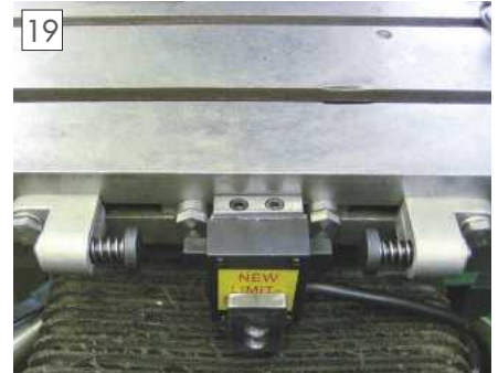
The limit switch and plungers in place. Note also the original stops.
