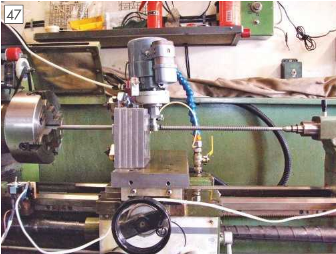
Milling a right hand 1/2 inch 10 TPI lead screw.
