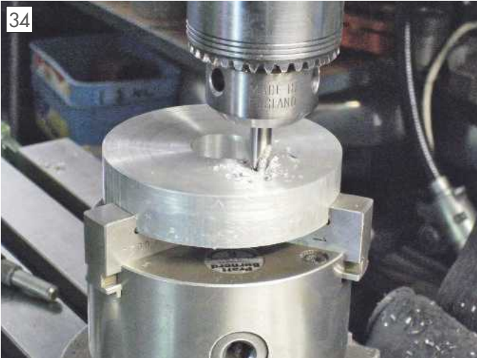
The motor mounting plate, the driven gear position marked with centre drill.
