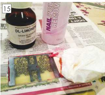
When you are satisfied that the process has completed, remove the toner resist. A combination of nail varnish and solvent, in this case Di-Limonene, is very effective but MUST be carried out preferably out of doors, or at the very least where an adequate supply of fresh air is available AND use an effective respirator to avoid breathing the fumes that the process gives off. Both acetone (nail varnish) and Di-Limonene fumes are dangerous by themselves. When used together, they are even more so. After all, if they can dissolve solid toner, think what they might be doing to you if unprotected.
