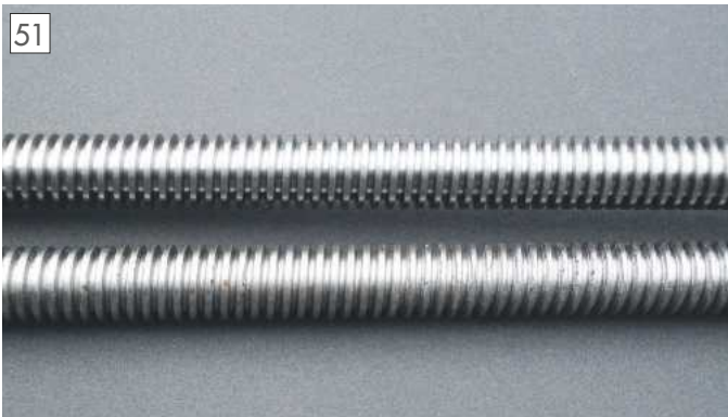
The milled leadcrew alongside the failed screwcut version.
