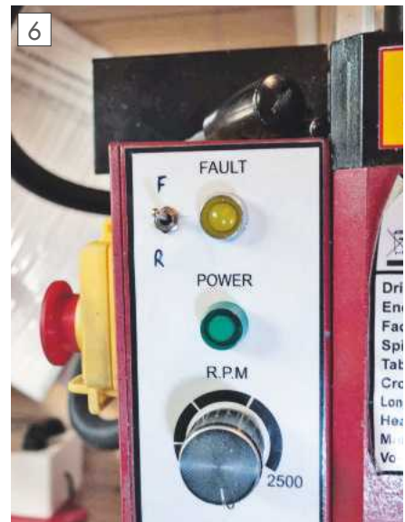
Outside of the control box with forward/reverse switch.
