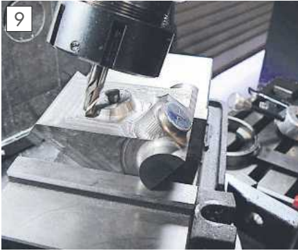
Draft on boss not parallel with parting plane.
