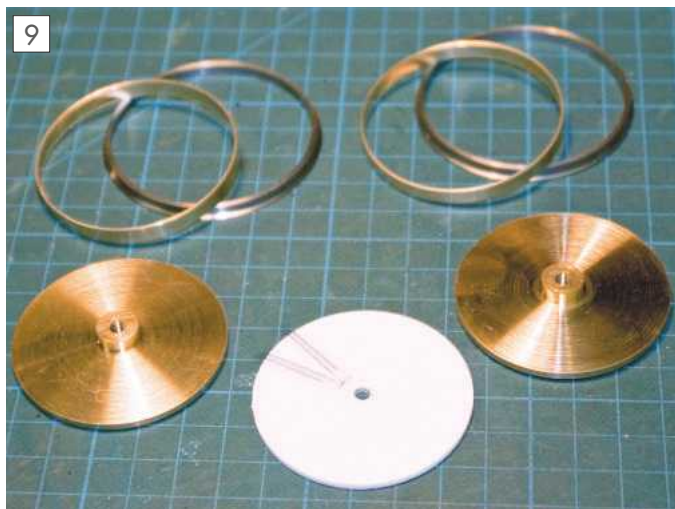
Wheelmaking. The photo shows two wheel centres that will be cut for the spokes, and two rims that will be soldered on when the spokes are cut. The plastic disk is one I used to make sure the slitting saw settings on the mill were correct before cutting metal.
