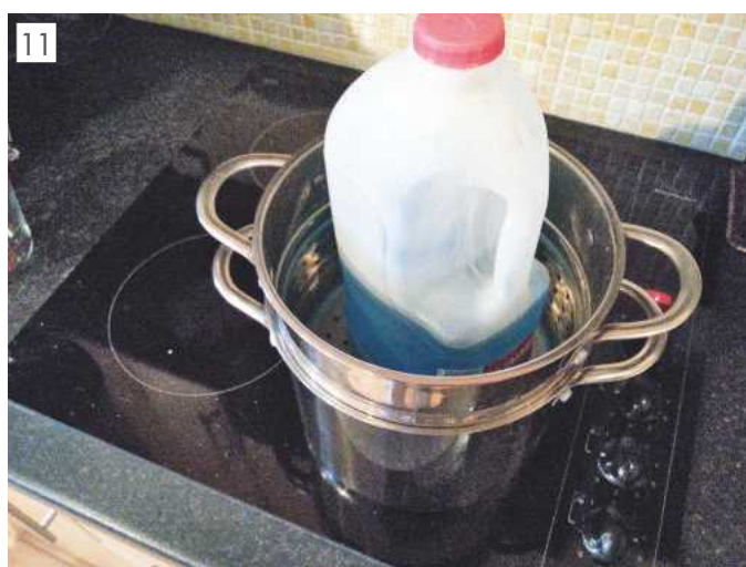
Warm the etchant in a bath of hot water to bring its temperature up to around 50 degrees celsius. Making it hotter will not benefit the process and making it colder will lengthen the etching time.
