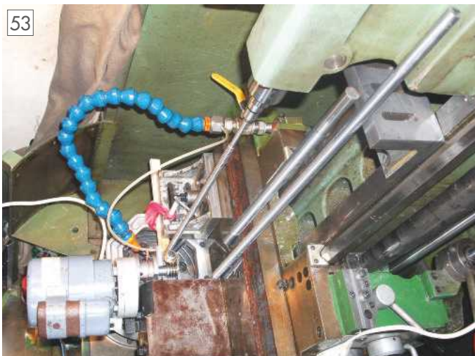
3/8, 1/2, 5/8 inch 10 tpi milled leadscrews for shaper machine.
