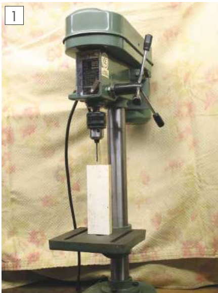
Finished extension showing extra height gained.
