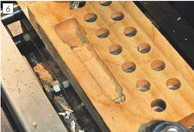
Collet holes and chuck seat left by the milling cutter.
