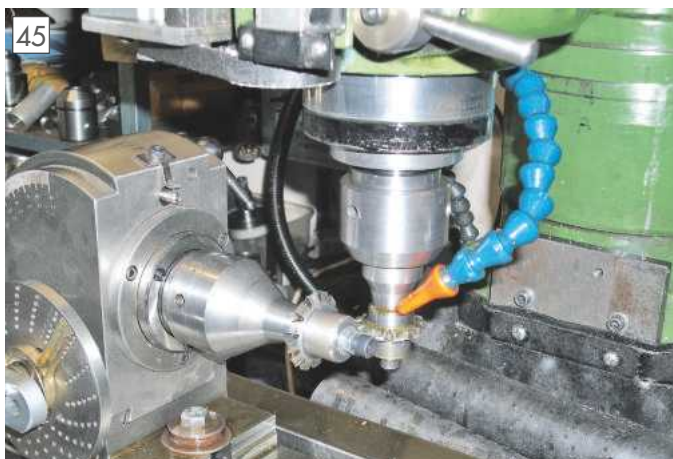
Gashing the tooth spaces on the partly formed cutters.
