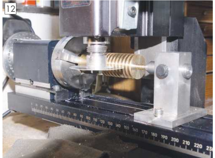
A batch of carrying wheel centres being cut out together.
