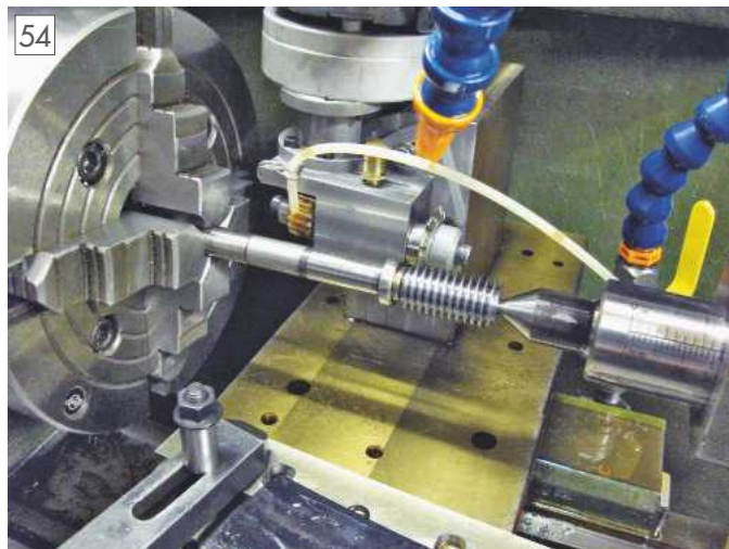
A cnc milled 1 module worm being cut.
