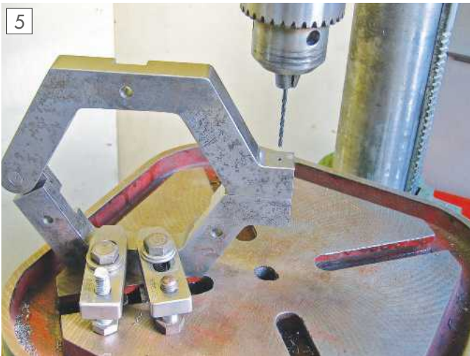
Drilling for clamp bolt hole.
