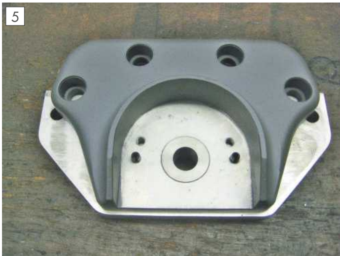
The supplied end plate located over the new plate by means of the bush, thus ensuring the fixing holes are accurately positioned.
