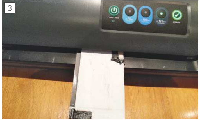
Inserting the prepared work into the converted laminator. The tape that holds the printed photopaper in place will be melted but does not seem to adversely affect the laminator. Two or even three passes will ensure that the toner has melted on to the copper satisfactorily. Only apply the fixing tape to the leading edge of the prints and workpiece as they will enter the laminator. A piece on, say, the trailing edge may well come adrift in the hot laminator and be the very devil to remove!
