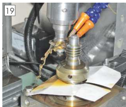
19 CNC milling the 1.25 module worm.
