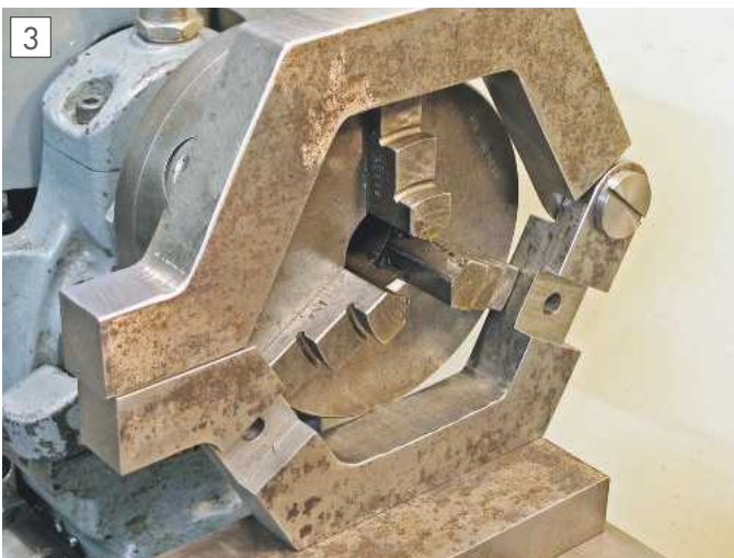
Using chuck jaws for marking out the finger slots.
