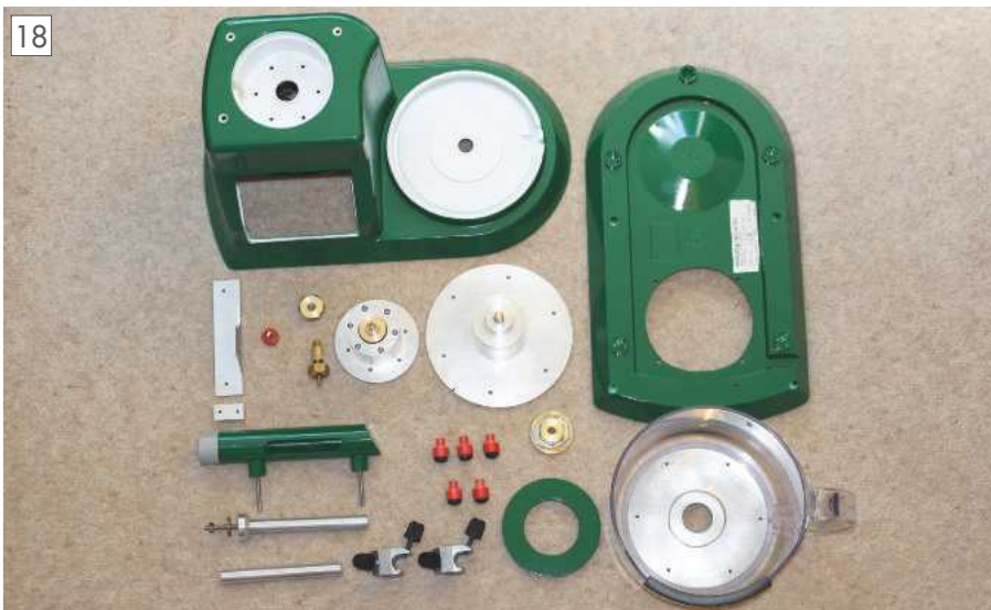
18 Major components used in converting the Morphy Richards food processor into the MincerMultiGrind.
