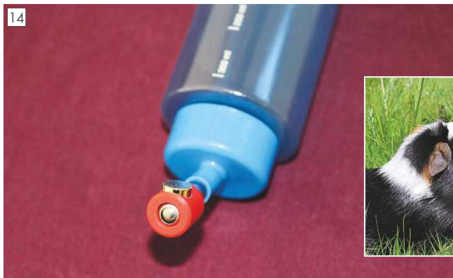
Close-up of the MagnaDrip control valve on the guinea pig water bottle. A rare earth magnet slides up and down the exit tube, positioning the steel ball that controls the flow.
