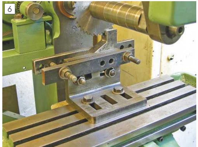
Milling out the slot for the clamp bolt.
