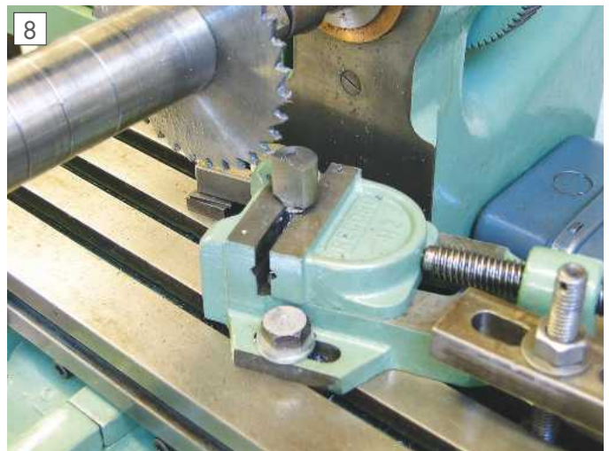
Forming pivot end of clamping bolt.
