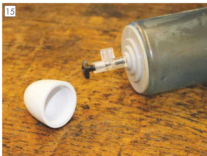
An aquarium air valve is fitted to the top of the water bottle to control release of the vacuum, thus adding another means of regulating the flow. This valve is enclosed by a plastic radiator cap.
