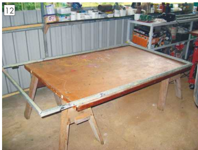
The first frame, welded up.
