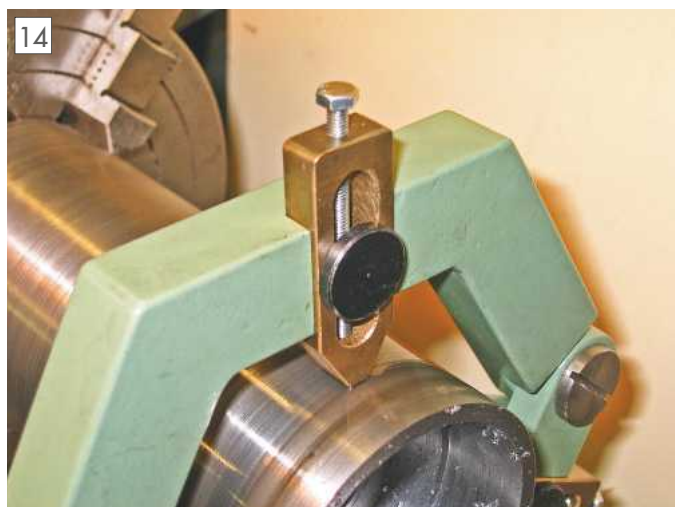
Mod 2, fit screw adjusters to fingers.
