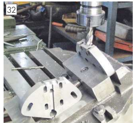
Milling clearance for worm and housing on mounting bracket.
