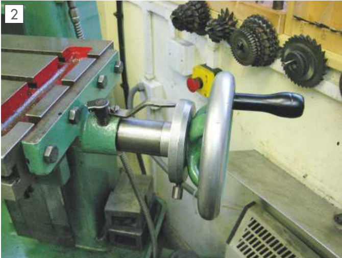
The original winding handle assembly as fitted to the machine.
