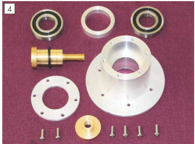
Components of the high speed spindle (the low speed is similar). When assembled, compression of the O-ring pre-loads the ball bearings, minimising free play of the shaft.
