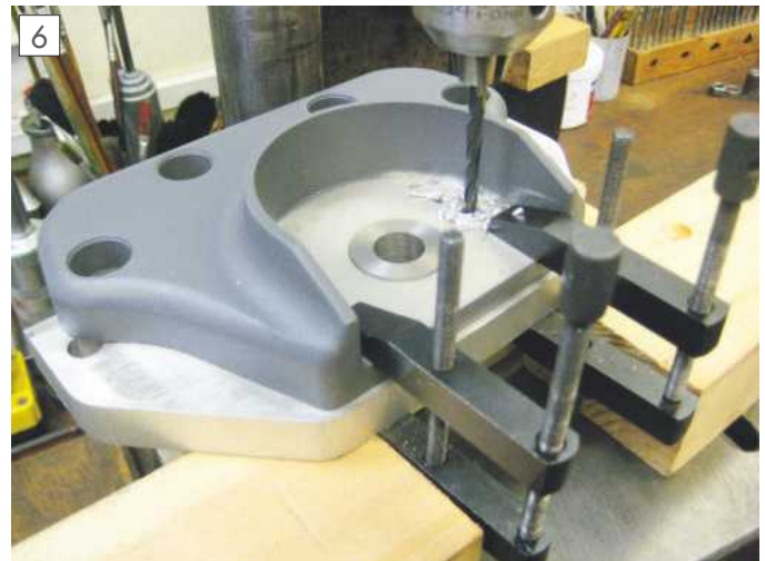
Drilling holes for the roll pins, using the original roll pin holes as a template.
