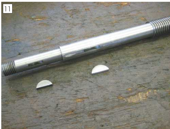
The finished shaft, complete with the two keys and keyways.
