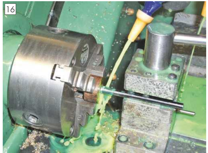
16 Boring out the taper on the wormwheel blank.
