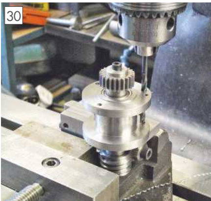
Spotting through wormshaft mounting holes into spindle block.
