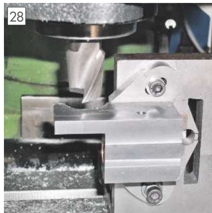
Final cut for location diameter.
