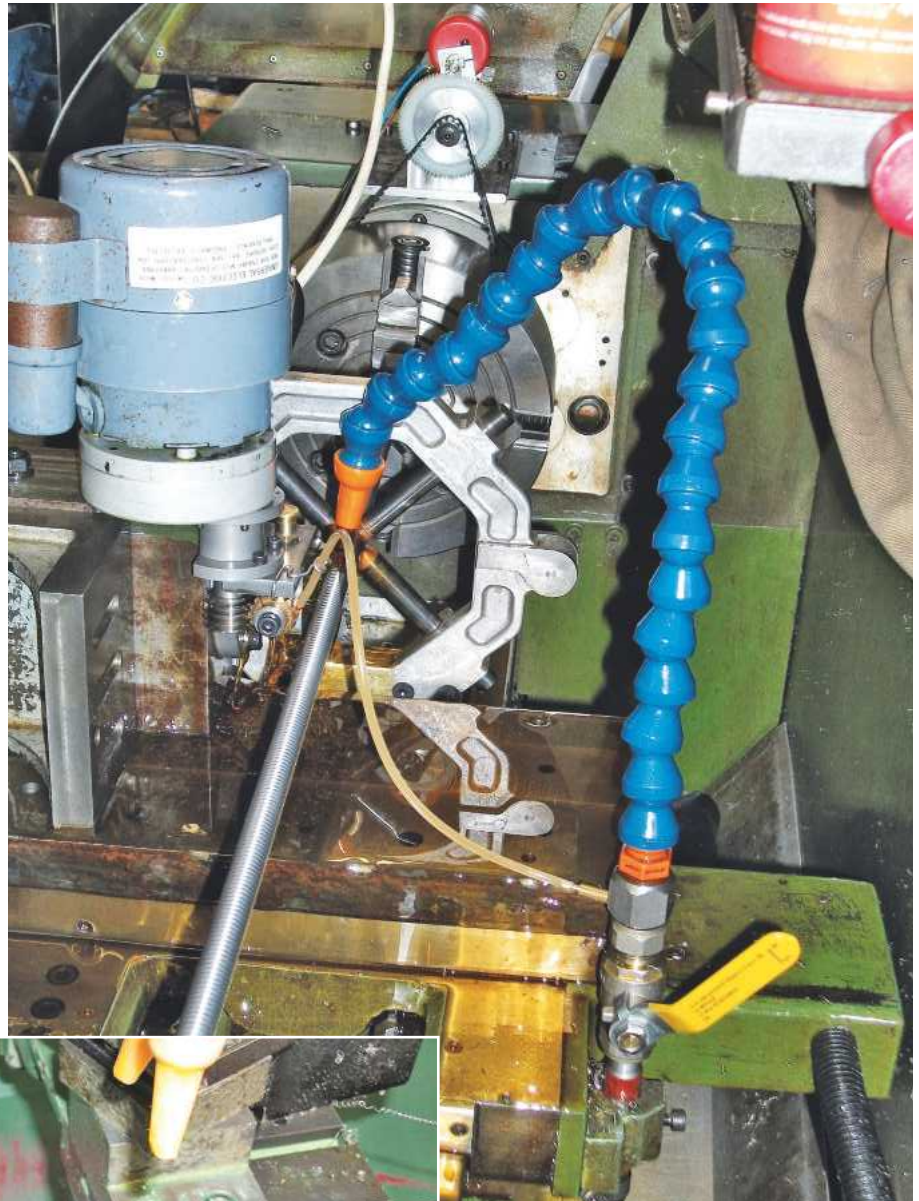
Set-up for Milling leadscrews.
