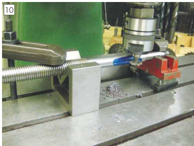
Machining the woodruff keyway on the milling machine.
