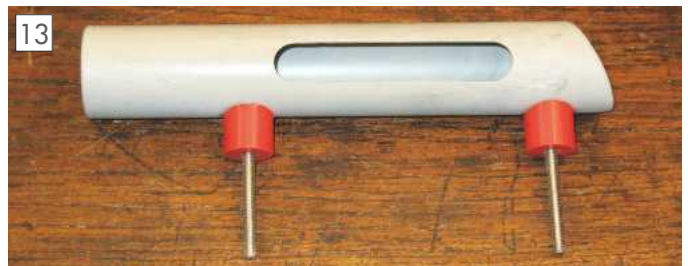
13 Dust extractor module for the high speed spindle, made from the centre tube of a fax paper roll.
