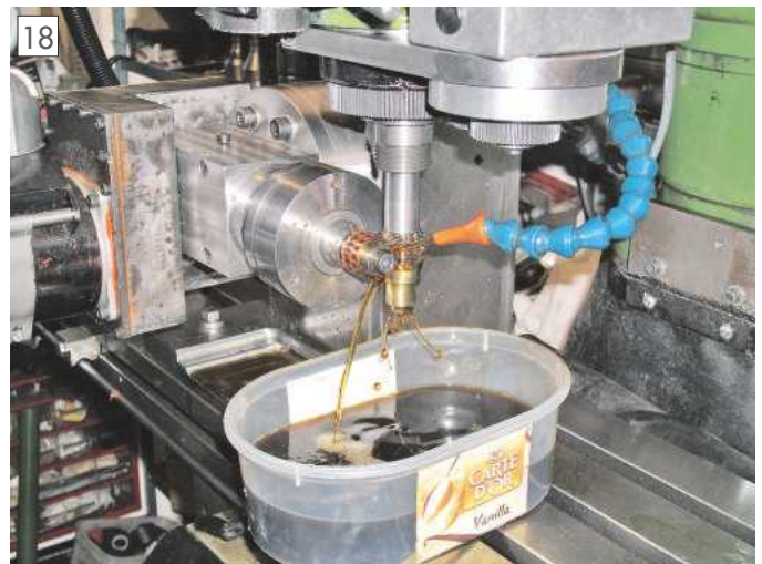
18 Hobbing the wormwheel 1.25 mod.
