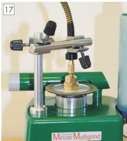
17 Tool rest bar in the upper position with a retort clamp for holding the Proxxon Flexishaft body. A Permagrit file collet fitted to the wheel nut provides drive to the shaft.
