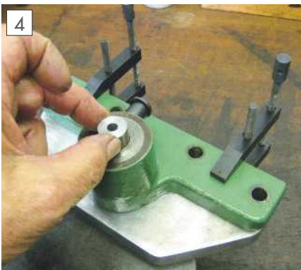
Placing the bush into original end plate to ensure accurate location of the hole for the power feed unit bearing.
