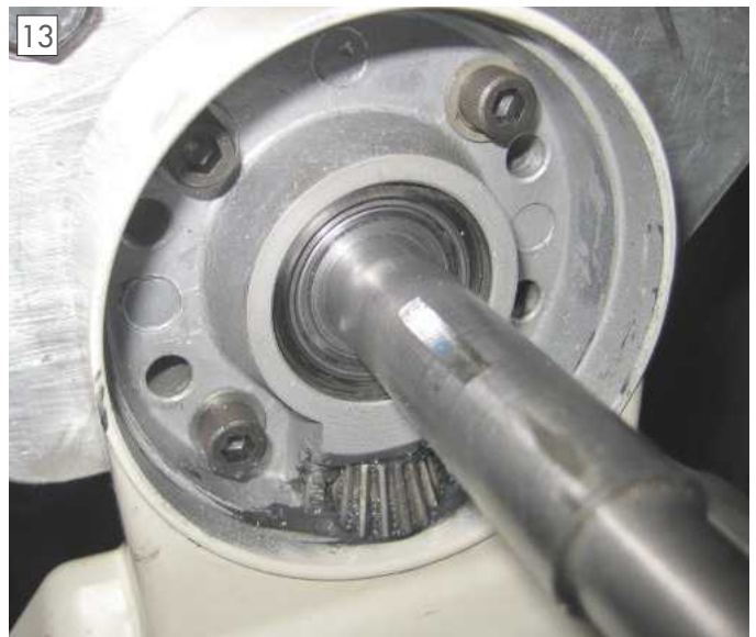
The power feed unit in place, with the bearing seated on its inner ring.
