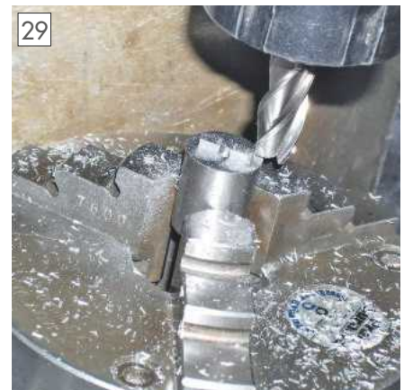
Milling the keyed washer.
