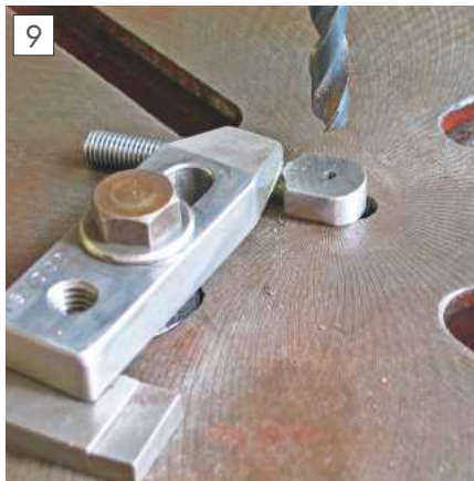
Drilling pivot hole in clamping bolt.
