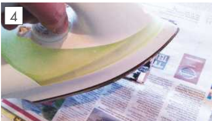
The hot iron (not quite at its hottest setting but almost) pressed firmly on to the work after it has been through the laminator will add to the assurance that the toner has adhered to the copper.
