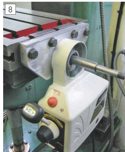
The unit bolted in place on the end of the table, using the original bolts.
