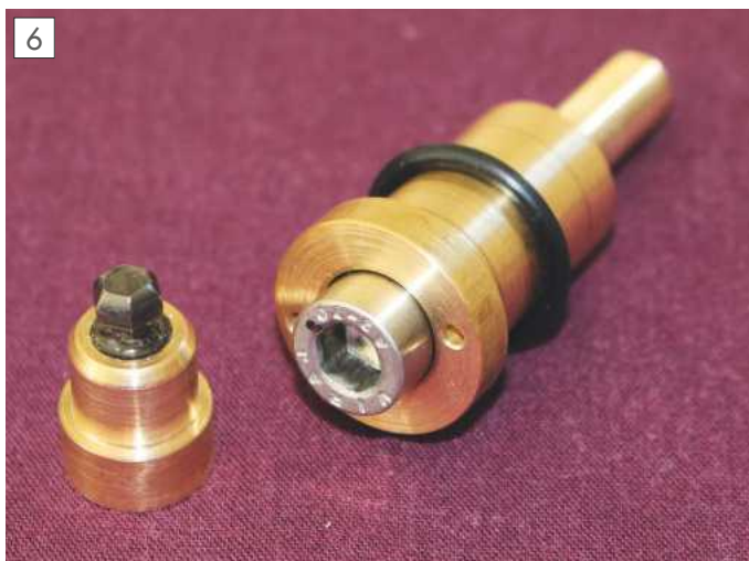
Close-up of the components for coupling drive from the motor to the shaft of the high speed spindle. This is based on an 8mm socket screw and matching ball-ended Allen key.
