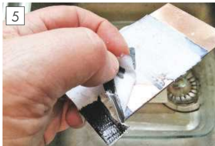
The paper on which the image has been printed can now be removed to leave the melted etchant adhered to the copper. Soften the paper with warm (but definitely NOT hot!) water and GENTLY rub the wet paper to remove it. Take your time!
