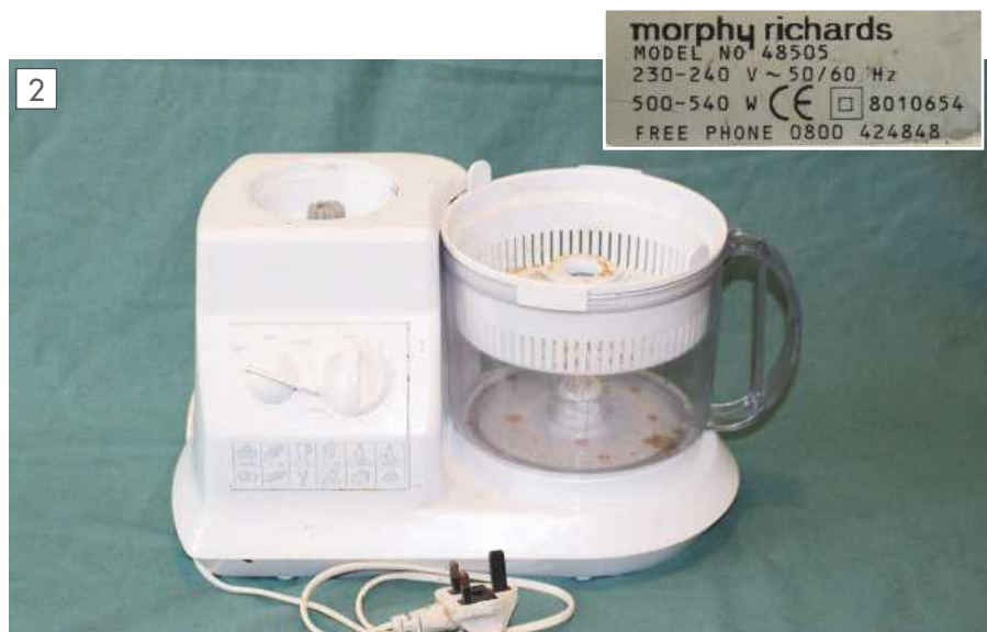
The 1998 Morphy Richards food processor as recovered from the amenity site. Note that the high speed blender jug is missing. The surviving low speed jug was used as the basis for a wet grinding vessel.
