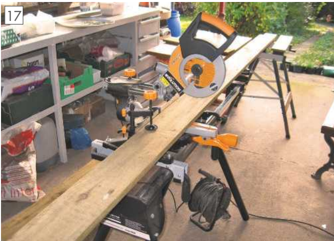
Cutting the timber to length.
