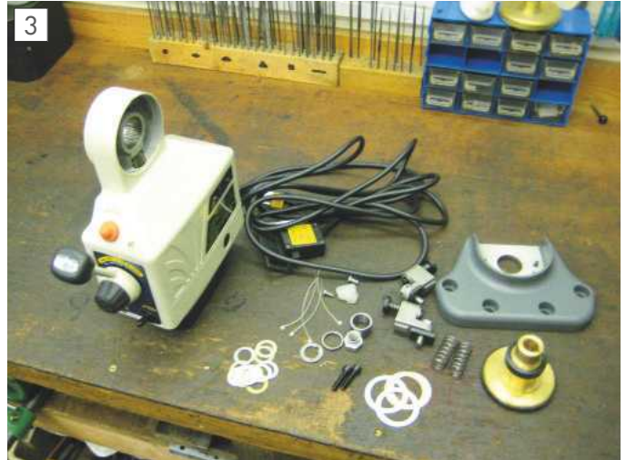
The parts of the power feed unit kit as supplied.
