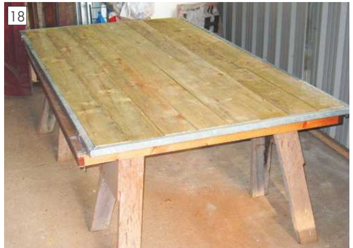
Timber fitted to the frame.
