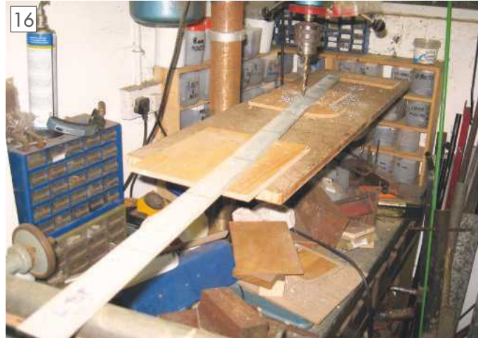
Drilling the supports.
