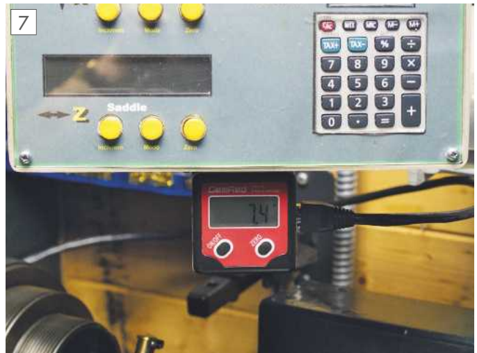
Digital rotary encoder.
