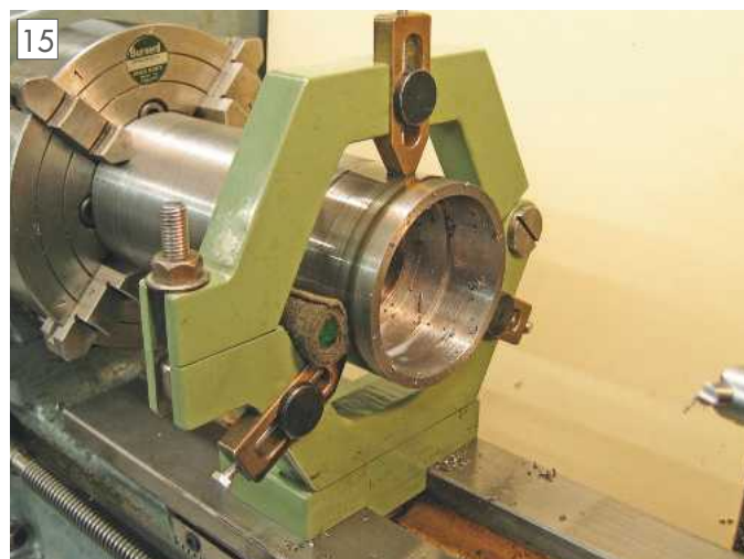
Turning 3 inch diameter.
