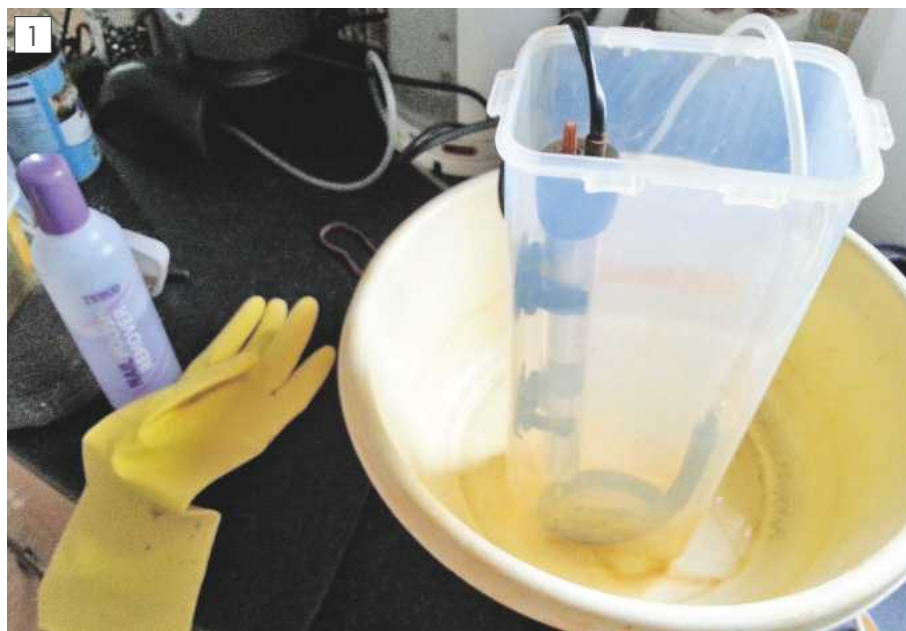
The etching bath, showing the spaghetti jar with the aquatic aerator in place. The bath is placed in a bowl to catch any etchant splashes. The all-important rubber glove is at the ready!
