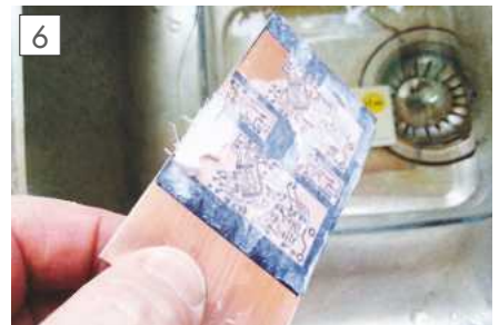
The paper on which the image has been printed can now be removed to leave the melted etchant adhered to the copper. Soften the paper with warm (but definitely NOT hot!) water and GENTLY rub the wet paper to remove it. Take your time!
