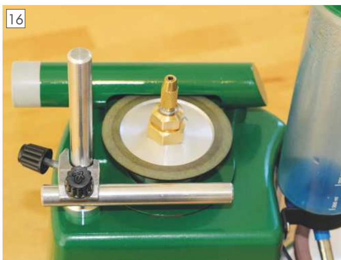
Tool rest bar in the lower position for tool sharpening on the high speed wheel.
