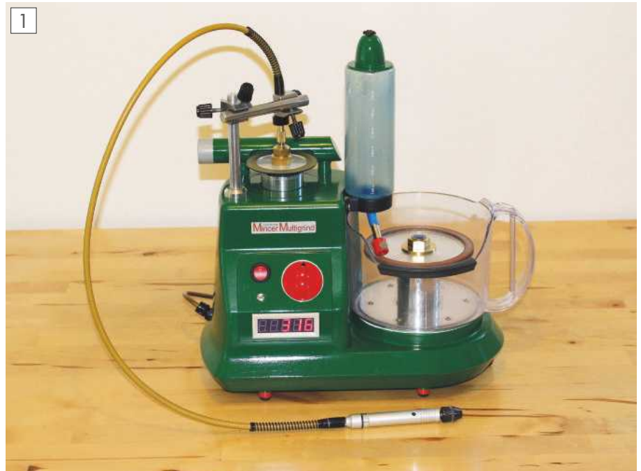
The completed MincerMultiGrind, with Proxxon flexible shaft attached using the high speed wheel collet fixture.
