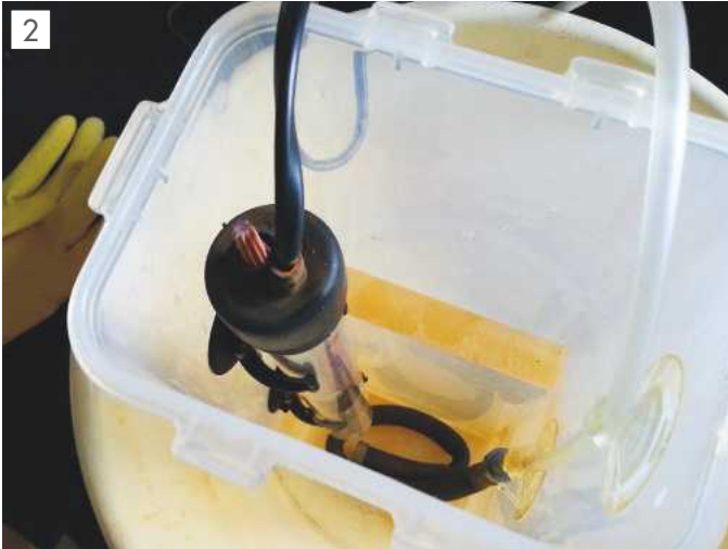
A 12mm thick piece of perspex has been placed in the spaghetti jar both to add weight (to prevent the bath being top heavy when the etchant is added) and to take up volume to reduce the amount of etchant needed to cover the work.
