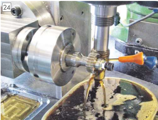
Hobbing the 23 tooth gear.
