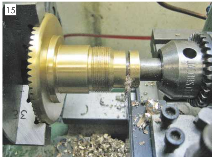
Parting off the gear. Note the stationary mandrel which supports the end of the gear.
