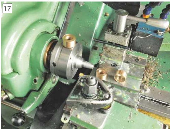
17 Three wormwheel blanks and turning mandrel.
