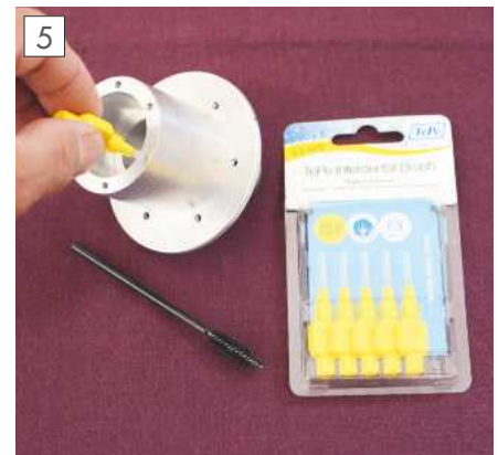
Cleaning blind threaded holes in the spindle casing using an interdental brush. For larger tapped holes a mascara brush comes in handy.
