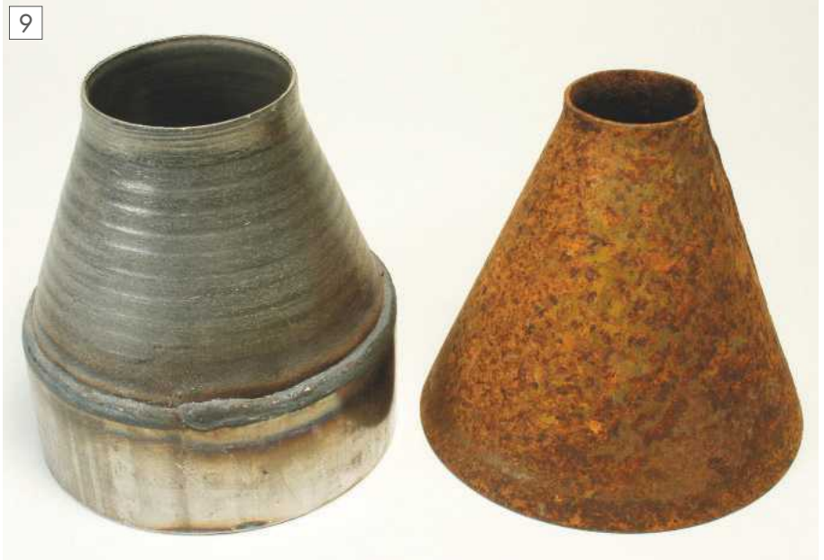
Two commercially-made cones, each showing the small parallel section at the small end which helps when welding the cone to an exhaust pipe.
