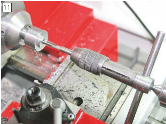
Tapping for securing screw.
