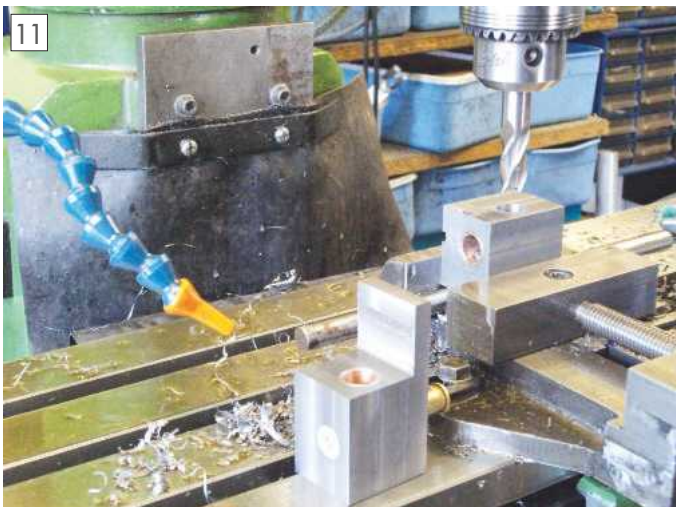
Boring out the oil chamber.
