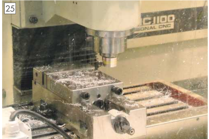
The mill set up as a lathe with the TTS holder in the spindle and the cutting tool set in the machine vice.
