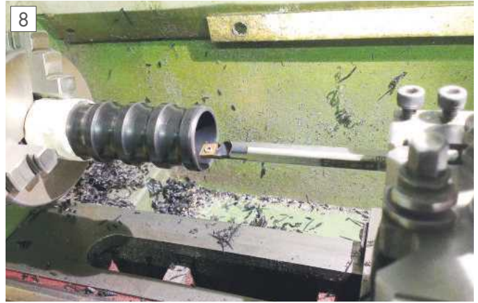
Boring out the bulk of the hand grip. Lots of overhang but no vibration.
