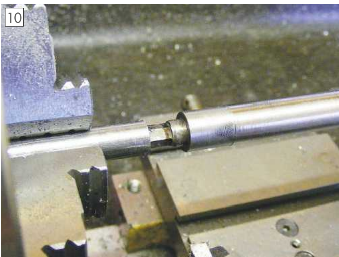
The lathe set up for rotary broaching.
