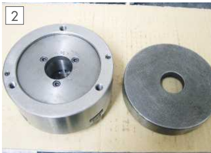
The rear of the chuck and the plain face of the backplate, as supplied.
