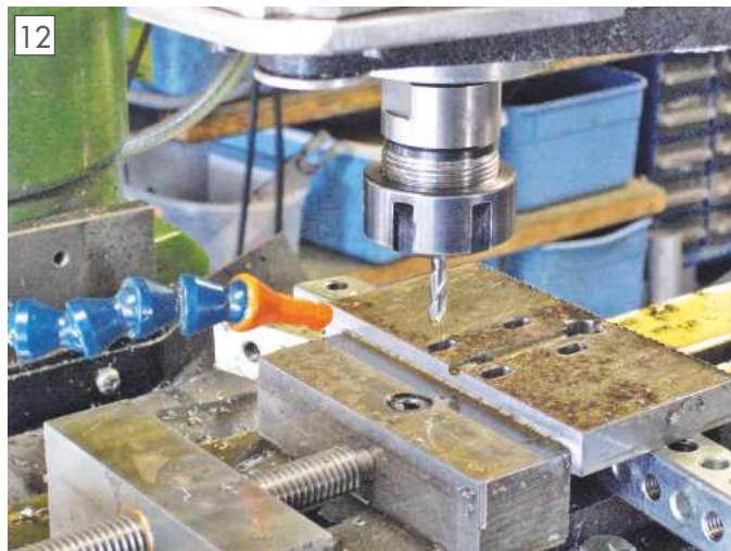
Milling out the slots mounting plate.
