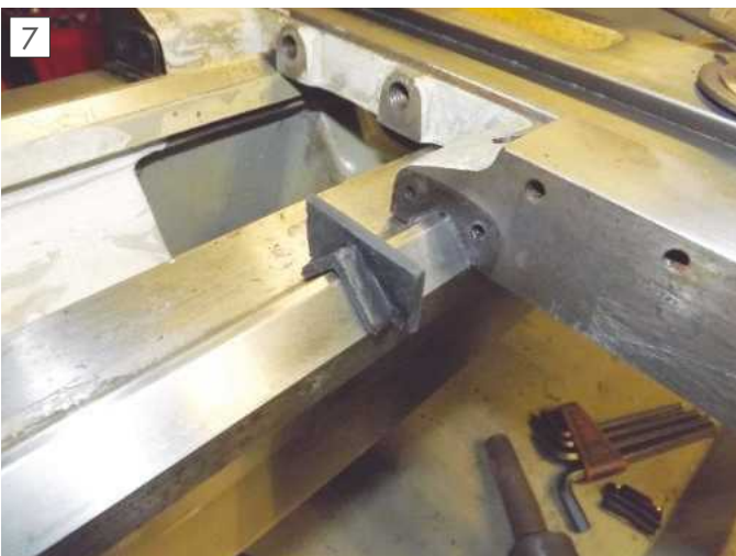
The wiper was left for a day to allow the cure to complete.
