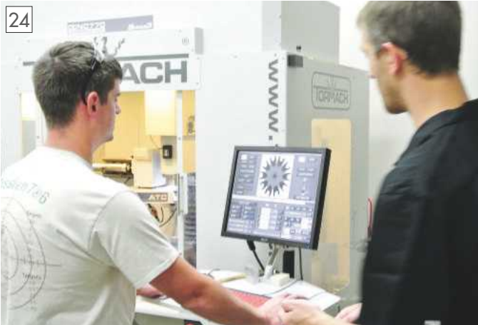
Jason Showing one of the attendees how to load the ATC and enter its dimensions in the tools library.
