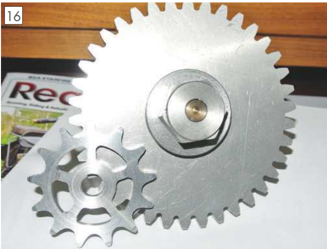
The large gear was cut with a round nosed end mill because that was the only small cutter available, hence the wrong root profile.
