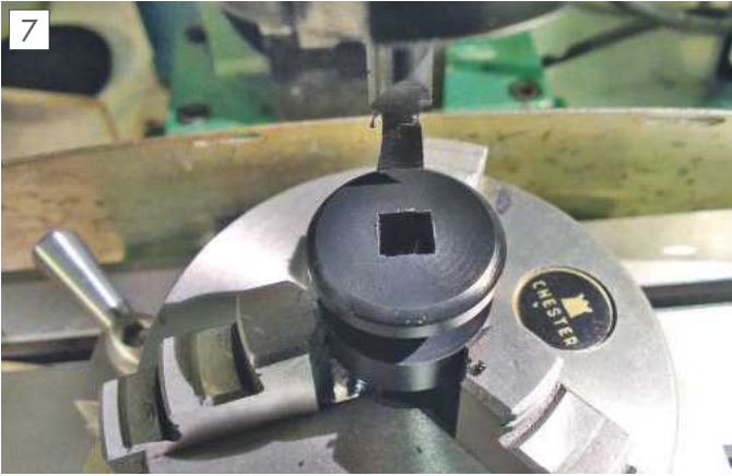
Using slotting tool to form square hole in the zoom wheel.
