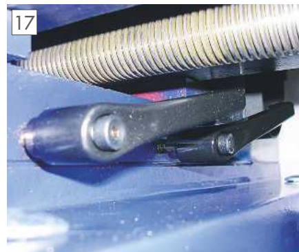
Indexable locking handles for the y-axis.
