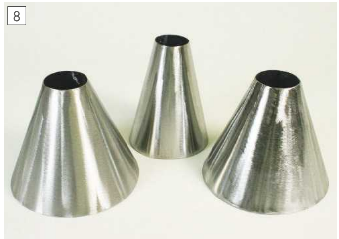
Two truncated cones rolled from 0.7mm and 1mm sheet (on the left and right respectively) and a third (centre) truncated cone with a smaller half-angle.
