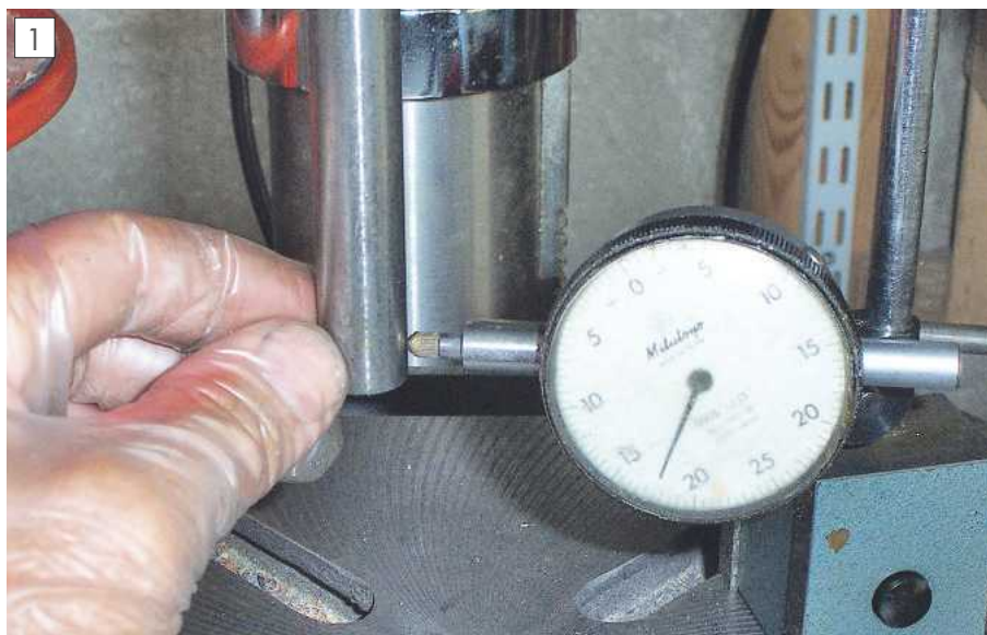
Checking play with a clock gauge.
