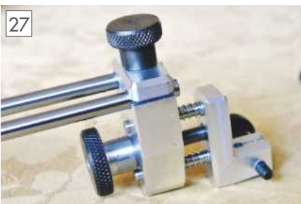
The DTI Holder (On right hand end) and the Block (Larger item below the rails).
