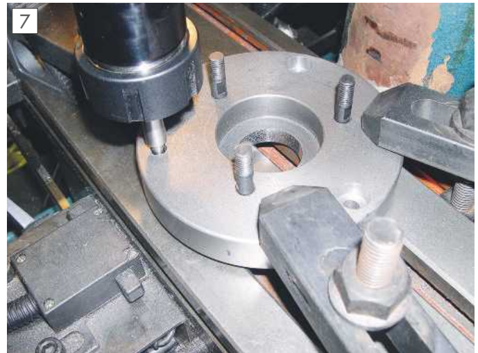
Drilling the new holes using co-ordinates.
