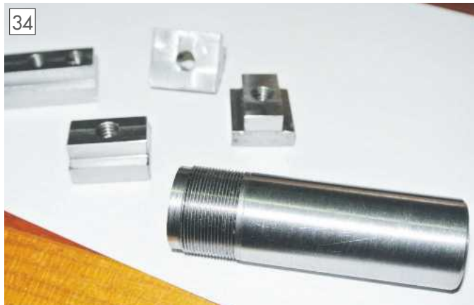
The Tee Nuts and Motor Cycle inlet tube made using conversational programming.
