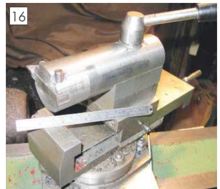
Cylindrical tool post for the larger female nosepieces.
