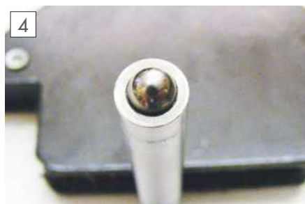
The other end of the cutter showing the conical hole.
