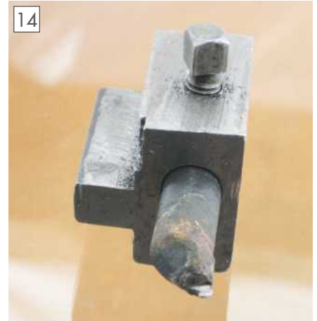
Boring bar made to fit the small female nosepieces.
