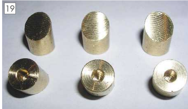
New 'bullets' for locking handles.
