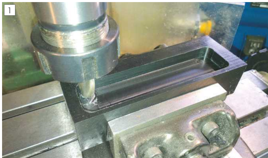
Roughing out the base from Acetal block with 12mm slot mill.
