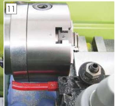
Reducing the backplate diameter to match the chuck.
