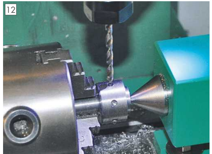
Holes for clamping bar.
