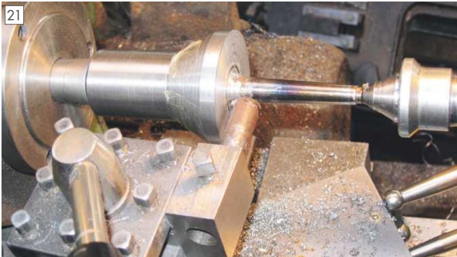
Male nosepiece held between a female nosepiece and tail stock while finishing.
