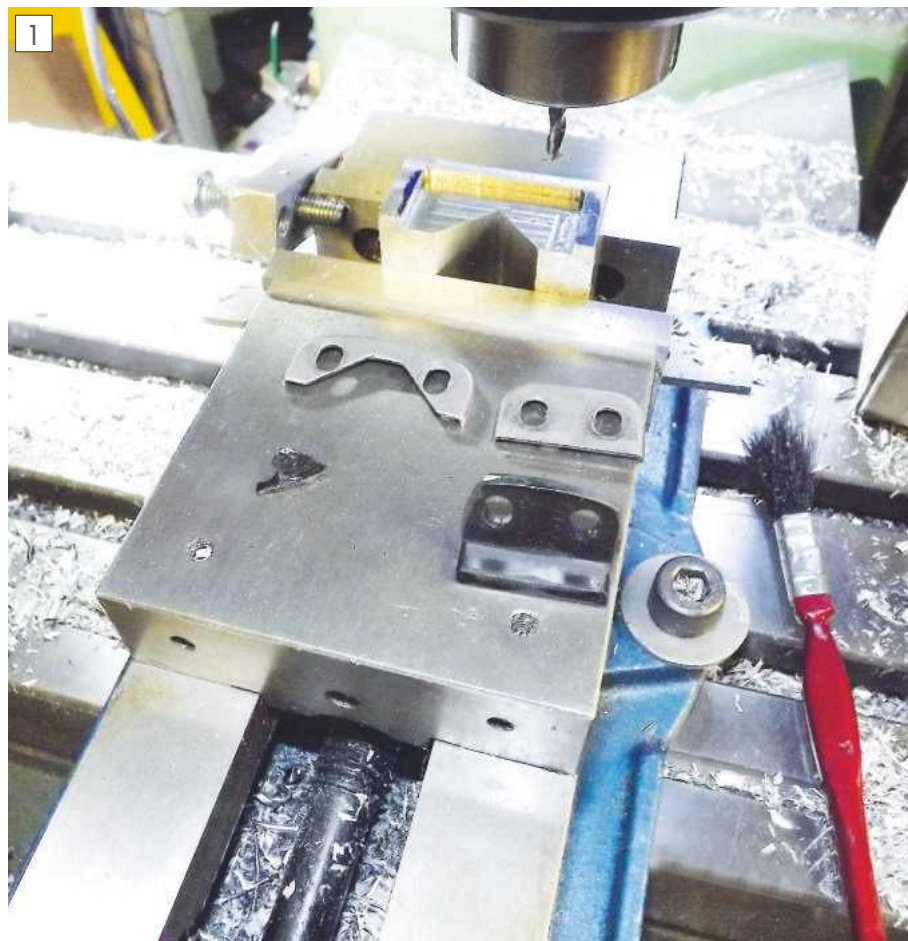
The front and rear wiper clamps and the remaining rear wiper.
