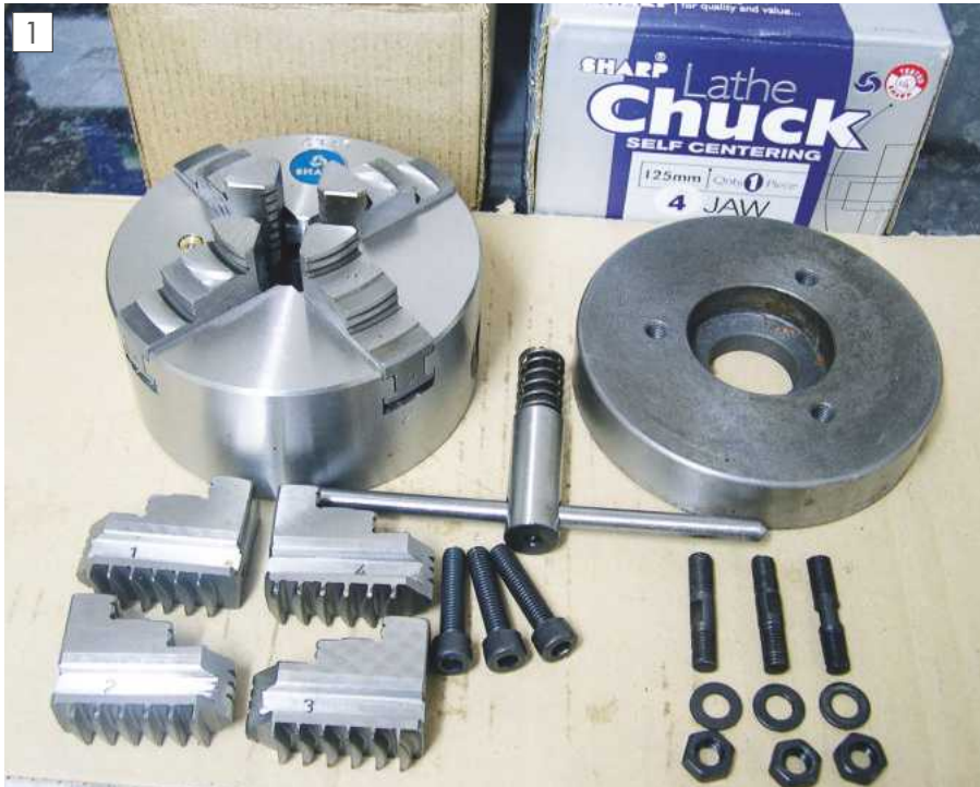
The supplied chuck and the backplate before fitting.
