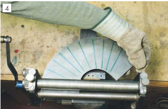
An overhead view of the rolls and the sheet positioned ready for rolling.
