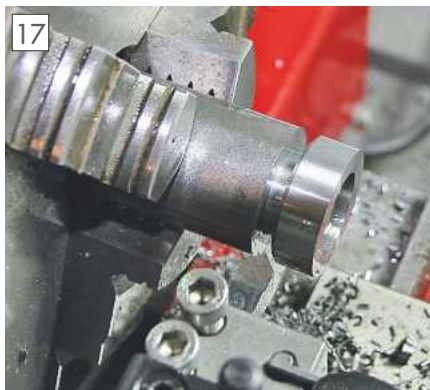
Chamfering before completing parting.
