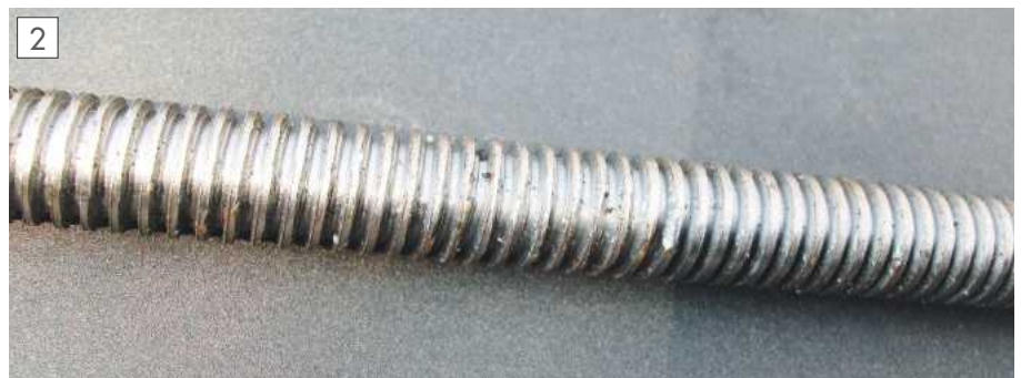
Damaged screwcut leadscrew.
