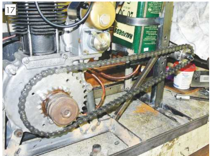
Sprockets made on the Tormach and drawn up using Gearotic.
