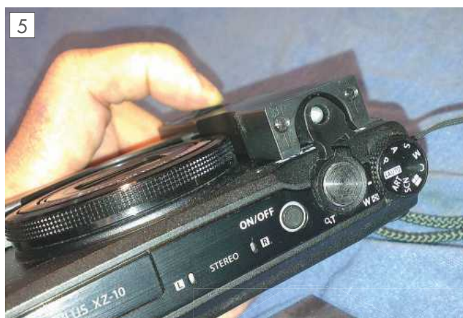
Top view showing fork action on zoom control and shutter button push rod.
