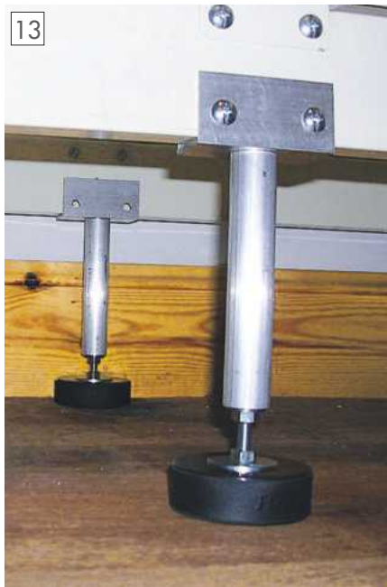
Extra supports for the centre of the workbench.
