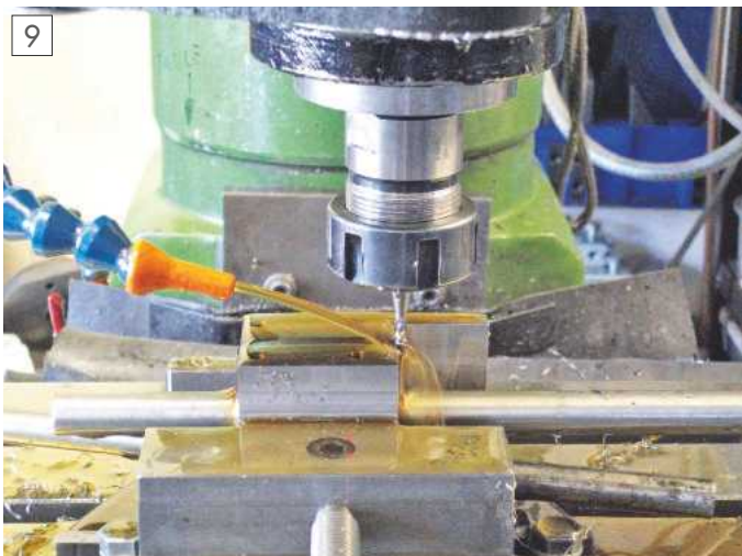
Milling the key slot.
