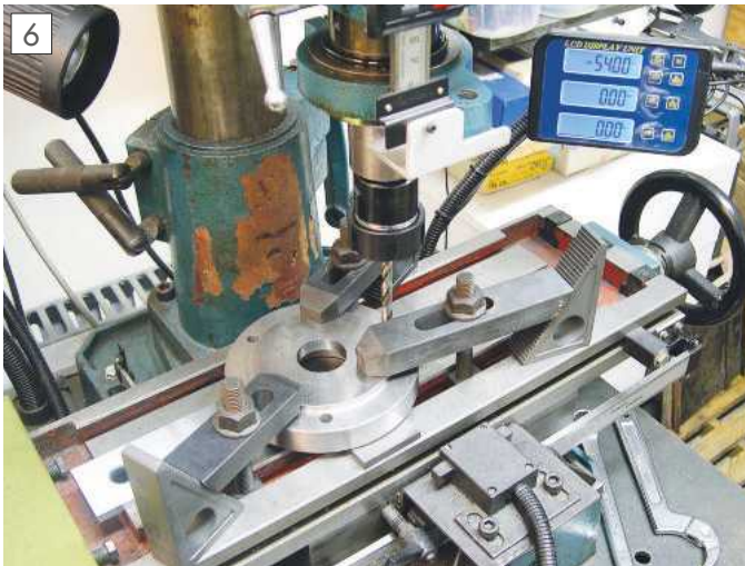
Setting up to drill chuck mounting holes.
