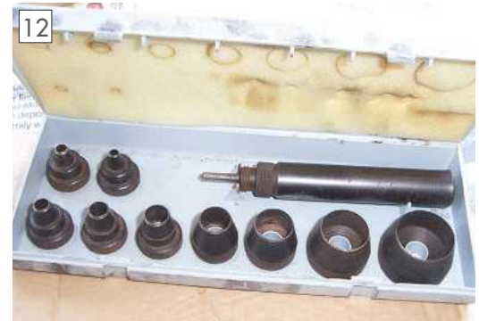
12 Use of wad punch to produce clean holes in card.
