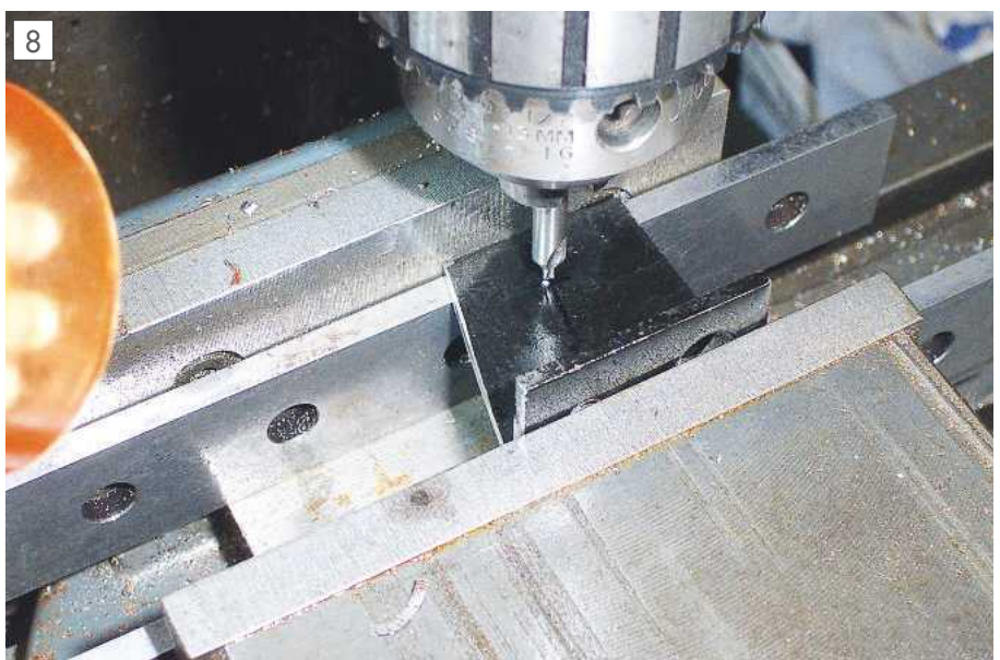
Utilising parallels to drill square.
