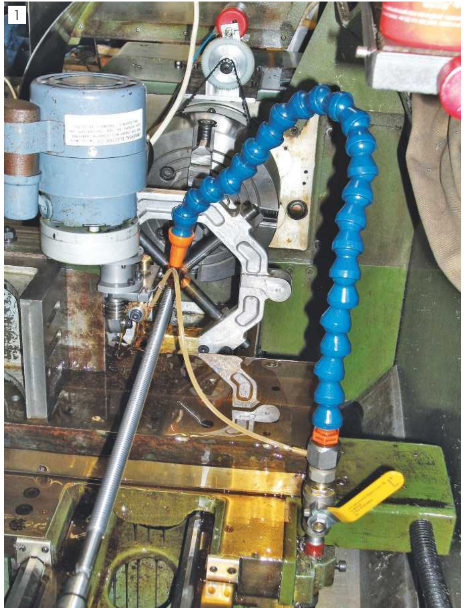
Set-up for Milling leadscrews.
