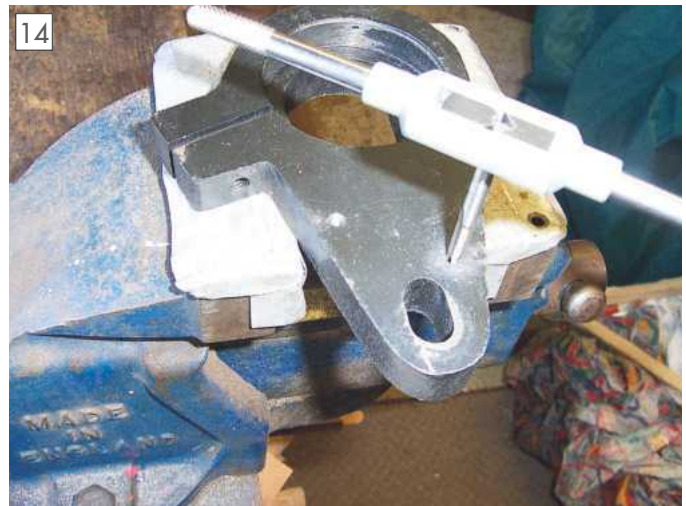
14 Tapping the screw holes in the yoke: the substantial nature of the yoke.
