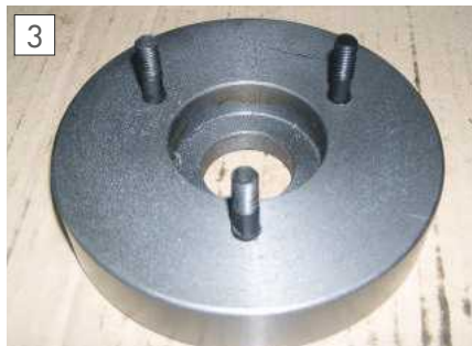
Studs fitted to the backplate.
