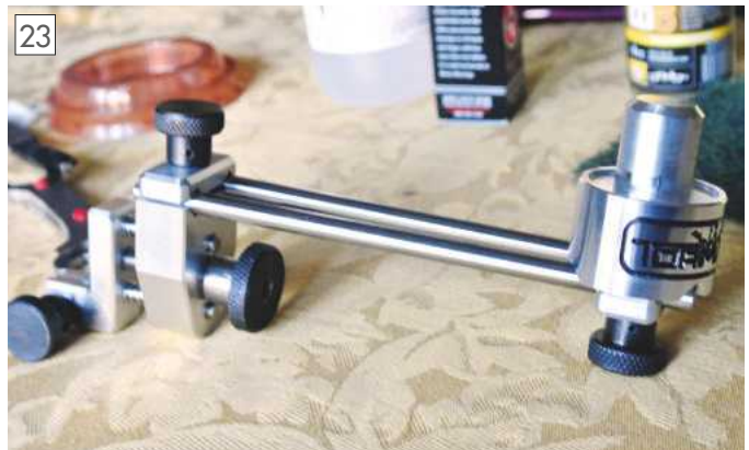
The Swing Indicator holder that is made during the workshop.
