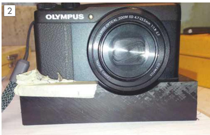
Relief radius cut into base for the lens rotating bezel.
