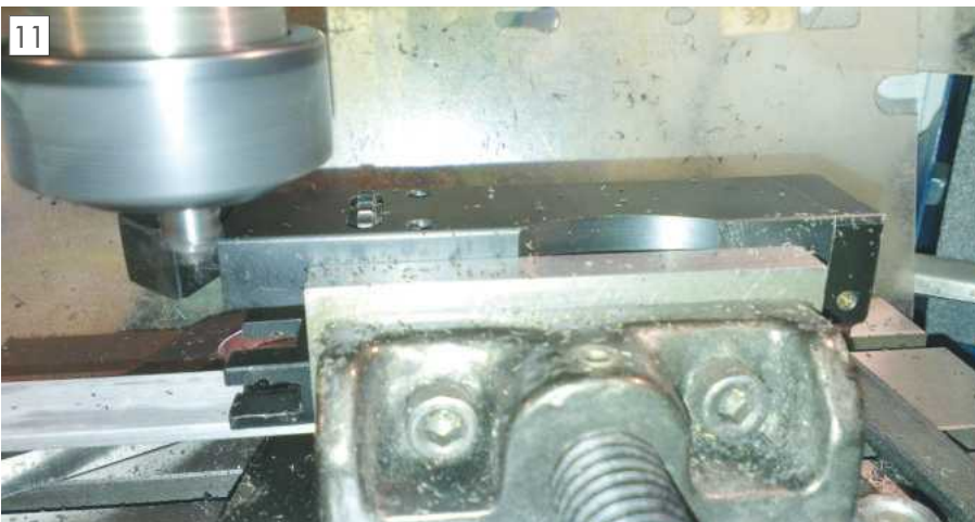
Using the homemade radius cutter.
