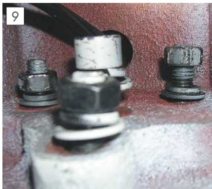
The four bolts securing the spindle head to the z-axis saddle.
