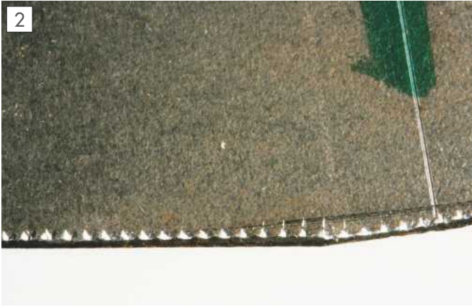
Aircraft-style snips leave serrations along a cut edge.
