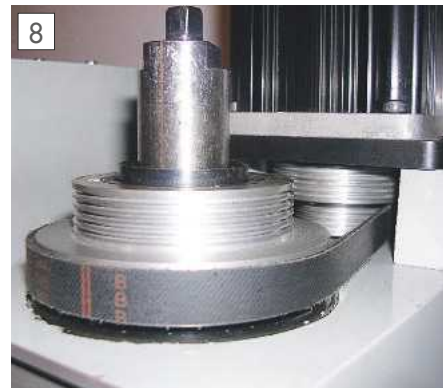
View of the belt drive.
