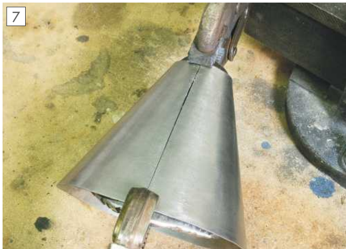
The ends of the seams can be clamped onto pieces of curved steel in preparation for welding.
