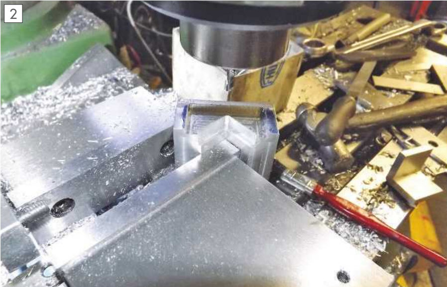
The block with vee and pocket.
