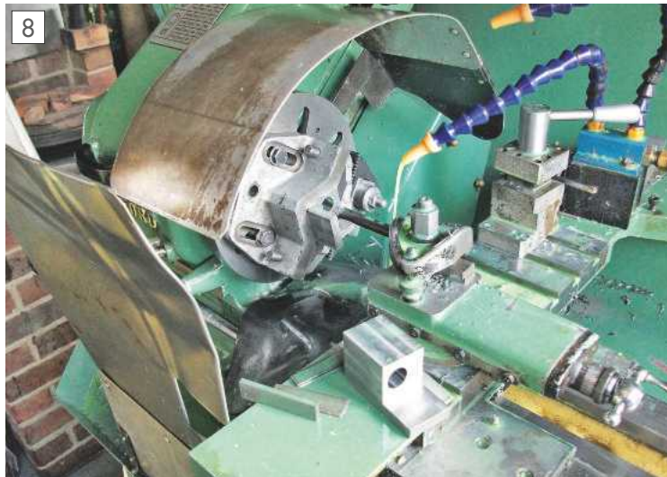
Boring the spindle mounting block.
