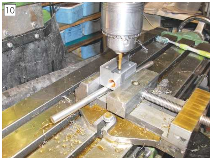
Tapping the mounting holes spindle block.
