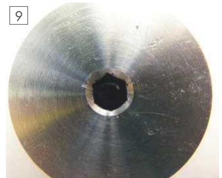
The completed hexagonal hole.
