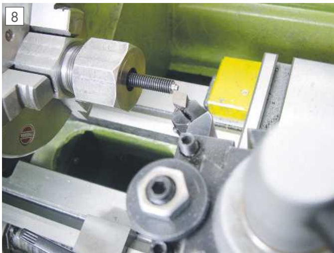
Using a 'lantern chuck' to hold screws for shortening.
