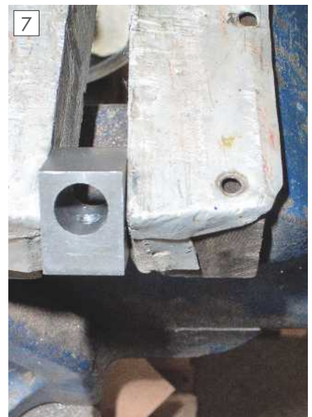
Burr thrown in the stabiliser housing by tapping.
