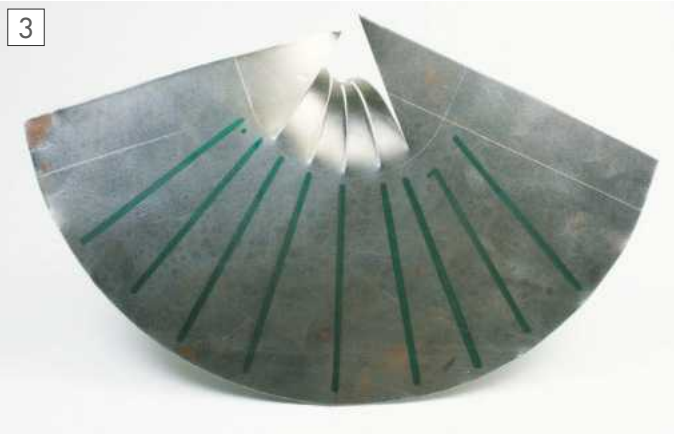
A series of radial cuts will help reduce distortion when removing the smaller area.
