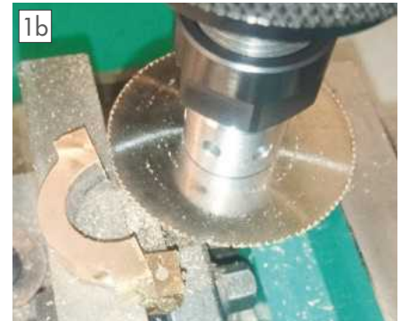
Splitting an eccentric strap.
