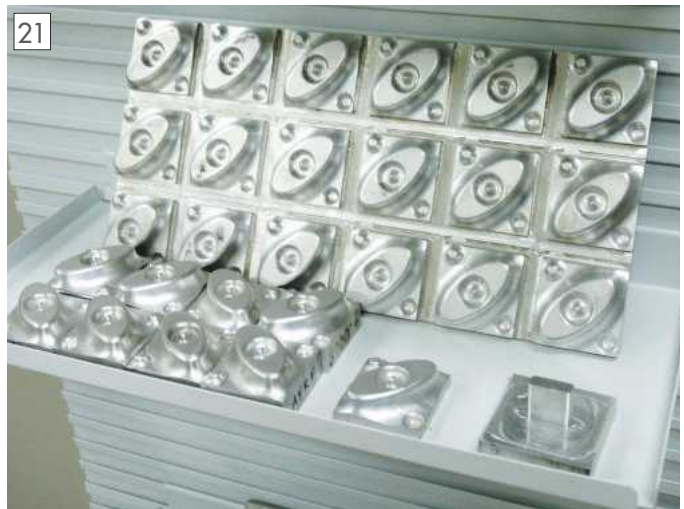
Some work produced on the PCNC Mills. They show the contouring capabilities of the mills well.
