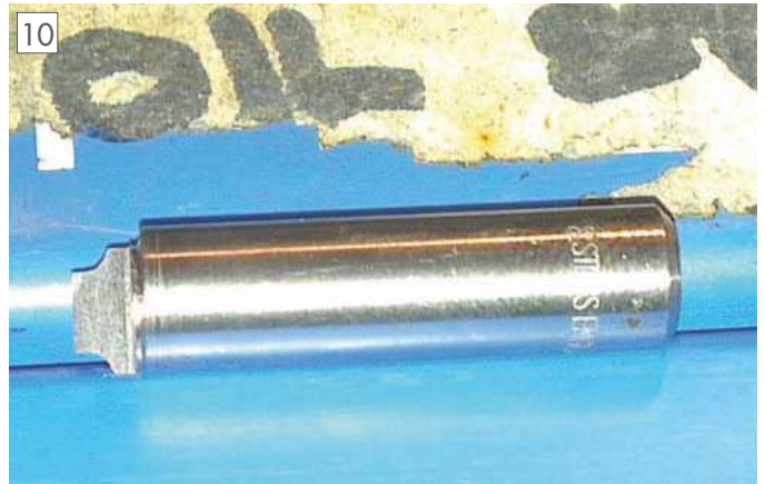
View of the radius cutter profile off set.
