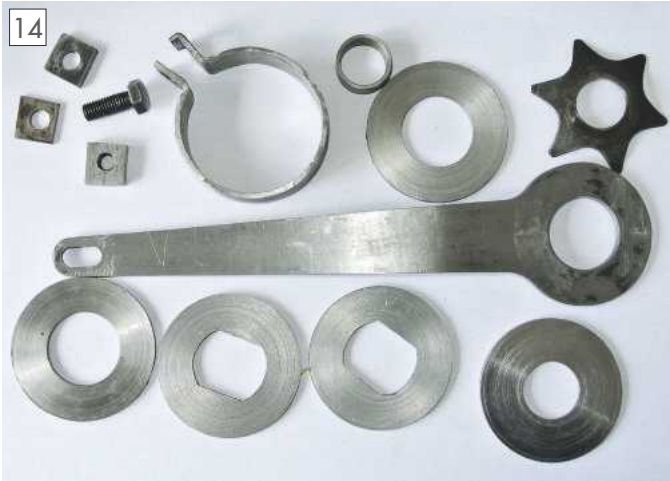
The long piece in the centre was successfully made on the CNC Mill. It is part of a steering damper for a 1929 Terrot motorcycle.
