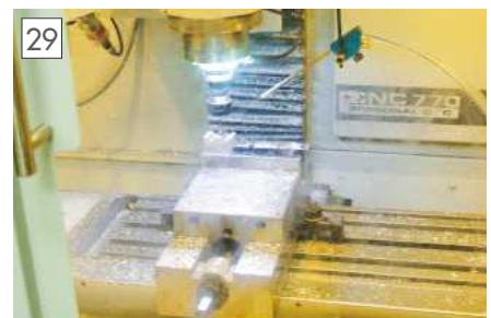
The block mounted in the soft jaw fixture having the large hole threaded using a thread mill.
