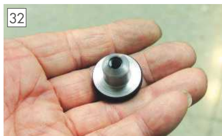
This knurled nut was modified using the mill.
