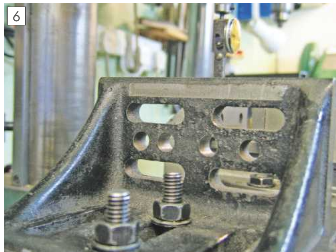
Machined flat at top rear of angle plate.
