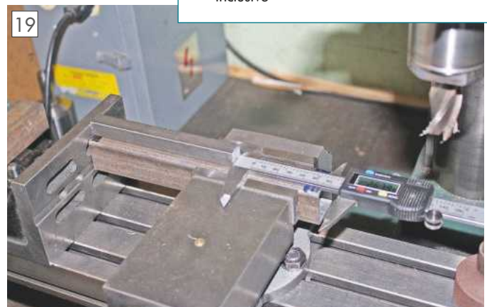
Using the digital vernier to check the length of the bar.
