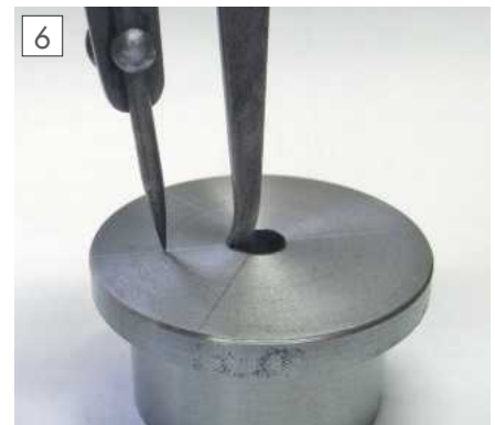
Setting out the screw hole PCDs using odd legs.
