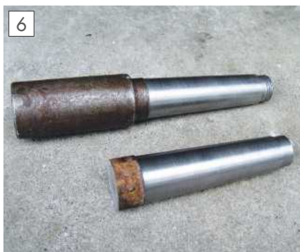
MT3 tapers, upper to make the MT1 drill, lower for the MT1/MT3 adapter.
