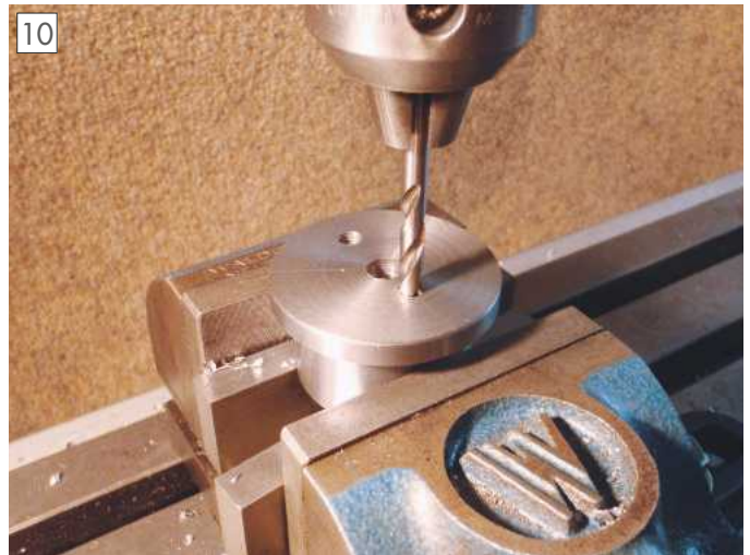
Drilling a clamping screw hole.
