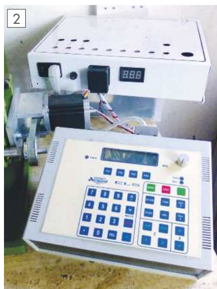
My system: controller, stepper, and power supply.
