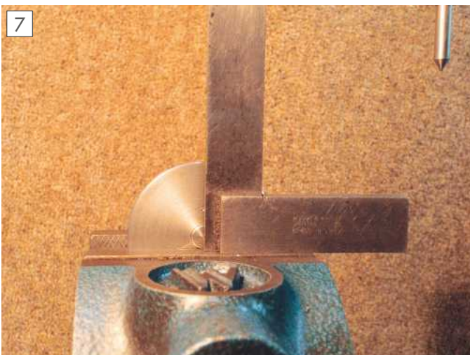
Setting up for drilling a pin hole.
