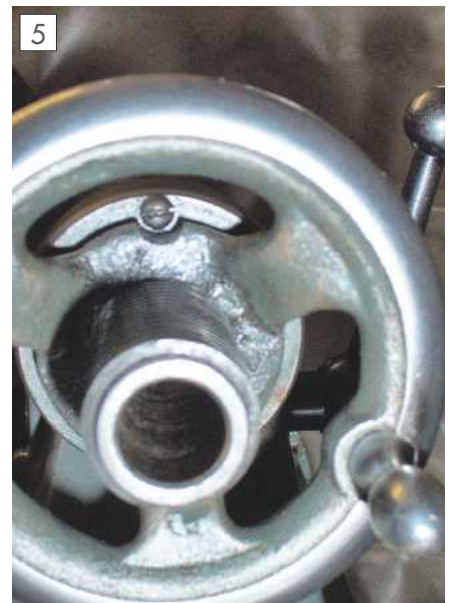
Tailstock handwheel rotated to give access to the 'c' locking plate screw.
