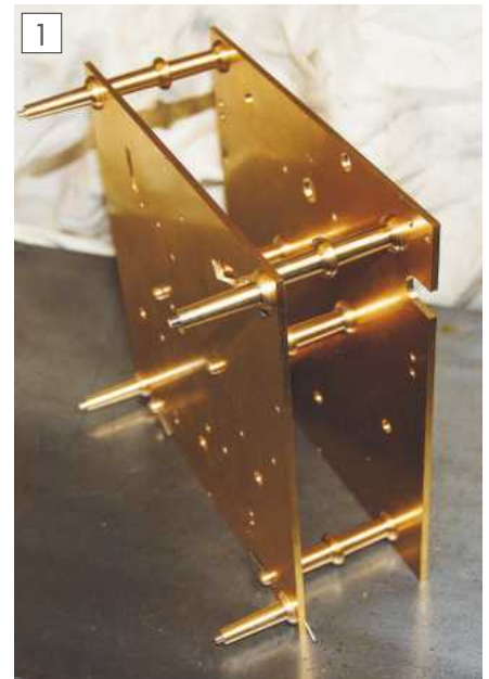
The finished clock pillars.
