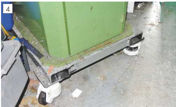
4 inch channel and 500kg castors provide support for my manual mill ...and the lathe.
