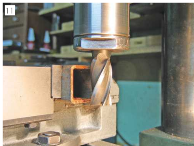
Cutter just touching the work.
