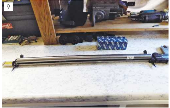
Setting trammel with length bars and slips.
