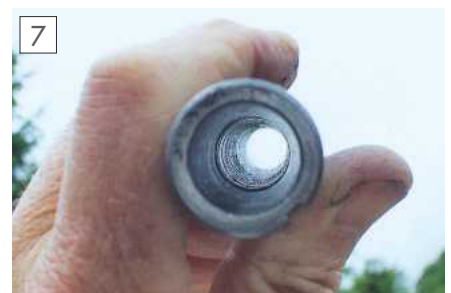
Visible signs of scoring in tailstock barrel.
