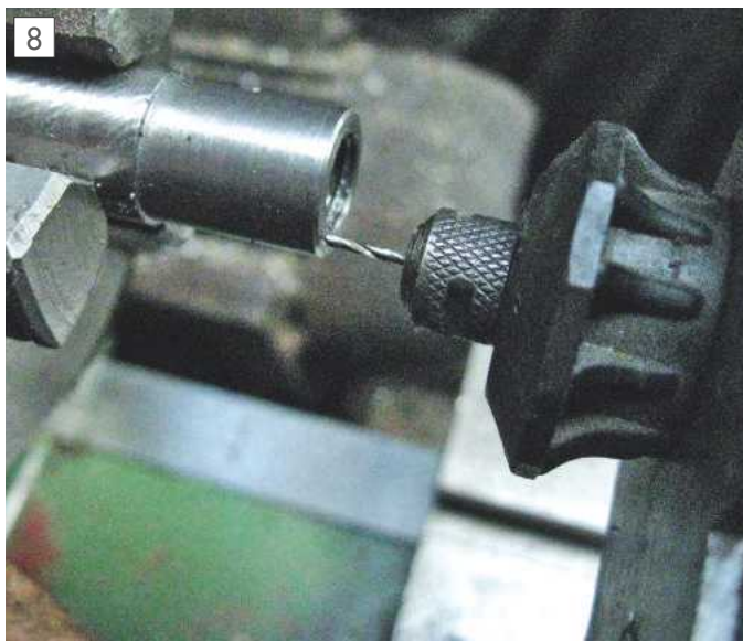
Drilling spanner holes in the back bearing nut.
