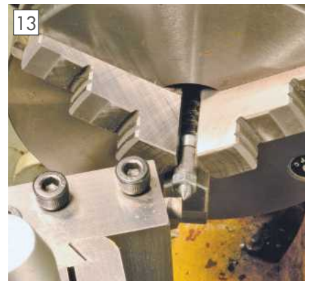
Setup for machining the 45 degree taper on a clamping pin.
