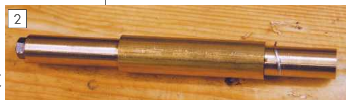
The holding device and brass bar ready for profile turning.
