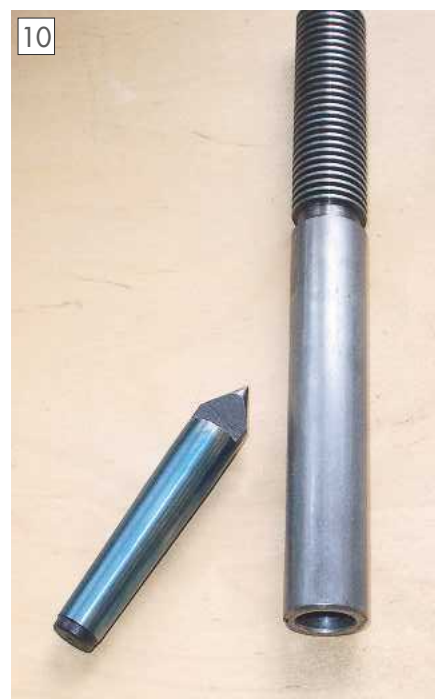
Even bluing on centre from reamed barrel.
