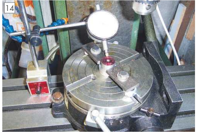
Centring the new drain branch on the rotary table.
