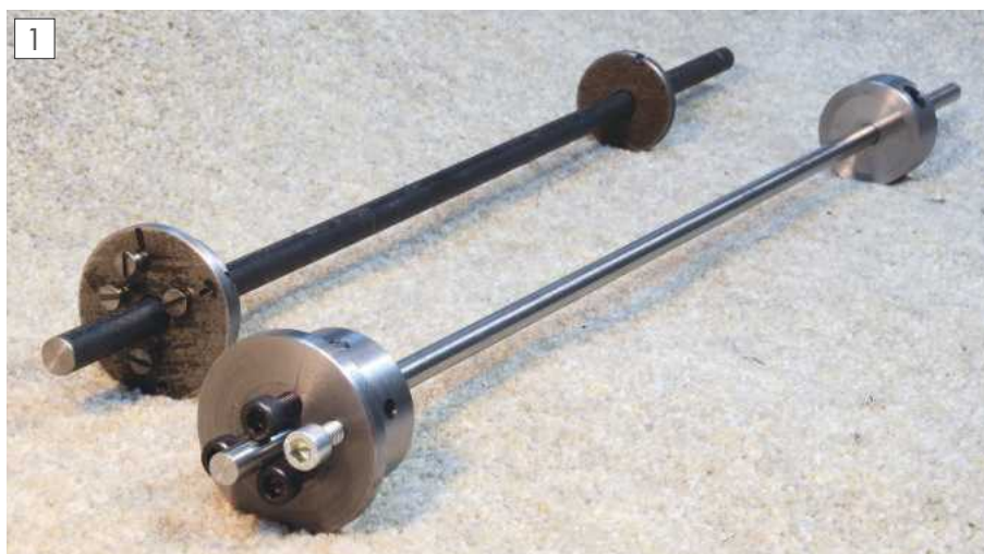
Original Depth Stop (left) and the New one (right).
