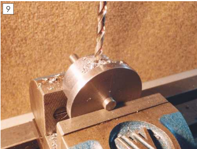
Drilling the pin holes.
