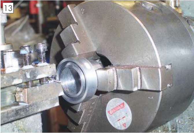
Machining the o-ring groove.
