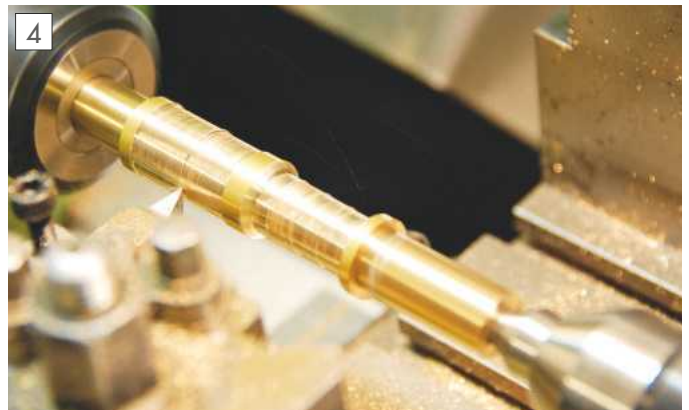
The brass bar being rough turned.
