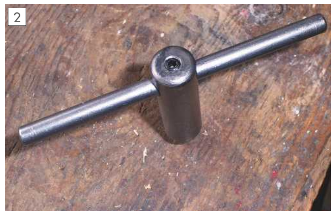
Chuck key with grub screw fitted.
