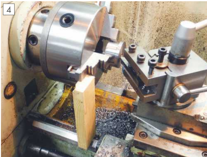
Method of dividing a circle into 3 using a block of wood.
