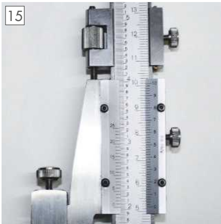
Scale of a vernier height gauge.
