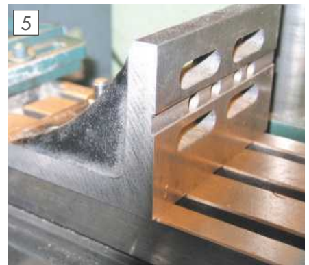
This groove accepts a tenon to help with accurate location.
