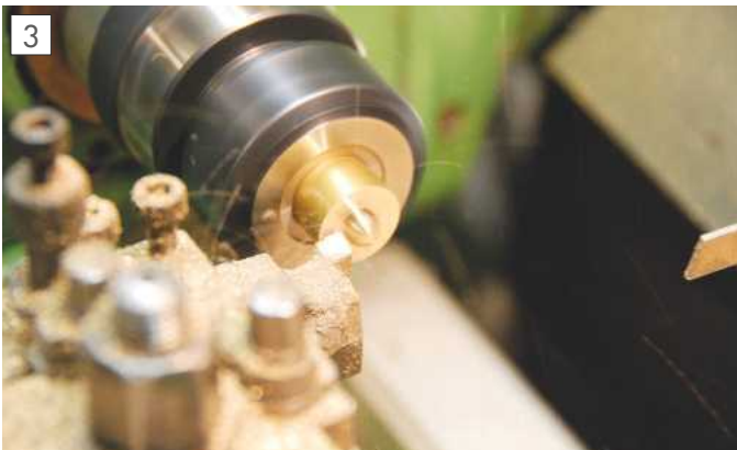
The front spigot and shoulder of the clock pillar being turned.
