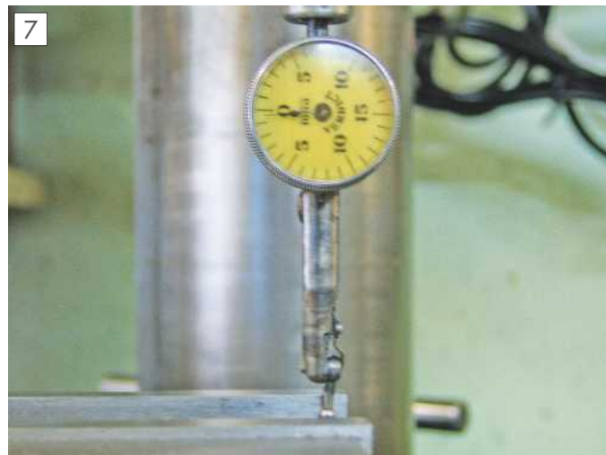
Checking alignment of chuck jaws at RHS...
