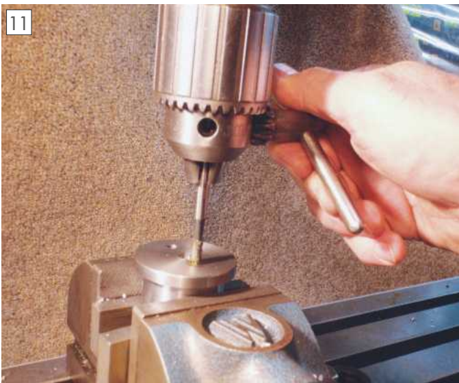
Starting a tap by hand using the drill press to keep it square.
