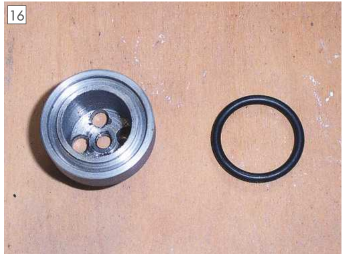
The new drain branch and o-ring.
