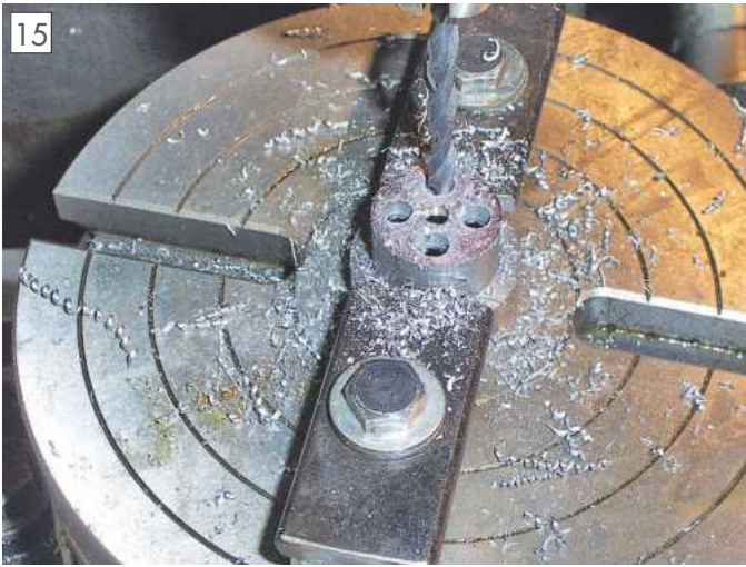
Drilling the drain holes in the branch on the milling machine.
