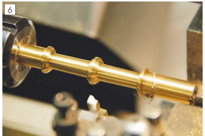
The finished clock pillar.
