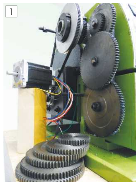
Gear change wheels and the stepper motor alternative.
