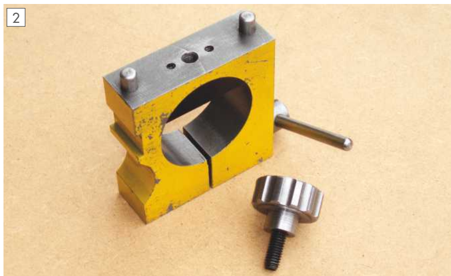
Modified accessory base and steady fastener.
