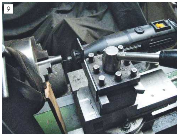
Indexing the back bearing nut using a piece of wood between the chuck jaws and lathe bed, the chuck key is slung with a weighted strap keeping pressure on the stick (the lathe motor was immobilised for this operation).
