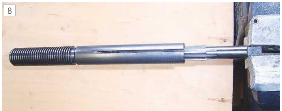
Set up for hand reaming barrel.
