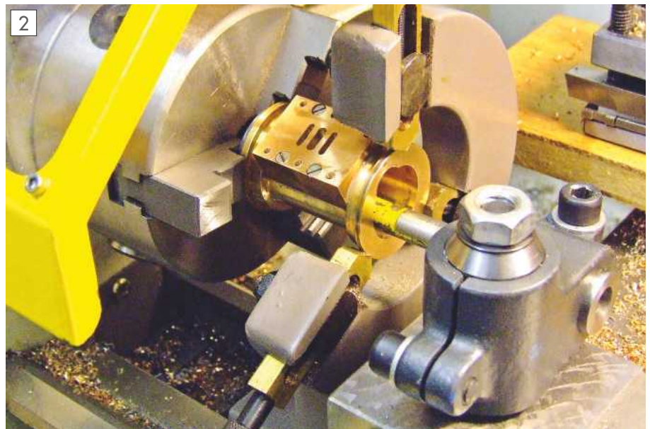
Boring a fabricated cylinder using an alternative holder design.
