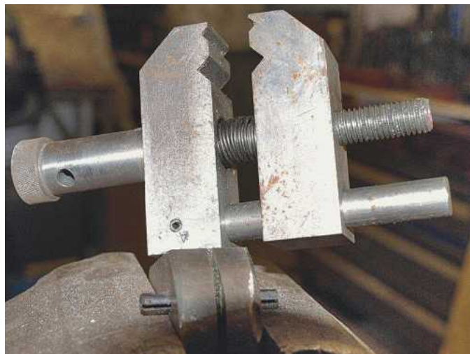
How the cross bar facilitates angle setting.
