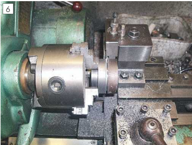
Parting off the finished part.
