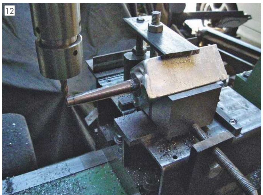
Milling cutting facets in MT1 drill.
