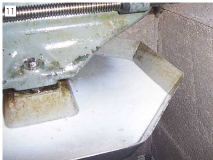
The problem: pool of suds at the non drain end of the tray.
