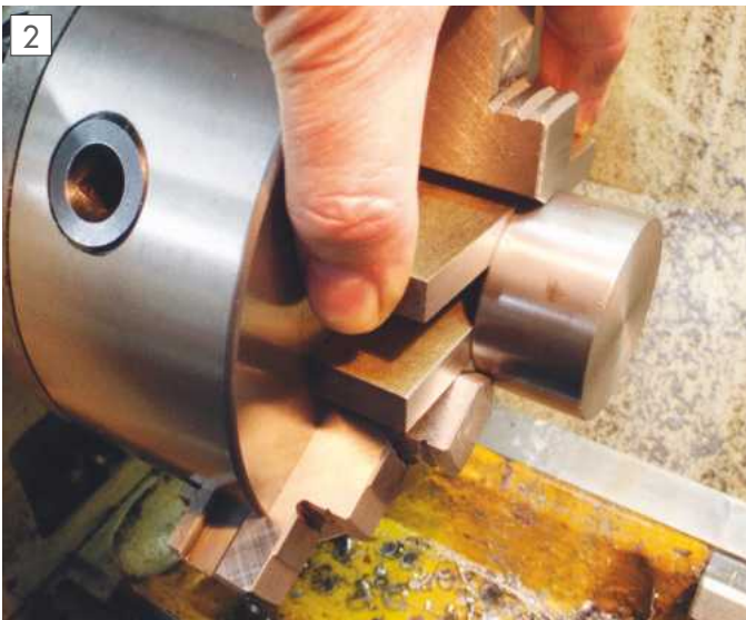
Using parallels to set the work for machining the spigot.
