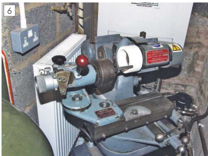
Grinding the relief on the taps.
