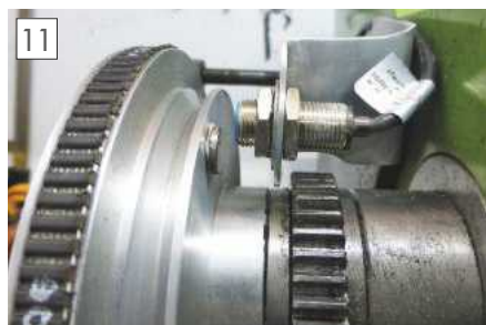
Hall effect spindle sensor bracket and magnet.
