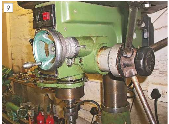
Modified index dial and hand wheel.
