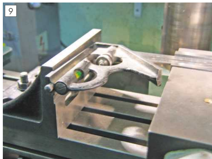
Setting angle plate with a square.
