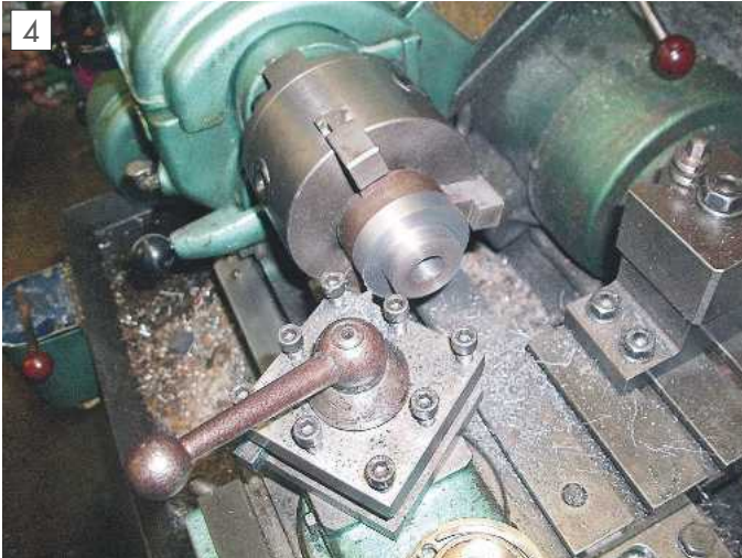
Machining the 35mm diameter portion.
