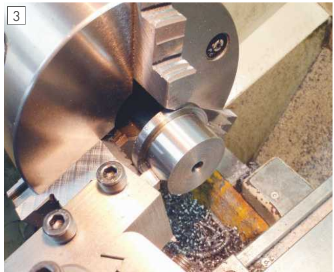
Machining the spigot, the central hole has been drilled.
