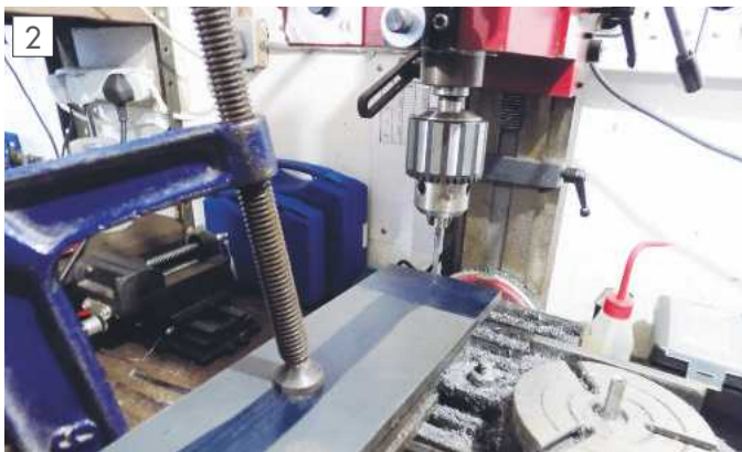
Using a scribe tip to locate a centre.
