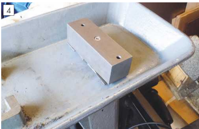
Datum block in position.
