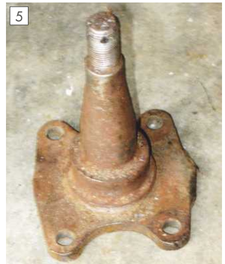
Stub axle used as material for inner body.
