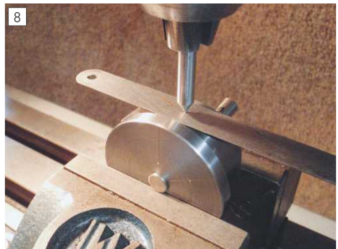
Centralizing the drill press on the diameter.
