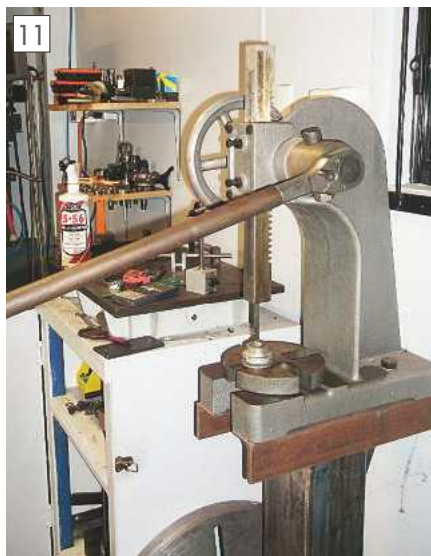
Broaching a keyway into a pulley.
