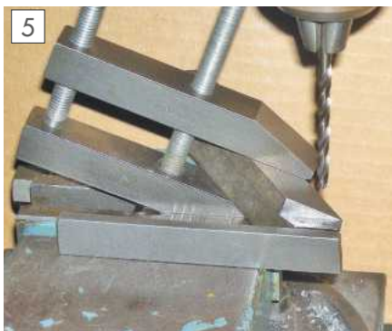
Drilling holes for the clamping screws.
