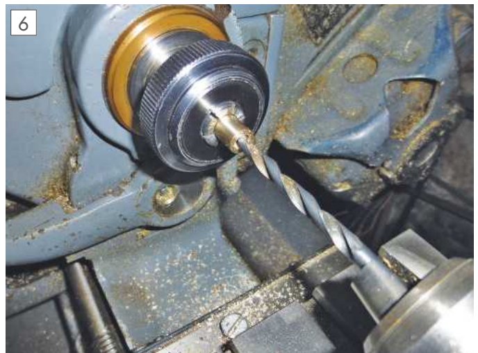
Drilling out the centre part.
