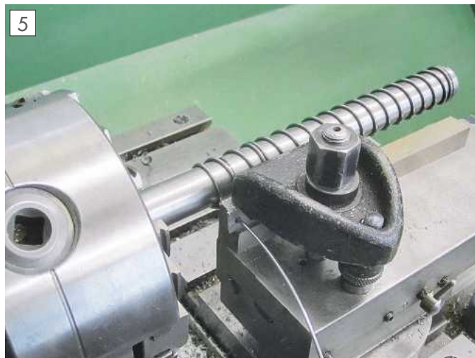
Spring winding on the lathe.
