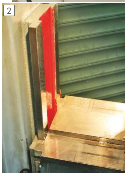
The Grimston (Beaver model A-style) Mill. INSET: The knee slide.
