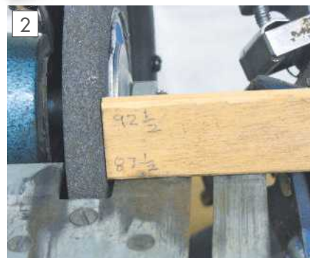
Setting the grinding angle.
