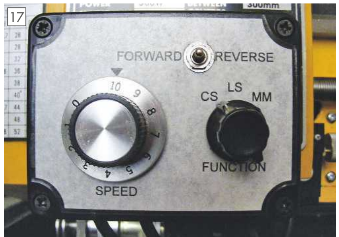
The control box for the cross slide, lead screw and lathe motor. Note: CS is cross slide, LS is lead screw and MM is the main lathe motor.
