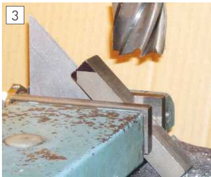
Start by putting the 45-degree angles on a steel blank.
