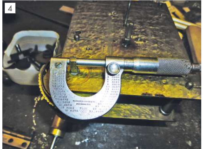
Measuring the square on the clock winder.
