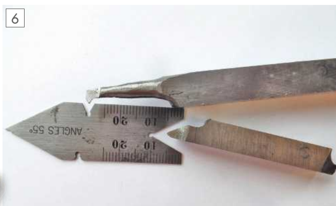
Hand shaped thread tool tips.
