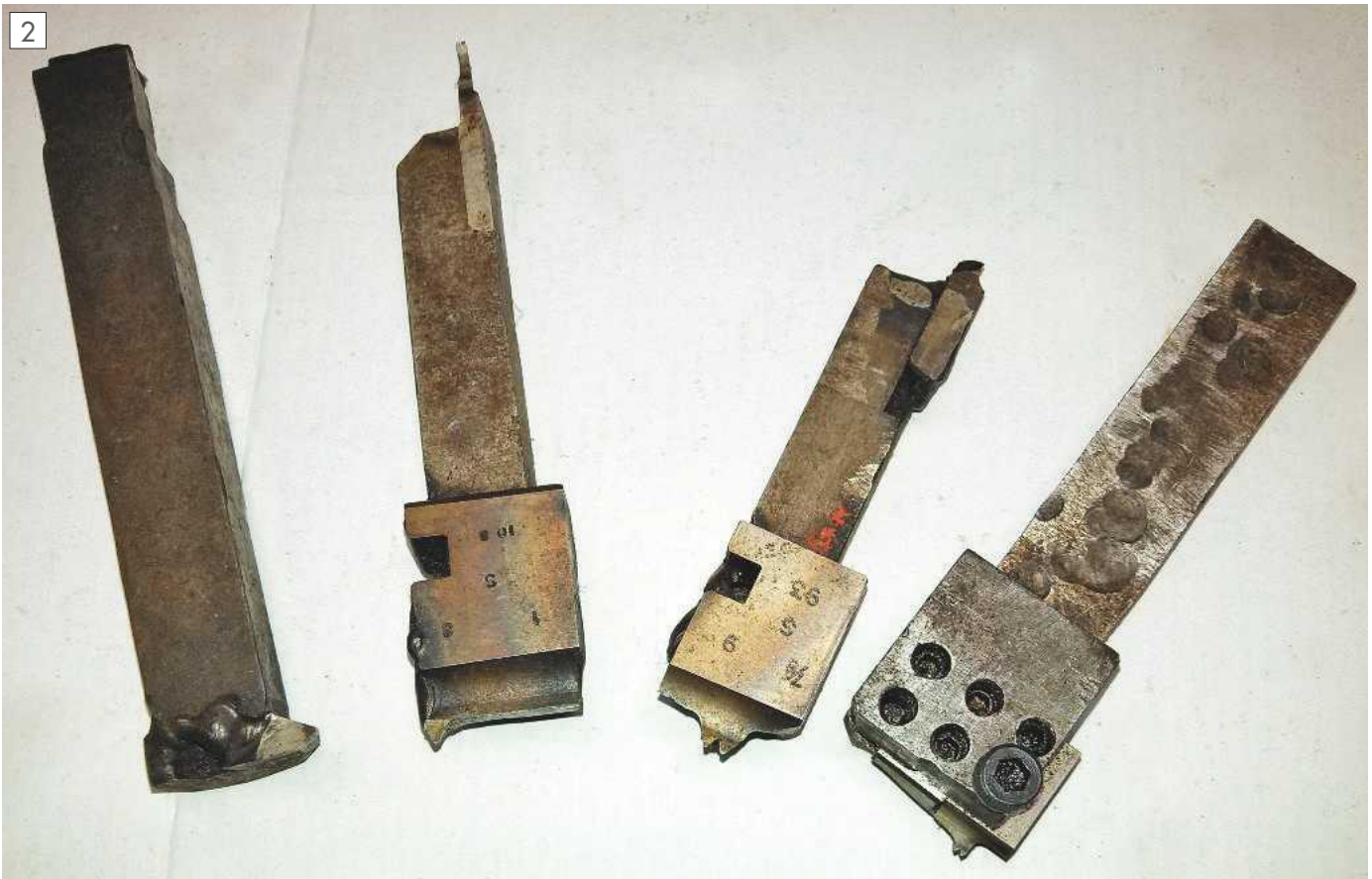
2 A selection of Coventry Dies, some welded to shanks and all ground to leave just the required teeth.
