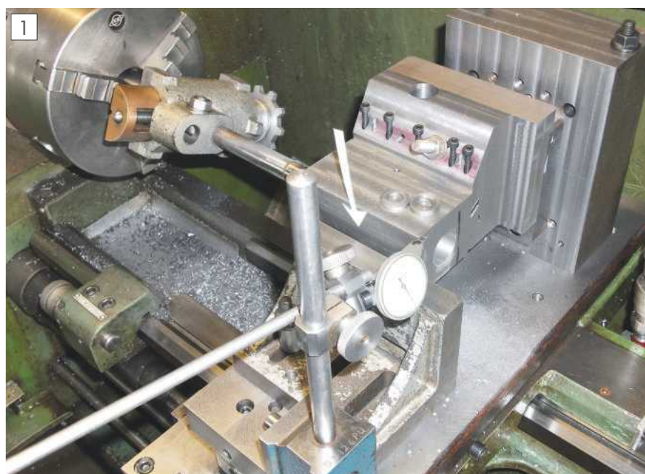
Cast iron tailstock set in position with the aid of a spherical washer.
