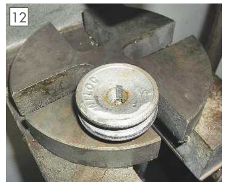
The finished keyway.
