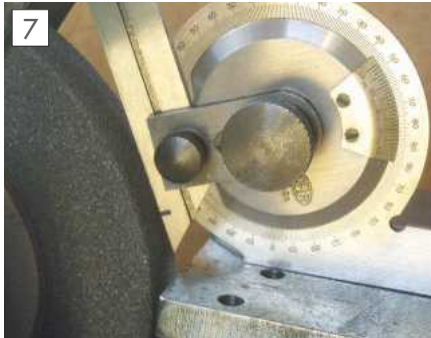
Setting the clearance angle, a card template could be used.
