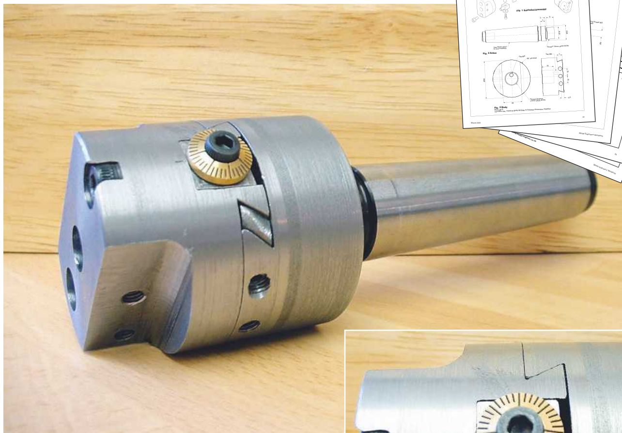
The completed boring head.
