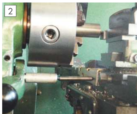
Radius rod in position the cut the external washer.
