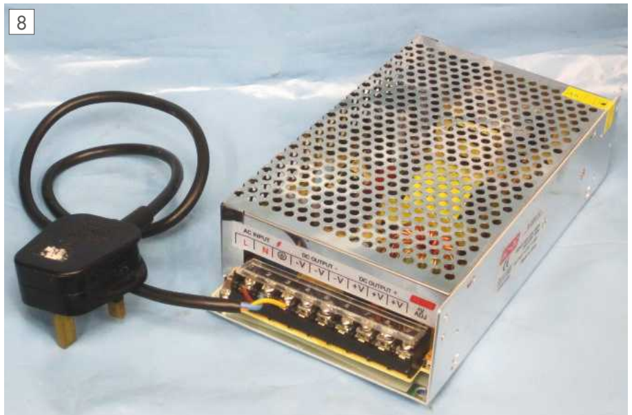
The 25 amp power supply, a suitable outer enclosure is needed for electrical safety.
