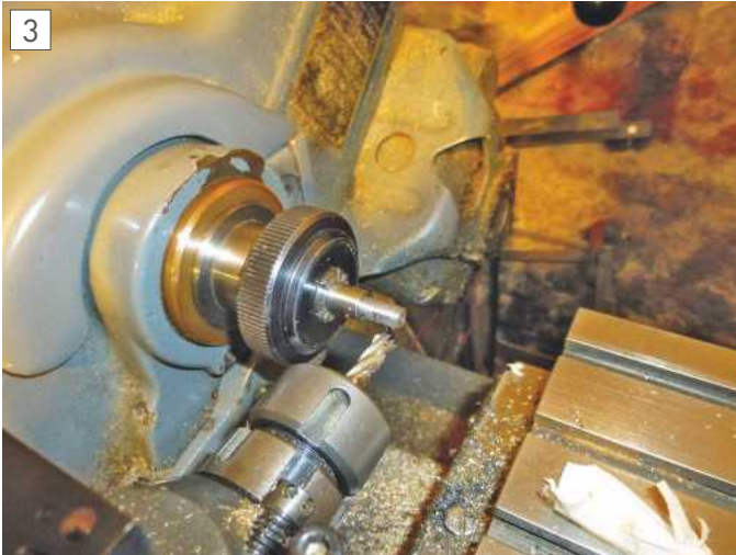
Machining a flat on the adaptor.
