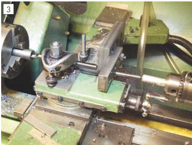
Setup to cut the internal washer.
