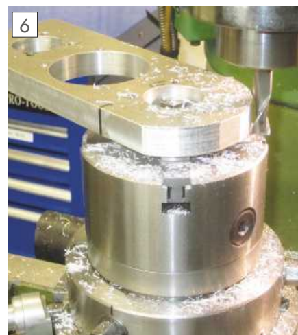
Profiling the motor support on the rotary table.
