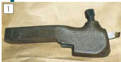
A robust, traditional inserted HSS tip holder.
