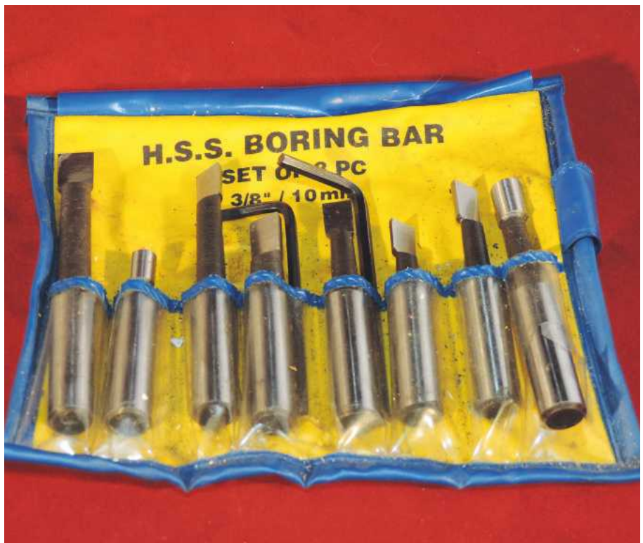
A set of boring tools, together with allen keys to fit the boring head.
