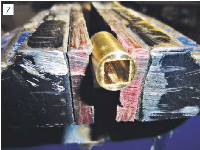
The finished square after filling, note the soft jaws.
