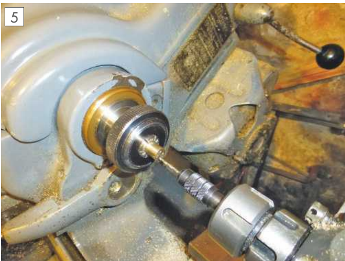
Drilling out the corners of the 'square' recess.
