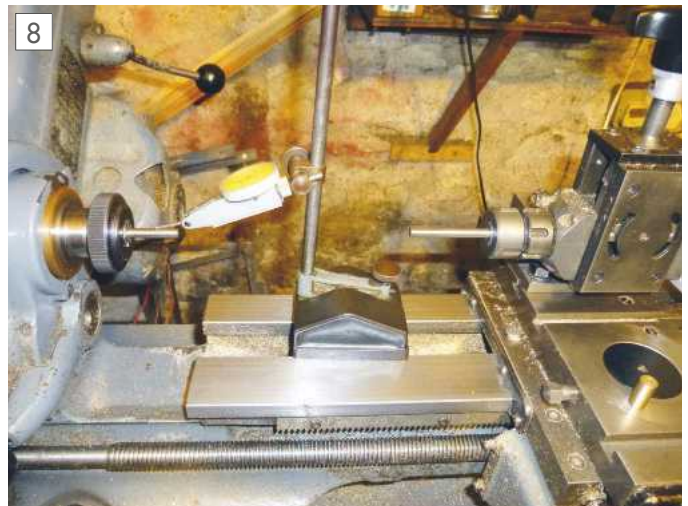
Using a DTI to compare the height of a bar and a milling cutter.
