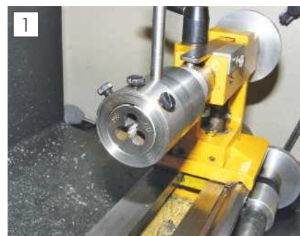
My first tool, a tailstock die holder.
