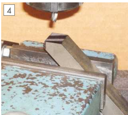
About to machine the tool tip groove.
