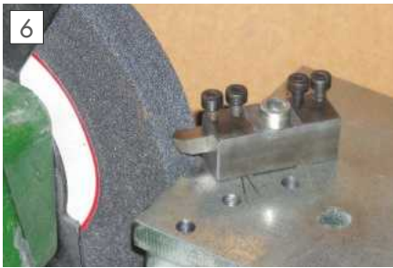
Grinding tips fitted to a holder risks fouling the wheel.
