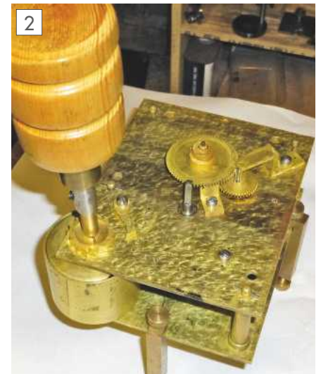
The tool in place after letting down a clock spring.
