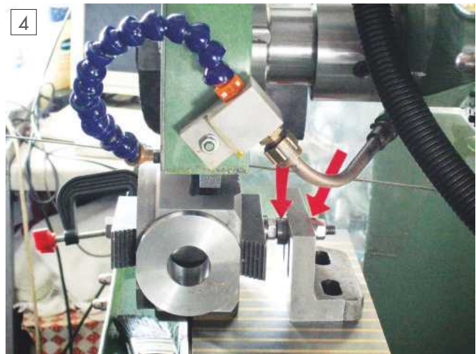
Providing some additional support on the magnetic chuck.
