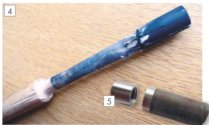
The unsuccessful wooden lap. INSET: End cap material.
