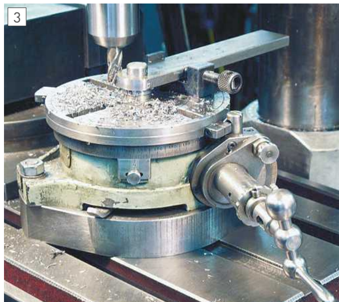
Starting rounding a bar end at the first stop.
