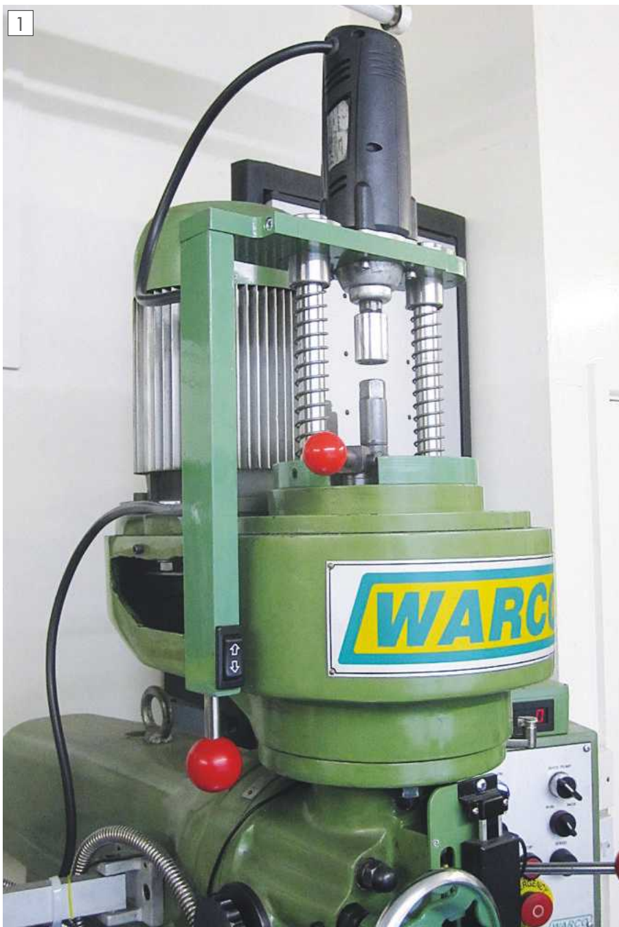
The completed power drawbar.
