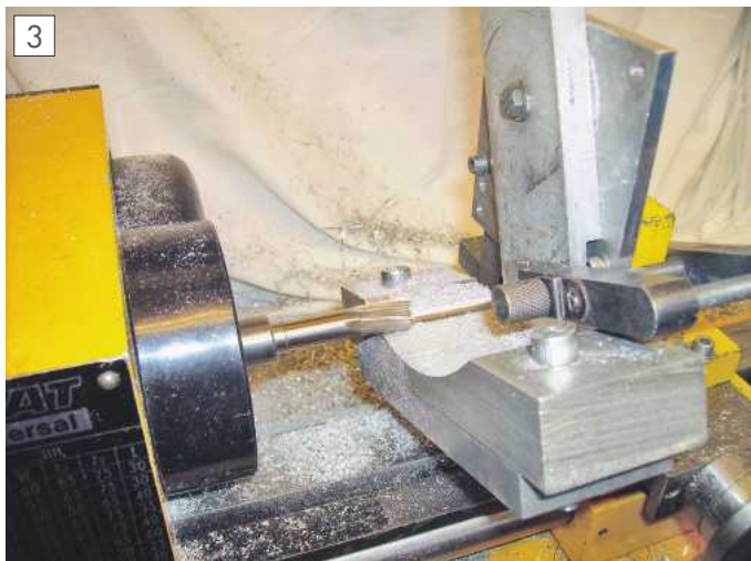
Machining the additional motor foot.
