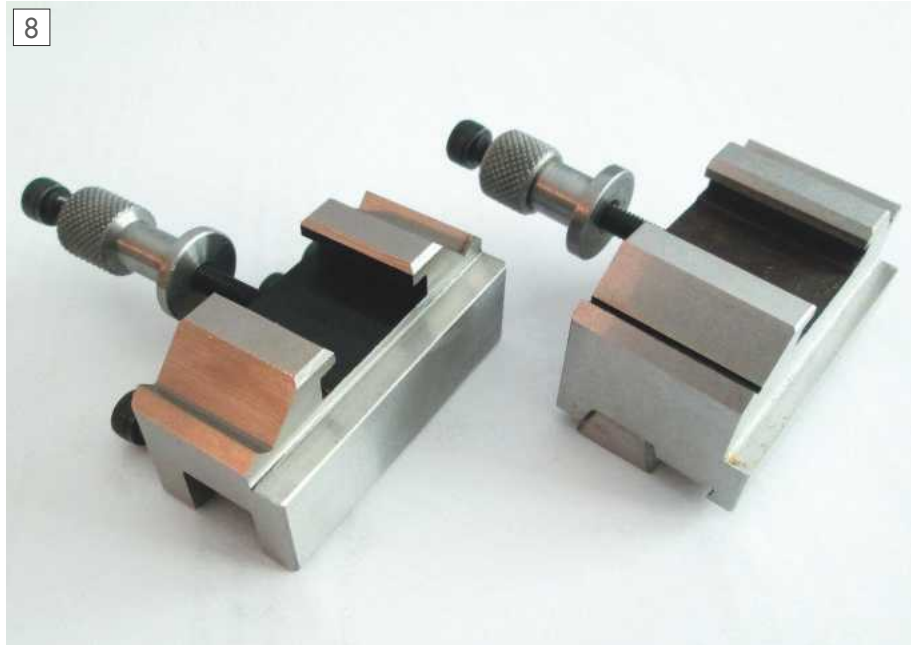
Modified toolholder showing stepped bottom face and standard parting toolholder.
