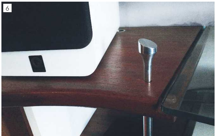
A shelf support finished on the Frankenstein Mill.
