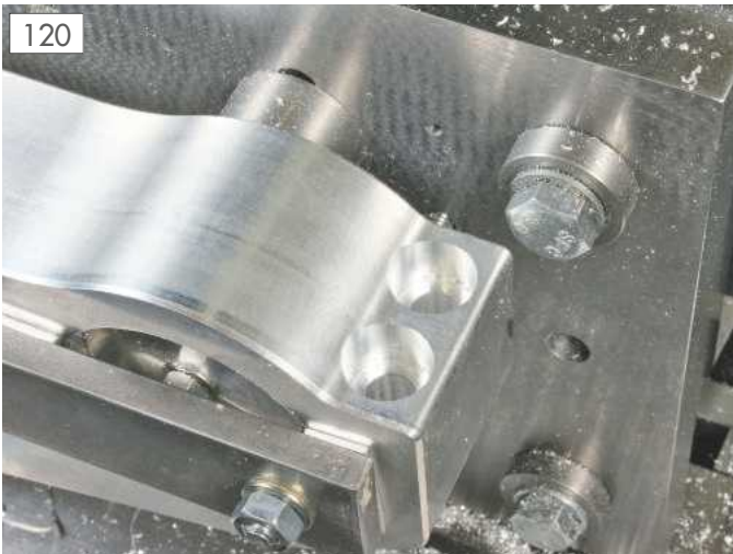
There is an attractive intersection between the edge of the pinch bolt holes and the curved face of the yoke.
