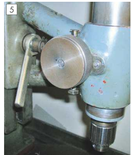
Attachment site for fine-feed bracket.
