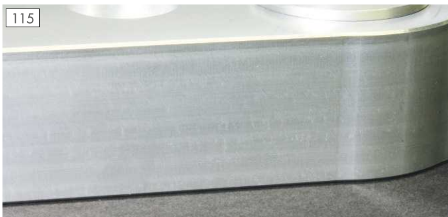
Using 5mm deep finishing cuts produced a good finish.
