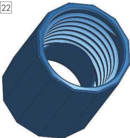
CAD view of the threaded inside of the connector.
