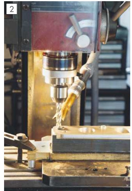
Profiling nearing completion.
