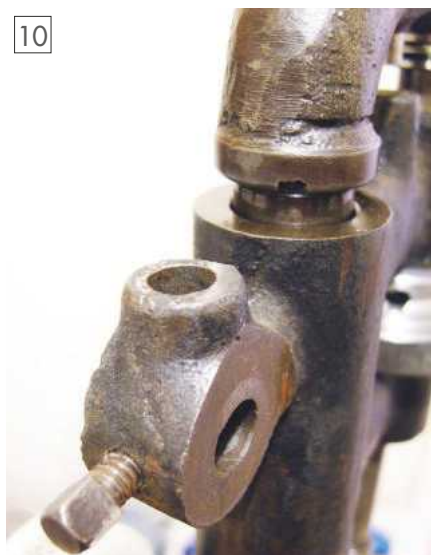
Holes for clevis and freely rotating pulley bracket.
