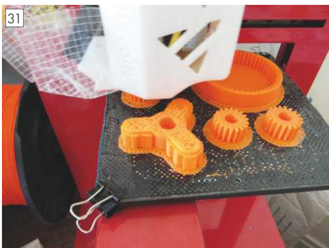
31 Gears are now complete and the spider arms are part way through with the internal structure again visible.
