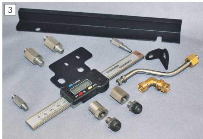
Parts for attaching scale to cross slide.
