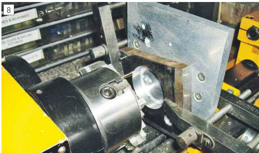
Method of boring brackets for clamping.
