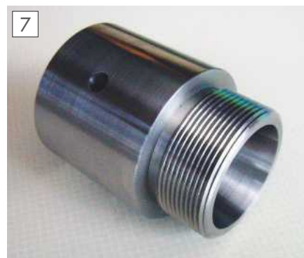
Finished collet chuck, minus closing ring.
