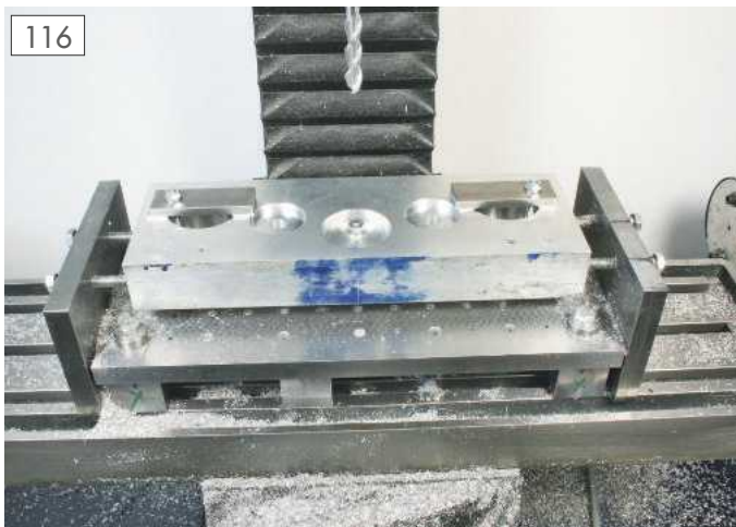
The best place for clamps is through the large holes for the fork legs. The third clamp uses an inverted top hat with a hole which is offset so that the bolt is aligned with one of the existing holes in the sub-table.
