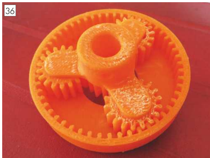
Less arty and more detail in this shot where the effects of removing the support structure from under the spider arms can be seen.
