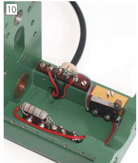
The microswitch can be seen at right.
