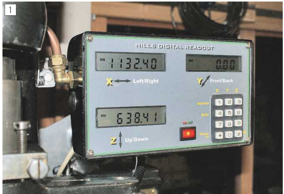
First attempt at a DRO using individual read outs combined into one case.
