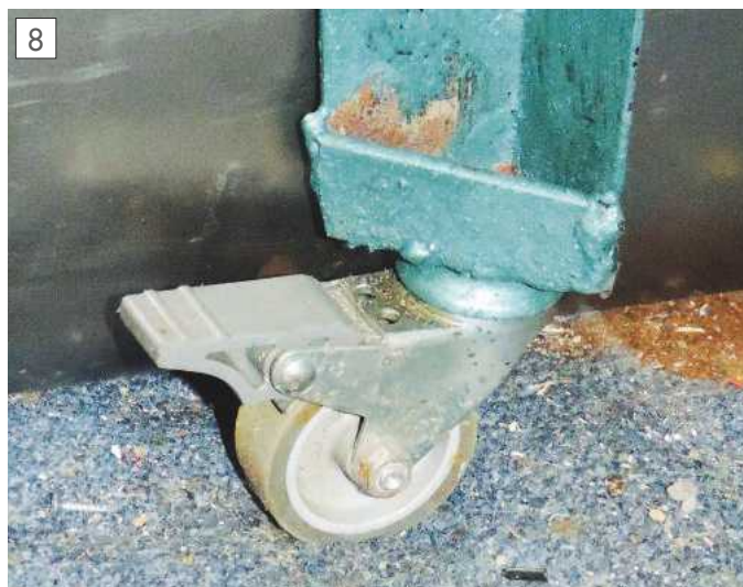
Reinforced wheel mount.
