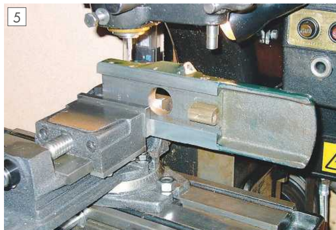
Drilling pillar holes in cross slide.
