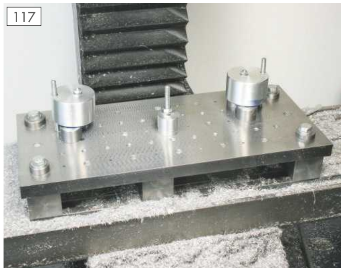
Plugs can be fixed to the sub-table to retain alignment of the yoke when it is flipped over.
