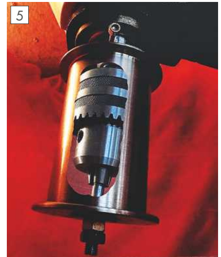
Cutaway showing how the drive pulley fits over a drill chuck.
