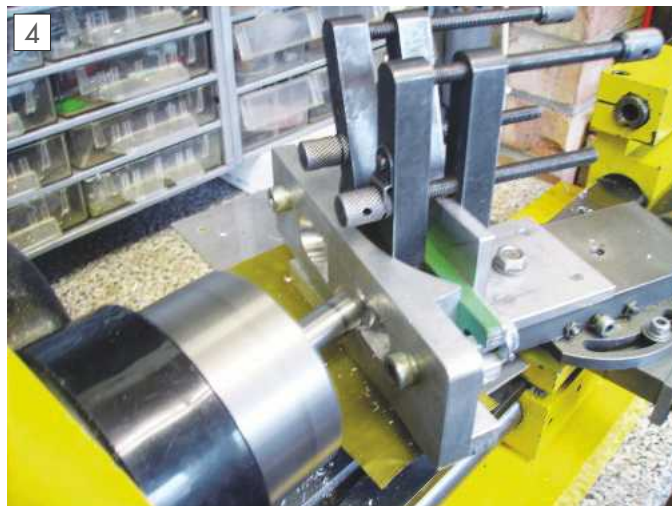
Setup for milling pockets and drilling mounting holes in the second foot.
