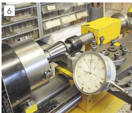
Setting top slide for boring the collet taper.
