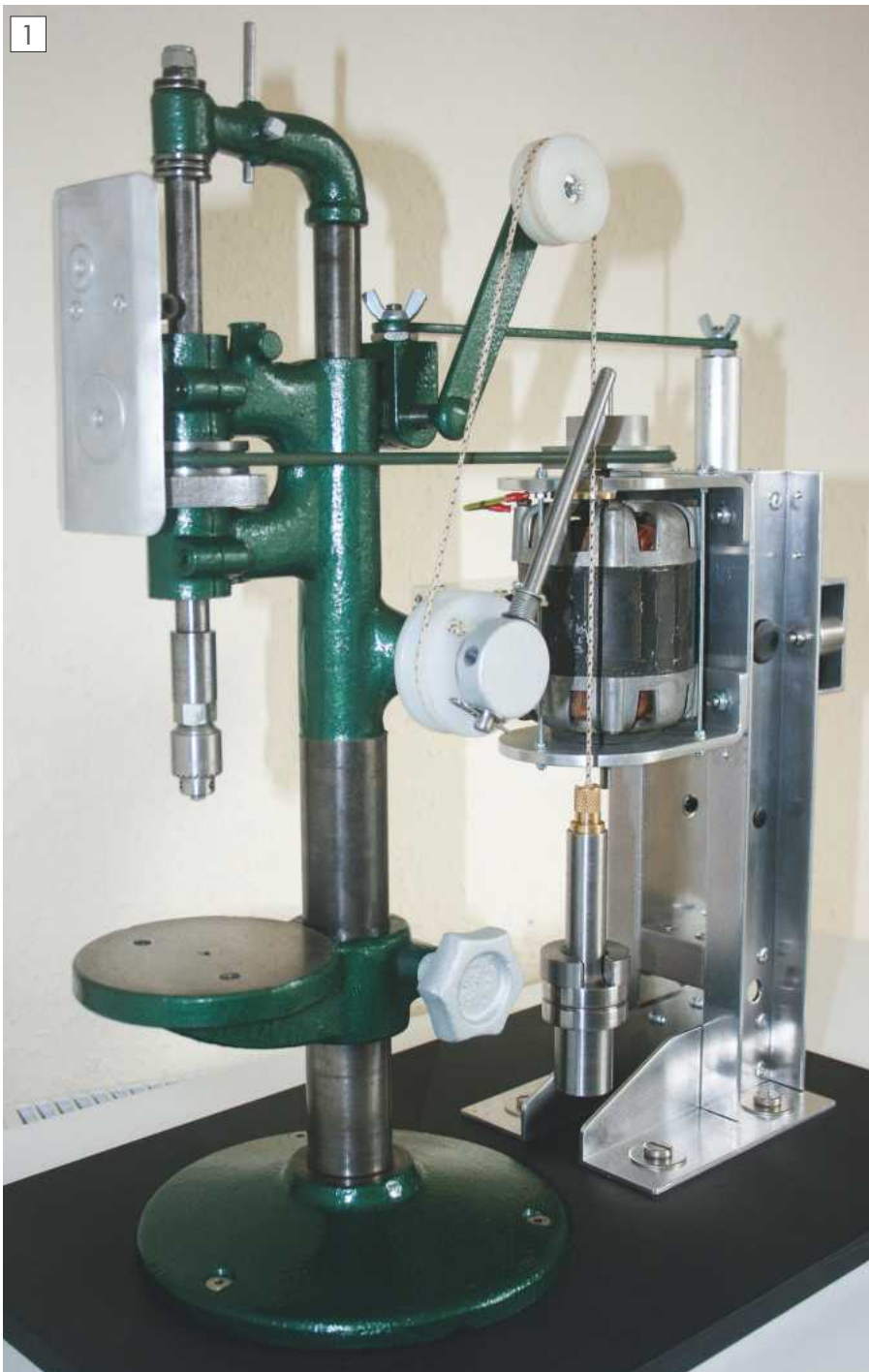
The finished machine, note the simple belt guard.
