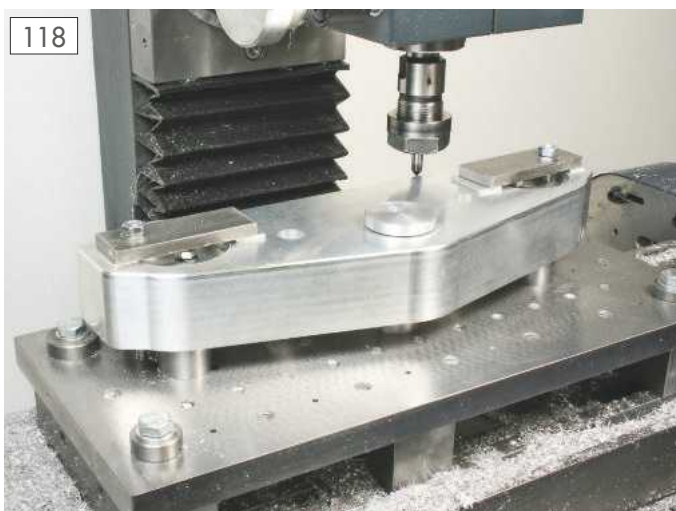
The alignment plugs remain fixed, but allow additional clamps to be used to secure the yoke.
