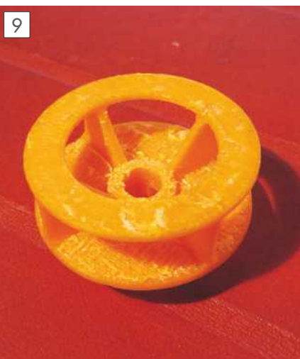
Top view of the replacement showing top disk (this was the test piece so not completely cleaned of support material).
