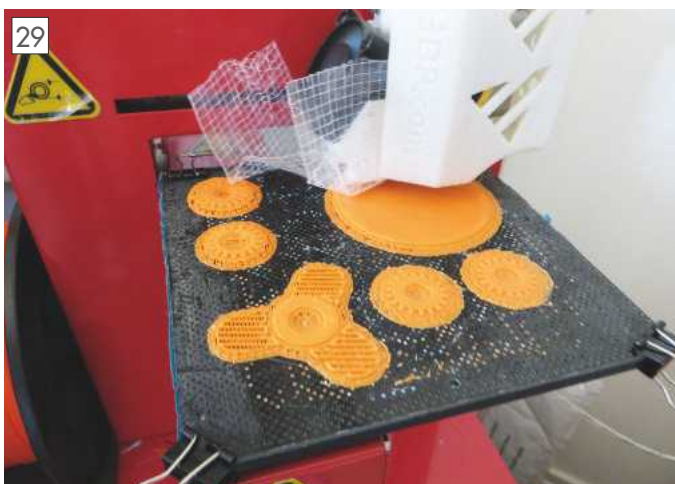
29 Bed (to ensure a good adhesion to the base plate) and initial layers are printed.
