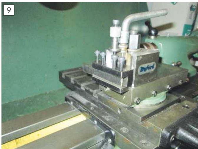
Modified toolholder on top slide showing restriction of positioning.
