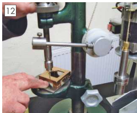
Operating lever weight when tapping.
