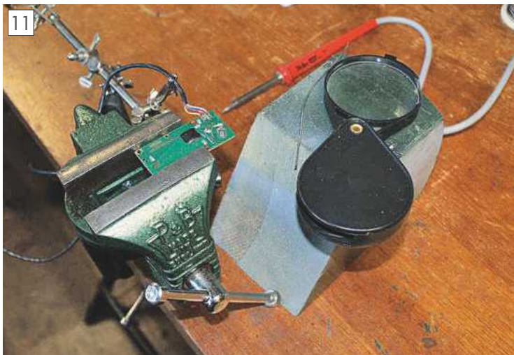
Soldering leads to reading head pcb.
