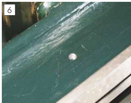
Hole drilled in rear of bed for saddle scale support.
