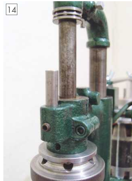
Simple guard location pin.
