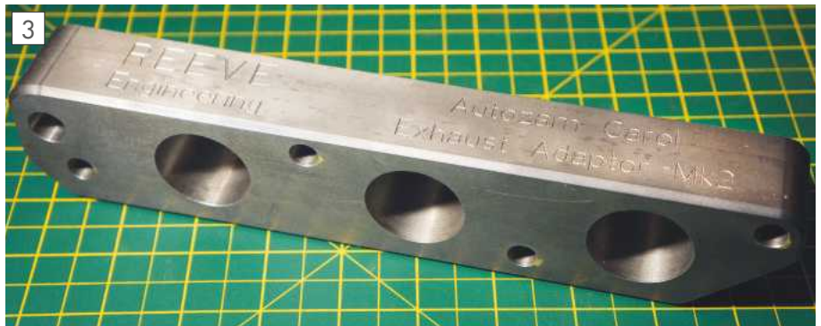
The completed adaptor.
