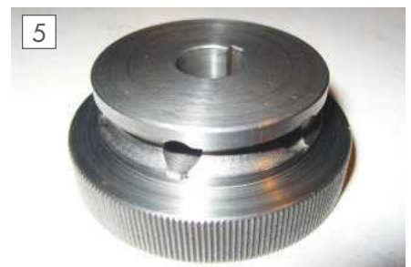
New driven pulley.
