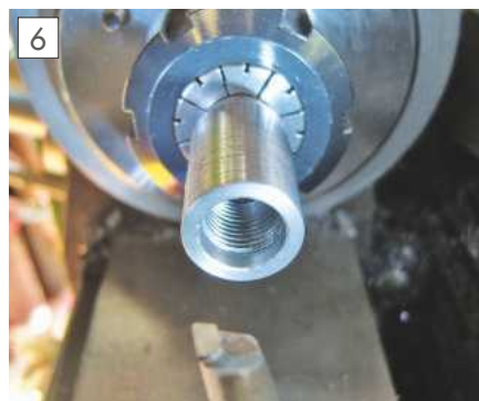
Threaded bottom end of drilling spindle.
