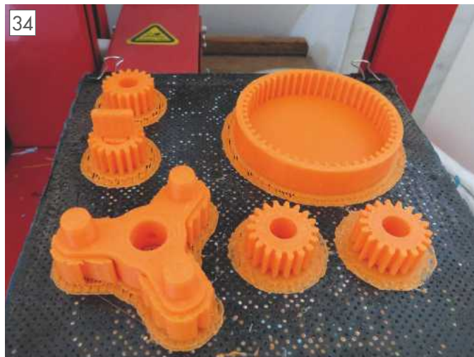
End result having just finished – caution required because the bed is still heated to 105°C. The eagle eyed will notice that the planet wheel is lacking the large centre hole – which had to be swiftly machined out!
