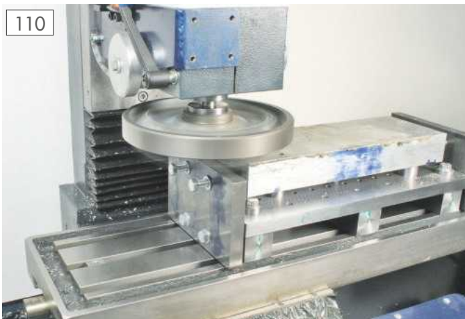
End plates were added to the sub-table, to allow the material to be gripped from the side.
