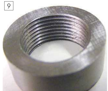
A 1mm pitch thread in steel.
