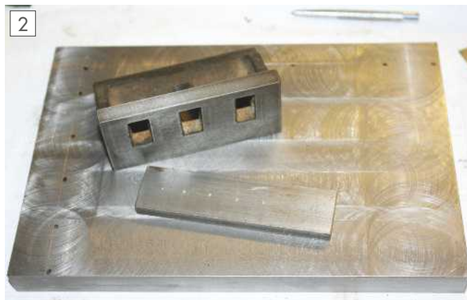
Angle plate and marked up clamp bar.
