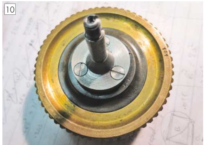
Finished mounting arbour fitted to the chuck.
