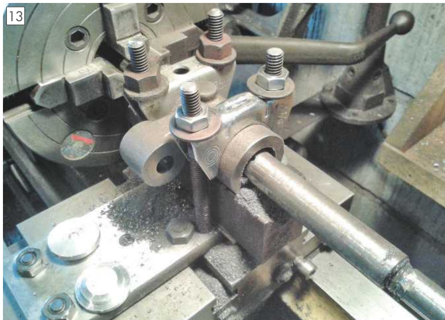
Boring a Potts casting – a new use for exhaust brackets!
