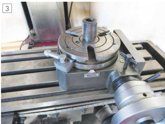
Arbour fitted to rotary table.
