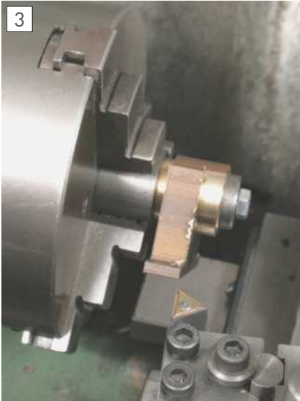
The Parallel Stub Mandrel being used conventionally, that is with a securing screw on the end.
