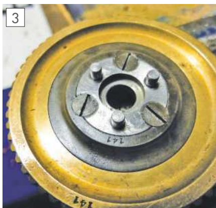
Silver steel plugs in the mounting holes.
