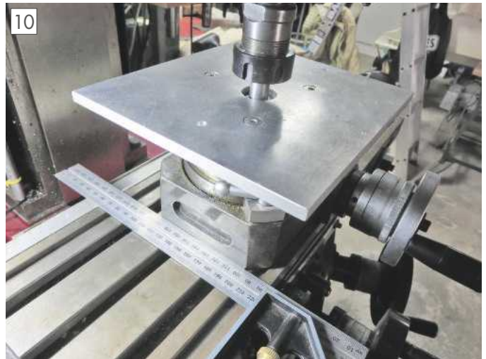
Setting up for use, note the first few fixing holes in the table.
