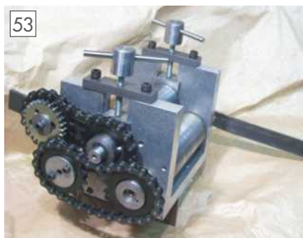
Tee bars in position.
