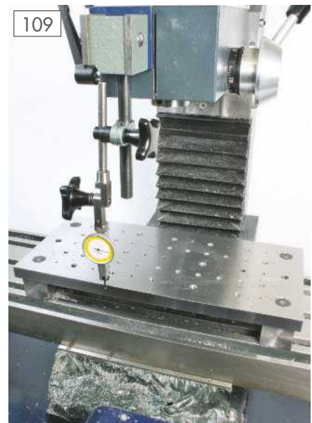
Using a lever-style DTI for final adjustments.
