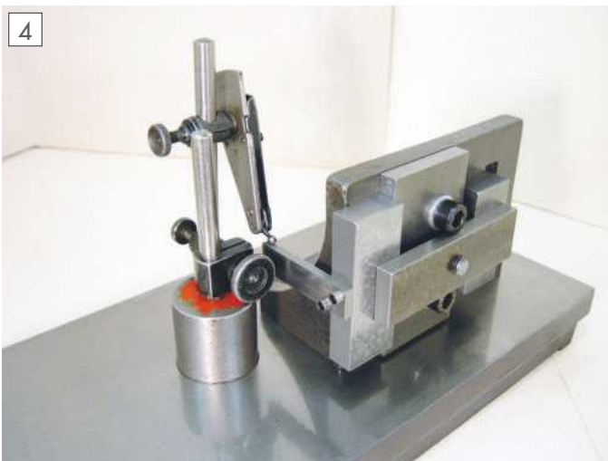
Clocking the upper edge of the blade.
