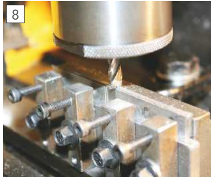
Truing one edge of a parallel.
