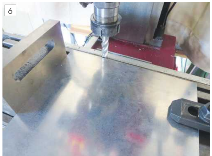
Machining edge of the table.
