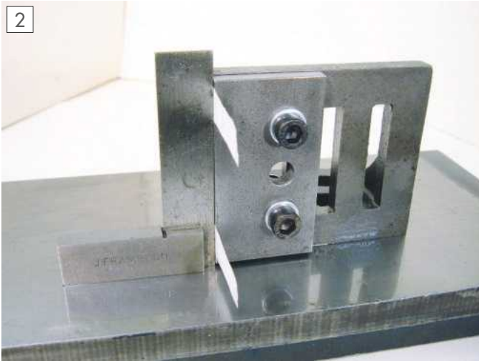
Setting a fence square to the surface plate.
