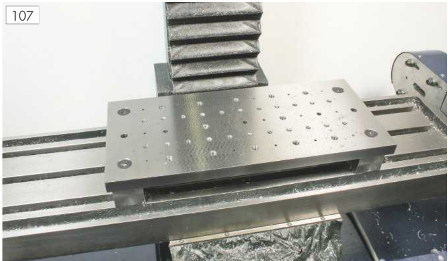
A sub-table with a selection of tapped and reamed holes.
