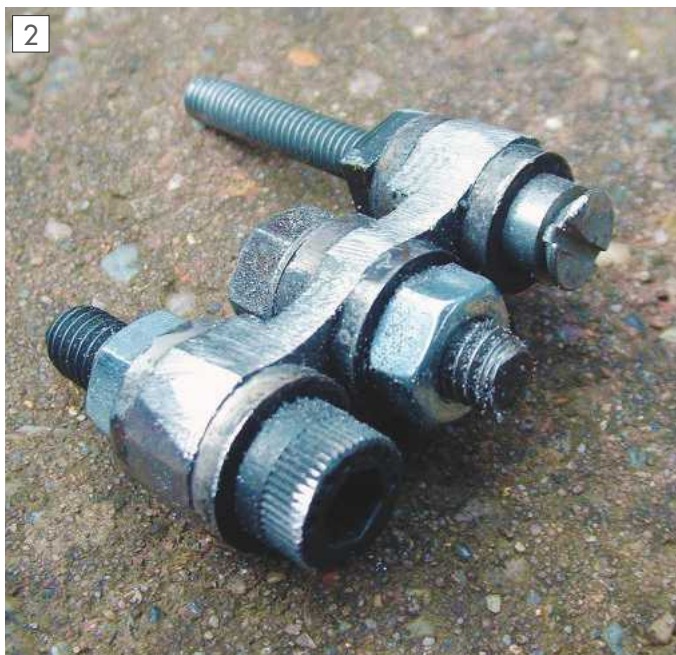
Three pairs of filing buttons screwed to an embryo crank.
