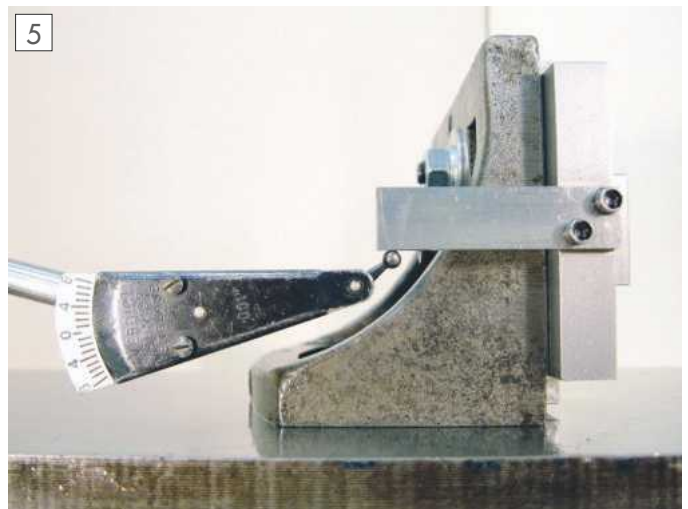
Double checking the setting by clocking the lower edge of the blade.
