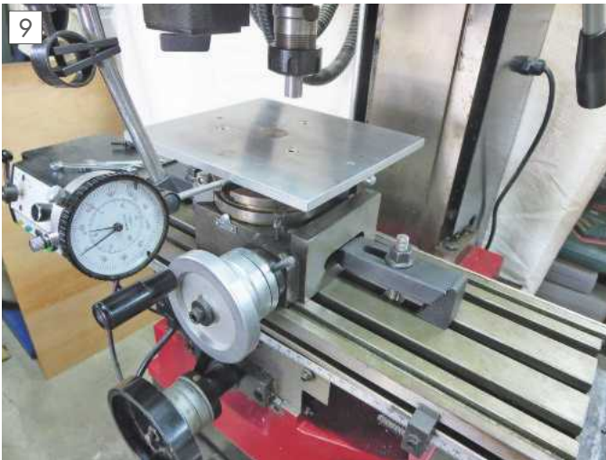
Testing X/Y alignment.
