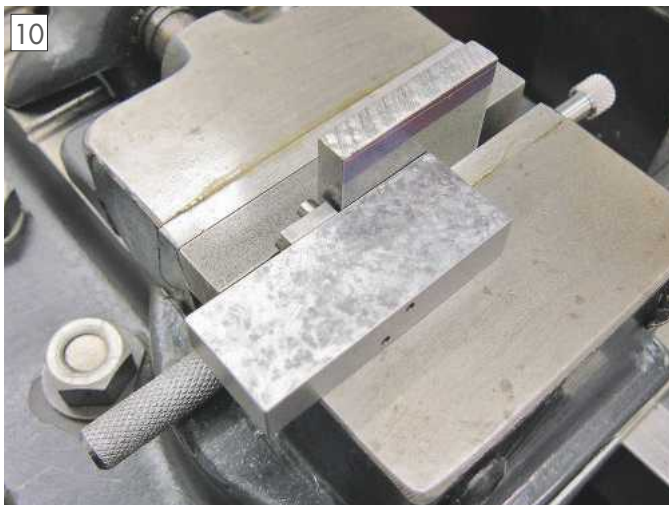
Using the square. A piece of plate to be squared up.
