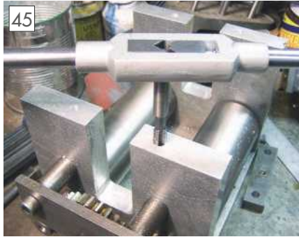
Hold down screws being tapped.
