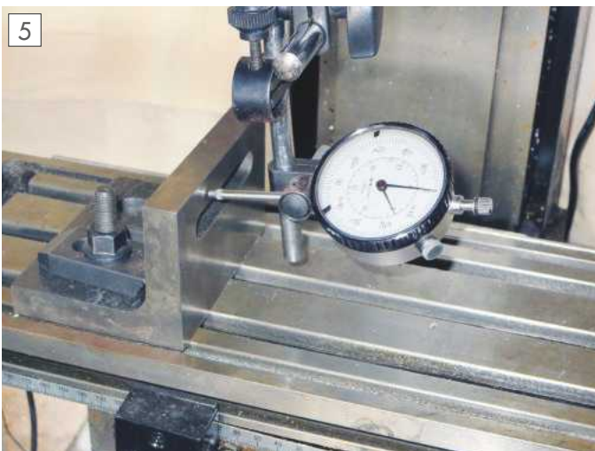
Aligning angle plate with mill Y axis.
