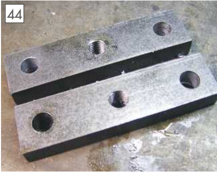
The pressure plates drilled and tapped.
