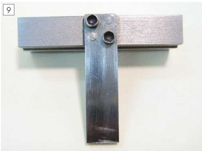
Pins pressed home and flushed off. The completed tee-square.
