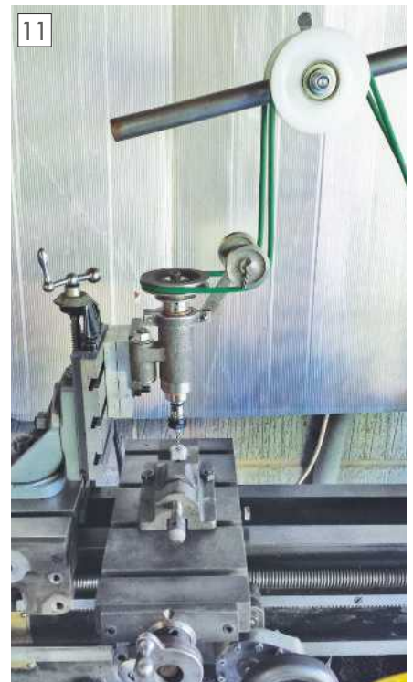
Milling with the Potts on the Drummond lathe.
