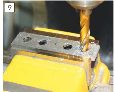
Drilling holes in a parallel.
