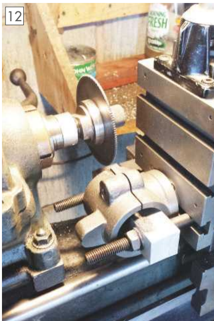
Slitting the Potts trunk casting.
