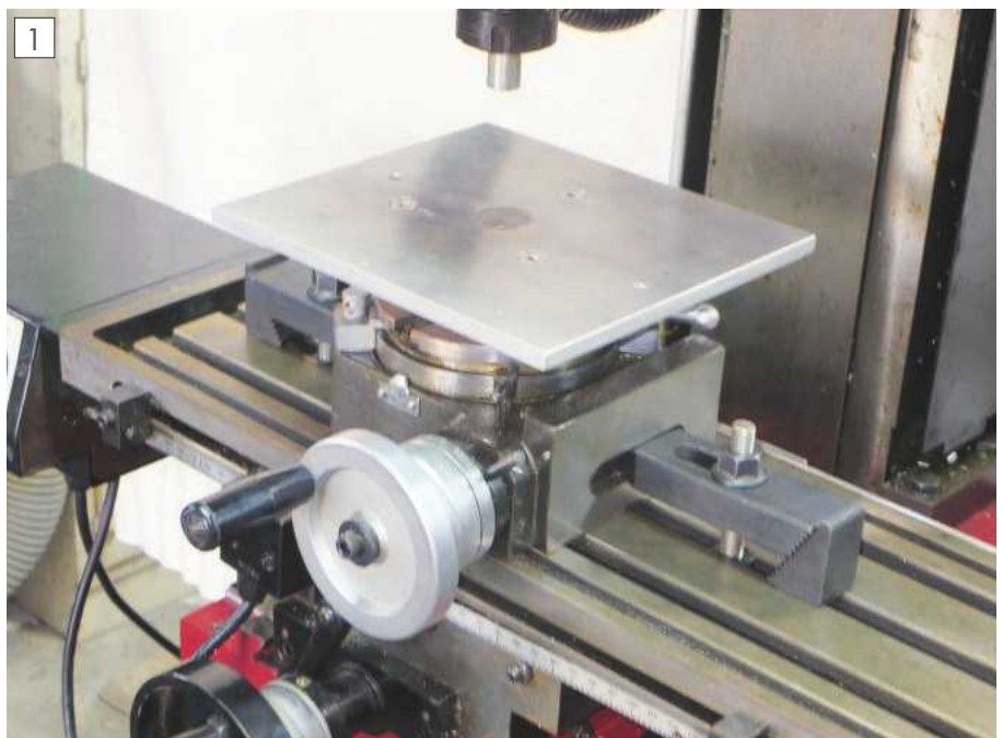
The new table mounted above the rotary table.
