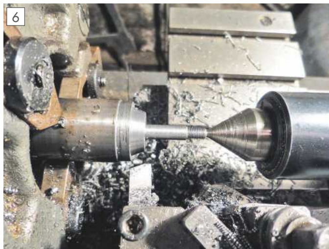
Using a form tool to form the chamfer.
