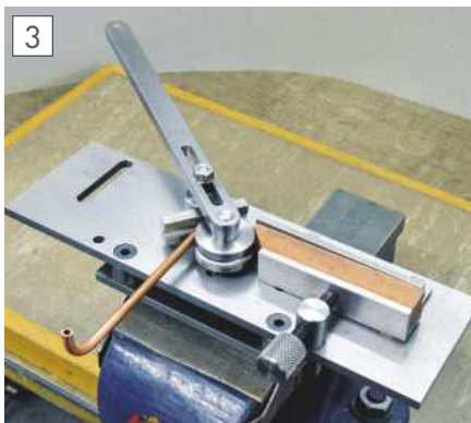
Mike Chrisp's bench mounted pipe bender.
