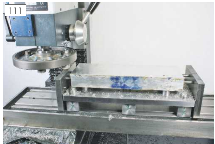
The workpiece was faced using a flycutter bolted to a lathe faceplate.
