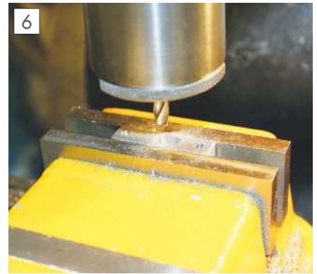
Slotting one end of a clamp.
