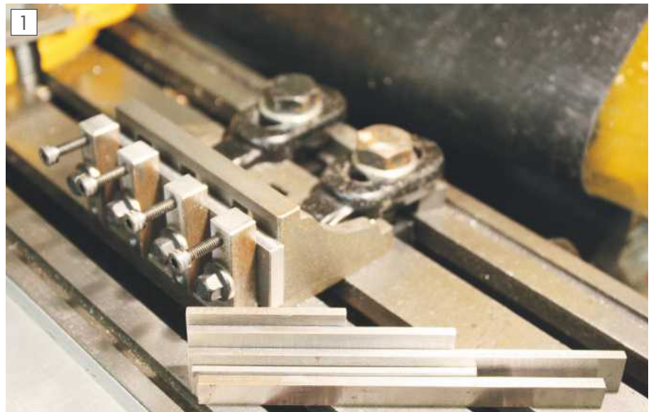
The production jig and a few finished parallels.
