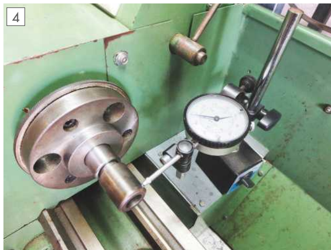
Checking runout of the arbour.
