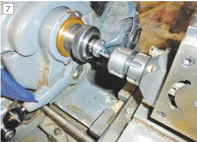
Drilling mounting holes, the small size of the backplate is apparent!
