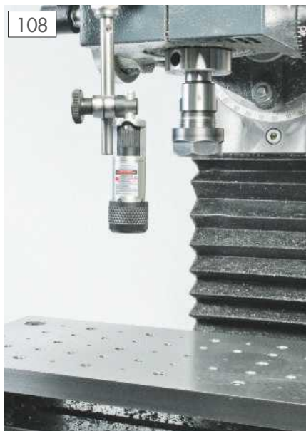
Using a laser edge-finder to help set the front edge of the sub-plate parallel to the X axis.
