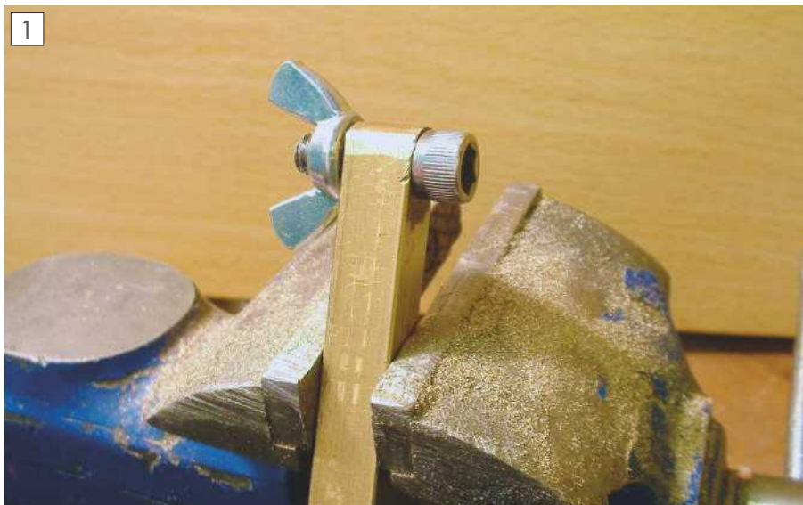
Using a cap screw as a crude filing button.
