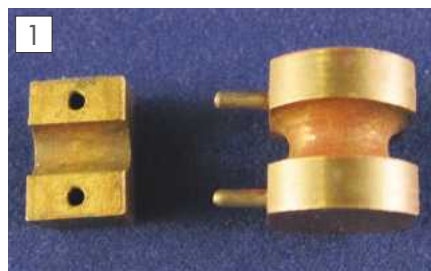
A simple former for manual bending.
