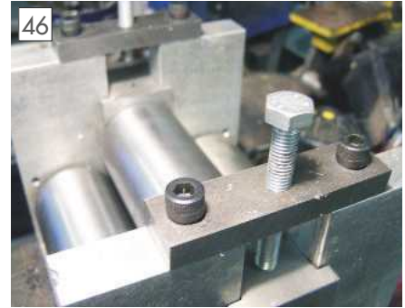
The pressure plates in position.
