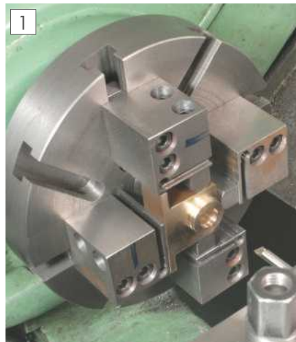
The initial machining of the bearing block with the part held in my alternative to a Four Jaw Chuck.
