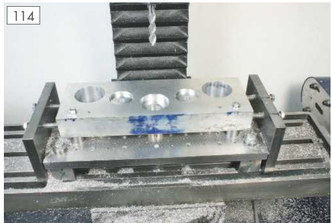
The block was clamped using bolts through holes drilled in areas of waste.
