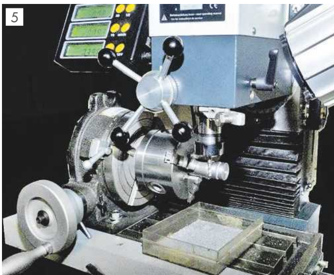
5 Milling a forming groove.
