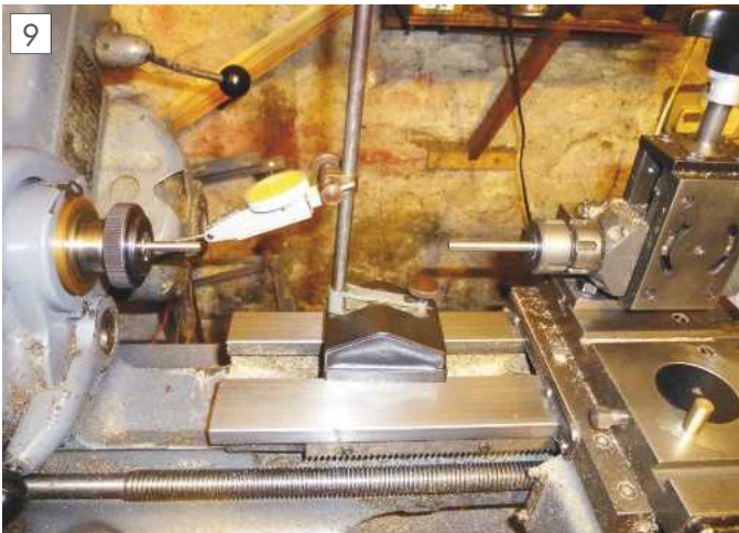
Procedure for setting the milling attachment at centre height.
