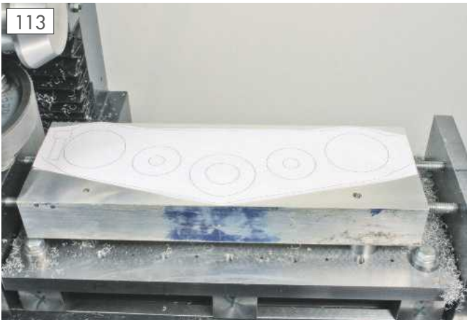
A paper template gives an approximate visual indication of the position of the main features of the work.
