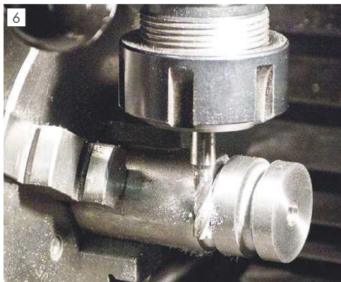
6 A closer view of groove making process.
