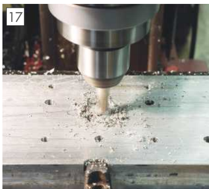
Roughing the centre port.
