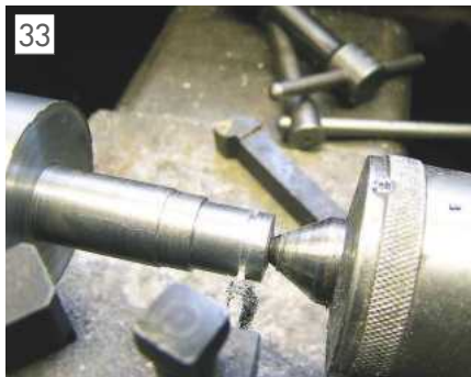
Cutting the clip grooves.
