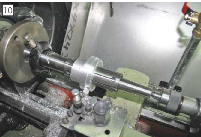
Turning a pulley on an expanding mandrel to reveal the grooves. The lower flange is formed at the same operation.
