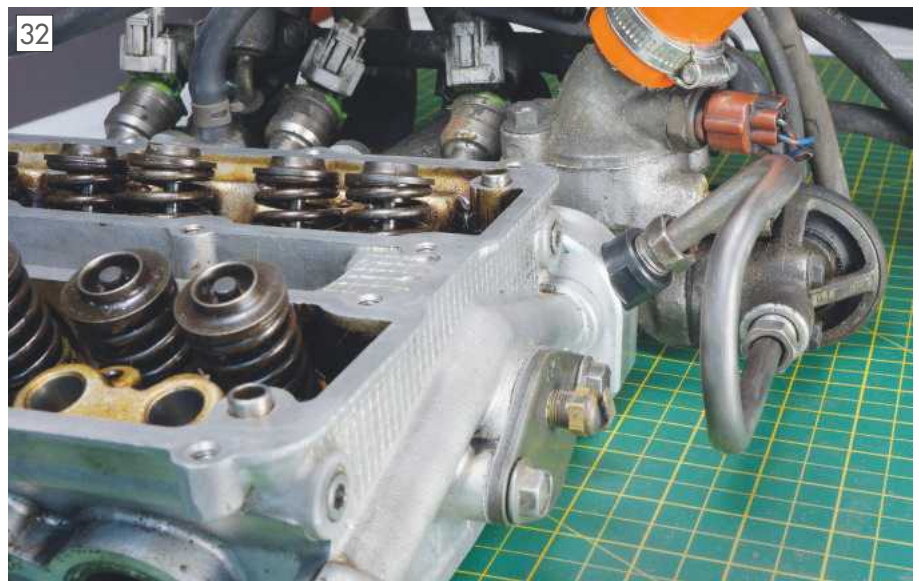
Completed EGR installation.
