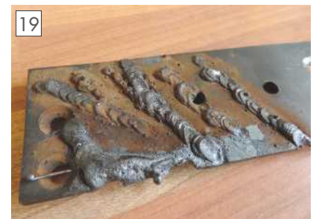
My first test piece with the MIG, note the blobby weld.
