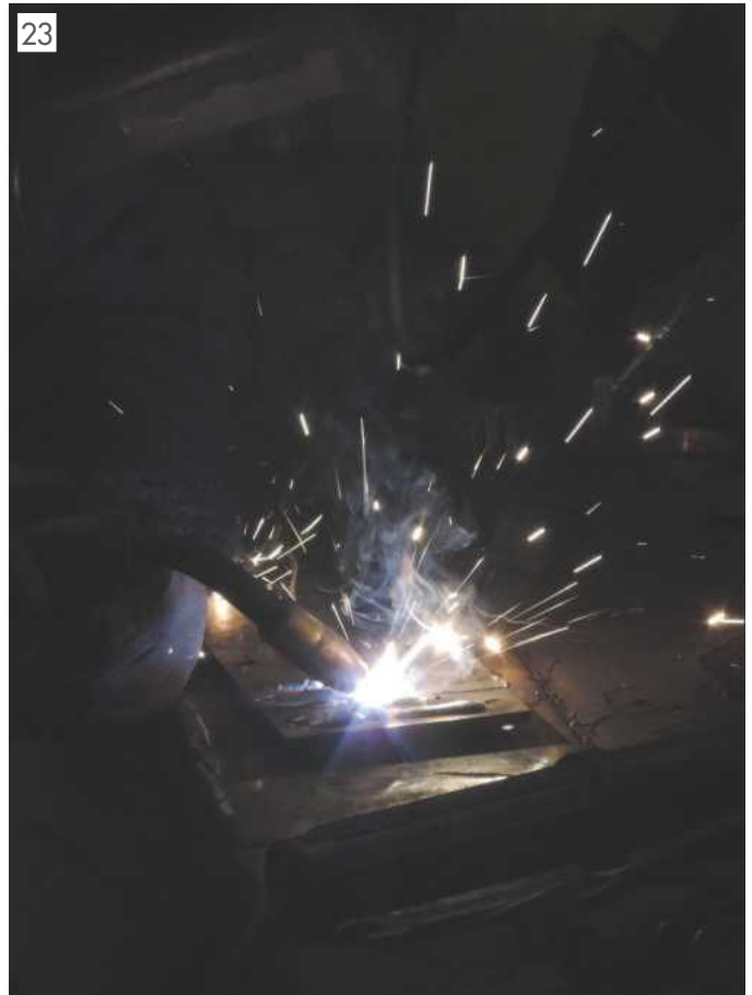
John laying down a bead with the MIG145.
