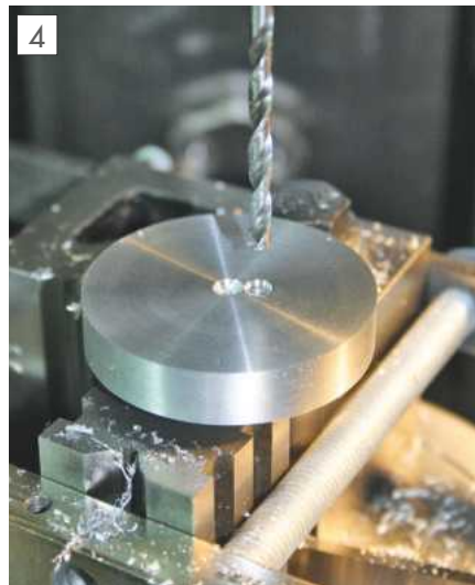
Drilling a 4mm keyway pilot hole.
