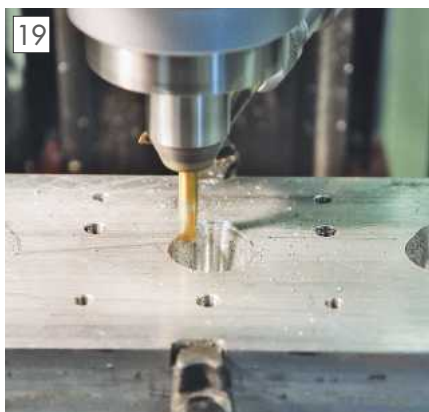
Manifold side finishing cut.
