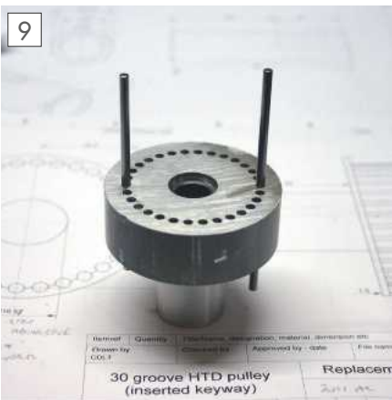
A pulley ready for final machining. The 3mm rods were for a final calliper check on the hole PCD.
