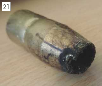
Damage to the shroud caused by slow wire feed.
