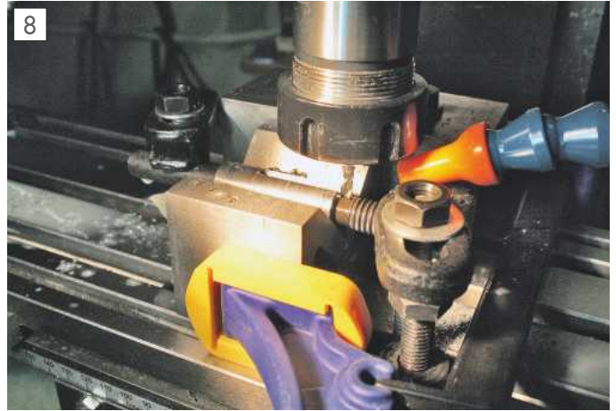
Milling the 4mm keyway in the insert. A V-block is clamped to an angle plate and the insert held down into it with a bar through the central hole.
