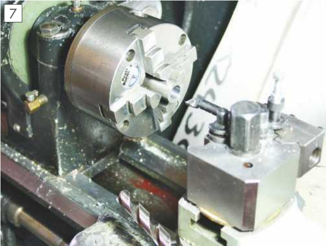
Boring a keyway insert.
