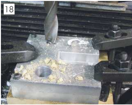
Drilling the bearing holes.
