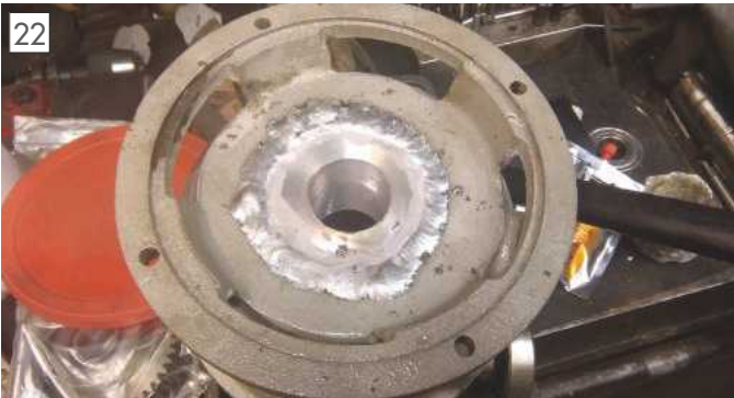
A pump housing welded up at the Bodger's Lodge (John Stevenson).
