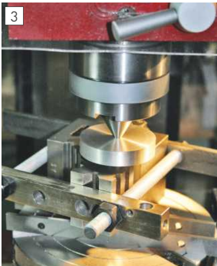
Aligning a pulley blank in the rotary table.
