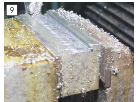
Cutting the slots in the support.
