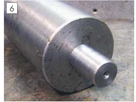
One end of the pressure roller.
