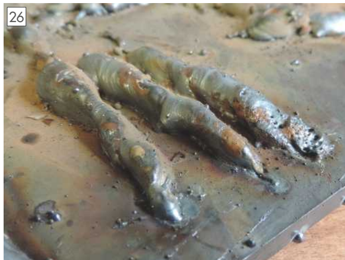
Wire feed too fast - the weld sits on top of the steel.
