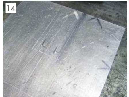
Marking out for slots and holes in the sides.
