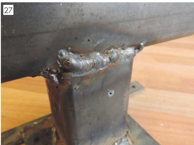
A passable weld, that would tidy up nicely with the grinder.
