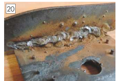
The rusty coating should have told me the gas wasn't getting through.
