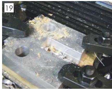
Both holes are drilled.
