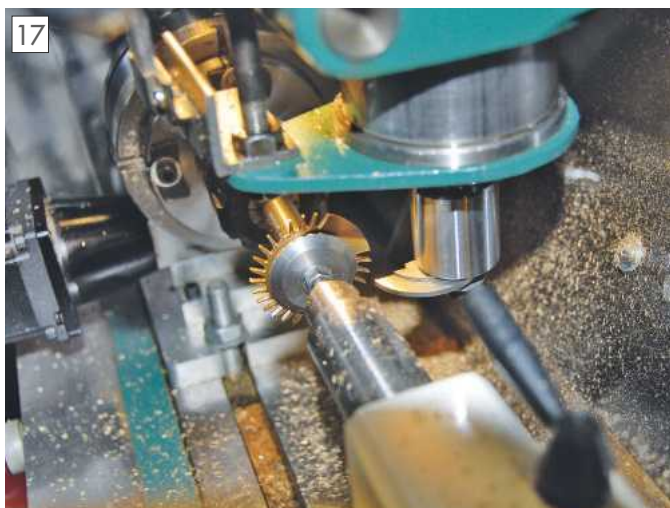
Single blade cutter cutting a escapement wheel.
