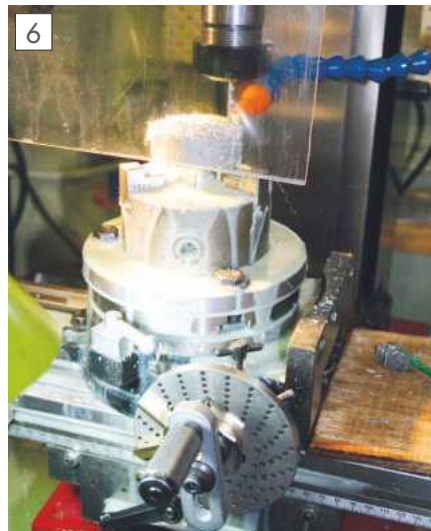
Drilling the 3mm holes.
