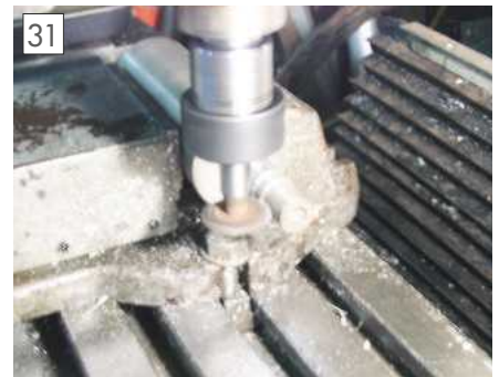
Cutting the keyway.
