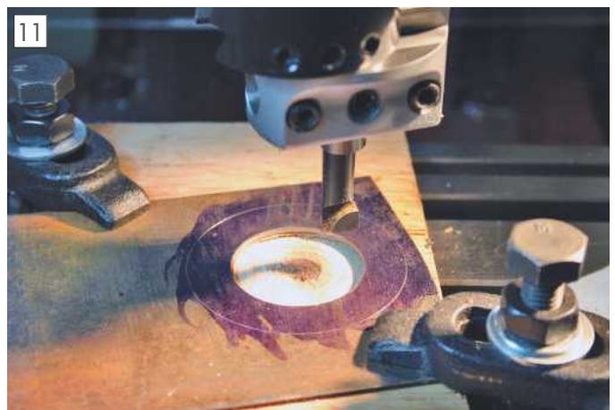
Boring a pulley upper flange.
