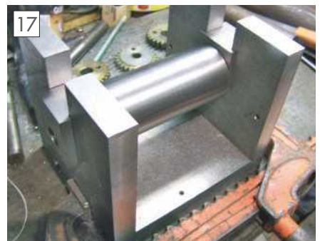
Testing for fit of the roller.
