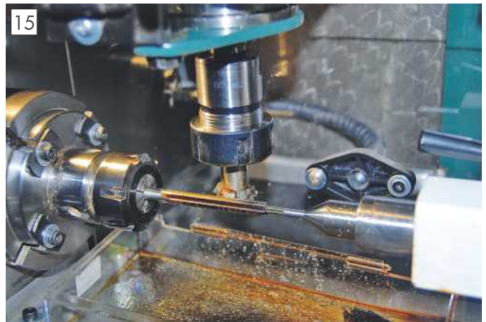
Slowly forming the pinion blank teeth.
