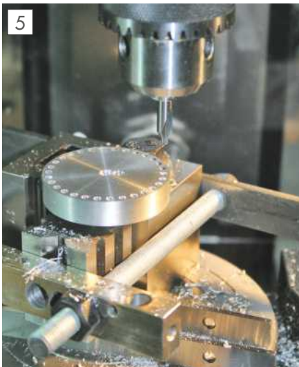
Pilot drilling on the rotary table.
