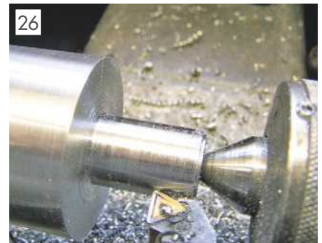
Bearing pin nearly finished.
