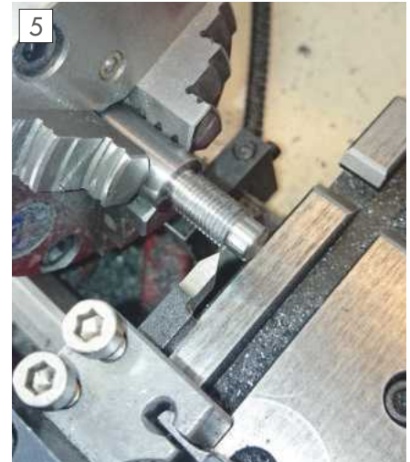
\frac{3}{8} -24UNF thread cutting.
