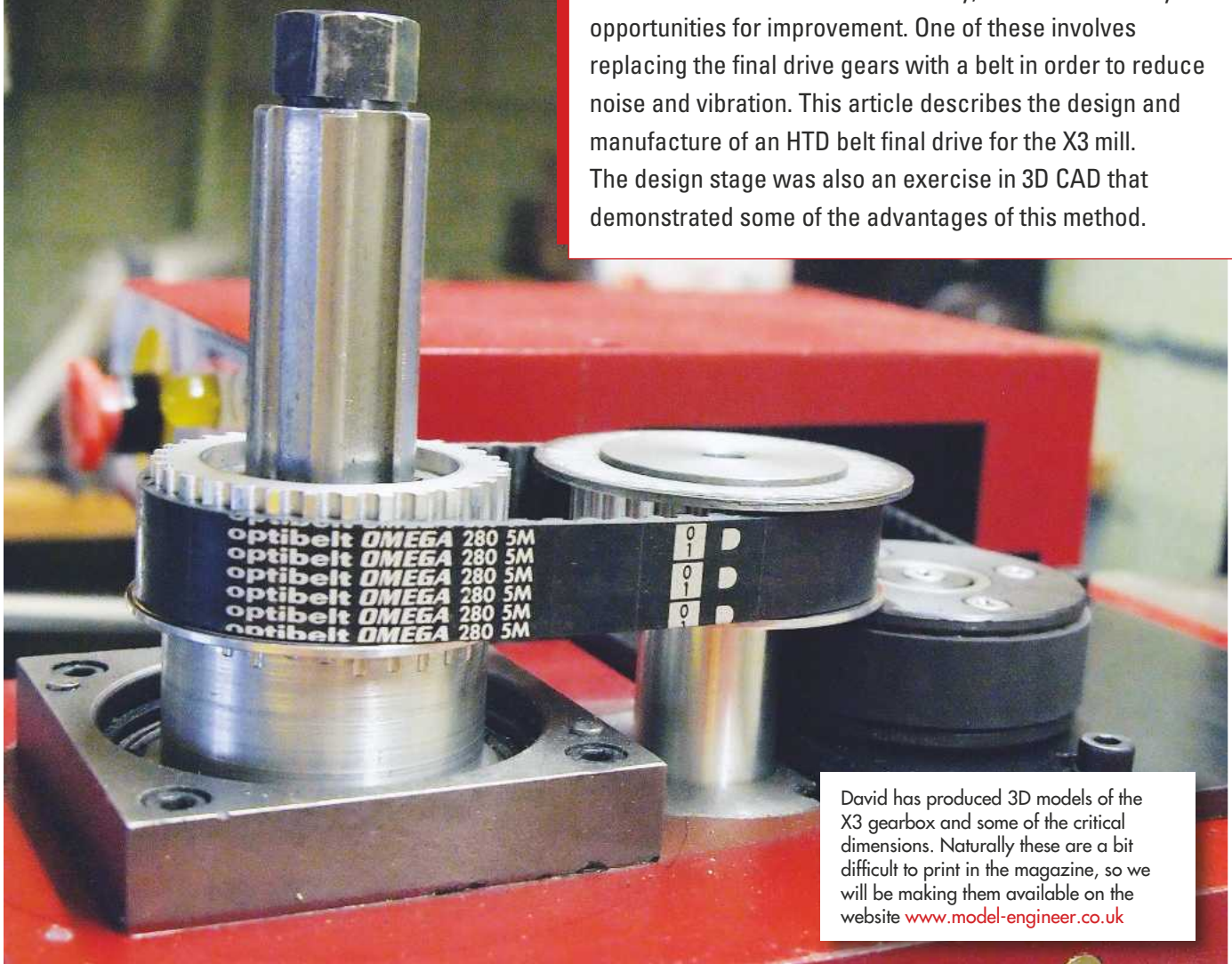
The finished HTD belt drive.
