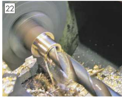
Drilling the bushes.
