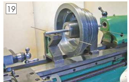
Static balance setup for static balancing of spindle pulley.
