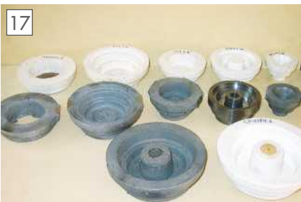
Pulley patterns and castings – one part machined.
