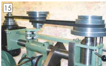
Three pulley Poly V belt drive.
