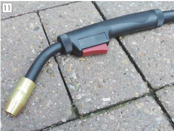
The MIG torch with its prominent shroud and trigger.
