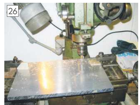
26 Machining the alloy plate.
