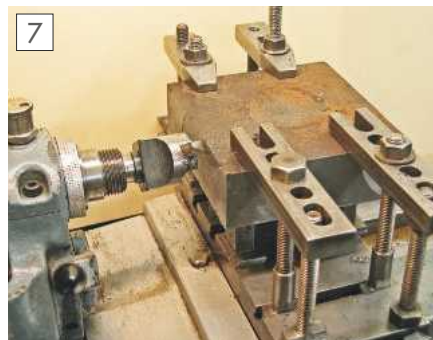
Fly cutting bracket plate mounted on the lathe.
