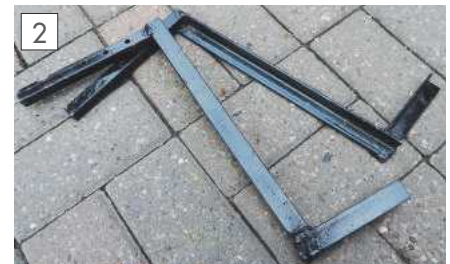
Foot rests for my driving car, welded up from mild steel and angle.
