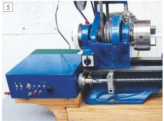
The control box.
