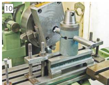
Bracket plate being bored out for the overarm on the mill.
