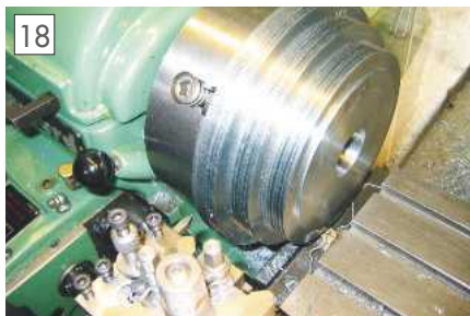
Bottom half of the spindle pulley with part turned belt grooves.
