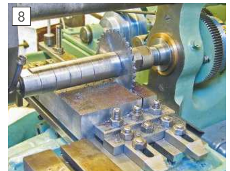
Bracket plate being milled to size on the mill.
