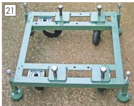
Milling trolley with castoring wheels and corner screw jacks.
