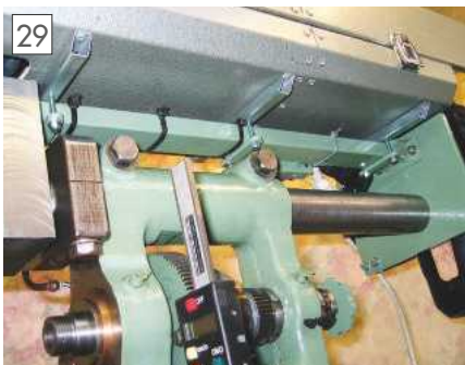
Method of fixing belt guard to a rectangular tube.
