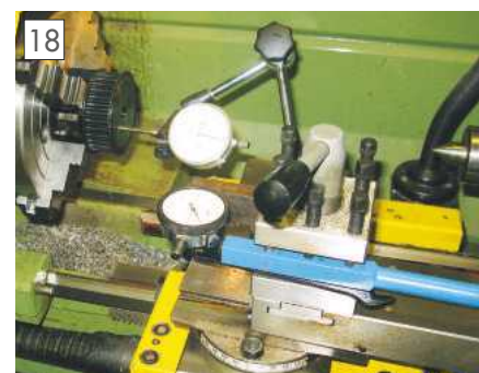
Preparing to bore the taper.
