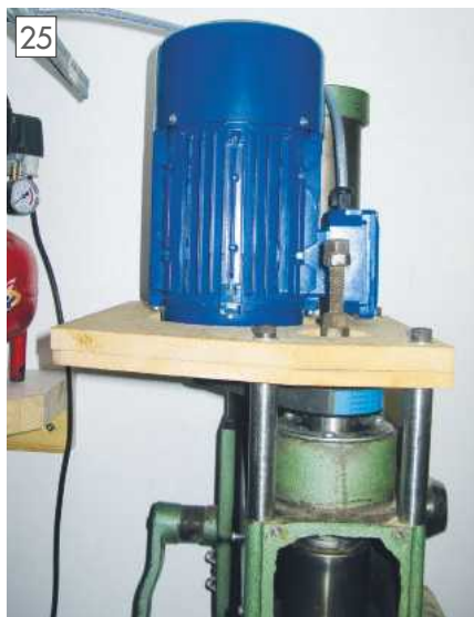
25 Motor on temporary MDF plate.
