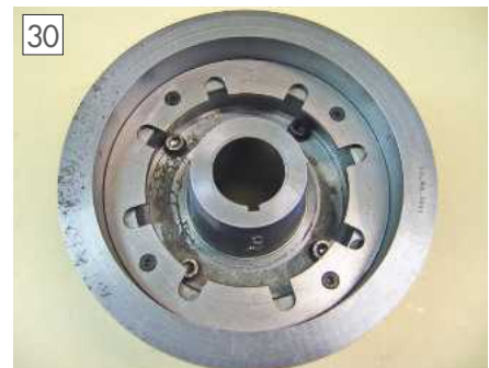
Steel locking ring on underside of spindle pulley.
