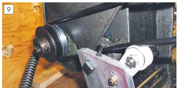
Belt tensioner installed.
