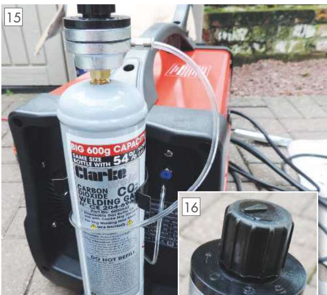
The regulator simply screws to the bottle.
