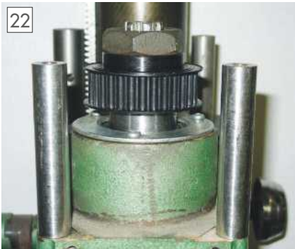
22 Fitting the pulley.
