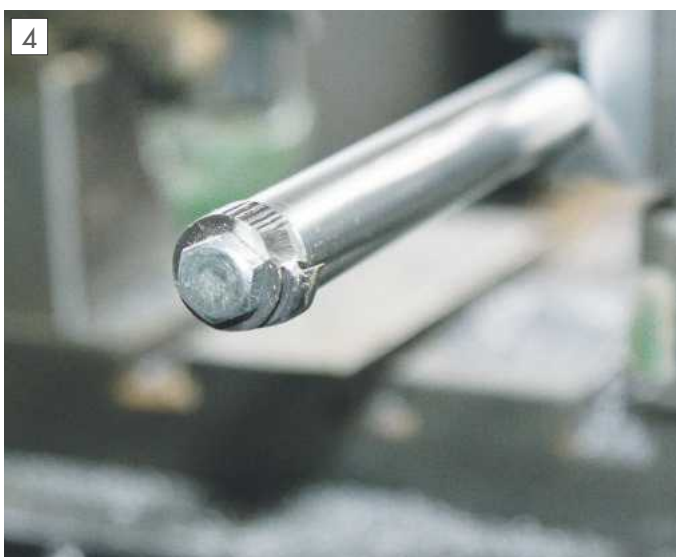
The 'snail tool' fitted to a boring bar.
