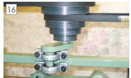
Middle pulley mounted on a swinging arm.
