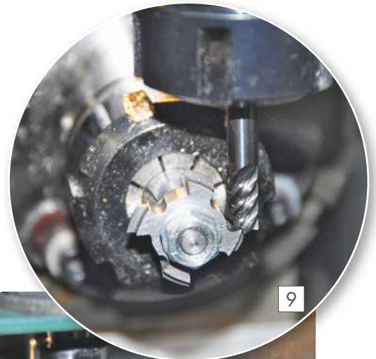
ABOVE: Machining the pinion cutter blank rake angle.
