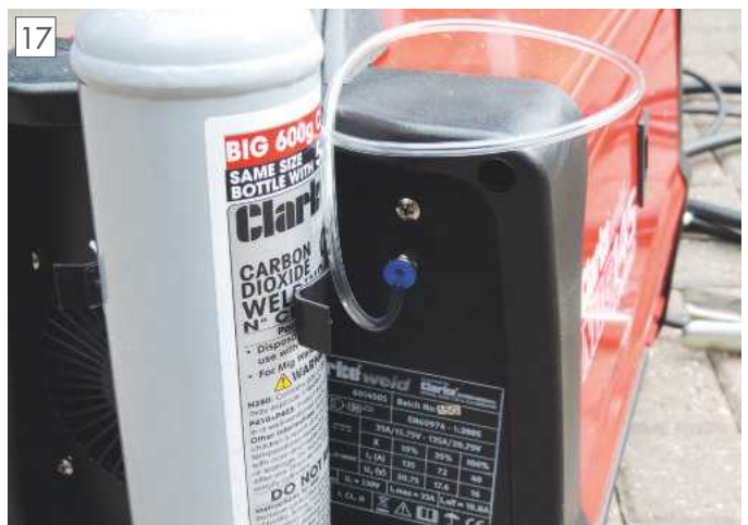
Low pressure gas is fed into the welder by this plastic tube.
