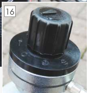
The regulator simply screws to the bottle.
