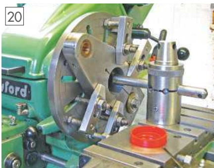
Reboring the overarm bracket for fit new overarm.
