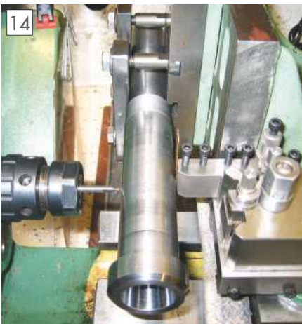
Drilling hole for collet guide pin in the spindle.
