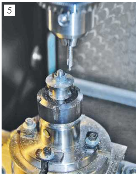
Indexing holes for the pinion cutter.
