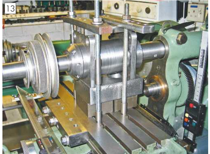
Reboring the overarm bore to 1.850" diameter.
