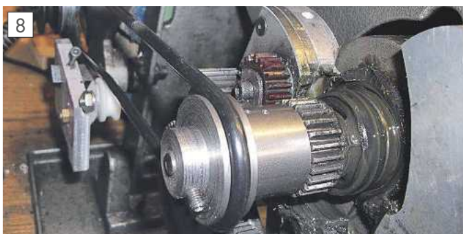
Drive belt and tensioner fitted on the lathe.
