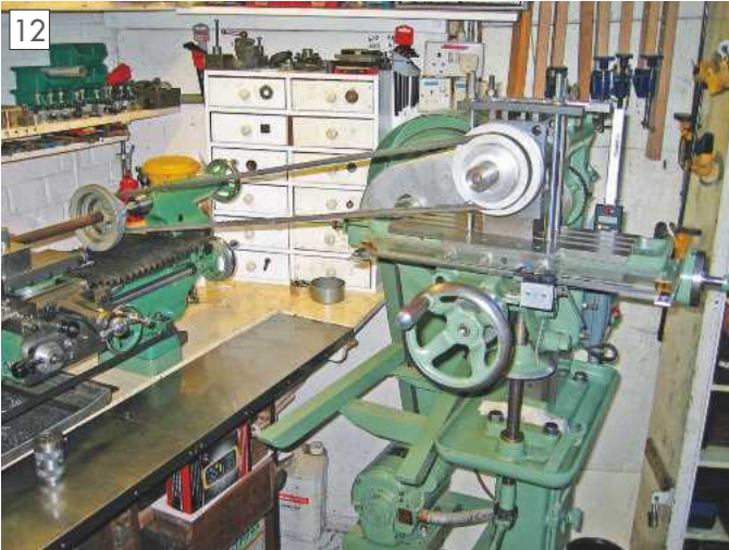
Using the lathe to drive the boring bar on the mill.
