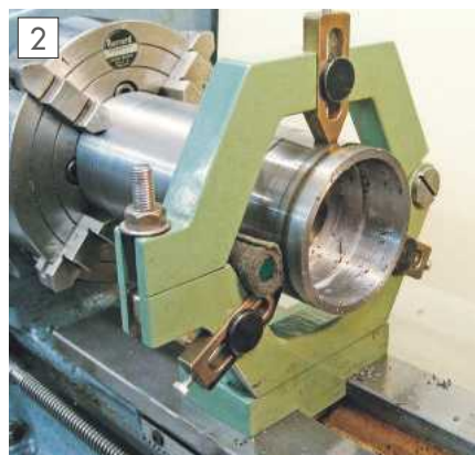
Screw adjusters added to fixed steady.
