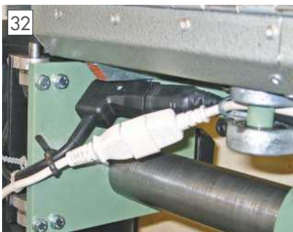
I.E.C. plugs and sockets to enable vertical head to be easily removed.
