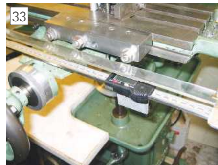
X axis DRO with Perspex swarf guard.
