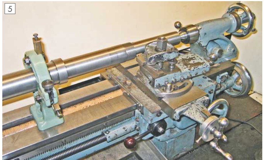
Spindle, with integral boring bar to LHS.
