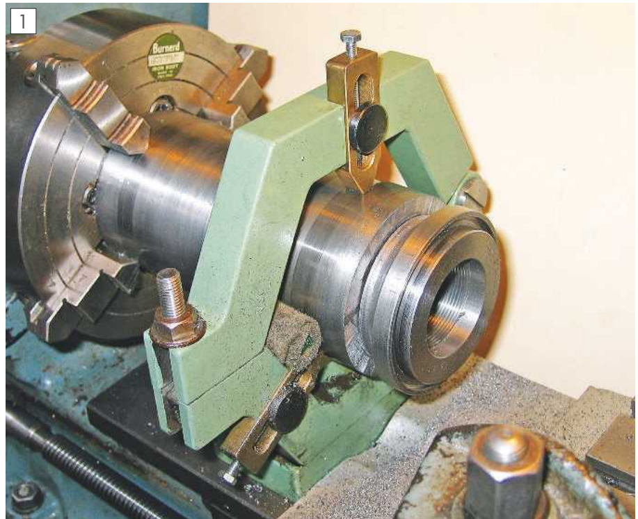
Spindle top cover being separated from spindle body.
