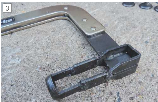
A delicate job – extension pieces for a valve spring compressor.
