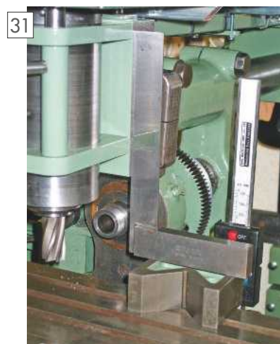
Initial setting spindle vertical with a square against the bracket plate.
