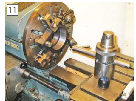
Brackets being bored to size as a pair.
