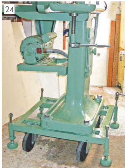
Trolley in place and mill bolted down.
