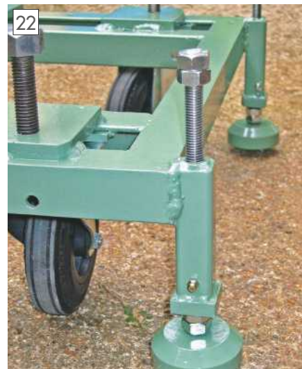
Close up of a corner jack – note greasing nipple.
