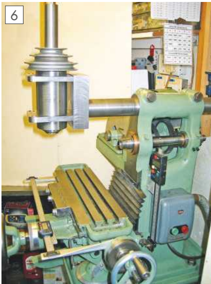
Bracket plate Loctited to new overarm, and trial fit of spindle.
