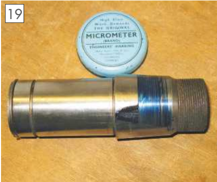
19 Checking the taper with blue.
