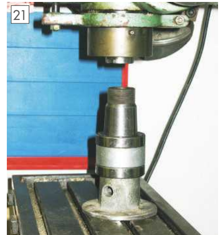
21 Pressing the bearing in place.
