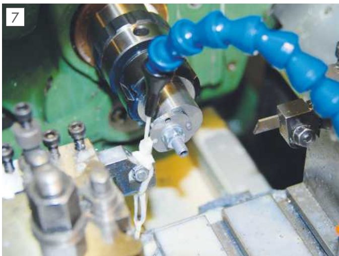
Turning the four lobes onto the pinion cutter blank.
