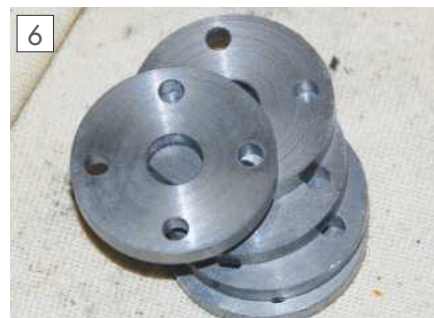
The completed indexing holes in the pinion cutter blanks.
